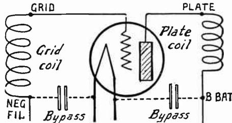
FIG. 1.—Grid Circuit and Plate Circuit Bypass Condensers.
