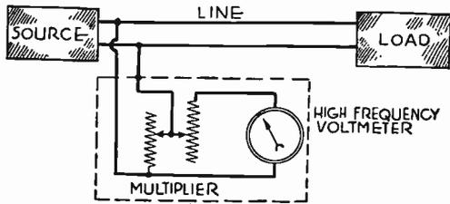
FIG. 1.—Simple Form of Volume Indicator.
