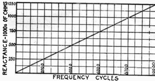
FIG. 5.—Frequency Effect on Inductive Reactance.
