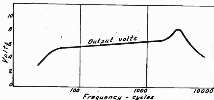
FIG. 5.—Result of Frequency Distortion in Amplifier.
