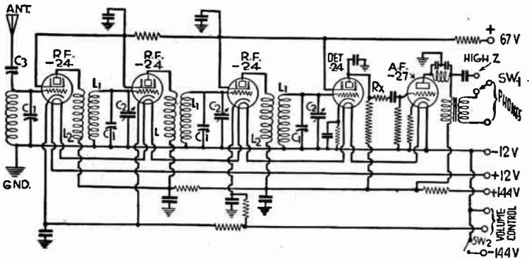
FIG. 15.—Circuits of Typical Airplane Receiver.
