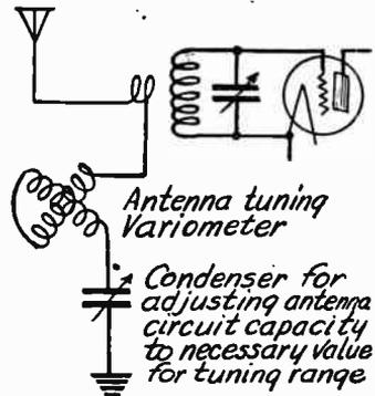
FIG. 2.—Use of Variometer for Antenna Tuning.
