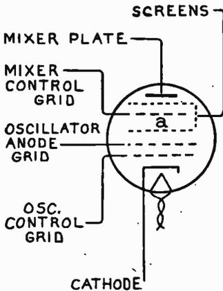
FIG. 23.—The Pentagrid Converter.
