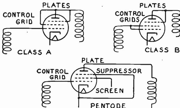
FIG. 6.—Connections for Voltage-amplifier Pentodes.
