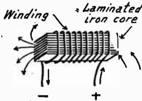
FIG. 4.—An Electromagnet with Its Field
