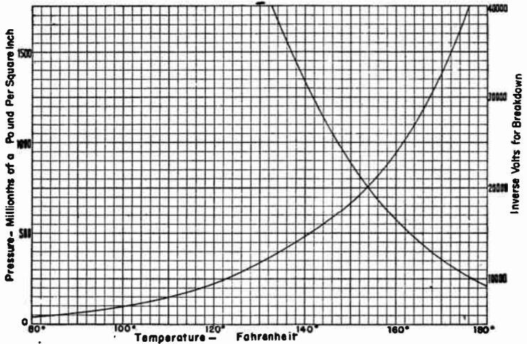
FIG. 2.—Relations between Operating Temperature of a Mercury-vapor Tube and Internal Vapor Pressure (curve starting from left), Also between Temperature and Inverse Voltage for Breakdown.
