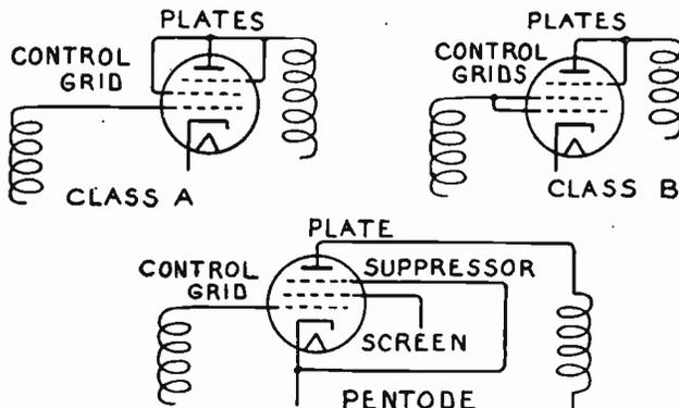
FIG. 6.—Connections for Voltage-amplifier Pentodes.
