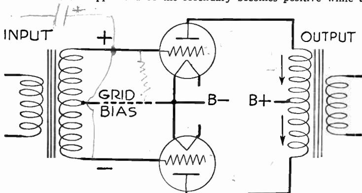
FIG. 1.—Elementary Push-pull Circuit.
