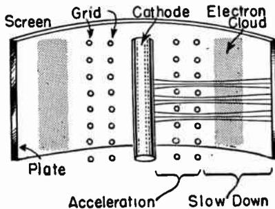
FIG. 2.—Electron Streams in the Beam Power Tube.
