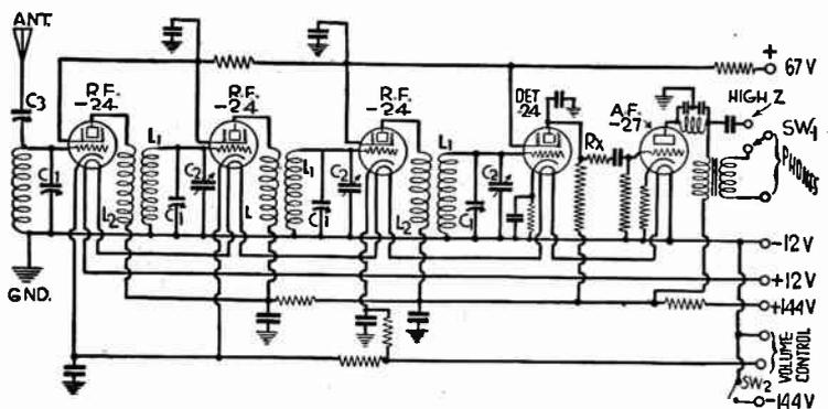
FIG. 15.—Circuits of Typical Airplane Receiver.
