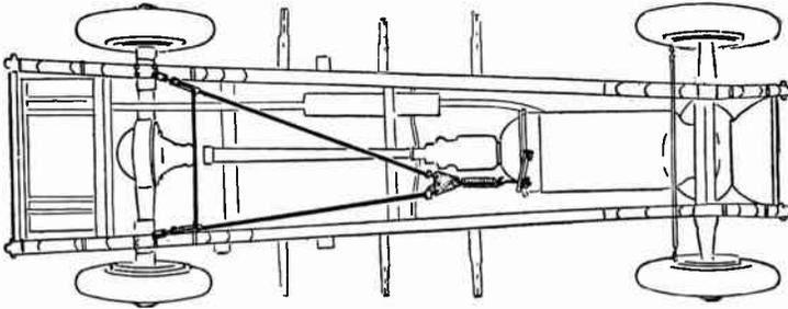
FIG. 3.—Installation of Triangular Under Chassis Automobile Antenna.
