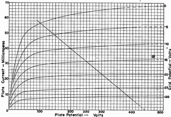
FIG. 4.—A 6,000-ohm Load Line on the Plate Characteristics.
