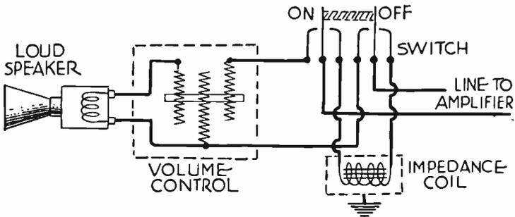
FIG. 10.—Switching and Volume Control at Loud Speaker.
