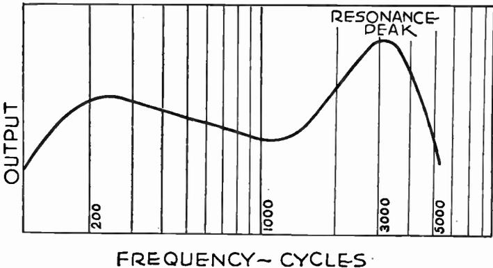
FIG. 9.—Output of Record and Pickup Working Together.
