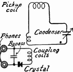
FIG. 3.—Inductively Coupled Indicator Circuit for Frequency Meter.
