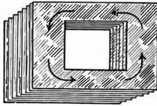
FIG. 7.—Laminated Core Construction for Audio Frequency Transformer.
