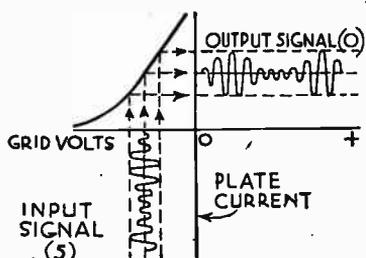
FIG. 1-A.—Class A Operating Characteristics.
