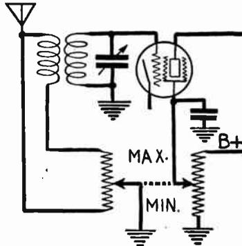
FIG. 21.—Twin Control for Antenna and Screen Voltage.
