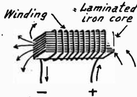
FIG. 4.—An Electromagnet with Its Field
