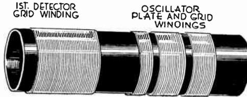
FIG. 8.—Coupling of Oscillator and First Detector Coils.
