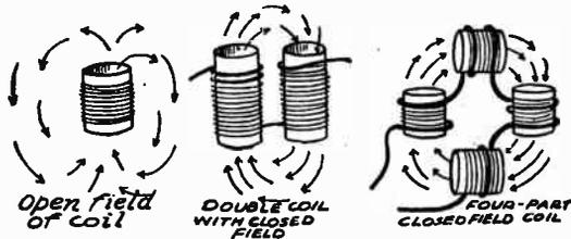
FIG. 1.—Coils with Open Fields and Closed Fields.
