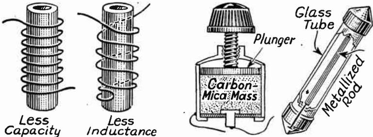
FIG. 1.—Space Winding and Non-inductive Winding of Resistors.
