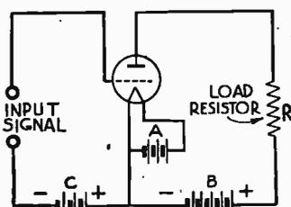
B.—Circuit Connections for Class A Operation.
