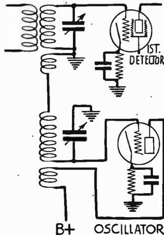
FIG. 11.—Oscillator Coupled to Detector's Tuned Grid Coil.
