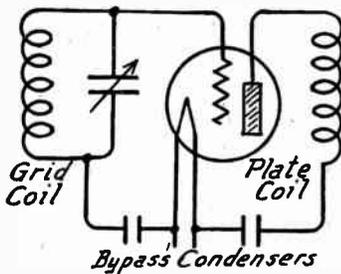
FIG. 1.—Grid and Plate Coils Entering into Regeneration.
