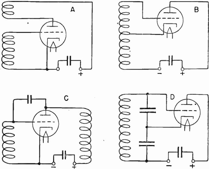
FIG. 2.—Methods of Providing Feedback.
