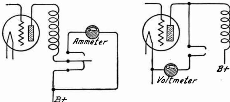
FIG. 4.—Meter Connections Made with Switches.
