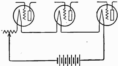
FIG. 1.—A Series Circuit.
