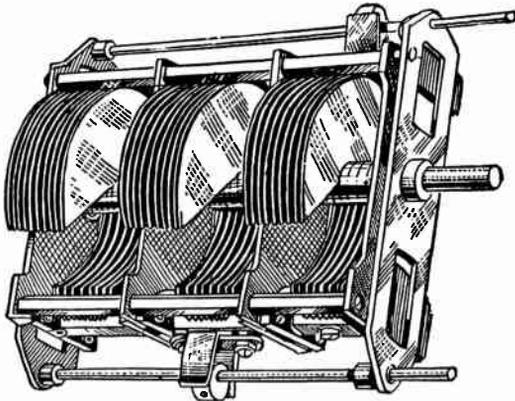
A Ganged Condenser for Tuning Three Circuits.
