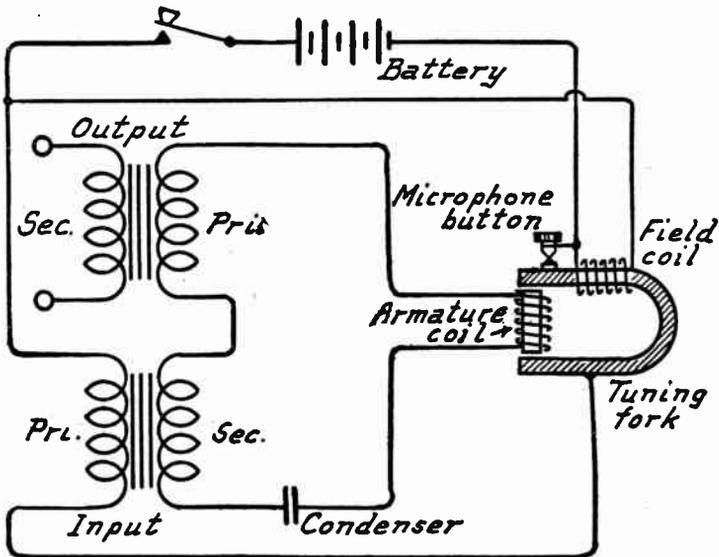
FIG. 2.—Tuning Fork Audio Oscillator.
