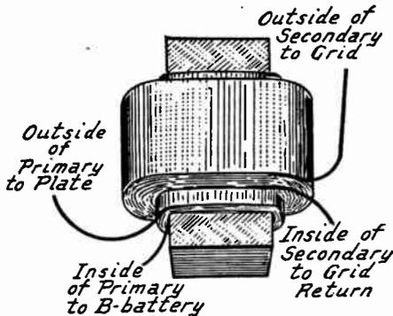
FIG. 6.—Windings and Connections of Audio Frequency Transformer.
