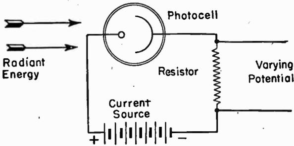
FIG. 3.—The Basic Phototube Circuit.
