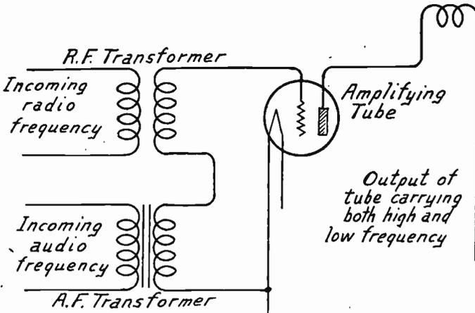
FIG. 1.—Effect of Reflexing on Amplifying Tube.
