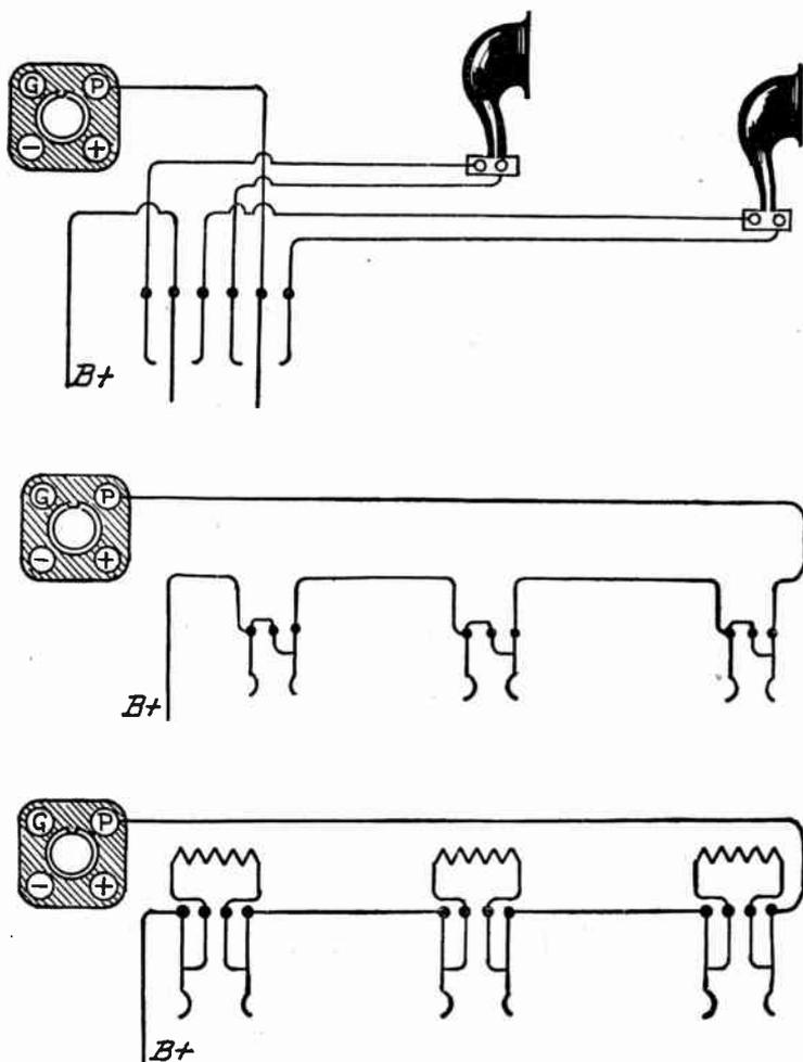
FIG. 6.—Jacks for Connection of Several Speakers.
