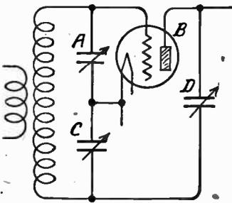
FIG. 7.—The Isofarad Method of Balancing.
