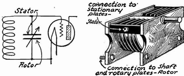
FIG. 4.—Connections to Rotor and Stator of Condenser.
