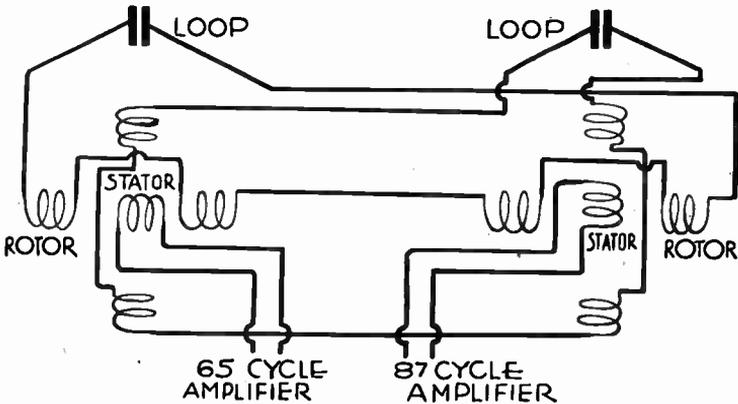
FIG. 11.—Circuit for Beacon Loops.
