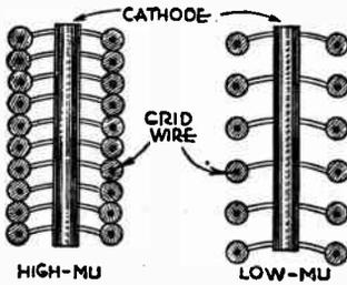
FIG. 1.—Control Grid Spacing and Extent of Fields.
