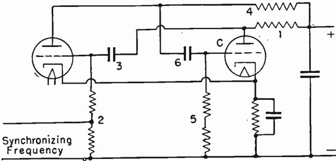
FIG. 3.—Circuit of Multivibrator Oscillator..
