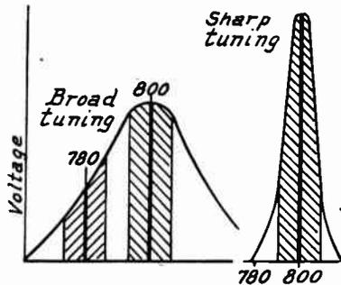
FIG. 2.—Response of Resonant Circuits
