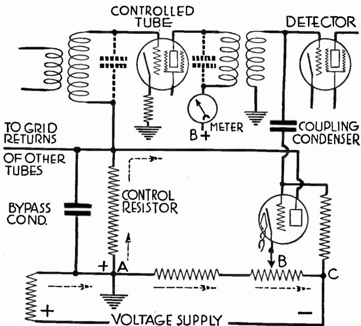
FIG. 22.—Automatic Volume Control by Grid Bias Variation.
