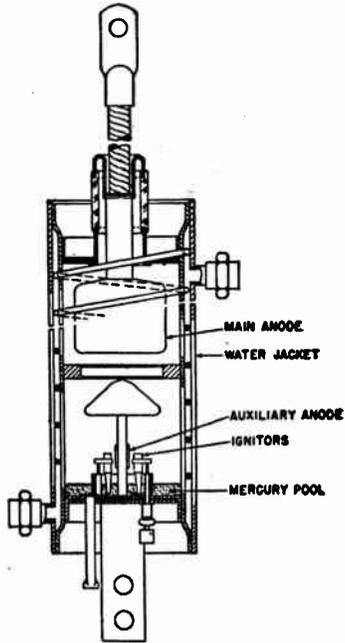
FIG. 3.—A General Electric Sealed Ignitron Having Two Ignitrons and an Auxiliary Anode.
