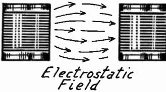
FIG. 5.—Capacity Effect between Coils Which Causes Oscillation.
