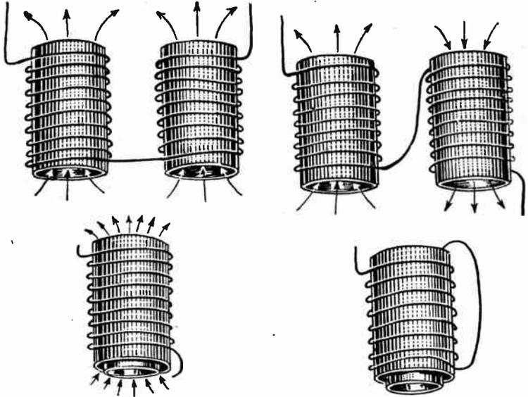
FIG. 3.—Coils Working Together to Add Their Inductances as in a Variometer.
