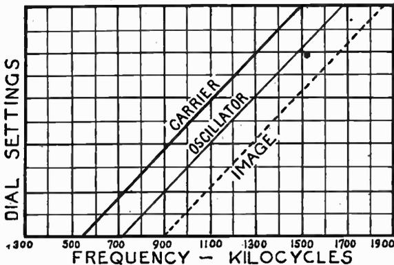
Fig. 17.—Relations Between Image, Oscillator and Carrier Frequencies.
