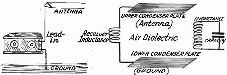
FIG. 2.—The Principle of the Capacity Antenna.
