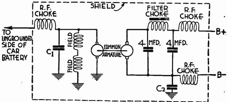
FIG. 6.—Circuit Diagram of Dynamotor Type Automobile "B" Supply.
