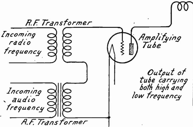
FIG. 1.—Effect of Reflexing on Amplifying Tube.
