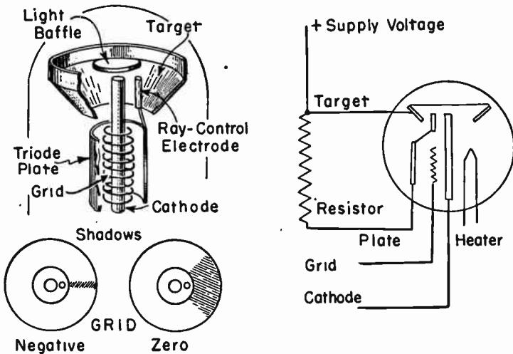
FIG. 2.—Tube and Circuit for Single Control Electrode.
