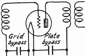
FIG. 3.—Bypass Condensers for Reducing Feedback Couplings and Oscillation.
