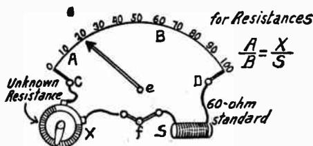
FIG. 6.—Resistance Measurement with Bridge.
