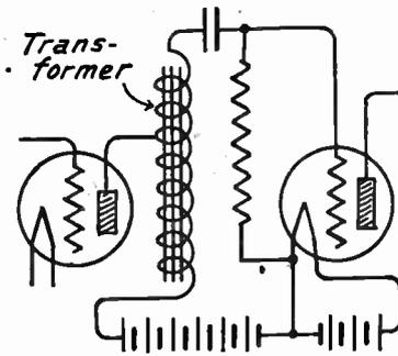
FIG. 3.—Auto-Transformer Interstage Coupling.
