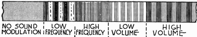
FIG. 6.—Changes in Variable Density Sound Track.
