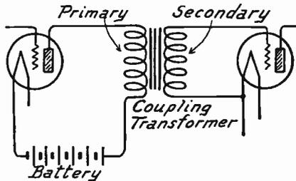
FIG. 1.—Connection of Audio Frequency Transformer Between Tubes.
