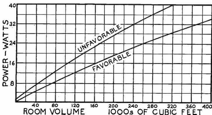
FIG. 12.—Power Requirements According to Room Volume.
