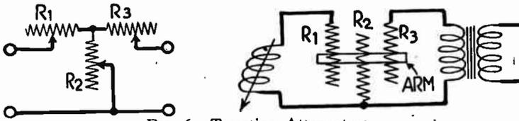
FIG. 6.—T-section Attenuators.
