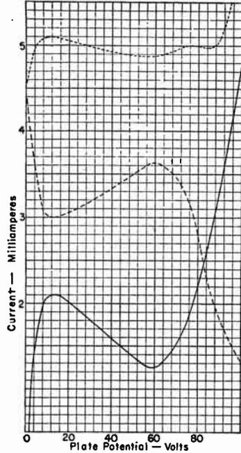
FIG. 7.—Relations of Currents and Potential with Dynatron.
