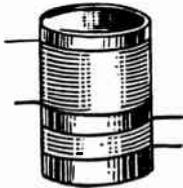
FIG. 5.—Air Core Radio Frequency Transformer.
