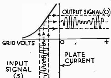
FIG. 1-A.—Class A Operating Characteristics.
