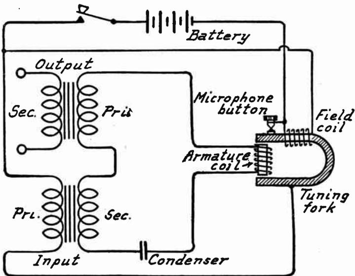
FIG. 2.—Tuning Fork Audio Oscillator.
