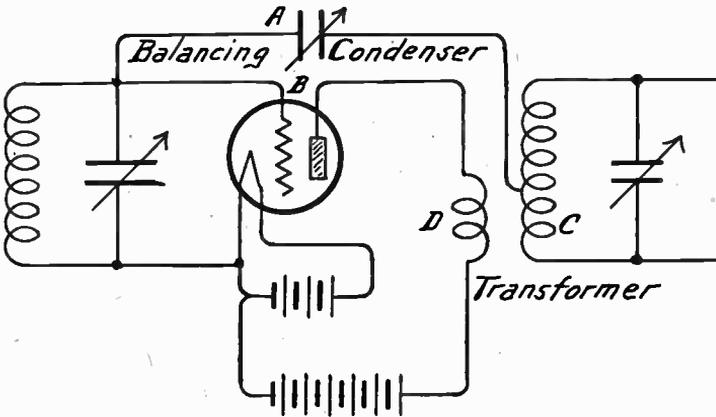
FIG. 2.—Neutrodyne Method of Balancing.
