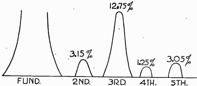
FIG. 6.—Harmonics with Push-pull Amplification.
