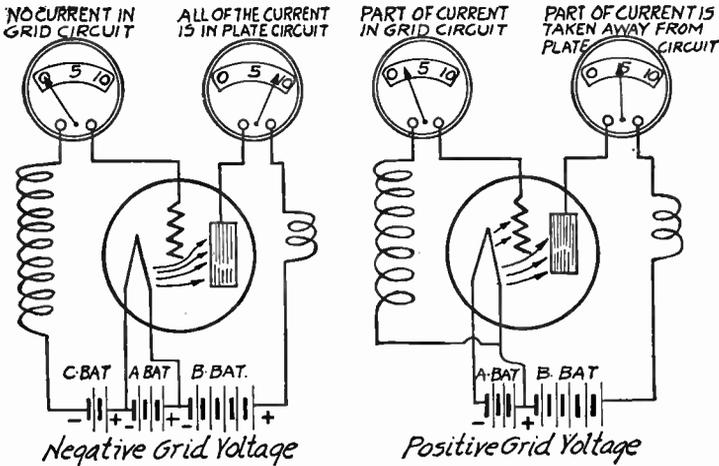
FIG. 4.—Electron Flow with Negative Grid Bias Voltage.
