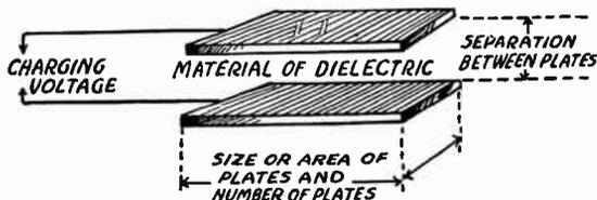
FIG. 4.—The Four Factors Affecting a Condenser's Charge.
