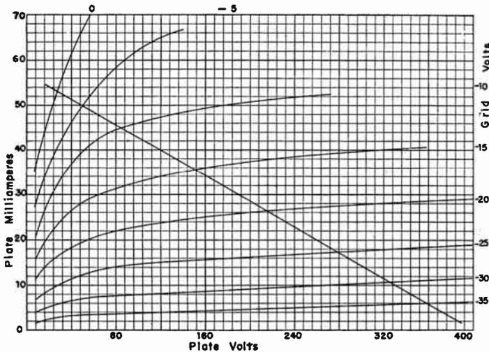
FIG. 5.—Plate Characteristics of a Power-amplifier Pentode.
