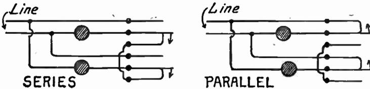
FIG. 7.—Switch for Series or Parallel Connection.
