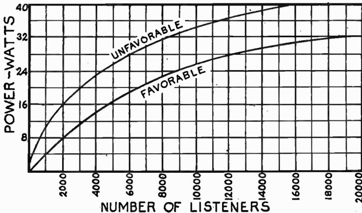
FIG. 11.—Power Requirements According to Number of Listeners.
