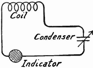
FIG. 1.—The Simplest Frequency Meter Circuit.
