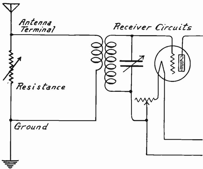
FIG. 1.—Using Resistance to Reduce Effect of Interference.
