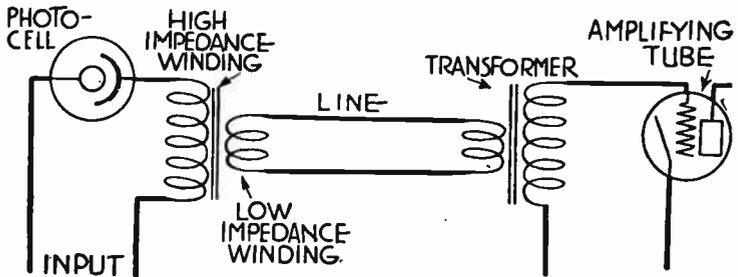
FIG. 13.—Use of Low Impedance Line in Photocell Amplifier.
