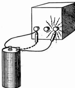
FIG. 14.—Test for Open Circuit or Short in Transformer or Choke.
