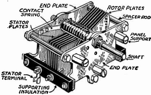
FIG. 1.—The Parts Considered in Design of a Typical Variable Condenser.
