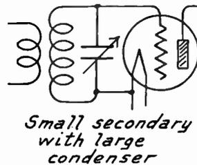
FIG. 5.—Small Secondary Reducing Voltage and Increasing Stability.
