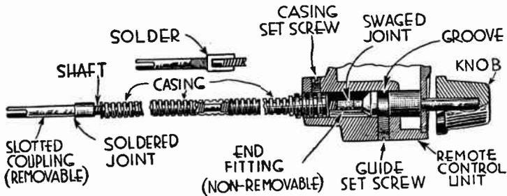
FIG. 5.—Construction at "Dental Cable" Flexible Control Shaft.
