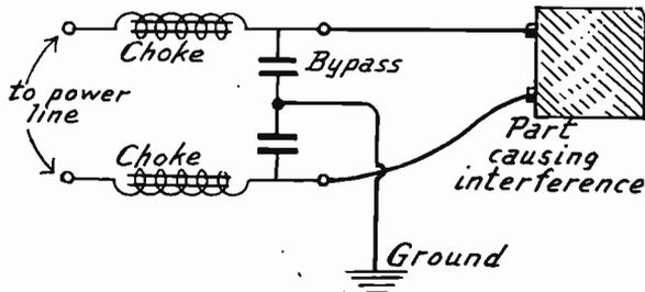
FIG. 8.—Interference Filter with Grounded Center Tap.
