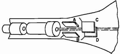
FIG. 3.—Electrostatic Deflection of the Beam.
