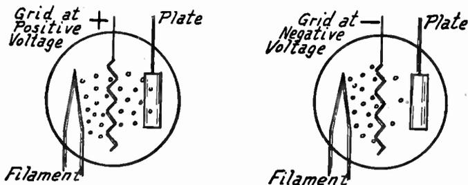
FIG. 3.—Effect of Positive and Negative Grid on Electron Flow.
