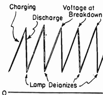
FIG. 5.—Output Wave Form of Neon Oscillator.
