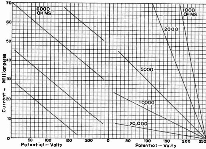
FIG. 2.—Load Lines for 6,000 Ohms Resistance.
