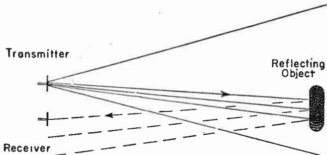
FIG. 3.—The Angle of Reflected Waves Indicates Direction.
