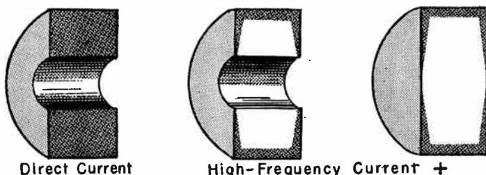
FIG. 3.—High-frequency Currents Are Induced Chiefly in the Skin or Outer Part of Heated Metals.
