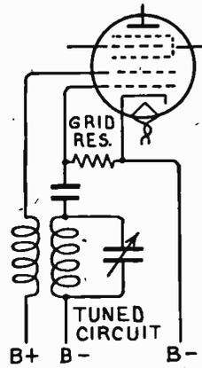
FIG. 24.—Pentagrid Oscillator Circuit.
