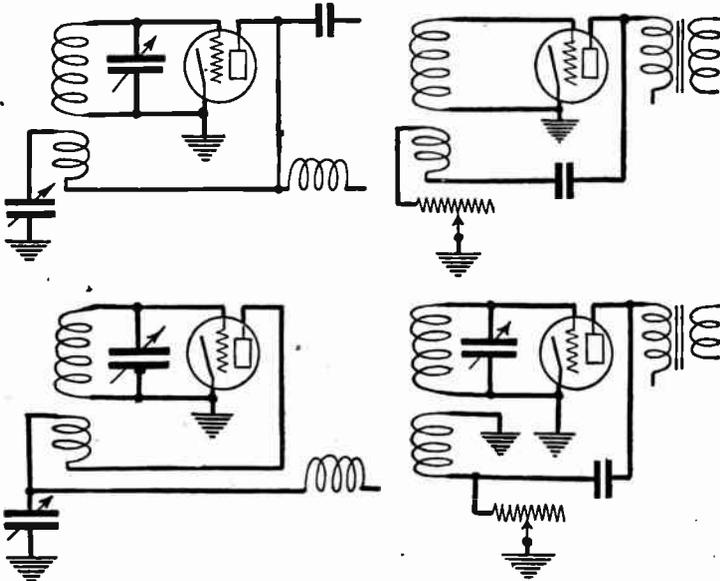
FIG. 5.—Regeneration Control Devices Having One Side Grounded
