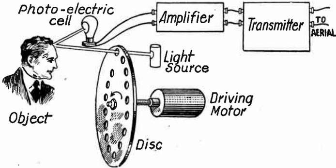
FIG. 1.—Nipkow Disc Scanning at Televisor or Transmitter.
