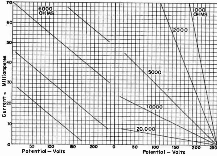
FIG. 2.—Load Lines for 6,000 Ohms Resistance.
