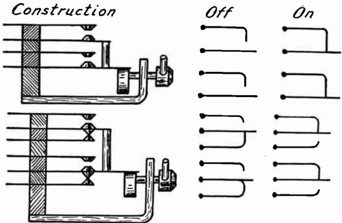
FIG. 2.—Operation of a Jack Switch.
