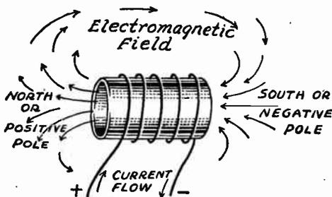
FIG. 2.—Electromagnetic Field around a Solenoid or Coil.
