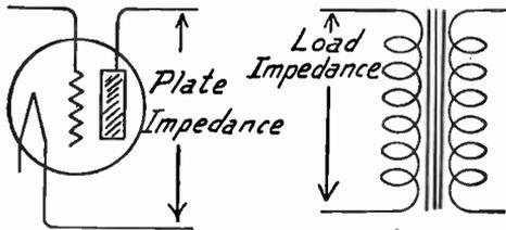
FIG. 1.—Impedances of Plate Circuit and of Load.
