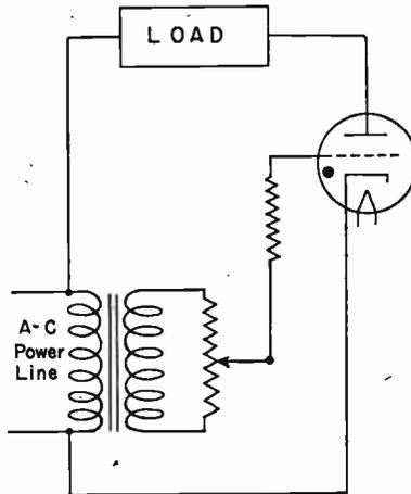
FIG. 4.—Method of Varying the Amplitude of Control Voltage Applied to the Grid.
