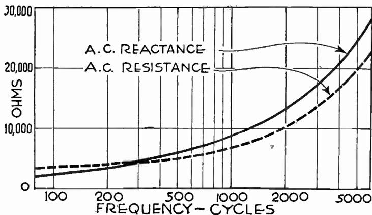
FIG. 8.—Effect of Frequency on Impedance of Pickup.
