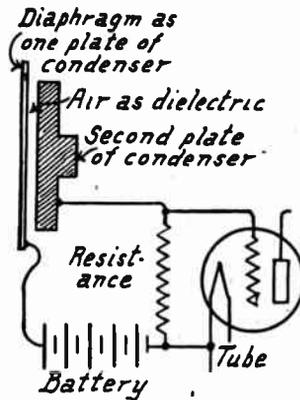
FIG. 3.—Condenser Microphone.
