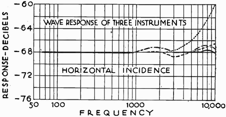
FIG. 2.—Response Curves of Several Multi-cell Crystal Microphones.
