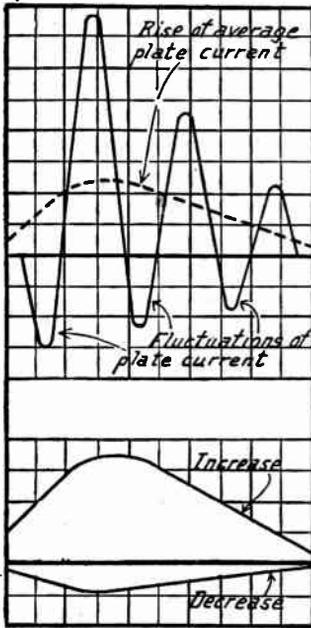
FIG. 2.—Current Change During Plate Current Detection.
