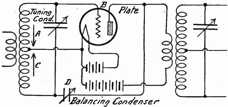
FIG. 4.—Rice Method of Balancing.
