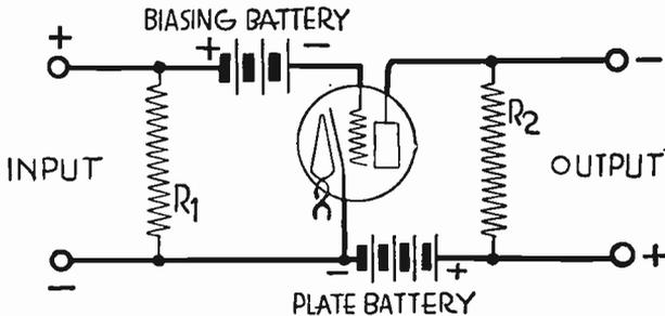
FIG. 1.—Simple Form of Direct Current Amplifier.
