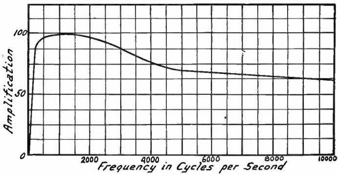
FIG. 5.—Curve for Poor Audio Transformer Drawn on Arithmetic Scale.
