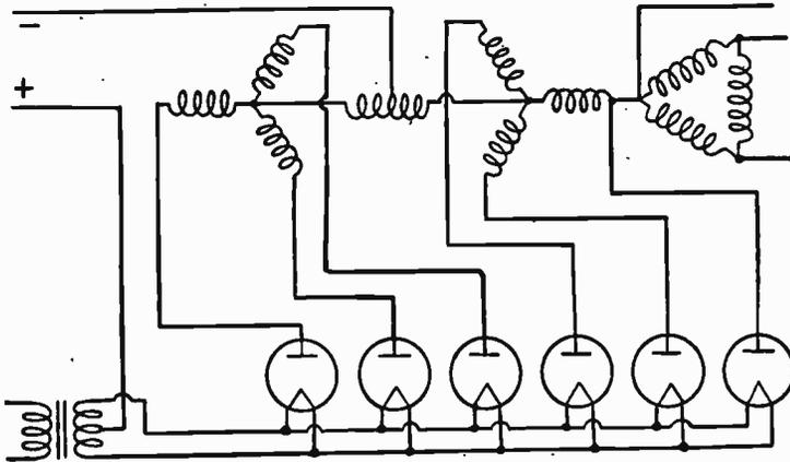
FIG. 3.—Three-phase Double-Y Parallel Rectifier.
