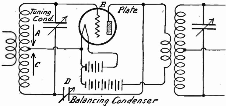
FIG. 4.—Rice Method of Balancing.
