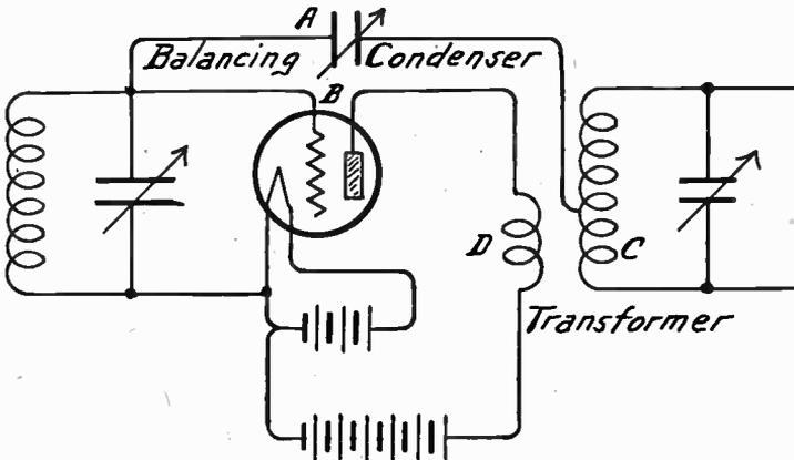
FIG. 2.—Neutrodyne Method of Balancing.
