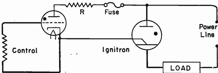
FIG. 2.—Thyatron Used for Control of an Ignitron.
