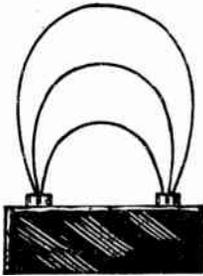
FIG. 1.—Circuits with Resistances in Parallel on Battery.
