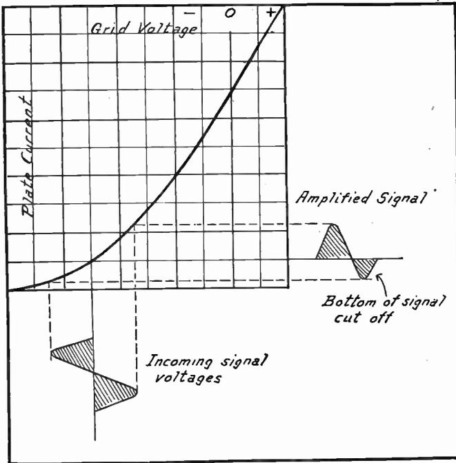
FIG. 3.—Distortion Caused by Excessive Negative Grid Bias.
