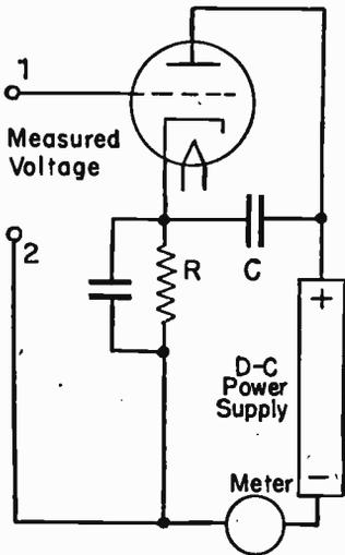
FIG. 1.—Plate Current Detector Used as VT Voltmeter.
