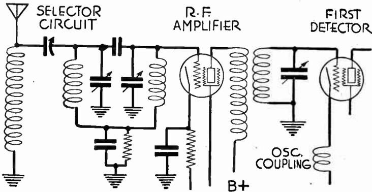
FIG. 13.—Band Selector Type of Pre-amplifier for Superheterodyne.
