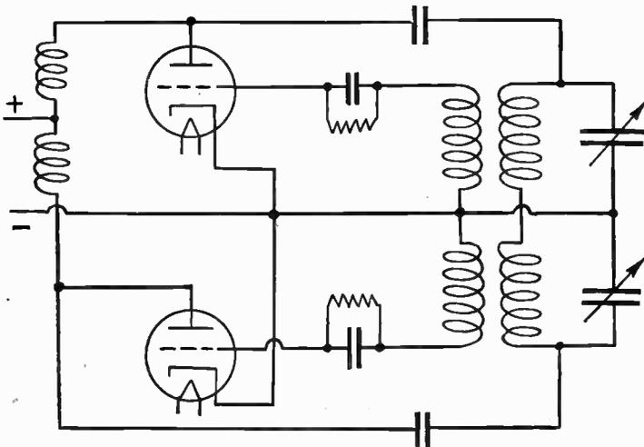
FIG. 12.—Two Oscillator Tubes with Single Resonant Circuit.
