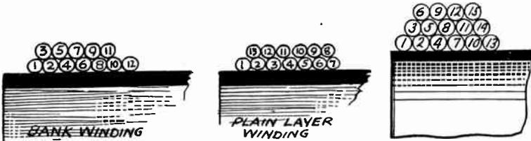
Placing of Turns in Bank and Layer Windings.
