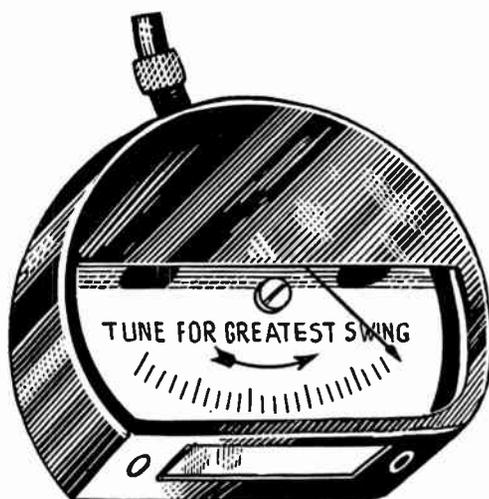
FIG. 11.—Reversed Scale Meter Tuning Indicator
