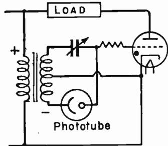
FIG. 11.—Phase-shift Control by Means of Varying Resistance of a Phototube.
