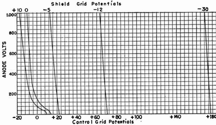
FIG. 3.—Control Grid Breakdown Potentials of Four-element Thyatron.
