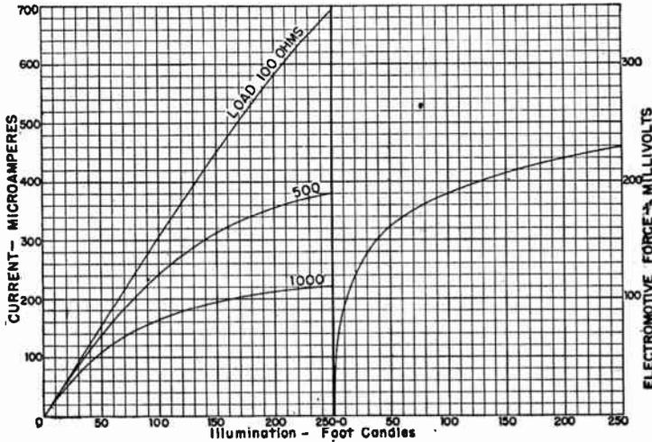
FIG. 2.—Current and Emf in Barrier Layer Photocells.
