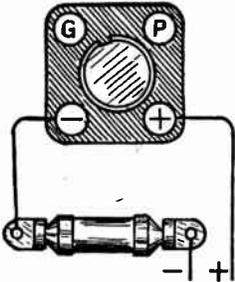
FIG. 1.—Filament Resistor.
