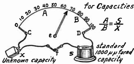
FIG. 8.—Capacity Measurement with Bridge.
