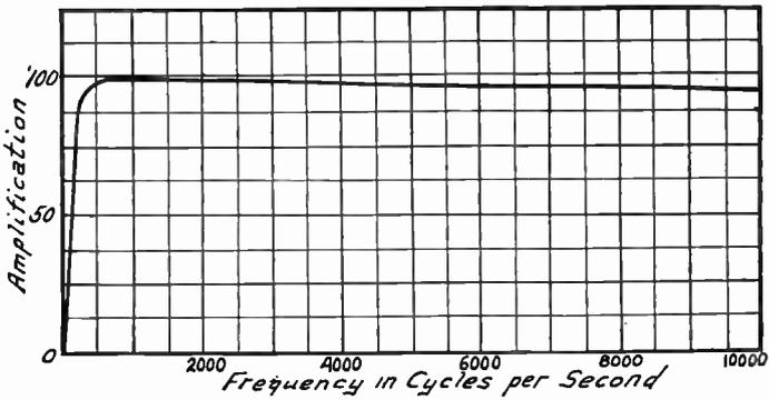
FIG. 4.—Curve for Good Audio Transformer Drawn on Arithmetic Scale
