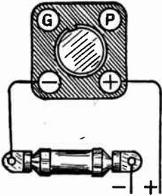
FIG. 1.—Filament Resistor.
