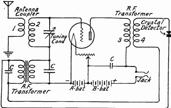
FIG. 3.—Single Tube Reflex Receiver with Crystal Detector.
