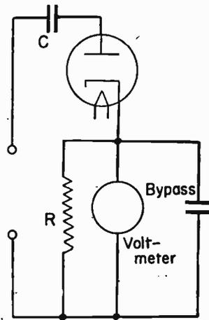
FIG. 6.—Diode Used for a VT Voltmeter.
