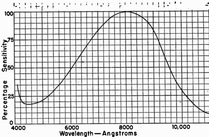
FIG. 4.—Wavelength Sensitivity of One Type of Phototube.
