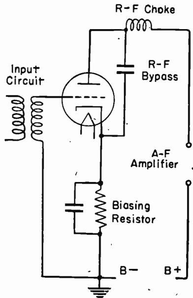
FIG. 3.—Typical Circuit for a Plate Current Detector.
