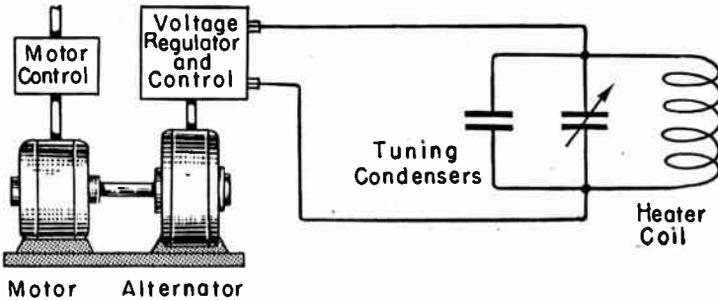
FIG. 4.—Medium Frequencies for Induction Heating Are Produced by Rotating Machines.
