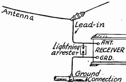
FIG. 1.—Connection of Lightning Arrester to Antenna and Ground.
