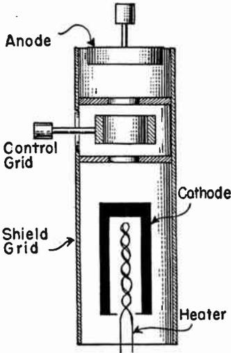
FIG. 1.—Element Arrangement in Heavy-duty Four-element Thyatron.
