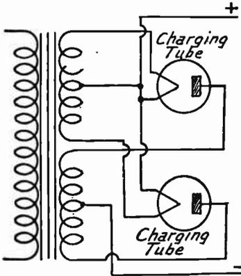
FIG. 3.—Charging Tubes Used as Filament Supply Rectifier.
