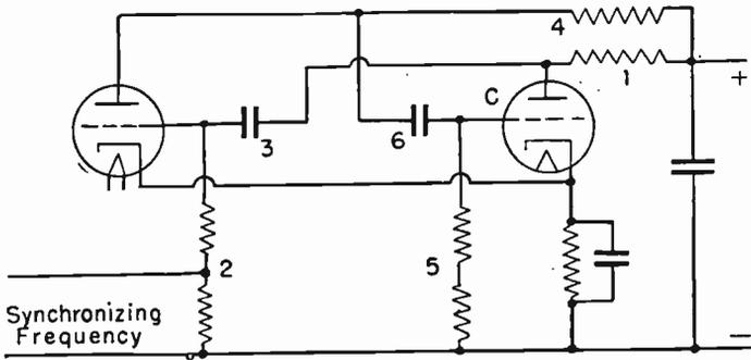
FIG. 3.—Circuit of Multivibrator Oscillator..
