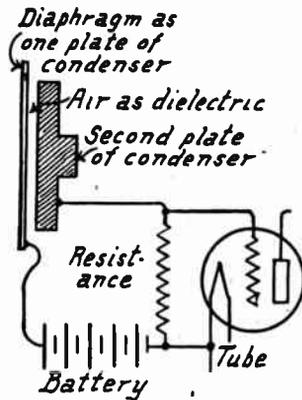
FIG. 3.—Condenser Microphone.
