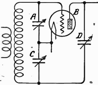
FIG. 7.—The Isofarad Method of Balancing.
