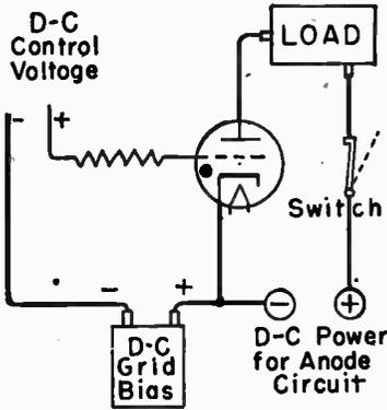
FIG. 3.—D-c Control of D-c Power for Load.
