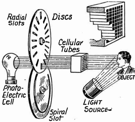
FIG. 3.—Action of Baird Discs in Television.
