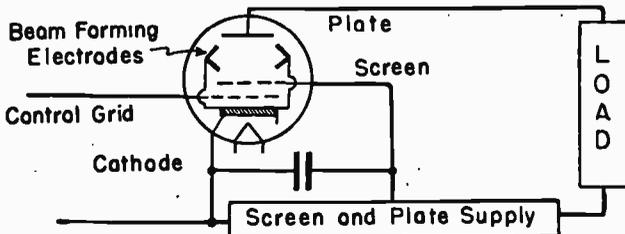
FIG. 3.—Circuit Connections to a Beam Power Tube.
