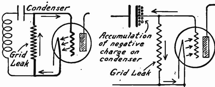
FIG. 2.—Action of a Grid Leak Detector. At the left is shown conventional current flow, positive to negative, while the grid is positive. At the right is the corresponding electron flow and charging of the grid condenser.
