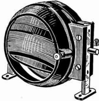
FIG. 1.—Variometer with Spherical Windings.
