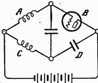
FIG. 10.—The Rice Balanced Circuit in Bridge Form.
