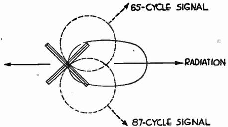
FIG. 10.—Radiation from Visual Beacon Transmitter.
