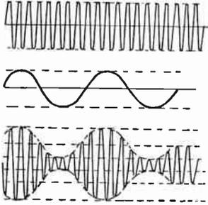
FIG. 7.—Combining the Frequencies in Modulation.
