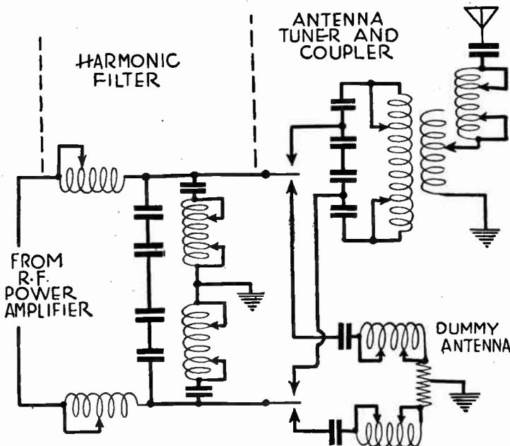
FIG. 10.—Antenna System and Harmonic Filter.
