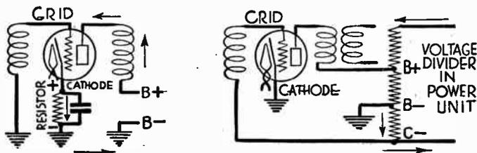
FIG. 6.—Biasing for Heater Tubes.
