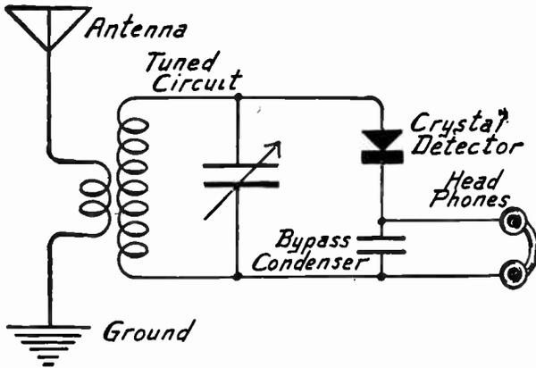
Receiver Circuit with Crystal Detector.
