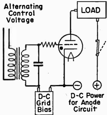
FIG. 4.—A-c Control of D-c Power for Load.
