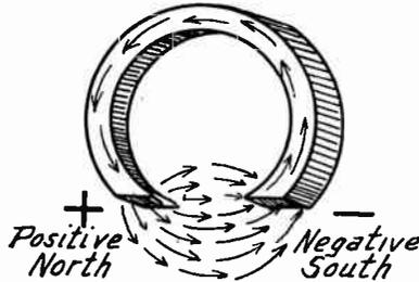
FIG. 1.—The Poles and Field of a Magnet.
