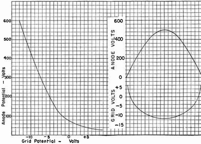
FIG. 1.—Average Breakdown Potentials for a Gas-filled Tube.
