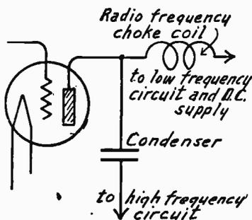
FIG. 1.—Separation of Frequencies with a Choke Coil.
