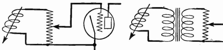
FIG. 11.—Volume Controls for Phonograph Pickups.
