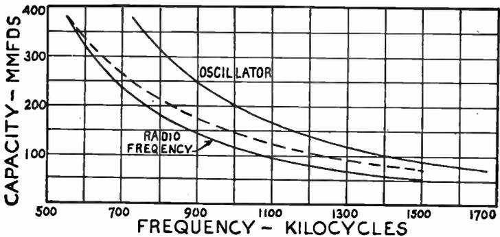
FIG. 19.—Change of Capacity to Maintain Oscillator Frequency.
