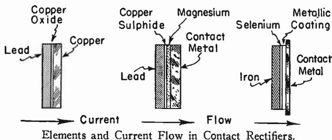
Any number of rectifier units may be connected in parallel to handle larger currents provided all the units so connected have the same voltage rating.
