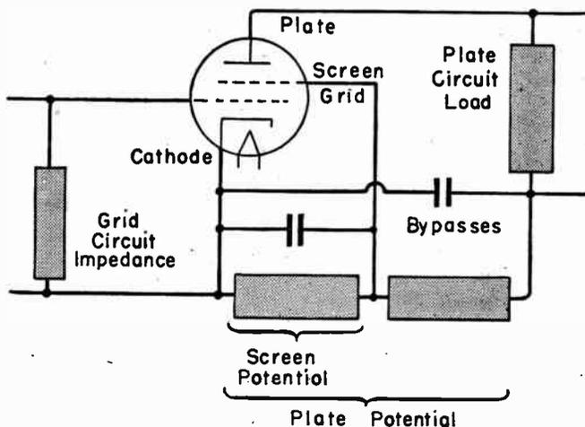
FIG. 1.—Typical Connections for a Screen Grid Tube.
