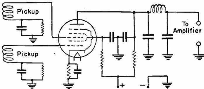
FIG. 2.—Separate Frequencies Combined in Pentagrid Mixer for Output of Beat Frequency Oscillator.
