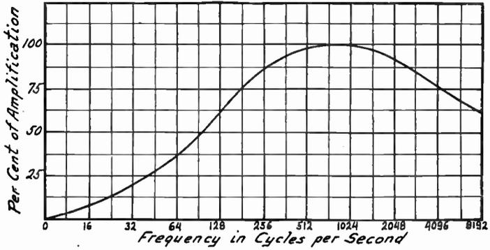
FIG. 3.—Amplification Curve of a Poor Audio Transformer.
