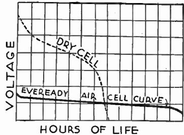
FIG. 2.—Dry Cell Air Cell Life Comparison Chart.
