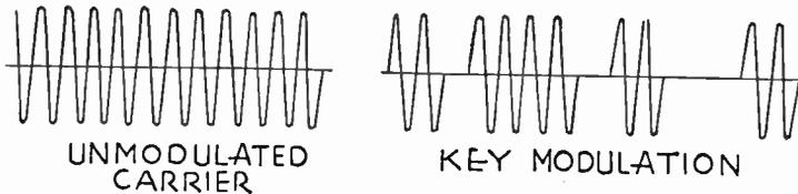
FIG. 1.—Unmodulated Carrier Wave and Key Modulation.
