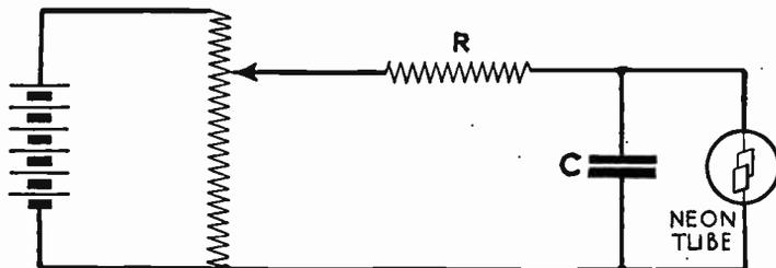
FIG. 9.—Simple Neon Type Saw-tooth Wave Shape Generator.
