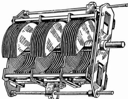
A Ganged Condenser for Tuning Three Circuits.
