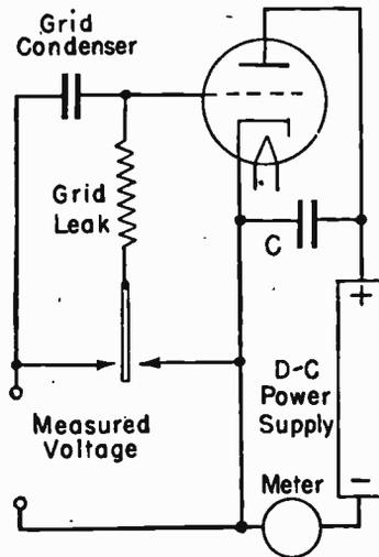
FIG. 2.—Grid Leak Detector Used as VT Voltmeter.
