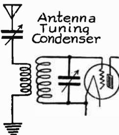
FIG. 1.—Connection of Series Condenser for Antenna Tuning
