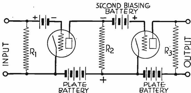
FIG. 2.—Two-Stage Direct Current Amplifier.
