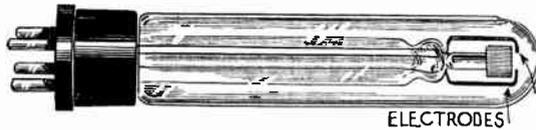
FIG. 9.—Glow Lamp for Sound Recording on Film.
