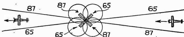
FIG. 7.—Reversal of Signals as Beacon Is Passed.
