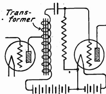
FIG. 3.—Auto-Transformer Interstage Coupling.
