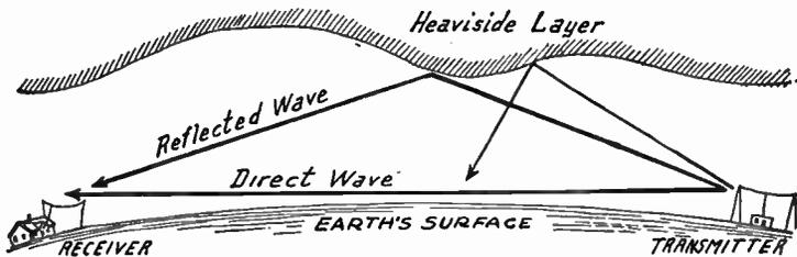
FIG. 1.—Effect of Heavyside Layer on Fading
