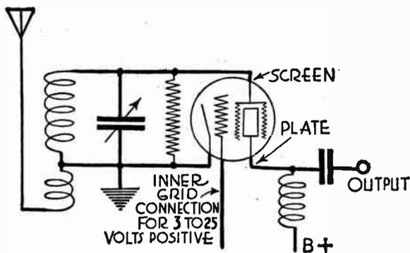
FIG. 7.—Screen Grid Tube as Space Charge Detector
