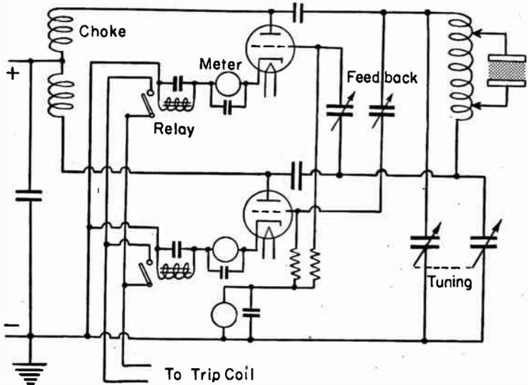
FIG. 3.—Typical Circuit for Electrostatic Heating.
