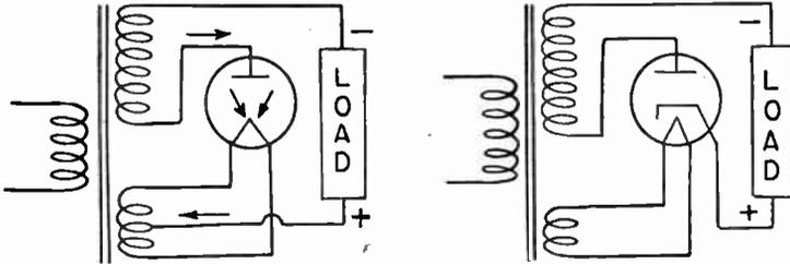
FIG. 1.—Tubes Used as Half-wave Rectifiers.
