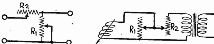
FIG. 5.—L-section Attenuators.
