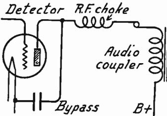
FIG. 7.—Radio Frequency Choke and Bypass on Detector for Prevention of Oscillation.
