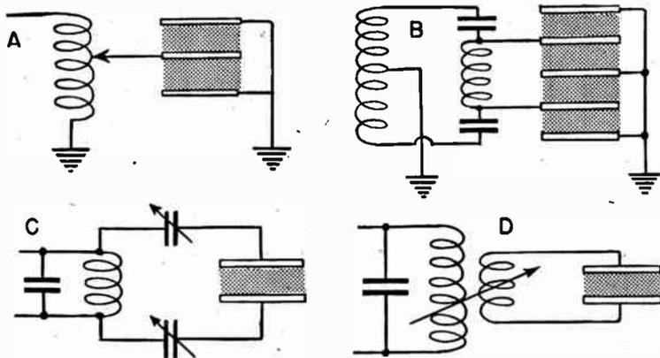
FIG. 2.—Electrode Arrangements for Electrostatic Heating.
