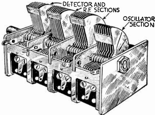
FIG. 20.—Oscillator Tuning Condenser with Special Plates.
