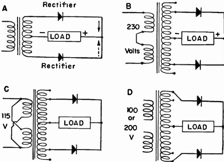
FIG. 5.—Contact Rectifiers in Full-wave Circuits.
