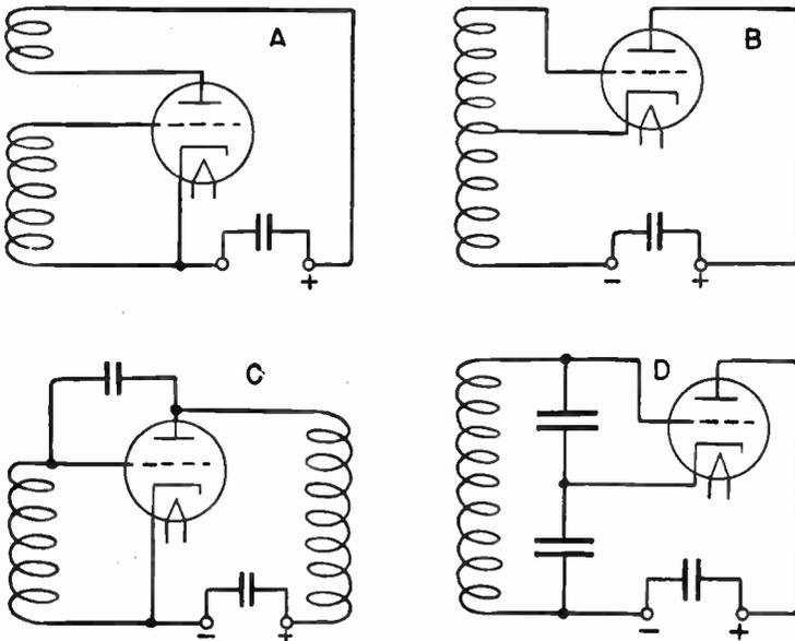
FIG. 2.—Methods of Providing Feedback.
