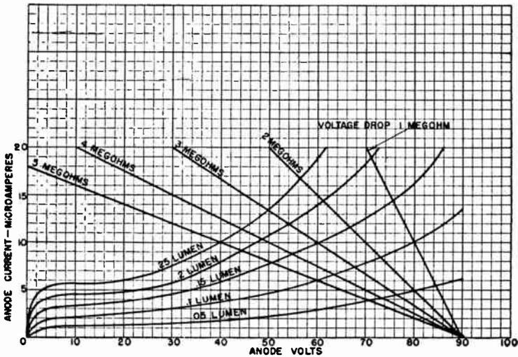
FIG. 9.—Load Lines Showing Phototube Performance.
