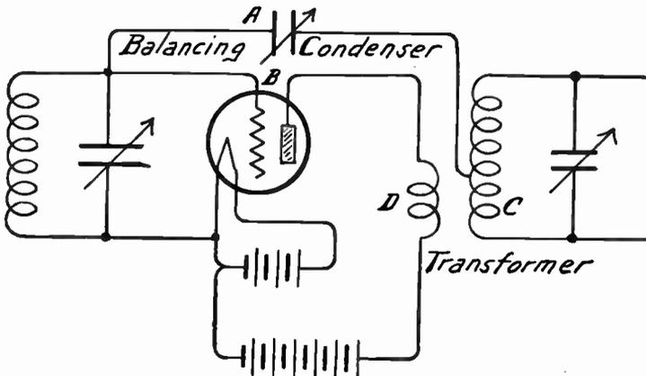
FIG. 2.—Neutrodyne Method of Balancing.
