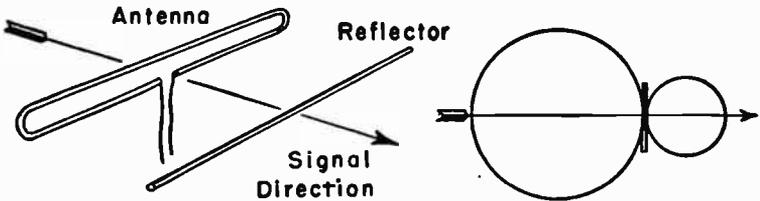
FIG. 9.—A reflector and the resulting directional pattern.
