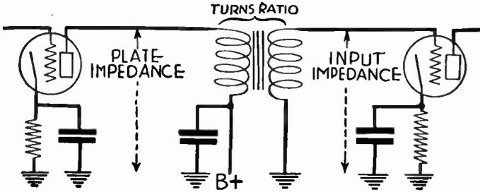
FIG. 2.—Circuit for Transformer Coupling.
