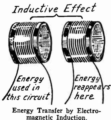
If the induction is brought about by the magnetic field around a conductor or coil, the voltage and current which are induced may be set up either in the conductor or coil having the field or in any other nearby conductor or circuit. If the induced voltage is in the same conductor whose field causes the induction, the action is called self-induction. If the voltage is induced in a nearby circuit the action is called mutual-induction.
