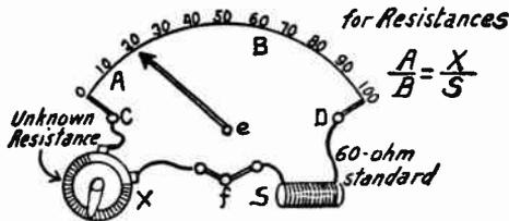
FIG. 6.—Resistance Measurement with Bridge.
