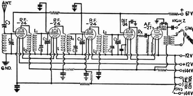
FIG. 15.—Circuits of Typical Airplane Receiver.
