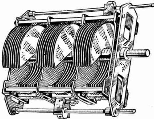
A Ganged Condenser for Tuning Three Circuits.
