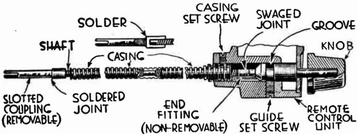
FIG. 5.—Construction at "Dental Cable" Flexible Control Shaft.
