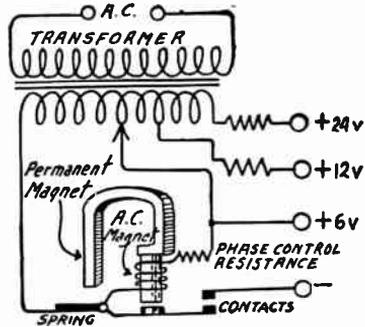
FIG. 2.—Half-wave Vibrating Rectifier.
