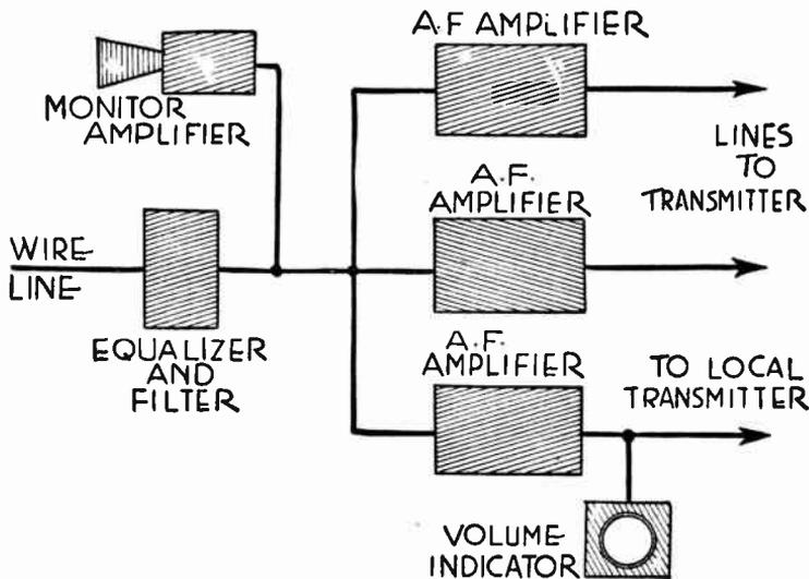
FIG. 5.—Bridging System Used in Chain Broadcasting.
