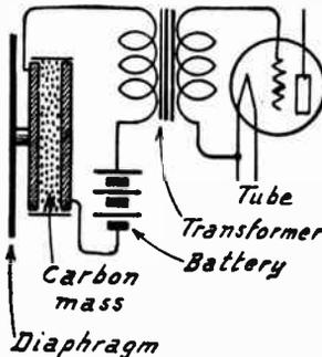
FIG. 1.—Simple Type of Microphone.
