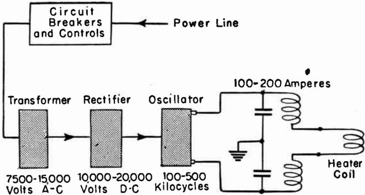
FIG. 5.—Principal Parts of an Induction Heating System.
