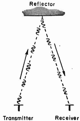
FIG. 2.—Wave Pulses between Transmitter and Receiver.
