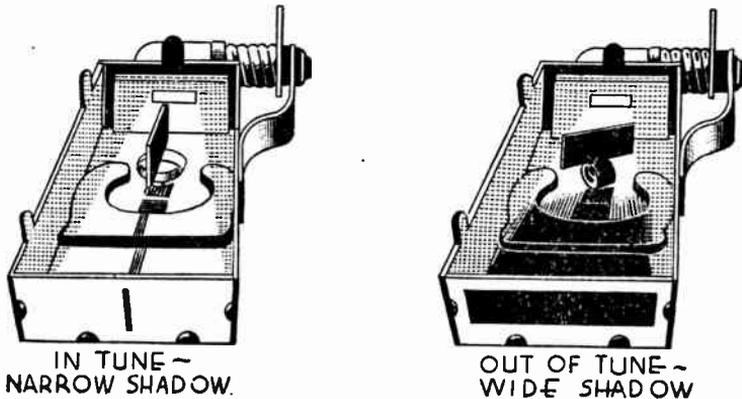
FIG. 12.—Iron Vane Tuning Meter
