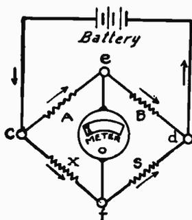
FIG. 1.—Principle of the Wheatstone Bridge.
