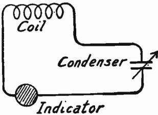
FIG. 1.—The Simplest Frequency Meter Circuit.
