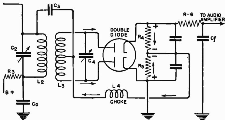
FIG. 6.—The Discriminator Stage of an FM Receiver.
