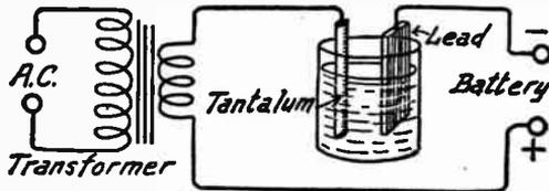
Tantalum Electrolytic Rectifier for Battery Charging.
