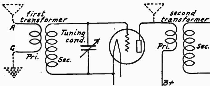
FIG. 1.—Antenna Connections for Testing Radio Stages.
