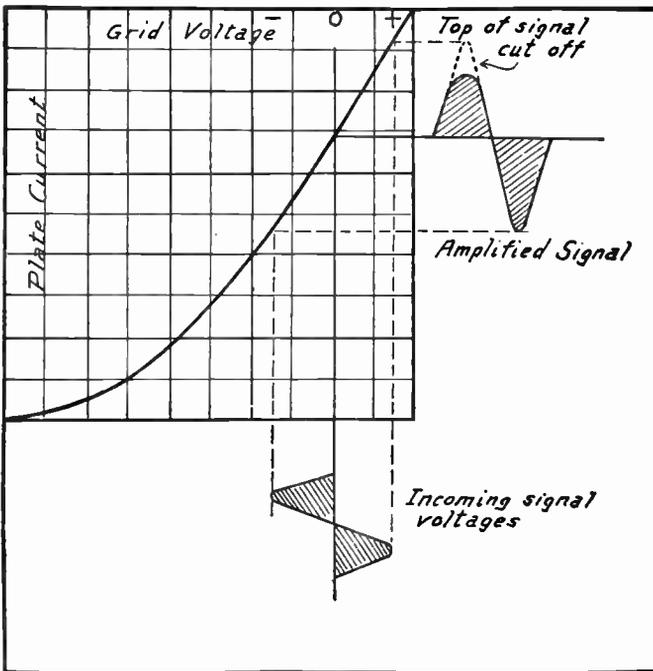
FIG. 2.—Distortion Caused by Zero Grid Bias.
