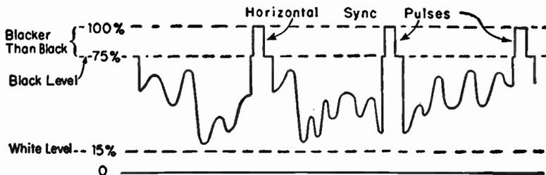
FIG. 7.—Horizontal Sync Pulses During Blanking Intervals.
