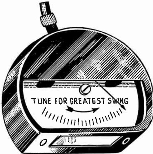
FIG. 11.—Reversed Scale Meter Tuning Indicator
