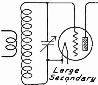
FIG. 4.—Large Secondary Giving Increased Power or Voltage.
