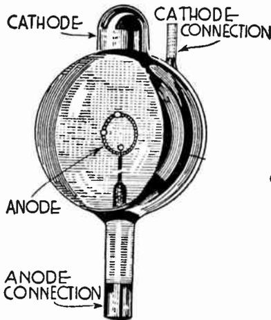
FIG. 1.—Phototube with Wall Type of Cathode.
