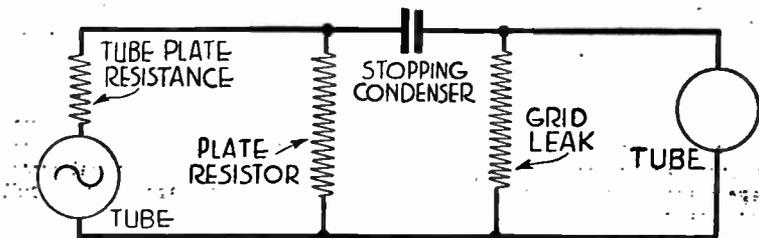
FIG. 2.—Simplified Diagram of Resistance Coupling.
