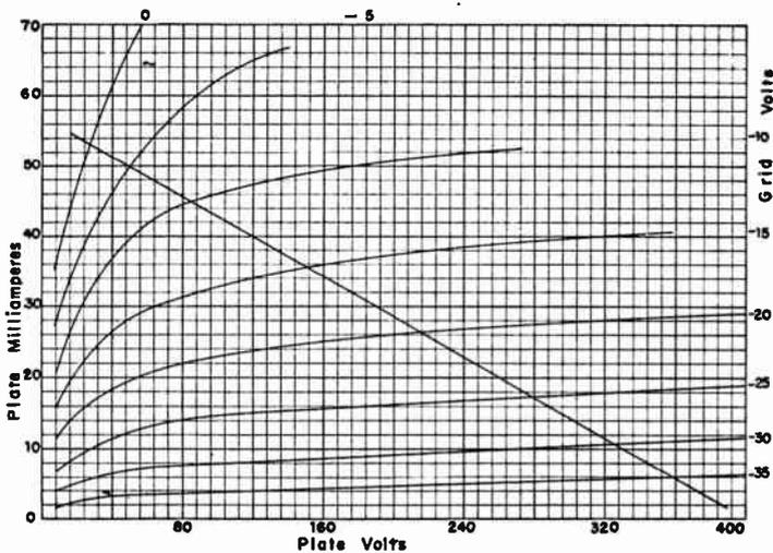
FIG. 5.—Plate Characteristics of a Power-amplifier Pentode.
