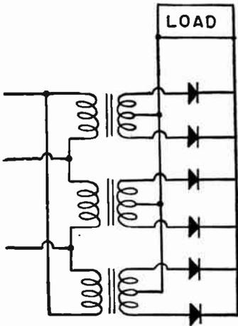
FIG. 4.—Six Elements with Center-tapped Transformer.
