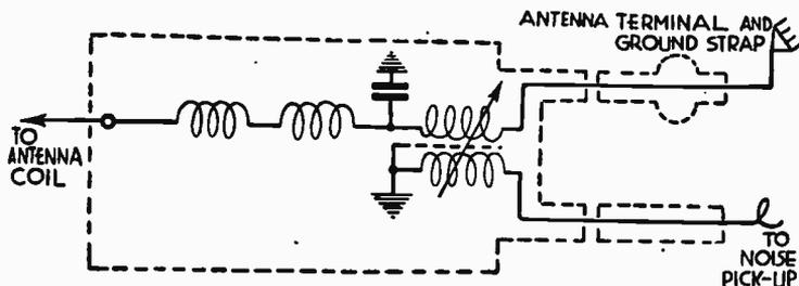
FIG. 11.—“Magic Eliminator” Used on Galvin Motorola Automobile Radio Receivers.
