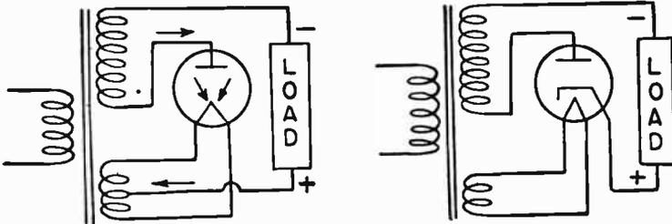
FIG. 1.—Tubes Used as Half-wave Rectifiers.
