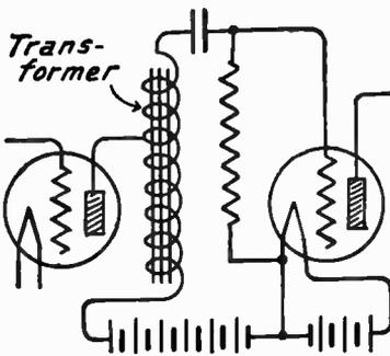
FIG. 3.—Auto-Transformer Interstage Coupling.
