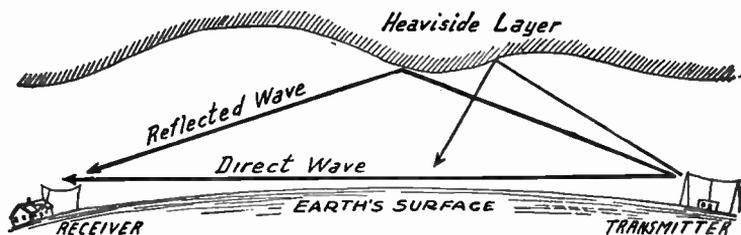
FIG. 1.—Effect of Heaviside Layer on Fading
