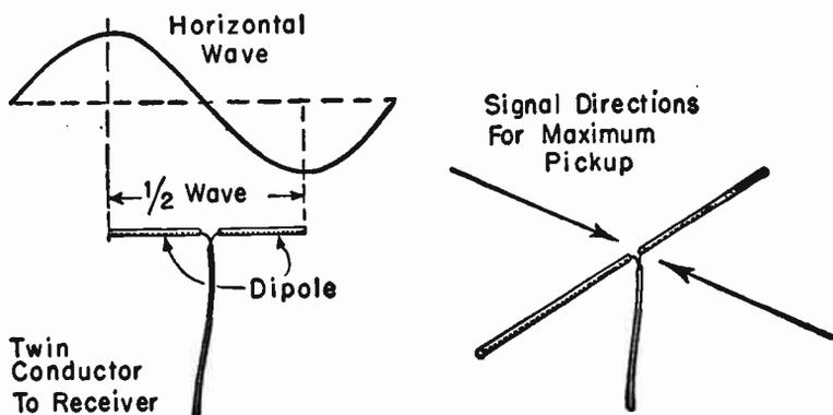
FIG. 14.—Half-wave Dipole Antenna.
