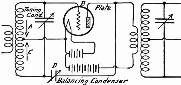
FIG. 4.—Rice Method of Balancing.
