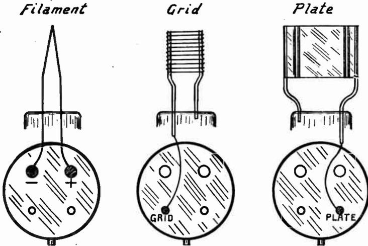
FIG. 2.—Connections Between Tube Elements and Base Prongs
