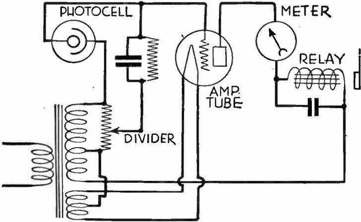
FIG. 11.—The Relay Opens upon Increase of Light.
