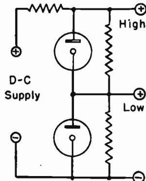
FIG. 4.—Two Tubes Regulating Two Voltages.
