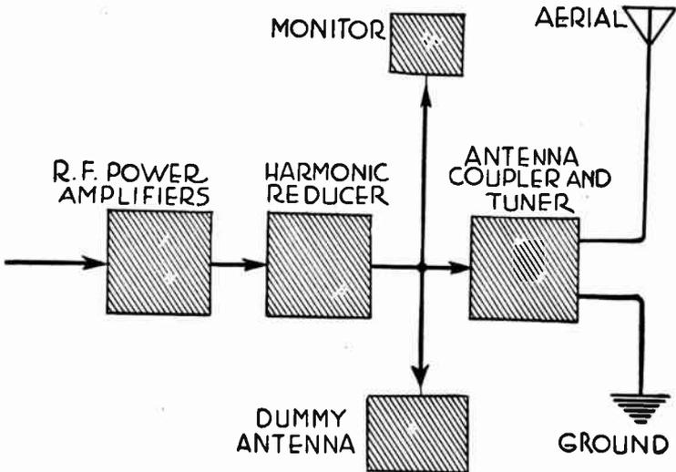
FIG. 3.—High Power Equipment Used at Transmitter.
