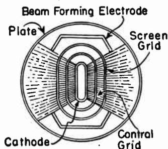
FIG. 1.—Element Arrangement in Beam Power Tube.
