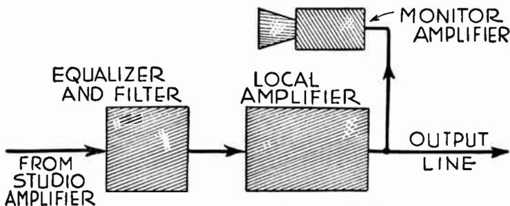
FIG. 4.—Equipment at Repeater Station.
