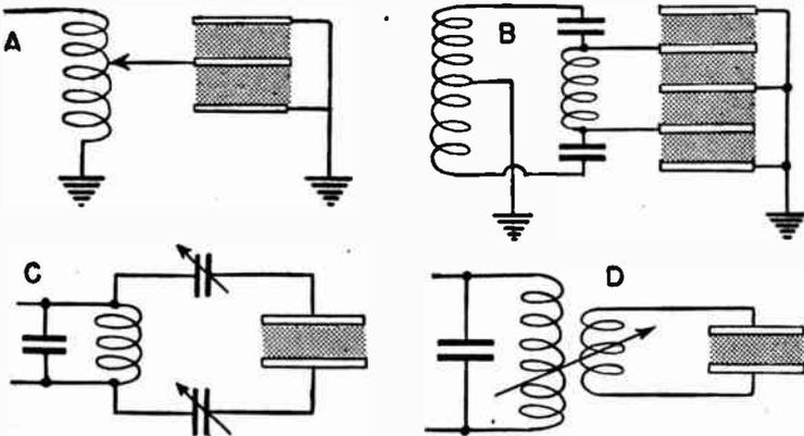
FIG. 2.—Electrode Arrangements for Electrostatic Heating.
