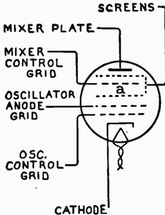
FIG. 23.—The Pentagrid Converter.
