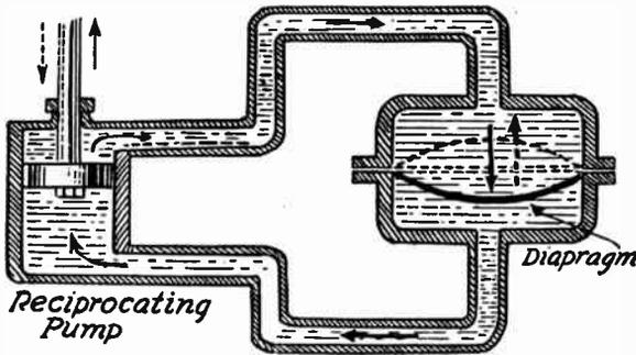
FIG. 5.—Hydraulic Explanation of Condenser Action.
