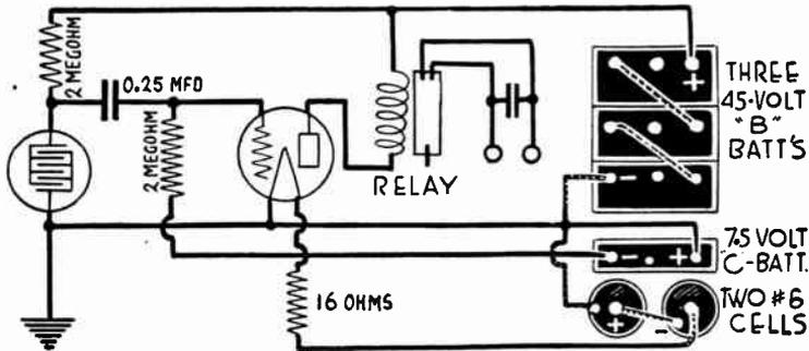
FIG. 6.—Photoconductive Cell Amplifier for Batteries.
