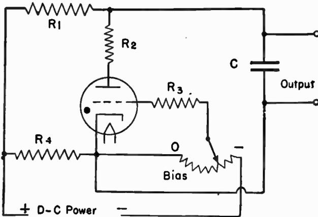
FIG. 6.—Relaxation Oscillator Using Thyratron Tube.
