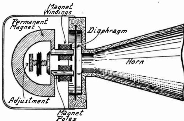
FIG. 1.—Electromagnetic Type of Loud Speaker.
