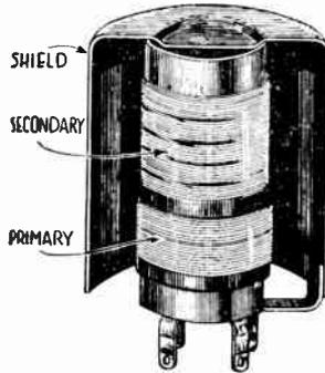
FIG. 2.—Shielded Radio Frequency Transformer.
