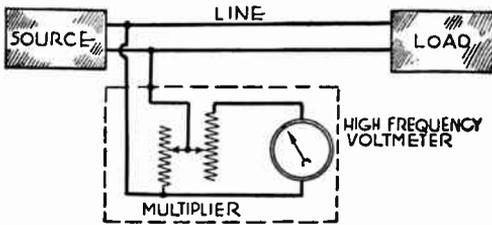
FIG. 1.—Simple Form of Volume Indicator.
