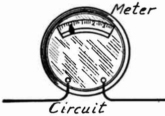
FIG. 1.—Ammeter in Series with Circuit.
