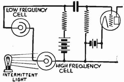
FIG. 15.—Phototube Amplification of Carrier Frequency.
