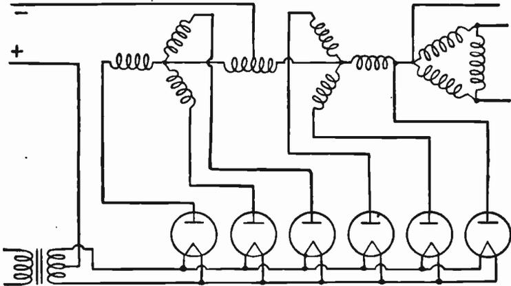
FIG. 3.—Three-phase Double-Y Parallel Rectifier.
