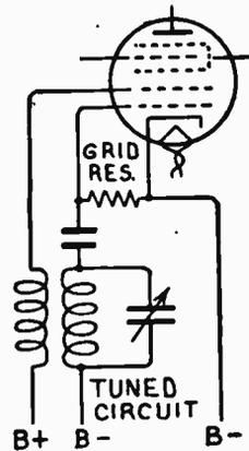
FIG. 24.—Pentagrid Oscillator Circuit.
