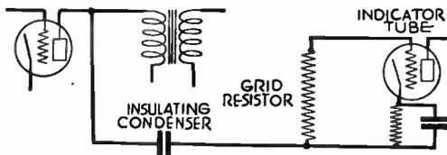
FIG. 3.—Indicator Connection Through Condenser.
