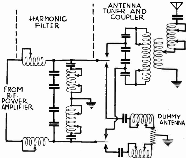
FIG. 10.—Antenna System and Harmonic Filter.
