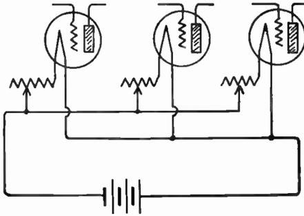
FIG. 2.—Tube Filaments in Parallel Circuit.
