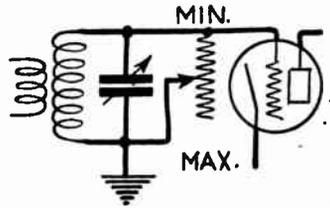
FIG. 17.—Volume Control in Grid Circuit.
