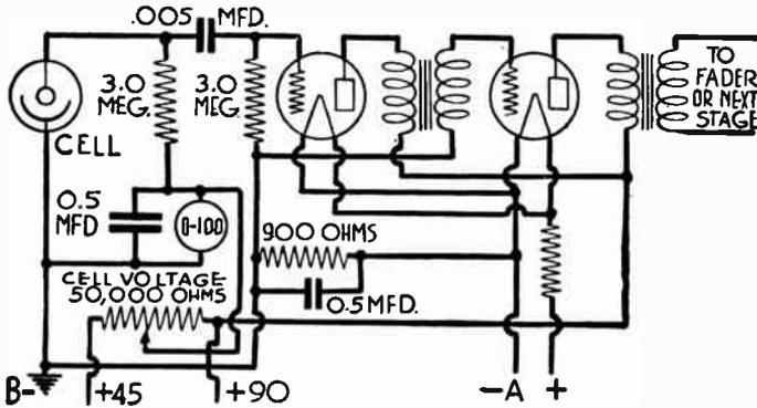
FIG. 14.—Sound Picture Amplifier with Phototube.
