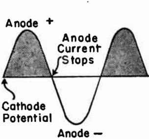
FIG. 5.—Anode Current Flows Only During Positive Half-cycles.
