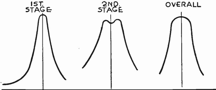
FIG. 15.—Resonance Curves for Intermediate Amplifier.
