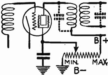
FIG. 16.—Screen Voltage Control of Volume.
