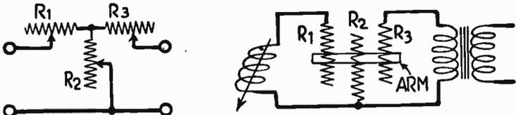
FIG. 6.—T-section Attenuators.
