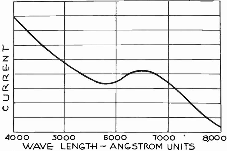
FIG. 5.—Color Sensitivity of Selenium Cell.
