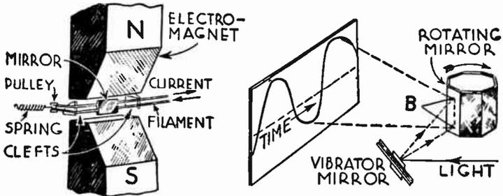
FIG. 2.—Principle of the Duddell Oscillograph.
