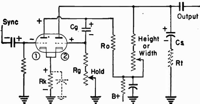
FIG. 27.—Multivibrator Oscillator for Television Sweep Circuits.
