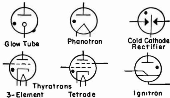
FIG. 1.—Symbols for Gas-filled Tubes.
