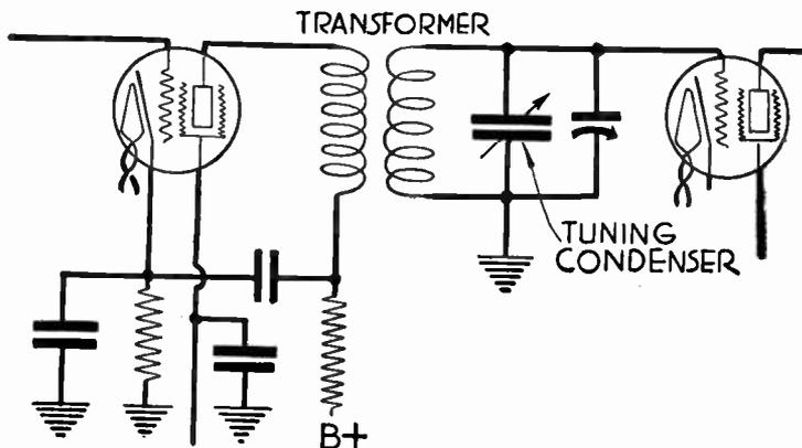
FIG. 1.—Transformer Coupling for Radio Frequencies.
