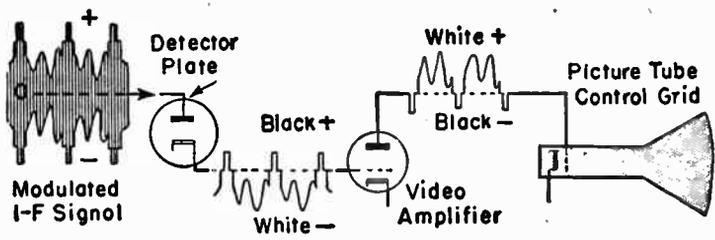
FIG. 20.—Signal Polarities with a Single Video Amplifier.
