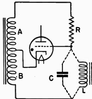
FIG. 7.—Principle of Phase-shift Control Employing Resistance and Capacity or Inductance.
