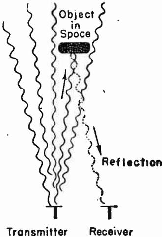
FIG. 1.—Reflection of Radar Waves.
