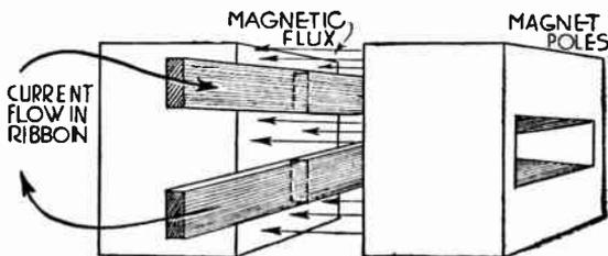
FIG. 8.—Magnetic Action in Light Valve.
