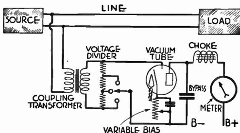
FIG. 2.—Vacuum Tube Type of Volume Indicator.
