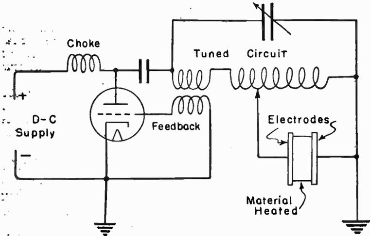
FIG. 1.—Simplified Circuit for Electrostatic Heating.
