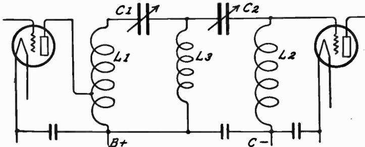
FIG. 7.—Circuit Arrangement of Vreeland Band Selector.
