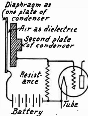
FIG. 3.—Condenser Microphone.
