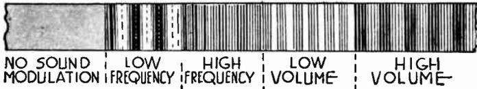
Fig. 6.—Changes in Variable Density Sound Track.
