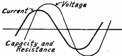
FIG. 2.—Current Leading Voltage.
