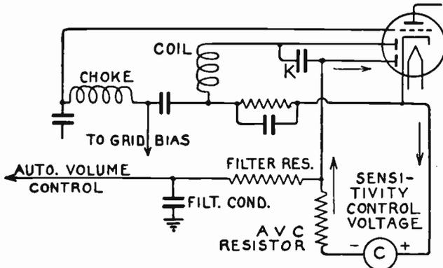
FIG. 5.—Sensitivity Control with Double-diode.
