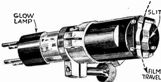
FIG. 10.—Glow Lamp Holder with Slit.
