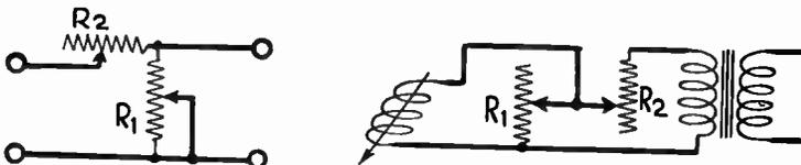
FIG. 5.—L-section Attenuators.
