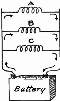
FIG. 1.—Parallel Circuits.
