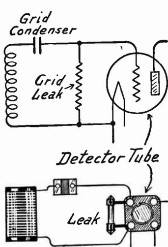
FIG. 1.—Grid Leak Connected to Detector Tube Terminals.
