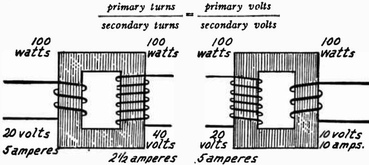
FIG. 7.—A Step-Up Transformer.
