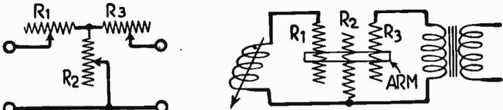
FIG. 6.—T-section Attenuators.
