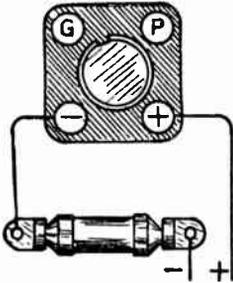
FIG. 1.—Filament Resistor.
