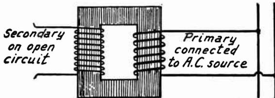
FIG. 9.—Transformer at No Load.
