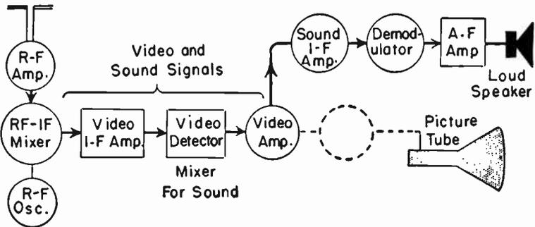
FIG. 23.—Path of Signal in Intercarrier Sound System.
