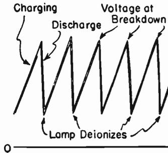
FIG. 5.—Output Wave Form of Neon Oscillator.
