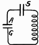
other. Any two condensers in series have a combined capacity less than the capacity of either one alone, therefore this lessened capacity used with the coil allows resonance or tuning at higher frequencies or lower wavelengths.
