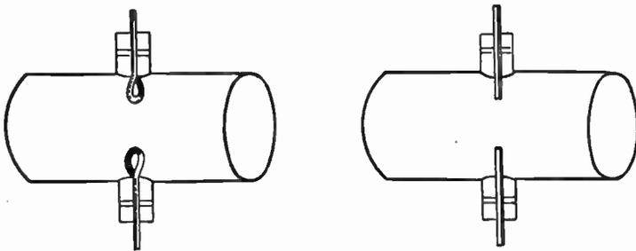
FIG. 2.—Energy Transfer Probes for Cavity Resonator.
