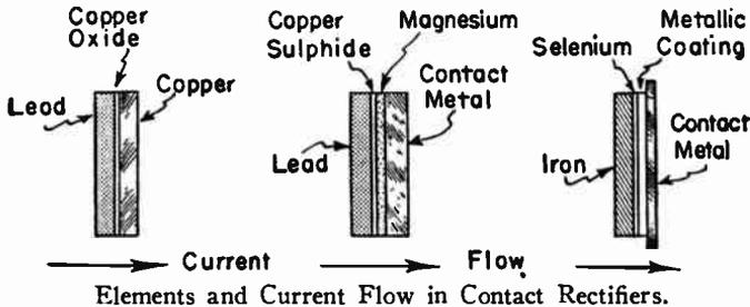
Any number of rectifier units may be connected in parallel to handle larger currents provided all the units so connected have the same voltage rating.
