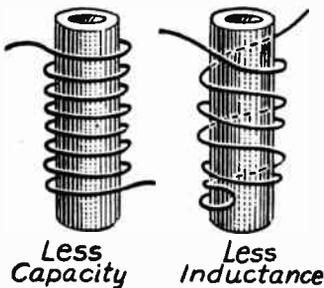
FIG. 1.—Space Winding and Non-inductive Winding of Resistors.
