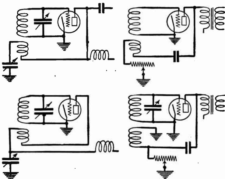
FIG. 5.—Regeneration Control Devices Having One Side Grounded
