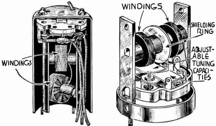
FIG. 16.—Construction of Intermediate Frequency Transformers.
