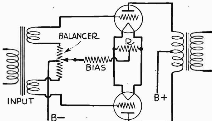
FIG. 8.—Equalizing Plate Currents in Push-pull Tubes.
