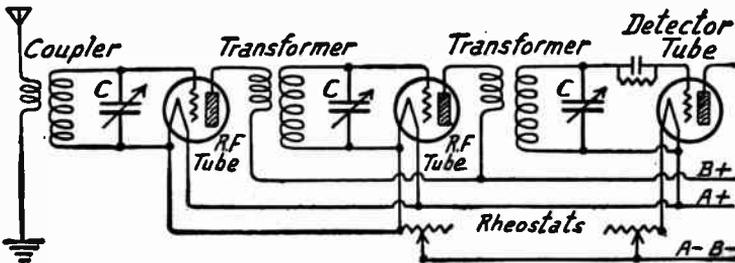
Radio Frequency Circuits of Tuned Radio Frequency Receiver.
