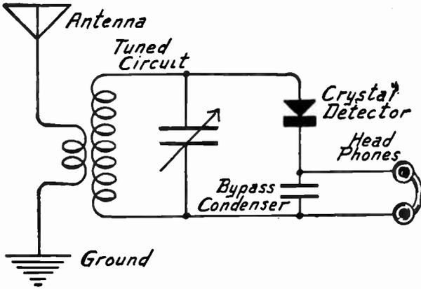
Receiver Circuit with Crystal Detector.
