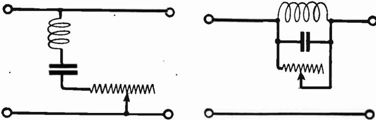
FIG. 6.—Filters for Reduction of Resonance Peaks.
