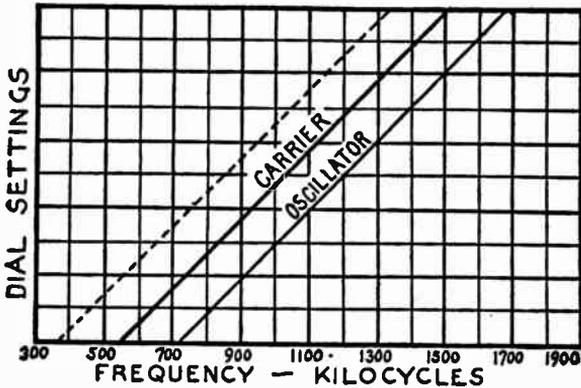
Fig. 5.—Relation of Oscillator and Carrier Frequencies.
