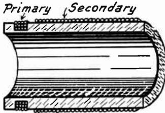
FIG. 6.—Primary and Secondary with Minimum Capacity Coupling to Reduce Oscillation.
