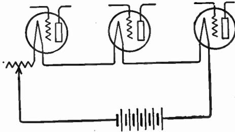
FIG. 2.—Tube Filaments in Series Circuit.
