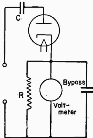
FIG. 6.—Diode Used for a VT Voltmeter.
