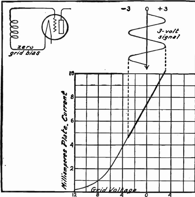
FIG. 1.—Effect of Zero Grid Bias, Distortion.
