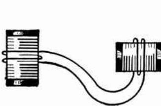
FIG. 1.—Link Circuit with Fixed Coupling.
