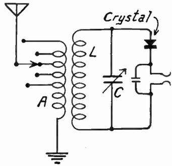
FIG. 2.—Crystal Receiver with Loosely Coupled Antenna Circuit.
