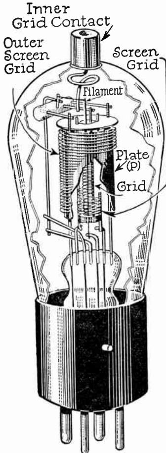
Fig. 1.—Internal Construction of a Screen Grid Tube.
