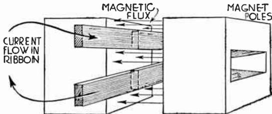
FIG. 8.—Magnetic Action in Light Valve.
