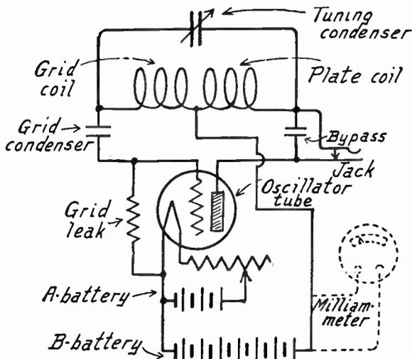
FIG. 4.—Circuits of Radio Frequency Oscillator.
