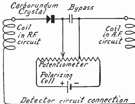
FIG. 5.—Use of Polarizing Battery with Crystal Detector.
