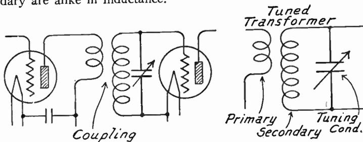
FIG. 1.—Tuned Radio Frequency Transformer Used as Coupler.
