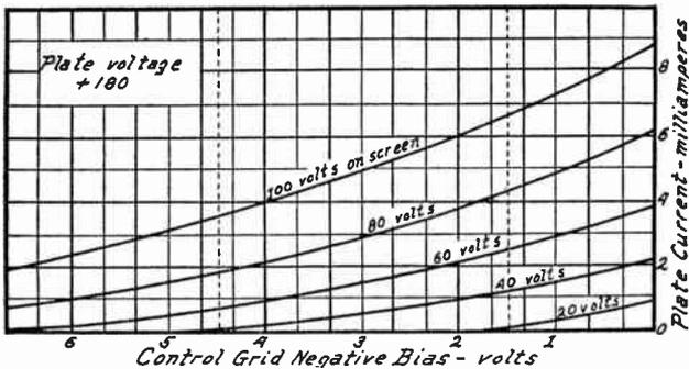
FIG. 3.—Effect of Grid Voltage Bias on Plate Current.
