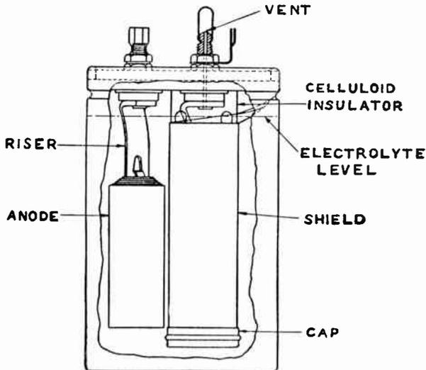
FIG. 5.—The Mershon Electrolytic Condenser.
