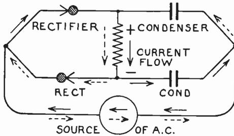
FIG. 10.—Equivalent Circuit for Voltage Doubler.
