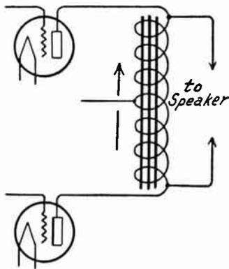
FIG. 10.—Remedies for Unbalance. FIG. 11.—Push-pull Output Choke.
