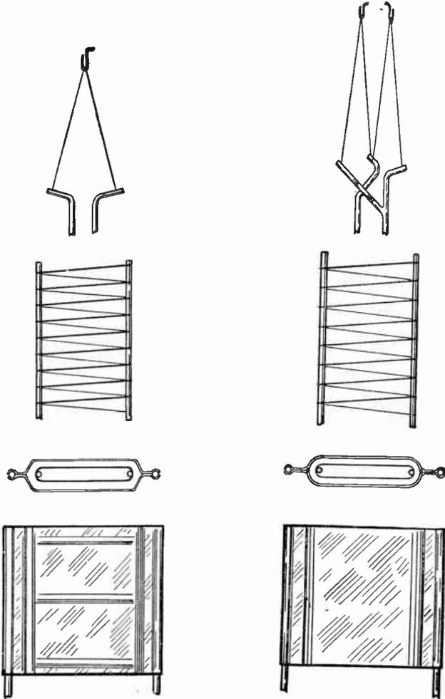
FIG. 4.—Design of a Semi-Power Tube.
