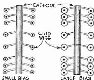
FIG. 5.—Effect of Grid Potential in Variable-mu Tube.
