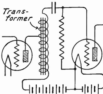
FIG. 3.—Auto-Transformer Interstage Coupling.
