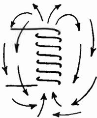
FIG. 7.—Electromagnetic Lines of Force Around a Coil.
