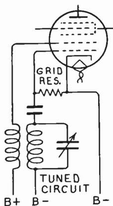
FIG. 12.—Pentagrid Oscillator Circuit.
