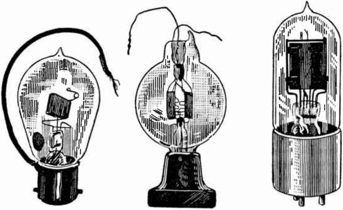
FIG. 1.—Early Experimental Types of Vacuum Tubes
