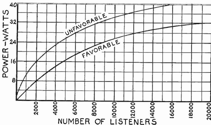
FIG. 11.—Power Requirements According to Number of Listeners.
