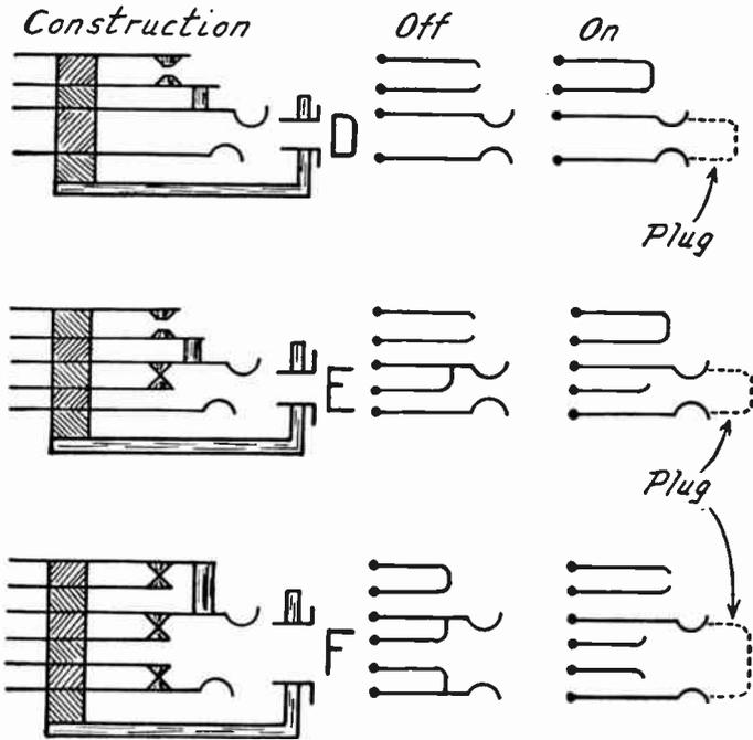
FIG. 2.—Jacks with Two Filament Control Contacts.
