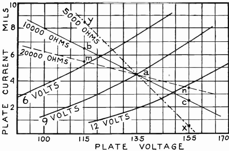
FIG. 7.—Load Line Construction.
