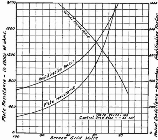
FIG. 5.—Effect of Screen Grid Voltage on Characteristics.
