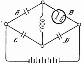
FIG. 9.—The Isofarad Balanced Circuit in Bridge Form.
