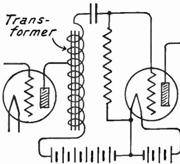
FIG. 3.—Auto-Transformer Interstage Coupling.
