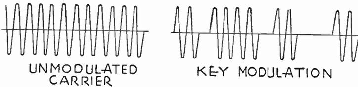
FIG. 1.—Unmodulated Carrier Wave and Key Modulation.
