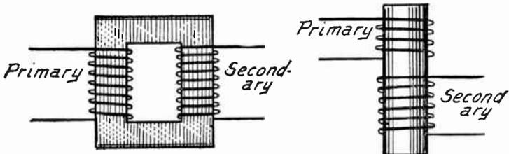
FIG. 1.—Core Type of Transformer.
