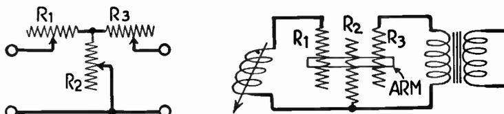
FIG. 6.—T-section Attenuators.
