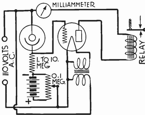
FIG. 12.—Relay Operated with Vacuum Tube and Photocell.
