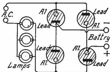
FIG. 3.—Lamp Resistance with Electrolytic Battery Charging Rectifier.
