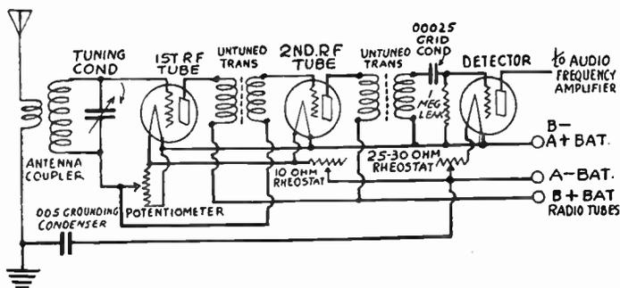
Radio Frequency Amplifier with Untuned Transformers.
