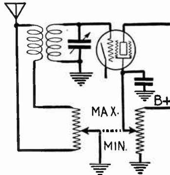
FIG. 21.—Twin Control for Antenna and Screen Voltage.
