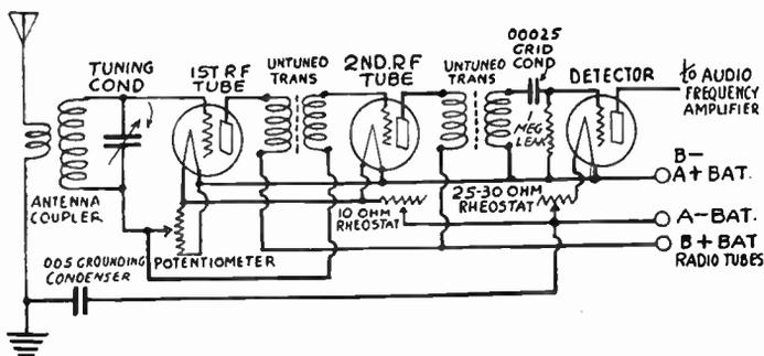
Radio Frequency Amplifier with Untuned Transformers.
