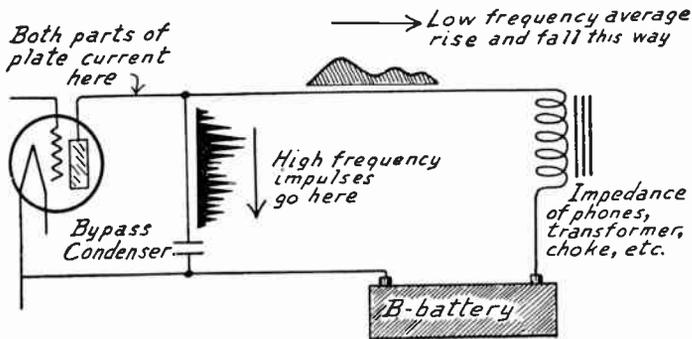
Separation of High and Low Frequencies with Detector Plate Bypass.
