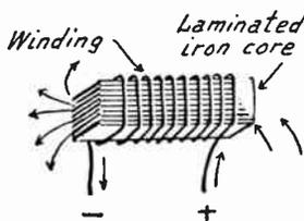
FIG. 4.—An Electromagnet with Its Field.
