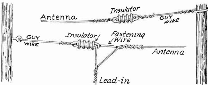
FIG. 1.—Installation of Antenna Insulators.
