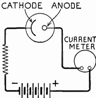
FIG. 2.—Photocell Circuit.
