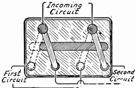
a pole changing switch. The connections of one such switch are shown. It is a form of double-pole, double-throw switch.
