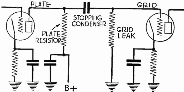
FIG. 1.—Resistance-capacity Coupled Amplifier.
