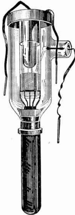
FIG. 5. — Water Cooled Tube
