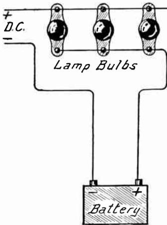
FIG. 1.—Direct Current Battery Charging with Lamp Resistance.
