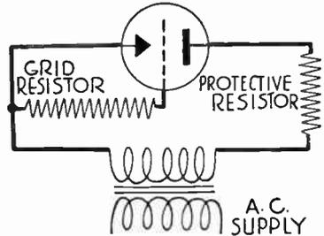
FIG. 5.—Alternating Current Operation of Grid-glow Tube.
