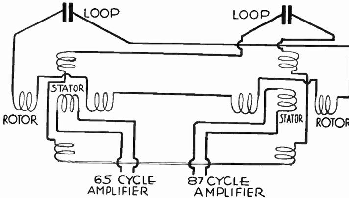
FIG. 11.—Circuit for Beacon Loops.
