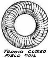
FIG. 1.—Toroid Type of Coil.
