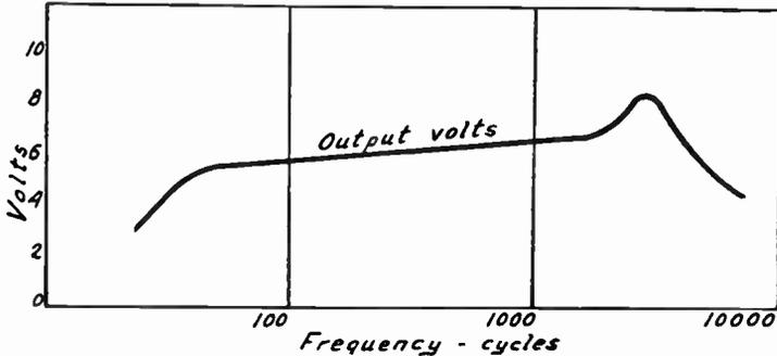
FIG. 7.—Result of Frequency Distortion in Amplifier.
