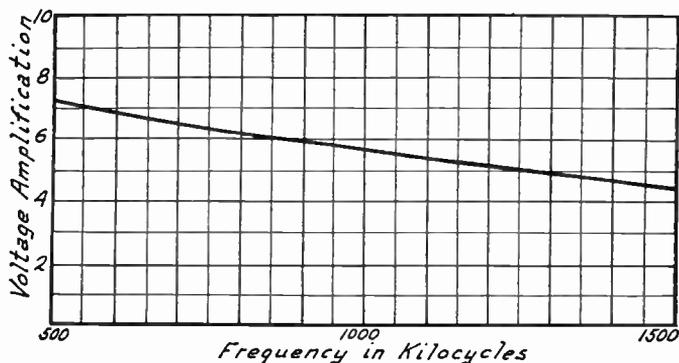
FIG. 3.—Decrease of Amplification with Increase of Frequency.
