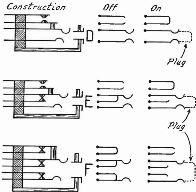
FIG. 2.—Jacks with Two Filament Control Contacts.
