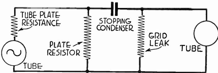
FIG. 2.—Simplified Diagram of Resistance Coupling.
