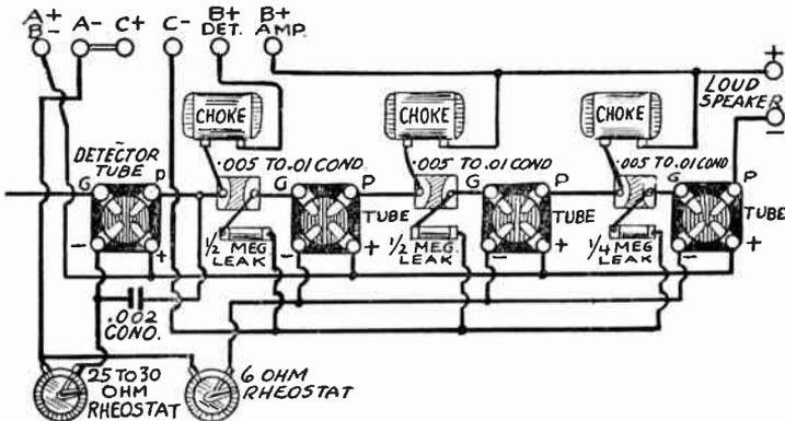
FIG. 3.—Three-Stage Impedance Amplifier Starting with the Detector.
