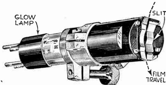
FIG. 10.—Glow Lamp Holder with Slit.
