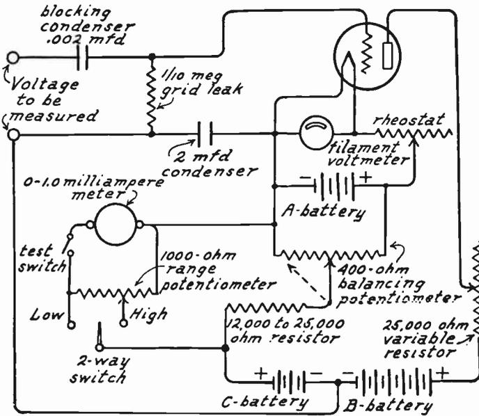
FIG. 2.—Circuits of Two Range Vacuum Tube Voltmeter.
