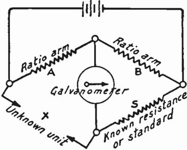
FIG. 3.—Functions of the Arms in a Bridge.
