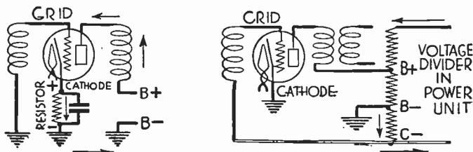
FIG. 6.—Biasing for Heater Tubes.
