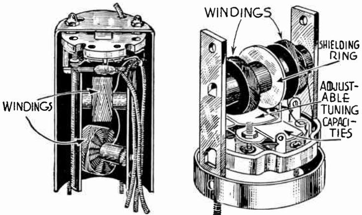
FIG. 16.—Construction of Intermediate Frequency Transformers.
