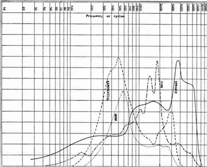
FIG. 5.—Response Curves of Various Types of Speakers.
