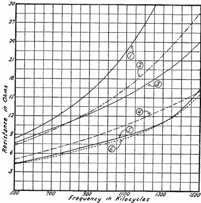
FIG. 2.—Change of Resistance with Change of Frequency in Coils.
