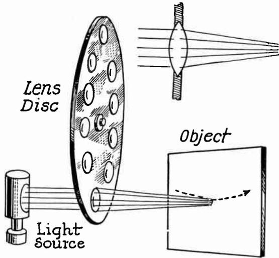
FIG. 13.—Concentration of Light with Lenses in Disc.
