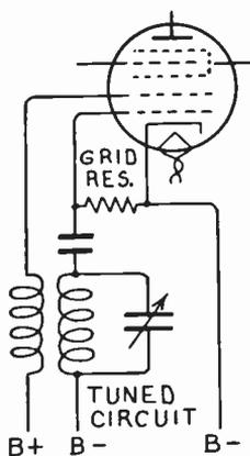
FIG. 12.—Pentagrid Oscillator Circuit.
