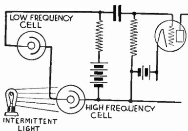
FIG. 16.—Carrier Frequency Produced with Photocells in Series.
