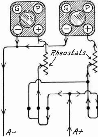
FIG. 8.—Filament Control with Two Tubes in Operation.
