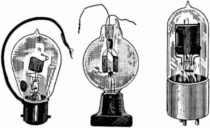
FIG. 1.—Early Experimental Types of Vacuum Tubes
