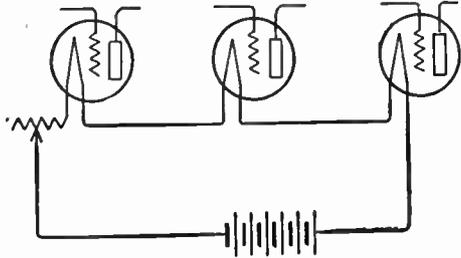
FIG. 2.—Tube Filaments in Series Circuit.
