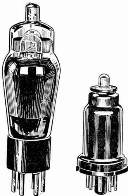
FIG. 7.—Glass Tube with Its Equivalent
