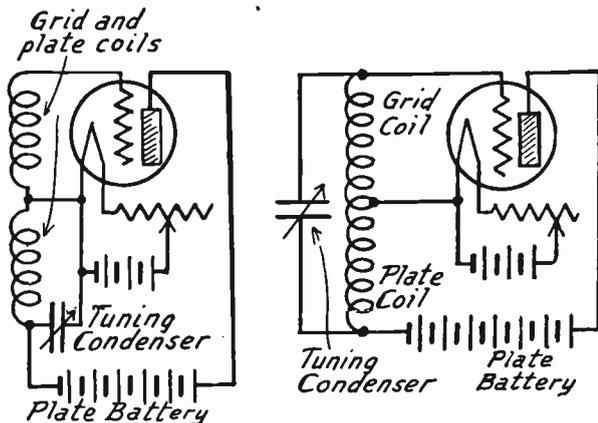
FIG. 1.—Radio Frequency Oscillator with Tuned Plate Coil.
