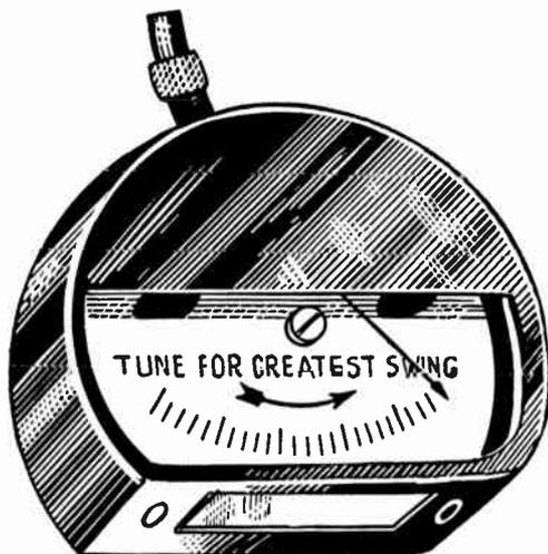
FIG. 11.—Reversed Scale Meter Tuning Indicator
