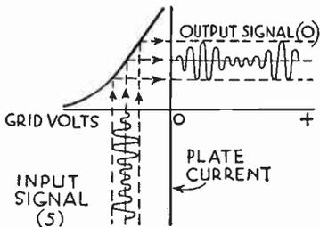
FIG. 1-A.—Class A Operating Characteristics.
