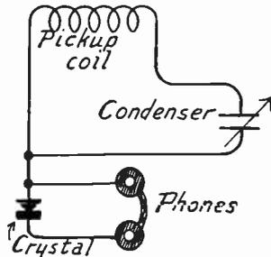
FIG. 6.—Frequency Meter Indicator Coupled through Single Wire.
