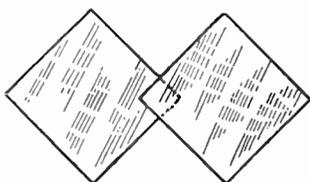
FIG. 3.—Square Plates for Straight Line Wavelength Condenser.
