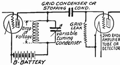
FIG. 1.—Tuned Impedance Coupling for Radio Amplifier.
