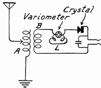
FIG. 4.—Variometer for Tuning Crystal Circuit.
