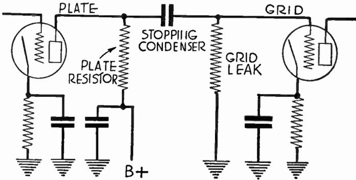
FIG. 1.—Resistance-capacity Coupled Amplifier.
