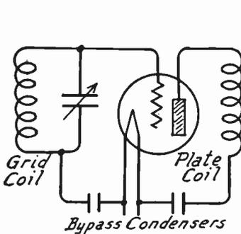
FIG. 1.—Grid and Plate Coils Entering into Regeneration.
