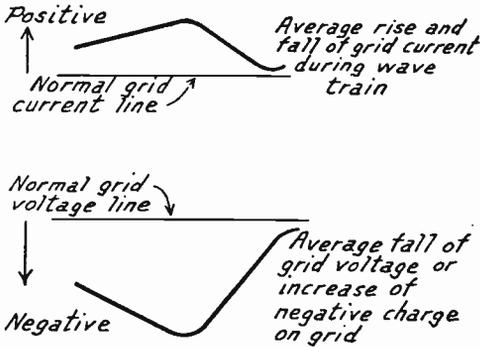
FIG. 7.—Effect of Signal on Grid Current and Grid Voltage in Detector.
