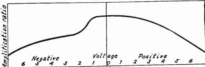
FIG. 9. Variation of Amplification with Changes of Input Voltage.
