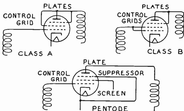
FIG. 1.—Using a Triple-purpose Tube.
