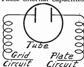
FIG. 1.—Internal Capacity of Tube Requiring Balancing.
