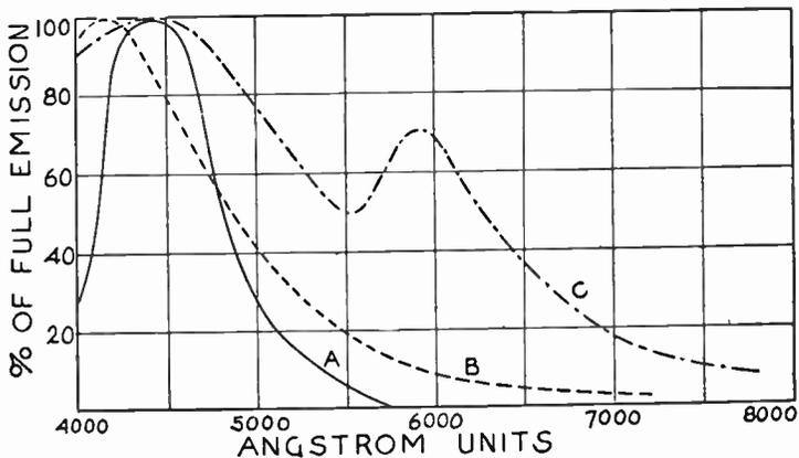
FIG. 9.—Effect of Cathode Form on Photocell Sensitivity.
