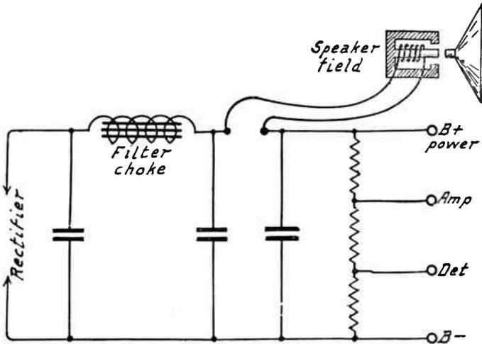
FIG. 10.—Speaker Field Used As a Filter Choke.
