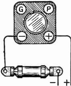
FIG. 1.—Filament Resistor.
