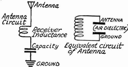
The Antenna Circuit and Its Electrical Equivalent.
