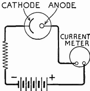
FIG. 2.—Photocell Circuit.
