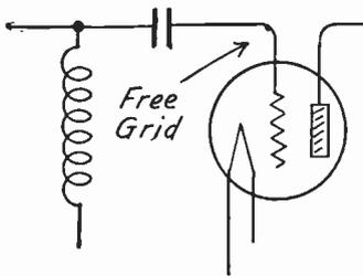
FIG. 3.—Grid Isolated by Condenser With No Leak in Use.
