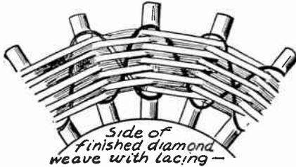
FIG. 3.—Lacing the Finished Diamond Weave Spiderweb Coil.
