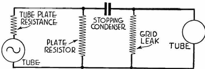
FIG. 2.—Simplified Diagram of Resistance Coupling.
