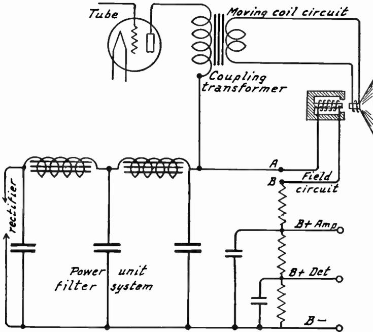
FIG. 9.—Plate Power Unit Connection to Speaker Field.
