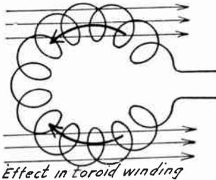
FIG. 3.—Opposing Voltages Set Up in Toroid Winding.
