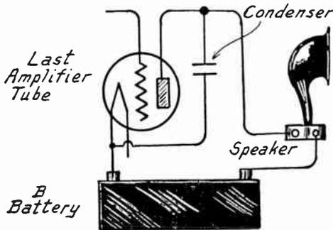
FIG. 1.—Loud Speaker Connected Directly to Last Tube.
