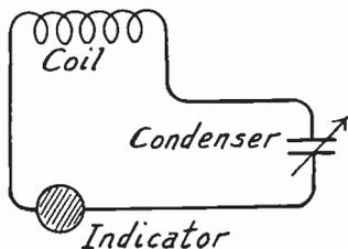
FIG. 1.—The Simplest Frequency Meter Circuit.
