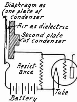
FIG. 3.—Condenser Microphone.
