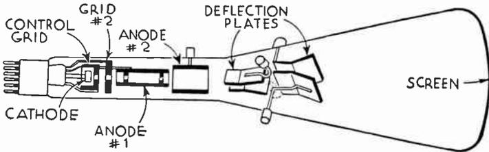
FIG. 3.—Details of 9 in. Cathode Ray Tube.
