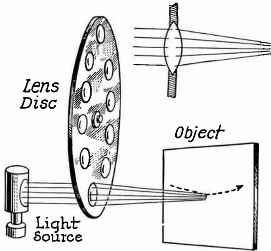
FIG. 13.—Concentration of Light with Lenses in Disc.
