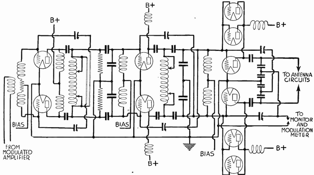
FIG. 9.—Power Amplifier Used at Transmitter.
