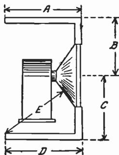
FIG. 13.—Measurements for Box Type Baffle.
