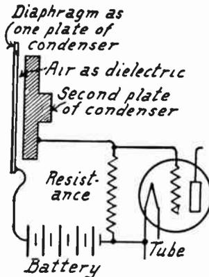
FIG. 3.—Condenser Microphone.
