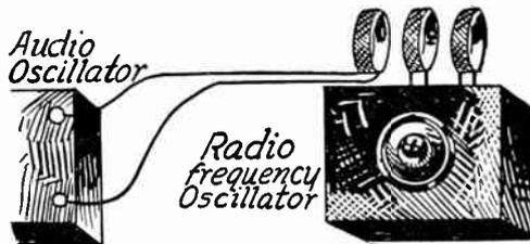
FIG. 6.—Modulating Radio Frequency Oscillator with Audio Oscillator.
