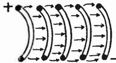
FIG. 2.—Electrostatic Field of a Coil Winding.
