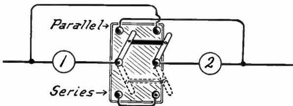
FIG. 2.—Double-Pole, Double Throw Switch with Series-Parallel Connections.
