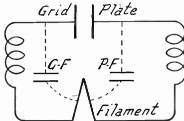
FIG. 5.—Internal Capacities in Parallel with External Circuits.
