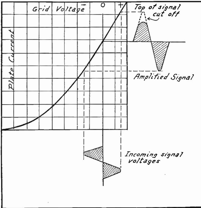
FIG. 2.—Distortion Caused by Zero Grid Bias.
