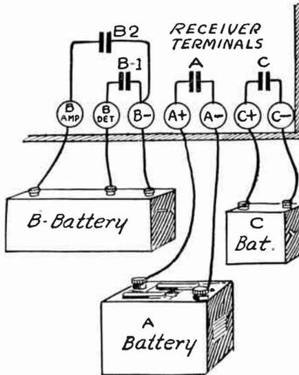
FIG. 3.—Connections of Bypass Condensers to Receiver Terminals.
