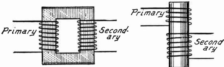
FIG. 1.—Core Type of Transformer.
