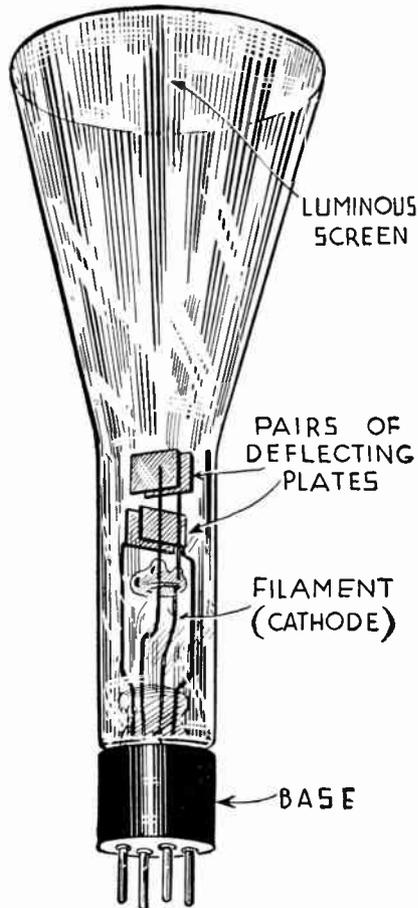
FIG. 2.—Early Type Western Electric Cathode Ray Tube.
