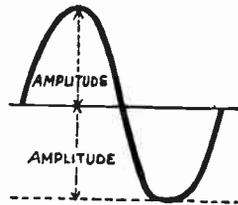
The Amplitude of an Alternating Current Wave.
