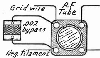
FIG. 12.—Radio Frequency Choke and Bypass on Detector for Prevention of Oscillation.
