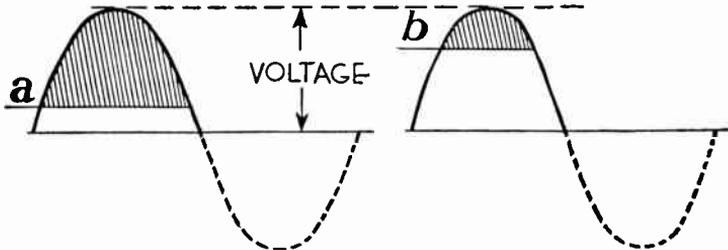
FIG. 6.—Variation of Glow Period with A.C. Operation.
