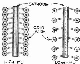
FIG. 4.—Effect of Grid Potential in High-mu and Low-mu Tubes.
