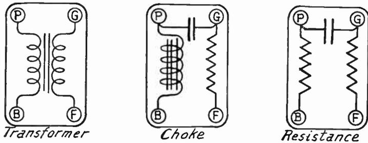
FIG. 5.—Similarity of Terminal Connections with Various Couplers.
