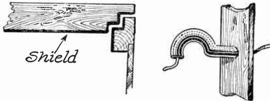
FIG. 8.—Protection of Joints in Shielding.
