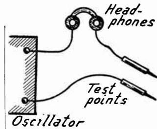
FIG. 4.—Using Audio Oscillator as a Circuit Tester.
