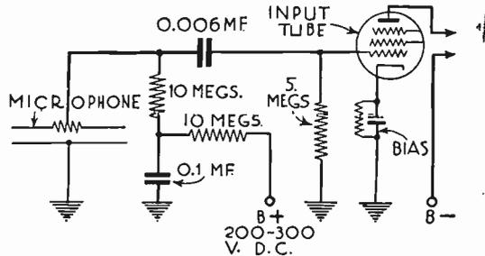
FIG. 2b.—Circuit Connection of Static Velocity Microphone.
