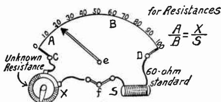
FIG. 6.—Resistance Measurement with Bridge.
