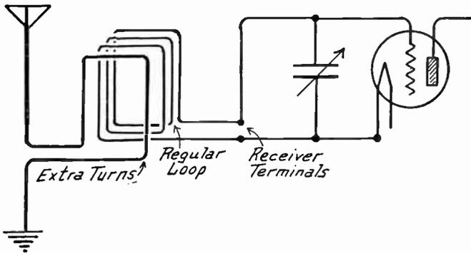
FIG. 2.—Additional Turns for Antenna with Loop.
