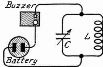
FIG. 2.—Buzzer Excited Oscillator Circuit.
