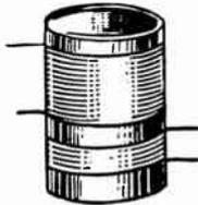
FIG. 5.—Air Core Radio Frequency Transformer.
