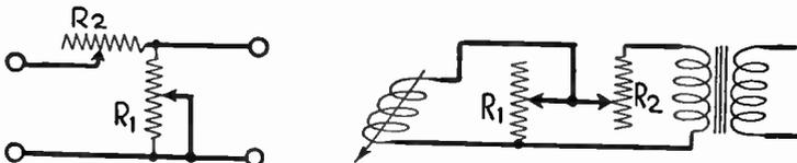
FIG. 5.—L-section Attenuators.
