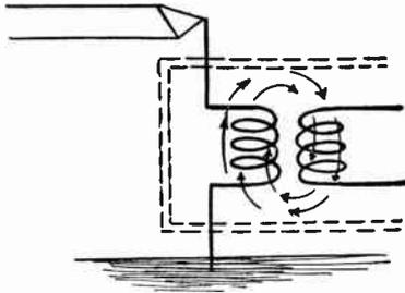
FIG. 9.—Coupled Coils as First Circuit in Receiver.
