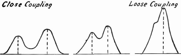
As the coupling is made looser the two peaks keep coming closer and closer together until, with very loose coupling, they practically merge and form a single resonance peak of greater height or amplitude than either of the others alone. This explains the broadness of tuning when using very close coupling in radio frequency circuits.
