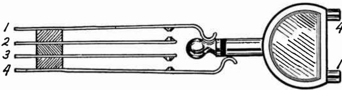
FIG. 2.—Plug Inserted in Jack.
