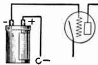
FIG. 3.—Amplifying Circuit for Direct Current.
