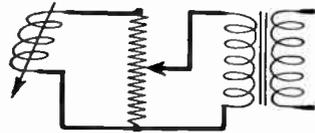
FIG. 3.—Voltage Divider or Potentiometer Control.
