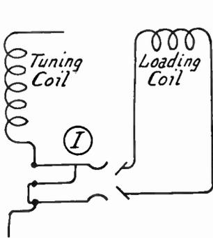
FIG. 28.—Jack for Insertion of Loading Coil.
