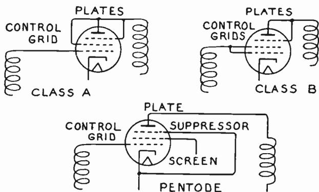
FIG. 1.—Using a Triple-purpose Tube.
