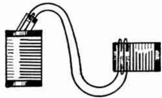
FIG. 2.—Link Circuit with Variable Coupling.
