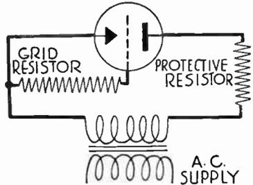
FIG. 5.—Alternating Current Operation of Grid-glow Tube.
