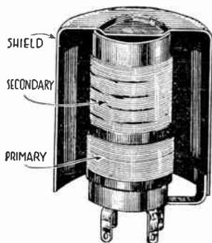
FIG. 2.—Shielded Radio Frequency Transformer.
