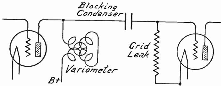
FIG. 1.—Tuned Impedance Coupling with Variometer.
