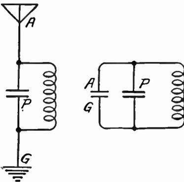
FIG. 2.—Connection of Parallel or Shunting Antenna Condenser.
