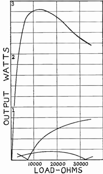
FIG. 5.—Effect of Load on Output. Lower Curves Show Harmonic Output.
