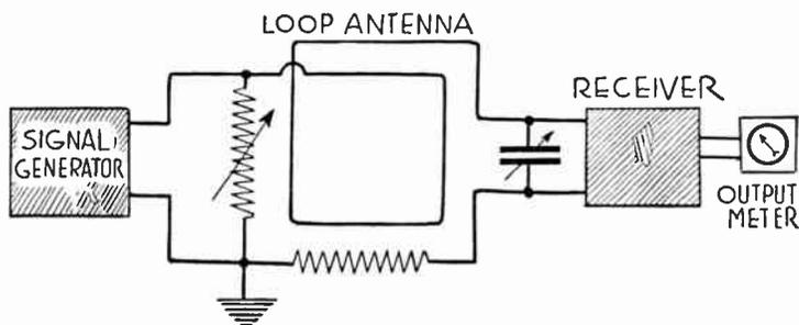
FIG. 12.—Method of Measuring Field Intensity.
