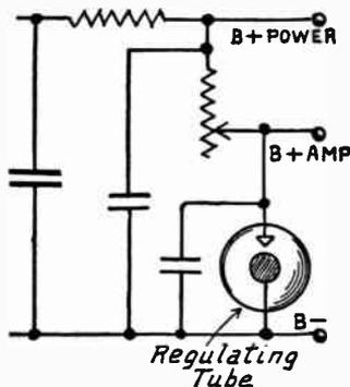
FIG. 3.—Voltage Regulator Tube on Intermediate Plate Voltage.
