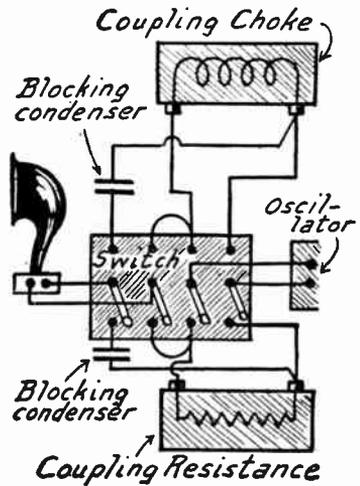
FIG. 2.—Comparative Test of Chokes or Resistances with Audio Oscillator.
