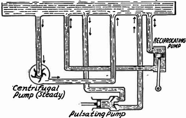
FIG. 1.—Three Water Circuits with One Common Tank.
