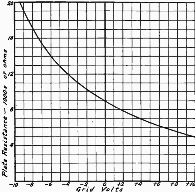
FIG. 7.—Relation Between Grid Voltage and Plate Resistance.
