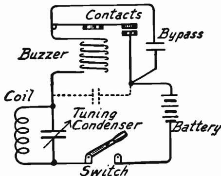
FIG. 1.—Circuits of Buzzer Type Oscillator.
