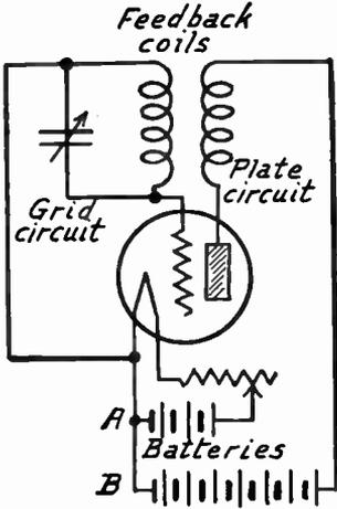
FIG. 3.—Oscillator with Tuned Grid Circuit.
