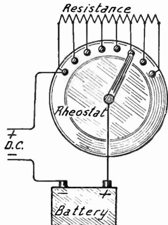
FIG. 2.—Direct Current Battery Charging with Rheostat.
