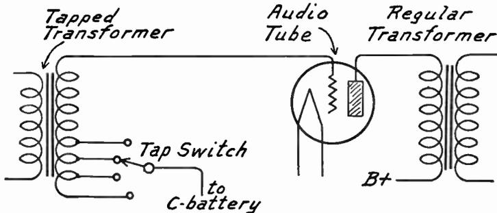
FIG. 5.—Volume Control with Tapped Secondary in Transformer.
