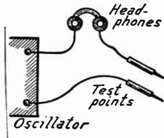
FIG. 4.—Using Audio Oscillator as a Circuit Tester.
