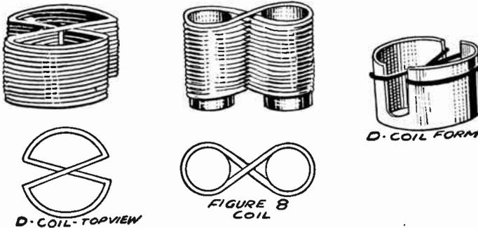
FIG. 2.—Coils of the Closed Field Type.
