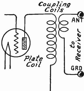
FIG. 6.—Output Coupling Coils for Added Radio Stage.
