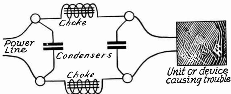
FIG. 7.—Filter Placed between Interfering Device and Power Line.
