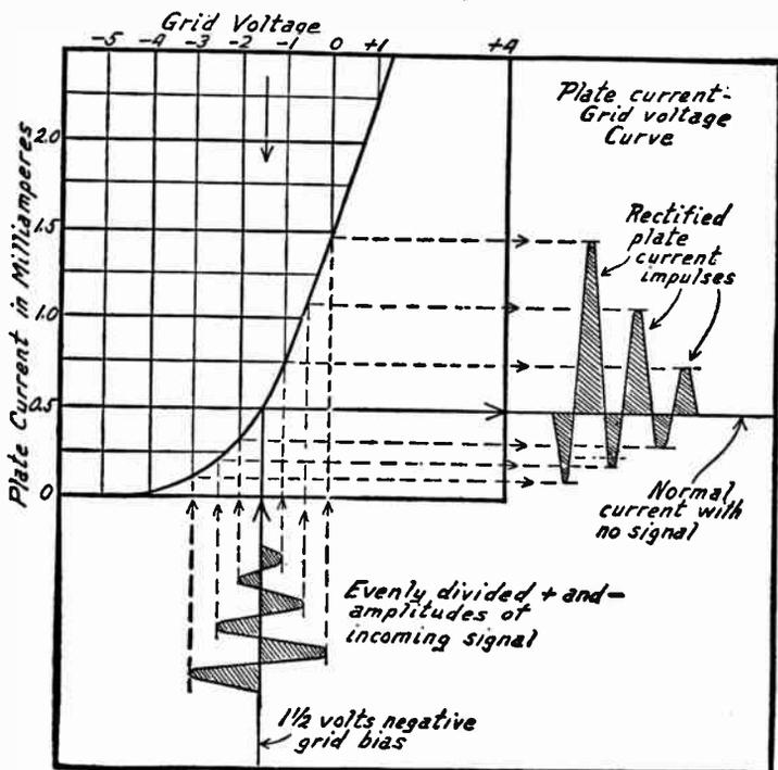
**FIG. 1.**—Action of Detector Using Grid Bias for Plate Current Rectification. one-half milliampere. Assuming that the grid biasing voltage, or the grid's voltage with no signal coming in, is one and one-half volts negative, the steady plate current that flows under this condition is one-half milliampere.
