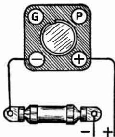
FIG. 1.—Filament Resistor.
