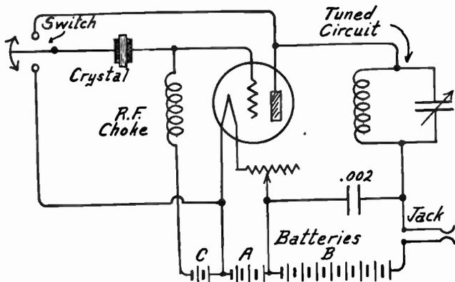
FIG. 3.—Crystal Controlled Oscillator with Tuned Plate Circuit.
