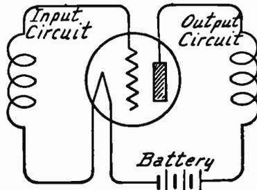
FIG. 3.—Tube Connected to Input and Output Circuits.
