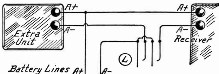
FIG. 31.—Switch for Control of Filament Current in Two Units.
