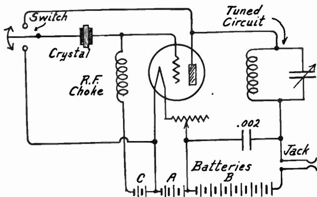
FIG. 3.—Crystal Controlled Oscillator with Tuned Plate Circuit.
