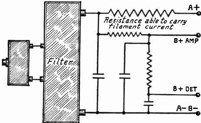
FIG. 3.—Voltage Control for Filament Current in Complete Receiver Supply.
