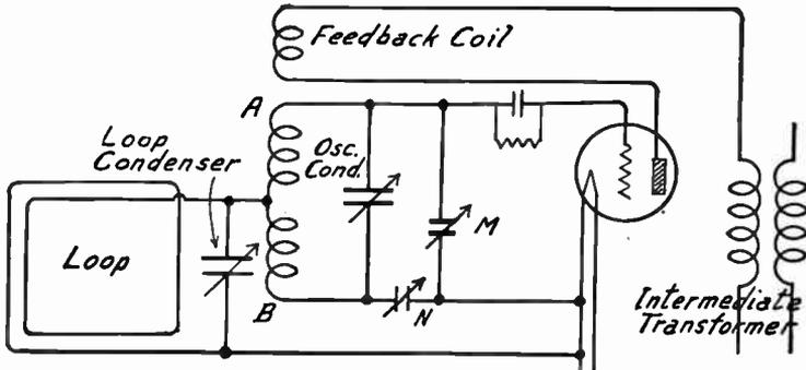
FIG. 8.—Autodyne Combination of Detector and Oscillator Tube.
