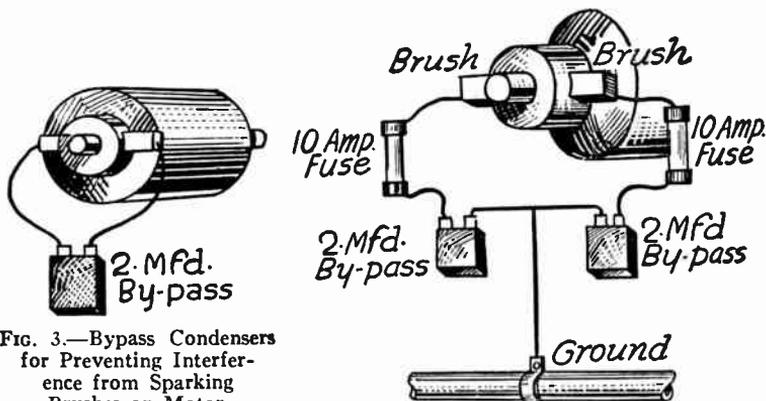
FIG. 3.—Bypass Condensers for Preventing Interference from Sparking Brushes on Motor.
