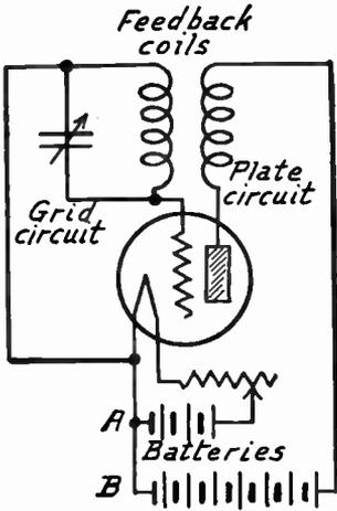
FIG. 3.—Oscillator with Tuned Grid Circuit.
