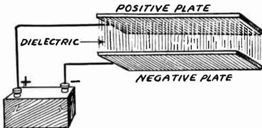
FIG. 2.—The Plates and Dielectric of a Condenser.
