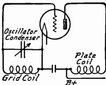
FIG. 2.—Simple Form of Oscillator Used in Superheterodyne.
