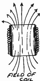
FIG. 1.—Coil Mounting in Weak Field.
