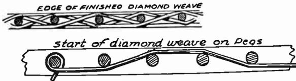
FIG. 2.—Method of Winding Diamond Weave Spiderweb Coil.
