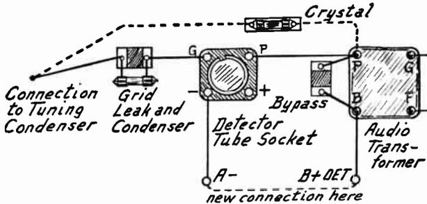
FIG. 6.—Using Crystal in Place of Tube Detector.
