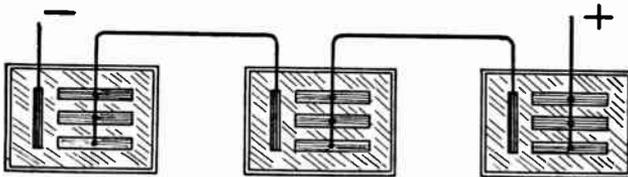
FIG. 4.—Electrolytic Condensers in Series for High Voltages.
