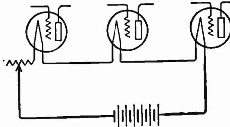
FIG. 2.—Tube Filaments in Series Circuit.
