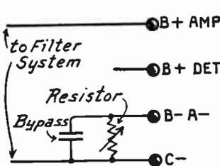
FIG. 10.—Grid Bias from Plate Voltage Supply.
