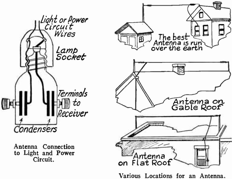
**ANTENNA, LOCATION OF.**—Among the first things to consider about the antenna is location. To begin with it is better to run an antenna out over the earth, with nothing between the wire and the earth except air. An antenna on a roof may be very good but it cannot be as good as one that does not have a building underneath it.
