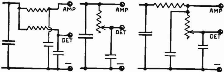
FIG. 1.—Plate Voltage Control Resistors in Series with Receiver Lines.
