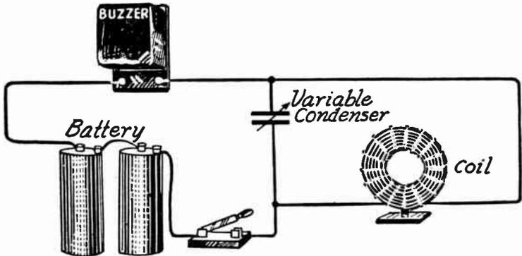
FIG. 2.—Layout of Buzzer Oscillator.
