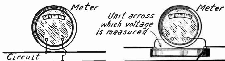
FIG. 2.—Voltmeter Connected Across a Circuit.
