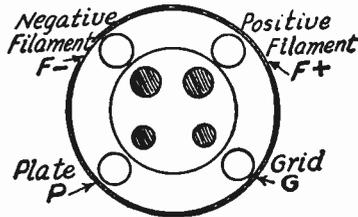
FIG. 4.—Socket for Dry Cell Power Tube.
