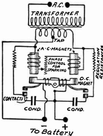
FIG. 1.—A Full-Wave Type of Vibrating Battery Charger.
