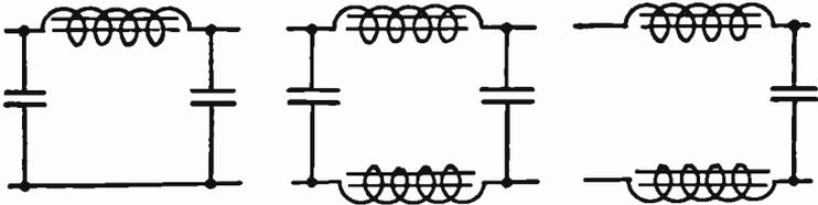
FIG. 11.—Arrangements of Power Unit Filter Condensers and Chokes.
