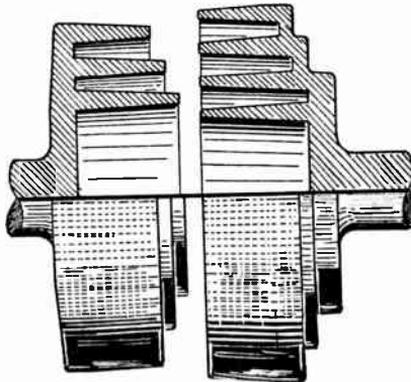
FIG. 6.—Dovetail Type of Variable Condenser.
