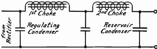
FIG. 9.—Power Unit Filter System with Three Condensers.
