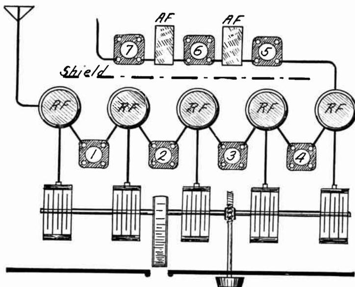
FIG. 7.—Single Control with More Than Three Stages.
