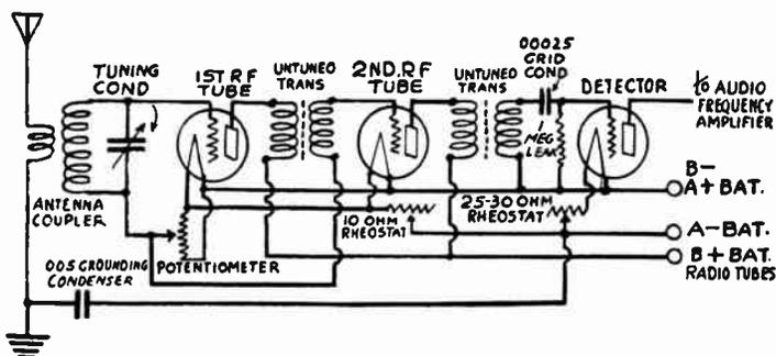
Radio Frequency Amplifier with Untuned Transformers.
