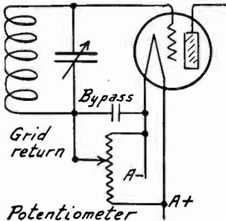
FIG. 4.—Detector Grid Bias with Potentiometer.
