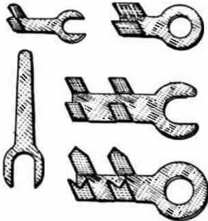
FIG. 5.—Wiring Terminals.
