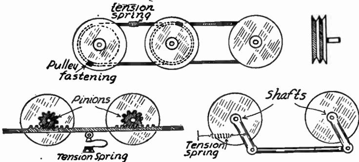
FIG. 3.—Single Control for Side-by-Side Tuning Units.
