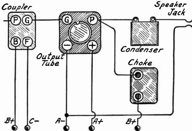
FIG. 4.—Connection of Condenser and Choke for Speaker.
