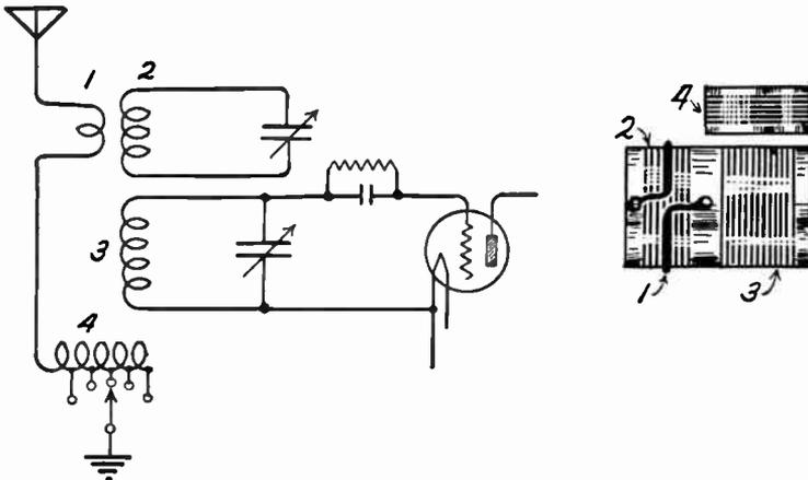
Circuits of Four-Circuit Receiver.
