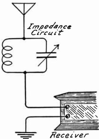
FIG. 1.—Circuit of Impedance Wave Trap.
