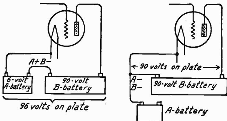
Effect on Plate Voltage of Connecting A+ and B— or of Connecting A— and B—
