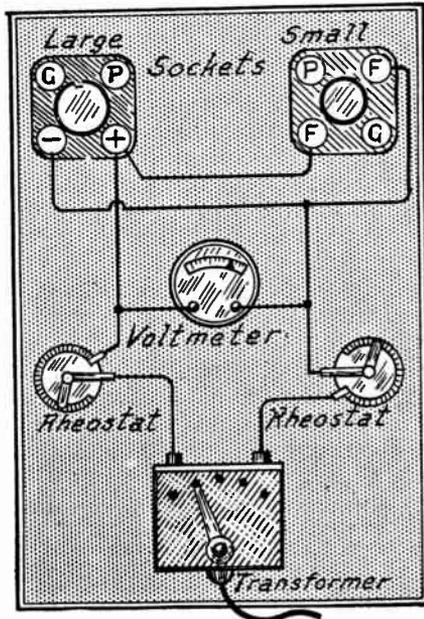
FIG. 1.—Tube Restorer with Transformer.
