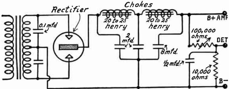
FIG. 6.—Full Wave Rectifier with Two Chokes in Filter.
