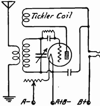
FIG. 3.—One-Tube Receiver with Tickler Coil Regeneration.
