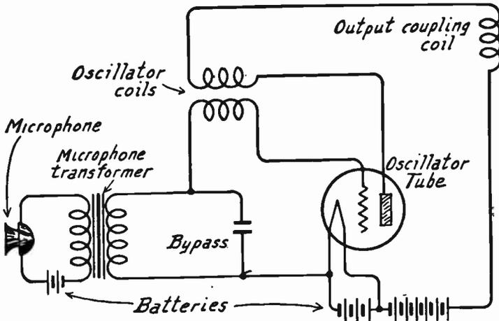
FIG. 1.—Grid Modulation of Oscillator Tube.
