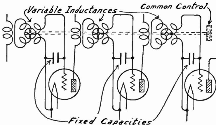
FIG. 2.—Single Control with Variable Inductances or Variometers.
