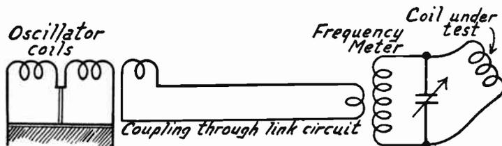
FIG. 5.—Measuring Distributed Capacity of Coil with Radio Oscillator.
