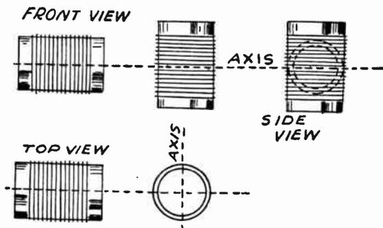
FIG. 2.—Coils Properly Aligned for Minimum Coupling Angle.
