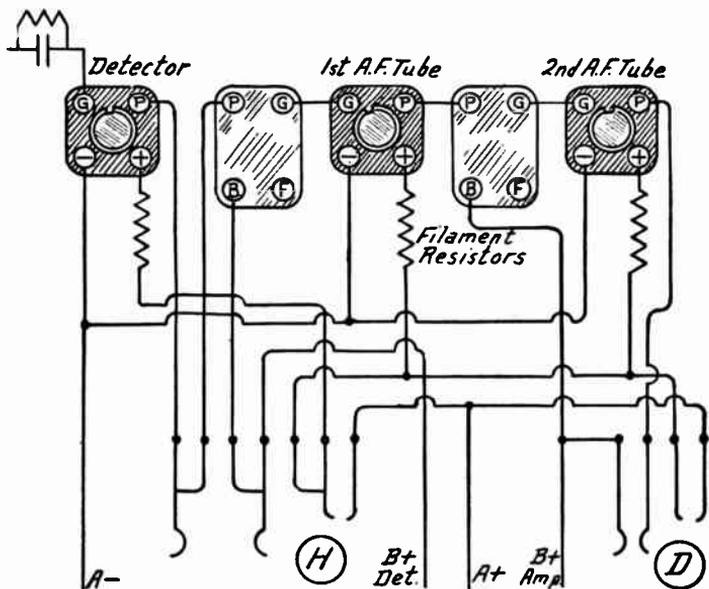
FIG. 9.—Filament Control Jack Following Detector Tube.
