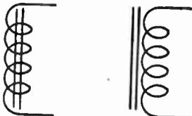
*Coil, iron core or choke*
