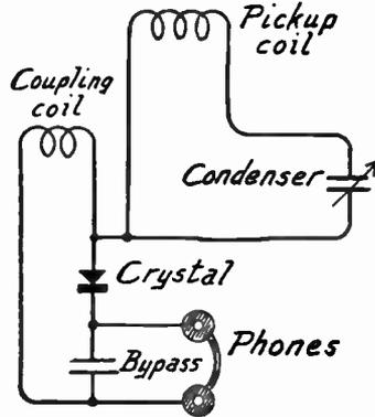
FIG. 8.—Frequency Meter with Special Coupling for Indicator.
