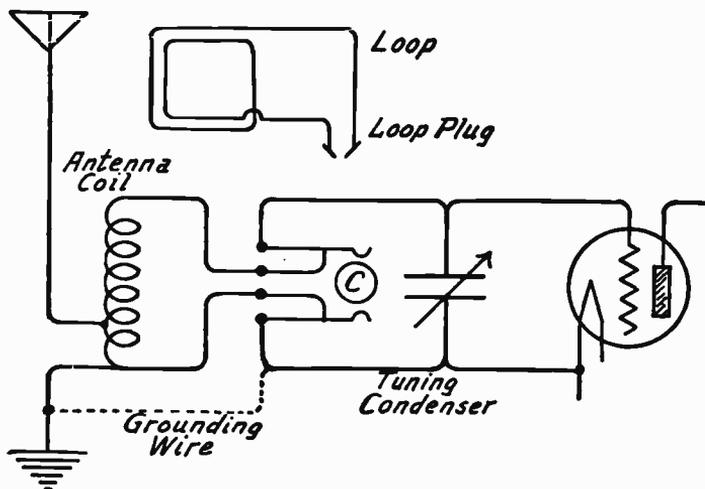
FIG. 26.—Jack for Changing from Antenna to Loop.
