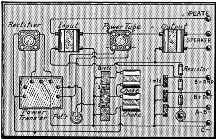
FIG. 2.—Layout for Power Amplifier with Full Wave Rectifier.
