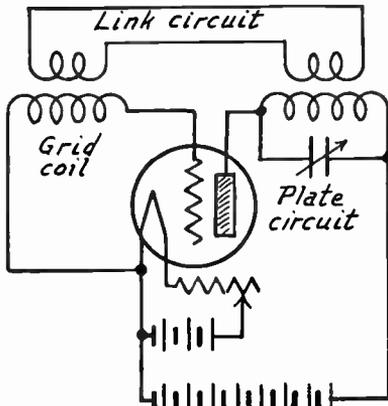
FIG. 6.—Link Circuit Coupling for Oscillator.
