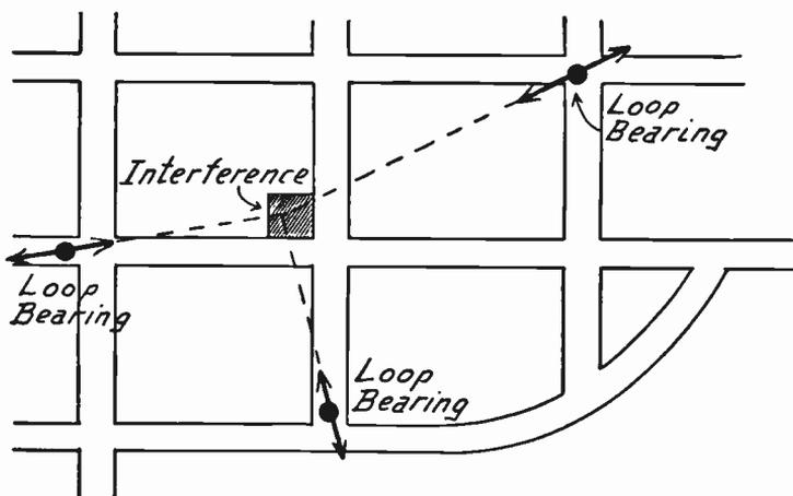
FIG. 2.—Locating Interference with Portable Receiver.
