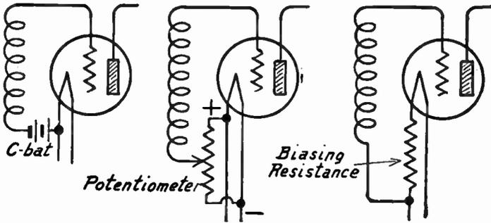
FIG. 2.—Grid Returns to C-Battery and Resistances.
