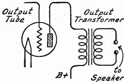
FIG. 7.—Circuits for Output Transformer for Speaker Connection.
