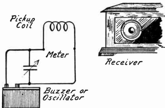
FIG. 2.—Calibrating Receiver with Frequency Meter.
