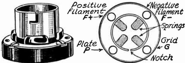
FIG. 1.—Navy Type of Tube Socket.
