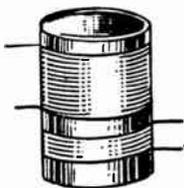
FIG. 5.—Air Core Radio Frequency Transformer.
