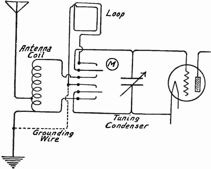
FIG. 27.—Switch for Using Either Antenna or Loop.
