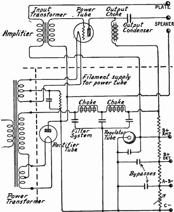
FIG. 3.—Complete Power Amplifier with Half Wave Rectifier.
