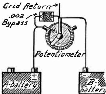
FIG. 7.—Single Biasing Voltage from Potentiometer.
