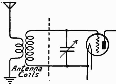
FIG. 2.—Loop Replaced with Antenna Coils.
