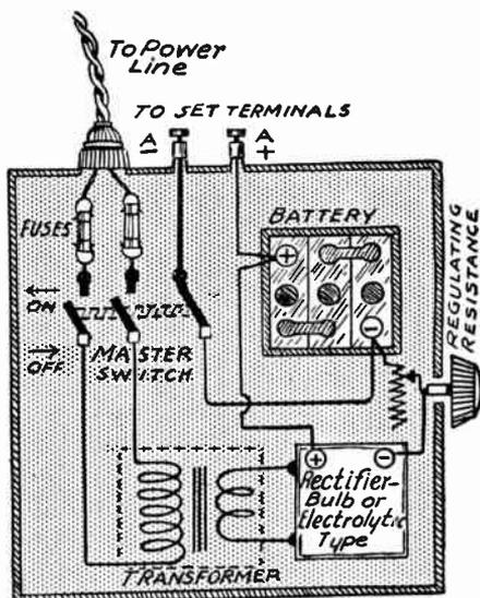
Parts and Circuits of Trickle Charger or an A-Power Unit.
