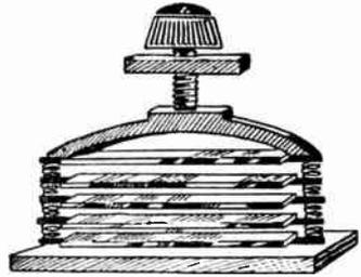
FIG. 3.—Compression Type of Variable Condenser.
