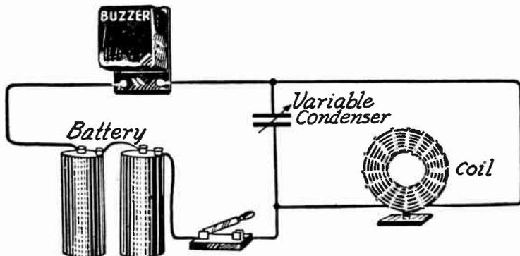
FIG. 2.—Layout of Buzzer Oscillator.
