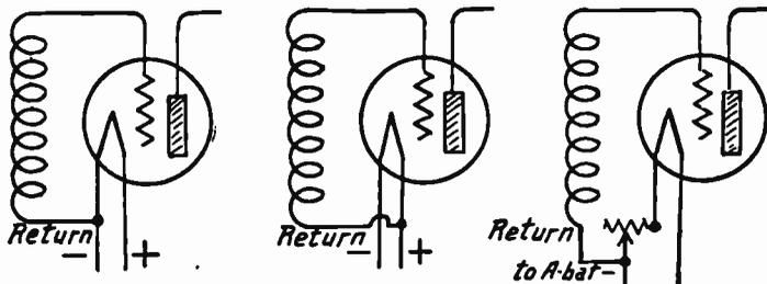
FIG. 1.—Grid Returns to Filament or Battery Lines.
