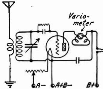
FIG. 4.—One-Tube Receiver with Variometer Regeneration.
