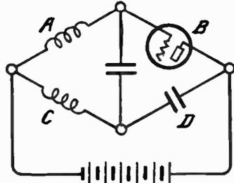
FIG. 11.—The Rice Balanced Circuit in Bridge Form.
