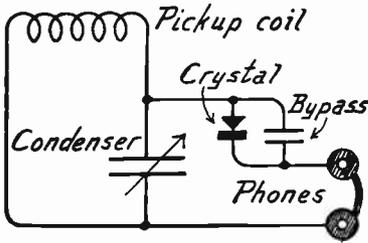
FIG. 5.—Frequency Meter with Direct Coupled Indicator Circuit.
