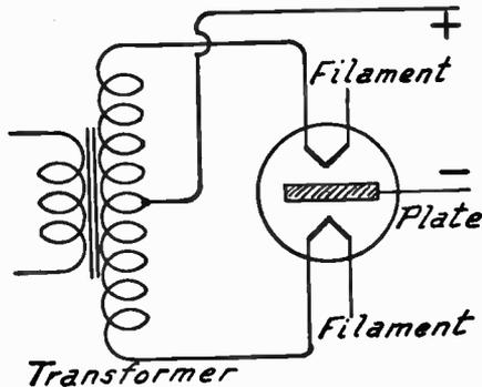
FIG. 2.—Connections of Full-Wave Rectifying Tube.
