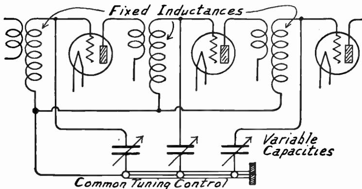
FIG. 1.—Single Control with Variable Condensers.
