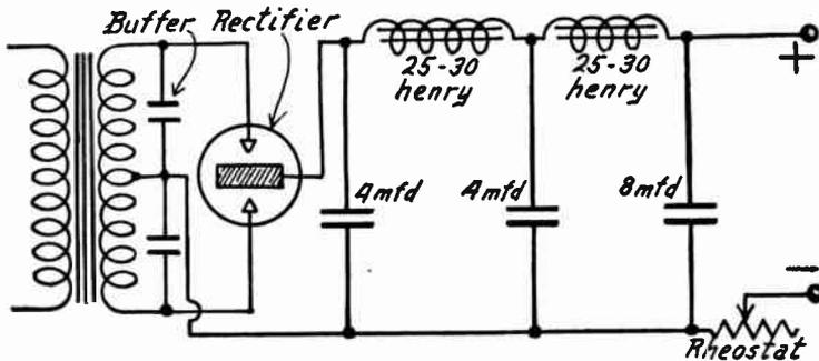
FIG. 5.—Full Wave Rectifying Tube for Filament Supply.
