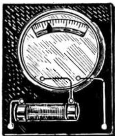
FIG. 5.—Milliammeter Used as Voltmeter.
