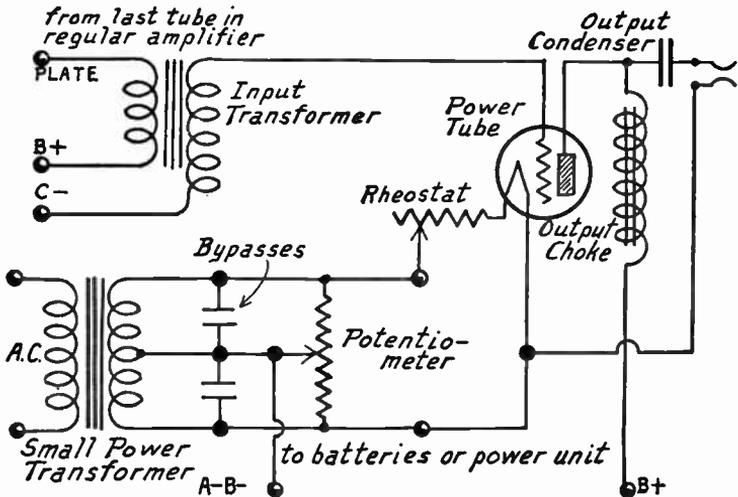
FIG. 7.—Power Tube Filament Supply from Tapped Transformer.
