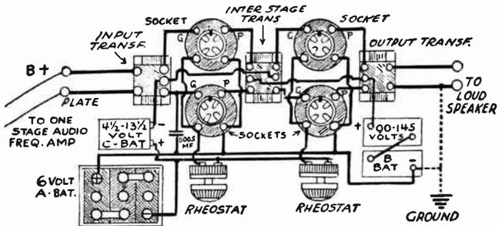
FIG. 3.—Two Stages of Push-Pull Amplification.
