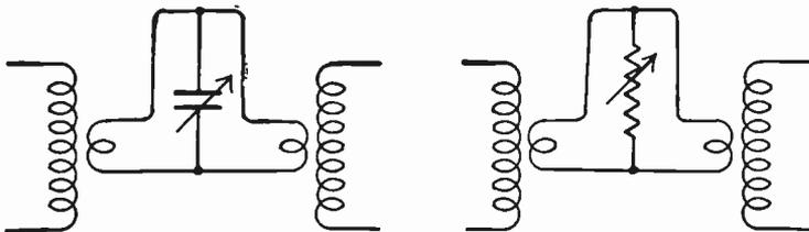
FIG. 3.—Variable Units in Shunt with Link Circuits.
