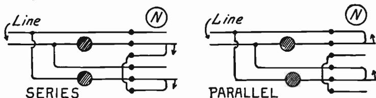
FIG. 30.—Double-Pole, Double-Throw Switch for Series-Parallel Work.
