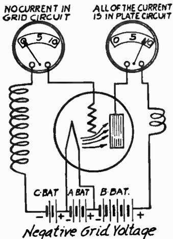
FIG. 4.—Electron Flow with Negative Grid Bias Voltage.
