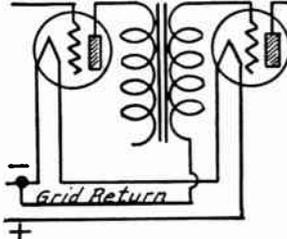
FIG. 3.—Grid Return to Filament of Preceding Tube.
