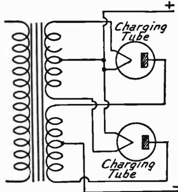
FIG. 6.—Charging Tubes Used as Filament Supply Rectifier.
