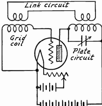
FIG. 6.—Link Circuit Coupling for Oscillator.
