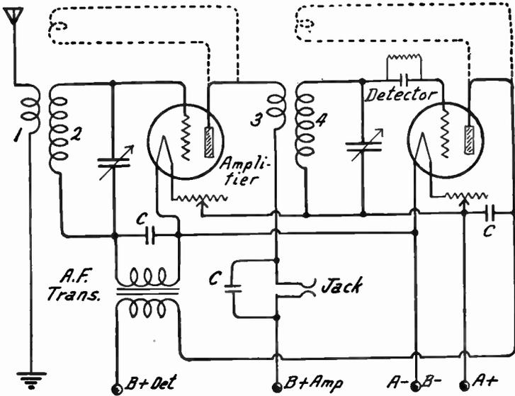
FIG. 4.—Reflex Receiver with Tube Detector.
