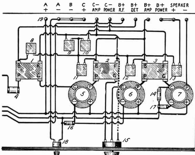
AUDIO AMPLIFIER WITH TWO TRANSFORMER STAGES AND POTENTIOMETER CONTROL
