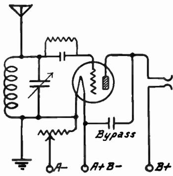
FIG. 4.—Single Circuit Receiver with Negative Grid Return for Soft Detector Tube.
