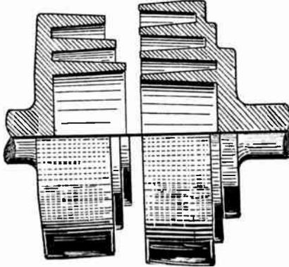
FIG. 6.—Dovetail Type of Variable Condenser.
