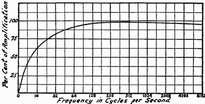
FIG. 2.—Amplification Curve for a Good Audio Transformer.
