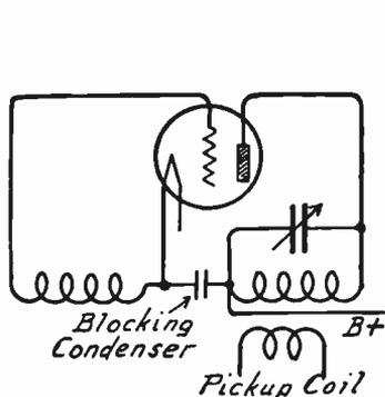
FIG. 6.—Oscillator with Tuned Plate Circuit in Superheterodyne.
