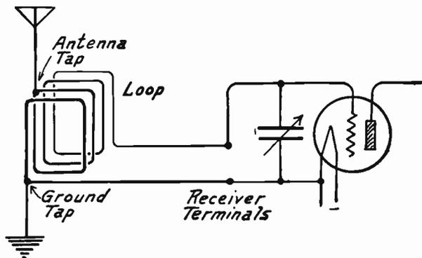
FIG. 1.—Using Antenna and Ground with a Loop.
