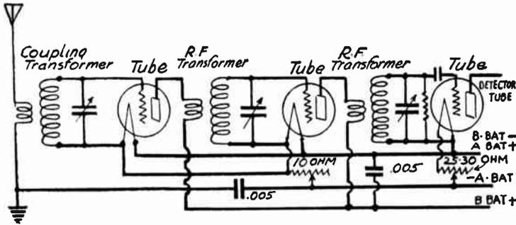
FIG. 7.—Circuits of Two-Stage Tuned Transformer Radio Amplifier.
