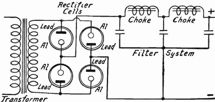
FIG. 4.—Power Unit with Electrolytic Rectifier.
