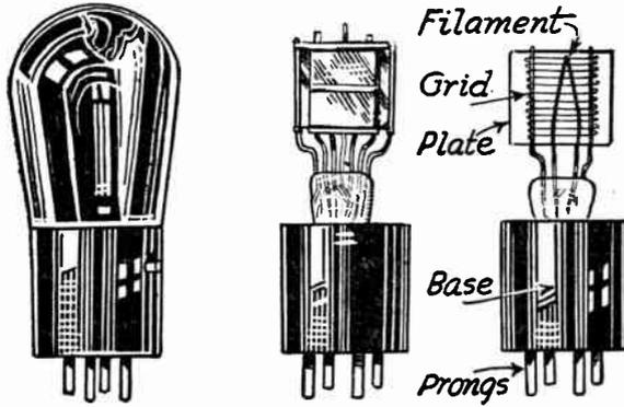
FIG. 1.—A Vacuum Tube and Its Principal Parts.
