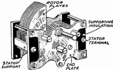
FIG. 3.—Terminal Positions Considered in Condenser Design.
