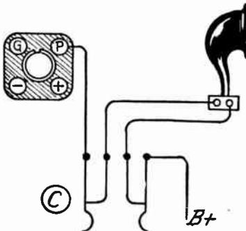
FIG. 21.—Jack for Completely Disconnecting Speaker.
