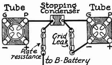
FIG. 1.—Arrangement of Parts for Resistance Coupled Amplifier.
