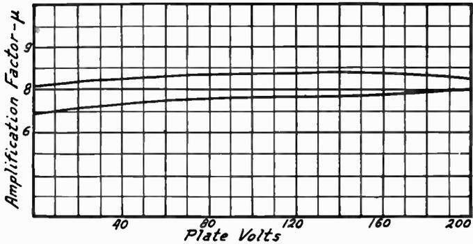
FIG. 16.—Effect of Plate Voltage on Amplification Factor.
