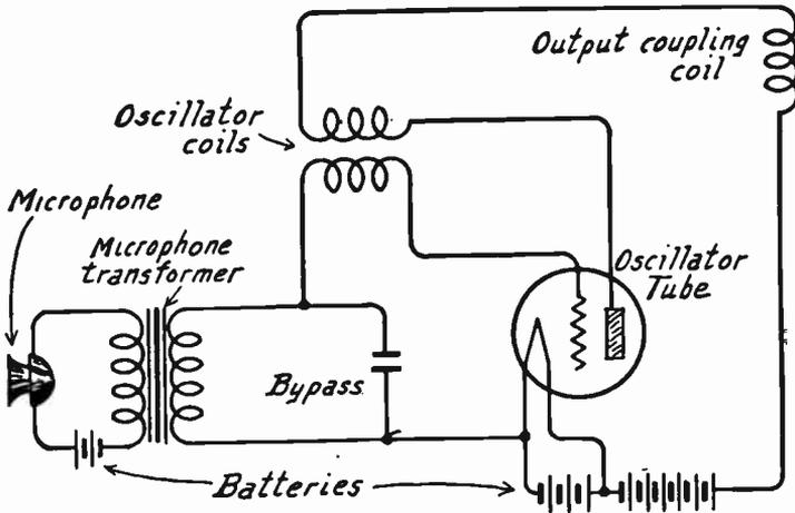
FIG. 1.—Grid Modulation of Oscillator Tube.
