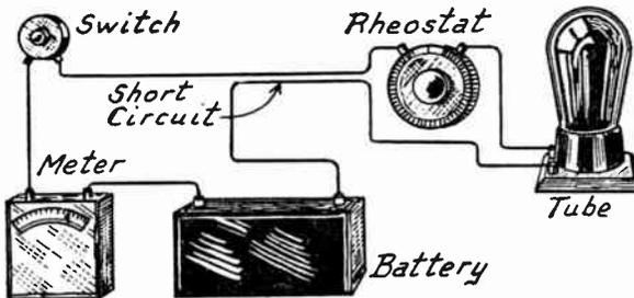
FIG. 2.—Testing for Short Circuit with Voltmeter.
