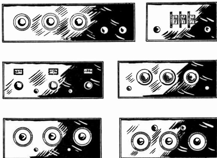
FIG. 11.—Panels with Three Tuning Controls.
