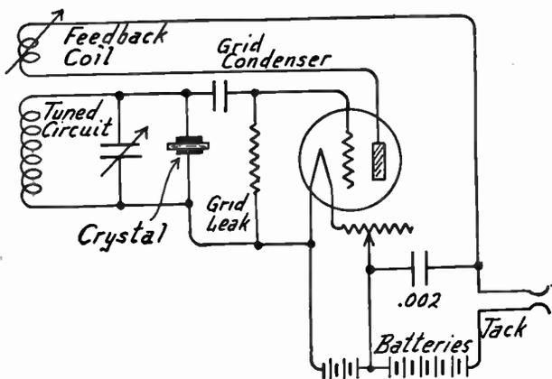
FIG. 4.—Crystal Controlled Oscillator with Tuned Grid Circuit.
