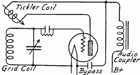
FIG. 1.—Regeneration Obtained with Movable Tickler Coil.
