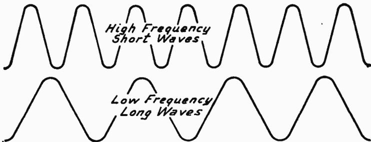
FIG. 2.—Frequency Relation to Wavelength.
