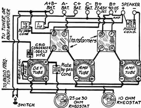
FIG. 9.—Layout of Two-Stage Transformer Coupled Audio Amplifier.
