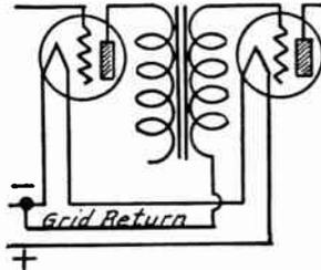
FIG. 3.—Grid Return to Filament of Preceding Tube.
