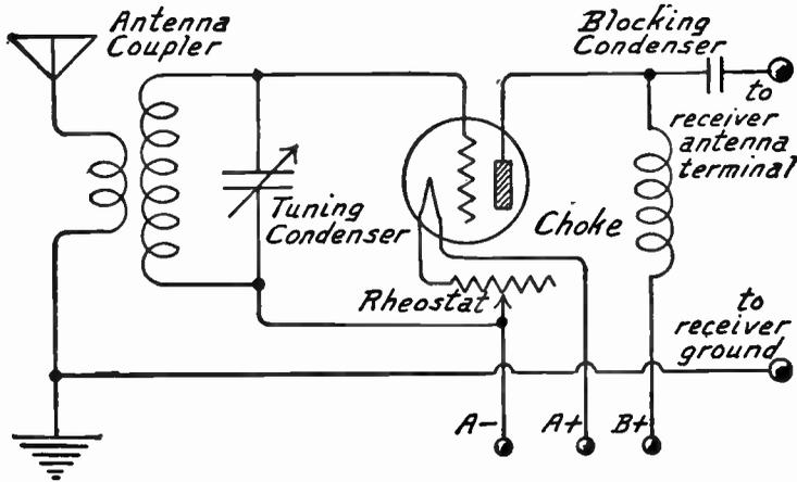
FIG. 3.—Circuit of Added Radio Stage Without Balancing.
