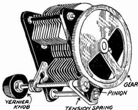
FIG. 3.—Geared Vernier for Tuning Condenser.
