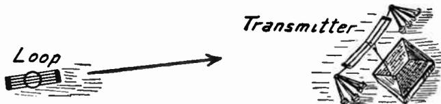
FIG. 1.—Loop Pointed at Most Favorable Direction Toward Transmitter.
