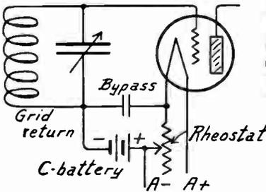
FIG. 6.—Detector Grid Bias with C-battery and Rheostat.
