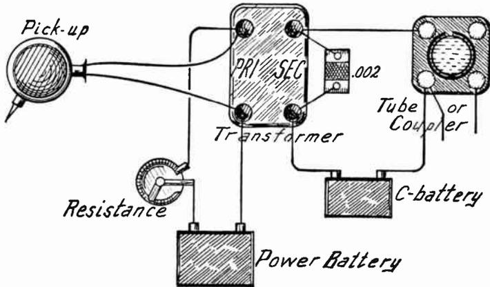
FIG. 6.—Using a Battery with Phonograph Pick-up Unit.
