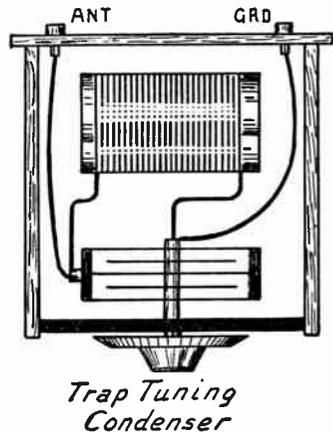
FIG. 2.—Layout of Impedance Wave Trap Unit.
