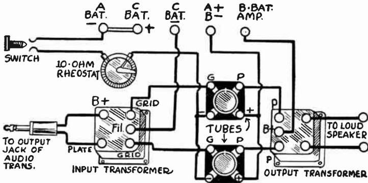
FIG. 2.—Layout for Single Stage of Push-Pull Amplification.
