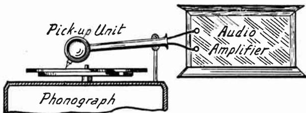
FIG. 2.—Phonograph Pick-up Unit Connected to an Amplifier.
