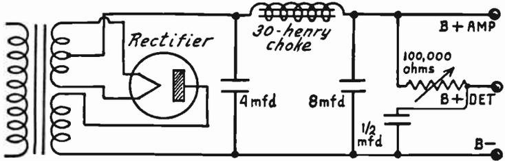
FIG. 5.—Half Wave Rectifier with Single Choke in Filter for Plate Voltage Supply.
