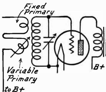
FIG. 12.—Regeneration Control with Variable Split Primary Winding.
