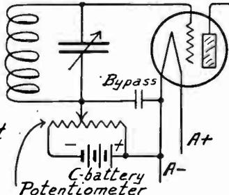
FIG. 7.—Detector Grid Bias with C-battery and Potentiometer.
