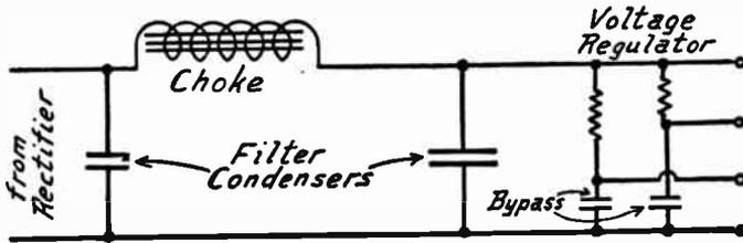
FIG. 10.—Power Unit Filter System with Single Choke.
