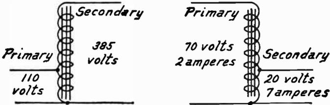
FIG. 2.—Voltage Ratios of Auto-Transformers.
