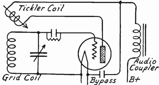
FIG. 1.—Regeneration Obtained with Movable Tickler Coil.
