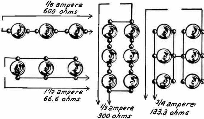
FIG. 3.—Lamp Bank Resistances for Voltage Reduction in Power Units.
