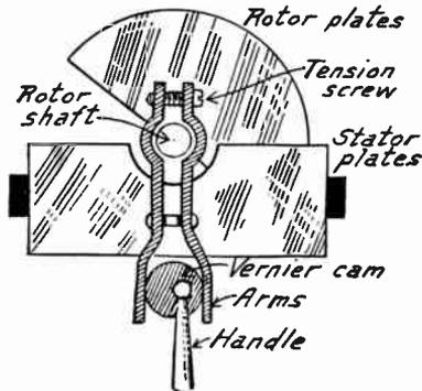
FIG. 2.—Cam Vernier for Moving Condenser Rotor Plates.
