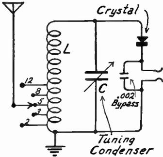
FIG. 1.—Simplest Type of Crystal Receiver.
