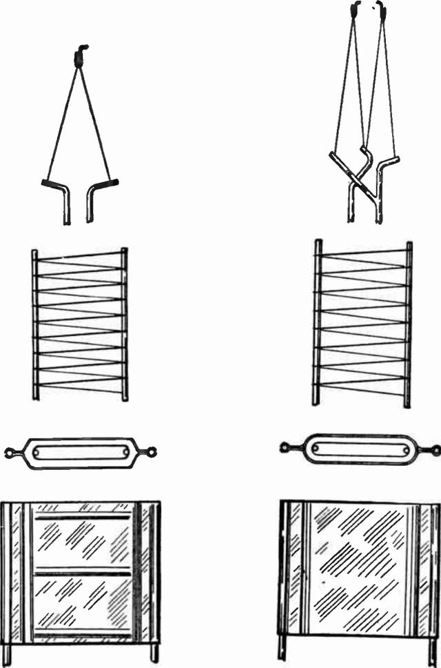
FIG. 4.—Design of a Semi-Power Tube.
