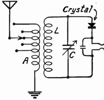
FIG. 2.—Crystal Receiver with Loose Coupled Antenna Circuit.
