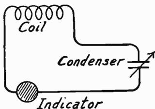
FIG. 1.—The Simplest Frequency Meter Circuit.
