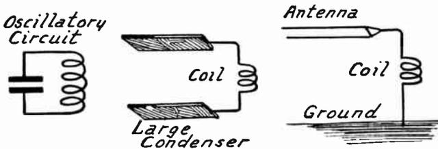
FIG. 5.—Oscillatory Circuit Formed by Antenna and Ground.
