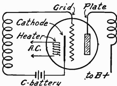
FIG. 1.—Circuits of Alternating Current Tube.
