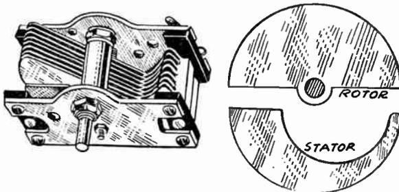
FIG. 4.—Stator Plates Shaped for Straight Line Frequency Condenser.
