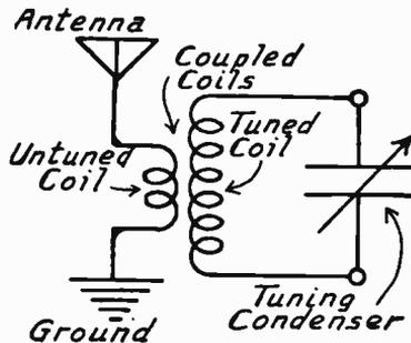
FIG. 11.—Tuned Circuit Coupled to Antenna Circuit.
