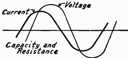
FIG. 2.—Current Leading Voltage.
