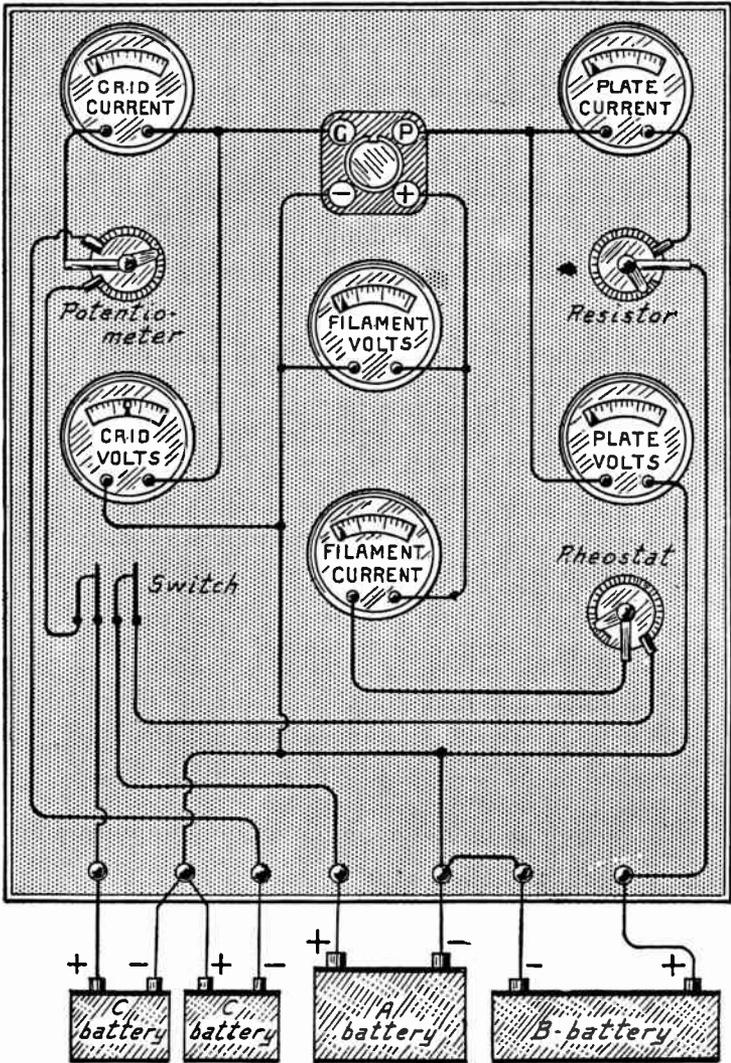
FIG. 5.—Tube Tester with Meters for All Readings.
