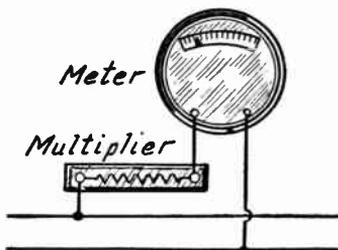
FIG. 3.—Multiplier Used with Voltmeter.
