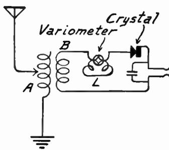
FIG. 4.—Variometer for Tuning Crystal Circuit.
