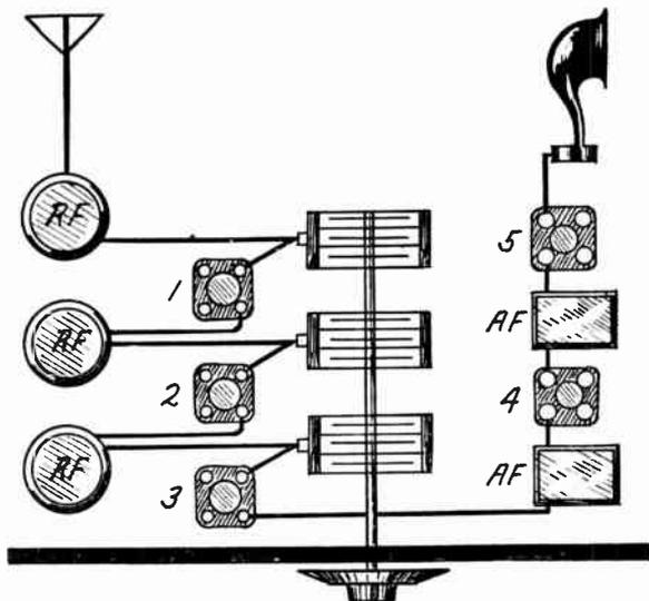
FIG. 6.—Three Tuned Stages on One Control Shaft.
