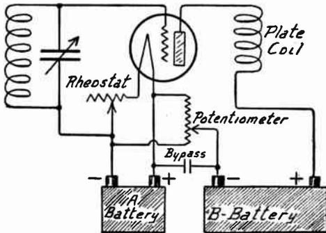
FIG. 8.—Detector Grid Bias with Potentiometer on B-Battery.
