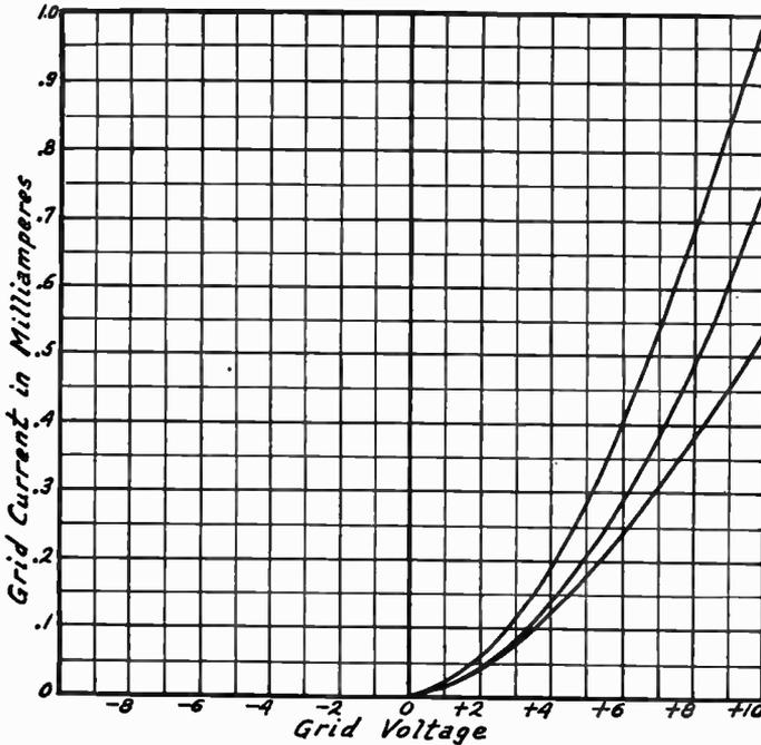
FIG. 10.—Grid Voltage Effect on Grid Current.
