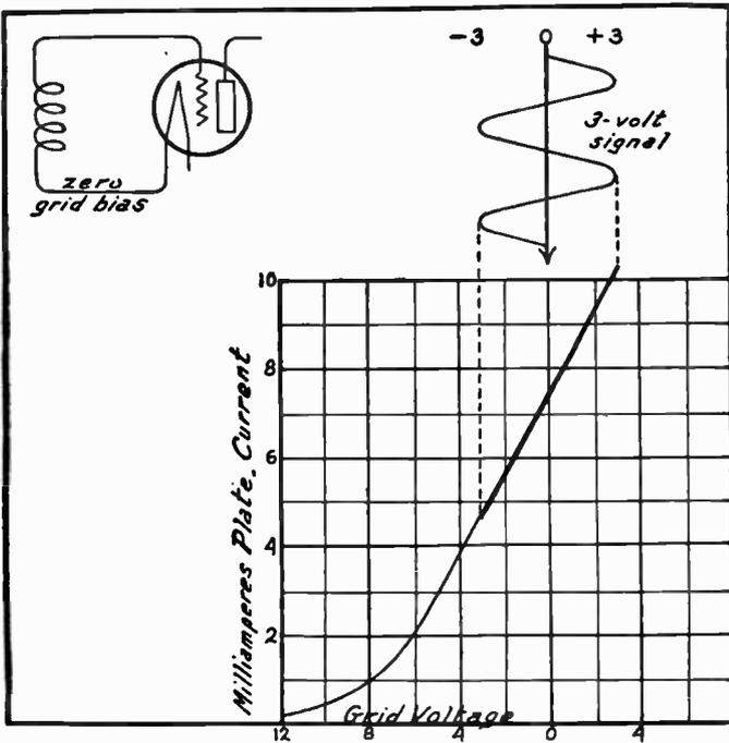
FIG. 1.—Effect of Zero Grid Bias, Distortion.
