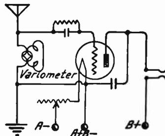
FIG. 2.—One-Tube Variometer Tuned Receiver.
