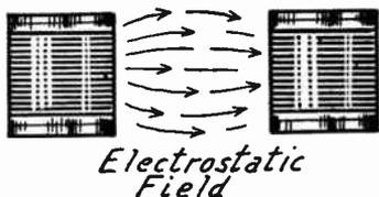
FIG. 10.—Capacity Effect between Coils Which Causes Oscillation.
