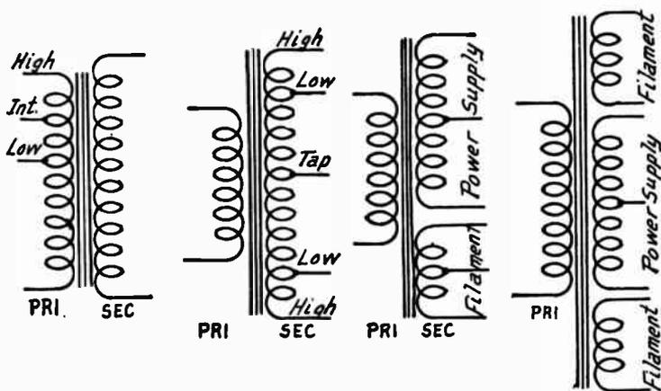
FIG. 2.—Types of Tapped Transformers for Power Units.
