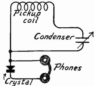
FIG. 6.—Frequency Meter Indicator Coupled through Single Wire.
