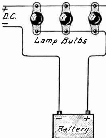
FIG. 1.—Direct Current Battery Charging with Lamp Resistance.
