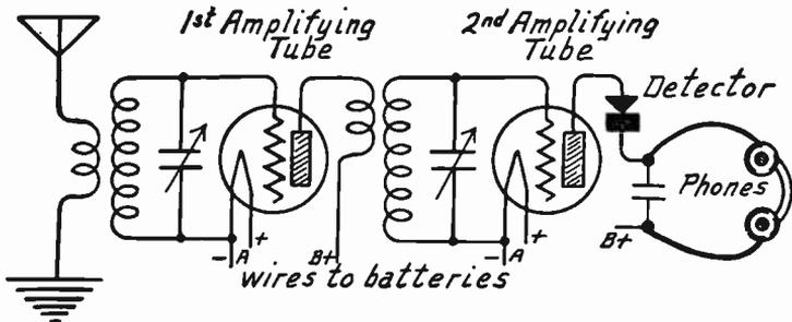
FIG. 18.—Two Stages of Amplification Before the Detector.
