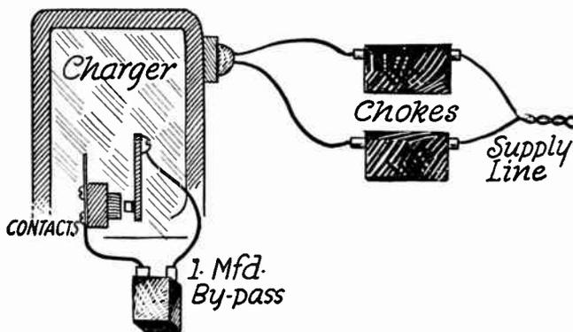
FIG. 5.—Handling Interference of Vibrators and Flashers.
