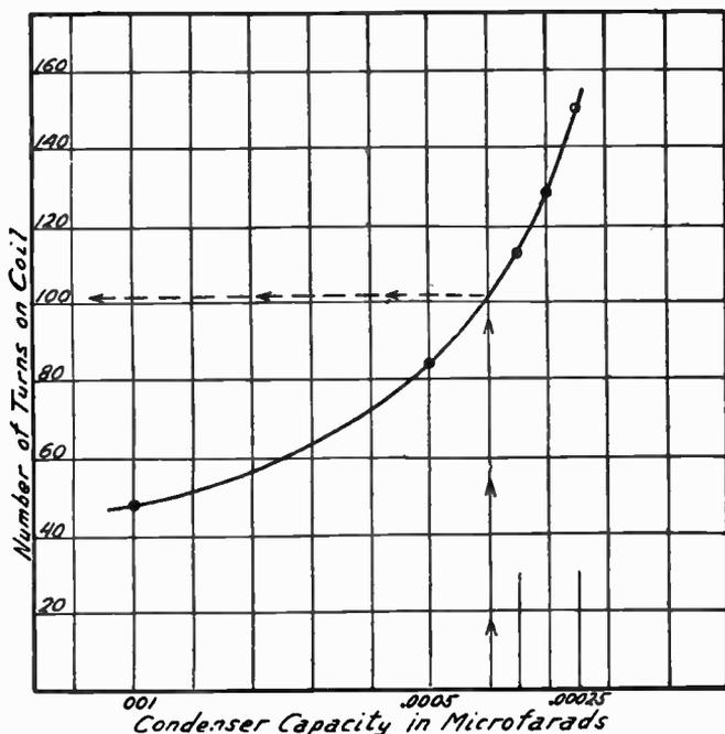
FIG. 5.—Graph Showing Condenser Capacity and Number of Turns.
