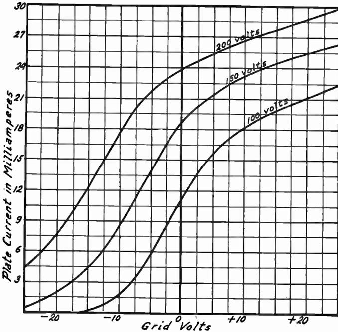
FIG. 5.—Effect of Grid Voltage on Plate Current.
