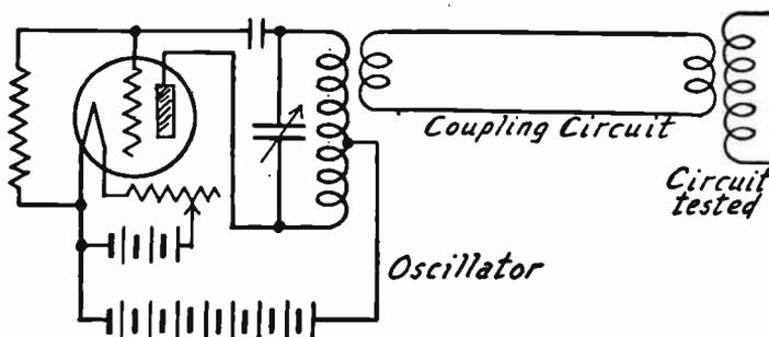
FIG. 3.—Link Circuit for Radio Oscillator Coupling.
