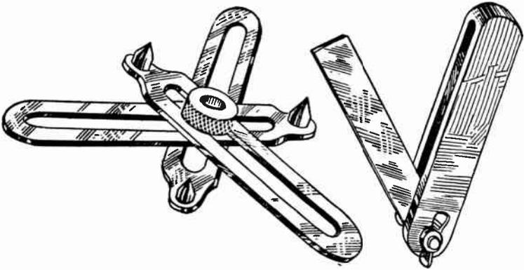
FIG. 1.—Adjustable Template and Adjustable Square.
