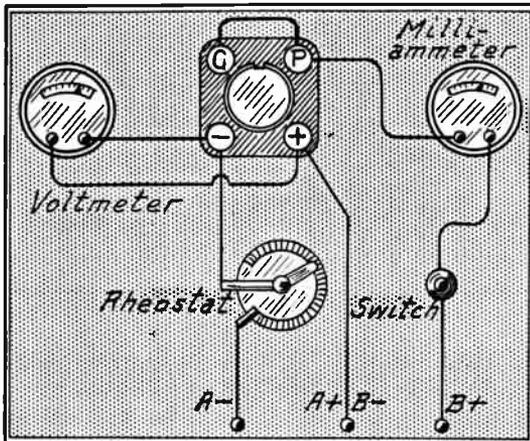
FIG. 2.—Filament Emission Tester Used in Tube Restoration.
