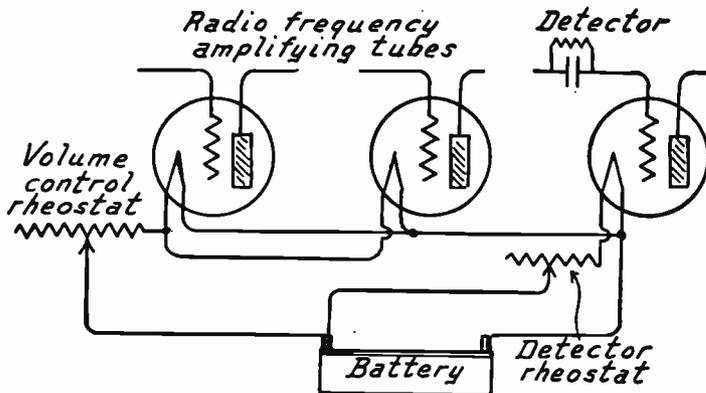
FIG. 1.—Volume Control with Radio Frequency Rheostat.
