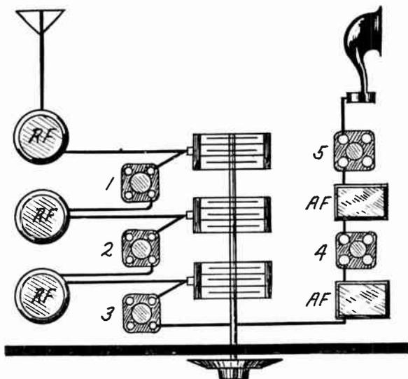
FIG. 6.—Three Tuned Stages on One Control Shaft.
