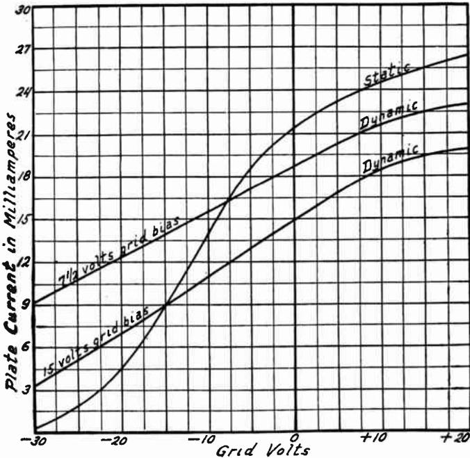
FIG. 6.—Grid-Voltage, Plate Current Curves Compared for Static and for Dynamic or Working Conditions.
