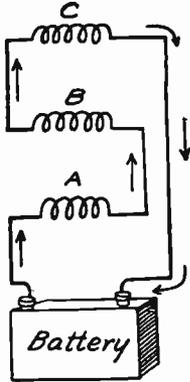
FIG. 1.—A Series Circuit.
