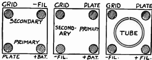
FIG. 3.—Similarity of Amplifier Transformer and Tube Terminals.
