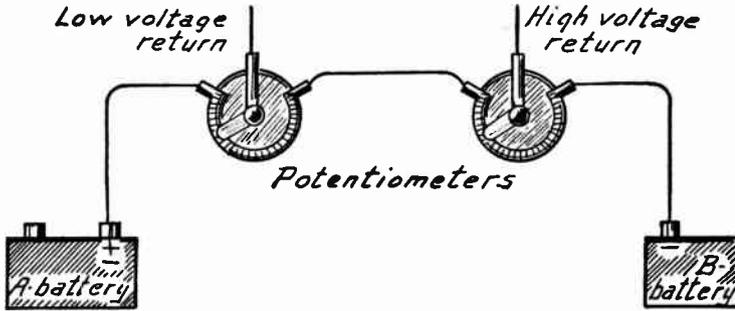
FIG. 9.—Two Variable Biases from Potentiometers.
