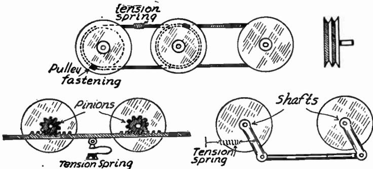
FIG. 3.—Single Control for Side-by-Side Tuning Units.
