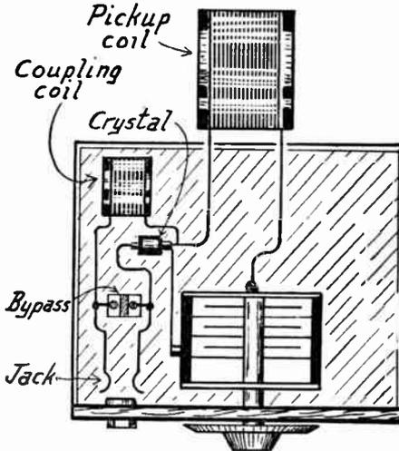
FIG. 9.—Layout for Frequency Meter with Special Indicator Coupling.
