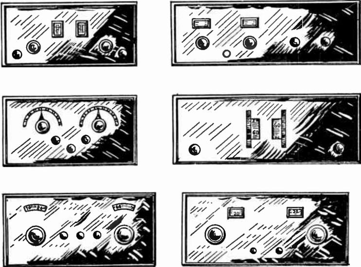
FIG. 9.—Panel Arrangements for Two Tuning Controls.
