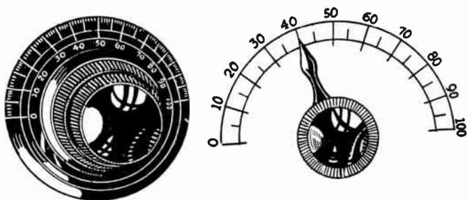
FIG. 1.—Graduations on Tuning Dial and on Panel.
