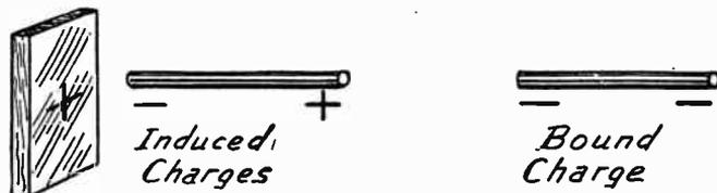
Charges Produced by Electrostatic Induction.
