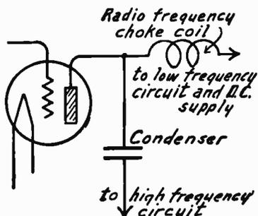
FIG. 1.—Separation of Frequencies with a Choke Coil.
