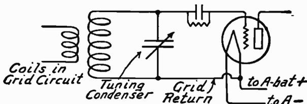
FIG. 2.—Positive Grid Return for Hard Tube as Detector.
