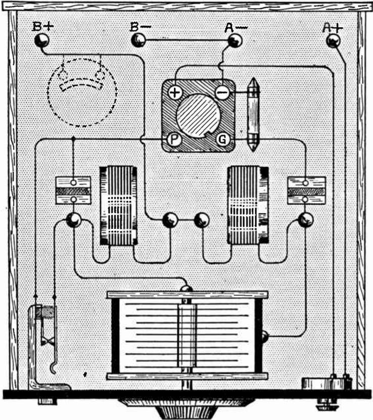
FIG. 5.—Layout and Plan of Radio Frequency Oscillator.
