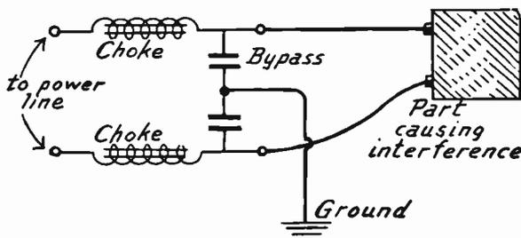
FIG. 8.—Interference Filter with Grounded Center Tap.
