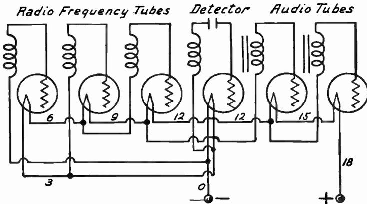
FIG. 11.—Biasing for Six Tube Receiver with Three-Volt Tubes Using Filament Power Unit.
