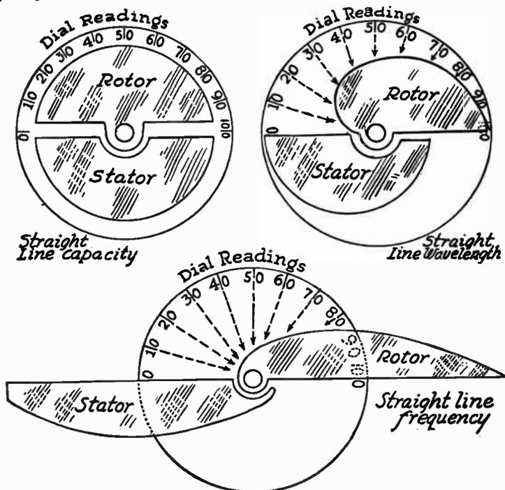
FIG. 1.—Plate Forms of the Different Straight Line Condensers.
