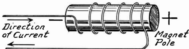
FIG. 3.—Current Flow Around an Electromagnet.
