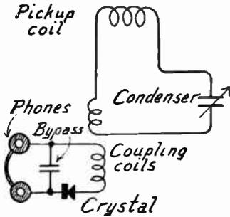
FIG. 7.—Inductively Coupled Indicator Circuit for Frequency Meter.
