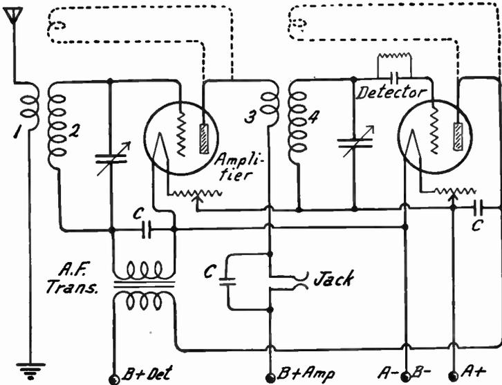
FIG. 4.—Reflex Receiver with Tube Detector.
