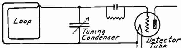
FIG. 1.—Tuned Loop Connected to a Detector as Used in a Superheterodyne Receiver.
