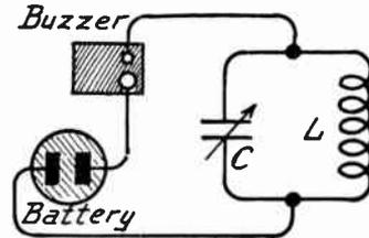
FIG. 2.—Buzzer Excited Oscillator Circuit.
