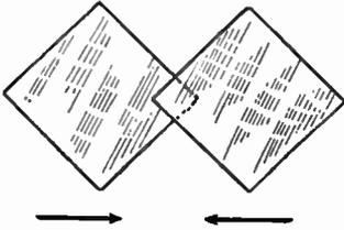
FIG. 3.—Square Plates for Straight Line Wavelength Condenser.
