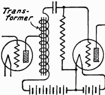
FIG. 3.—Auto-Transformer Interstage Coupling.
