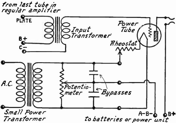
FIG. 6.—Power Tube Filament Current from Untapped Transformer.
