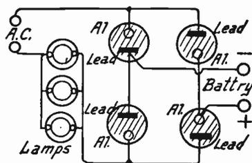
FIG. 3.—Lamp Resistance with Electrolytic Battery Charging Rectifier.
