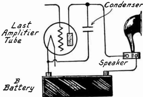
FIG. 1.—Loud Speaker Connected Directly to Last Tube.
