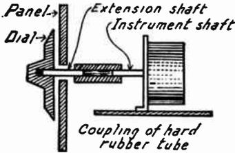
Extension Shaft for Avoiding Body Capacity Effect.
