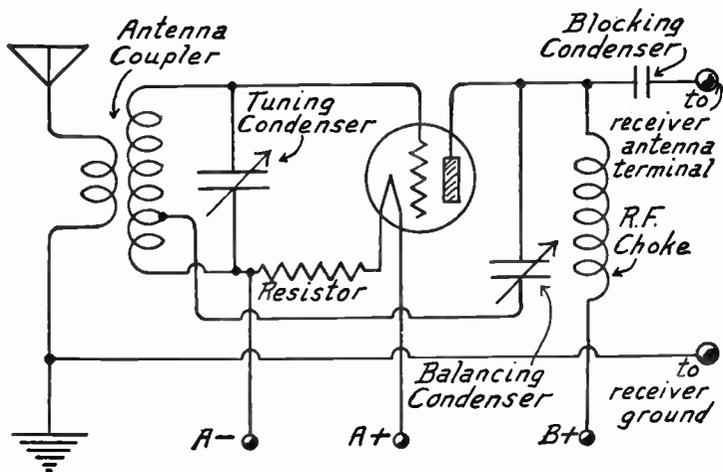
FIG. 1.—Circuit of Added Radio Stage with Balanced Control of Oscillation.
