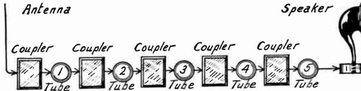
FIG. 1.—Process of Amplification Considered in Receiver Construction.
