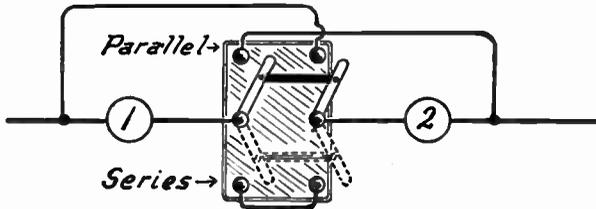
FIG. 2.—Double-Pole, Double Throw Switch with Series-Parallel Connections.
