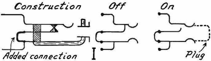
FIG. 4.—Jack Remodeled for Closed Circuit Work.
