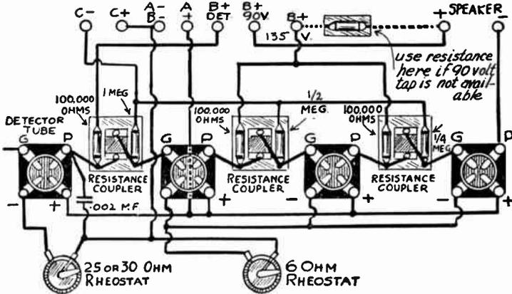
FIG. 3.—Arrangement of Parts in Three-Stage Resistance Amplifier.
