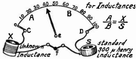
FIG. 7.—Inductance Measurement with Bridge.
