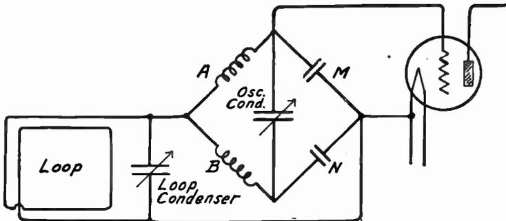
FIG. 9.—Bridge Circuit Equivalent of Autodyne Circuit.
