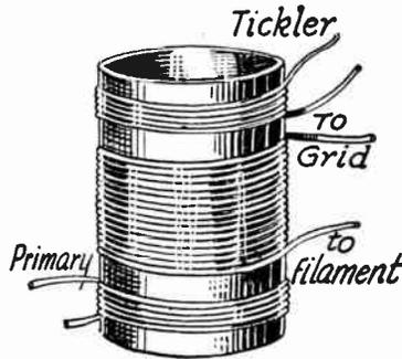
FIG. 5.—Construction of Fixed Ticker Coil for Regeneration.
