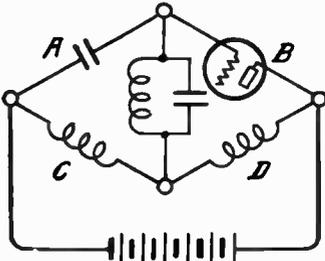
FIG. 10.—The Neurodyne Balanced Circuit in Bridge Form.
