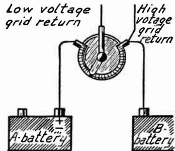
FIG. 8.—Two Biasing Voltages from Potentiometer.
