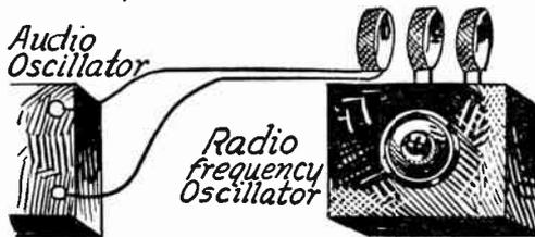
FIG. 6.—Modulating Radio Frequency Oscillator with Audio Oscillator.
