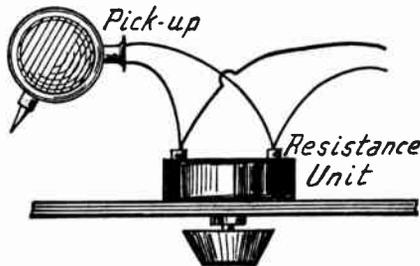
FIG. 5.—Resistance Control of Volume in Phonograph Amplifier.
