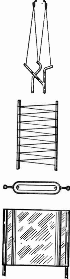
FIG. 5.—Design of a Half-Ampere Power Tube.
