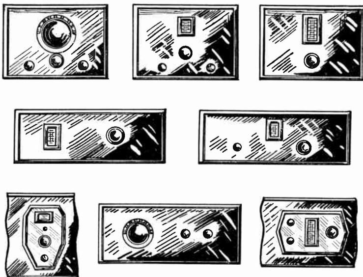
FIG. 8.—Panel Layouts for Single Control Receivers.
