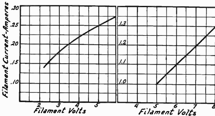
FIG. 1.—Effect of Filament Voltage on Filament Current.
