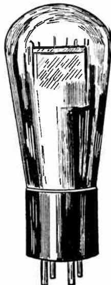
FIG. 4.—Large Type of Power Amplifier Tube.
