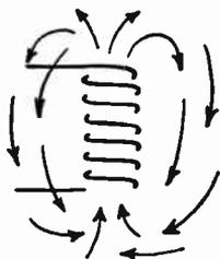
FIG. 7.—Electromagnetic Lines of Force Around a Coil.
