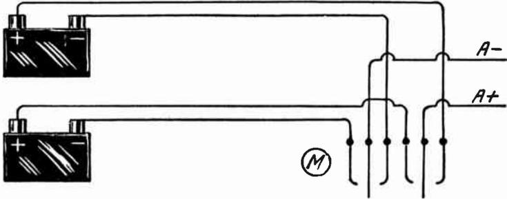
FIG. 32.—Switch for Using Either of Two Power Units.
