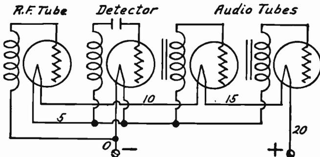
FIG. 9.—Grid Biasing with Five-Volt Tubes in Series.
