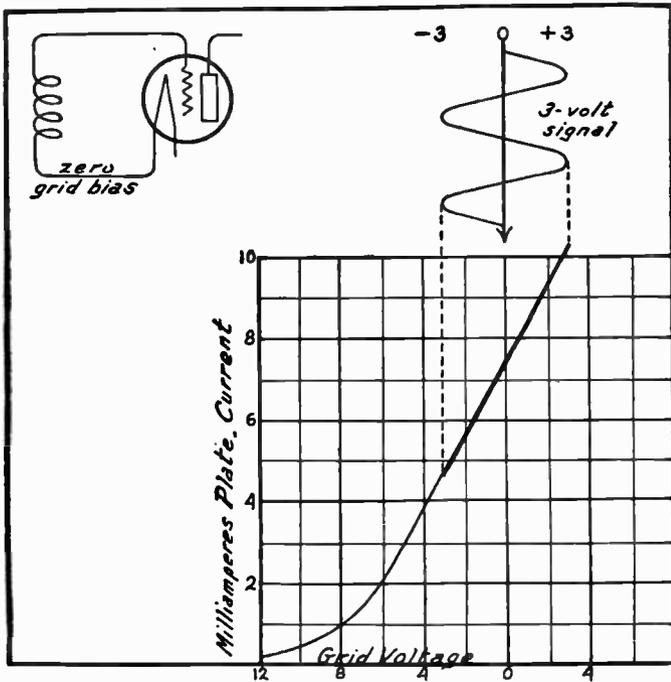
FIG. 1.—Effect of Zero Grid Bias, Distortion.
