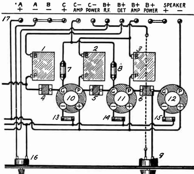
AUDIO AMPLIFIER WITH THREE-STAGE CHOKE COUPLING
