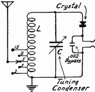
FIG. 1.—Simplest Type of Crystal Receiver.
