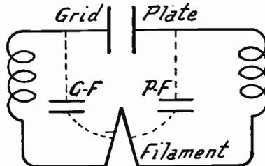
FIG. 5.—Internal Capacities in Parallel with External Circuits.
