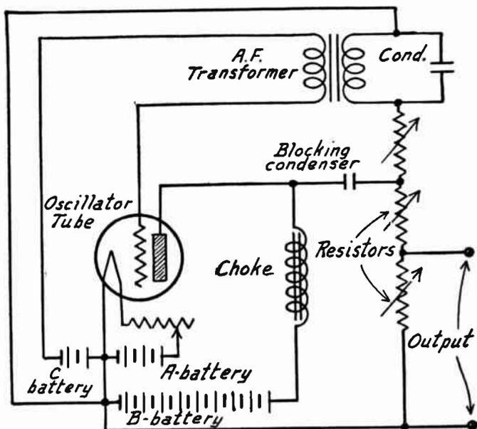
FIG. 2.—Circuits of Practical Audio Oscillator.
