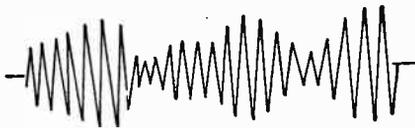
FIG. 3.—Carrier Modulated with Sound Frequency.
