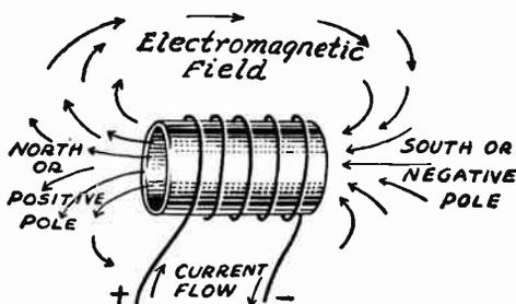
FIG. 2.—Electromagnetic Field around a Solenoid or Coil.
