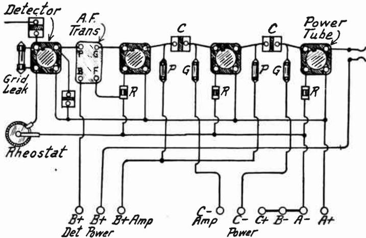
FIG. 6.—Layout of Amplifier with Two Resistance Stages and One Transformer Stage.
