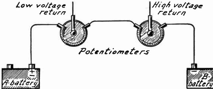
FIG. 9.—Two Variable Biases from Potentiometers.
