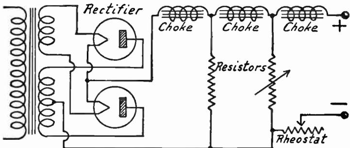
FIG. 4.—Filament Supply with Resistors in Filter System.
