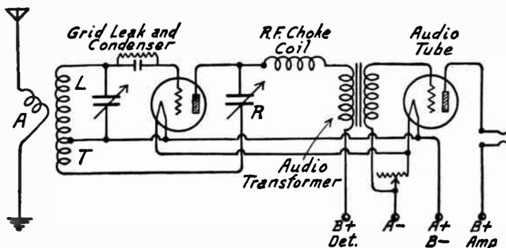
FIG. 1.—Short Wave Receiver.
