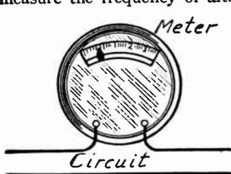
FIG. 1.—Ammeter in Series with Circuit.
