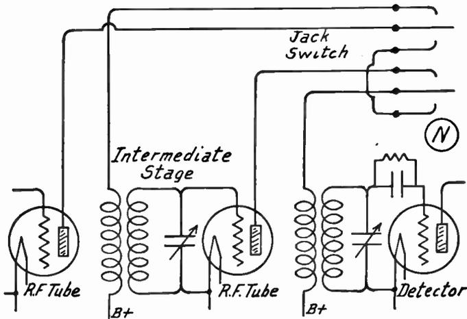
FIG. 12.—Jack Switch for Cutting Out Intermediate Radio Tube.
