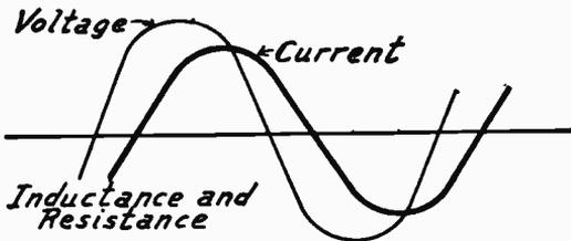
FIG. 3.—Current Lagging Behind Voltage.
