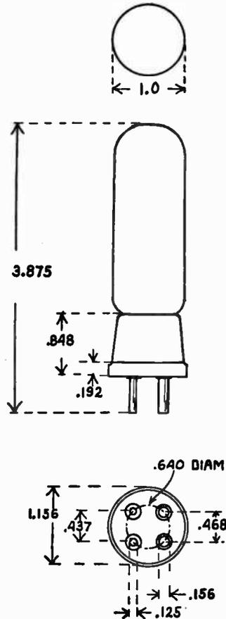
FIG. 2.—Dimensions in Inches of Dry Cell Power Amplifying Tube.
