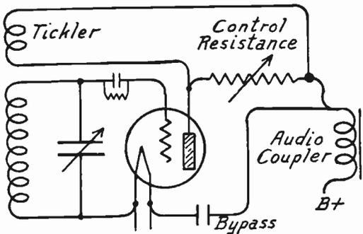
FIG. 6.—Fixed Ticker Control with Shunt Resistance.
