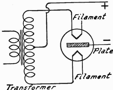
FIG. 2.—Connections of Full-Wave Rectifying Tube.
