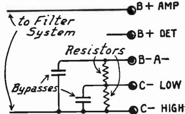
FIG. 11.—Two Grid Biases from Single Plate Voltage Supply.
