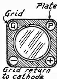
FIG. 2.—Socket Connections for A. C. Tube.
