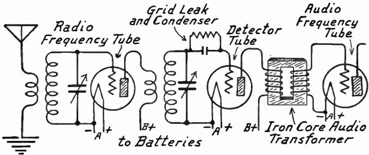
FIG. 22.—Audio Frequency Coupling with Iron-Core Transformer.
