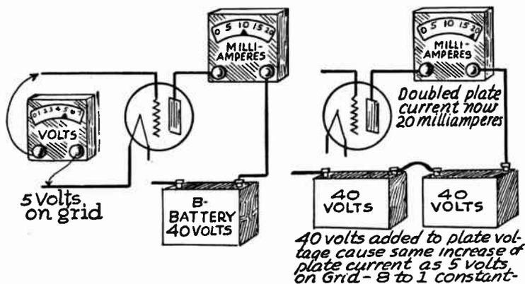
FIG. 1.—The Voltage Amplification of a Vacuum Tube.
