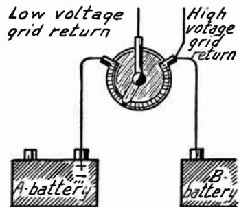
FIG. 8.—Two Biasing Voltages from Potentiometer.
