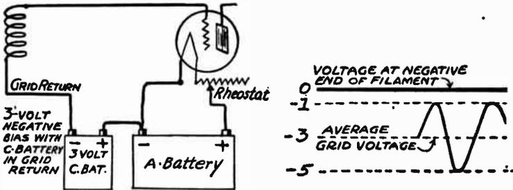
FIG. 4.—Negative Bias with C-Battery Alone.
