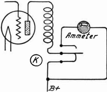
FIG. 19.—Switch for Plate Milliammeter.
