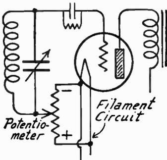
FIG. 15.—Potentiometer in Grid Return to Control Regeneration.
