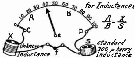
FIG. 7.—Inductance Measurement with Bridge.
