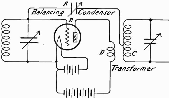
FIG. 3.—Neurodyne Method of Balancing.
