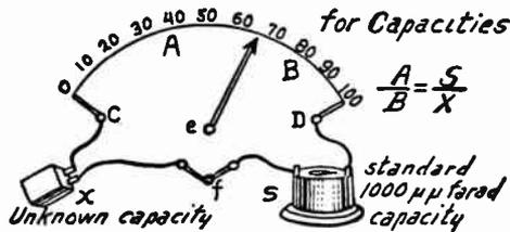
FIG. 8.—Capacity Measurement with Bridge.
