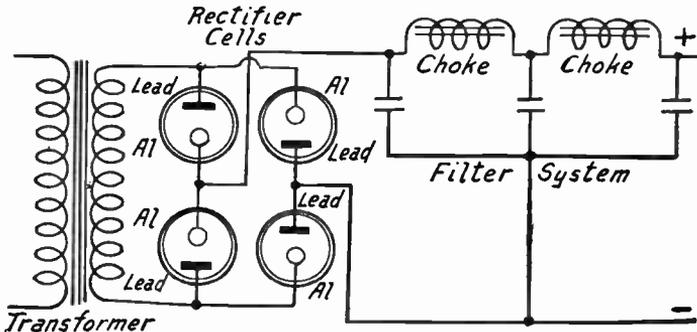
FIG. 4.—Power Unit with Electrolytic Rectifier.
