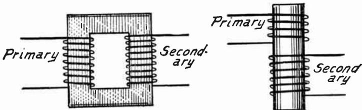
FIG. 1.—Core Type of Transformer.
