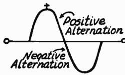
**ALTERNATOR.**—An electric generator producing alternating voltages and current. See *Current, Alternating*.
