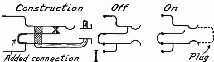
FIG. 4.—Jack Remodeled for Closed Circuit Work.
