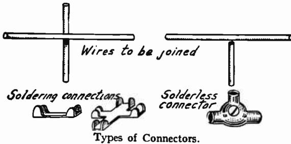
pose. A solder type of connector consists of a piece of thin tinned brass or copper with the ends formed into lips or ears. These lips are turned up around the wires to be joined, clamped over the wires with pliers, and soldered securely.
