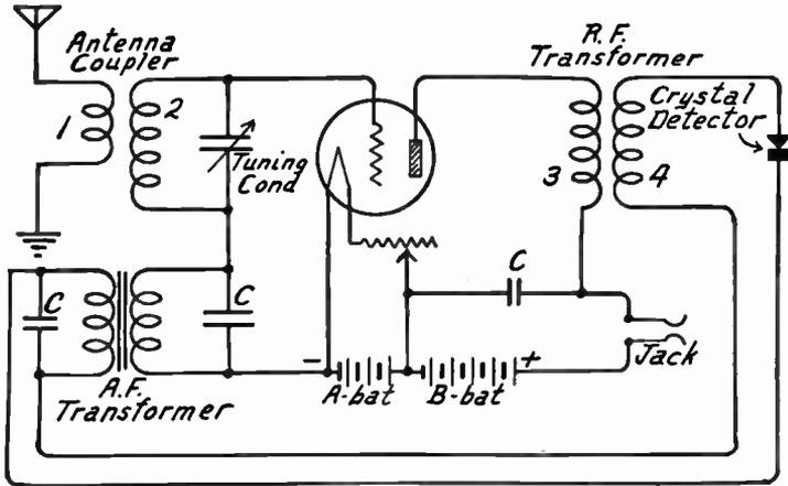
FIG. 3.—Single Tube Reflex Receiver with Crystal Detector.
