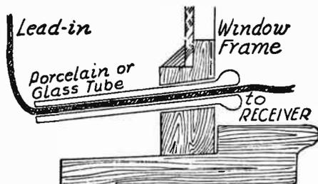
Antenna Lead-in Carried Through Tube.
