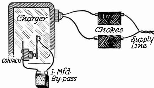
FIG. 5.—Handling Interference of Vibrators and Flashers.
