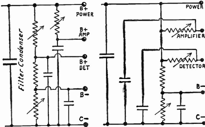
FIG. 1.—Obtaining Grid Biasing Voltage from Plate Supply Unit in Complete Receiver Supply Type of Power Unit.
