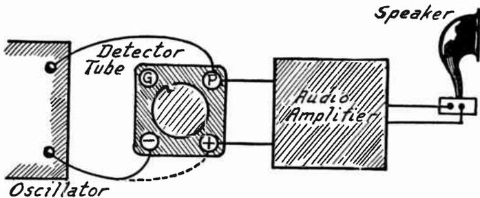
FIG. 5.—Testing Complete Audio Amplifier with Audio Oscillator.
