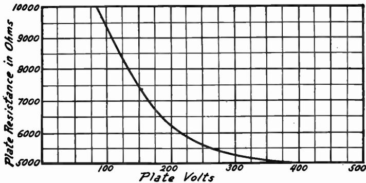
FIG. 15.—Plate-Voltage, Plate-Resistance Curve with Changing Grid Bias.
