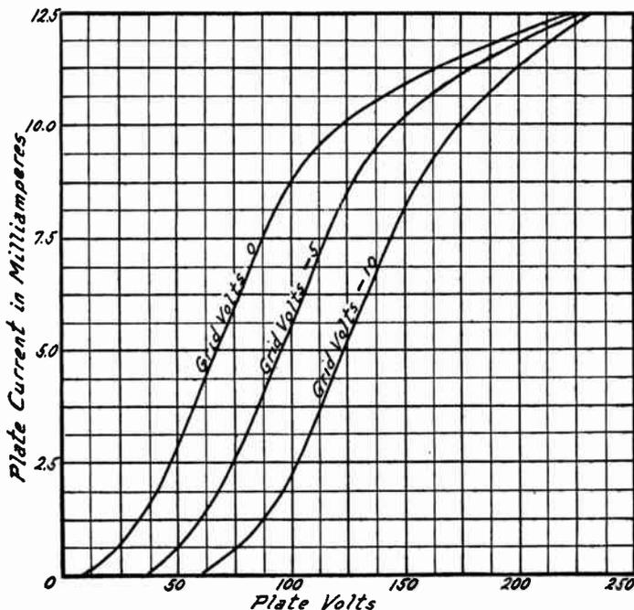
FIG. 12.—Plate-Voltage, Plate-Current Curves for Various Grid Voltages.
