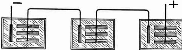
FIG. 4.—Electrolytic Condensers in Series for High Voltages.
