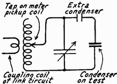
FIG. 4.—Variations of Test for Matching Condensers with Radio Oscillator.
