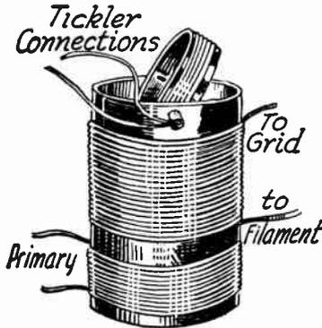
FIG. 2.—Construction of Movable Tickler Coil Used to Obtain Regeneration.
