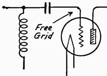
FIG. 3.—Grid Isolated by Condenser With No Leak in Use.
