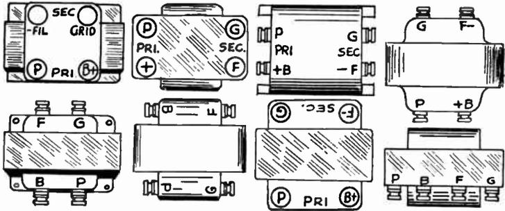
FIG. 2.—Terminal Arrangements on Audio Transformers for Amplifiers.
