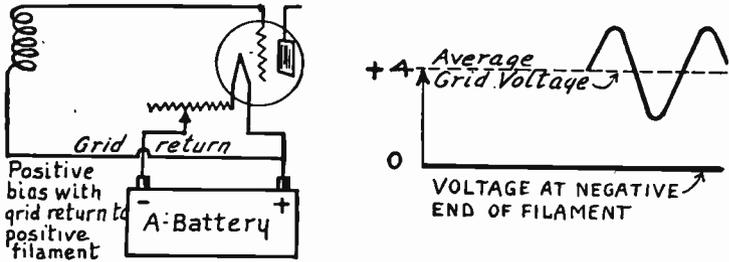
FIG. 6.—Obtaining Positive Grid Bias.
