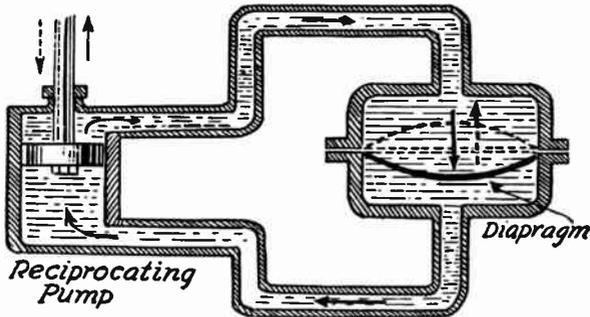
FIG. 5.—Hydraulic Explanation of Condenser Action.
