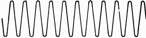
FIG. 1.—Carrier Wave of Constant Frequency and Amplitude.
