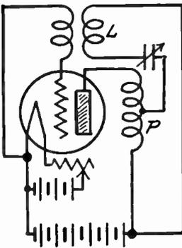
FIG. 5.—Oscillator with Part of Plate Coil in Tuned Circuit.
