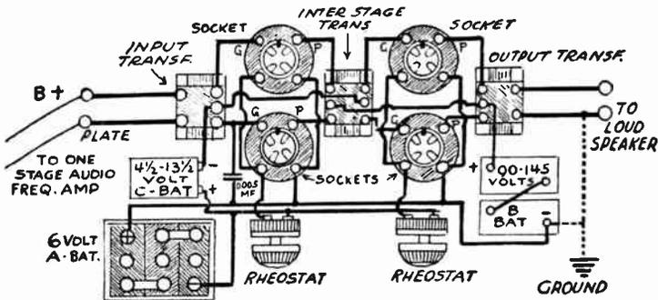
FIG. 3.—Two Stages of Push-Pull Amplification.
