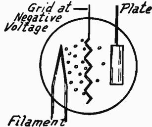
FIG. 9.—Effect of Negative Grid Voltage on Electron Flow.
