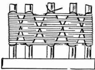
FIG. 4.—Finished Basket Winding with Lacing in Place.
