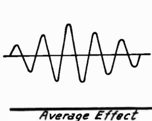
FIG. 19.—Voltages as Received by Detector Tube.
