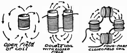
FIG. 1.—Coils with Open Fields and Closed Fields.
