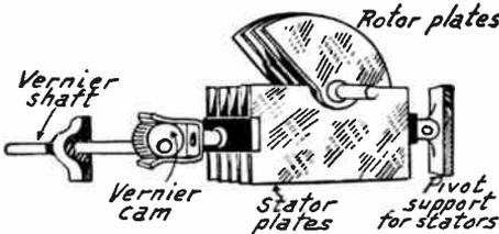
FIG. 1.—Hinged Condenser Plates with Cam Vernier.
