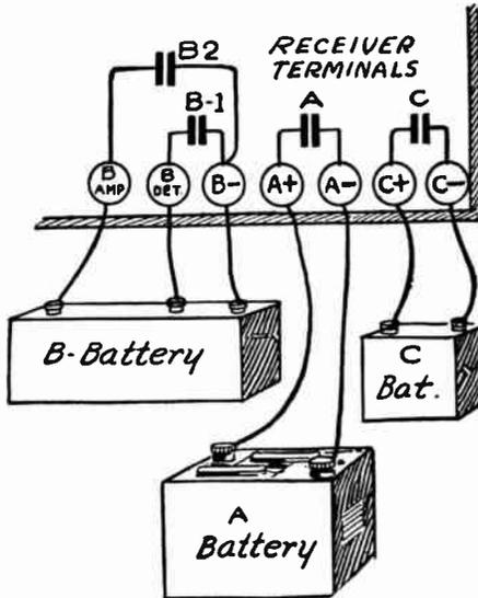
FIG. 3.—Connections of Bypass Condensers to Receiver Terminals.
