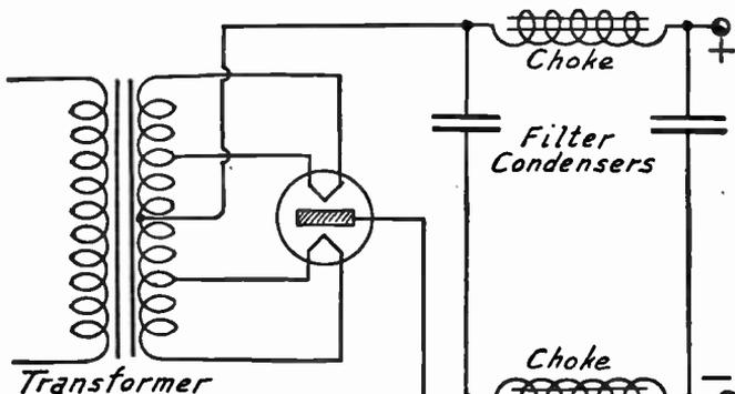
FIG. 8.—Full Wave Rectifier with Chokes in Both Lines.
