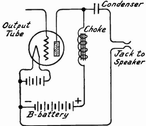
FIG. 3.—Circuits of Condenser and Choke for Speaker Connection.
