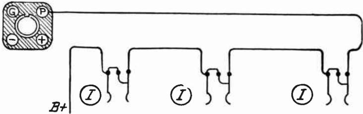
FIG. 24.—Plug-In Outlets for Several Speakers.
