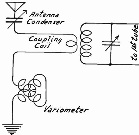
FIG. 5.—Variometer Tuned Antenna with Loose Coupling.
