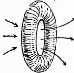
FIG. 2.—Magnetic Field of Toroid
