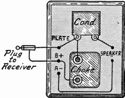
FIG. 5.—Condenser and Choke Unit for Speaker Connection.
