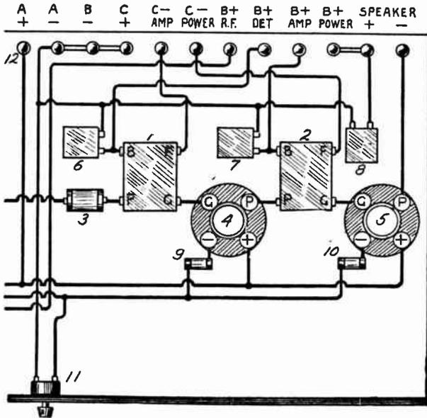
AUDIO AMPLIFIER WITH TWO TRANSFORMER STAGES
