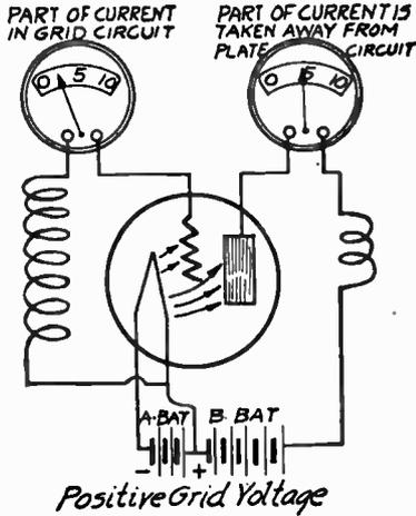
FIG. 5.—Current in Grid Circuit with Positive Bias.
