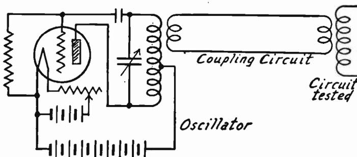
FIG. 3.—Link Circuit for Radio Oscillator Coupling.
