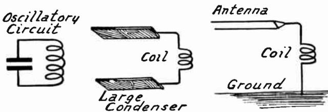
FIG. 5.—Oscillatory Circuit Formed by Antenna and Ground.
