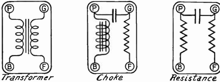
FIG. 5.—Similarity of Terminal Connections with Various Couplers.
