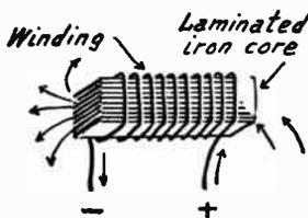
FIG. 4.—An Electromagnet with Its Field.
