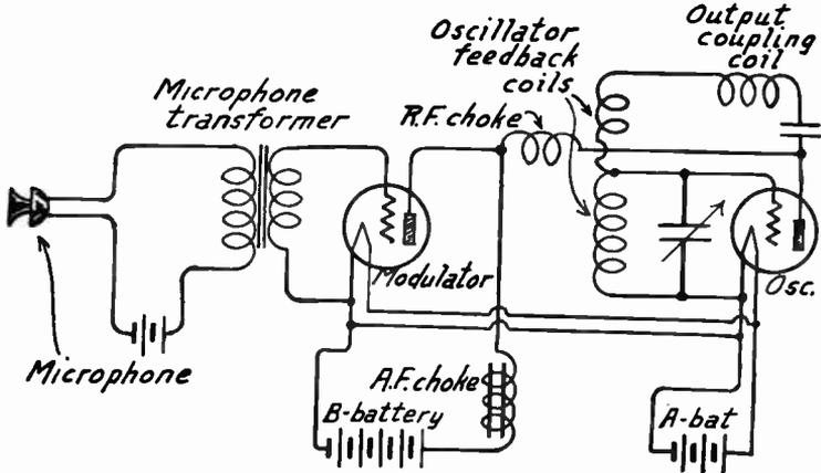
FIG. 2.—Absorption Method of Modulation.
