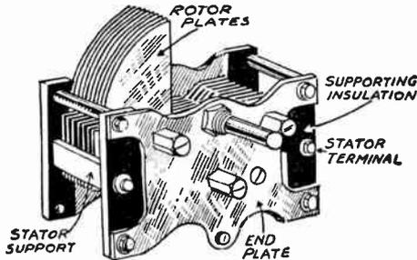
FIG. 3.—Terminal Positions Considered in Condenser Design.
