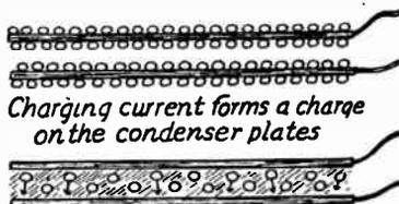
*Charging current forms a charge on the condenser plates*
