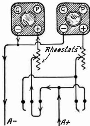
FIG. 7.—Filament Control Operating One Tube.
