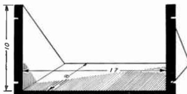
**RELAY RACK SHELF:** This recessed shelf will fit any standard relay rack, and is particularly useful for supporting portable equipment, instruments, test equipment, etc.
