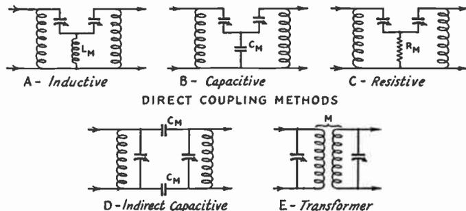
FIG. 407 — BASIC TYPES OF CIRCUIT COUPLING
