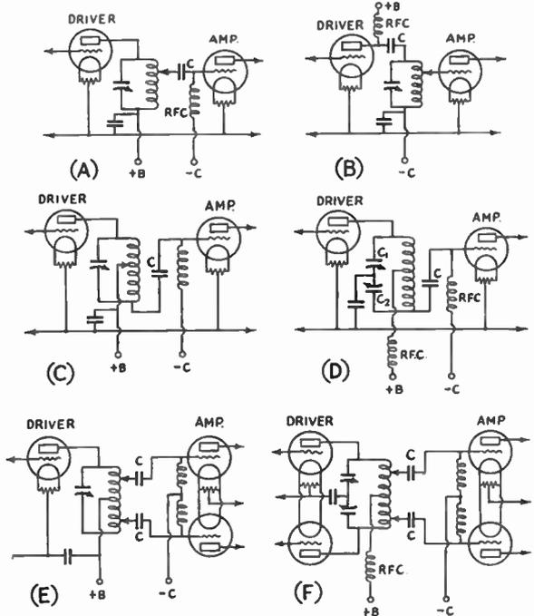
FIG. 814—DIRECT OR CAPACITY-COUPLED DRIVER AND AMPLIFIER STAGES
