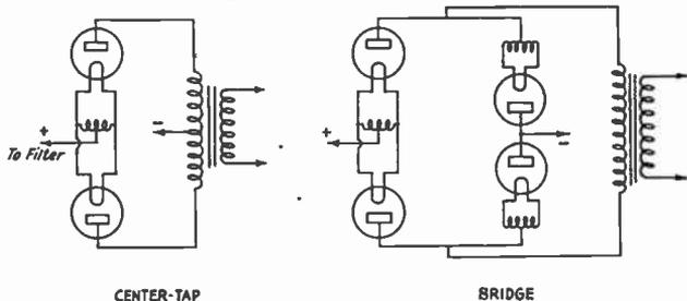
FIG. 1504 — CENTER-TAP AND BRIDGE RECTIFIER CIRCUITS
