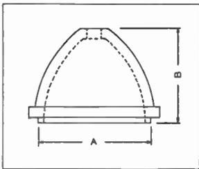
**H.F. BUSHING.** Larger in size than the bushings described above, and shaped to conform to the lines of electrical stress, these Steatite insulators are suitable for higher H.F. voltages. Prices are per pair, with metal fittings.
