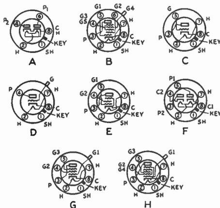
FIG. 518 — BASE DIAGRAMS OF METAL RECEIVING TUBES
