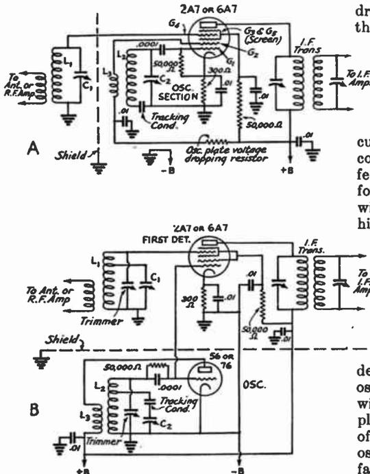
FIG. 609 — THESE FREQUENCY-CONVERTER CIRCUITS ARE FOR USE WITH PENTAGRIDS TUBES
