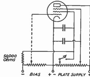
**FIG. 1004 — SUPPRESSOR KEYING OF A PENTODE TRANSMITTING TUBE**
