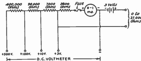
FIG. 1712 — A COMBINATION OHMMETER AND D.C. VOLTMETER SUITABLE FOR RECEIVER TESTING
