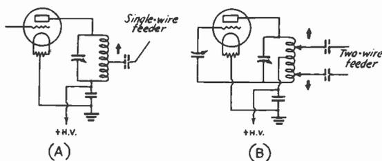
**FIG. 827 — DIRECT COUPLING TO THE ANTENNA OR FEEDERS**
