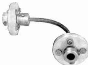
This new and extremely useful coupling combines Isolantite insulation with a short length of flexible shafting. It provides a driving means between offset shafts, or shafts at any angle up to 90 degrees. It virtually eliminates
