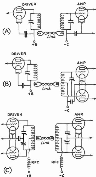
**FIG. 817 — LINK COUPLING, USING A LOW-IMPEDANCE TRANSMISSION LINE**
