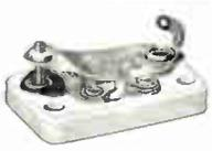
New improved type. Conditioned Isolantite base. Most expensive imported mica used. Tested for capacity, power factor and breakdown at 500 V D.C. 1" x 1 1/8".
