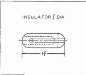
**STRAIN INSULATOR.** This aircraft-type insulator, in spite of its short leakage path, has a variety of uses in small portable, mobile and police installations. Being loaded in compression, the insulator provides great mechanical strength.
