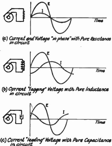
FIG. 309 — VOLTAGE AND CURRENT PHASE RELATIONS WITH RESISTANCE AND REACTANCE CIRCUITS
