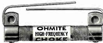
These small high frequency chokes are made especially for use in five and ten meter transmitters. The winding is protected against contact with other live parts and against corrosion. Because of their small size these chokes may be used even in the smallest transceivers. Characteristics of chokes are as follows: Maximum current—1,000 mls. Inductance—5.4 mic. henries. Resistance—0.85 ohms. Larger chokes or chokes with other characteristics may be secured upon order.
