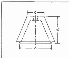
**H.F. BUSHING.** This small Steatite bushing has a variety of uses in transmitter construction, not only as a neat and efficient means of bringing H.F. leads through partitions, but as a support for coils, etc. Each pair of cones includes suitable metal fittings.
