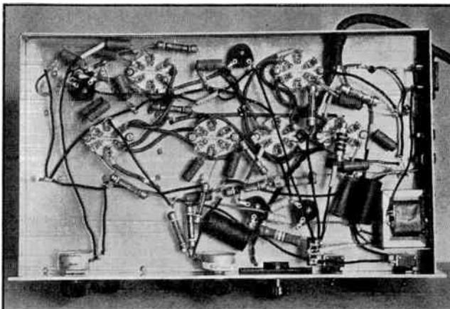
FIG. 724 — A BOTTOM VIEW OF THE SIX-TUBE SUPERHET
