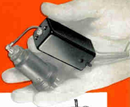
Polyiron Core I.f. Transformers reduce QRM and improve any air-core superheterodyne.
