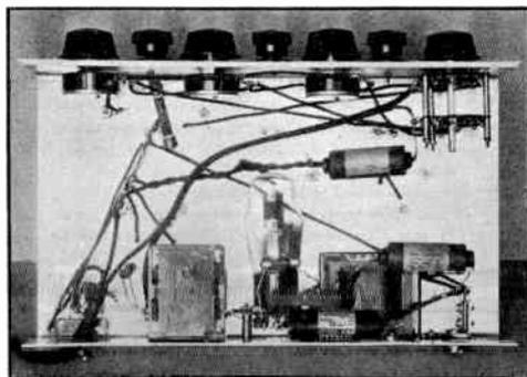
FIG. 1308 — SHOWING THE ARRANGEMENT OF THE AUDIO TRANSFORMER, DETECTOR VOLTAGE-CONTROL POTENTIOMETERS AND WIRING OF THE THREE-BAND RECEIVER
