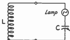
FIG. 1703 — ABSORPTION FREQUENCY METER CIRCUIT
