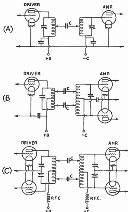
FIG. 815 — TRANSMISSION-LINE OR "MATCHED IMPEDANCE" COUPLING
