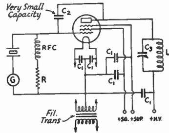
FIG. 808 — CIRCUIT FOR A HIGH-POWER PENTODE OSCILLATOR WITH EXTERNAL FEEDBACK
