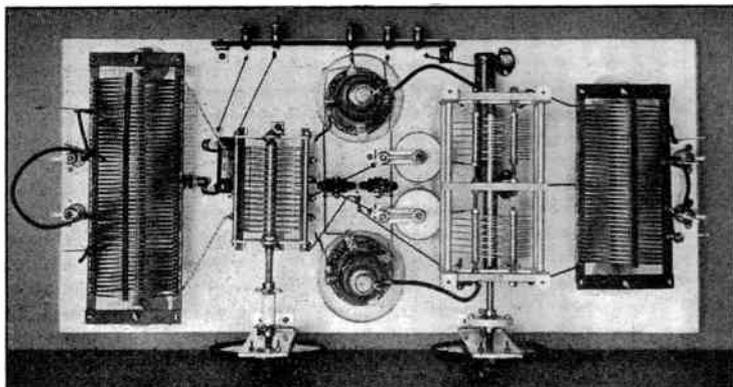
The complete circuit of the amplifier is shown in Fig. 925. Provision is made for link coupling to the grids and similar output coupling to an antenna tuning unit. Any of three bands, 3.5, 7 and 14 mc., can be selected by proper placement of the shorting clips on the grid and plate coils; shorting is from the center out-
