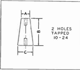
**STAND-OFF INSULATOR.** This popular style of insulator is offered in three sizes, all of low-loss Steatite. The smallest model is tapped 8-32 each end, the larger 10-24.
