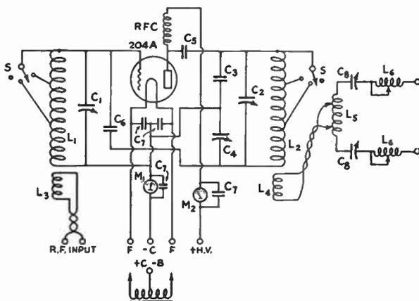
FIG. 930 — CIRCUIT DIAGRAM OF THE 204-A AMPLIFIER
