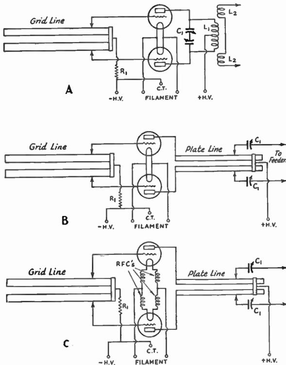
FIG. 1407 — THREE BASIC CIRCUITS FOR THE SHORT-LINE-CONTROLLED OSCILLATOR
