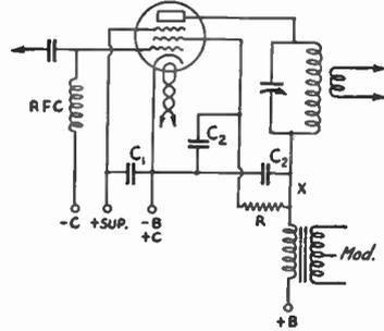
FIG. 1209-A — PENTODE PLATE-MODULATION CIRCUIT WITH SCREEN-DROP RESISTOR
