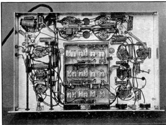
**FIG. 731 — THE UNDER-CHASSIS ASSEMBLY OF THE RECEIVER**
