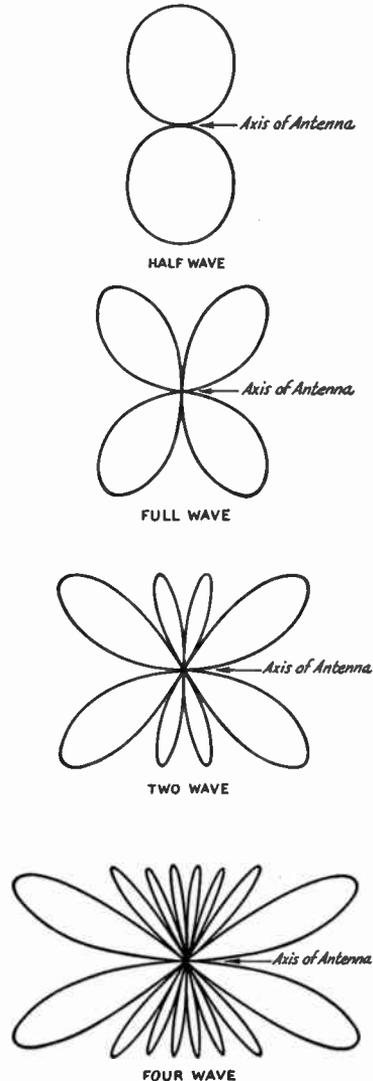
**FIG. 1601 — CROSS-SECTIONS OF SPACE DIRECTIONAL PATTERNS OF HERTZ ANTENNAS**
