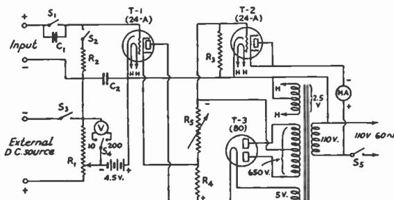
FIG. 1715 — A VACUUM TUBE VOLTMETER WITH D.C. AMPLIFIER
