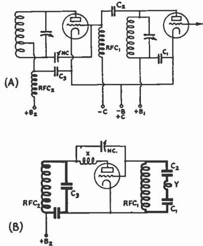
FIG. 833—HOW LOW-FREQUENCY PARASITIC OSCILLATIONS CAN BE GENERATED
