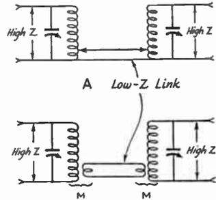
FIG. 409 — METHODS OF USING LINK COUPLING FOR IMPEDANCE MATCHING
