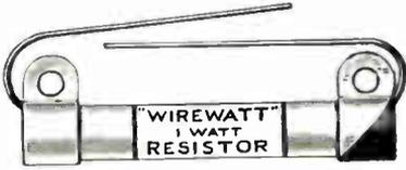
These small one-watt wire wound resistors have many uses, especially in receivers; they are available in resistance values from 100 ohms through 25,000 ohms. Because they are wire wound, they have no voltage or temperature characteristics and are absolutely quiet in operation. Winding is covered with moisture proof material which also insulates against short circuits. Wire leads tinned for quick soldering.
