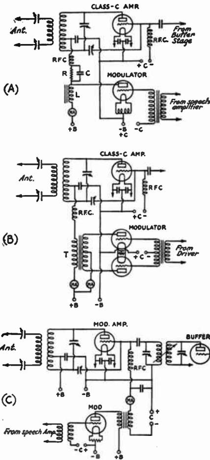
**FIG. 1103 — CIRCUITS FOR THREE METHODS OF MODULATION**
