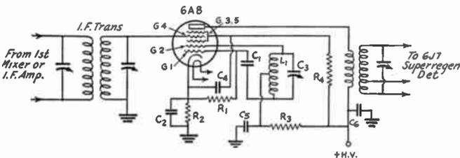
FIG. 1323 — A SUGGESTED CIRCUIT FOR THE 6A8 CONVERTER
