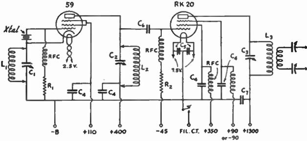
FIG. 932 — CIRCUIT DIAGRAM OF THE TWO-STAGE PENTODE TRANSMITTER
