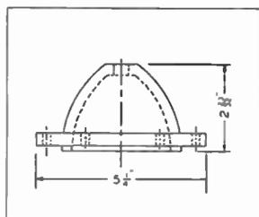
**H.F. BUSHING.** A heavy bowl-type lead-in, suitable for large transmitters, this Steatite insulator provides a weatherproof joint for antenna lead-in purposes. Leakage Path 3 1/4".
