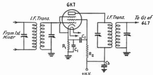
FIG. 1324 — WIRING OF THE SUGGESTED I.F. AMPLIFIER
