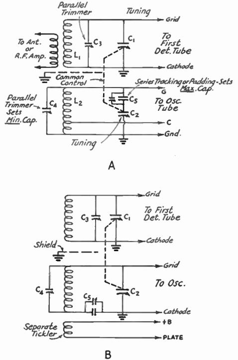
FIG. 613—CONVERTER CIRCUIT TRACKING METHODS
