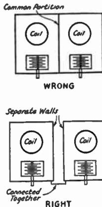
FIG. 605 — SHIELDING ALWAYS SHOULD BE COMPLETE ABOUT EACH PIECE OR GROUP OF APPARATUS SHIELDED
