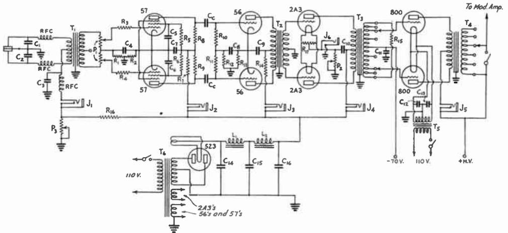
FIG. 1206 — CIRCUIT OF THE 100-WATT AUDIO SECTION
