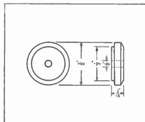
**H.F. BUSHING.** A small, inexpensive Steatite bushing that has a variety of uses in H.F. Transmitters. Convenient as well as efficient, they give a professional appearance to amateur equipment.
