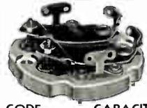
New double Isolantite type with all the outstanding features of the single type. Phosphor bronze flexible plates shaped to provide substantially straight line capacity increase. Constant capacity and power factor maintained under all varying conditions of temperature, humidity, and vibration. Base 1 15/16". Mounting centers 1 1/2".
