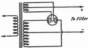
FIG. 1503 — HOW FULL-WAVE TUBE RECTIFIERS ARE CONNECTED
