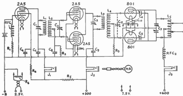
FIG. 936 — CIRCUIT DIAGRAM OF THE TRANSMITTER
