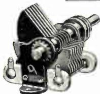
Ideal variable condensers for ultra-short wave and short wave tuning; laboratory, and test equipment. Isolantite insulation. Dielectric losses minimized. All contacts riveted or soldered. Vibration proof. Rotor and stator plates non-corrosive brass—.0025". Shaft— $\frac{1}{4}$ " extending  $5\frac{1}{16}$ " beyond rear frame for ganging. End mounting plates—heavy aluminum. Single hole panel or base mounting. Tested for breakdown on 500 V—A.C.
