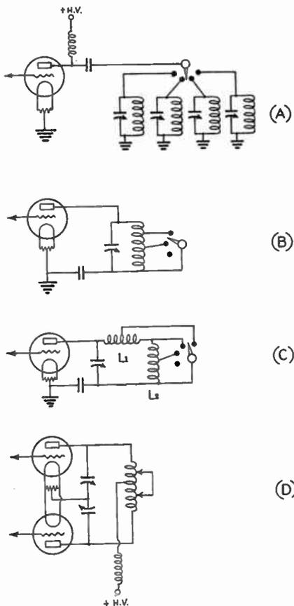
**FIG. 831 — METHODS OF SWITCHING THE AMPLIFIER PLATE TANK CIRCUIT FOR CHANGING BANDS**
