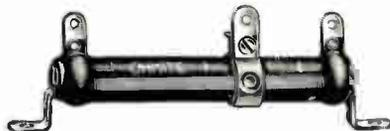
These vitreous enameled adjustable units have a great many uses in radio work; they make excellent voltage dividers as several adjustable lugs may be used on one unit; the "ball-point" contact shorts out little resistance yet makes a firm connection to the bared space on the winding. Made in six sizes—25 watt, 50 watt, 75 watt, 100 watt, 160 watt, and 200 watt, in resistance values from 1 ohm through 100,000 ohms. Mounting brackets and one adjustable lug furnished with each unit.
