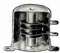
For use in high gain circuits. Universal impregnated wound pies inclosed in an aluminum shield 1 1/8" high x 1 3/8" in diameter. Mounting legs on 1 11/16" center. Connections to terminal are on one side of the can properly indicated. Inductance — 10 mh. D.C. resistance — 65 ohms. Current carrying capacity — 100 ma.
