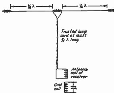
**FIG. 1621 — DOUBLET RECEIVING ANTENNA**
