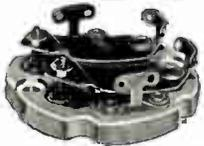
New double Isolantite type with all the outstanding features of the single type. Phosphor bronze flexible plates shaped to provide substantially straight line capacity increase. Constant capacity and power factor maintained under all varying conditions of temperature, humidity, and vibration. Base 1 15/16". Mounting centers 1 1/2".
