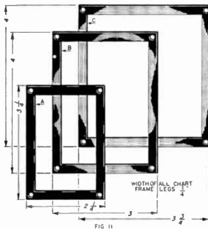
**COIL CHART FRAMES:** Nickel Silver Chart Frames are available in the sizes shown above. The largest frame is the same as that used on the AGS, the medium frame is the same size as that on the FB-7, and the smallest is the same as the HRO frame. Prices include celluloid sheet to protect the chart.
