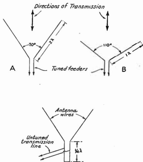
FIG. 1626 — ILLUSTRATING THE MODEL D OR "V" TYPE LONG-WIRE ARRAY
