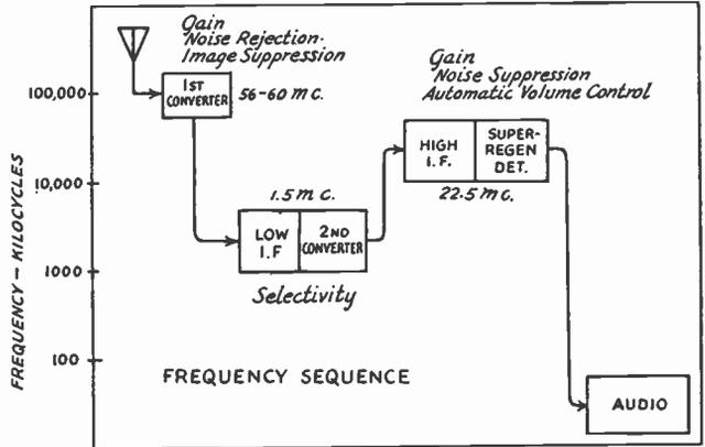
FIG. 1319 — ILLUSTRATING THE PRINCIPLE USED IN THE SUPER-INTRAGENERATOR RECEIVER
