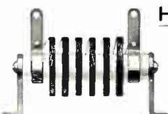
For parallel feed in high powered transmitters — 20- 40- 80- and 160-meter amateur bands. High equivalent impedance more than 500,000 ohms. Effective from 1500 to 15,000 K.C. Six thin universal pies — Isolantite core. Ind. — 2.5 mh. Dist. cap. less than 1.5 mmf. D.C. res. — 8 ohms. Max. recommended D.C. (continuous) 500 ma. Overall size less brackets — 1 3/16" x 2 3/8".
