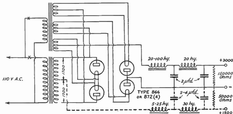
**FIG. 1508 — HIGH POWER BRIDGE RECTIFIER CIRCUIT. WHEN THE CENTER-TAP FILTER SHOWN IN DOTTED LINES IS USED, A TAP AT HALF MAXIMUM VOLTAGE WITH GOOD REGULATION IS PROVIDED. THE TOTAL CURRENT DRAWN FROM BOTH TAPS SHOULD NOT EXCEED 300 MA. FOR 866'S OR 1600 MA. FOR 872'S**
