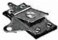
Standard type, illustrated at left, is popular for neutralizing, balancing and trimming. Mica dielectric — phosphor bronze flexible plates — bakelite base 1 1/4" x 1 1/16".
