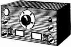
The HRO is a 9 tube communication-type superheterodyne for amateur use providing extreme band-spread on amateur bands as well as a continuous frequency coverage from 500 K.C. to 30 M.C. An additional range 175-400 K.C. is also available. Two stages of preselection are used. A booklet describing the HRO will be mailed on request.
