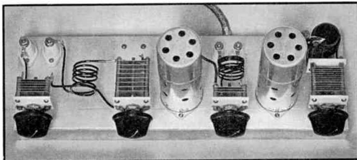
same tubes in the oscillator as in the amplifier, or at least tubes having the same power capabilities. The adjustment of such a transmitter, with respect to neutralization and excitation, will be carried out exactly in accordance with the principles given in Chapter VIII.
