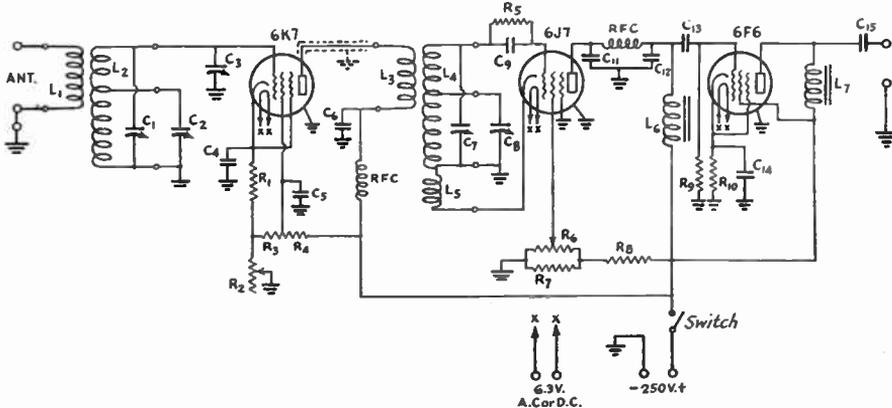
**FIG. 720 — CIRCUIT DIAGRAM OF THE METAL-TUBE T.R.F. RECEIVER**
