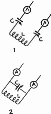
**FIG. 1606 — SERIES AND PARALLEL FEEDER TUNING**
