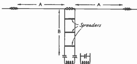
FIG. 1608 — CENTER-FED ANTENNA WITH TUNED FEEDERS
