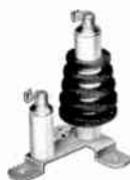
**R-152 and R-154.** These two universal transmitter chokes have windings of the honeycomb type, divided in five sections, and are rated to carry 0.6 amperes continuously. Inductance 4 m.h., D.C. resistance 10 ohms. The R-152 is designed to give maximum impedance in the 160 meter band, and the R-154 in the 40 meter band.
