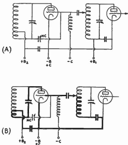
**FIG. 834 — A HIGH-FREQUENCY PARASITIC CIRCUIT RESULTING FROM THE USE OF A TAPPED EXCITATION COIL**
