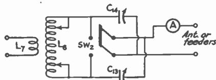
FIG. 939 — WIRING OF THE ANTENNA TUNER
