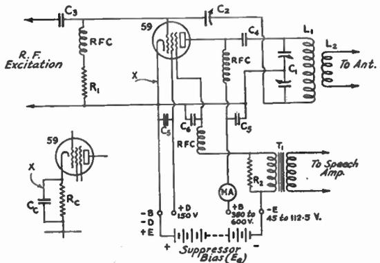
**FIG. 1104 — CIRCUIT OF THE SUPPRESSOR-GRID MODULATED R.F. AMPLIFIER**
