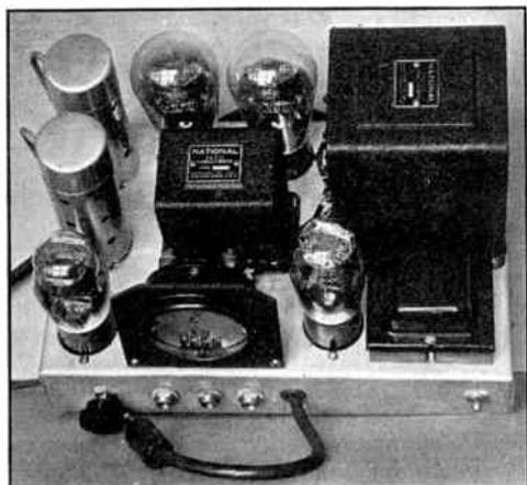
**FIG. 1203 — THE ECONOMY MODULATOR UNIT CONTAINS A CRYSTAL-MICROPHONE SPEECH AMPLIFIER, DRIVER AND CLASS-B MODULATOR, AS WELL AS A POWER SUPPLY FOR THE LOW-POWER STAGES**
