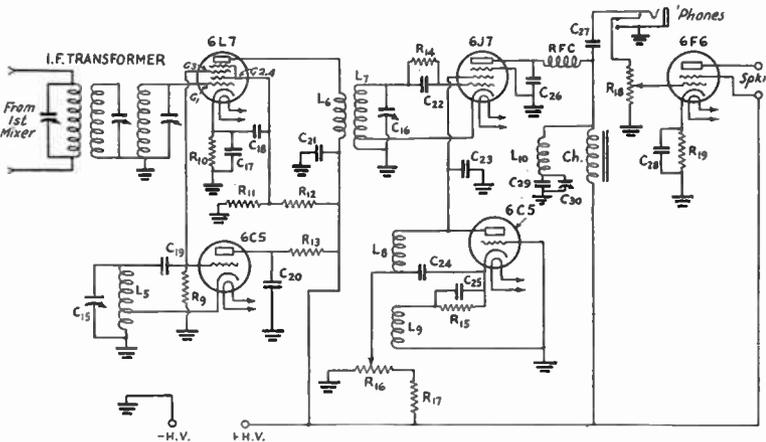
**FIG. 1321 — THE WIRING OF THE INTERMEDIATE-FREQUENCY SECTION**
