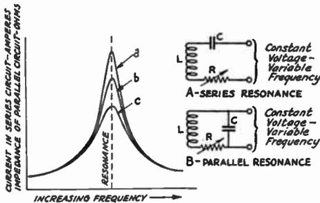
FIG. 402 — CHARACTERISTICS OF SERIES-RESONANT AND PARALLEL-RESONANT CIRCUITS
