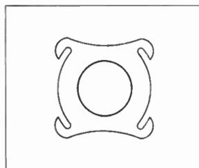
**TRANSPPOSITION BLOCK.** In addition to the popular AA-1 Victron Block, National now offers a smaller Steatite Block. Both are light in weight, both are highly efficient. The Victron Block AA-1 separates feeders 1 1/2", the Steatite Block, AA-2, provides 1" separation.
