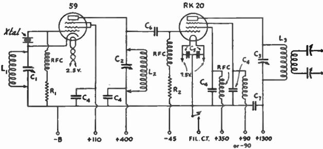
FIG. 932 — CIRCUIT DIAGRAM OF THE TWO-STAGE PENTODE TRANSMITTER
