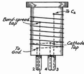
FIG. 706 — COIL SOCKET CONNECTIONS AND THE METHOD OF BRINGING OUT COIL TERMINALS
