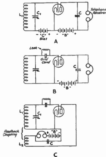
FIG. 512 — DETECTOR CIRCUITS OF THREE TYPES
