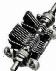
For perfect band spreading or for amateur band frequency meters. Tank section may be set and locked to any desired capacity. Tuning section spreads narrow frequency ranges over entire dial regardless of range of band or coils used. Tank cap.—100 mmf. Tuning cap. type "120-B"—20 mmf.; type "150-B"—50 mmf.; type "175-B"—80 mmf. Isolantite insulation at front and rear. Plates rigidly held in place.
