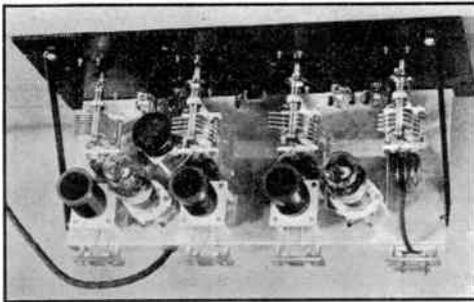
order of three to five watts is shown in Fig. 916. It uses two Type 53 tubes, each of which has two separate triodes in one bulb. The two tubes are therefore equivalent to four. Relay-rack type construction is used. The circuit diagram is given in Fig. 917.
