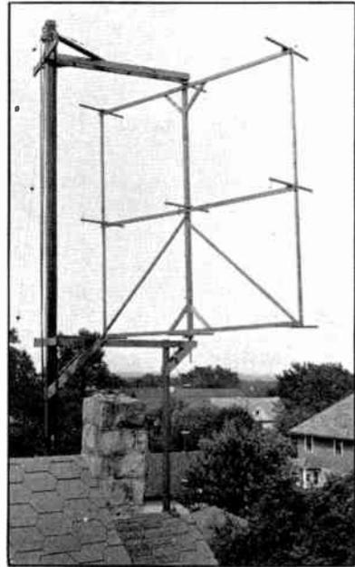
**FIG. 1624 — THE 112-MC. ARRAY AT W2CUZ: AN EXCELLENT EXAMPLE OF CONSTRUCTION TO ALLOW ROTATION OF THE SYSTEM**
