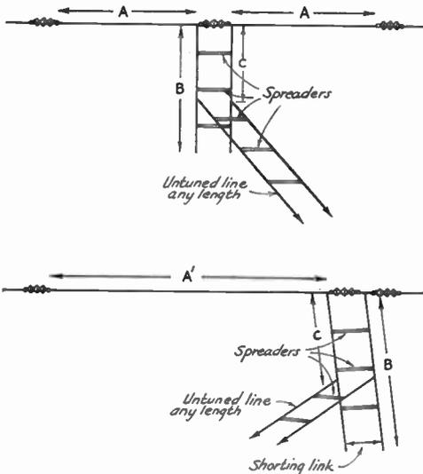
FIG. 1616 — IMPEDANCE-MATCHING ANTENNA SYSTEMS WITH QUARTER-WAVE OPEN WIRE MATCHING TRANSFORMERS
