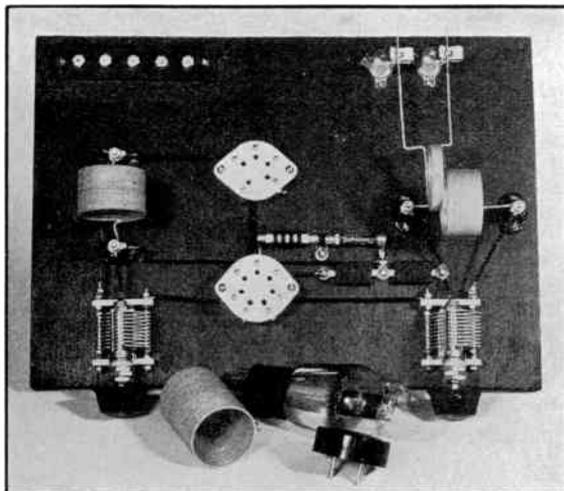
**FIG. 910 — A TOP VIEW OF THE CRYSTAL OSCILLATOR WITH THE TUBE AND CRYSTAL HOLDER REMOVED**
