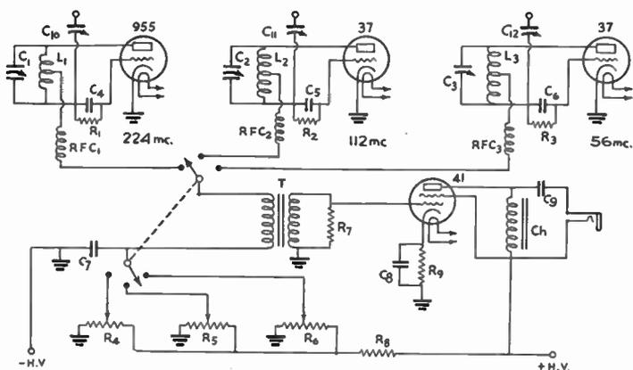
FIG. 1306 — WIRING OF THE THREE-BAND RECEIVER WITH SEPARATE DETECTOR UNITS
