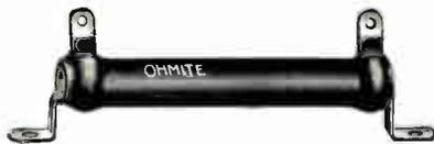
Now made in five sizes: 25 watt, 50 watt, 100 watt, 160 watt, and 200 watt. Resistance values range from 5 ohms through 250,000 ohms. Wire wound over porcelain core and covered with Ohmite vitreous enamel; connections made to terminal lugs both mechanically and by brazing thus assuring permanent, trouble-free, constant resistance units. All are furnished complete with mounting brackets as shown. These are units you can depend on for receivers or transmitters.
