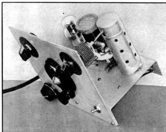
FIG. 708 — A TWO-TUBE RECEIVER HAVING THE EQUIVALENT OF THREE ORDINARY STAGES
