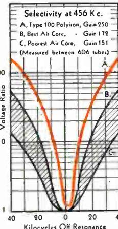
Curve A is that of a Polyiron transformer compared with the best (B) and poorest (C) types of commercial air-core coils.
