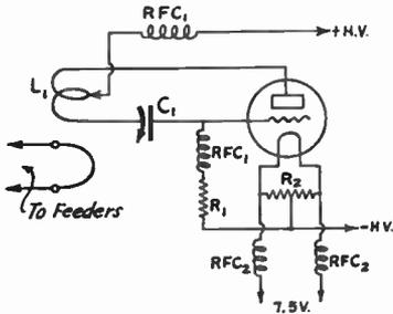
FIG. 1402—CIRCUIT SUITABLE FOR EXPERIMENT ON 112 OR 224 MC.
