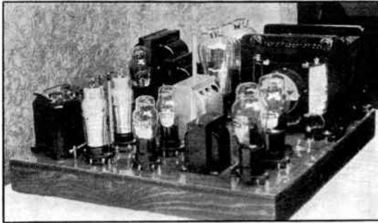
FIG. 1205 — THE SPEECH-AMPLIFIER AND 100-WATT CLASS-B MODULATOR
