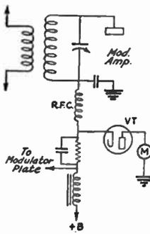
**FIG. 1221—SIMPLE NEGATIVE-PEAK OVERMODULATION INDICATOR (W8AGW)**
