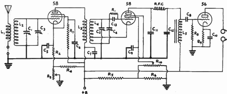
FIG. 713 — CIRCUIT DIAGRAM OF THE THREE-TUBE RECEIVER
