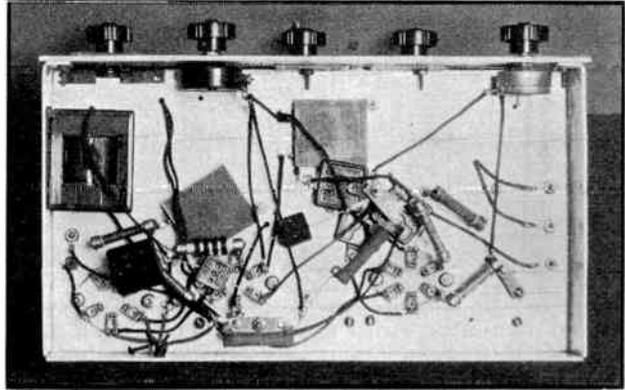
**FIG. 715 — UNDER THE BASE OF THE THREE-TUBE RECEIVER**
