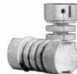
**COIL FORM.** This Steatite Choke Coil Form is ideally suited for small choke coils and precision resistors. The winding is divided in four sections by partitions. A slot is provided for leading the wire from section, and to the terminals.
