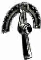
Highly attractive solid molded bakelite controls which enhance the appearance of any equipment. "Window" design makes possible three separate scales if desired. No. 204 has 4" diameter etched scale with polished figures on black background, and fits 1/4" shaft. No. 206 is similar, with 6" scale, fits 1/4" shaft, and has removable bushing for 3/8" shaft.
