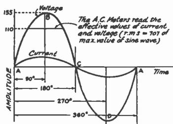
FIG. 306 — REPRESENTING SINE-WAVE ALTERNATING VOLTAGE AND CURRENT
