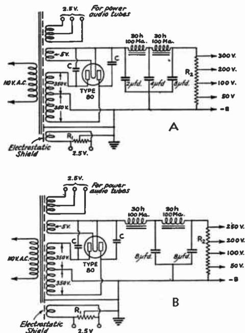
**FIG. 1513 — WIRING DIAGRAMS FOR RECEIVER POWER SUPPLIES**
