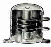
For use in high gain circuits. Universal impregnated wound pies inclosed in an aluminum shield 1 1/2" high x 1 3/8" in diameter. Mounting legs on 1 11/16" center. Connections to terminal are on one side of the can properly indicated. Inductance — 10 mh. D.C. resistance — 65 ohms. Current carrying capacity — 100 ma.
