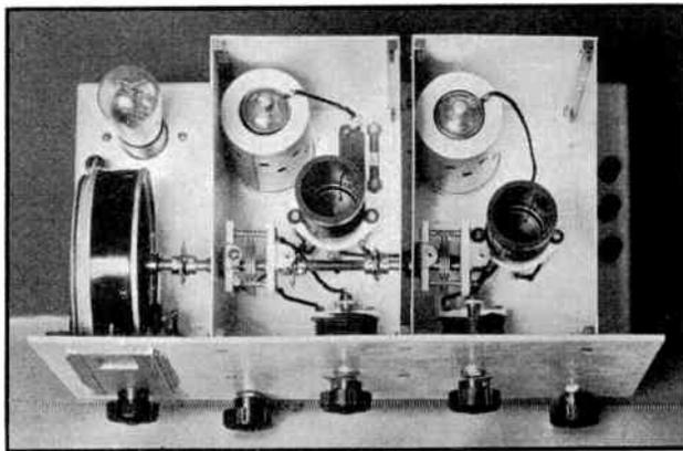
**FIG. 714 — PLAN VIEW OF THE THREE-TUBE AUTODYNE WITH SHIELD COVER REMOVED**
