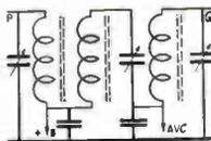
The most popular types of Aladdin Polyiron I.f. transformers are listed below. Where 6-volt tubes are specified, equivalent 2 1/2-volt tubes may be employed. All transformers are supplied with trimmer condensers of mica or air dielectric for both primary and secondary. Type C is in the small container. Type A is in the larger shield.
