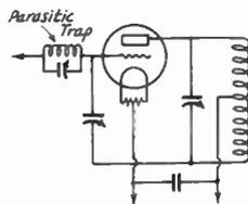
**FIG. 836 — ULTRA-HIGH FREQUENCY TRAP TO ELIMINATE PARASITIC OSCILLATIONS**
