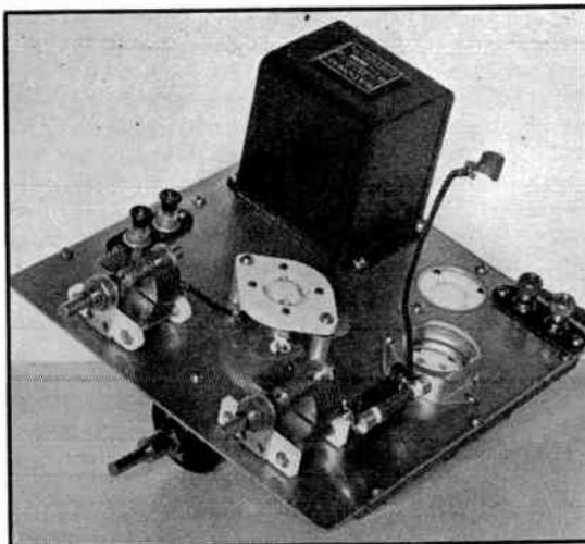
**FIG. 703—THE "CHASSIS" OF THE TWO-TUBE RECEIVER**
