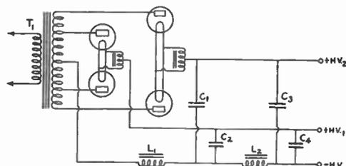
**FIG. 1509 — A POWER SUPPLY CIRCUIT IN WHICH A SINGLE TRANSFORMER AND SET OF FILTER CHOKES IS MADE TO SERVE FOR DIFFERENT VOLTAGES**
