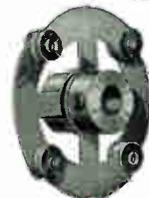
A convenience and time saver where tandem operation of independent units is required. Bakelized canvas with brass bushings for 1/4" shafts. The over-all diameter is 1 1/2". Four rust-proofed and hardened steel set screws guarantee and assure against any slipping of the shafts.
