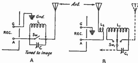
**FIG. 614 — CIRCUITS FOR TWO TYPES OF WAVE-TRAP IMAGE REJECTORS**
