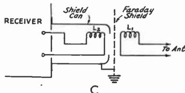
**FIG. 614-C — A SUGGESTED ARRANGEMENT FOR BALANCED INPUT COUPLING WITH A FARADAY SHIELD TO MINIMIZE CAPACITY EFFECTS**
