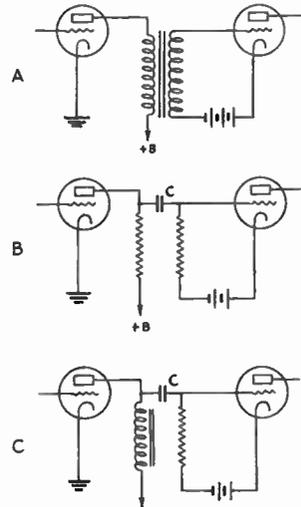
FIG. 507 — METHODS OF COUPLING BETWEEN AMPLIFIER TUBES
