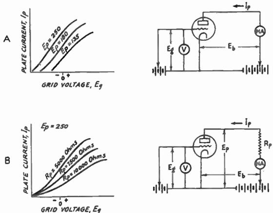
FIG. 504 — STATIC (A) AND DYNAMIC (B) CHARACTERISTICS
