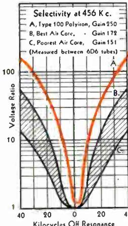
Aladdin Polyiron Core Coils are used in the finest commercial receivers. The diagram (Electronics, May, 1934) shows the band-pass I.f. circuit of the All-Wave Stromberg-Carlson Model 68 using Polyiron coils.
