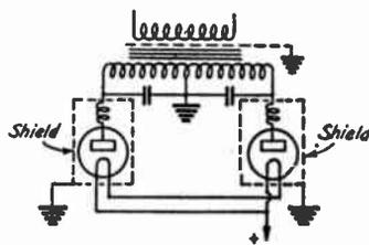
**FIG. 1015 — DEVICES FOR ELIMINATING NOISE FROM MERCURY-VAPOR RECTIFIER TUBES**
