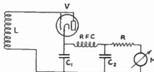
FIG. 1212 — CIRCUIT OF THE SIMPLE DIODE-TYPE CARRIER-SHIFT INDICATOR (W. C. Lent)
