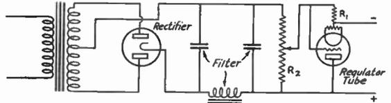
**FIG. 1514 — CIRCUIT OF THE AUTOMATIC VACUUM-TUBE REGULATOR AS APPLIED TO A BIAS- OR PLATE-SUPPLY POWER PACK**
