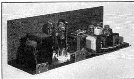
FIG. 1207 — REAR VIEW OF THE 250-WATT DRIVER-MODULATOR UNIT
