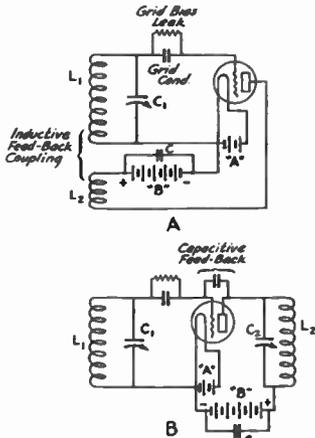
FIG. 511 — TWO GENERAL TYPES OF OSCILLATOR CIRCUITS
