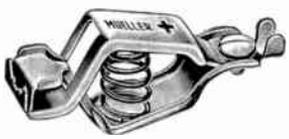
A medium sized clip for connections to storage batteries. Heavy, flanged construction. Lead Plated. Copper shunt protects spring. 25 Amperes.  $2\frac{3}{8}$ " long. Jaw spread 1".
