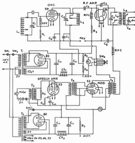
FIG. 1202 — CIRCUIT OF THE 10-WATT 53 MODULATOR UNIT FOR LOW-POWER 'PHONE TRANSMITTERS (W9FVM)
