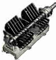
Identical to split stator condensers except that plates are widely spaced—actual air gap between adjacent rotor and stator plates—.0715". There is no shield between the stators. This condenser is ideal for ultra-high frequency transmitters using up to 245's or 210's in push pull.
