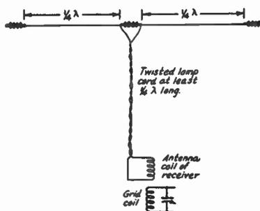
**FIG. 1621 — DOUBLET RECEIVING ANTENNA**
