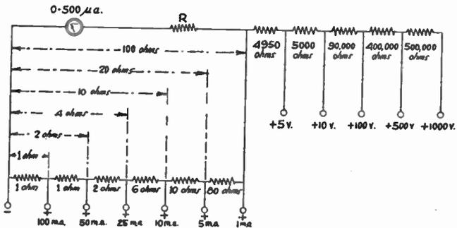
**FIG. 1711 — A MULTI-RANGE VOLTMETER-MILLIAMMETER USING A 0-500 MICROAMMETER**
