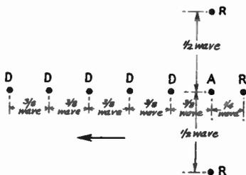
FIG. 1628—SHOWING THE ARRANGEMENT OF THE ANTENNA, REFLECTOR AND DIRECTOR ELEMENTS IN A "YAGI" DIRECTIVE SYSTEM
