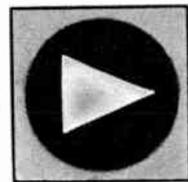
**FIG. 1213-G — ACTUAL PHOTOGRAPH OF TRAPEZOIDAL FIGURE FOR PROPER 100% MODULATION**
