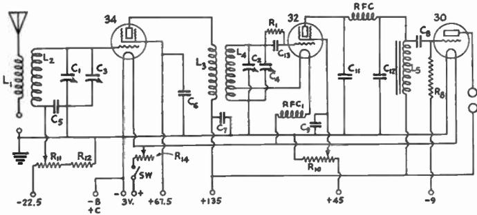
**FIG. 716 — THE THREE-TUBE RECEIVER CIRCUIT MODIFIED FOR USE WITH TWO-VOLT TUBES**
