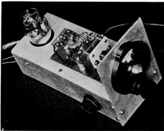
FIG. 1302 — THE THREE-BAND "ACORN" RECEIVER
