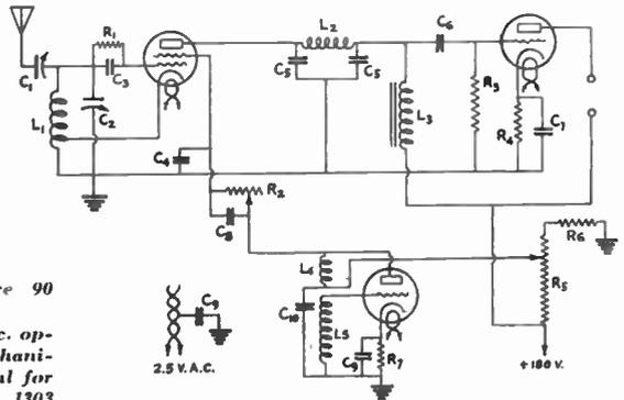
FIG. 1310 — AN ALTERNATIVE CIRCUIT FOR THE THREE-TUBE 56-MC. RECEIVER
