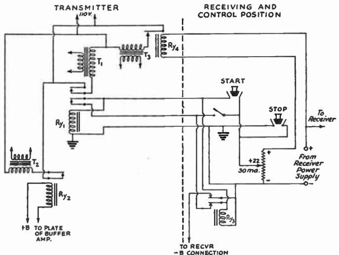
**FIG. 1802 — REMOTE-CONTROL SYSTEM INCORPORATING "PUSH-TO-TALK" WITH AUTOMATIC RECEIVER CUT-OUT AND EXCITATION-FAILURE PROTECTION**
