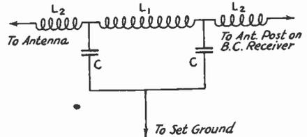
FIG. 1013—A LOW-PASS FILTER FOR REDUCTION OF INTERFERENCE WITH BROADCAST RECEPTION
