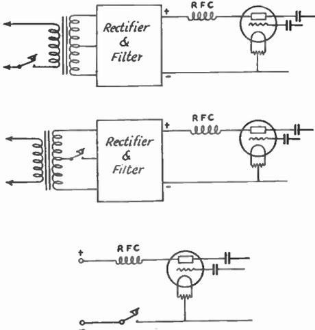
FIG. 1001 — PLATE-KEYING METHODS
