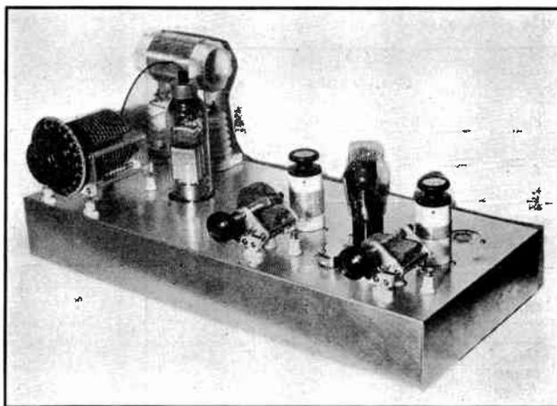
**FIG. 931 — A THREE-BAND TWO-STAGE PENTODE TRANSMITTER**
