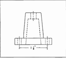
**STAND-OFF INSULATOR.** Another small insulator suitable for a variety of applications. Being made of Steatite, it is eminently suited for Low Loss H.F. circuits. It is available in a special model with a jack for mounting plug-in inductances.
