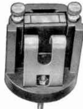
The National Crystal Holder mounts the crystal in a vertical position which permits it to vibrate freely. Crystals may be changed very readily. The cover is of metal and is used for protection and shielding only. The body of the holder is molded R-39, and has two prongs on the base for connections.
