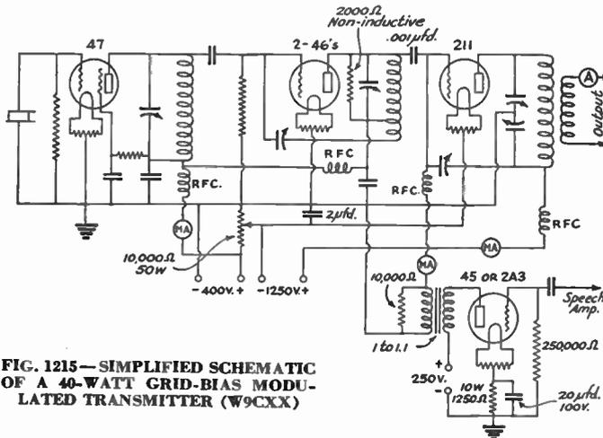
FIG. 1215 — SIMPLIFIED SCHEMATIC OF A 40-WATT GRID-BIAS MODULATED TRANSMITTER (W9CXX)
