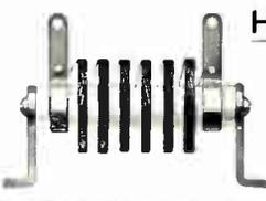
For parallel feed in high powered transmitters — 20- 40- 80- and 160-meter amateur bands. High equivalent impedance more than 500,000 ohms. Effective from 1500 to 15,000 K.C. Six thin universal pies — Isolantite core. Ind. — 2.5 mh. Dist. cap. less than 1.5 mmf. D.C. res. — 8 ohms. Max. recommended D.C. (continuous) 500 ma. Overall size less brackets — 1 3/16" x 2 3/8".
