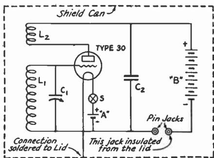
**FIG. 1702 — WIRING DIAGRAM OF THE MONITOR**
