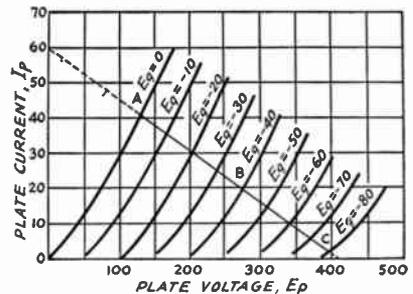
FIG. 505 — A TYPICAL "PLATE FAMILY," SHOWING THE METHOD OF DRAWING A LOAD LINE
