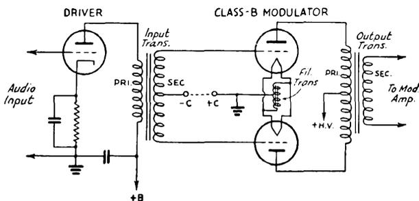
Fig. 610 — Class-B modulator and driver circuit.
