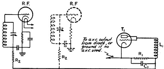
Fig. 1905 — Another protective device for receiver.  $L_1$  is a pick-up coil coupled to the transmitter output tank circuit. Size of coil must be determined by experiment.  $C_1$  — .002  $\mu$ fd.  $R_1$  — 100,000 ohms suggested for first trial. Experiment with particular set-up will be necessary.  $R_2$  — Decoupling resistors in receiver AVC system.
