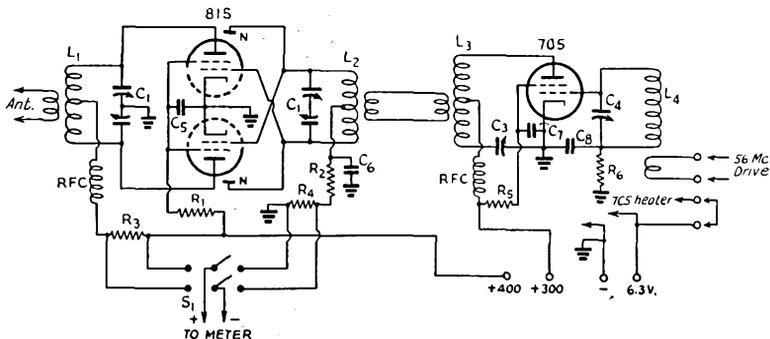
Fig. 2818 — Wiring diagram of the 815 amplifier.
