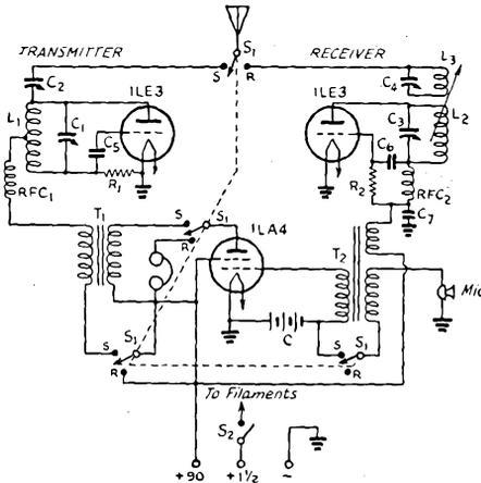
Fig. 2841 — Circuit diagram of the 112-Mc. transmitter-receiver.
