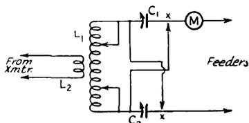
Fig. 1049 — Circuit diagram of the antenna-tuning unit.
