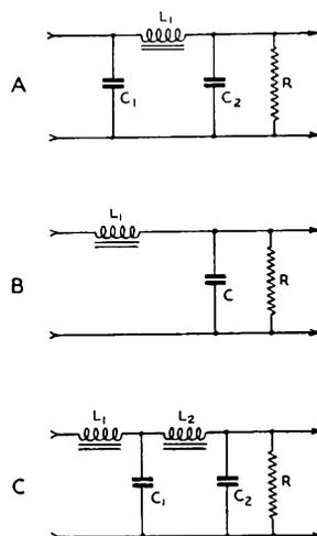
Fig. 1103 — A — Condenser-input filter. B — Choke-input filter, single section. C — Choke-input filter, double section.
