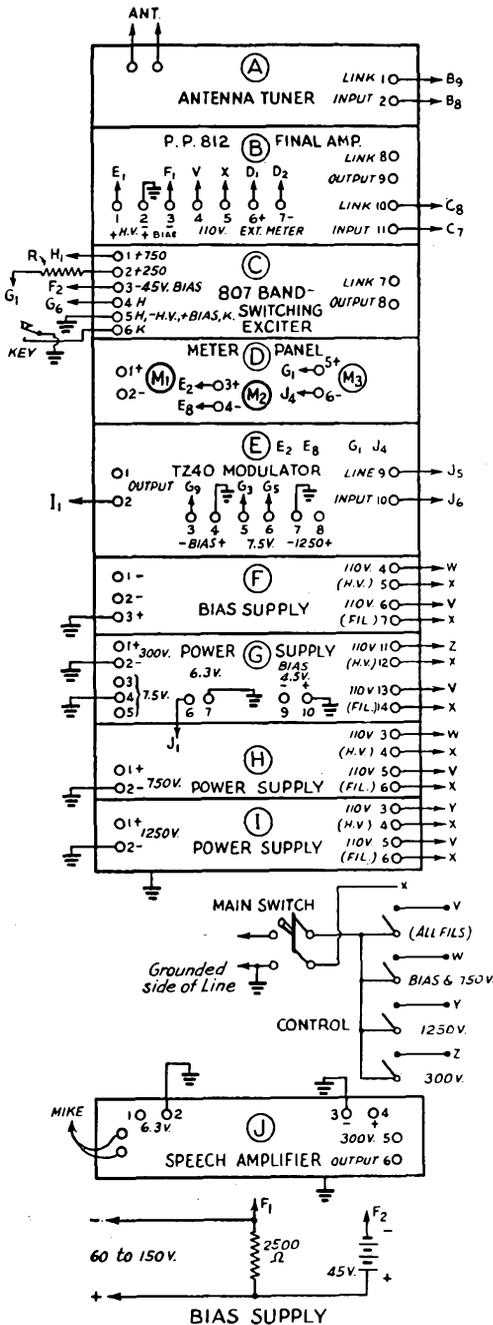
Fig. 1310 — Layout for 300-watt 'phone-c.w. transmitter.
