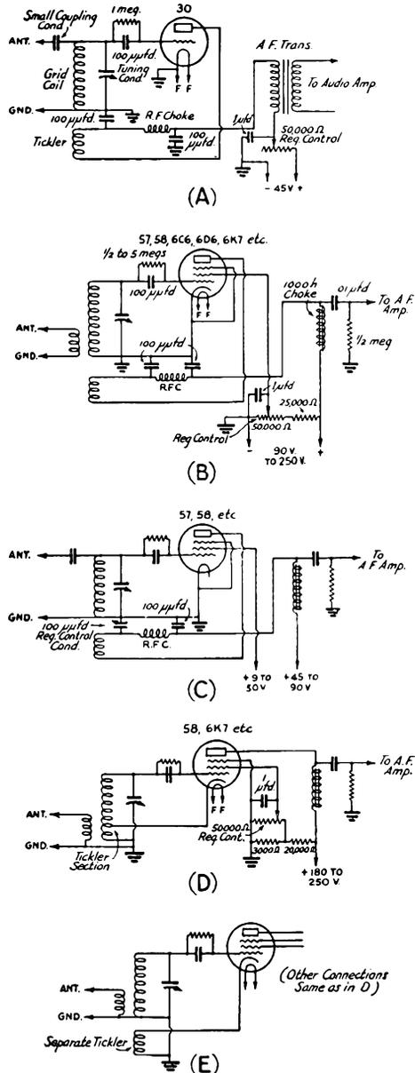
Fig. 405 — Triode and pentode (screen-grid) regenerative detector circuits.
