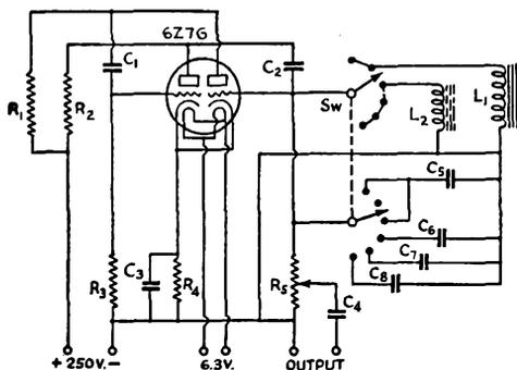
Fig. 1729 — Audio signal generator circuit diagram.
