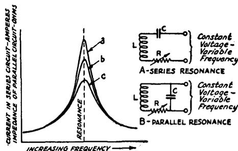
Fig. 311 — Characteristics of series-resonant and parallel-resonant circuits.
