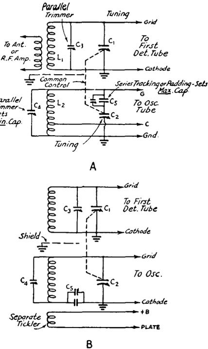
Fig. 418 — Converter circuit tracking methods. Approximate circuit values for 450- to 465-kc. intermediates with tuning ranges of approximately 2.15-to-1,  $C_1$  and  $C_2$  having a maximum of 140  $\mu\text{fd.}$  and the total minimum capacitance, including  $C_3$  or  $C_4$ , being 30 to 35  $\mu\text{fd.}$
