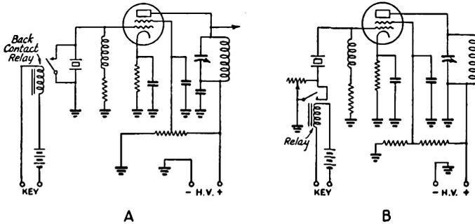
Fig. 1513 — Crystal keying circuits.
