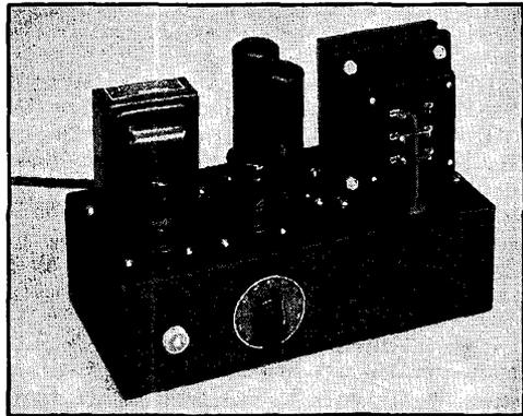
Fig. 1207 — A low-cost speech-amplifier or low-power modulator with a maximum audio output of 20 watts. The 6SJ7 is in the left near corner of the chassis, with the 6B4G to its right, just above the volume control.
