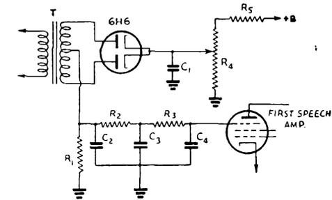
Fig. 616 — Output limiting circuit to prevent over-modulation.
