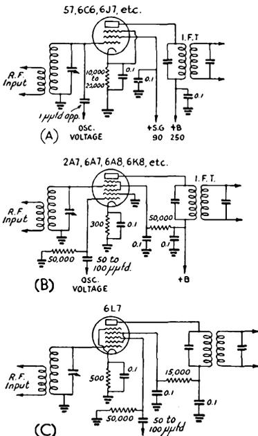
Fig. 416 — Mixer or Converter Circuits. *A*, grid injection; *B* and *C*, separate injection circuits for converter tubes. If an 1851 or 1852 is used in circuit *A*, the cathode resistor should be changed from 300 to 500 ohms.
