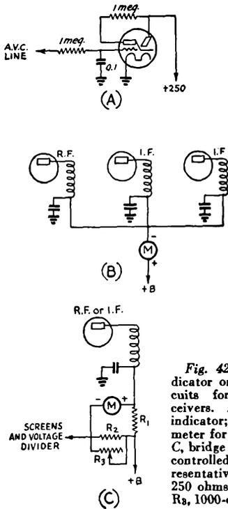
Fig. 428 — Tuning indicator or "S"-meter circuits for superhet receivers. *A*, electron-ray indicator; *B*, plate-current meter for tubes on a.v.c.; *C*, bridge circuit for a.v.c. controlled tube. In *C*, representative values are:  $R_1$ , 250 ohms;  $R_2$ , 350 ohms;  $R_3$ , 1000-ohm variable.
