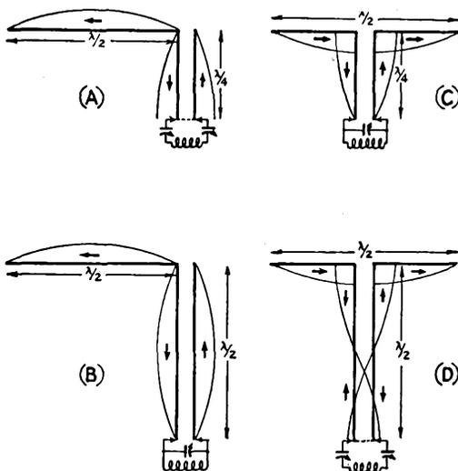
Fig. 2213 — Half-wave antennas fed from resonant lines. A and B, end feed with quarter- and half-wave lines; C and D, center feed. The current distribution is shown for all four cases.
