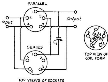
Fig. 1047 — Circuit diagram of the low-power antenna tuner.  $C_1$  is a 250- $\mu\text{fd}$ . midget variable condenser (National STH250).  $L_1$  is the antenna tuning winding, while  $L_2$  is a link input winding. Connections for series or parallel tuning are made automatically when the coil is plugged into the correct socket.
