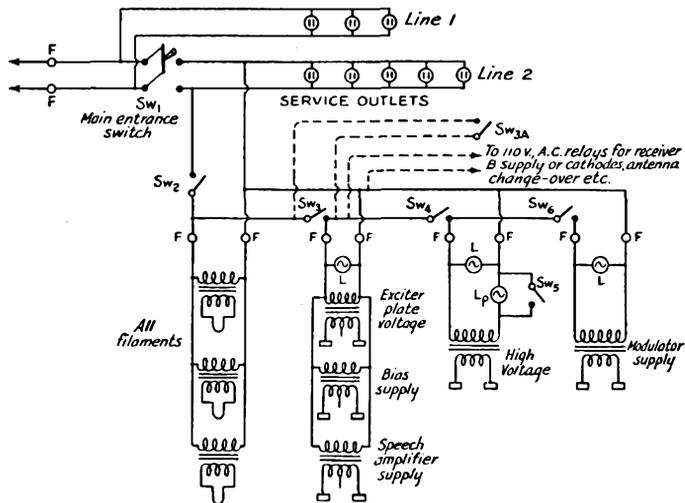
Fig. 1903 — Station control system. With all switches except  $SW_3$  closed,  $SW_3$  serves as the main control switch.  $SW_1$  — Enclosed entrance switch.  $SW_2$  — Filament switch.  $SW_3$  — Low plate-voltage and main control switch. (See text.)  $SW_4$  — High plate-voltage switch.  $SW_5$  — Low-power and tune-up switch. (See text.)  $SW_6$  — Modulator plate-voltage switch. F — Fuse. L — Warning light.  $L_p$  — Voltage-reducing lamp. (See text.)
