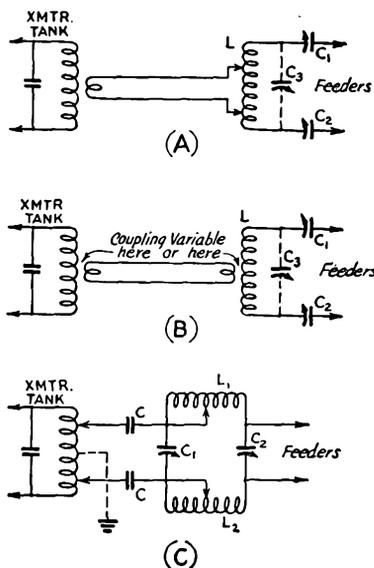
Fig. 2215 — Antenna coupling systems without movable coils. *A* and *B*, link-coupled circuits for series and parallel tuning; *C*, balanced low-pass filter. In *A* and *B*, dotted lines show connections for parallel tuning when called for; in such case the series condensers,  $C_1$  and  $C_2$ , may be set at maximum capacity or short-circuited. Constants for  $L$ ,  $C_1$ ,  $C_2$  and  $C_3$  are the same as for inductive coupling, and are discussed in the text.
