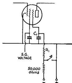
Fig. 1508 — Suppressor-grid keying. The condenser *C*<sub>1</sub> can be the usual 0.01- $\mu$ f. by-pass shunted by a larger condenser to give the proper time-constant.
