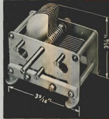
**National EMC Condensers** are made in large sizes for general purpose uses. They are similar in construction to the TMC Transmitting condenser, and have high efficiency and rugged frames. Insulation is Isolantite, and Peak Voltage Rating is 1000 Volts. Plate shape is Straight-Line Wavelength.
