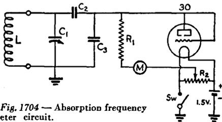
Fig. 1704 — Absorption frequency meter circuit.
