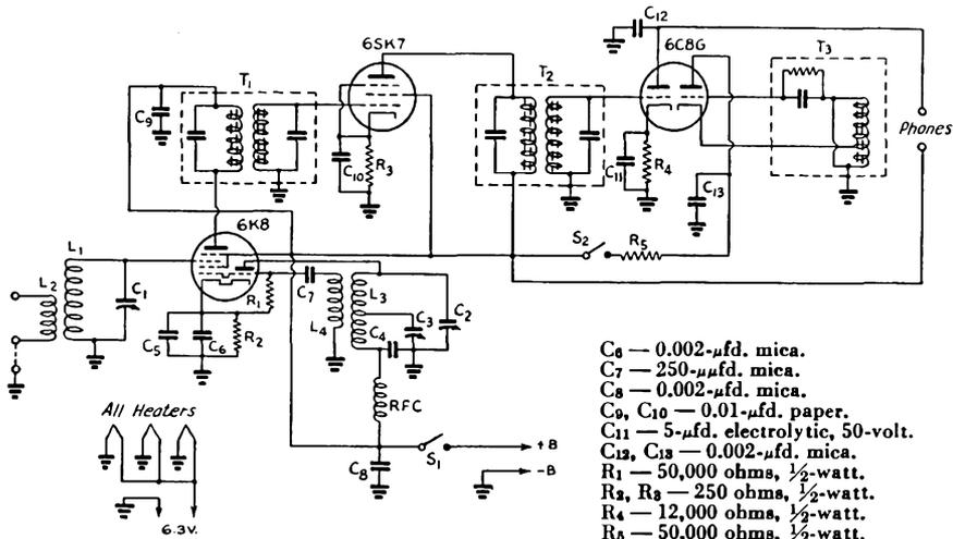
Fig. 807—The three-tube superhet wiring diagram.
