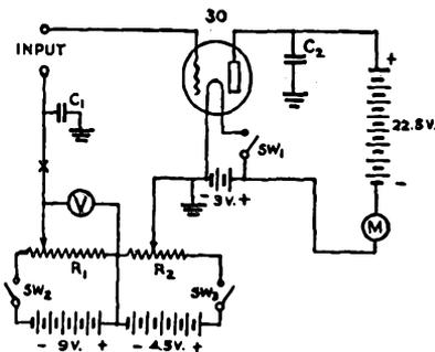
Fig. 1724 — Simple peak-type slide-back vacuum-tube voltmeter.
