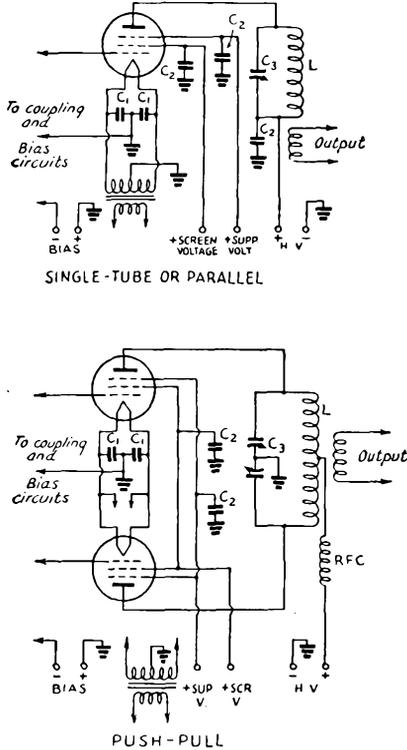
Fig. 510 — Tetrode-pentode r.f. amplifier circuits.  $C_1$  — 0.01  $\mu$ f.;  $C_2$  — 0.001  $\mu$ f. or larger;  $C_3$ -L — See section on tank-circuit design. In circuits for tetrodes, the suppressor-grid connection and by-pass are omitted.
