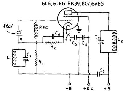
Fig. 506 — Tri-tet oscillator circuit, using pentodes or beam tetrodes.  $C_1$  and  $C_2$ , 200- $\mu\text{fd}$ . variables;  $C_3$ ,  $C_4$ ,  $C_5$ , 0.001 to 0.01  $\mu\text{fd}$ . by-passes, not critical;  $R_1$ , 20,000 to 100,000 ohms;  $R_2$ , 400 ohms for 400- or 500-volt operation.
