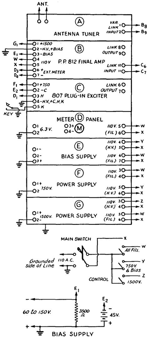
Fig. 1309 — Complete layout for 450-watt c.w. transmitter.
