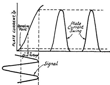
Fig. 327 — Operation of the *Class-B* amplifier.
