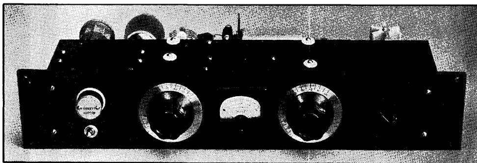
Fig. 1016 — The two-tube plug-in coil exciter is built to conserve space in the relay rack. The panel is  $3\frac{1}{2}$  in. by 19 in. A clearance hole is cut in the left end of the panel for the crystal socket which is mounted in the chassis directly above the cathode-circuit switch. The left-hand dial controls the tuning of the oscillator plate
