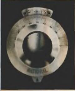
The four-inch N Dial has an engine divided scale and vernier of solid nickel silver. The vernier is flush with the scale. The planetary drive has a ratio of 5 to 1, and is contained within the body of the dial. 2, 3, 4 or 5 scale. Fits 1/4" shaft.
