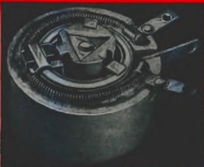
★ Left: New Clarostat Power Rheostat. Radically different. Selected resistance wire wound on insulated aluminum strip and imbedded in cold-setting inorganic cement. Ceramic casing. Graphited-copper shoe. Tripod rotor. Smooth, positive operation. Comparative tests invited. 25-watt rating. Popular resistance values.
