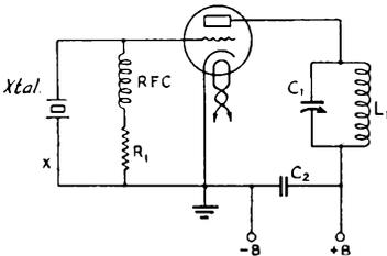
Fig. 503 — Triode crystal oscillator. The tank condenser  $C_1$  may be a 100- $\mu\text{fd.}$  variable, with  $L_1$  proportioned so that the tank will tune to the crystal frequency. (See coil charts, Figs. 516-517.)  $C_2$  should be 0.001  $\mu\text{fd.}$  or larger. The grid leak,  $R_1$ , will vary with the type of tube; high- $\mu$  types take lower values, 2500 to 10,000 ohms, while medium and low- $\mu$  types take values of 10,000 to 25,000 ohms.
