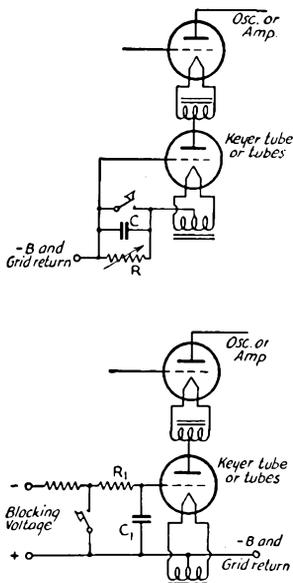
Fig. 1509 — Vacuum-tube keying. The series method is simple but does not completely cut off the current flow. It may be used in some applications where the following stage is heavily biased.  $C$  may be between 0.25 and 1.0  $\mu\text{fd}$ . Resistor  $R$  should be adjusted to cause the plate current to drop to a minimum when the key is open. A variable resistor of 50,000 ohms should give enough range.
