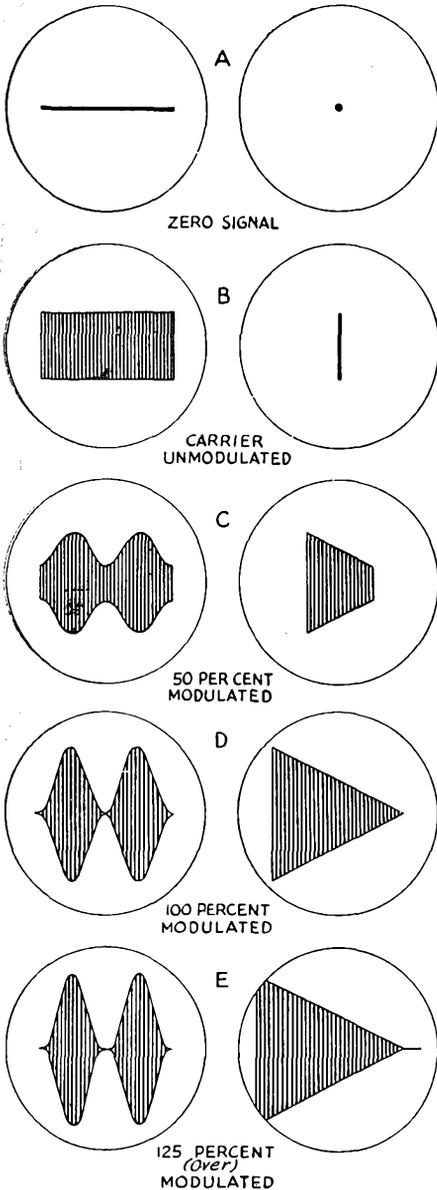
Fig. 1603 — Wave-envelope (left) and trapezoidal (right) oscilloscope patterns.
