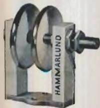
Improved neutralizing condensers with heavy polished aluminum plates. Rounded edges. Isolantite. Fine adjusting screw. Positive lock. Horizontal adjustment. Type "N-10", 2 1/2" high x 1-3/16" deep. "N-15" 4-15/16" high x 3 1/2" deep. "N-20", 5-11/16" high x 4" deep.
