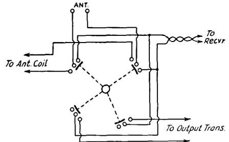
Fig. 821 — The converter antenna switch wiring diagram.
