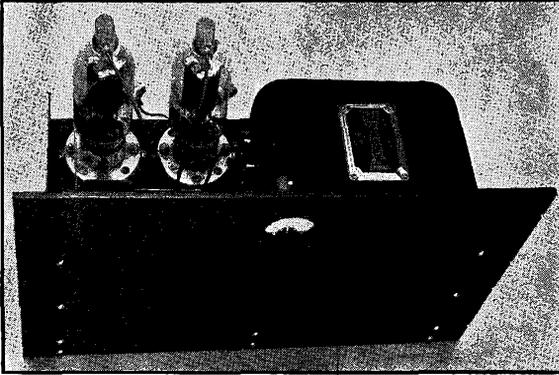
*Fig. 1226* — With high-power modulators, components become so large that chassis space is at a premium in relay-rack construction. There is, however, room for either the input transformer or a filament transformer on the chassis. See Fig. 1224 for discussion of meter mounting.
