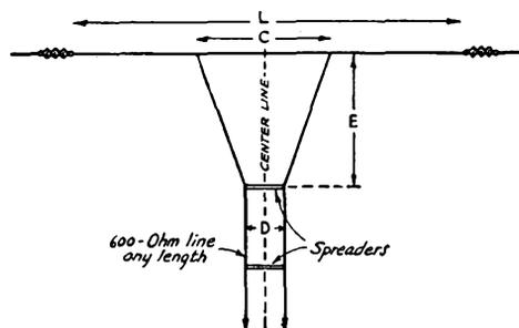
Fig. 2208 — Two-wire matched-impedance antenna system. The dimensions *C*, *D*, and *E* are given in the text. It is important that the matching section, *E*, come straight away from the antenna without any bends. *L* is one-half wavelength for the operating frequency.
