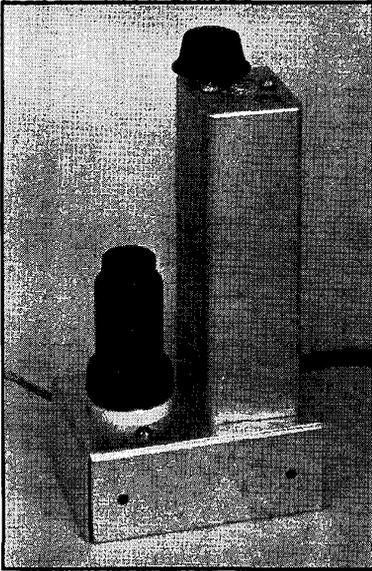
Fig. 825 — Top view of the beat oscillator assembly.
