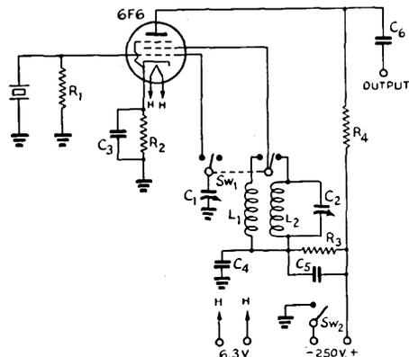
Fig. 1712 — Crystal calibrator circuit diagram.
