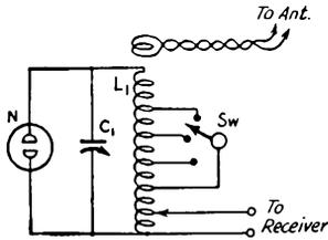
Fig. 1904 — Simple protective device for receiver. When the voltage induced across  $L_1$   $C_1$  by transmitter becomes too great, the neon tube breaks down, short-circuiting the tuned circuit.  $L_1$  and  $C_1$  are any coil and condenser which will tune over the required range. Bare wire is suggested for  $L_1$  so that adjustment of the taps will be simplified.
