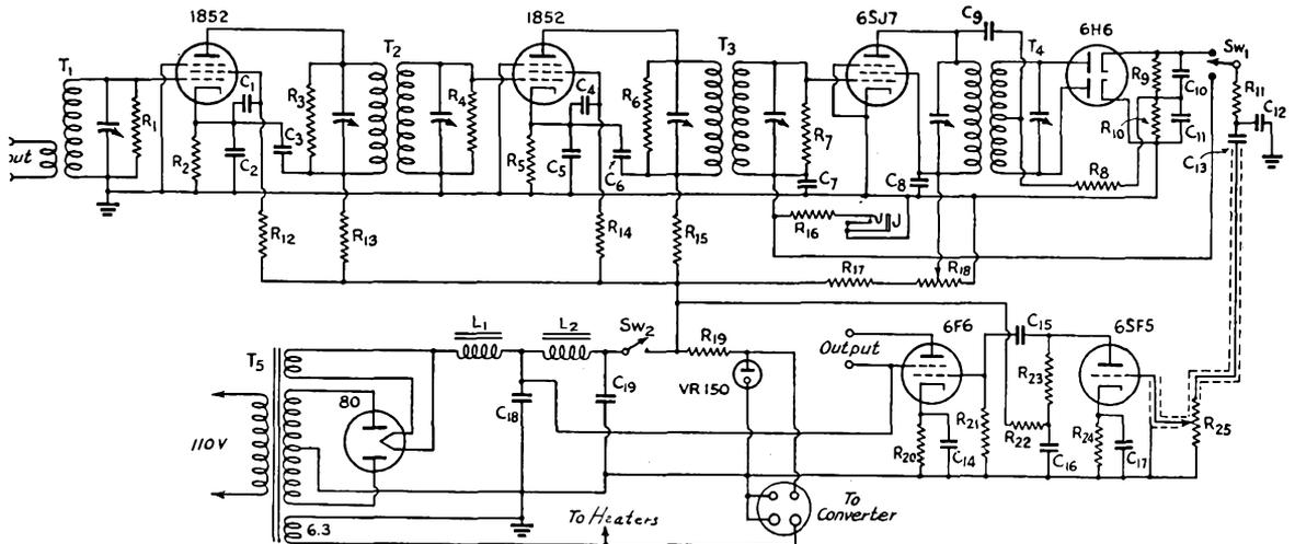
Fig. 2914 — Wiring diagram of the 5-Mc. f.m./a.m. amplifier.
