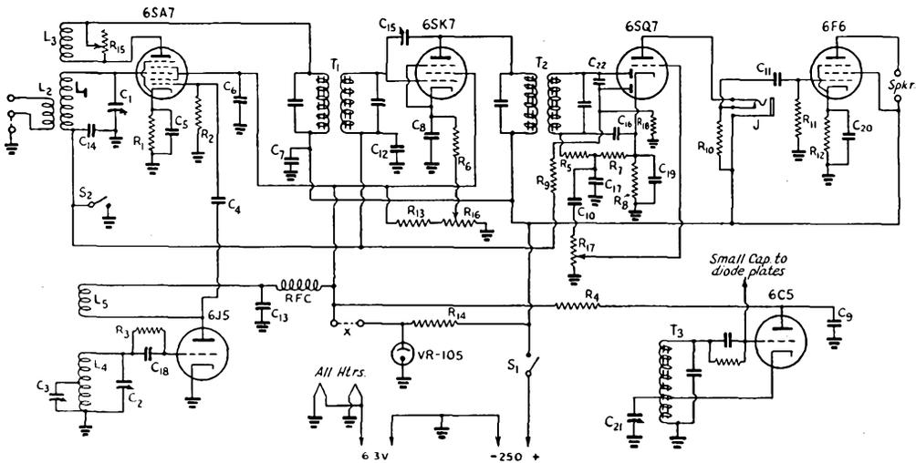
Fig. 815 — Circuit diagram of the regenerative superhet.
