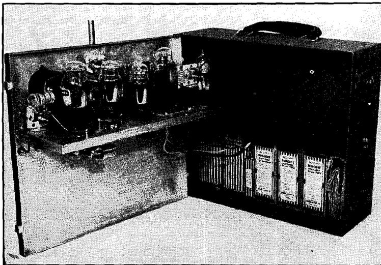
The tubes used have 6.3-volt heaters, which may seem a bit odd in a unit intended for dry-battery operation. This, however, was a matter of necessity rather than choice — necessity, that is, if sure-fire and non-critical operation
