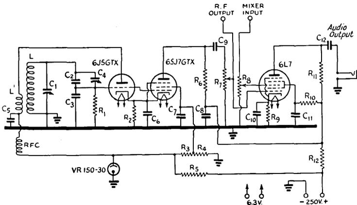
**Fig. 1707** — Circuit diagram of the stable frequency meter.
