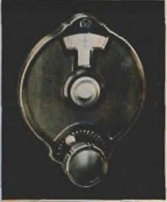
"Velvet Vernier" Dial, Type B, has a compact variable ratio 6 to 1 minimum, 20 to 1 maximum drive that is smooth and trouble free. An illuminator is available. The case is black bakelite. 1 or 5 scale. 4" diam. Fits 1/4" shaft.
