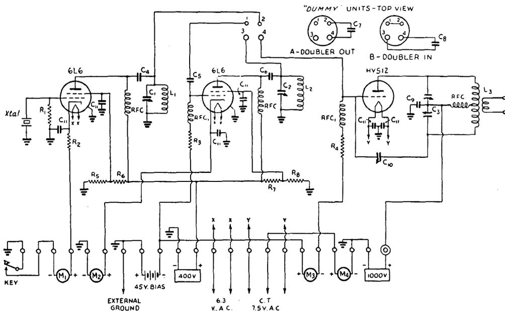
Fig. 1026 — Circuit diagram of 100- to 175-watt transmitter.
