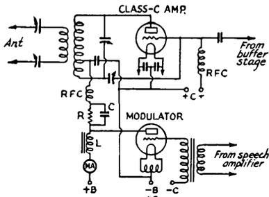
Fig. 606 — Choke-coupled or Heising plate modulation.
