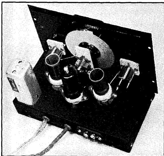
Fig. 822 — Top view of the converter.  $L_1$  and  $L_2$  are to the right and left of the 6K8. The output transformer stands at the left. The power-cable output leads and antenna terminals may be seen along the rear wall of the chassis.
