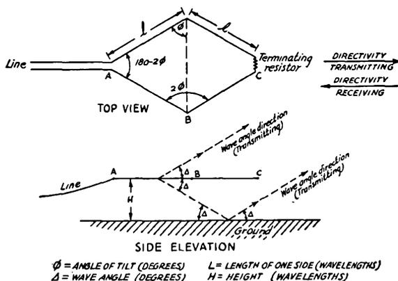
Fig. 2314 — The horizontal rhombic — or diamond antenna, terminated.
