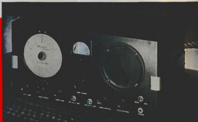
Specifically designed for marine service, in the range from 16.2 to 2150 meters (18.2 mc to 110 kc). Improved image rejection at the higher frequencies is achieved through the use of 1600 kc IF Transformers. The directly calibrated main tuning dial eliminates the use of complicated charts and tables. An efficient mechanical bandspread with separate dial provides easy logging.
