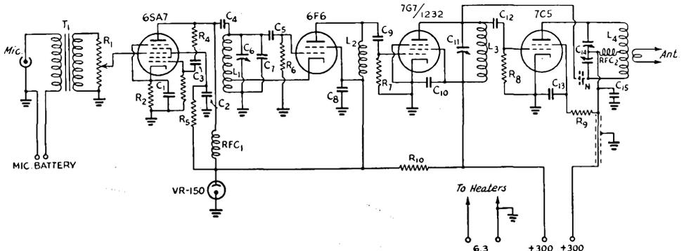
Fig. 2906 — Wiring diagram of the 56-Mc. f.m. transmitter.
