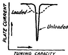
Fig. 1402 — D.C. plate current vs. plate tuning capacity with the Tri-tet oscillator.
