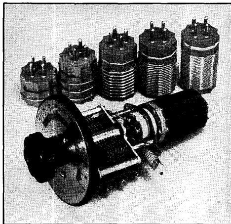
*Fig. 1701 — Simple absorption frequency meter. A coil socket — a condenser — a dial plate mounted on an insulating disc which also serves as a handle — a flashlight bulb on a bracket — and a set of coils. Indispensable for identifying harmonics, locating parasitics, checking oscillators.*
