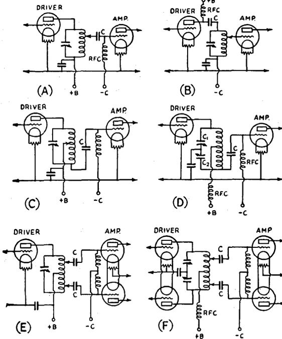
Fig. 508 — Direct- or capacity-coupled driver and amplifier stages. Coupling condenser capacity may be from 50  $\mu\text{fd.}$  to 0.002  $\mu\text{fd.}$ , not critical, except when tapping the coils for control of excitation is not possible.
