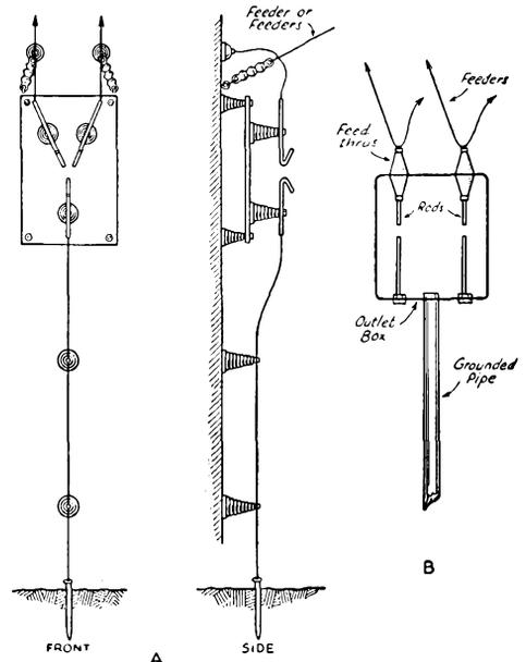
Fig. 1914 — Low-loss lightning arrestors for transmitter installations.
