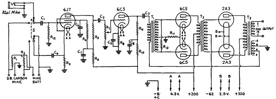
Fig. 1214 — Circuit diagram of the 15-watt speech amplifier.
