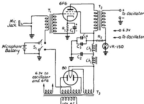
Fig. 1202 — A 4-watt modulator and associated power supply.
