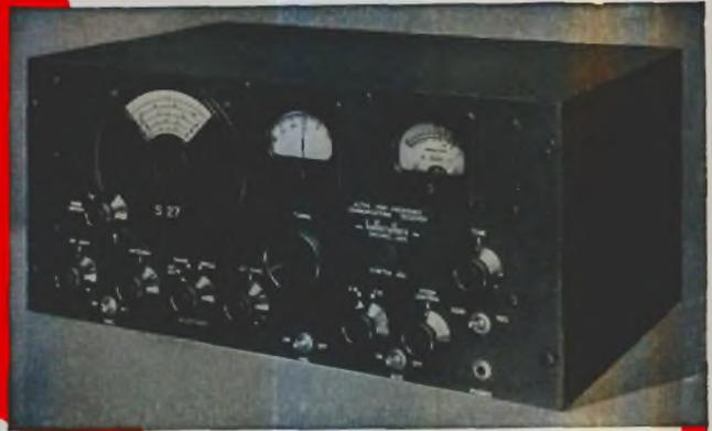
15 Tubes. 3 bands: 27 to 46 mc; 45 to 84 mc; 81 to 145 mc; Switch changing from FM to AM reception. Uses Acorn, 1852, and Beam Power tubes. Controls are: R.F. gain control. Band switch. Antenna trimmer. I.F. selectivity control and power switch. Volume, Pitch,
