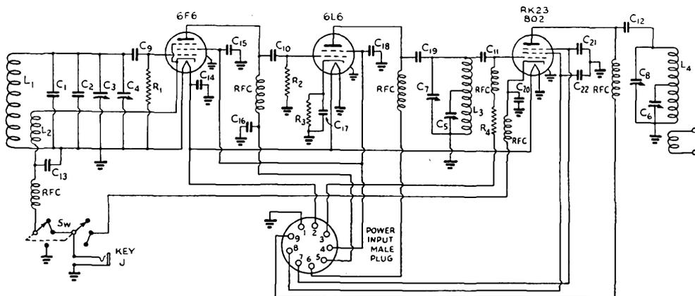
Fig. 1011 — Circuit diagram of the e.c.o. exciter.
