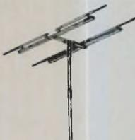
The elements consist of corrosion proof aluminum alloy tubes ADJUSTABLE to all frequencies between 80 mcs. and 40 mcs. mounted on high grade low absorption glazed porcelain standoff insulators which maintains its efficiency under all weather conditions. Light but rugged construction is met by the strong wooden supports. Complete with mounting poles and steel clamping.
