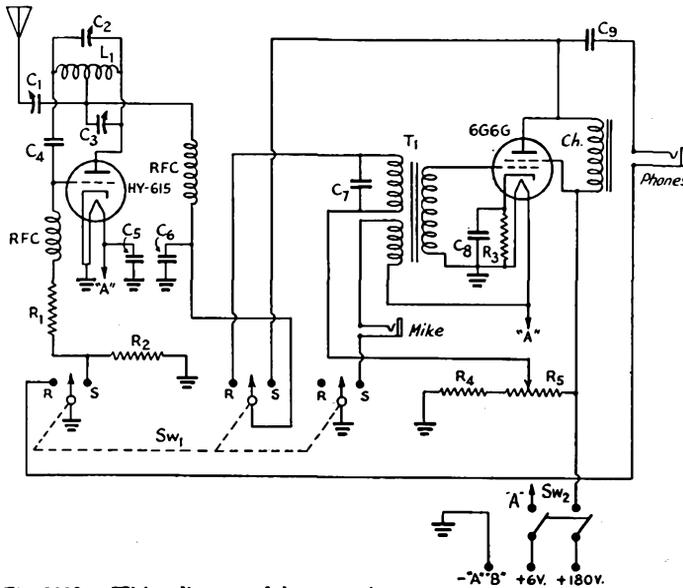
Fig. 2838 — Wiring diagram of the transceiver.
