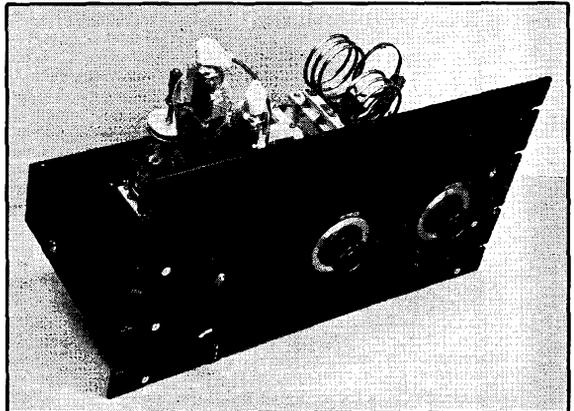
rating of 450 watts. It is intended that the amplifier will be driven by an exciter similar to the one shown in Figs. 2801-2804.
