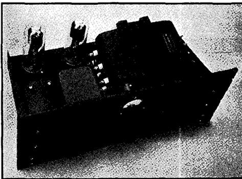
*Fig. 1224* — A chassis arrangement for a higher-power Class-B modulator. This unit has a filament transformer for the tubes mounted on the chassis, as well as the input and output transformers. In cases where the input transformer is included with the speech amplifier, less chassis space is needed. The tubes are placed to the rear where ventilation is good.
