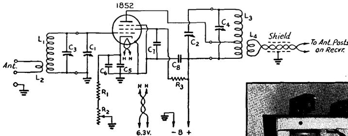
Fig. 829 — Circuit diagram of the preselector.
