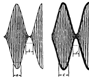
from the output of the modulator rather than from a preceding stage of the audio system. Fig. 1606 is a photograph of the pattern which resulted when the sweep voltage for a trapezoidal pattern was obtained from the output of the audio driver stage instead of the output of the modulator.
