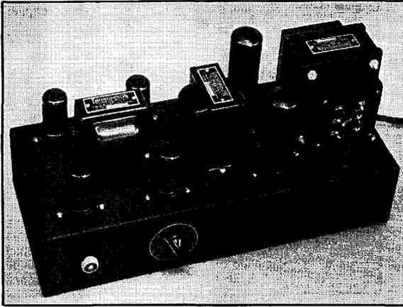
Fig. 1210 — A 40-watt speech amplifier or modulator of inexpensive construction. The 6SJ7 and first 6J5 are at the front, near the microphone socket and volume control, respectively. T<sub>1</sub> is just behind them, and the push-pull 6J5's are at the rear of the chassis behind T<sub>1</sub>. T<sub>2</sub>, the 6L6's, and T<sub>3</sub> follow in order to the right.
