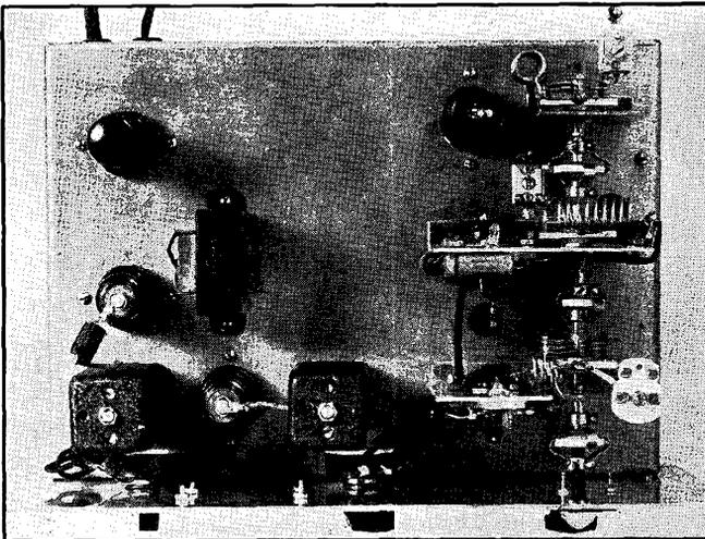
*Fig. 2716* — Plan view of the 56-Mc. superhet. The r.f. section, at right, is separated from the i.f. amplifier, second detector and audio amplifier. The acorn mixer and oscillator tubes are mounted on aluminum partitions.
