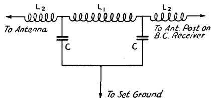
Fig. 1520—A low-pass filter for reduction of interference with broadcast reception. It should be installed at the receiver. Constants are as follows:  $L_1$ , 54 turns of No. 24 d.s.c. on  $1\frac{1}{8}$ -inch diameter form;  $L_2$ , 33 turns same; C, 500  $\mu\text{fd}$ . fixed. Cut-off frequency is approximately 1600 kc.
