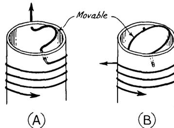
Fig. 413 — Methods of adjusting inductance for ganging. The half turn in *A* can be moved so that its magnetic field either aids or opposes the field of the coil. The shorted loop in *B* is not connected to the coil, but operates by induction. It will have no effect on the coil inductance when the plane of the loop is parallel to the axis of the coil, and will give maximum reduction of the coil inductance when perpendicular to the coil axis.
