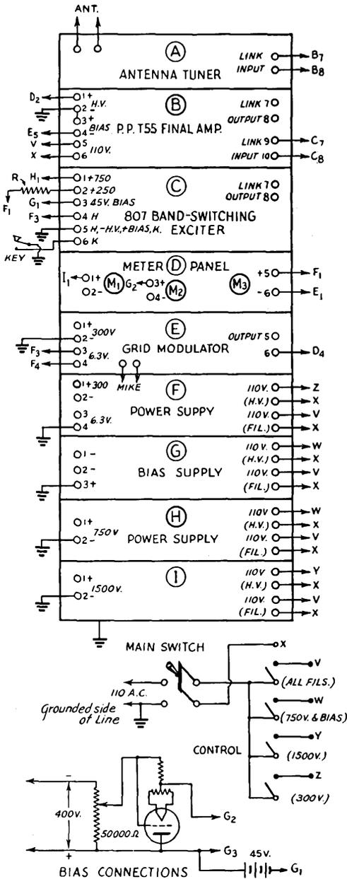
Fig. 1308 — Complete layout of grid-modulated phone-c.w. transmitter.
