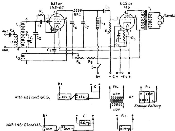
Fig. 803 — Wiring diagram of the two-tube receiver.
