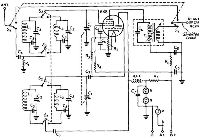
Fig. 2711 — Circuit diagram of the 28-56-Mc. mobile converter.
