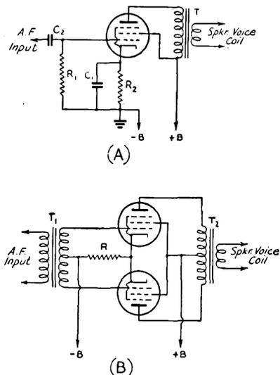
Fig. 408 — Audio power output amplifier circuits.
