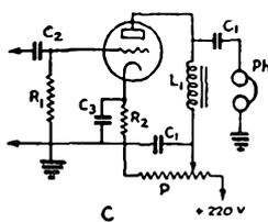
Fig. 424 — Output limiter circuits.
