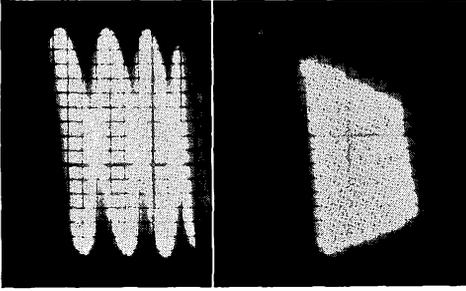
Fig. 1607 and Fig. 1608 — Wave-envelope and trapezoidal patterns which lean because of r.f. coupling between vertical and horizontal deflection circuits.
