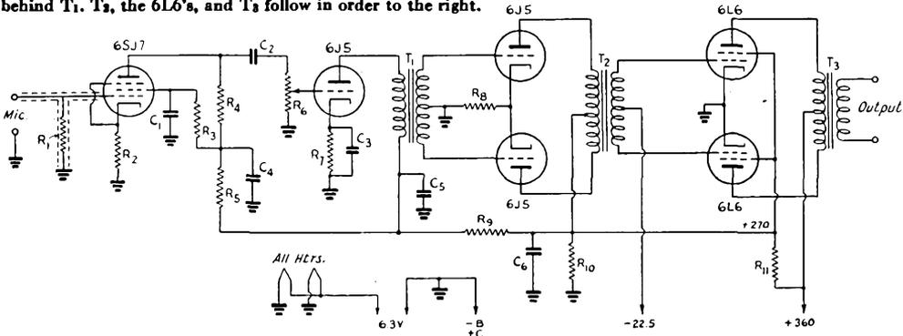
Fig. 1211 — Circuit diagram of the 40-watt speech amplifier-modulator.
