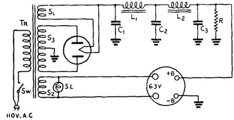
Fig. 1121 — Circuit diagram for receiver power supplies.
