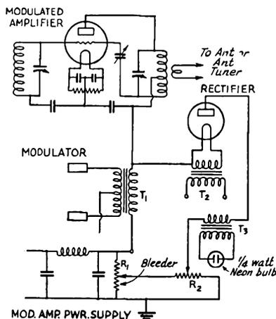
Fig. 1601 — A negative-peak modulation-per cent and overmodulation indicator.
