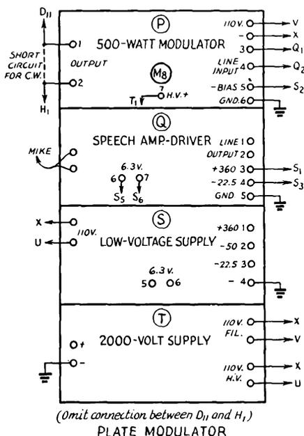
Fig. 1314A — Plate modulator for 1-kw. transmitter.
