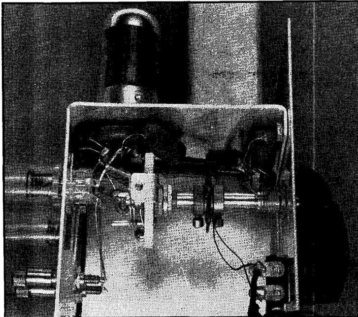
Fig. 2705 — The mixer circuit can be seen when the side panel is removed, giving an idea of the placement of the parts. The tie strip at the lower right takes the output leads from the transformer. The through-hushing can be seen just to the left of the tuning condenser, with a wire from it running to the 1232 grid.
