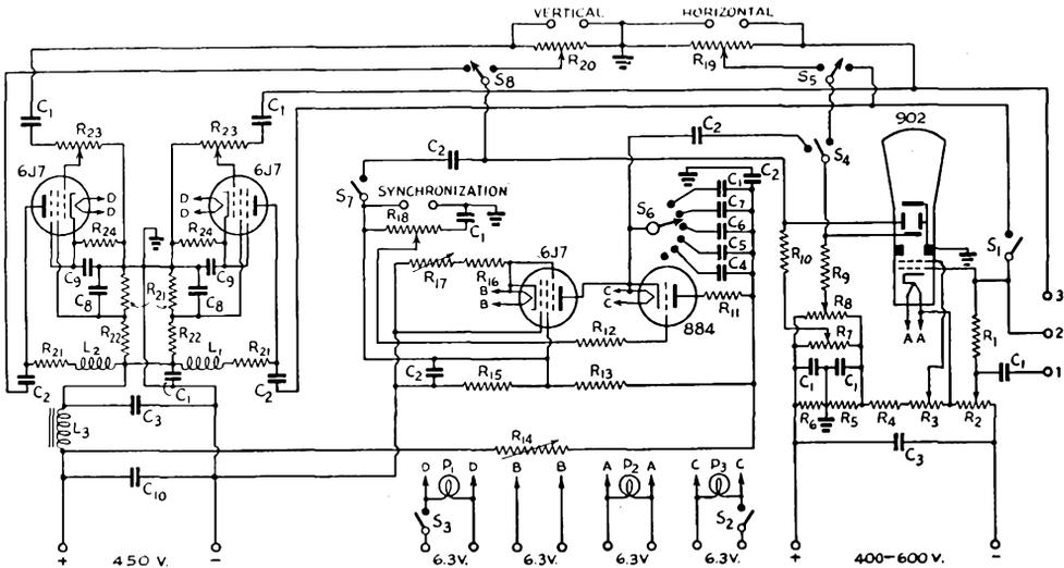
Fig. 1733 — Complete circuit diagram of sweep-circuit oscilloscope.
