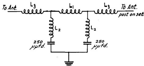
Fig. 1521—Circuit diagram of sharp cut-off low-pass filter.
