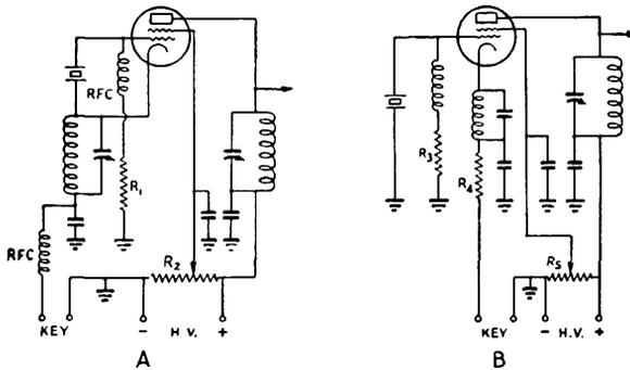
Fig. 1511 — Cathode keying for tri-tet oscillator. Typical values for 6L6:  $R_1$  — 50,000 ohms;  $R_2$  — 20,000 ohms. B — Cathode keying for grid-plate oscillator. Typical values for 6L6:  $R_3$  — 50,000 ohms;  $R_4$  — 400 ohms;  $R_5$  — 20,000 ohms.
