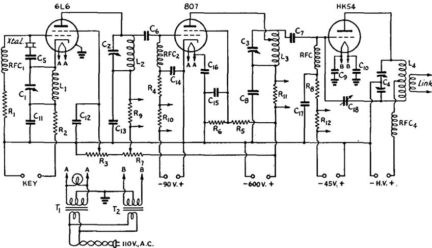
Fig. 2803 — Wiring diagram of the 6L6-807-HK-54 exciter.
