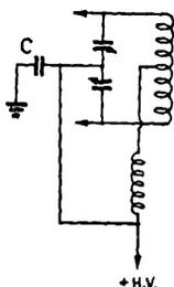
Fig. 515 — Use of blocking condenser permits smaller plate spacing with split-stator condensers.  $C$  should have a capacity of 0.001 to 0.002  $\mu\text{f.}$  and a voltage rating 3 to 4 times the d.c. voltage. Condenser control must be suitably insulated.
