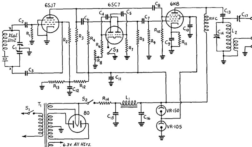
Fig. 1715 — Circuit diagram of the frequency standard.
