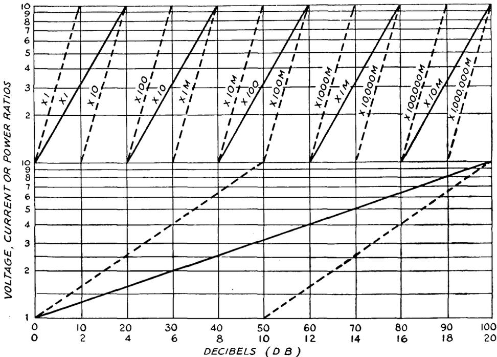
cessive gains and losses expressed in db can be added algebraically. If the ratio of the two power values is greater than 1 there is a power gain; if the ratio is less than 1 there is a loss of power. A gain is expressed in "plus db"; a loss in "minus db."
