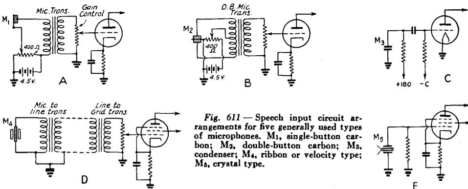
Fig. 611 — Speech input circuit arrangements for five generally used types of microphones.  $M_1$ , single-button carbon;  $M_2$ , double-button carbon;  $M_3$ , condenser;  $M_4$ , ribbon or velocity type;  $M_5$ , crystal type.
