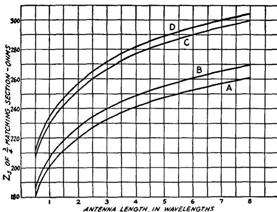
Fig. 2307 — Required surge impedance of quarter-wave matching sections for radiators of various lengths. Curve A is for a transmission line impedance of 440 ohms, Curve B for 470 ohms, Curve C for 580 ohms and Curve D for 600 ohms.
