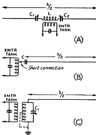
Fig. 2201 — Methods of direct feed to the half-wave antenna. *A*, current feed, series tuning; *B*, voltage feed, capacity coupling; *C*, voltage feed with inductively coupled antenna tank. In *A*, the coupling apparatus is not included in the antenna length.
