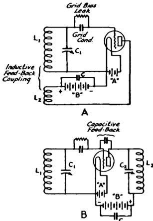
Fig. 330 — Two general types of oscillator circuits.
