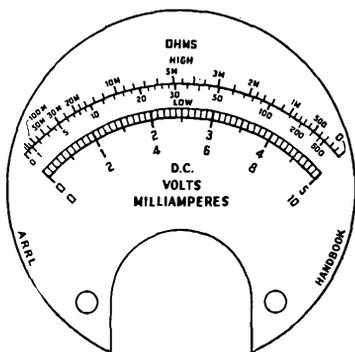
Instrument scale for inexpensive volt-ohm-milliammeter, to be cut out and pasted over existing scale of Triplett No. 221 0-1 ma. milliammeter or any equivalent 2-inch meter with 33 ohms internal resistance. Calibration should be checked with standard of moderate accuracy after assembly, to allow for variations in individual meters, inaccuracies in multipliers, resistance of test leads, paper shrinkage, etc.
