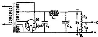
Fig. 1112 — A practical circuit for the "C" supply. A single 8- $\mu$ f. condenser often will suffice for the filter but if trial shows that more is needed, a choke and second condenser, shown in dotted lines, may be added. The condensers should be rated at 500 volts, especially if the "C" supply is to be used on a high-power stage where the excitation is likely to be large.
