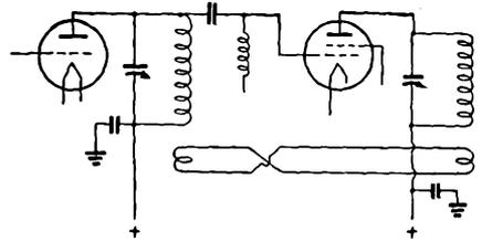
Fig. 1404 — Link neutralizing for tetrodes and pentodes, such as 6L6, 6V6 and other tubes sometimes difficult to neutralize by other methods. The link coils should have one or two turns and should be coupled to the "cold" ends of the tank coils. Neutralization is adjusted by moving the link coils in relation to the tank coil. Reversal of connections to one of the coils may be required.
