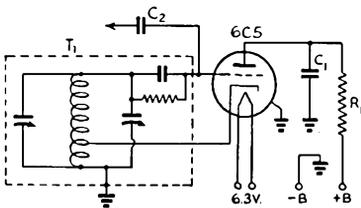
Fig. 826 — Circuit diagram of the beat frequency oscillator.
