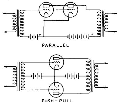
Fig. 325 — Parallel and push-pull amplifier connections.
