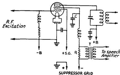
Fig. 608 — Suppressor-grid modulation of a pentode r.f. amplifier.
