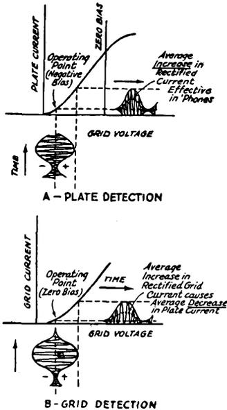
Fig. 332 — Operating characteristics of plate and grid detectors.
