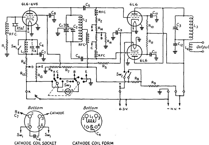
Fig. 1008 — Circuit diagram of the two-stage 6L6 transmitter.
