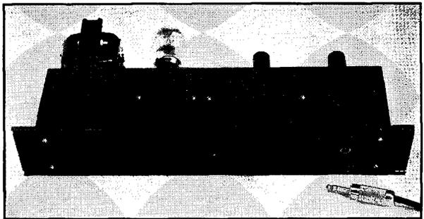
Fig. 1204 — Relay-rack mounting amplifier with 3-watt output.
