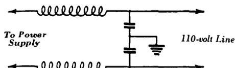
Fig. 1516 — R.f. filter for the power line.
