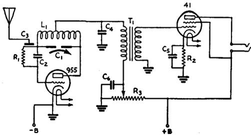
Fig. 2721 — Circuit of an "Acorn" receiver.
