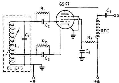
**Fig. 1709 — Circuit of the e.c. band-setting oscillator.**
