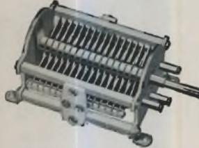
Compact types, Isolantite insulation. Base or panel mounting. Polished aluminum plates. Stainless steel shaft. Size of 150 mmf. with .070" plate spacing only 4 1/2" behind panel. All type "B" condensers have round edge plates .025" in thickness. Type "C" has plain edge plates .025" thick. Self-cleaning wiping contact.
