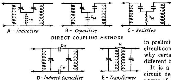
Fig. 316 — Basic types of circuit coupling.
