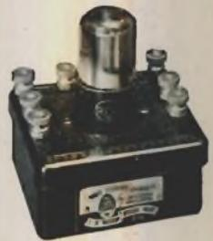
Same pretty plastic cabinet as Model A-700. A remarkably good audio oscillator giving a beautiful clear 1000 cycle note. Uses 1 1/2 volt for A battery and 2 1/2 volts or 45 volts B battery depending upon volume desired. Terminals: 2 right for key; 2 left for phones or speaker. Rear terminals, left to right: B plus, B minus; A plus, A minus.
