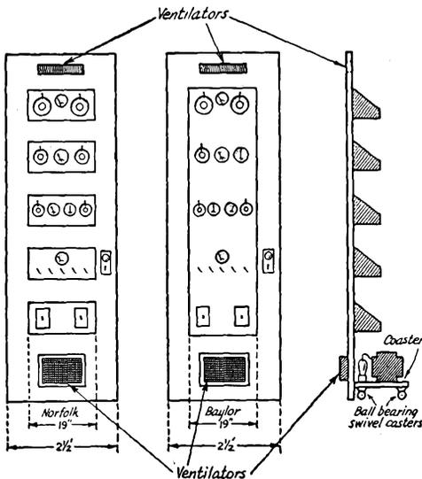
Fig. 1901—Transmitter mounted on clothes-closet door. Standard rack construction may be followed. Weight of heavy units is taken up by rollers at bottom. The door may be replaced at little expense.
