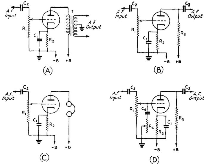
Fig. 407 — Audio amplifier circuits for voltage amplification and headphone output.
