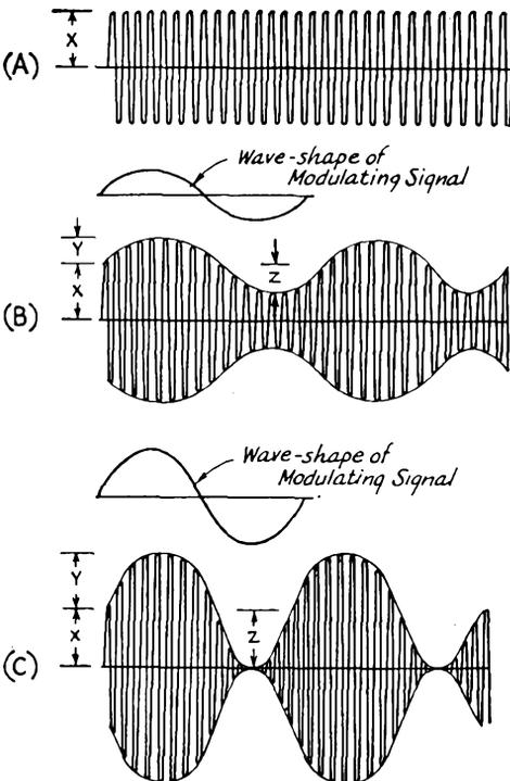
Fig. 602 — Graphical representation of (A) unmodulated carrier wave, (B) wave modulated 50%, (C) wave modulated 100%.
