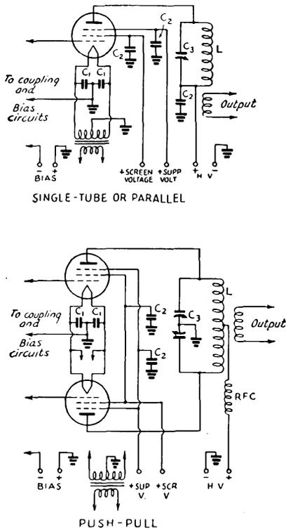
Fig. 510 — Tetrode-pentode r.f. amplifier circuits.  $C_1$  — 0.01  $\mu\text{f.}$ ;  $C_2$  — 0.001  $\mu\text{f.}$  or larger;  $C_3$ -L — See section on tank-circuit design. In circuits for tetrodes, the suppressor-grid connection and by-pass are omitted.
