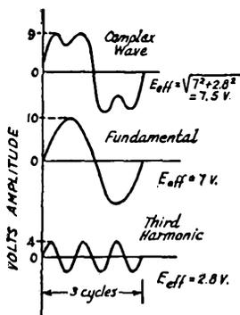
Fig. 319 — A complex wave and its sine-wave components.
