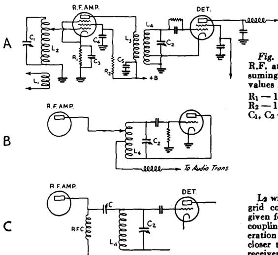
Fig. 2726 — Three effective methods of coupling an R.F. amplifier to the superregenerative detector. Assuming that the r.f. amplifier is a 954 acorn, suitable values for the various components marked will be:
