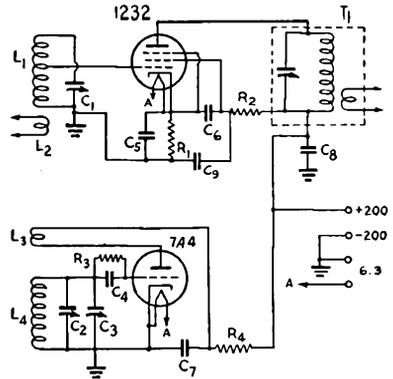
5 Mc.: 45 turns No. 30 d.s.c. closewound; coupling coil is 14 turns No. 30 d.s.c. closewound  $\frac{1}{8}$  inch from ground end of coil.
