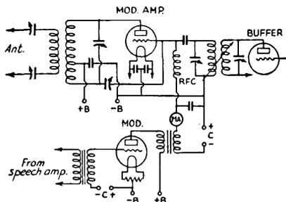
Fig. 607 — Grid-bias modulation of a Class-C amplifier.
