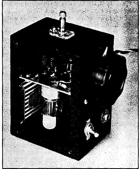
*Fig. 2717* — A 112-Mc. receiver using 1.4-volt tubes, mounted in a 5- by 4- by 3-inch can. The tuning knob, phone jack and battery switch are seen on the front panel — the binding post on top takes the antenna. Note the C battery mounted in the can.
