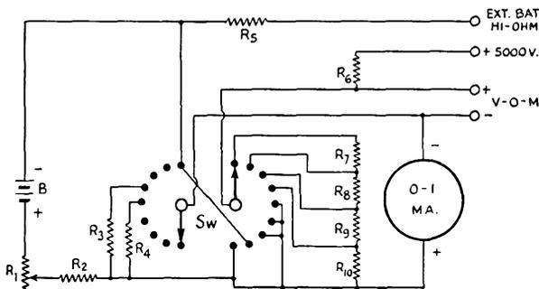
so that very little current will be drawn in making voltage measurements. A voltmeter taking considerable current will give inaccurate readings when connected across a high-resistance source, as is often the case in checking voltages at various parts of a receiver cir-
