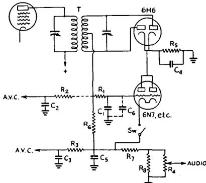
Fig. 426 — Automatic noise limiting circuit for superhet receivers.
