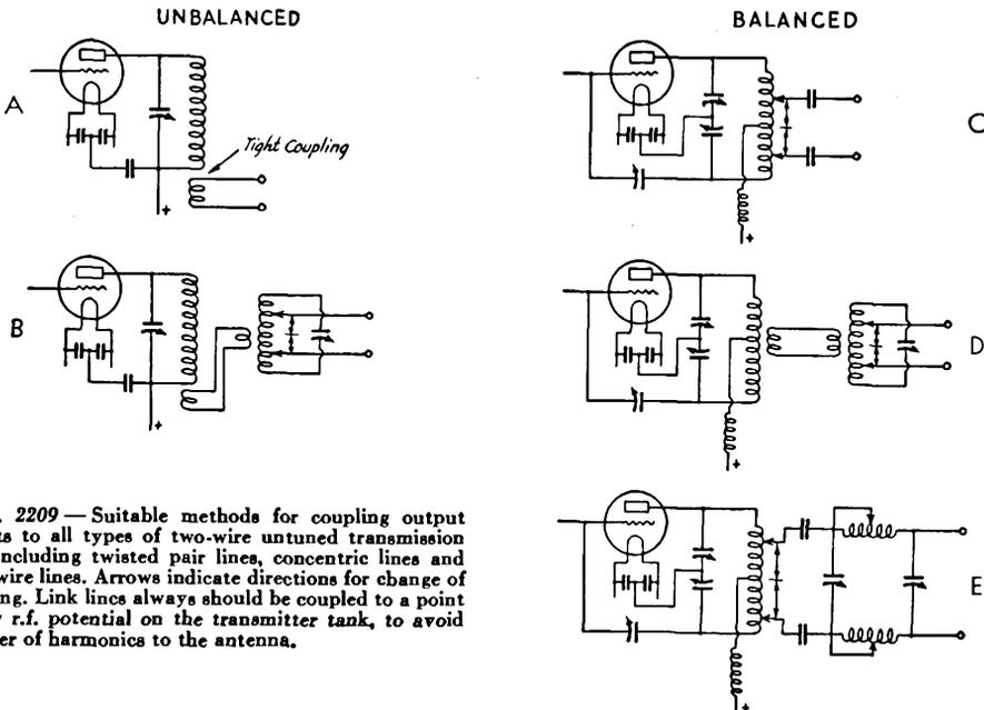
Fig. 2209 — Suitable methods for coupling output circuits to all types of two-wire untuned transmission lines including twisted pair lines, concentric lines and open wire lines. Arrows indicate directions for change of coupling. Link lines always should be coupled to a point of low r.f. potential on the transmitter tank, to avoid transfer of harmonics to the antenna.
