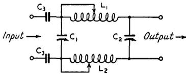
Fig. 1054 — Diagram of pi-section antenna coupler.  $C_1$ - $C_2$  — 300  $\mu\text{fds.}$ , 0.07-in. spacing (National TMC-300).  $L_1$ - $L_2$  — 26 turns No. 14, 2½-in. diameter, 3½-in. long (National XR10A form wound full).  $C_3$  — 0.01- $\mu\text{fd.}$  mica, 5000 volts.
