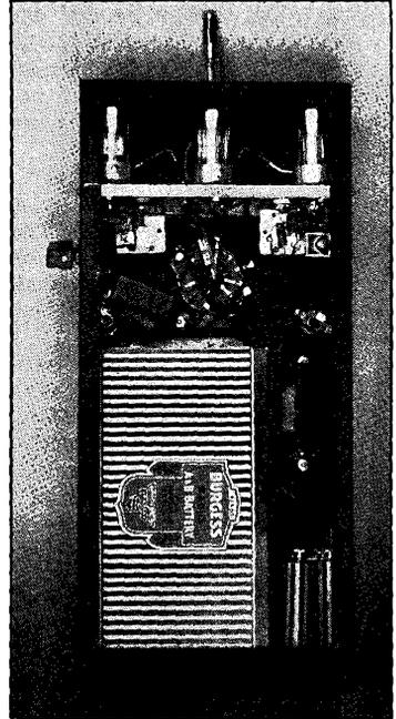
Fig. 2842 — The rear view of the transmitter-receiver shows the position of the batteries and the sub-chassis which supports the tubes and tuning condensers.
