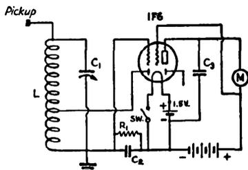
Fig. 1727 — The two-stage field-strength meter circuit diagram.
