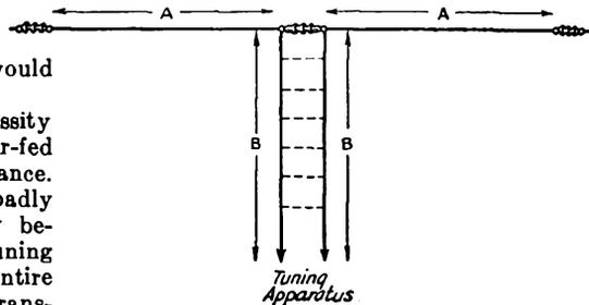
Fig. 2310 — Practical arrangement of a shortened antenna. The total length  $A + B + B + A$ , should be a half-wavelength for the lowest-frequency band, usually 3.5 Mc. See Table II for lengths and tuning data.
