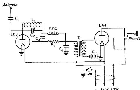
Fig. 2718 — Circuit diagram of the 112-Mc. battery receiver.
