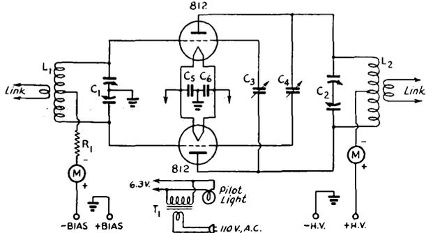
inch diam. Coil is made in 2 sections each section having 3 turns; 1 $\frac{1}{2}$ -inch space between sections (Barker and Williamson 10TVL).
