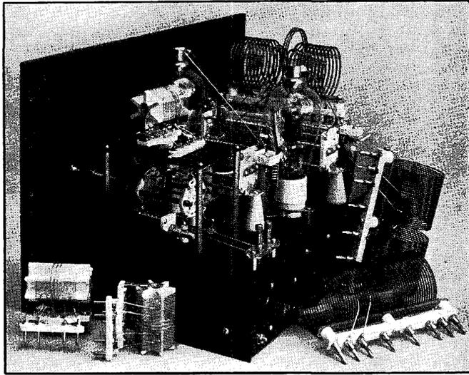
Fig. 1040 — Grid-circuit end of hand-switching push-pull amplifier showing switching arrangement and the 1.75-Mc. paddler.
