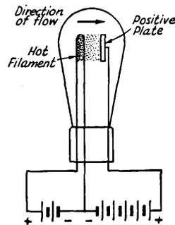
Fig. 305 — Illustrating conduction by thermionic emission of electrons in a vacuum tube. One battery is used *only* to heat the filament to a temperature where it will emit electrons. The other battery places a positive potential on the plate, with respect to the filament, and the electrons are attracted to the plate. The flow of electrons completes the electrical path, and current flows in the plate circuit.
