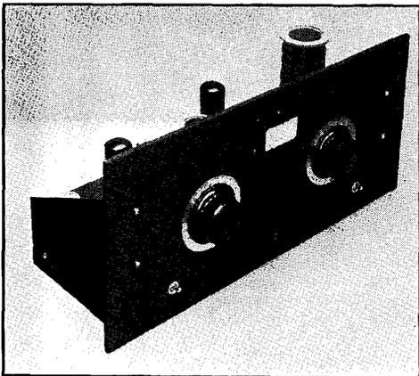
Fig. 1006 — The panel of the two-stage 6L6 transmitter is  $8\frac{3}{4}$  by 19 inches. The toggle switch at the left is  $SW_1$  and the one at the right  $SW_2$ . The meter switch is below the meter.
