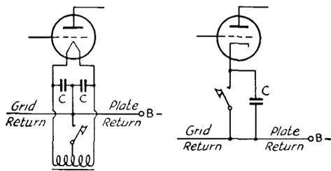
Fig. 1507 — Center-tap keying. Keying for filament type tubes is shown at the left and for cathode types at the right. The by-pass condensers, *C*, should be about 0.001  $\mu$ f. and capable of withstanding full plate voltage. They are necessary to furnish an r.f. return to ground. Full plate voltage appears across the key, so a relay should be substituted for the key if high voltages are used.
