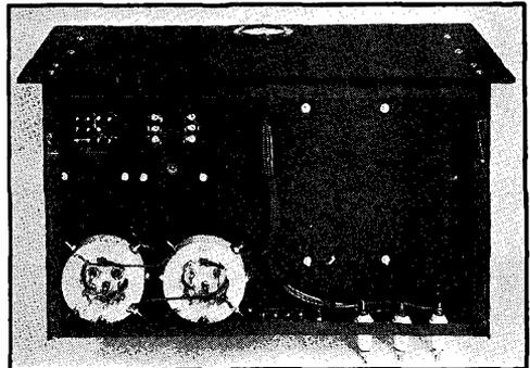
*Fig. 1225* — Bottom view of the modulator of *Fig. 1224*. Mounting the sockets below the chassis saves panel height and conceals the wiring. The output terminals should be protected as described in connection with *Fig. 1222*.
