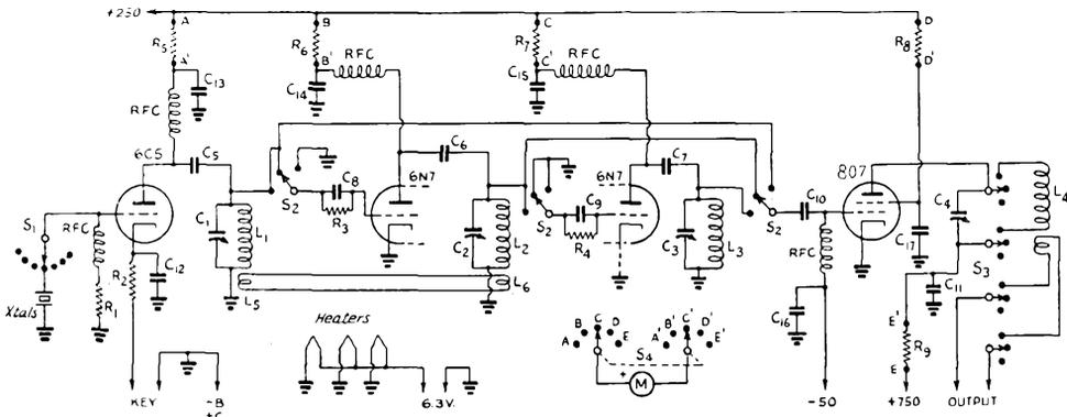
Fig. 1022 — Circuit diagram of the 807 band-switching exciter.
