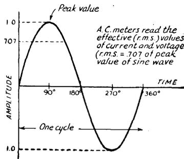
Fig. 308 — Representing sine-wave alternating current and voltage.
