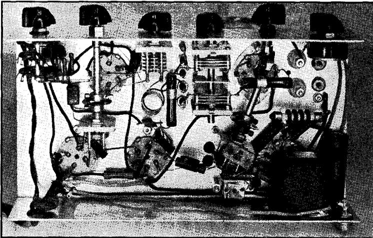
Fig. 2911 — A view underneath the chassis shows the location of parts. The microphone transformer is at the lower right, right next to the microphone connector. The small 3- $\mu$ fd. condenser used in the modulator can be seen to the left of the transformer, and directly above is the oscillator tuning condenser. The power cable runs out the back of the set at the lower left-hand corner; the twisted pair taken out the same hole goes to the meter.
