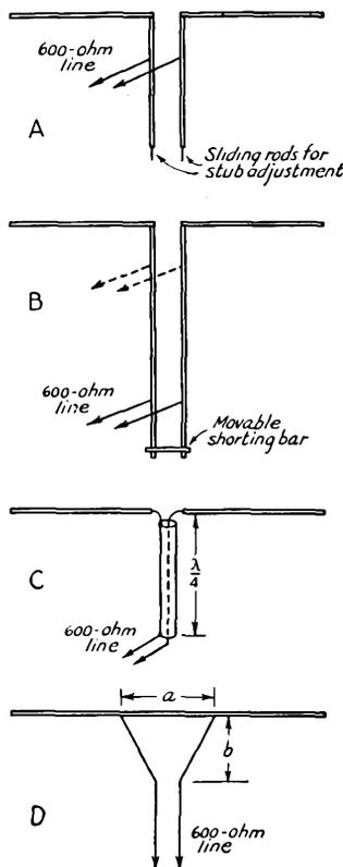
Fig. 2409 — Recommended methods of feeding the driven antenna element in close-spaced parasitic arrays. The parasitic elements are not shown. A, quarter-wave open stub; B, half-wave closed stub; C, concentric-line quarter-wave matching section; D, delta matching transformer.
