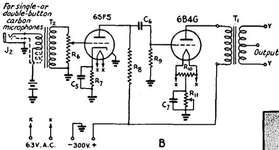
Fig. 1205 — Circuits of the 3-watt speech unit.
