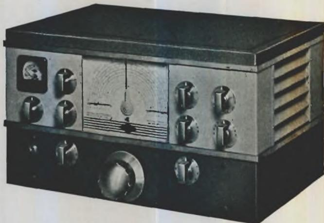
circuits of the audio power stage thus providing maximum battery economy. The B supply filter and the standby switch are wired to the battery terminals, so that the filter is available for vibrator or dynamotor B supplies.
