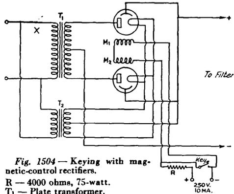
Fig. 1504 — Keying with magnetic-control rectifiers.
