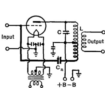
FIG. 27 F. A plate-neutralized r.f. amplifier circuit
