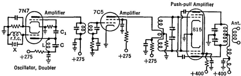
FIG. 37 E. Circuit diagram of an u.h.f. transmitter
