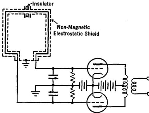
FIG. 34 J. A balanced and shielded loop
