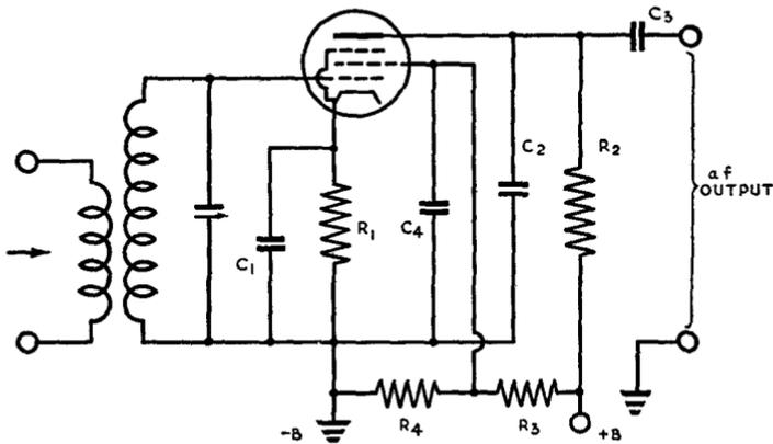
FIG. 17 G. A pentode plate detector
