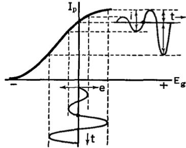
FIG. 23 D. Rectifier action on the upper knee of a triode
