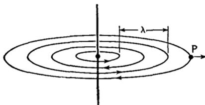
FIG. 8 B. A radiating magnetic field
