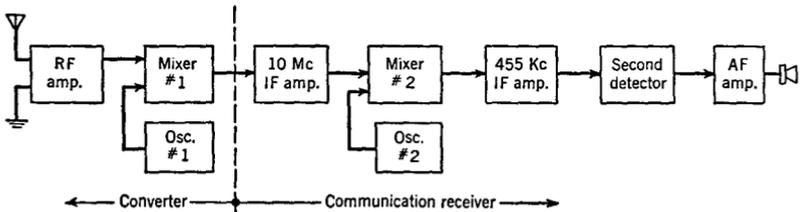
Fig. 37 A. Block diagram of a 5-meter, double-superheterodyne receiver
