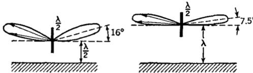
FIG. 8 G. High- and low-angle radiations from vertical half-wave Hertz antennas one-half and one wave-length above the ground
