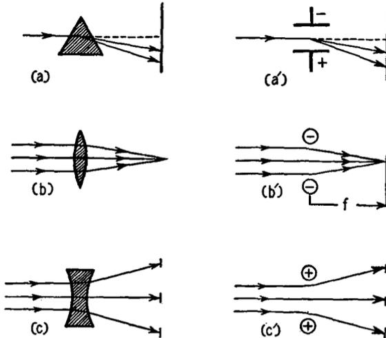
FIG. 21 A. A comparison of light rays passing through glass systems (on the left) with cathode rays in electrostatic fields (on the right). (From E. & N. P.)
