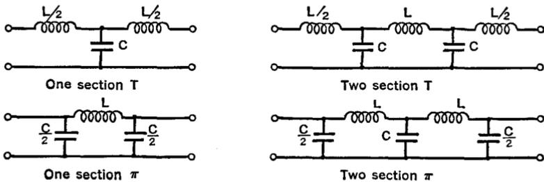
FIG. 7 E. — T- and  $\pi$ -type, low-pass filters
