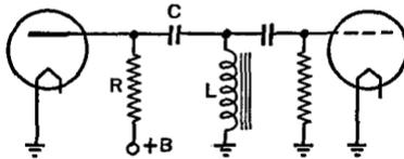
FIG. 25 F. Coupling unit for an impedance-coupled a.f. amplifier using parallel plate feed
