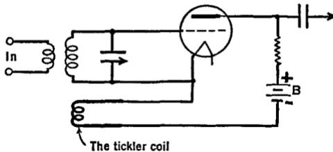
FIG. 13 N. A simple feedback amplifier
