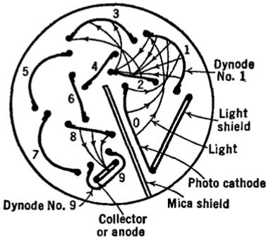
FIG. 20 M. The R.C.A. 931 multiplier phototube
