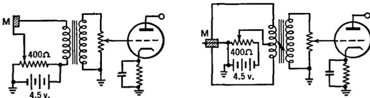
FIG. 25 J. Speech input circuits for carbon-button microphones
