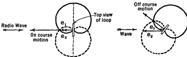
FIG. 34 M. Principle of a homing device
