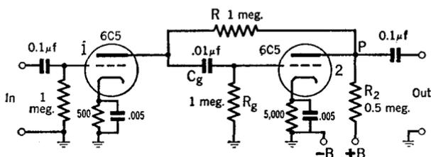
FIG. 30 G. Biased-tube method of producing pulses
