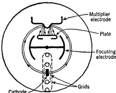
FIG. 15 I. An orbital beam multiplier tube
