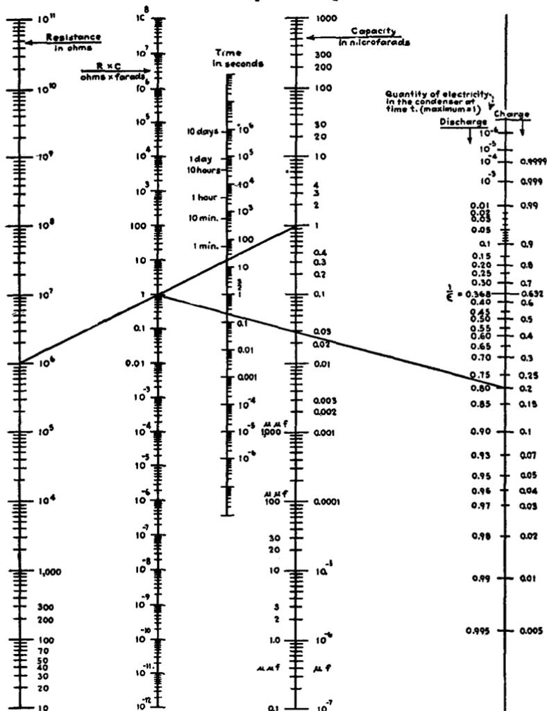
FIG. 3 J. From *Electronics*, Sept. 1937. *Instructions for use:* Connect resistance and capacitance values to obtain  $RC$  product. Connect  $RC$  product and time values to obtain quantity of electricity (charge) in condenser at the end of given time value. Example: One microfarad and one megohm gives  $RC$  product of unity. At the end of 0.2 second, the condenser is 20 per cent charged or 80 per cent discharged
