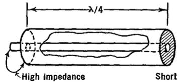
FIG. 36 H. A concentric resonant-line
