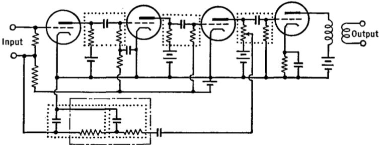
FIG. 26 G. An  $R$ - $C$  coupled feedback amplifier
