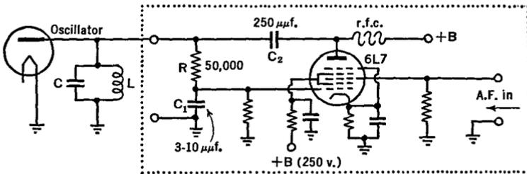
FIG. 33 B. A reactance modulator
