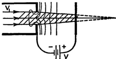
FIG. 21C. A single-aperture electron lens. (From E. & N. P.)
