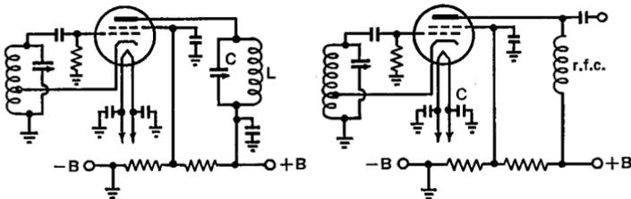
FIG. 29 A. Electron-coupled oscillator circuits
