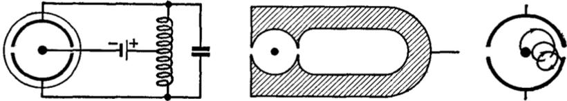
FIG. 38 F. The split-anode magnetron
