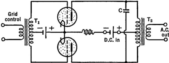
FIG. 19 N. The inverter changes d.c. to a.c.
