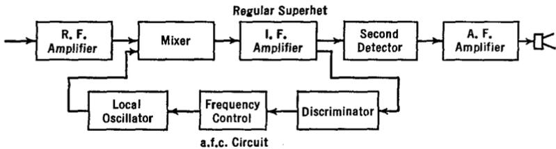
FIG. 32 T. Block diagram for automatic-frequency control
