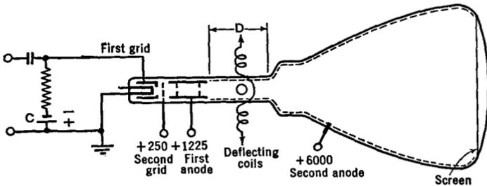
FIG. 21 L. A kinescope (No. 1804)
