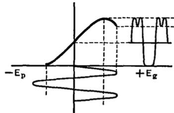
FIG. 23 F. Grid current distortion
