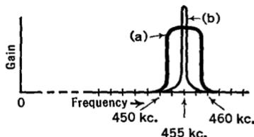
FIG. 27 B. I. F. band widths
