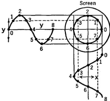
FIG. 22 Q. A circle is obtained when the two waves have the same amplitude and frequency but are in phase quadrature ( $90^\circ$ )
