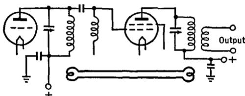
FIG. 27 H. Inductive neutralization of a r.f. amplifier
