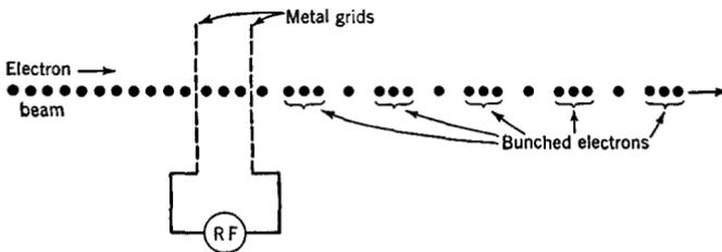
FIG. 38 I. Velocity modulation of a cathode ray
