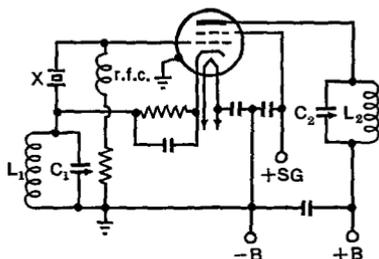
FIG. 29 H. A tri-tet oscillator circuit
