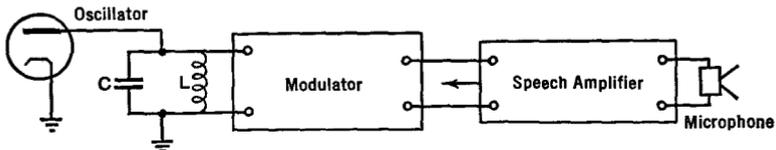
FIG. 33 A. Principle of a reactance modulator
