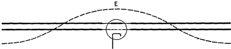
FIG. 38 B. Double tuning of a B-K oscillator
