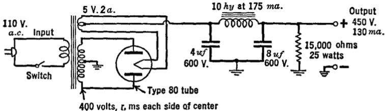
FIG. 11 H. A typical rectifier circuit
