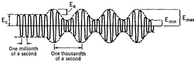
FIG. 16 C. An amplitude-modulated carrier wave
