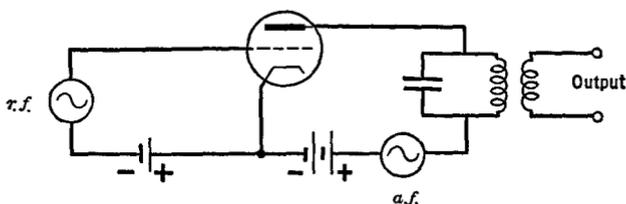
FIG. 16 F. Elementary circuit for plate modulation
