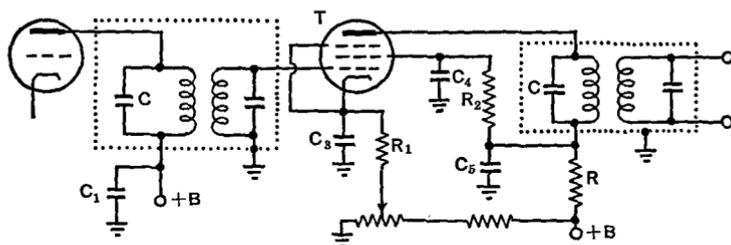
FIG. 27 C. A one-stage i.f. amplifier.  $T$  = variable-mu pentode. Typical values;  $C_1, C_3, C_4, C_5 = 0.1 \mu\text{fd}$  at 455 kc. ( $= 0.01 \mu\text{fd}$  at 1600 kc. or higher);  $R_1 = 300$  ohms;  $R_2 = 0.1$  megohm;  $R = 2000$  ohms
