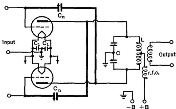
FIG. 27 I. Neutralization of a push-pull amplifier
