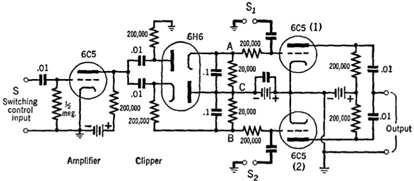
FIG. 30 N. An electronic switch
