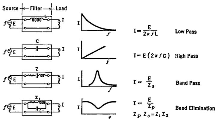
FIG. 7 C. Crude filters. Low-pass types use series inductance (top figure). High-pass use series capacitance. Band-pass use series  $LC$  circuits. Band-elimination use parallel  $LC$  circuits (bottom figure)
