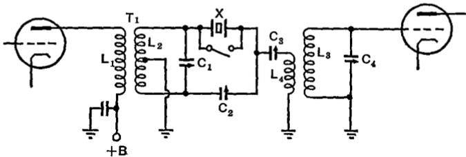
FIG. 27 D. A crystal-filter circuit.  $T_1$  = center-tapped i.f. input transformer with high- $L$ , primary closely coupled to secondary.  $C_1$  and  $C_3$  =  $100 \mu\text{mf}$ .  $C_2$  =  $10$  to  $15 \mu\text{mf}$ .
