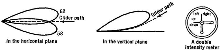
FIG. 34 R. Glider path and indicator for instrument landing
