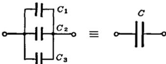
The diagram shows three capacitors labeled C1, C2, and C3 connected in parallel between two terminals. This is shown to be equivalent to a single capacitor labeled C. To the right of the diagram is the formula:
