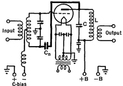
FIG. 27 G. A grid-neutralized r.f. amplifier circuit
