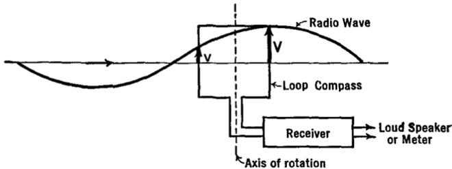
FIG. 34 A. Directional principle of a loop antenna
