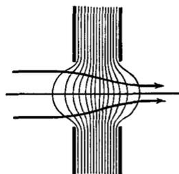
FIG. 21 D. A two-aperture lens
