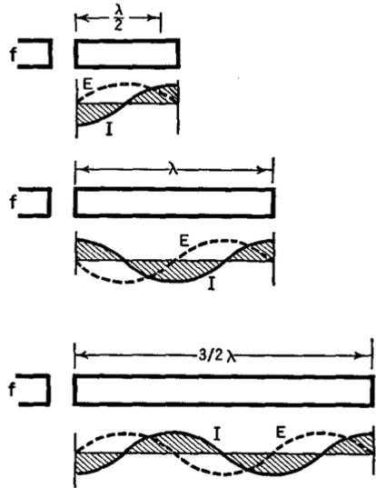
FIG. 36 D. Tuning a short-line to an oscillator of fixed frequency
