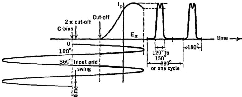
FIG. 27 J. Operation of Class C amplifiers
