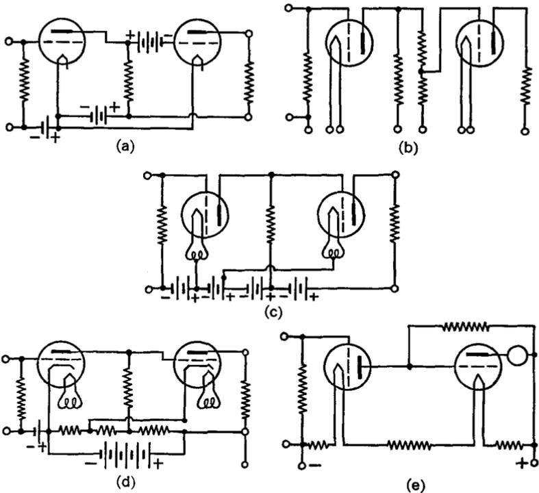
FIG. 24 E. Simple forms of multistage d.c. amplifiers
