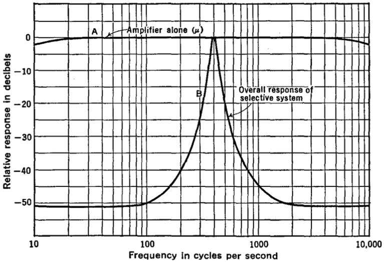
FIG. 26 L. Response curve of the circuit of Fig. 26 K
