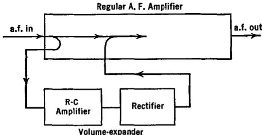
FIG. 32 S. Block diagram of a volume expander
