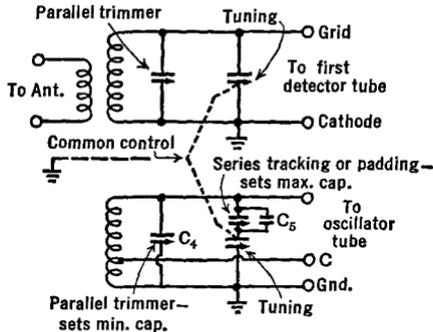
FIG. 32 M. Tracking a converter
