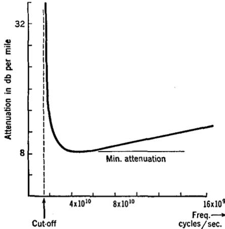
FIG. 38 R. Loss in a square wave-guide,  $H_{01}$  waves
