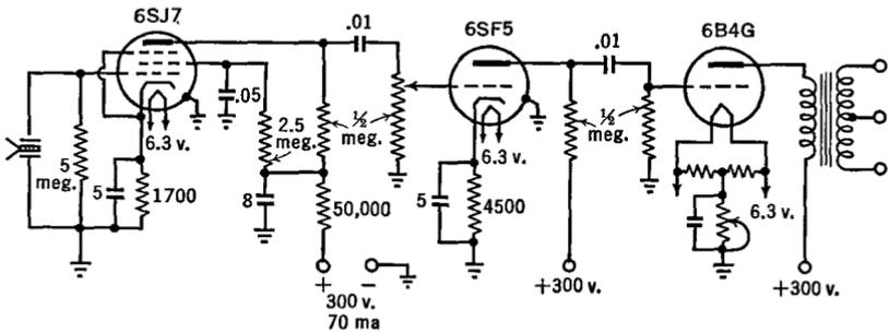
FIG. 25 P. A speech amplifier suitable for crystal microphones
