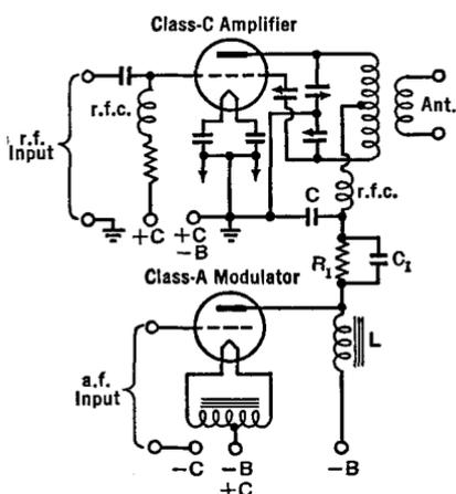
FIG. 28 B. Choke-coupled plate-modulation of a r.f. amplifier
