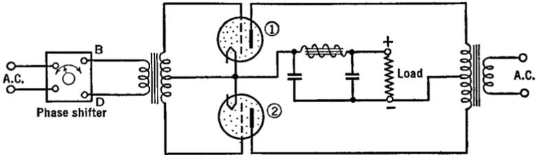
FIG. 19 L. Phase controlled thyatron rectifier circuit
