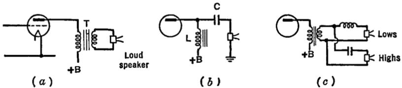
FIG. 13 M. Types of output circuits: (a) transformer coupled; (b)  $LC$  coupled ( $L$  and  $C$  must both have large values); (c) frequency division, the low and high notes operating separate speakers
