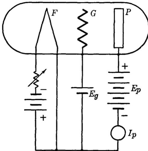
Fig. 12 A. Circuit used to plot the characteristic curves of a triode.
