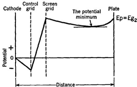
FIG. 15 E. Potential distribution in a beam-power tube
