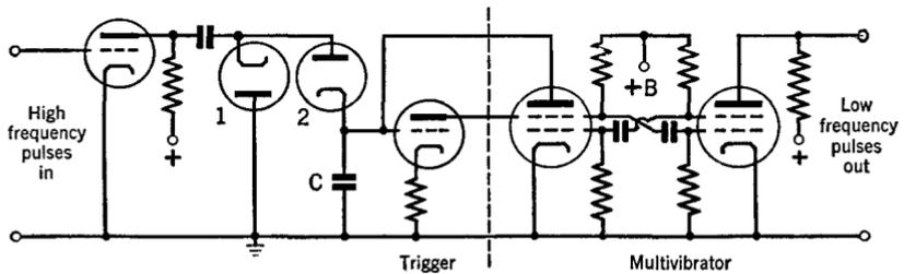
FIG. 30 L. A frequency divider. (See *R.C.A. Rev.*, p. 57, July 1940)
