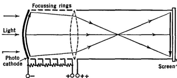
FIG. 21 O. An electron telescope
