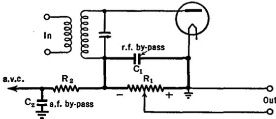
FIG. 32 N. Principle of automatic volume control (a.v.c.)
