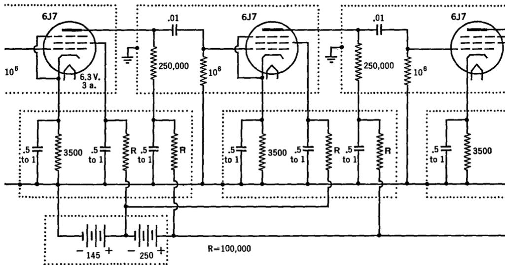
FIG. 25 D. A linear amplifier, filtered and shielded
