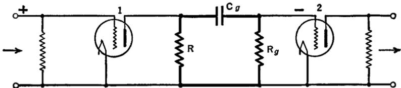
FIG. 13 G. Resistance-capacitance coupling
