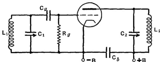
FIG. 14 D. A tuned-plate tuned-grid oscillator
