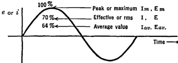
FIG. 4 C. Effective, peak, and average values of sinusoidal currents and voltages
