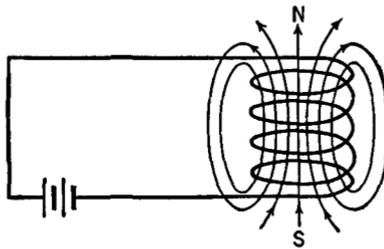
FIG. 3 G. Magnetic field of a solenoid
