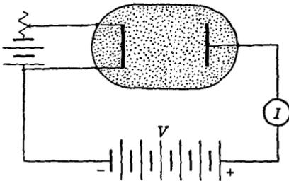
FIG. 18 E. A gas-filled diode.
