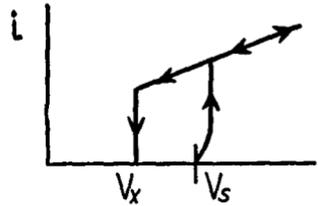
FIG. 18 C. Striking and extinction voltages of a glow-tube. (From E. & N. P.)
