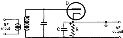
FIG. 17 C. A simple diode detector circuit
