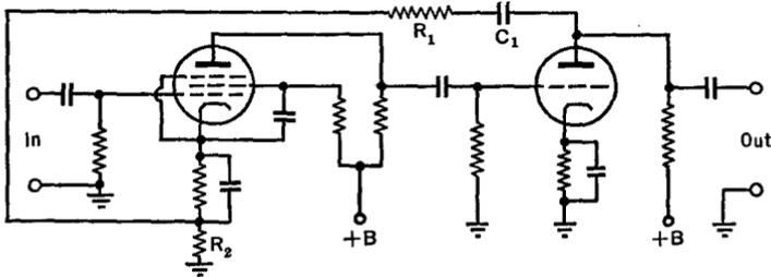
FIG. 26 D. A typical two-stage degenerative amplifier
