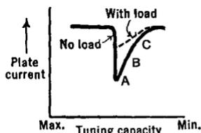
FIG. 29 F. Adjustment of a crystal oscillator
