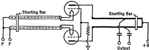
FIG. 37 I. A tuned-filament, tuned-plate, push-pull u.h.f. oscillator
