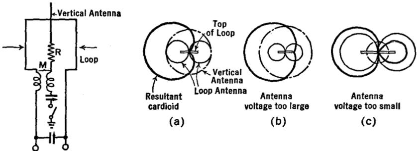
FIG. 34 G. A sense-determining radio-compass
