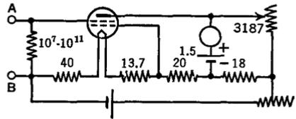
FIG. 24 C. A simple, stabilized d.c. amplifier
