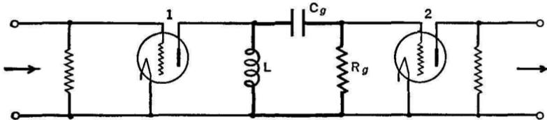
FIG. 13 H. Impedance coupling
