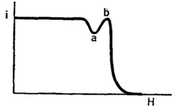
FIG. 38 G. The effect (at a b) of electron bombardment of the filament
