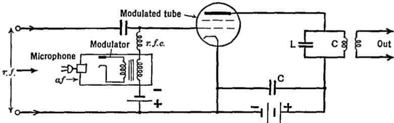
FIG. 16 J. Further details of grid-bias modulation
