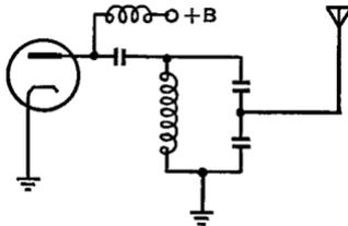
FIG. 31 M. A capacitively-coupled antenna circuit
