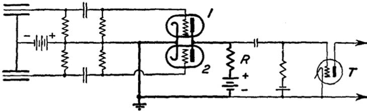
FIG. 30 J. A coincidence counter circuit. (From E. & N. P.)
