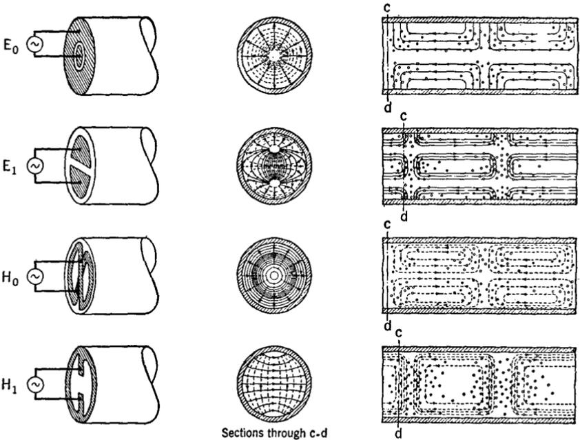
FIG. 38 P. Various feeding methods and the resultant field patterns for a cylindrical wave-guide. Electric lines of force, solid; magnetic lines, black dots when toward observer, small circles when away. (See references to Southworth at end of chapter)
