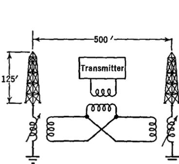
FIG. 34 O. One-half of an A and N transmitting antenna system
