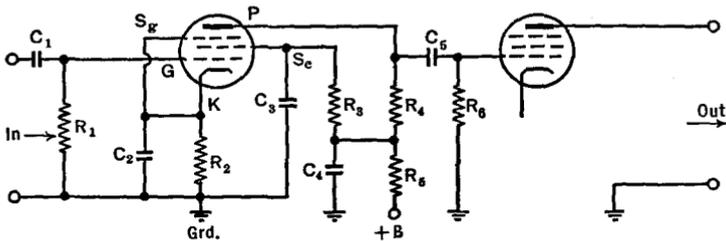
FIG. 25 A. A typical resistance capacitance coupled amplifier
