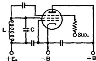
FIG. 29 B. A negative-resistance or "transitron" oscillator
