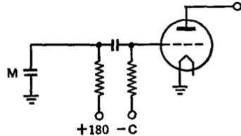
FIG. 25 L. Amplifier circuit for a condenser "mik"
