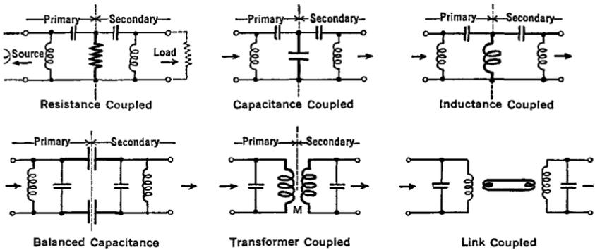
Fig. 7 A. Typical coupling methods
