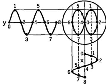
FIG. 22 R. The voltages on the deflection plates are equal in amplitude and phase but the frequency applied to  $y$  is twice that on  $x$
