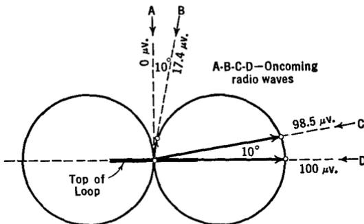
FIG. 34 D. Sharper direction finding can be obtained using the minimum rather than the maximum output of a loop
