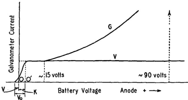
FIG. 20 D. The photoelectric currents for different voltages applied to a vacuum (*V*) and a gas-filled tube (*G*). (From E. & N. P.)
