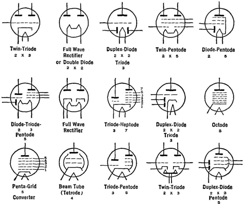
FIG. 15 F. The names and symbols of some multi-electrode and combination tubes
