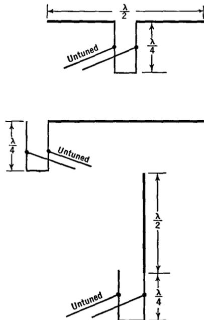
FIG. 36 L. Matching impedances with linear-transformers
