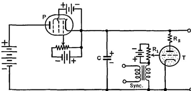
FIG. 22 H. The thyratron  $T$  replaces the glow-tube  $G$  of Fig. 22 G
