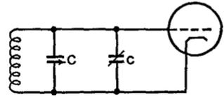
FIG. 32 L. Tracking with a trimmer
