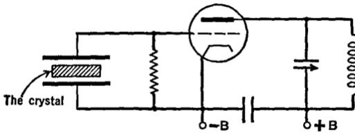
FIG. 14 F. A quartz crystal oscillator circuit
