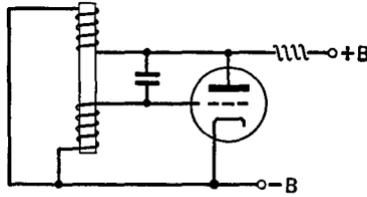
FIG. 14 I. Elementary form of a magnetostriction oscillator
