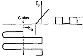
FIG. 30 C. Action of the second tube in Fig. 30 A.
