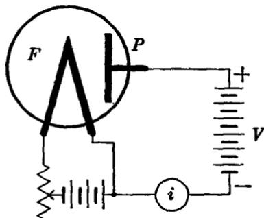
FIG. 10 A. A high vacuum two-electrode tube or diode. (From E. & N. P.)
