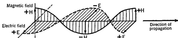
FIG. 8 A. The electric and magnetic fields of a radio wave are at right angles to each other and also at right angles to the direction in which energy is propagated
