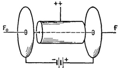
FIG. 38 H. An end-plate magnetron
