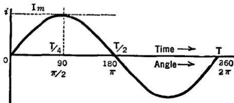
FIG. 4 B. A sine curve
