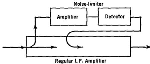
FIG. 32 Q. Block diagram of a noise-limiter
