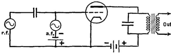
FIG. 16 I. Elementary circuit for grid-bias modulation
