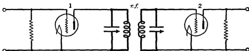
FIG. 13 J. Tuned transformer coupling for radio frequencies
