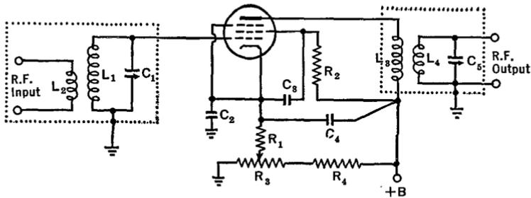
FIG. 27 A. A typical tuned radio-frequency amplifier
