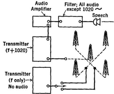
FIG. 34 P. Simultaneous message and beacon transmission
