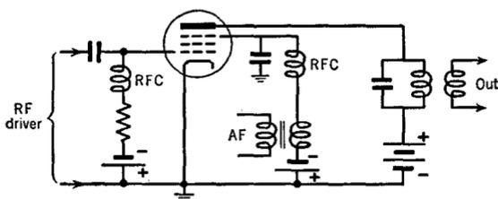
FIG. 16 L. Elementary circuit for suppressor-grid modulator
