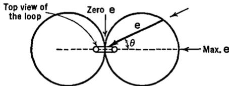
FIG. 34 B. Ideal response curve of a loop antenna
