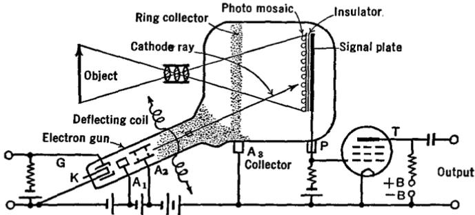
FIG. 21 M. An iconoscope and its circuits
