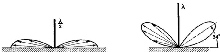
FIG. 8 E. Radiation patterns from vertical Marconi antennas
