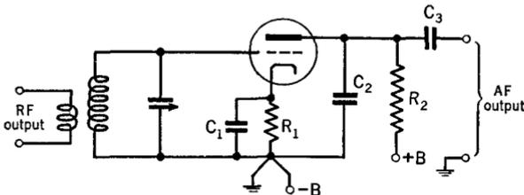
FIG. 17 E. A simple plate detector
