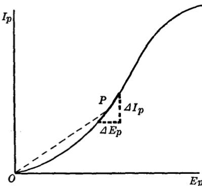
FIG. 12 F. The "plate resistance" of a triode is given by  $\Delta E_p/\Delta I_p$  ( $= e_p/i_p$  in the text) rather than as the inverse slope of the dotted line. The latter is called the d.c. plate resistance. (From E. & N. P.)
