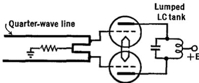
FIG. 37 J. A line-tuned-grid-tank, lumped-tuned-plate-tank, push-pull u.h.f. oscillator
