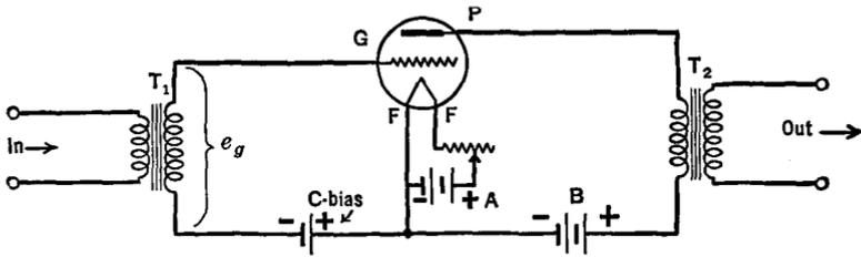
FIG. 13 B. A simple transformer-coupled single-stage triode amplifier
