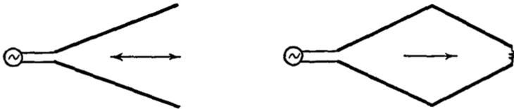
FIG. 35 I. "V" and Rhombic types of antenna
