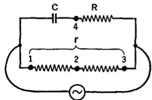
FIG. 19 H. An RC phase shifter
