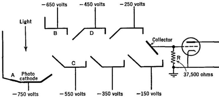
Fig. 20 L. A 6-stage electrostatic photo-multiplier tube
