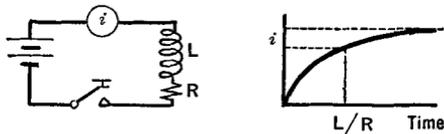
FIG. 3 K. The Time Constant of an inductive-resistive circuit is  $L/R$
