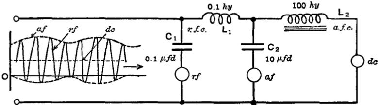
FIG. 5 B. To illustrate the separation or "filtering" of d.c., a.f. and r.f. currents from a complex current
