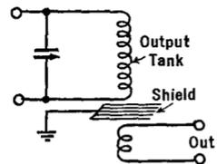
FIG. 31 G. The use of a Faraday shield to reduce the harmonics from a transmitter
