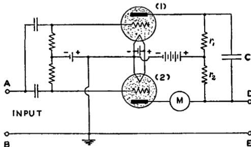
FIG. 30 K. A scale-of-two counter. (From E. & N. P.)
