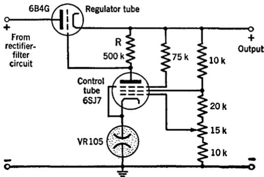
Fig. 30 Q. A voltage stabilizing circuit. ( $k = 1000$  ohms)
