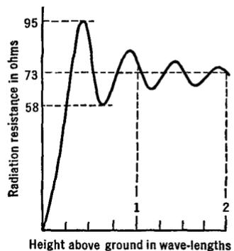
Fig. 36 M. Radiation-resistance of a half-wave horizontal antenna at various distances above the ground
