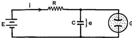
FIG. 22 A. A simple sweep circuit
