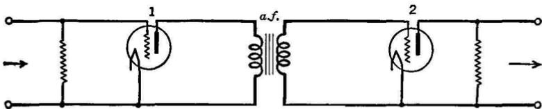
FIG. 13 I. Transformer coupling for audio frequencies
