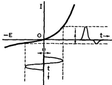
FIG. 23 B. Non-ohmic unsymmetrical element
