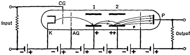
FIG. 15 G. Principle of a multiplier tube
