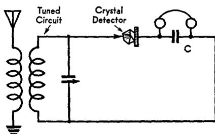
FIG. 17 A. A simple crystal receiver
