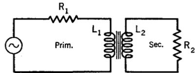
FIG. 5 D. A simple transformer circuit
