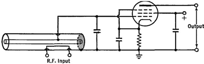
FIG. 37 D. An ultra-high frequency receiver using a quarter-wave concentric line in the tuning circuit
