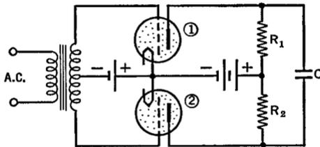
FIG. 19 M. The principle of operation of an inverter
