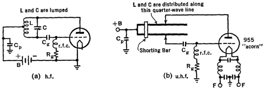
FIG. 37 F. Comparison of low and high frequency ultraudion oscillator circuits
