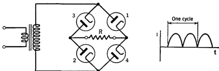
FIG. 11 D. Full-wave bridge rectifier
