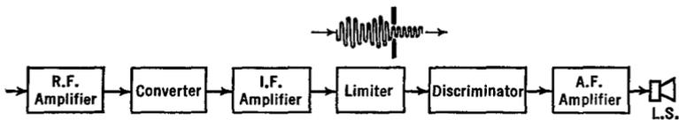
FIG. 33 C. Block diagram of an f.m. receiver
