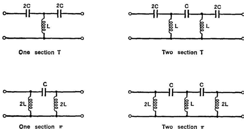
FIG. 7 G.—T- and  $\pi$ -type, high-pass filters
