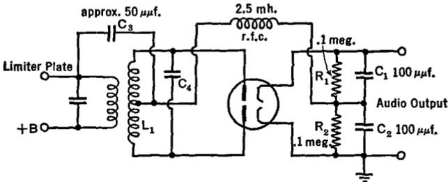
FIG. 33 E. A typical discriminator circuit
