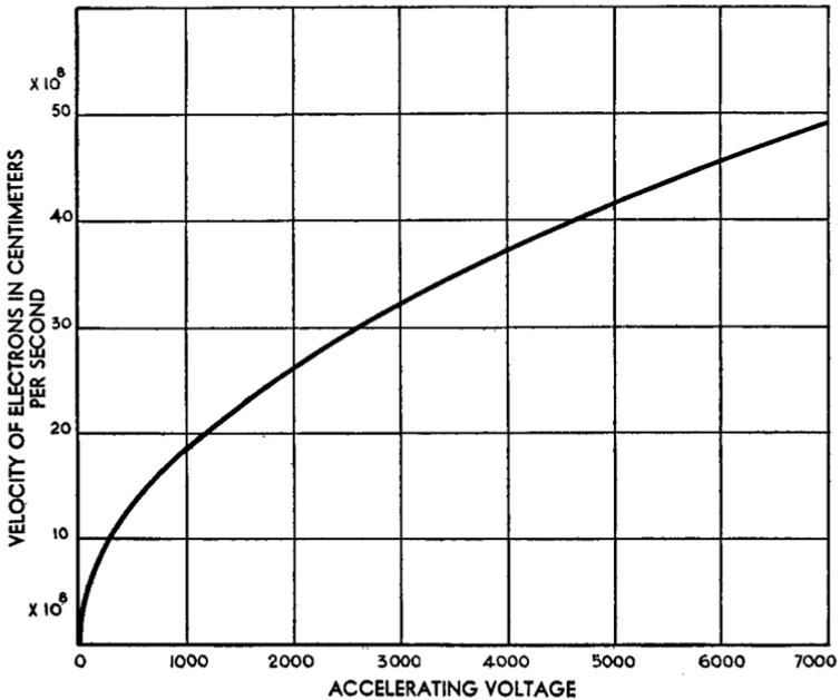
FIG. 1 C. Velocity of electrons accelerated by various voltages
