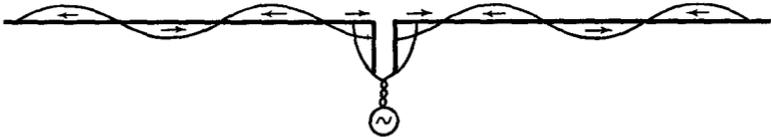
FIG. 35 H. Current distribution along a center-fed  $7/2$ -wave antenna
