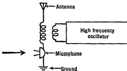
FIG. 16 E. A crude method of amplitude modulation
