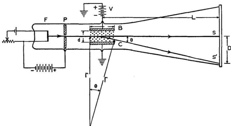
FIG. 1 B. Measurement of the mass and velocity of the electron.
