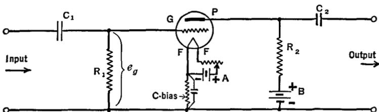
FIG. 13 A. A simple resistance-capacitance-coupled single-stage triode amplifier
