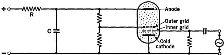
FIG. 18 D. A simple stroboscope circuit using a strobotron tube
