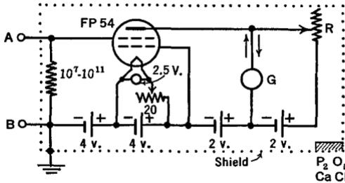
FIG. 24 A. A simple d.c. amplifier
