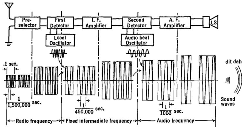
Fig. 32 H. Superheterodyne reception of c.w. signals
