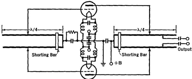
FIG. 37 H. A tuned-grid, tuned-plate, push-pull u.h.f. oscillator
