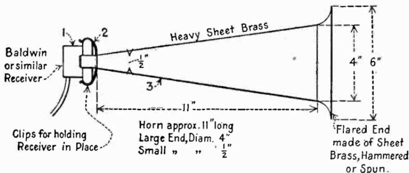
Fig. 70.—Loud speaking telephone unit complete.
