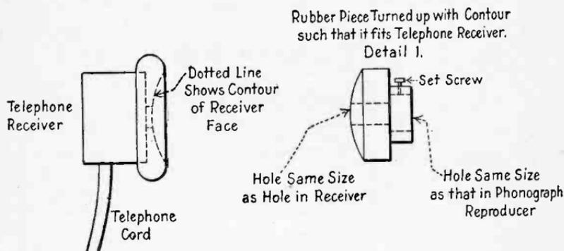
Fig. 74.—Details to adapt telephone receiver to phonograph.
