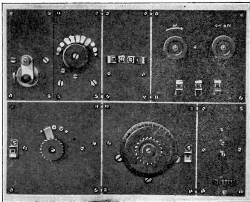
Fig. 17.—The instruments assembled, ready to wire.
