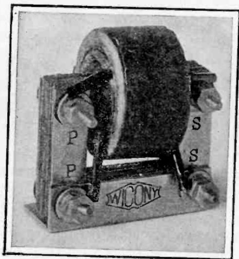
Fig. 62.—The amplifying transformer.
