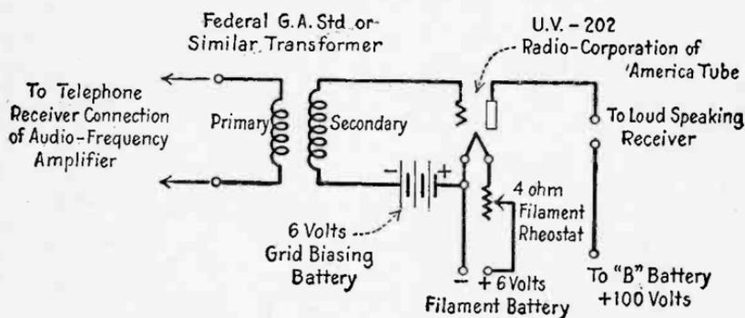
Fig. 69.—Circuit diagram of amplifier.
