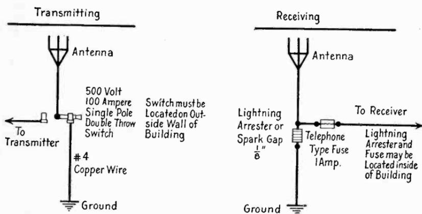
Fig. 3.—Protection of antenna systems from lightning.
