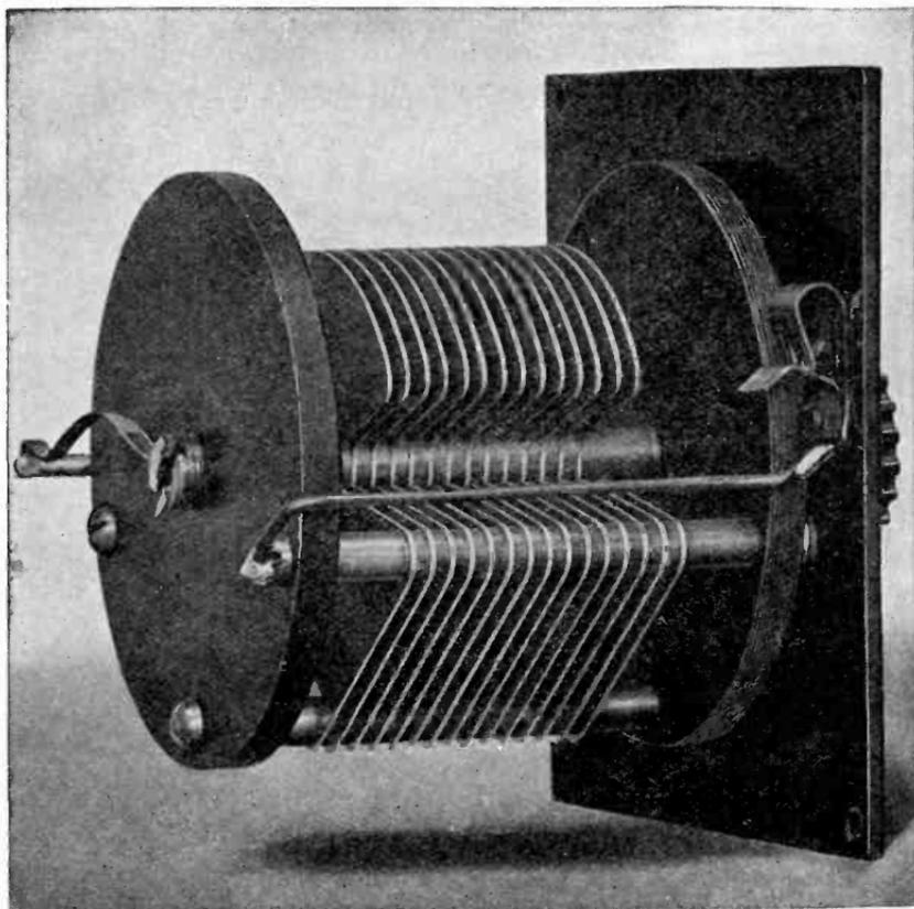
Fig. 19.—A close view of the tuning condenser. The method of connecting is shown clearly.
