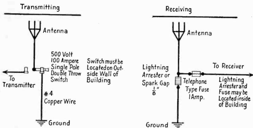
Fig. 3.—Protection of antenna systems from lightning.
