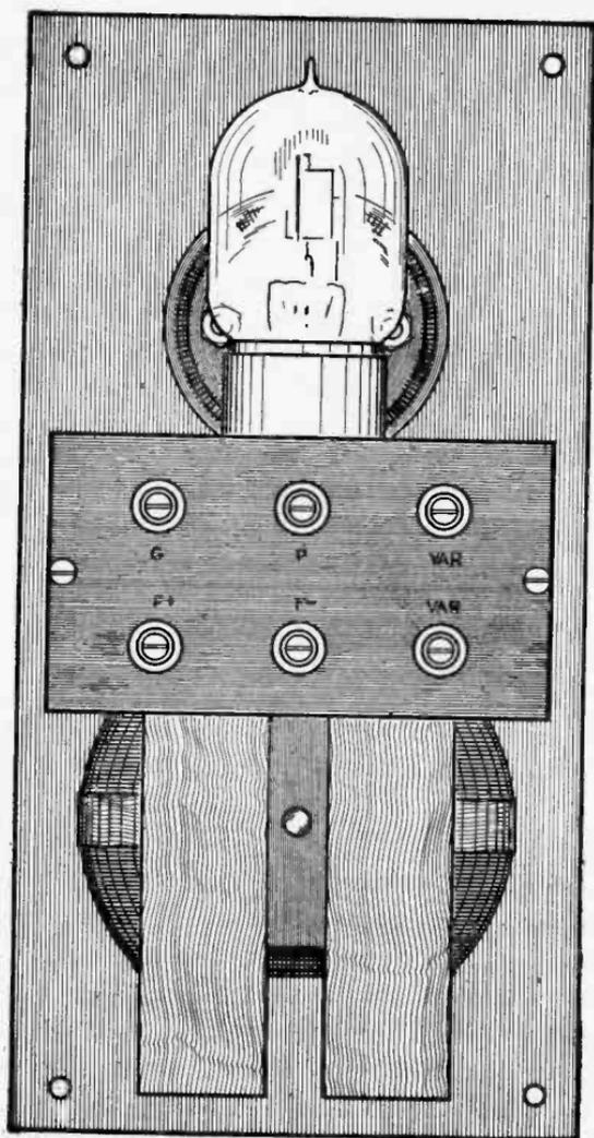
Fig. 45—Details of the audion and plate variometer mounting.
