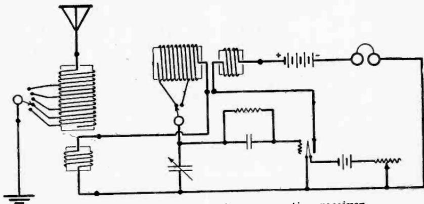
Fig. 43.—Connections for the regenerative receiver.
