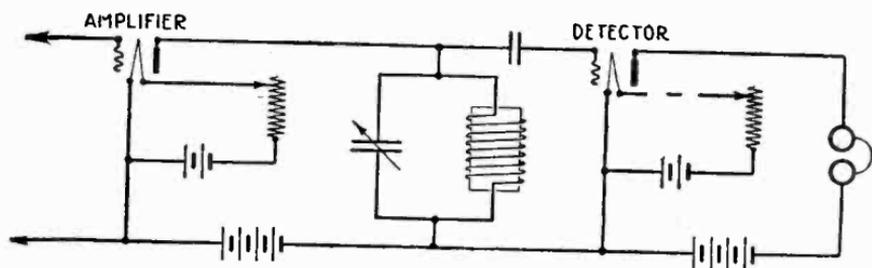
Fig. 64.—A simplified circuit of the amplifier.
