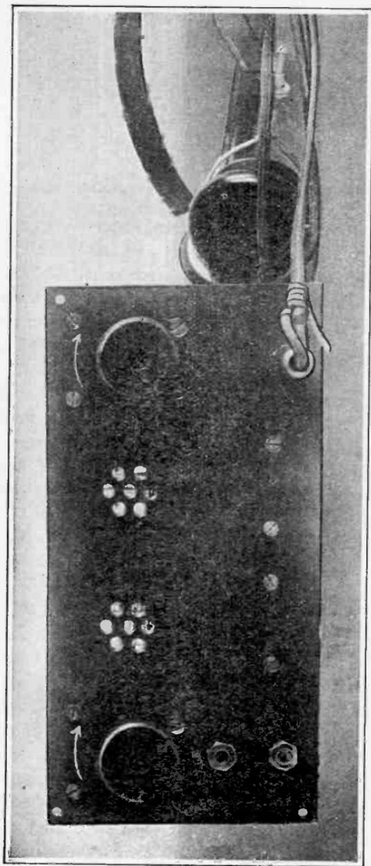
Fig. 49.—On the front of the panel are the rheostat controls, jacks for detector, first step and second step of amplification, and observation windows for the filaments.
