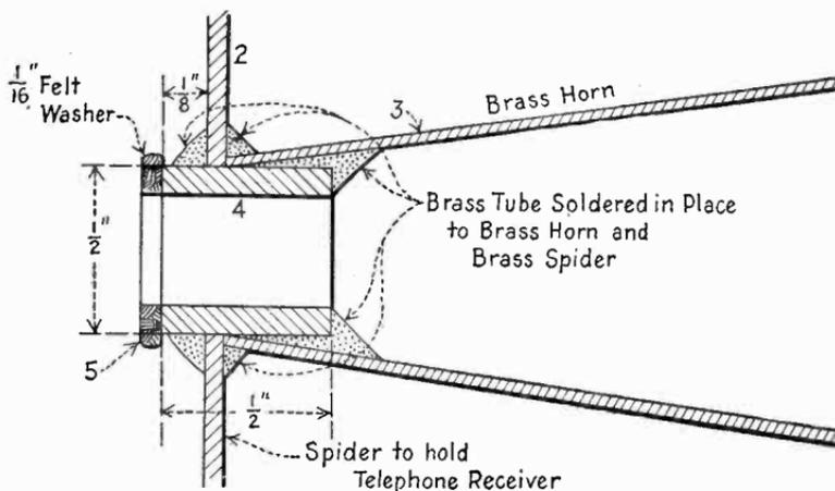
Fig. 71.—Details of receiver end of horn.
