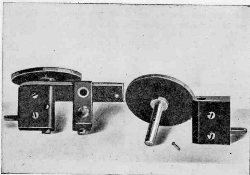
Fig. 38.—A new shaft, carrying a bakelite disc, was substituted for the other, so that the coils could be mounted behind the panel and moved from the front.
