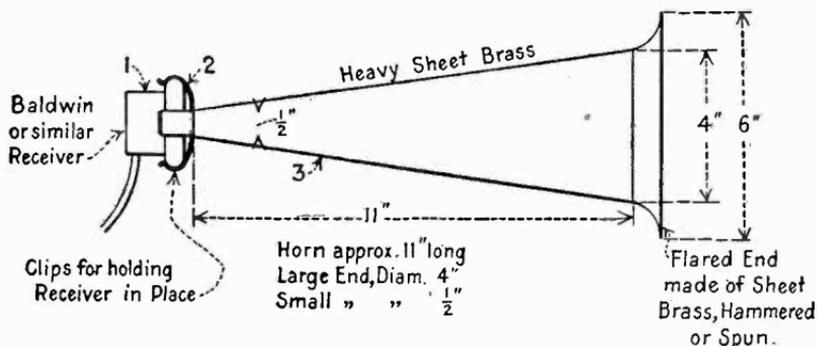
Fig. 70.—Loud speaking telephone unit complete.
