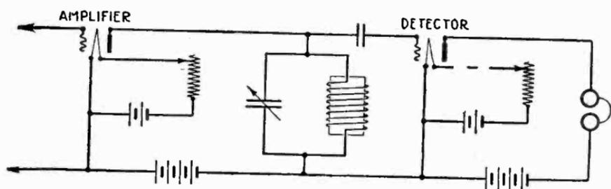
Fig. 64.—A simplified circuit of the amplifier.
