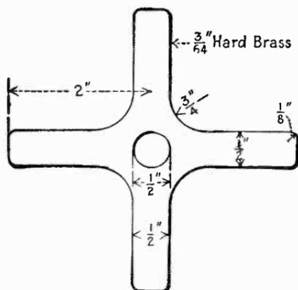
Fig. 72.—Details of the spider.
