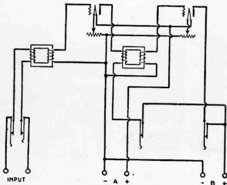
Fig. 54.—Diagram of connections for the two-step amplifier.
