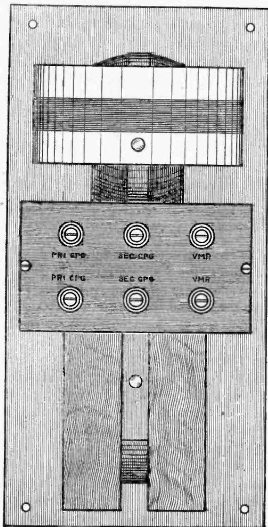
Fig. 47.—On the secondary panel are mounted the coupling coil and grid variometer. One-half scale.
