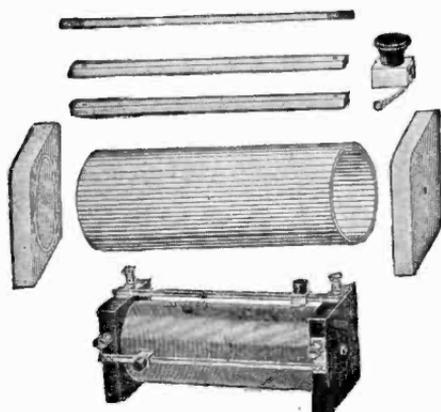
Fig. 8.—Details of the tuning coil
