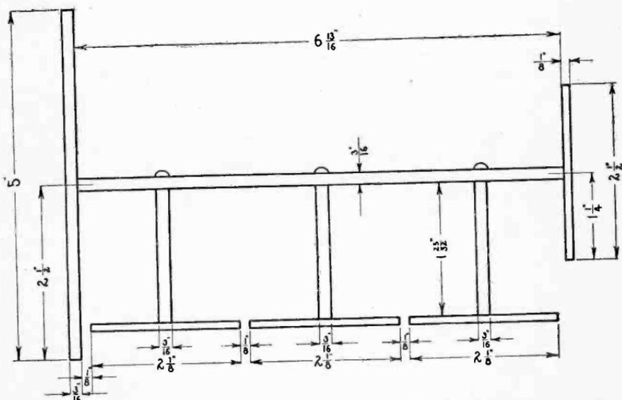
Fig. 59.—The framework which carries the instruments and binding posts.
