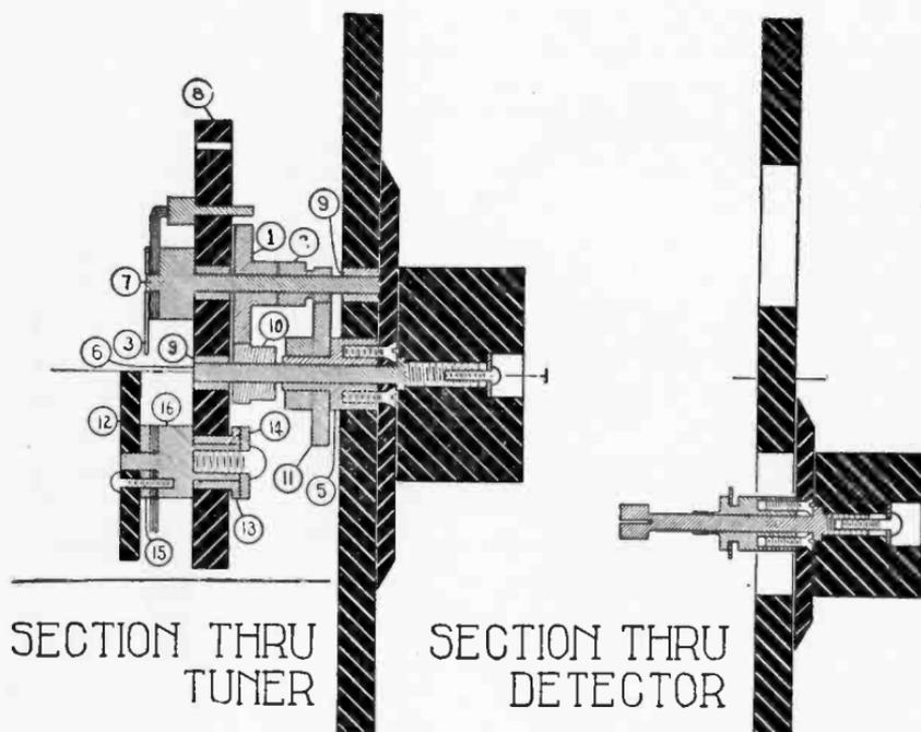
Fig. 33D.—Details of receiver for short wave traffic, specially designed for dependability and continuous use.
