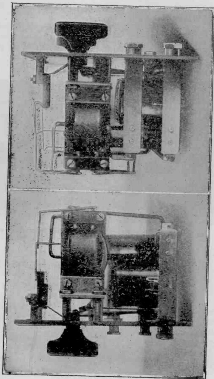
Fig. 51.—The methods of mounting the transformers and jacks are shown in these end views.
