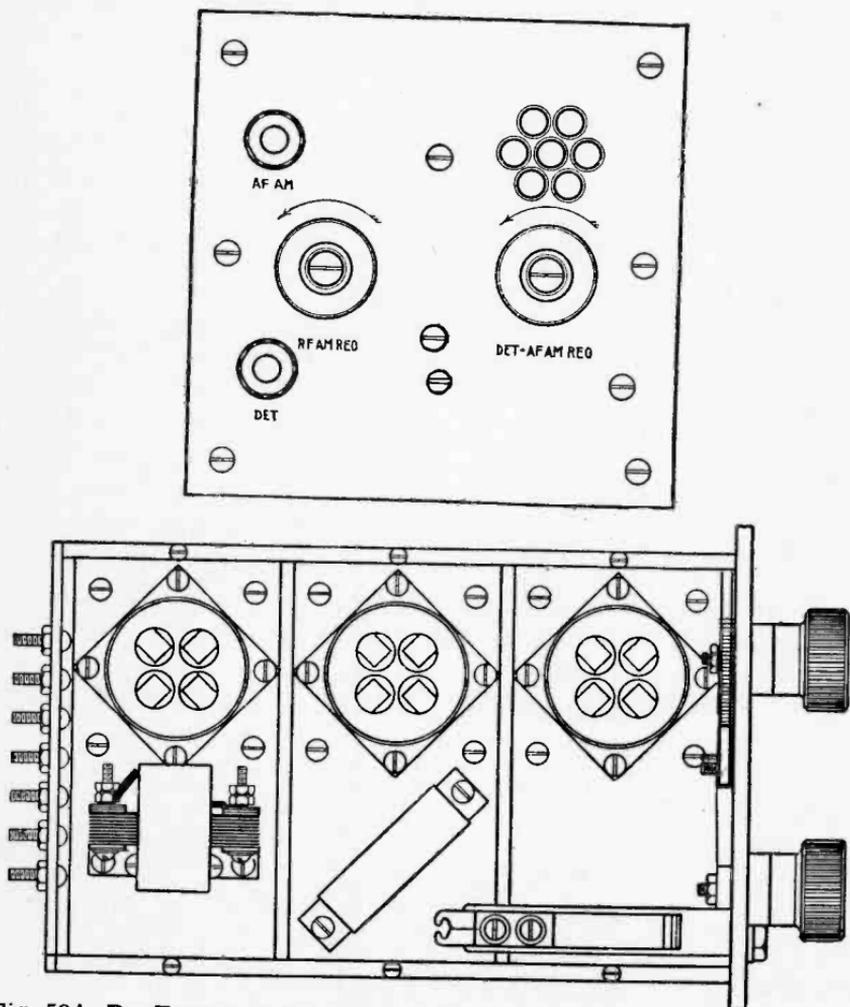
Fig. 58A, B.—Front and top views of the unit, showing the parts mounted on individual plates.
