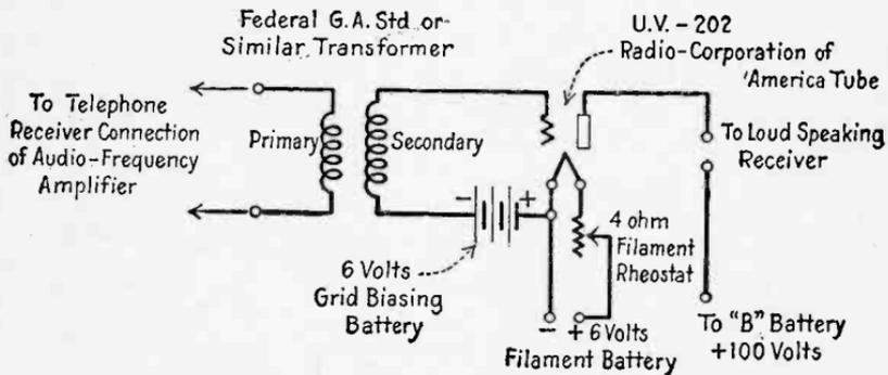
Fig. 69.—Circuit diagram of amplifier.
