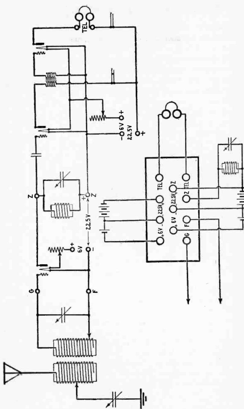
Fig. 63.—Above, the complete circuit for the combination radio and audio frequency amplifier. Below, connections from the binding post panel to the exterior apparatus.
