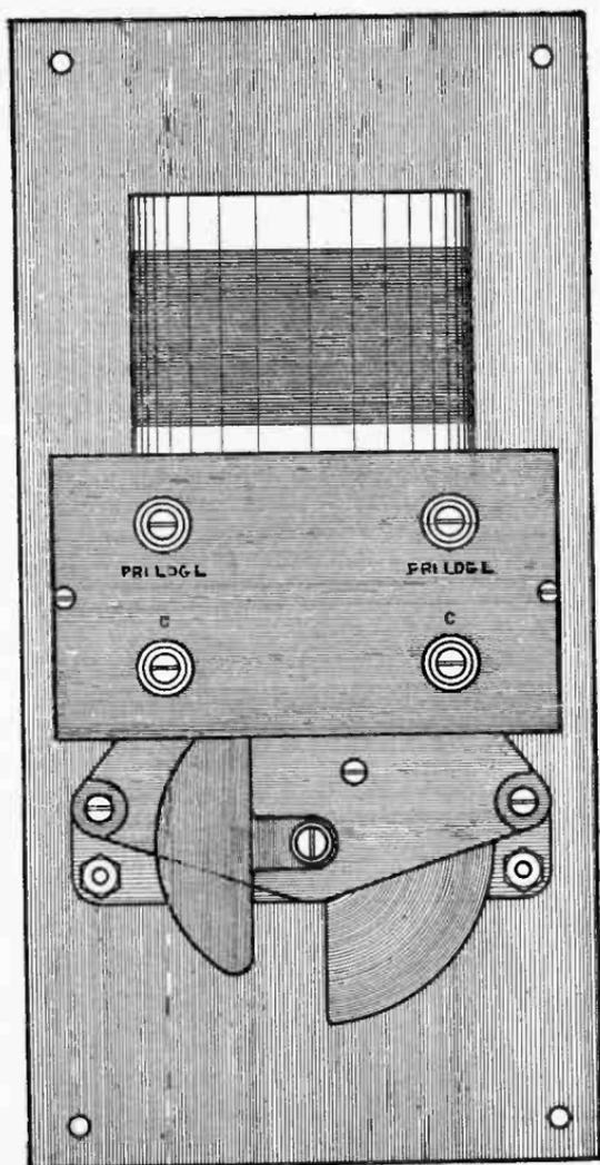
Fig. 48.—The antenna loading coil and 0.0006 mfd. condenser are carried on the primary panel. One-half scale.
