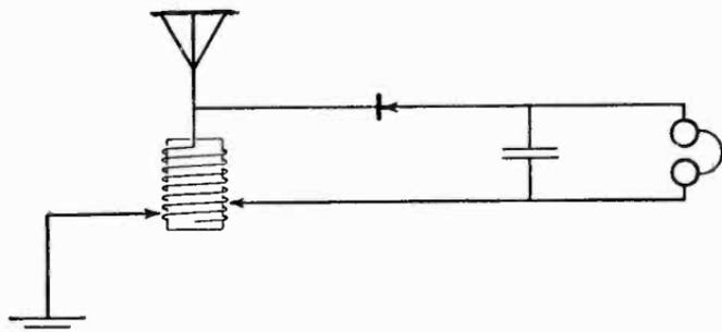
Diagram of connections of detector, two-slide tuning coil, phones and stopping condenser.
