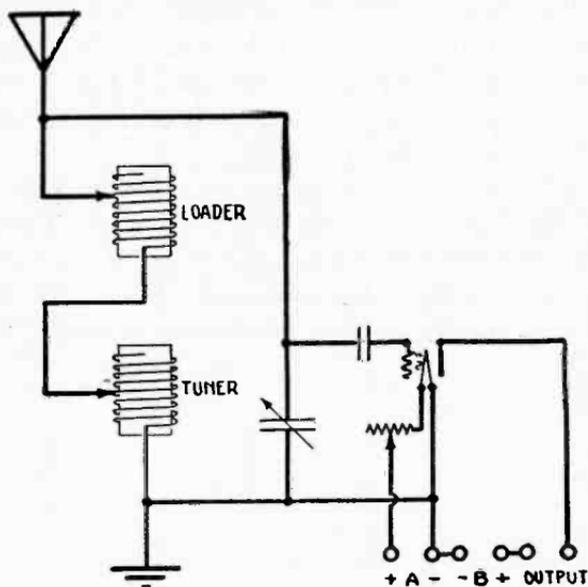
Fig. 55.—Wiring of the receiver, previously described, with the amplifier.
