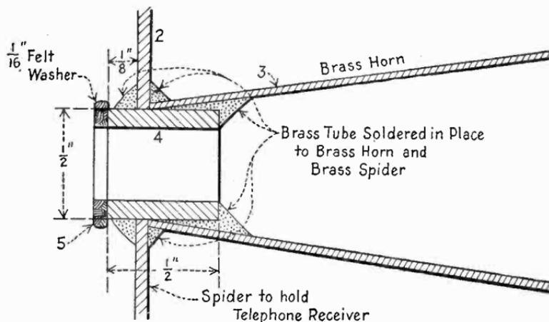
Fig. 71.—Details of receiver end of horn.
