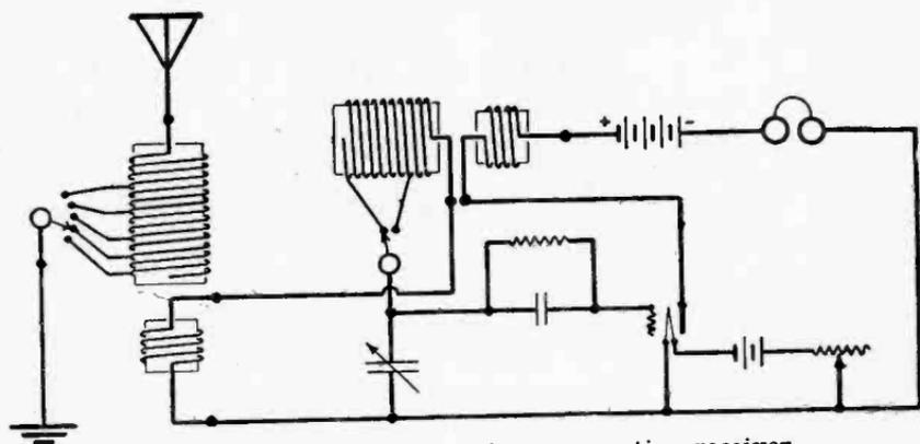
Fig. 43.—Connections for the regenerative receiver.
