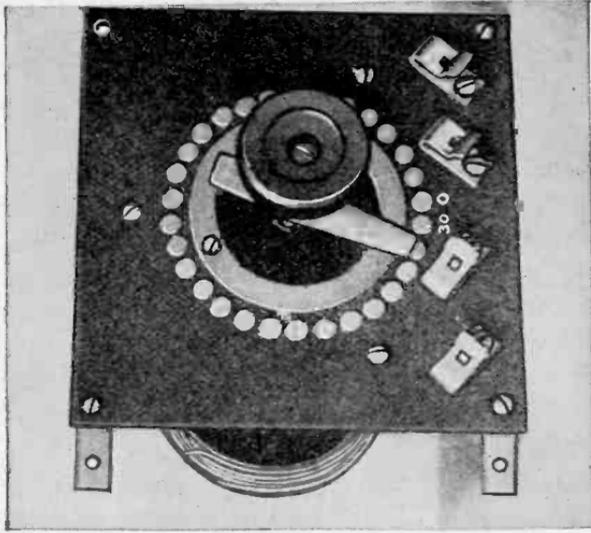
Fig. 15A, B.—Two views of the Standardized Panel type loose coupler. If a different coupler is made later, this can be removed and used for other purposes, and the new one set into place.
