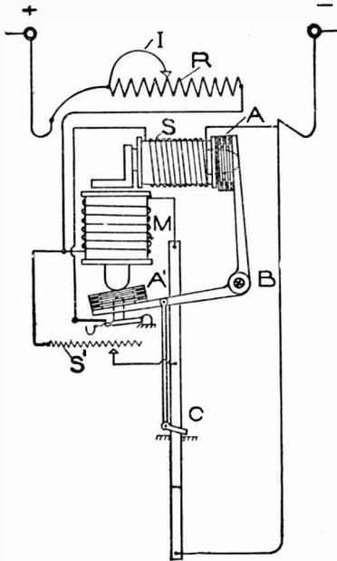
Fig. 36. Differential Mechanism for D. C. Arc Lamp.
