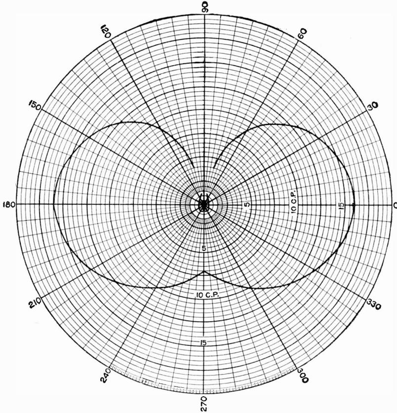
Fig. 8. Vertical Distribution Curve for Single-Loop Filament.
