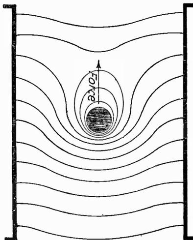
Fig. 13. Force on Motor Armature Conductor Moving Upward.
