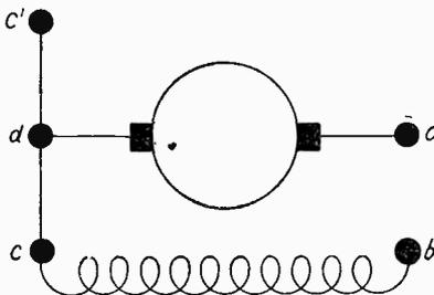
Fig. 21. Motor Field and Armature Terminals.
