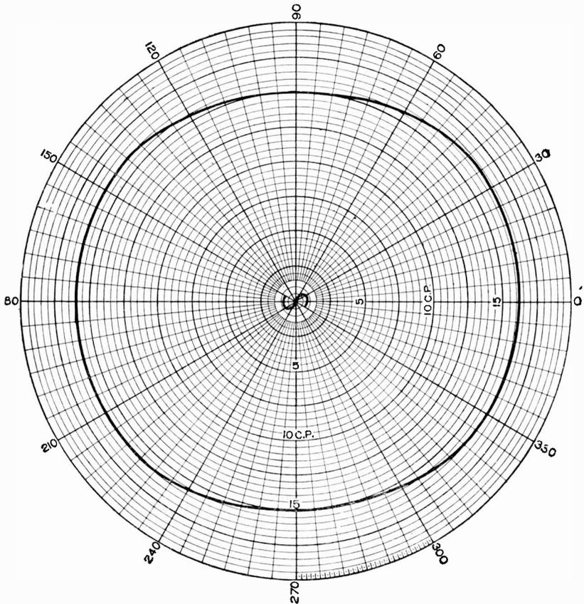
Fig. 7. Horizontal Distribution Curve for Single-Loop Filament.
