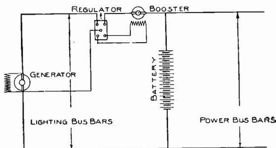
Fig. 35. External Control Constant-Current System.
