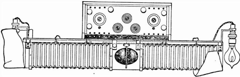
Fig. 81. Portable Photometer for Incandescent Lamps.
