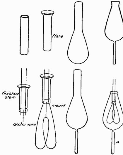
Fig. 2. Different Stages in Lamp Manufacture.
