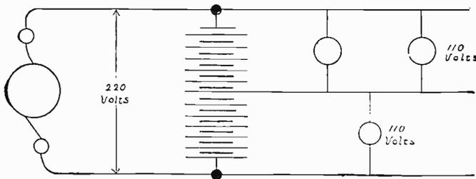
Fig. 21. Battery Used to Subdivide Voltage.
