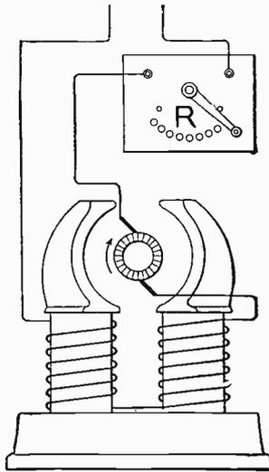
Fig. 34. Wiring Connections of a Series Motor.
