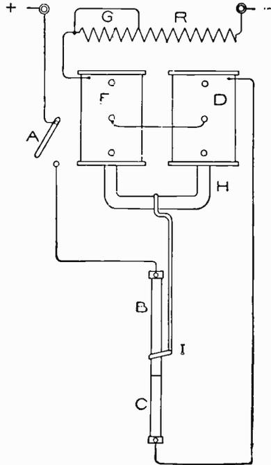
Fig. 35. Series Mechanism for D. C. Arc Lamp.
