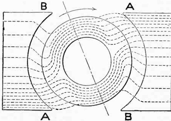
Fig. 8. Armature Reaction in Motor.
