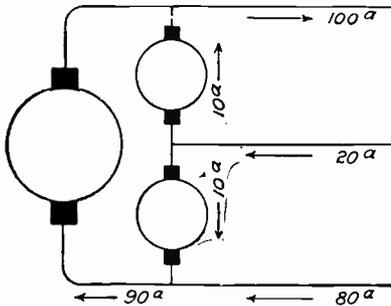
Fig. 41. Current through Balancer Set.
