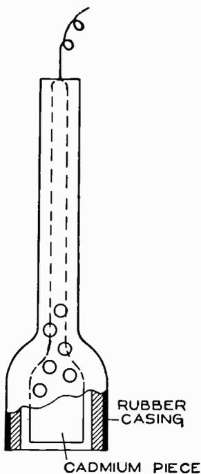
Fig. 15. Cadmium Test-Piece.
