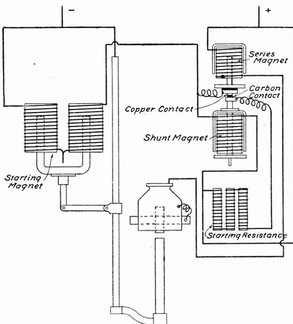
Fig. 42. Diagram of Connections for Magnetite Arc Lamp.
