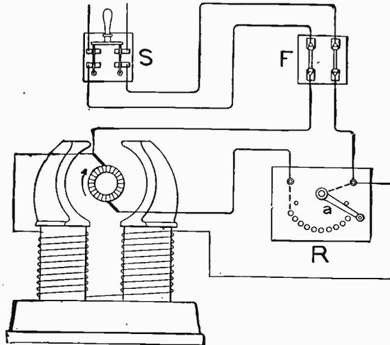
Fig. 19. Wiring Connections of Shunt Motor.
