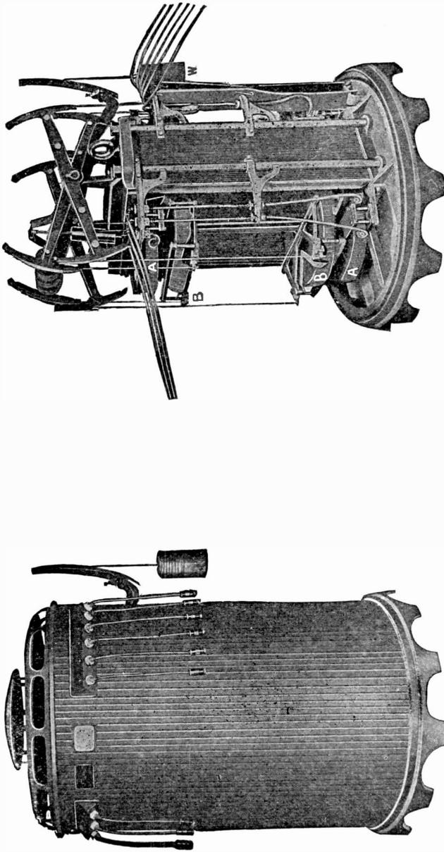
Fig. 46. Double-Coil Transformer (second view with case removed).
