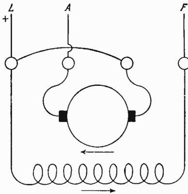
Fig. 24. Connections for Reversing a Motor.
