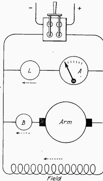
Fig. 5. Motor Connections to Show Counter-E.M.F.
