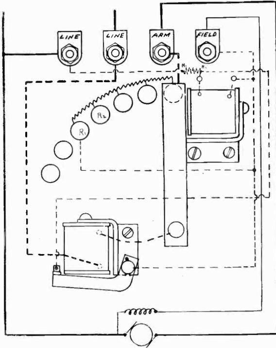
Fig. 23. Connections of Motor-Starting Rheostat with No-Voltage and Overload Release.
