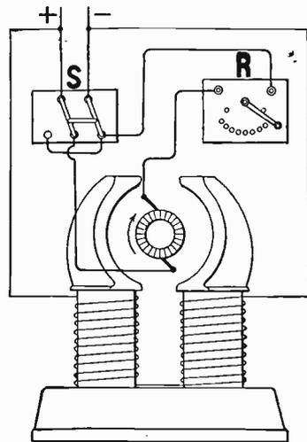
Fig. 26. Connections of Reversing Switch.
