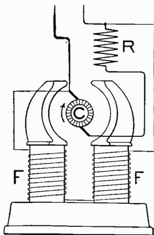
Fig. 30. Speed Control by Resistance in Armature Circuit.
