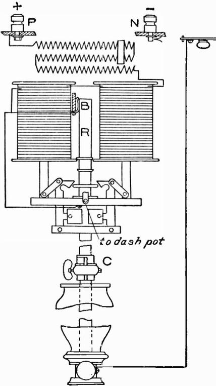
Fig. 37. Rod-Feed Mechanism.
