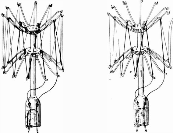
Fig. 12. Appearance of Filament After Having Been Used. Filament Frame Showing Broken Filament.
