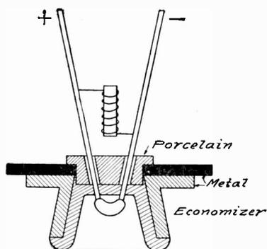
Fig. 39. Diagram of Bremer Flaming Arc.
