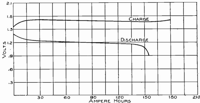
Fig. 10. Charge and Discharge Curves of Edison Cell.
