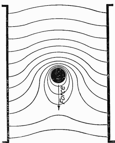
Fig. 12. Force on Dynamo Armature Conductor Moving Upward.
