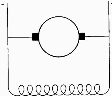
Fig. 10. Connections of Shunt Motor when Running.
