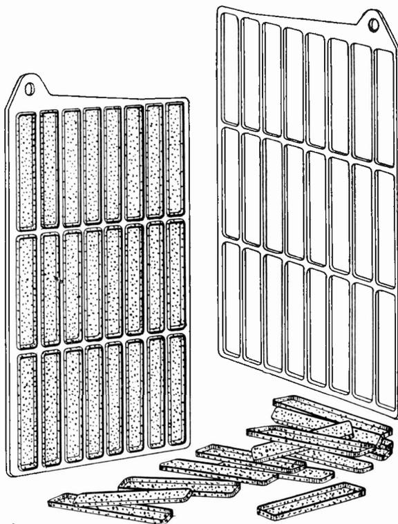
Fig. 8. Plates and Receptacles of the Edison Cell.
