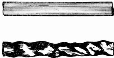
Fig. 11. Tantalum Filament Before and After 1,000 Hours' Use.
