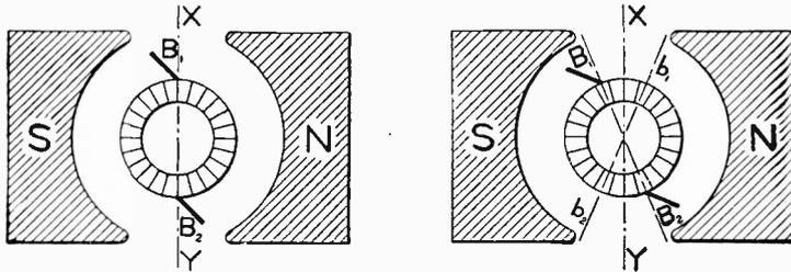
Fig. 11. Demagnetizing Effect of Motor Armature.
