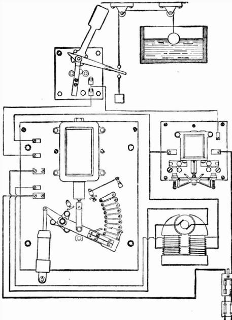
Fig. 28. Self-Starter Used with Motor-Driven Pump.
