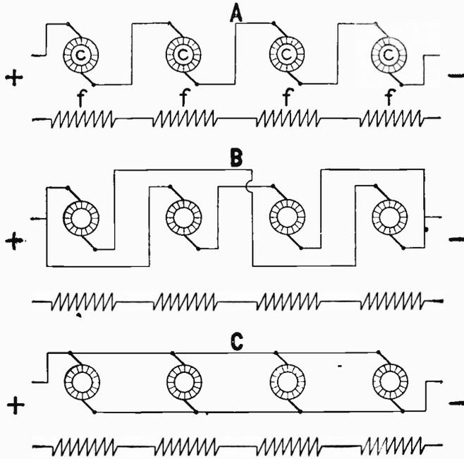
Fig. 9. Series-Parallel Connections of Four Motors.
