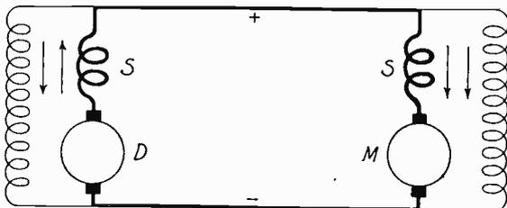
Fig. 36. Compound Dynamo Driving Compound Motor.
