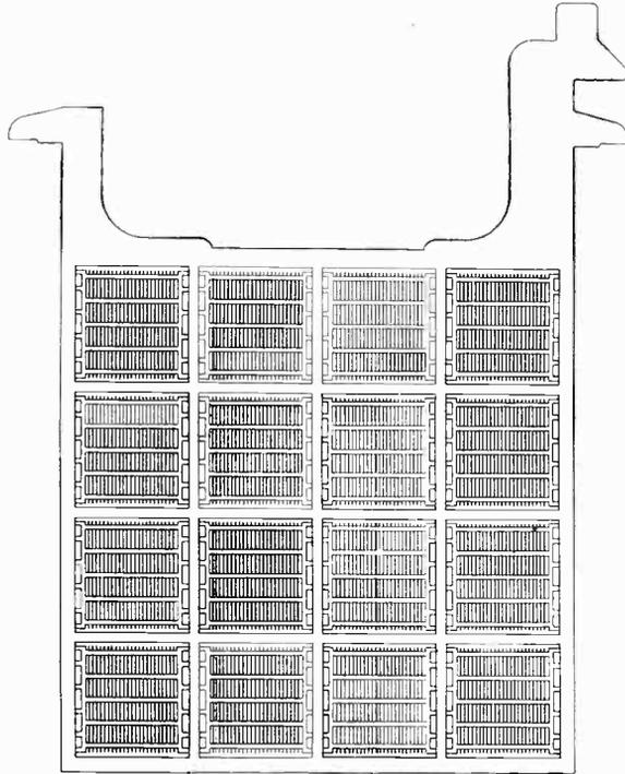
Fig. 2. Bijur High-Duty Battery Plate.
