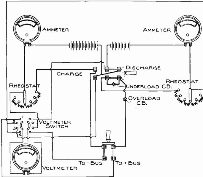
Fig. 28. Connections for Parallel Charge, Series Discharge.
