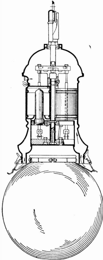
Fig. 20. Sectional View of Multiple-Glower Westinghouse Nernst Lamp.
