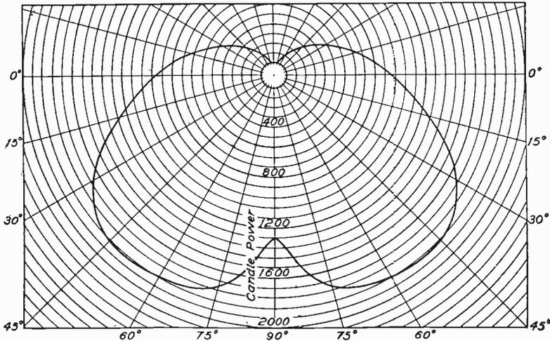
Fig. 43. Distribution Curve for Flaming Arc Lamp.
