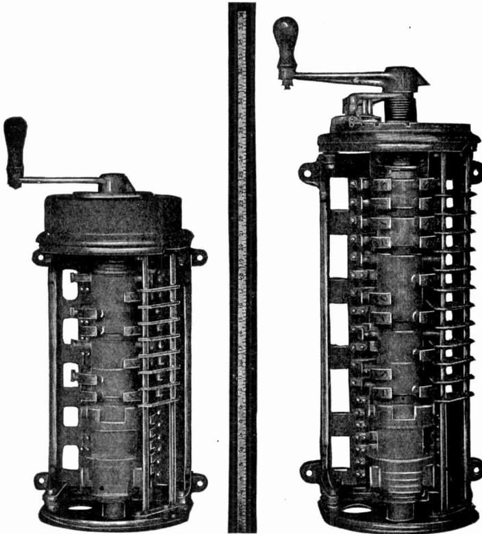
Fig. 42. Controllers Used with Bullock Multiple-Voltage System.
