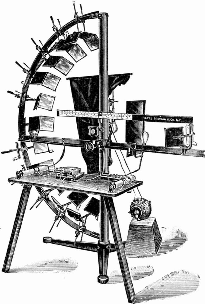
Fig. 77. Integrating Photometer.
