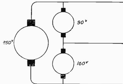
Fig. 39. Connections of Balancer Set.
