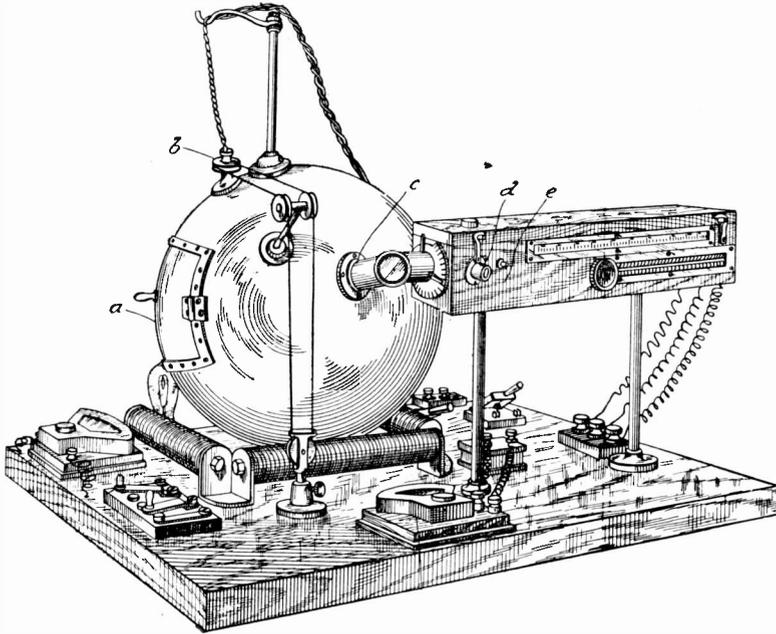
Fig. 78. Eighteen-Inch Integrating Sphere Equipped with Photometer.
