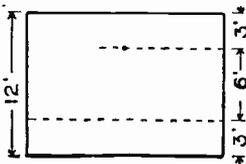
Fig. 53. Diagram Showing Method of Calculating Room Illumination.
