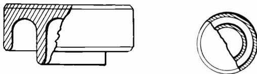
Fig. 11. Glass Insulator for Battery Support.
