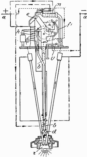
Fig. 41. Clock Feeding Mechanism for Luminous Arc Lamp.
