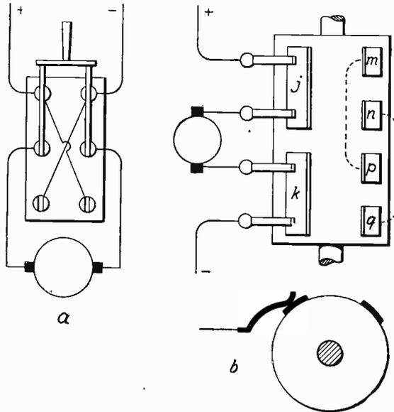
Fig. 27. Reversing Switches.
