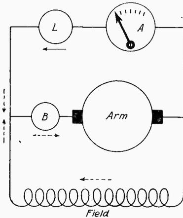
Fig. 6. Currents in Motor Circuits after Opening Main Switch.
