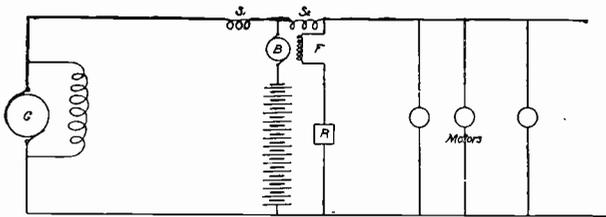
Fig. 32. Differential Booster Connections.
