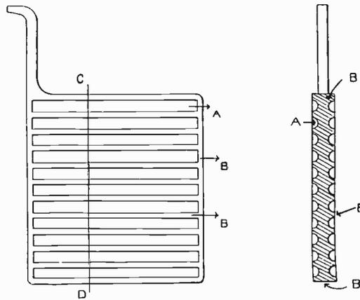
Fig. 7. The Tudor Battery Plate.
