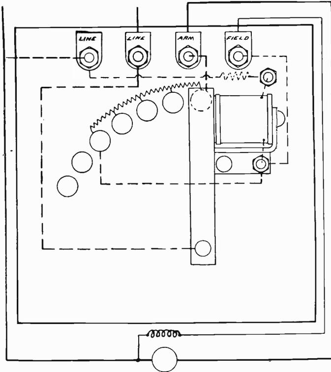
Fig. 20. Connections of Motor-Starting Rheostat with No-Voltage Release.
