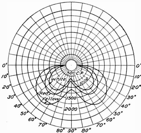
Fig. 40. Distribution Curves of a Luminous Arc.
