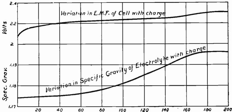
Fig. 16. Curve Showing Increase of E. M. F. in a Charging Cell.
