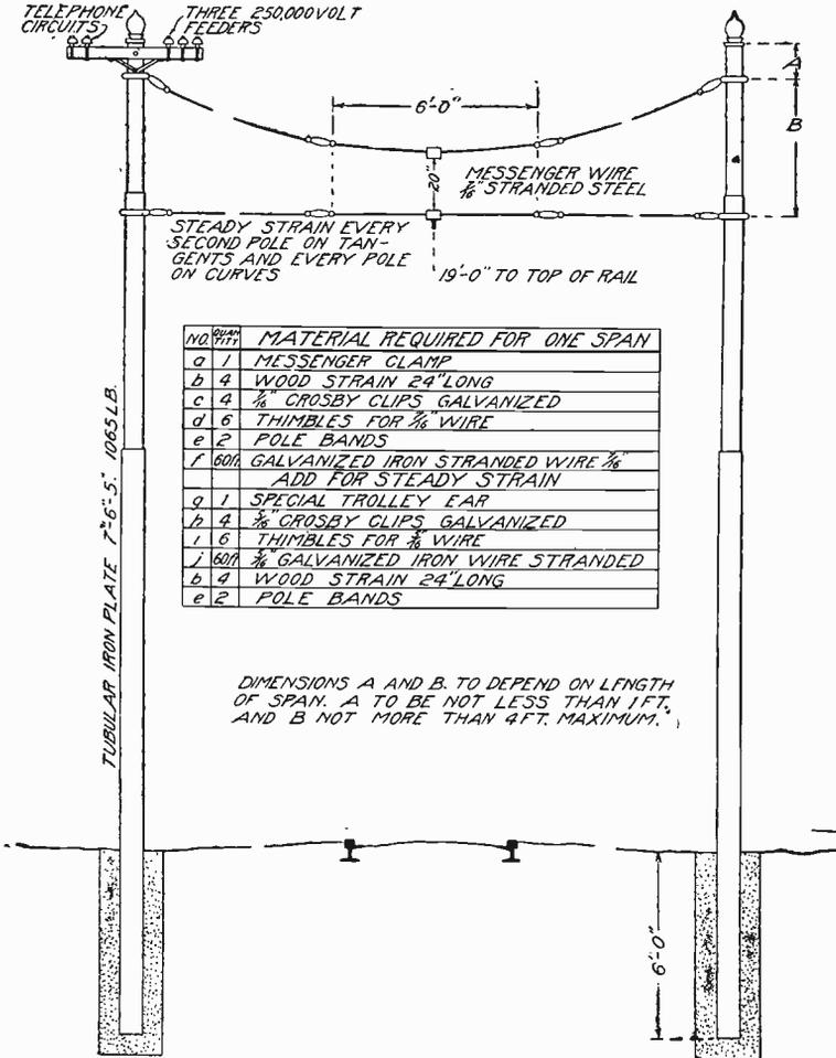
Fig. 198. Span Construction of the Catenary Type
