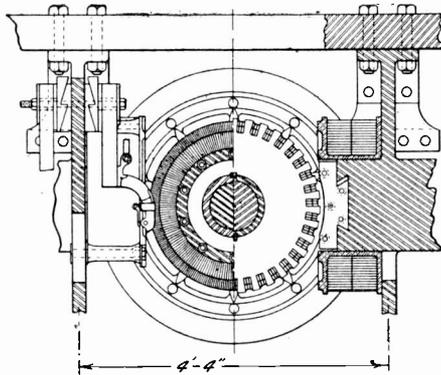
Fig. 248. End Section of New York Central Motor
