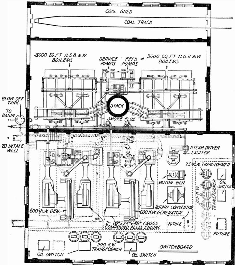
Fig. 146. Plan of Winona Railway Company Power House
