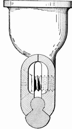
Fig. 188. Section Through Clamp for a "Figure 8" Wire
