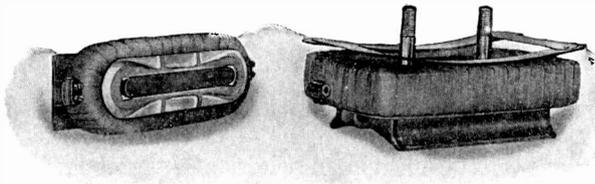
Fig. 34. Main Pole and Interpole Complete
