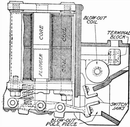
Fig. 60 Sprague-General Electric Contactor Diagram
