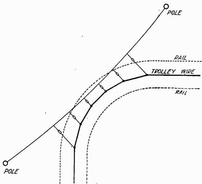
Fig. 193. Simple Curve Suspension Using Two Poles
