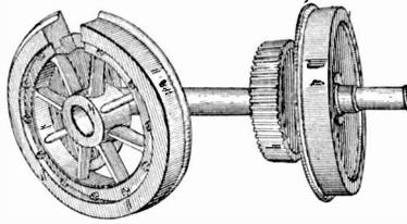
Fig. 25. Wheels and Gear Showing Section of Rim
