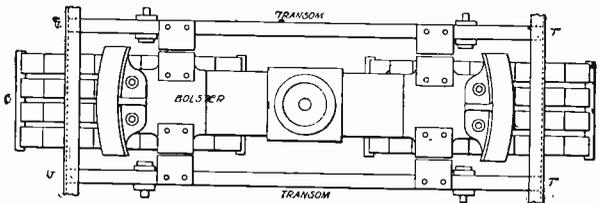
Fig. 12. Plan of Bolster and Spring Plank
