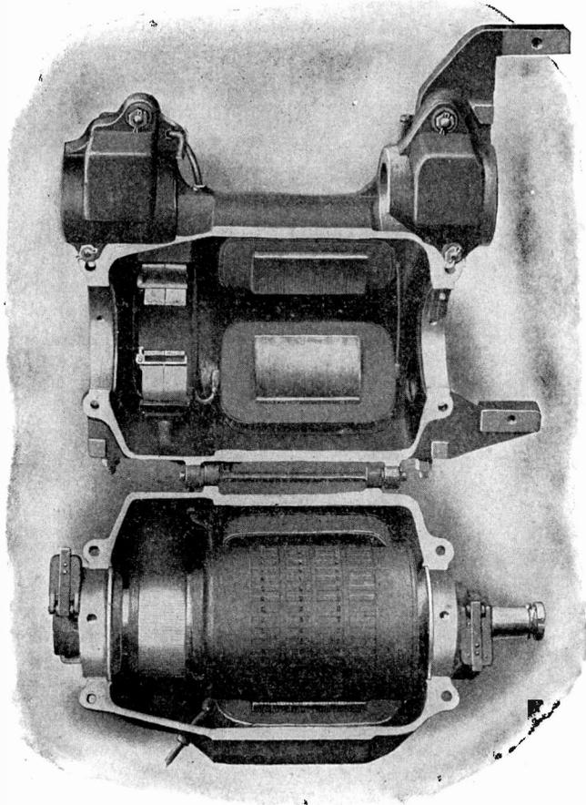
Fig. 32. Westinghouse Railway Motor—Lower Field Down
