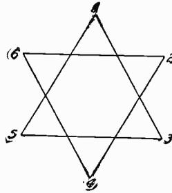
Fig. 36. " $\Delta$ " Diagram of Six-Phase Transformer Secondary Circuits
