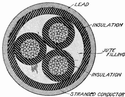
Fig. 50. Section of Polyphase Cable
