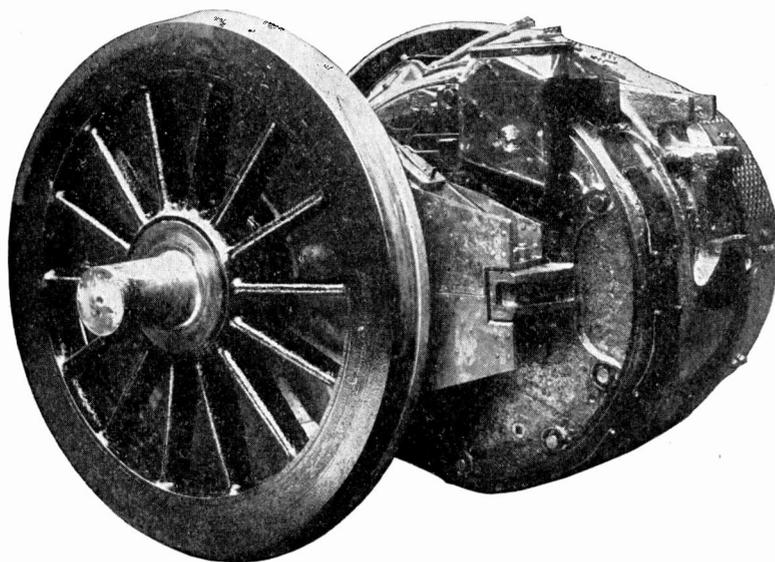
Fig. 264. Grand Trunk Locomotive Motor Mounted on Driving Wheels
