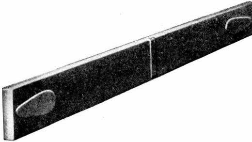
Fig. 230. Steel Bar for Electrically Welded Joint
