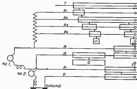
Fig. 54. Development of Controller Connections—Motors in Parallel
