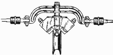
Fig. 220. Section of Block Switch
