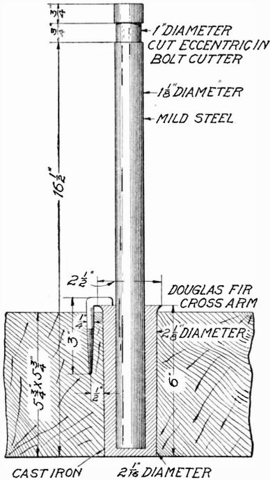
Fig. 42. Iron Pin Showing Dimensions
