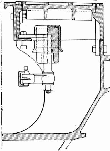
Fig. 242. Section of Underground Conduit Showing Handhole
