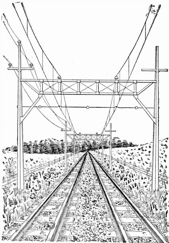
Fig. 199. Catenary System on Light Brace Construction
