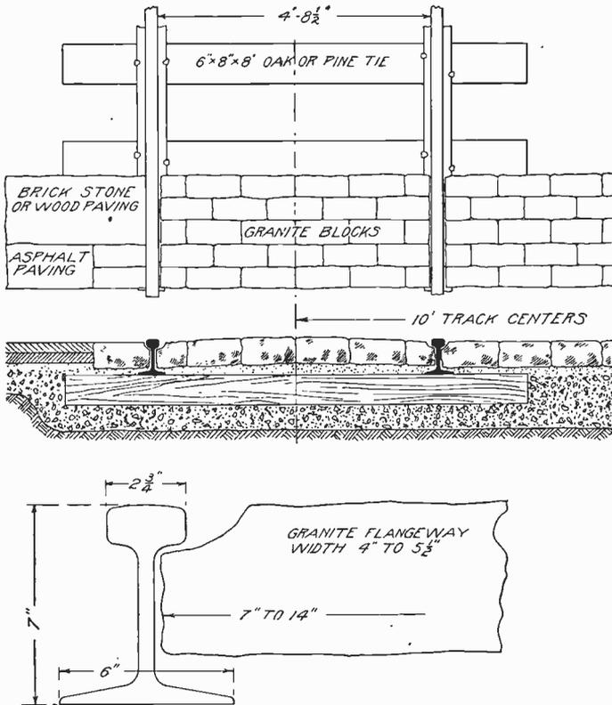
Fig. 221. Plan and Section of Typical City Track
