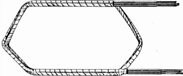
Fig. 36. Armature Coil
