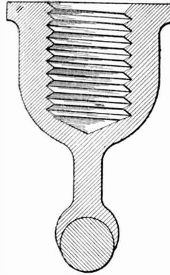
Fig. 185. Section of Ear with Trolley Wire Soldered in Place
