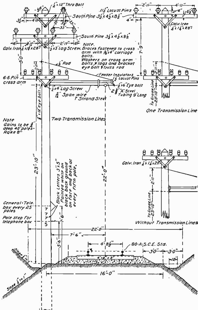
Fig. 172. Diagram of Construction of Single-Track Interurban Trolley Road
