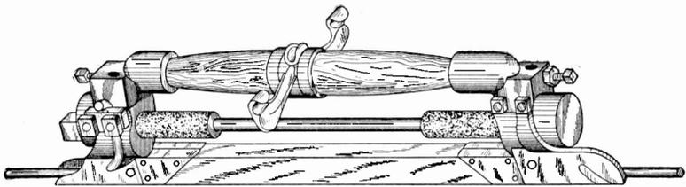
Fig. 189. Details of Section Insulator Used at Intervals in Trolley Line
