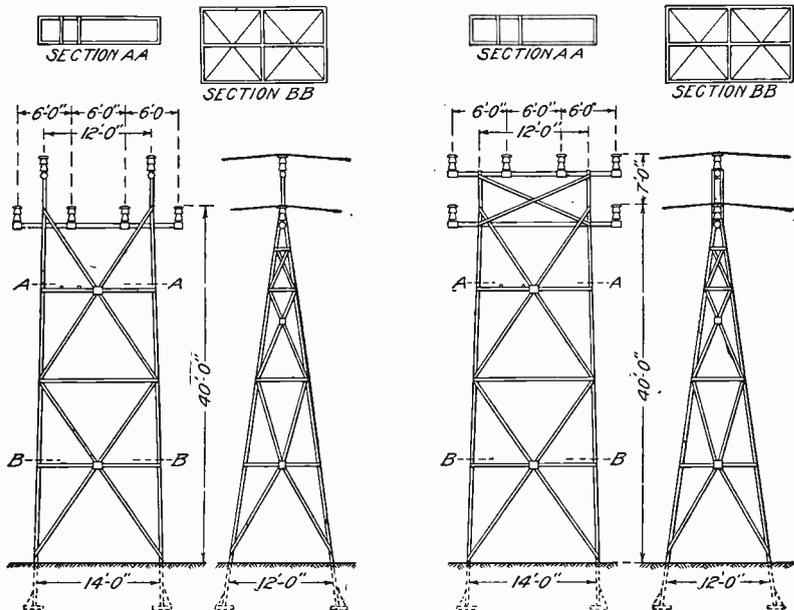
Fig. 39. Plan and Elevation of Steel Tower
