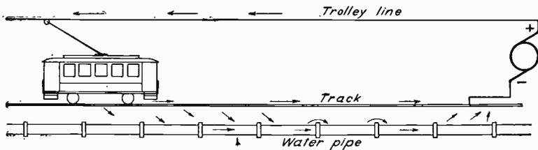
Fig. 210. Diagram Showing Stray Current to Water Pipe
