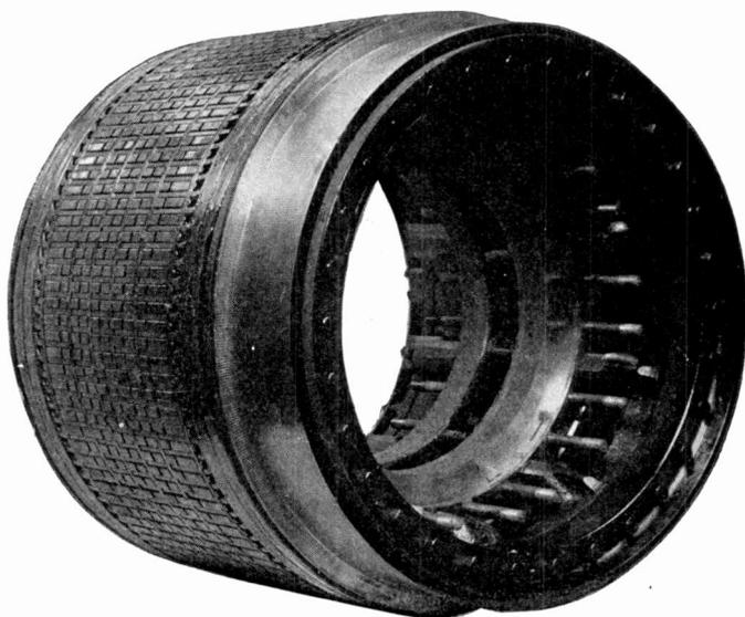
Fig. 253. Armature and Commutator of Pennsylvania Motor
