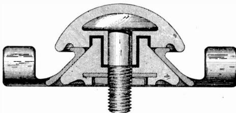
Fig. 182. Cross-Section of Hanger Showing Construction
