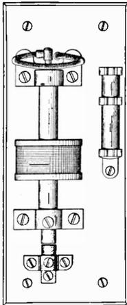
Fig. 125. Typical Form of Lightning Arrester
