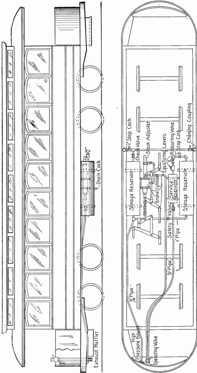
Fig. 98. Diagram of Storage Air-Brake Equipment
