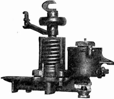
Fig. 69. Westinghouse Unit Switch Cylinder and Magnet Valve
