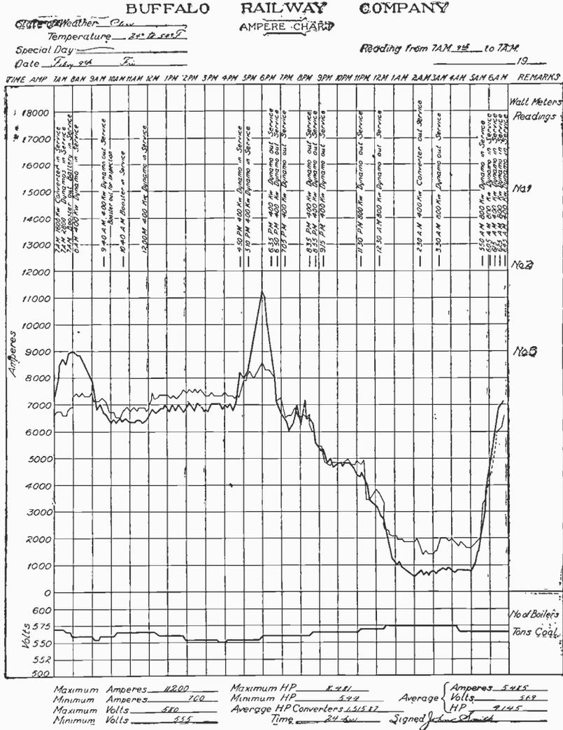
Fig. 142. Load Diagram for Large System
