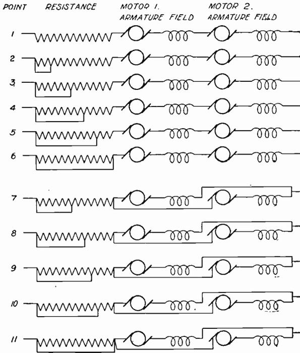
Fig. 48. Controller Diagram
