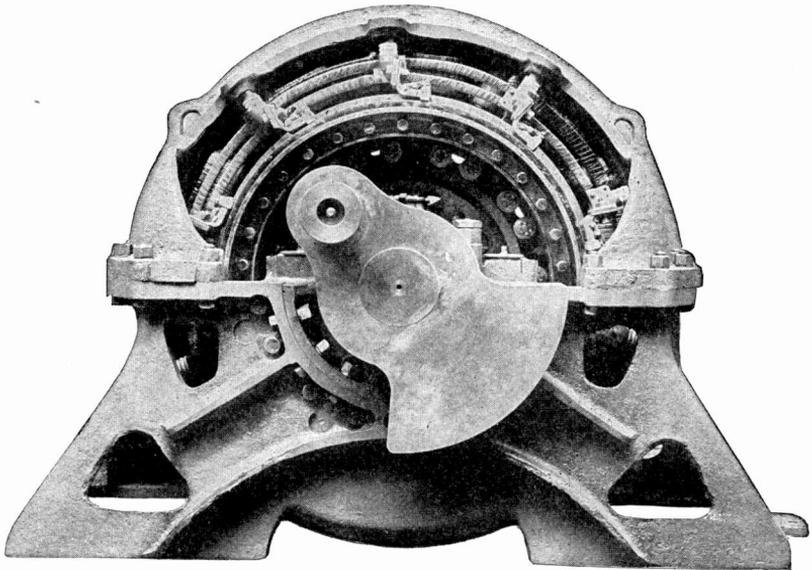
Fig. 252. Side View of Pennsylvania Locomotive Motor
