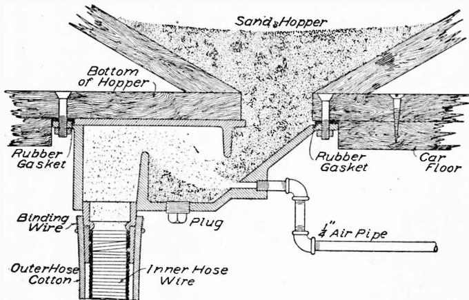
Fig. 123. Section of Pneumatic Sander
