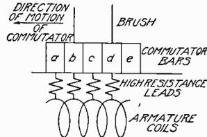
Fig. 51. High-Resistance Commutator Leads
