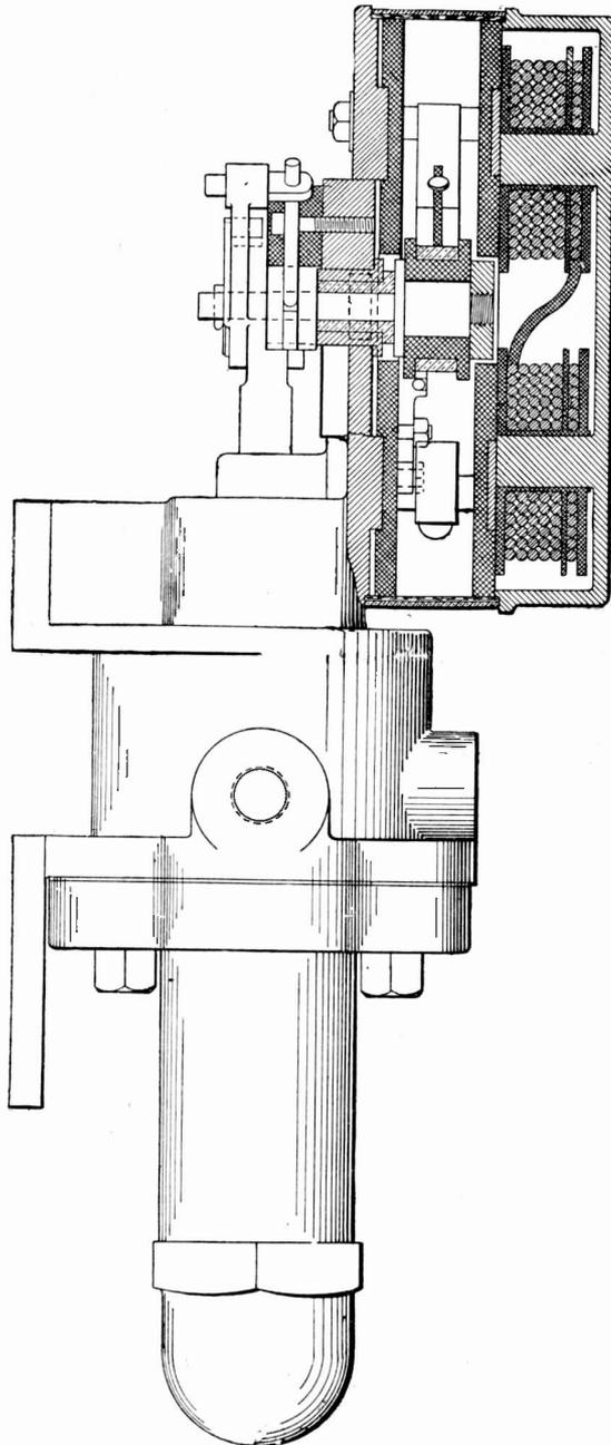
Fig. 91. Part Section of Pump Governor
