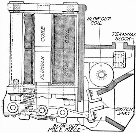
Fig. 60 Sprague-General Electric Contactor Diagram
