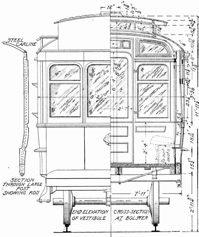
Fig. 3. End View and Cross-Section of Interurban Car
