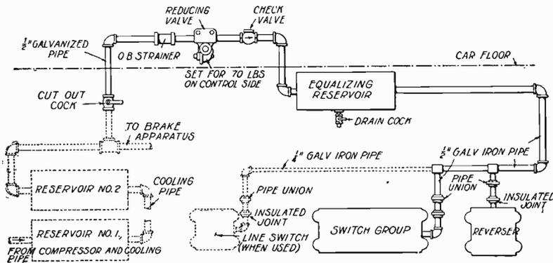
Fig. 73. Piping Diagram, Westinghouse Multiple-Unit System
