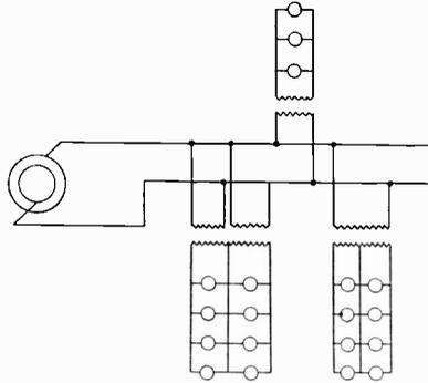
Fig. 15. Single-Phase System with Secondary 3-Wire System
