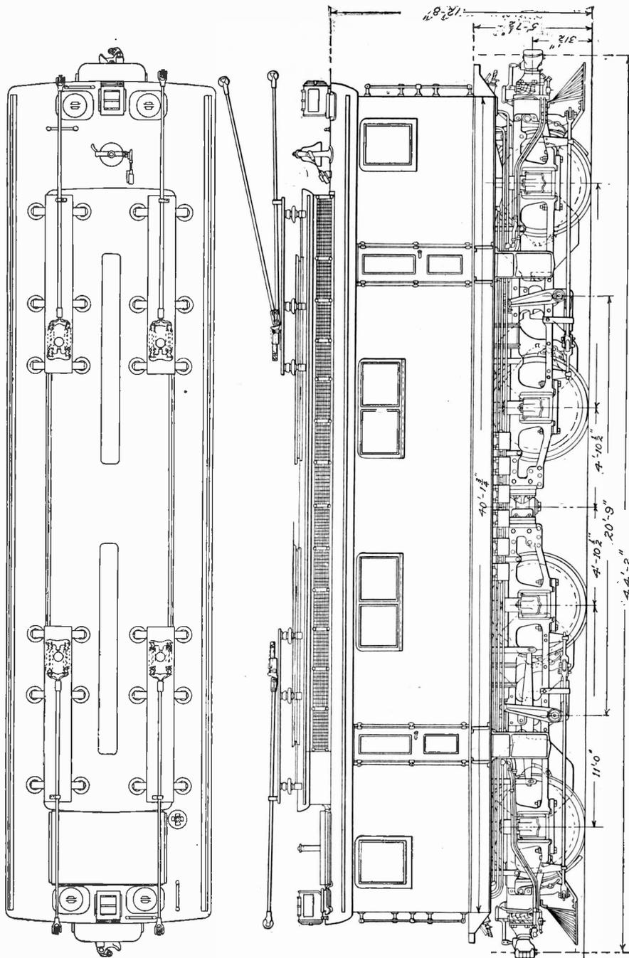
Fig. 267. Plan and Elevation of Great Northern Locomotive
