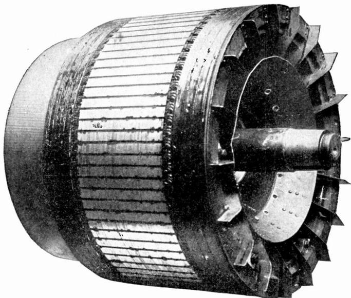
Fig. 263. Armature of Motor Shown in Fig. 261
