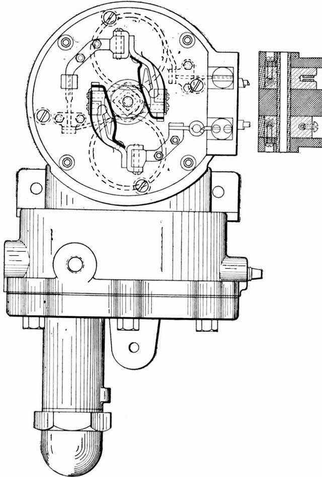
Fig. 89. Front View of Pump Governor
