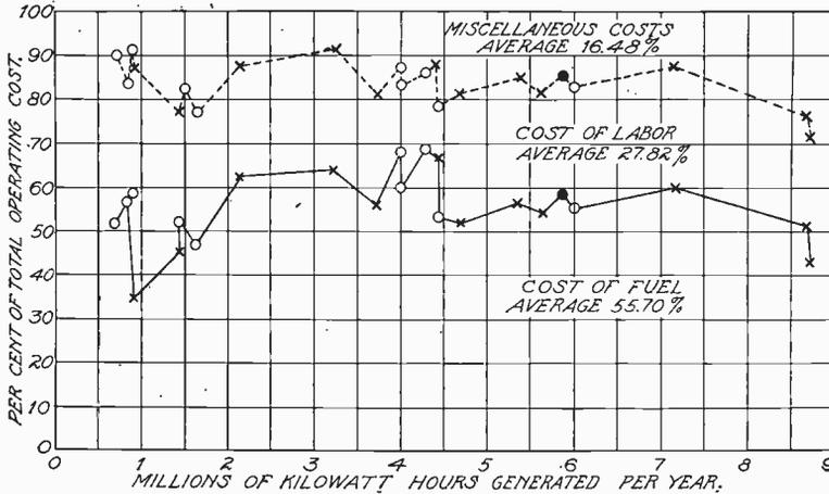
Fig. 162. Curve Showing Per Cent of Total Cost of Fuel, Labor, and Sundries for Given Quantity of Energy Generated Per Year
