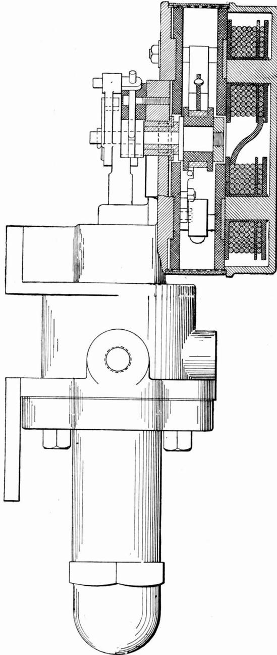
Fig. 91. Part Section of Pump Governor
