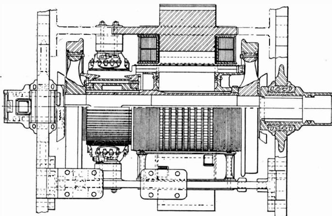
Fig. 247. Side Section of Motor Used on Locomotive Shown in Fig. 246.
