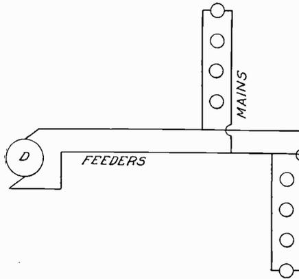
Fig. 5. Diagram of "Feeder and Main" System
