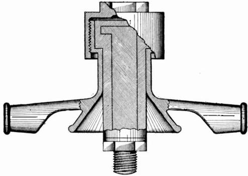
Fig. 183. Section of a Hanger
