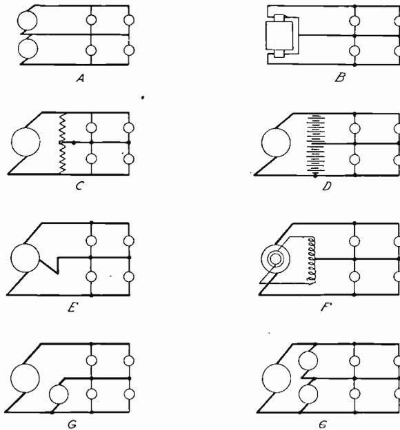
Fig. 13. Diagrams of 3-Wire Generating Methods
