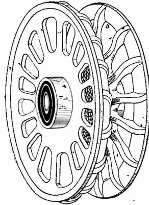
Fig. 107. Special Form of Trolley Wheel for Cutting Sleet
