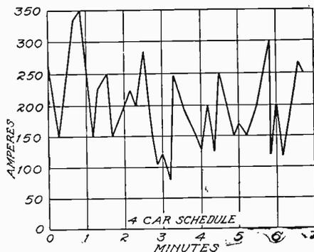
Fig. 141. Load Diagram for Small System
