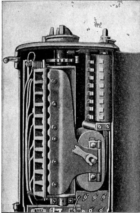
Fig. 77. Current Limit Relay Used by Denver Railway Company
