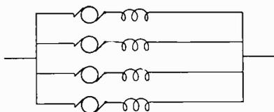
Fig. 50. Motors in Parallel
