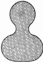
Fig. 180. Section of a "Figure 8" Trolley Wire
