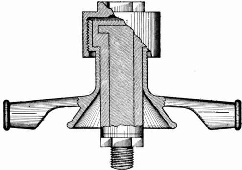
Fig. 183. Section of a Hanger
