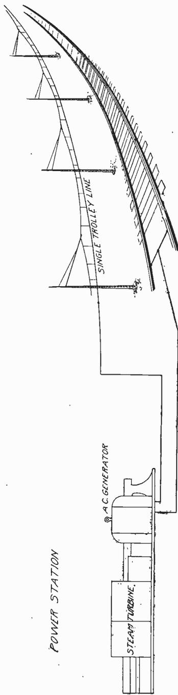
Fig. 170. Diagram of High-Tension Circuit Going Directly to the Cars, through Transformers into Single-Phase Series Motor
