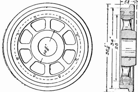
Fig. 24. Steel-Tired Wheel
