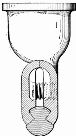
Fig. 187. Section Through Clamp Shown in Fig. 186
