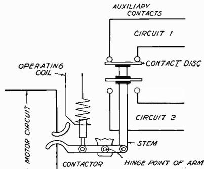
Fig. 62. Diagram of Sprague-General Electric Interlock
