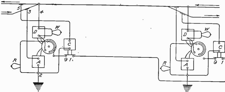
Fig. 213. Diagram of Automatic Block Signal System
