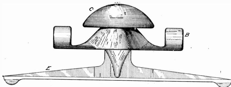
Fig. 181. Hanger and Ear for Round Trolley Wire
