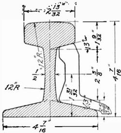
Fig. 222. Section of 65-pound T Rail
