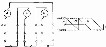
Fig. 4. Brush Multiple Circuit Arc Machine Connections
