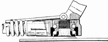
Fig. 103. Ball-Bearing of Fig. 102 in Detail
