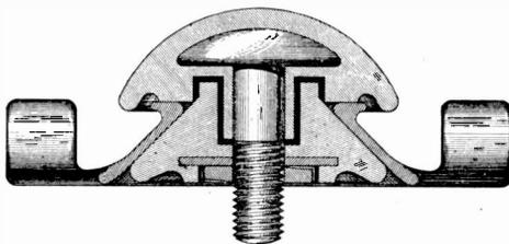
Fig. 182. Cross-Section of Hanger Showing Construction
