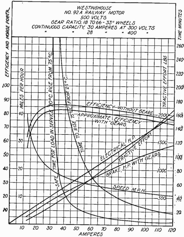
Fig. 47. Characteristic Curves—Westinghouse Railway Motor
