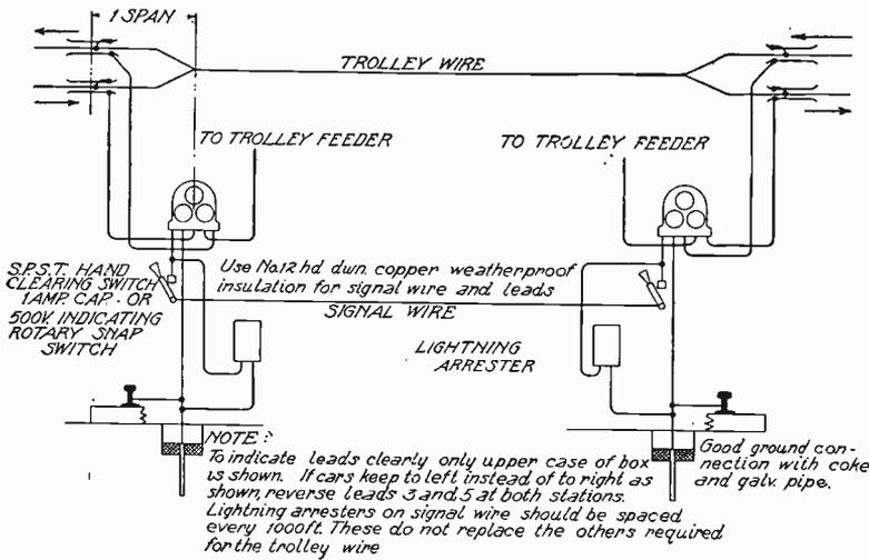
Fig. 214. Diagram of Automatic Block Signal System
