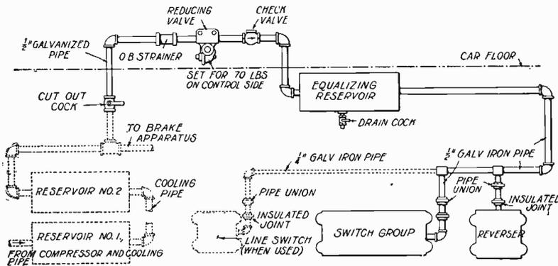
Fig. 73. Piping Diagram, Westinghouse Multiple-Unit System
