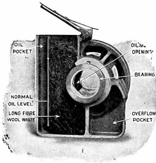
Fig. 41. Cross-Section of Bearing Housing
