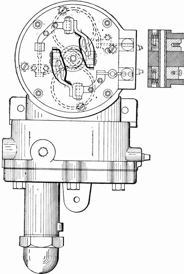
Fig. 89. Front View of Pump Governor
