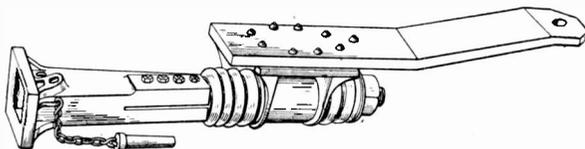
Fig. 119. Drawbar of a Simple Coupler
