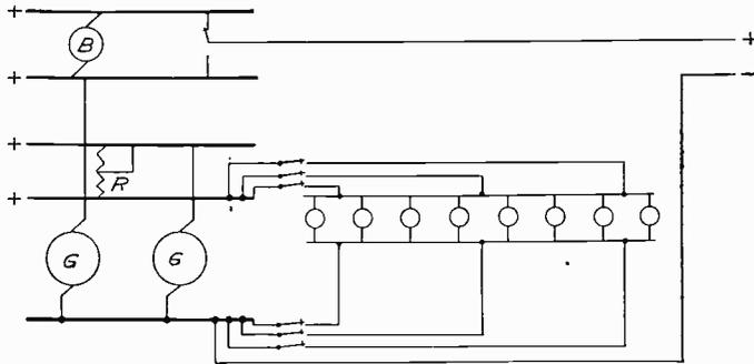
Fig. 14. Diagram of Connections for Voltage Regulation
