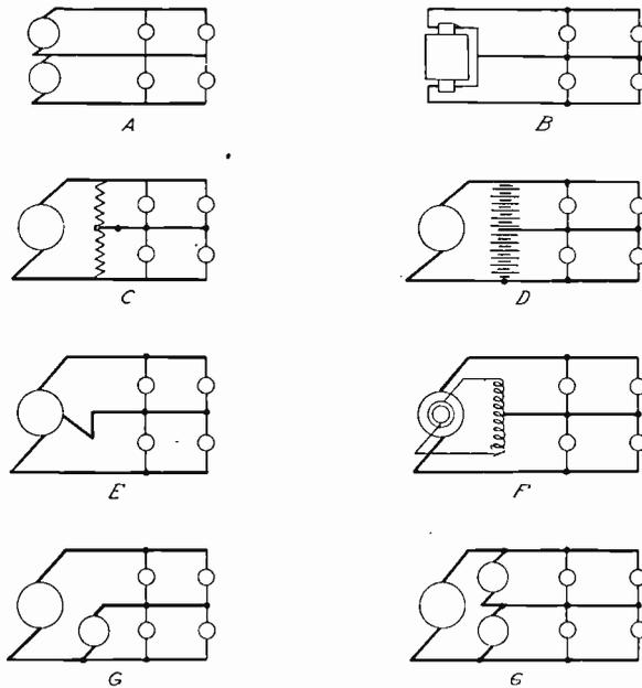
Fig. 13. Diagrams of 3-Wire Generating Methods
