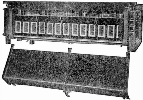
Fig. 61. Group of Sprague-General Electric Unit Switch
