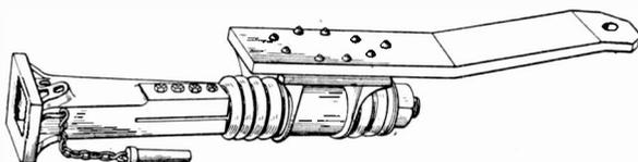
Fig. 119. Drawbar of a Simple Coupler
