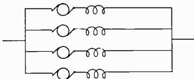
Fig. 50. Motors in Parallel
