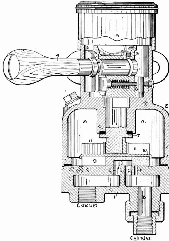
Fig. 93. Section of Air Operating Valve
