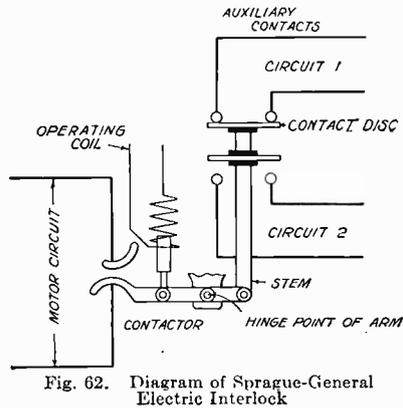
Fig. 62. Diagram of Sprague-General Electric Interlock
