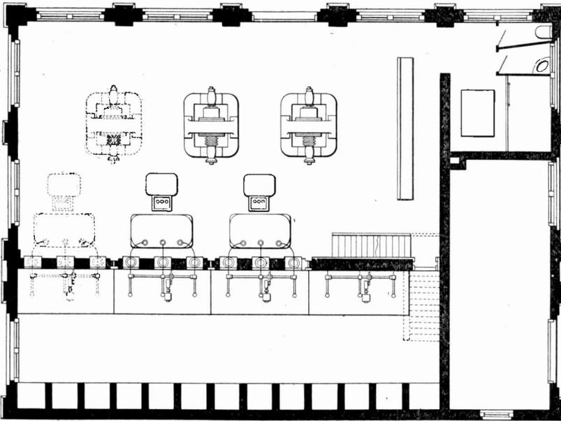
Fig. 168. Plan of Substation of West Shore Railroad
