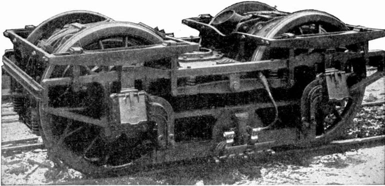
Fig. 257. End View of Truck Showing Spring Supports for Motor
