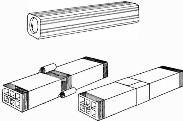
Fig. 47. Single- and Multiple-Duct Tile Conduits
