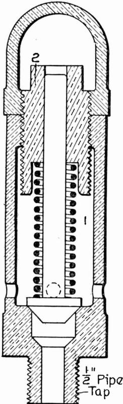
Fig. 97. Section of Safety Valve
