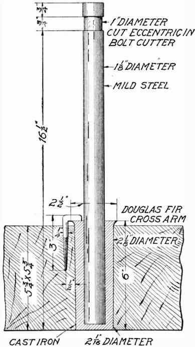
Fig. 42. Iron Pin Showing Dimensions
