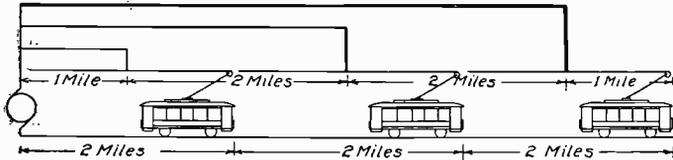
Fig. 209. Feeder System Using Separate Trolley Sections
