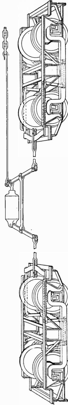
Fig. 84. Brake-Lever and Air-Brake Attachment for Double-Truck Car
