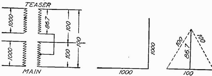
Fig. 32. Diagram of Scott Connections and Vector Diagrams for Same
