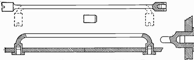
Fig. 205. Channel Pins of "Chicago" Type
