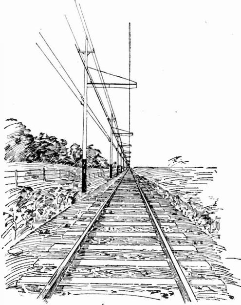
Fig. 194. Bracket Line Construction
