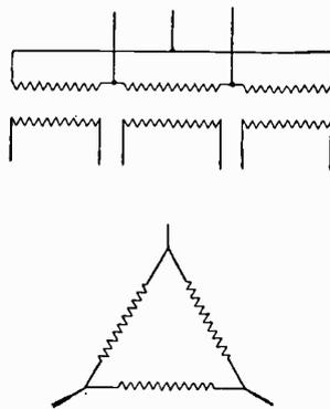
Fig. 30.  $\Delta$  Connections for Transformers
