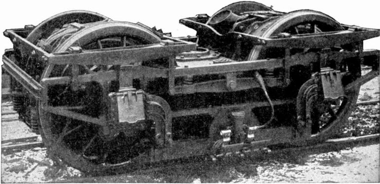
Fig. 257. End View of Truck Showing Spring Supports for Motor
