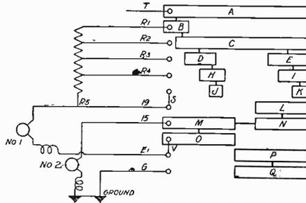
Fig. 53. Development of Controller Connections—Motors in Series
