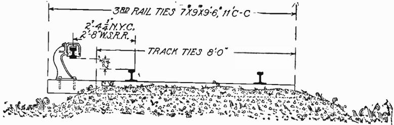
Fig. 203. Inverted Rail Insulator Mounted on Tie
