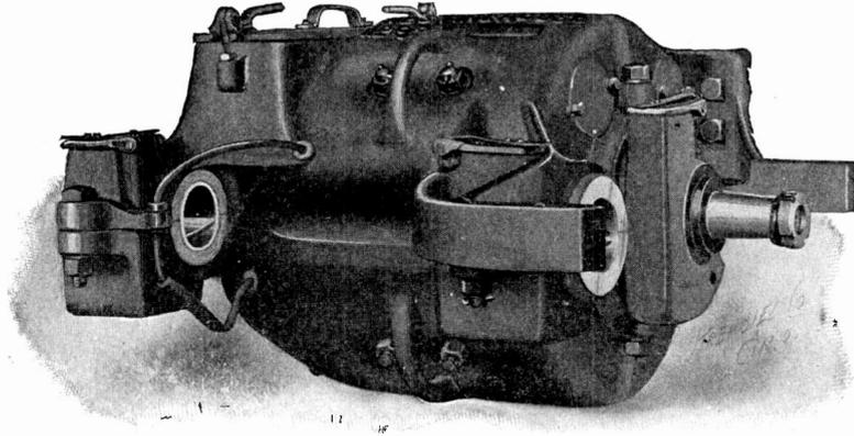
Fig. 30. Westinghouse Railway Motor, 35 H. P.
