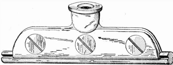
Fig. 186. Clamp Used with Groove Trolley Wire
