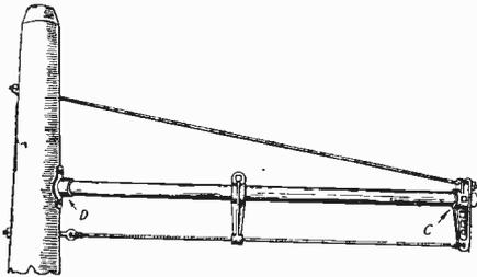
Fig. 195. One Type of Bracket for Trolley Line
