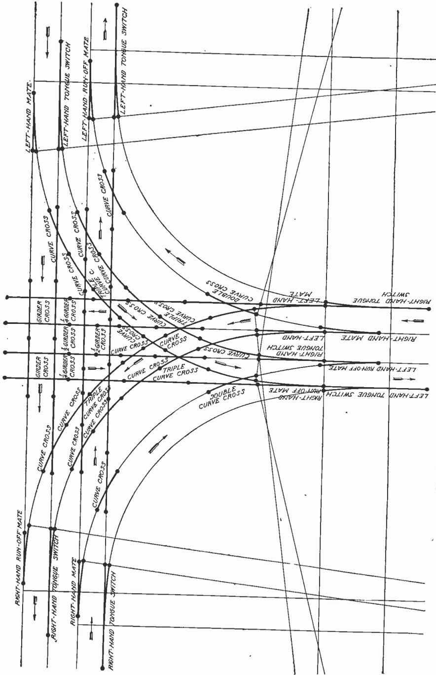
Fig. 238. Double Track Crossing with Connecting Curves
