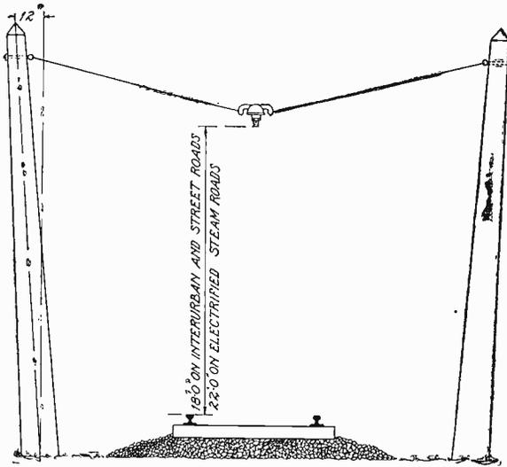
Fig. 191. Span Construction for Single Trolley Wire
