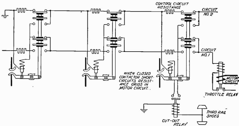
Fig. 66. Diagram of Interlocks, Sprague-General Electric Automatic Control
