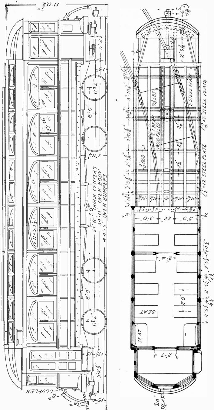
Fig. 2. Plan and Elevation of Interurban Car
