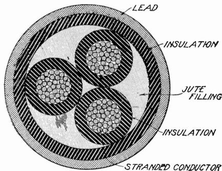
Fig. 50. Section of Polyphase Cable
