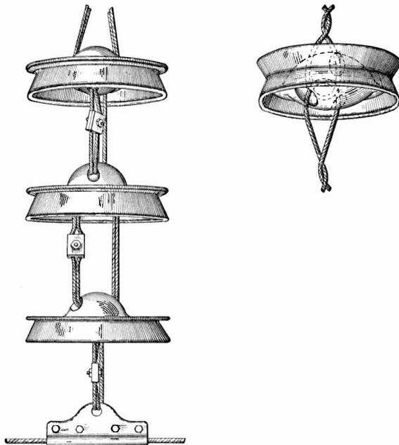
Fig. 40. Suspended or Disk Type of Insulator
