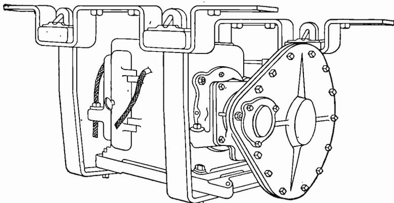
Fig. 88. Westinghouse Air Compressor Complete
