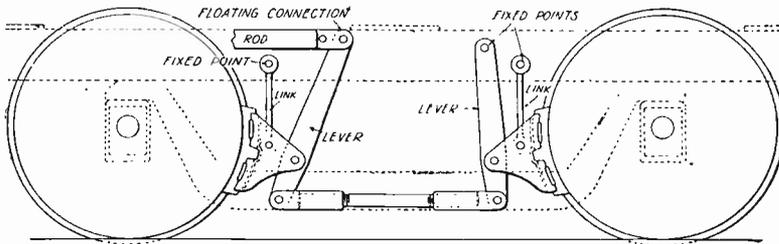
Fig. 80. Brake Mechanism, Showing Brake-Head, Shoes, and Hanger
