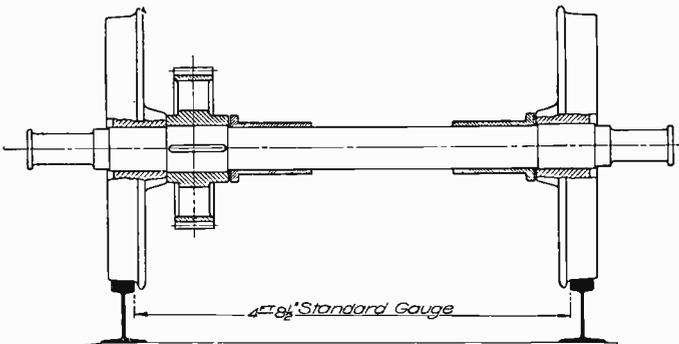
Fig. 26. Part Section of Wheels, Axle and Gear
