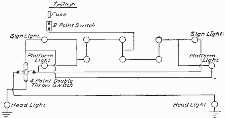
Fig. 114. Wiring Diagram for Car Lighting System
