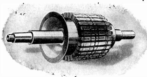
Fig. 35. Armature Core
