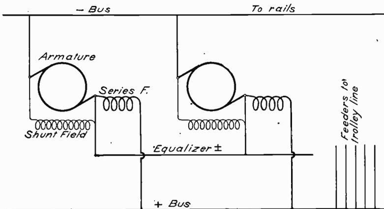
Fig. 150. Diagram of Connections for Direct-Current Power Plants
