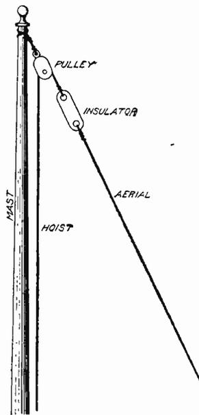
Fig. 41. Single Wire Experimental Aërial
