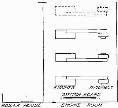
Fig. 47. Diagram of Simple Arrangement of Belted Machines
