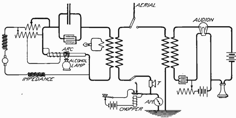
Fig. 19. Operating Circuits of the DeForest System
