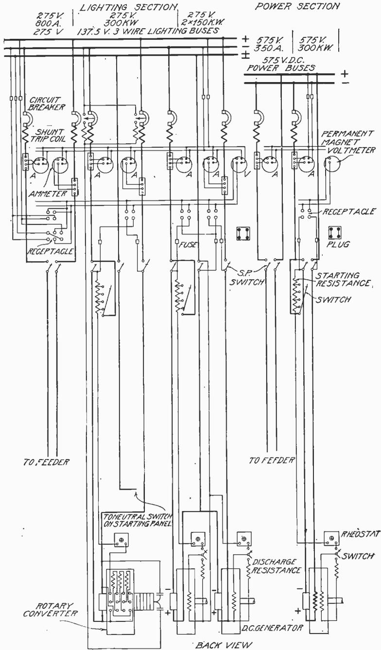
Fig. 39. Wiring Diagram for Standard Switchboard
