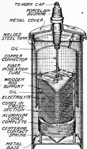
Fig. 38. Cross-Section of Aluminum Arrester
