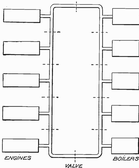
Fig. 2. Diagram of *Ring* System of Piping
