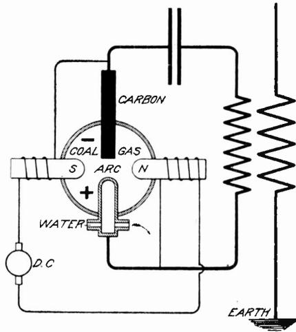
Fig. 36. Poulsen Direct-Current Method of Generating Oscillations
