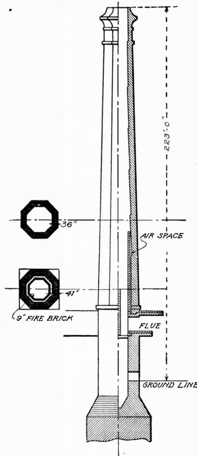
Fig. 7. Good Design of Brick Chimney
