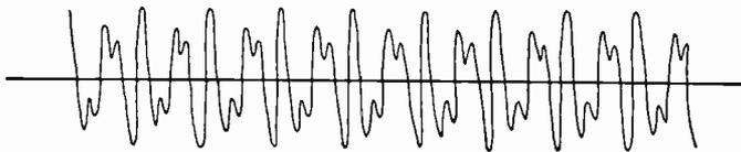
Fig. 5. Oscillogram of a Telephone Current
