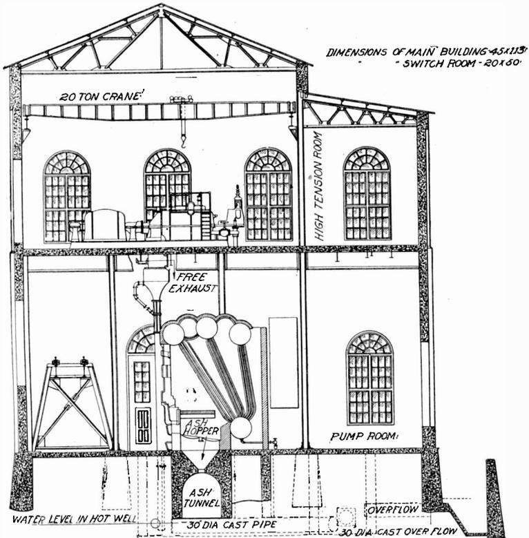
Fig. 53. Double-Deck Turbine Plant
