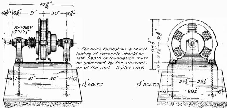
Fig. 46. Foundation for Rotary Converter
