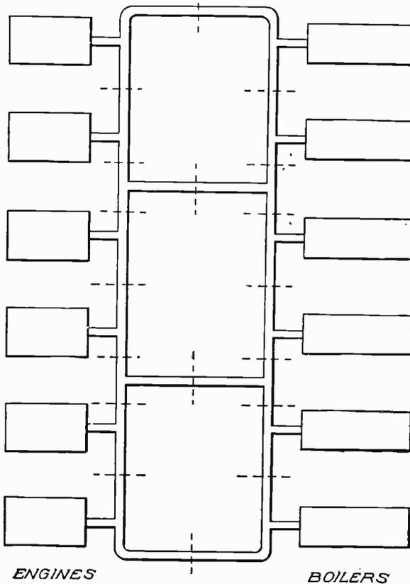
Fig. 3. Diagram of *Ring System with Cross-Connections*
