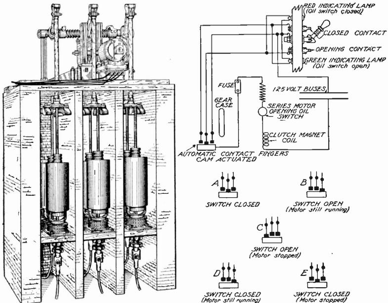
Fig. 29. Form of Oil Switch for High Potentials
