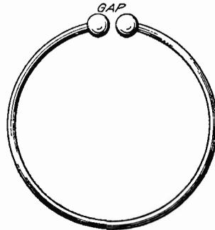
Fig. 6. Hertz Resonator
