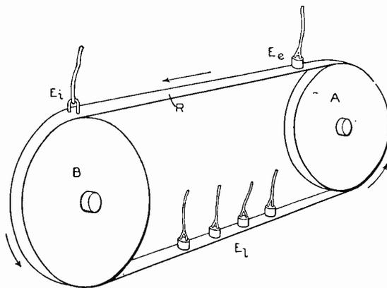
Fig. 6. Arrangement for Multiplex Transmission of Telegraphic Messages.
