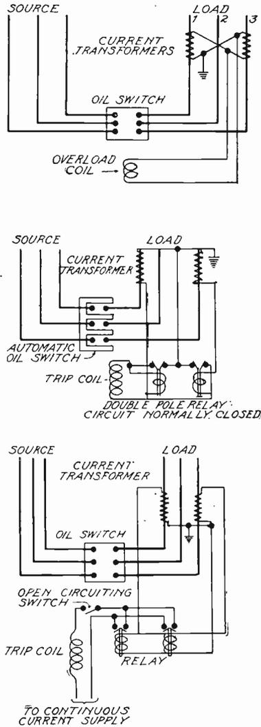
Fig. 30. Wiring Diagram for Tripping Devices
