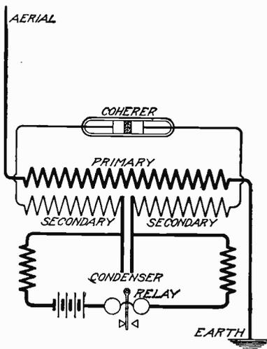
Fig. 19. Marconi Receiver-Circuit with Jigger
