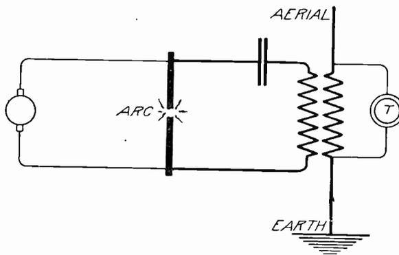
Fig. 10. Transmitter Shunted across the Aërial Inductance
