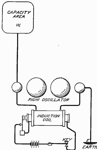
Fig. 15. Diagram Showing the Earthed Oscillator
