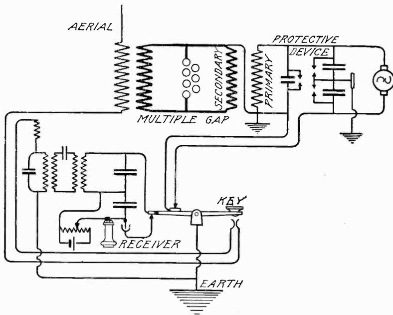
Fig. 65. Stone Sending and Receiving Circuits
