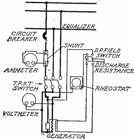
Fig. 21. Wiring Diagram of D. C. Generator Panel
