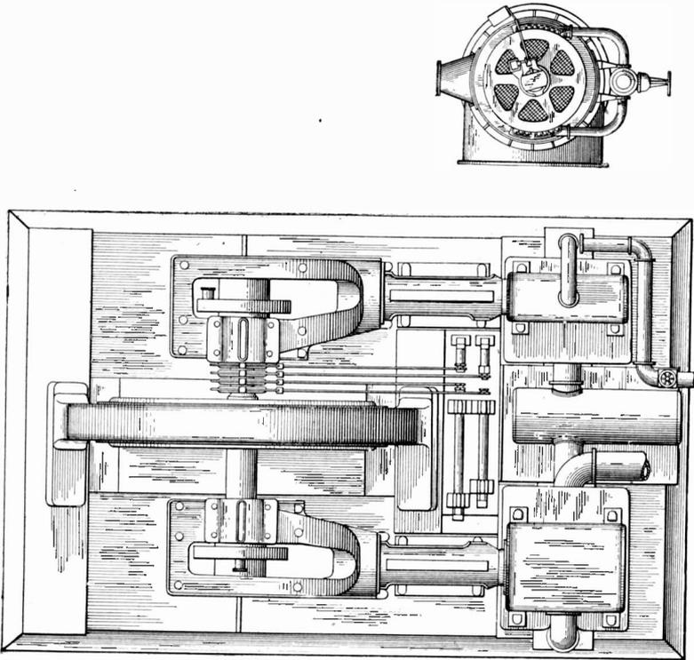
Fig. 54. Space Occupied by Turbo-Alternator Compared with that of Generator and Reciprocating Engine of Same Capacity
