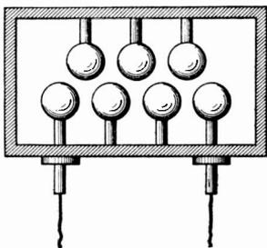
Fig. 31. Multiple-Ball Exciter
