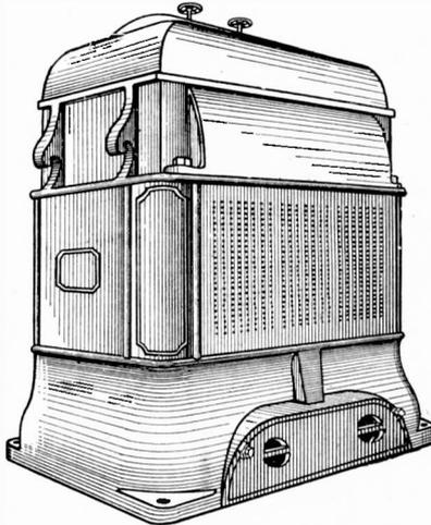
Fig. 14. Air-Cooled Transformer
