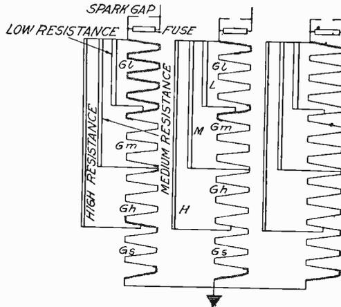
Fig. 34. Non-Inductive Resistances in Shunt with Lightning Arrester
