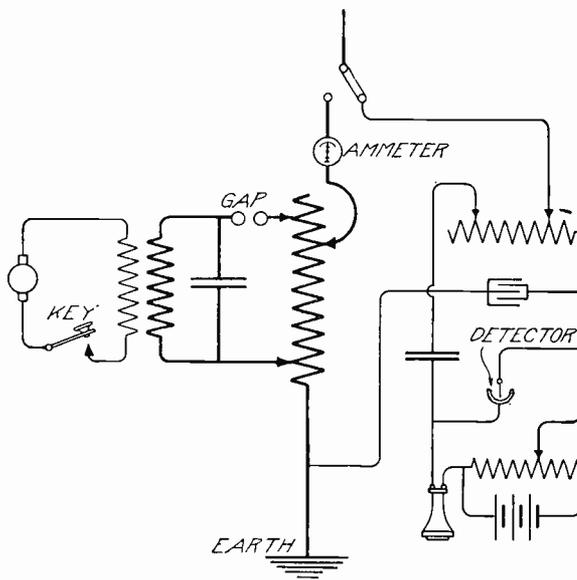
Fig. 66. Massie Sending and Receiving Circuits
