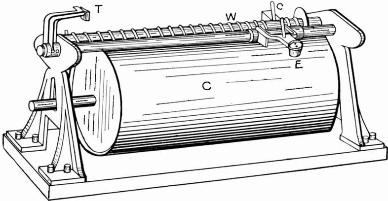
Fig. 2. Early Model of Telegraphone, Wire Type.
