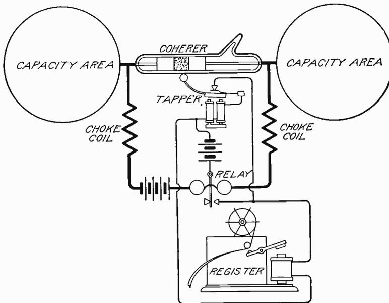
Fig. 13. Early Marconi Receiving Circuit
