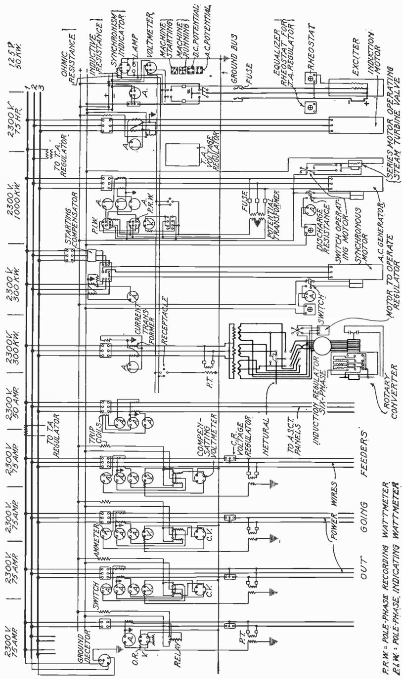
Fig. 40. Wiring Diagram for Standard Switchboard
