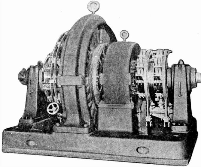
Fig. 41. Rotary Converter Equipped with Regulating Generator
