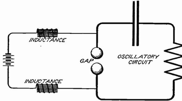
Fig. 34. Thomson Direct-Current Method of Generating Oscillations
