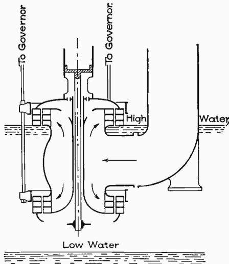
Fig. 11. Diagram of Reaction Turbines
