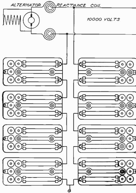
Fig. 33. Connections for 10,000-Volt Lightning Arrester
