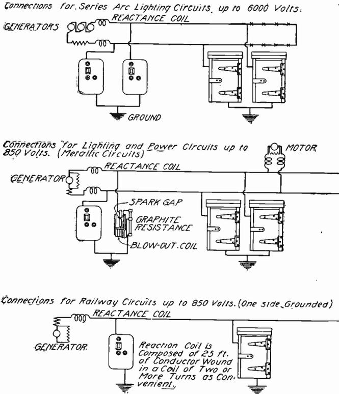
Fig. 32. Lightning-Arrester Diagrams of D. C. Work
