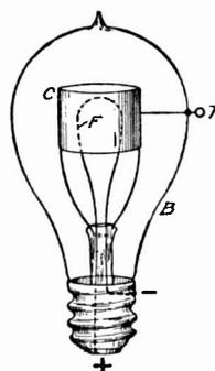
Fig. 47. Fleming Glow-Lamp Detector
