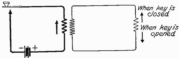
Fig. 13. Induction-Coil Action
