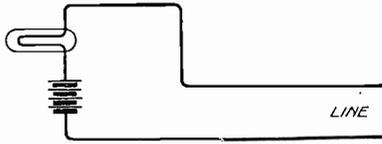
Fig. 26. Lamp Signal Directly in Line
