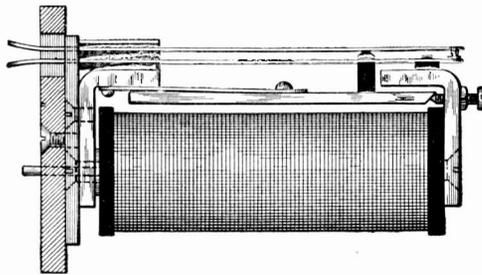
Fig. 204. Type of Cut-Off Relay
