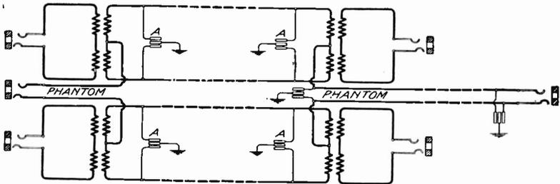
Fig. 227. Phantom Extended by Physical Circuit
