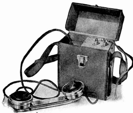
Fig. 252. Portable Telephone Set
