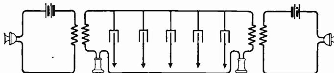
Fig. 31. Test of Line with Varying Shunt Capacity
