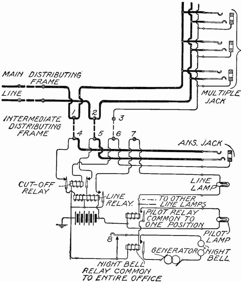
Fig. 190. Line Circuit No. 1 Board
