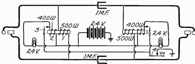
Fig. 139. Cord Circuit with Double Lamp Signals
