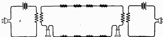
Fig. 34. Test of Line with Varying Serial Inductance
