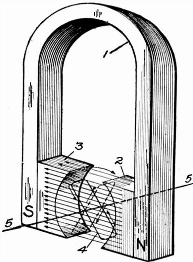
Fig. 60. Principles of Magneto Generator
