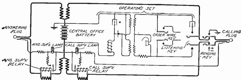
Fig. 188. Cord Circuit Western Electric No. 1 Board
