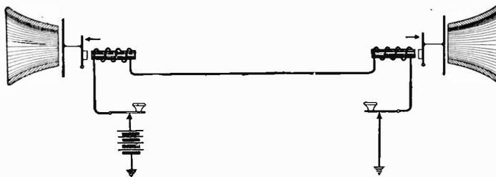
Fig. 6. Telegraph Equipment Converted into Telephone Equipment
