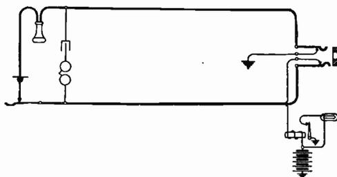
Fig. 157. Line Lamp with Relay
