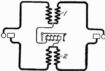
Fig. 134. Cord Circuit with Differential Windings
