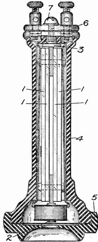
Fig. 49. Single-Pole Receiver
