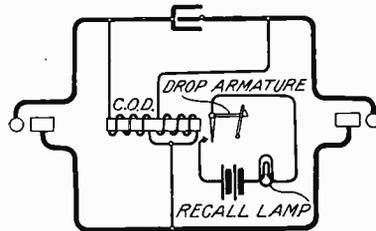
Fig. 138. Cord Circuit with Recall Lamp
