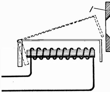
Fig. 23. Electromagnetic Visible Signal
