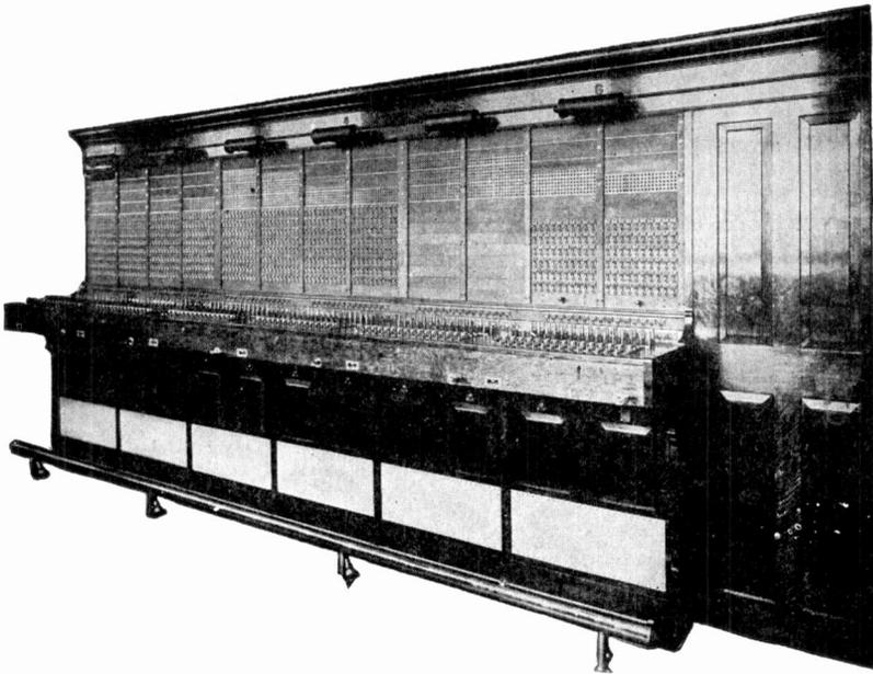
Fig. 183. Magneto Multiple Switchboard
