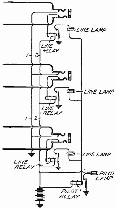
Fig. 158. Pilot-Lamp Operation
