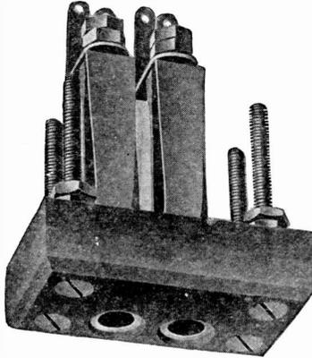
Fig. 119. Operator's Cut-In Jack
