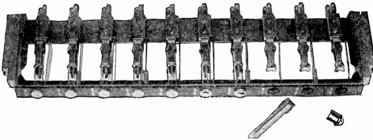
Fig. 164. Line Lamp Mounting
