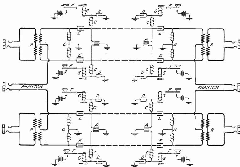
Fig. 235. Phantom of Two Composite Circuits
