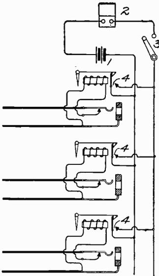
Fig. 122. Night-Alarm Circuit
