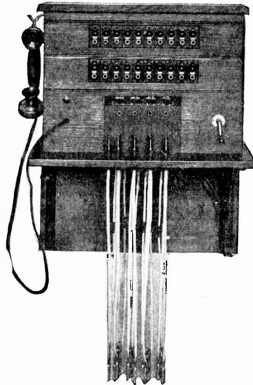
Fig. 151. Sectional Switchboard—Wall Type
