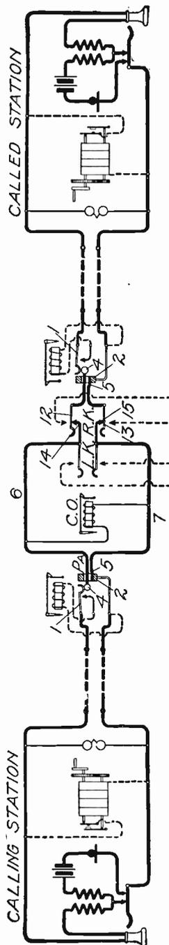
Fig. 92. Subscribers Connected for Conversation
