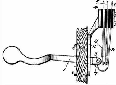
Fig. 76. Short Lever Hook Switch
