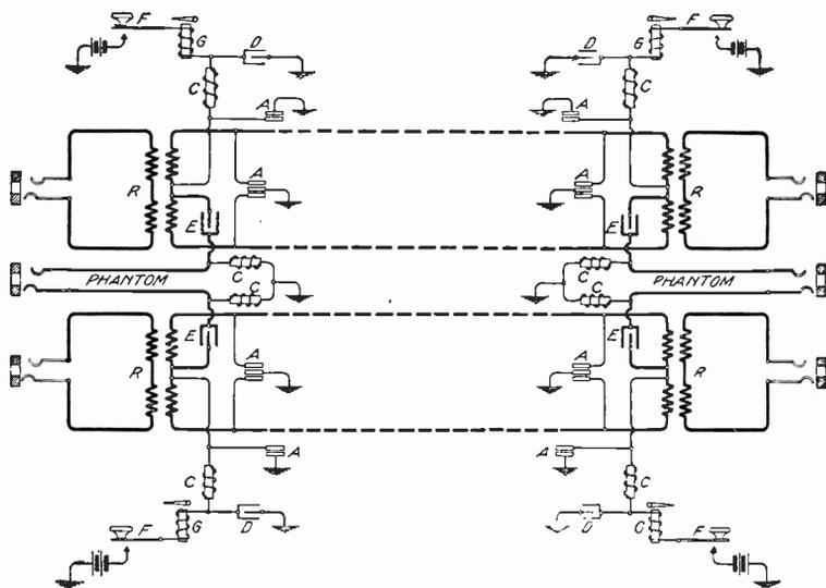
Fig. 234. Phantom of Two Simplex Circuits
