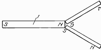
Fig. 18. Extension of a Permanent Magnet
