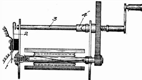
Fig. 67. Generator Cut-In Switch
