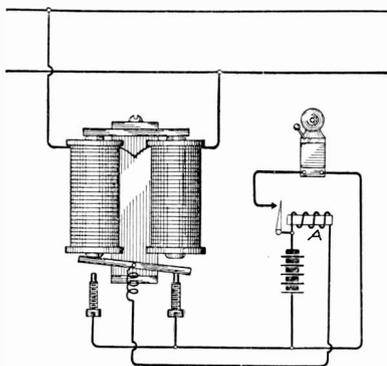
Fig. 236. Ringing Device for Composite Circuits
