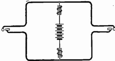
Fig. 159. Battery Supply Through Impedance Coils
