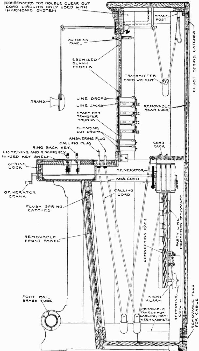
Fig. 145. Cross-Section of Upright Switchboard
