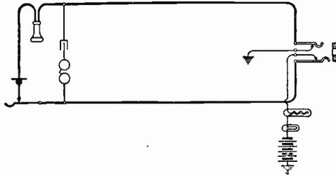
Fig. 156. Direct-Line Lamp with Ballast
