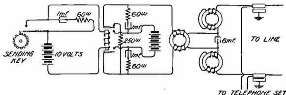
Fig. 253. Dispatcher's Station—Western Electric System
