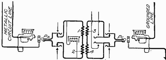
Fig. 127. Connection of Dissimilar Lines through Repeating Coil
