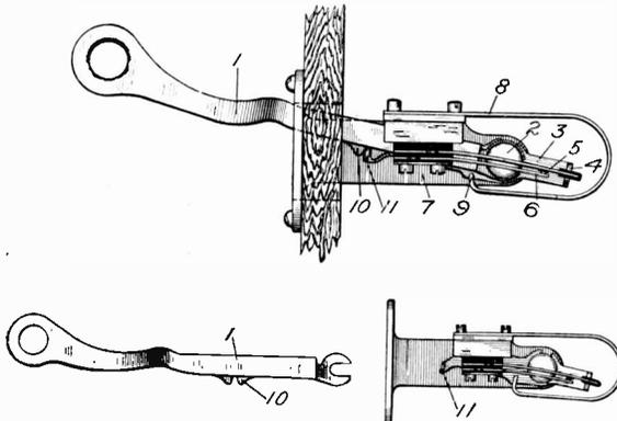
Fig. 77. Removable Lever Hook Switch
