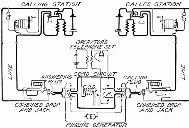
Fig. 121. Circuit of Simple Magneto Switchboard
