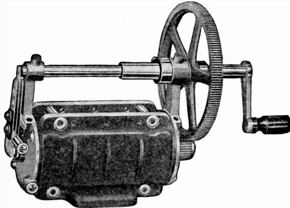
Fig. 64. Generator with Magnets Removed
