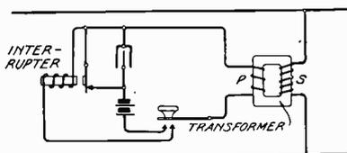
Fig. 237 Ringing Current Device
