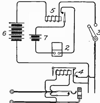
Fig. 123. Night-Alarm Circuit with Relay
