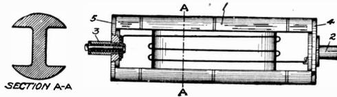
Fig. 62. Generator Armature
