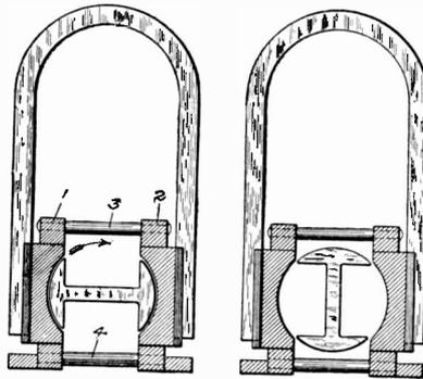
Fig. 63. Generator Field and Armature
