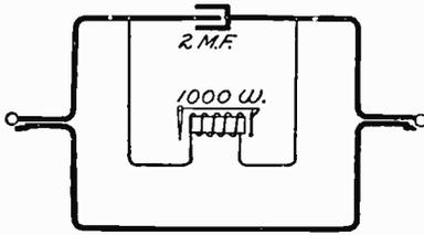
Fig. 130. Series Drop-Cord Circuit
