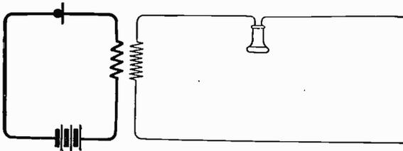
Fig. 12. Conventional Diagram of Talking Circuit
