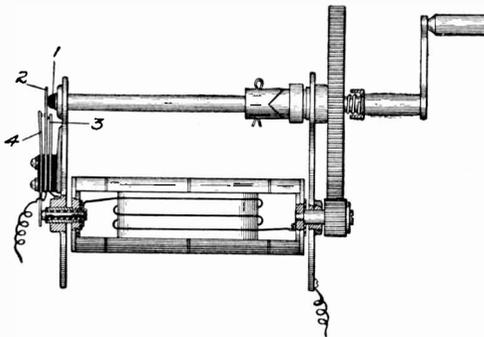
Fig. 68. Generator Cut-In Switch
