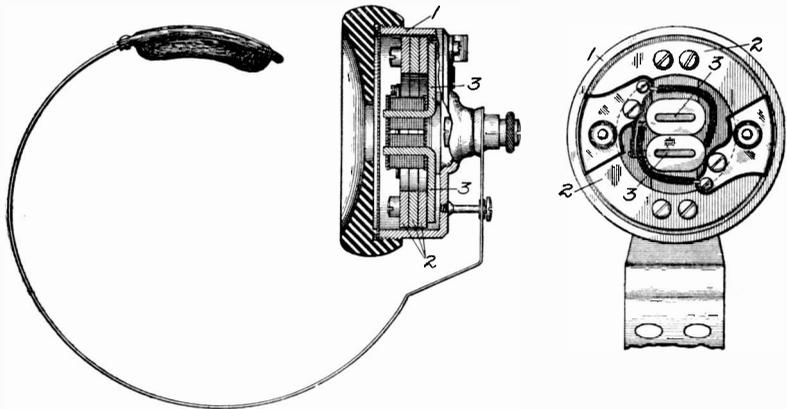
Fig. 57. Operator's Receiver
