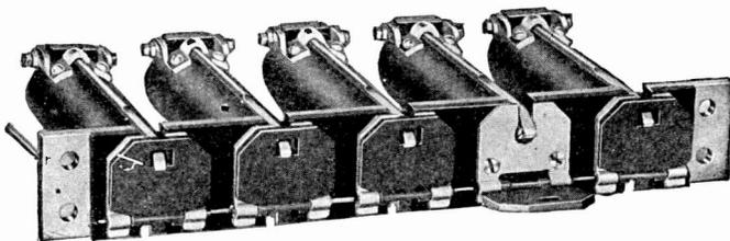
Fig. 96. Strip of Tubular Drops
