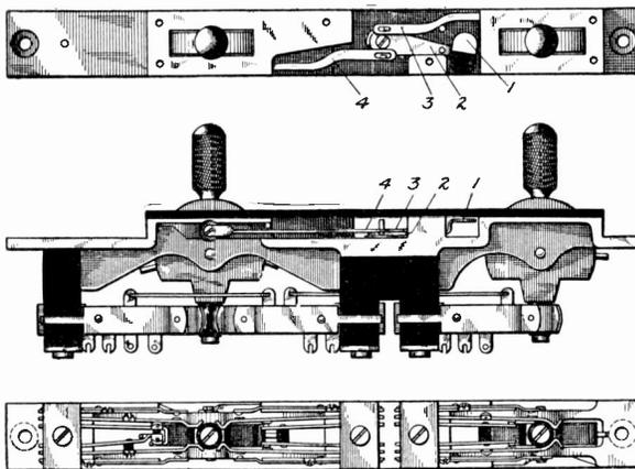
Fig. 114. Horizontal-Spring Listening and Ringing Key
