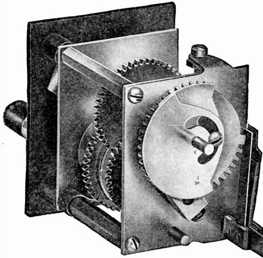
Fig. 243. Dispatcher's Key Mechanism
