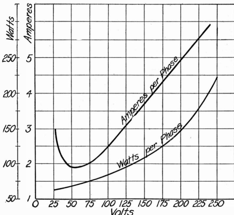
Fig. 356. Running Saturation Curves
