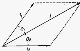
Fig. 5. Vector Diagram of Branched Circuit
