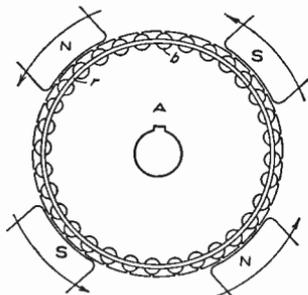
Fig. 320. Squirrel-Cage Rotor Mounted in Ordinary Four-Pole Field
