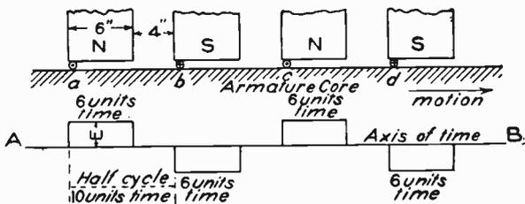
Fig. 78. Development and E. M. F. Curve for a Four-Pole Alternator
