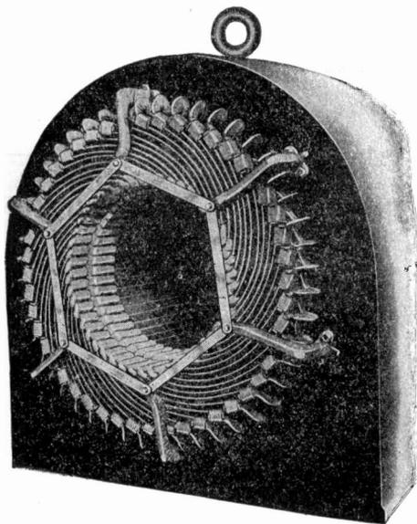
Fig. 151. Method of Bracing Armature Coils
