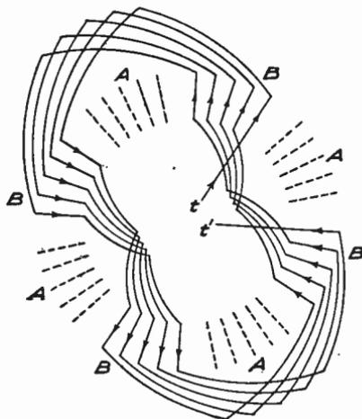
Fig. 322. Diagram of One-Half the Stator Conductors of Fig. 321
