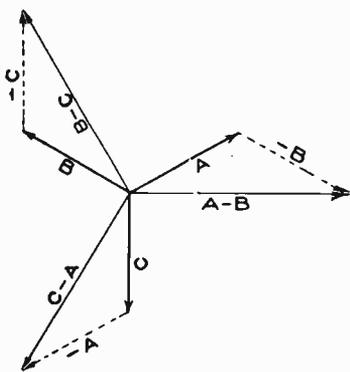
Fig. 100. Clock Diagram of E. M. F.s for Three-Phase "Y" Winding
