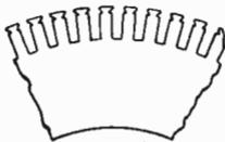
Fig. 111. Portion of Stamping for Twelve-Pole Three-Phase Alternator
