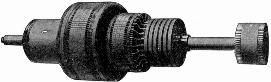
Fig. 302. Rotor of Westinghouse Six-Phase Rotary Converter with Synchronous Regulator
