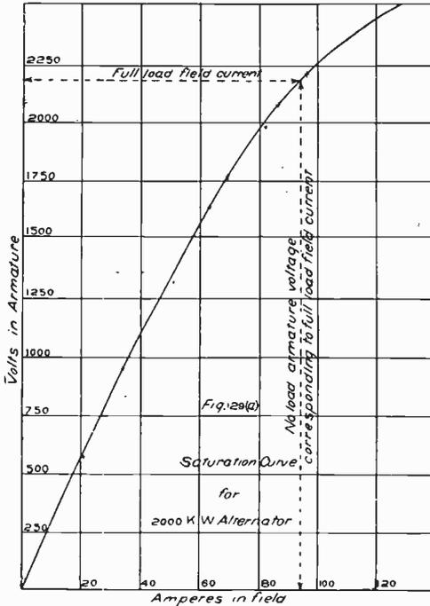
Fig. 161. Saturation Curve for 2000-Kw. Alternator
