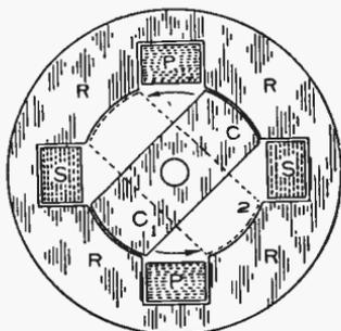
Fig. 392. Diagram of Magnetic Voltage Regulator
