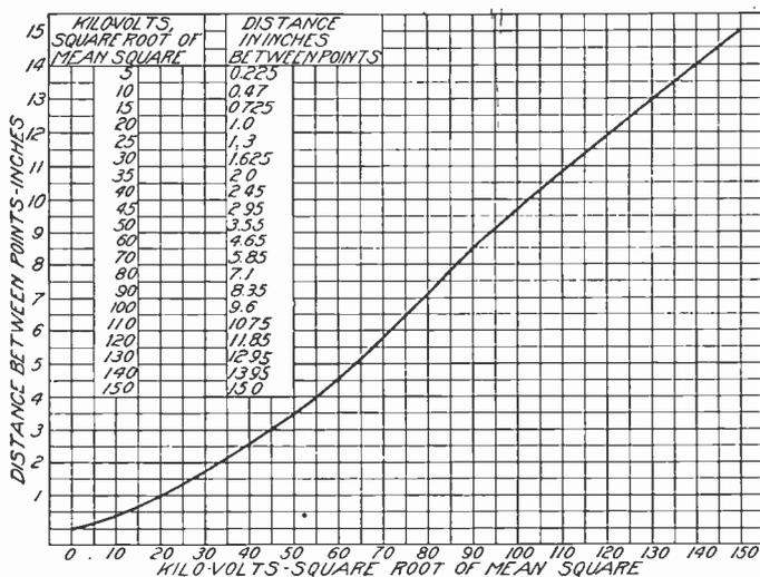
Fig. 159. Curve Showing Relation between Sparking Distance and Voltage
