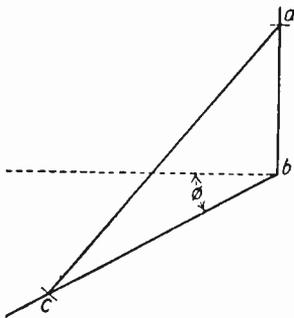
Fig. 168. Terminal Voltage without Reactance
