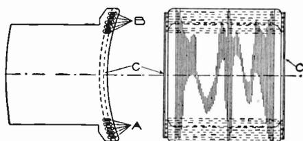
Fig. 301. Diagram Showing Copper Dampers in Place in Field Poles
