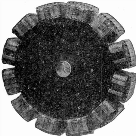
Fig. 141. Rotor of Fig. 140 with Field Coils in Place
