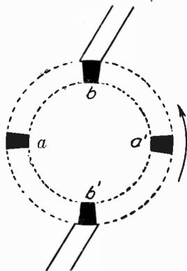
Fig. 291. Brush and Commutator Diagram for Four-Ring Converter
