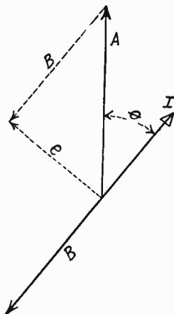
Fig. 186. Effect of Motor Under-Excited, Current Lagging
