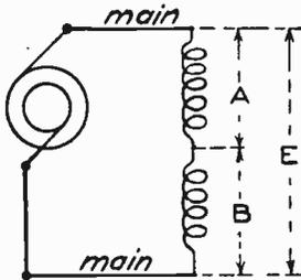
Fig. 37. Diagram of Two Coils in Series with an Alternator
