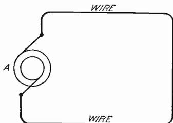
Fig. 10. Simple Alternating Circuit
