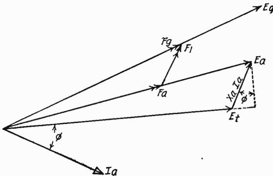
Fig. 173. Potier Construction Diagram
