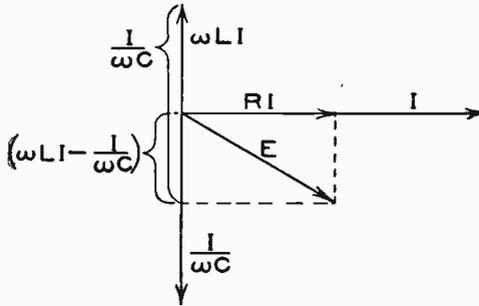
Fig. 48. Conditions of Fig. 45 When Total Reactance is Negative
