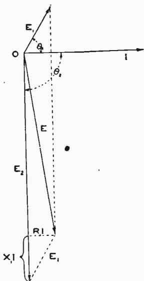
Fig. 70. E. M. F. Losses with Large Capacity Reactance
