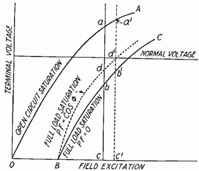
Fig. 166. Saturation Curves (Method b)
