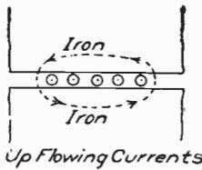
Fig. 323. Magnetic Action of Conductors Carrying Currents between Iron Poles
