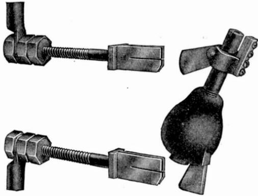
Fig. 368. Details of Switchboard Fuse Holder
