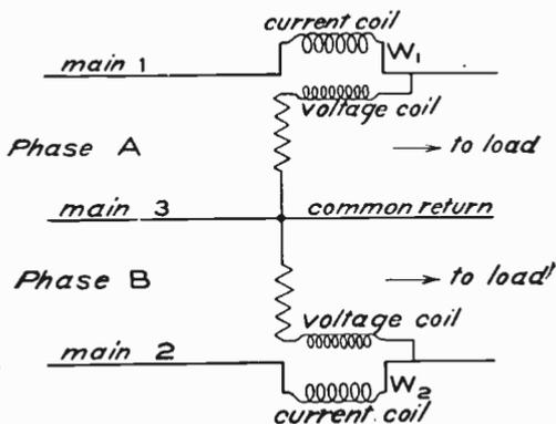
Fig. 107. Diagram of Power Connection for Three-Wire Two-Phase System
