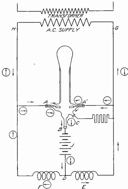
Fig. 285. Connections for Mercury-Vapor Arc Rectifier
