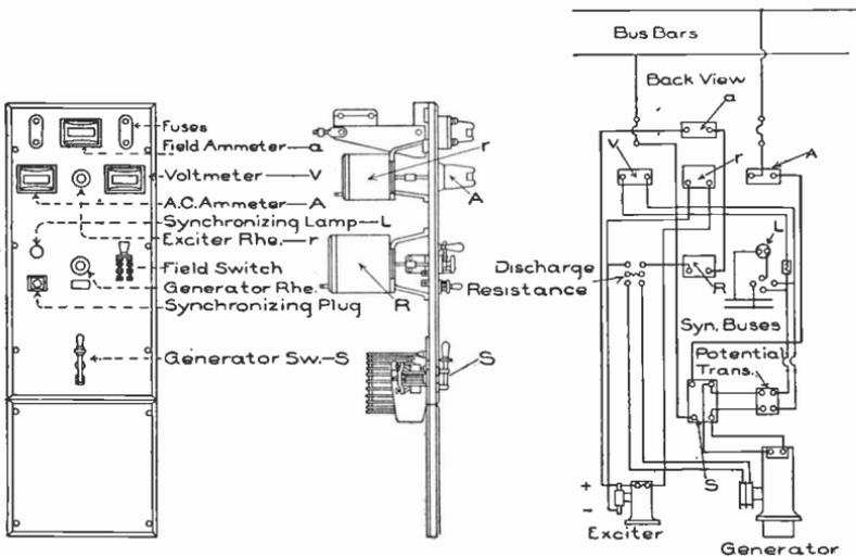
Fig. 369. Front and Side Views and Complete Diagram of Connections for Standard Panel for Two or More Single-Phase Alternators in Parallel
