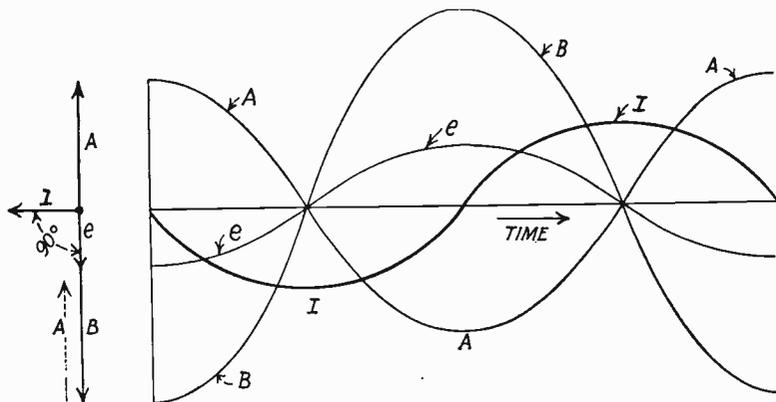
Fig. 190. Effect of Over-Excitation on Synchronous Motor
