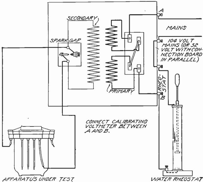
Fig. 158. Diagram of Connections for Dielectric Strength Test with High Potential Transformer
