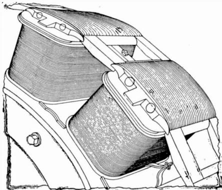
Fig. 181. Portion of Revolving Field Showing Copper Frame Dampers
