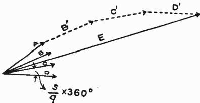
Fig. 77. Clock Diagram of Induced E. M. F.'s for Fig. 76
