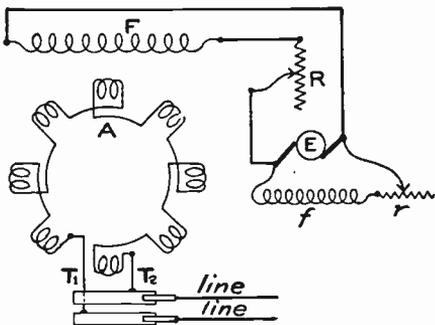
Fig. 81. Diagram Showing Method of Separate Excitation
