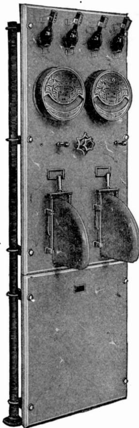
Fig. 366. Standard Switchboard for Single-Phase Generator and Two Feeder Circuits
