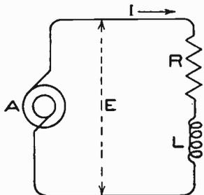
Fig. 51. Alternating Circuit Containing Resistance and Inductance
