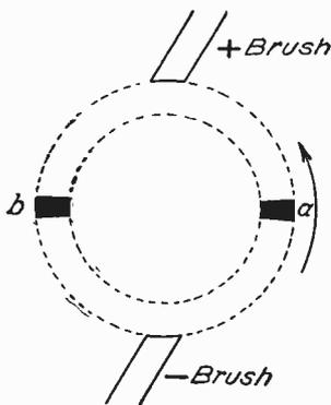
Fig. 288. Commutator and Brush Diagram for D. C. Dynamo as a Rotary Converter
