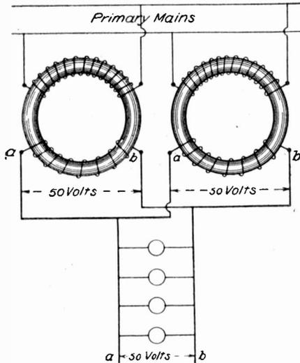
Fig. 205. Connections for "Banked" Transformers
