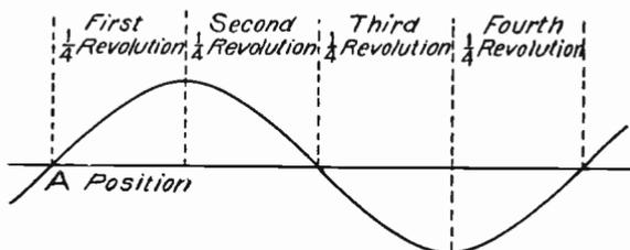
Fig. 289. E.M.F. Curve for One Revolution of D. C. Dynamo
