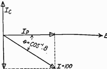
Fig. 192. Calculation of Leading Current
