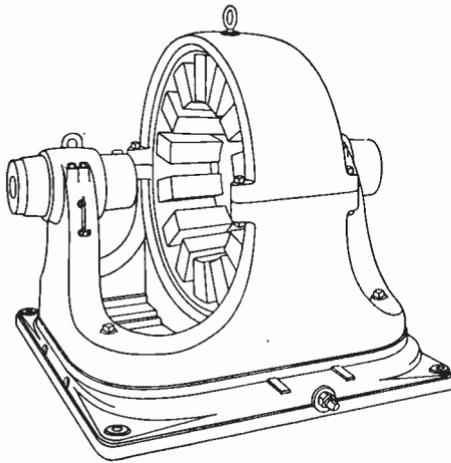
Fig. 129. Field Structure of a Westinghouse 180-Kw. Alternator
