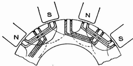
Fig. 91. Distributed or Multi-Coil Winding for Two-Phase Alternator
