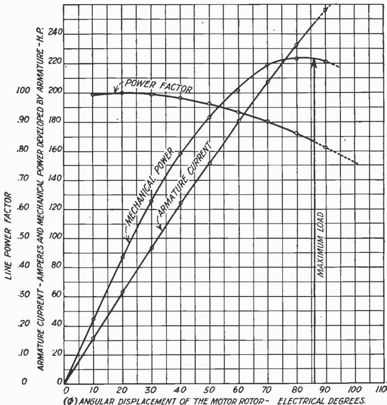
Fig. 180. Angular Displacement in Electrical Degrees of the Motor Rotor
