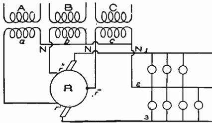
Fig. 304. Connections for a Three-Phase Rotary Converter on Edison Three-Wire System
