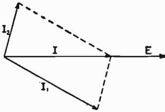
Fig. 191. Clock Diagram of Current Relations in Synchronous Motor
