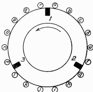
Fig. 293. Diagram of a D. C. Ring-Wound Armature
