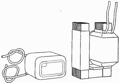
Fig. 229. Core with Upper Yoke Removed, Showing One Coil in Position
