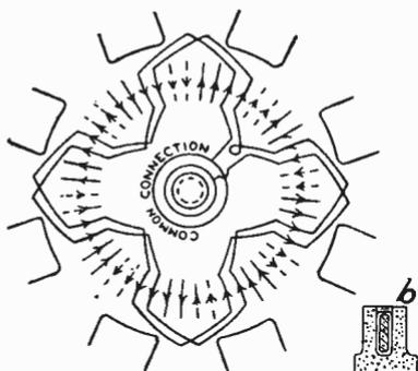
Fig. 120. Three-Phase Bar Winding, Two Slots Per Pole Per Phase
