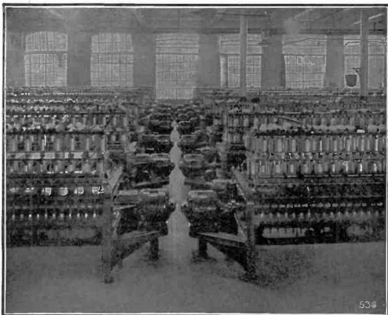
Fig. 345. Constant Speed Induction Motors Used for Driving Spindles in a Textile Mill
