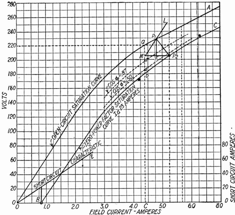
Fig. 170. Saturation and Short Circuit Characteristics
