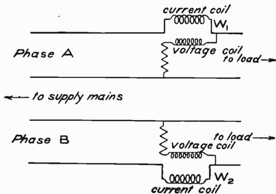
Fig. 106. Power Connection of Four-Wire Two-Phase System
