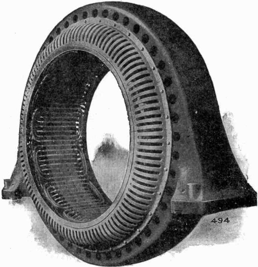
Fig. 149. Stationary Armature for 600-Kw. Allis-Chalmers "Water-Wheel Type" Alternator
