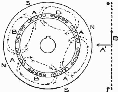
Fig. 327. Magnetic Effect of Alternating Current  $\frac{1}{4}$  of a Cycle Later Than in Fig. 325
