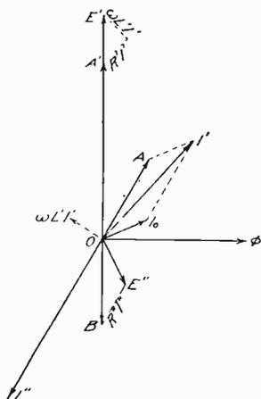
Fig. 197. Clock Diagram Showing Effects of Coil Resistance and Magnetic Leakage
