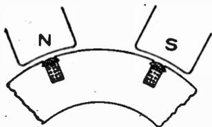
Fig. 73. Concentrated or Uni-coil Winding
