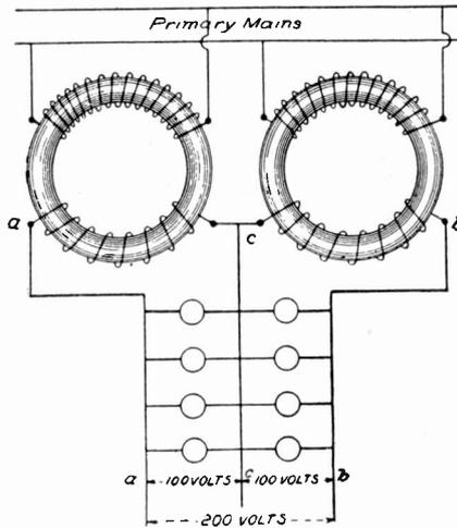
Fig. 203. Proper Transformer Connections to a Three-Wire System
