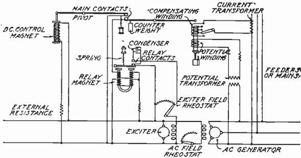
Fig. 88. Diagram of Electrical Connections for Generator Voltage Regulator
