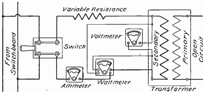
Fig. 279. Wiring Diagram for Core Loss and Exciting Current Test
