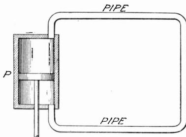
Fig. 11. Water Analogy for an Alternating Circuit
