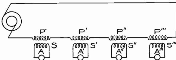
Fig. 206. Connections for Transformers in Series
