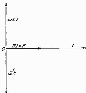
Fig. 56. Diagram Showing Multiplication of E. M. F.s by Resonance
