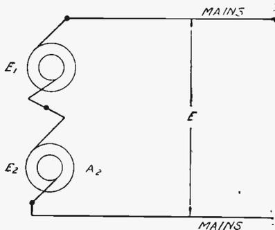
Fig. 6. Two Alternators in Series
