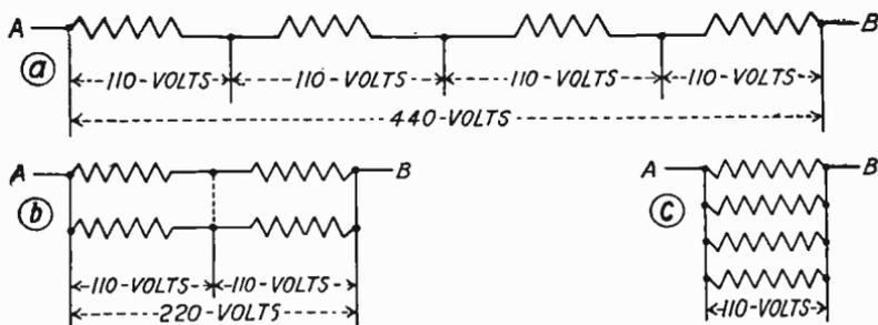
Fig. 359. Typical Series to Parallel Connections
