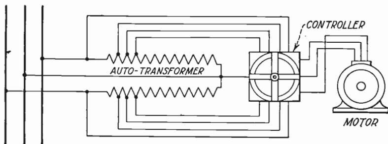
Fig. 342. Two-Coil Autotransformer with Three-Phase Induction Motor
