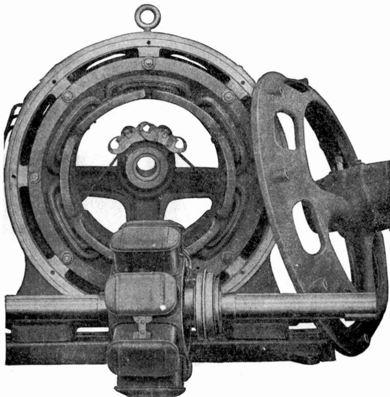
Fig. 132. Allis-Chalmers Revolving Field Alternator with One Bearing Removed and Rotor in Foreground
