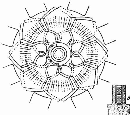
Fig. 121. Three-Phase Coil Winding, Two Slots Per Pole Per Phase
