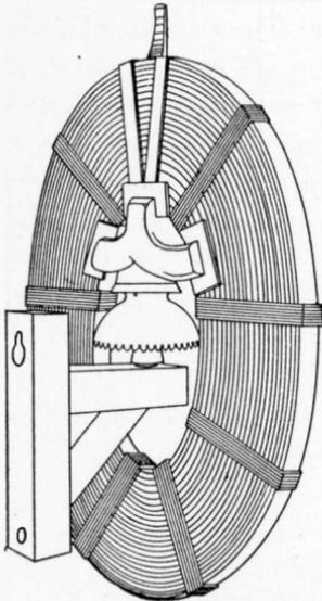
Fig. 403. Choke Coil made of Insulated Copper Strip
