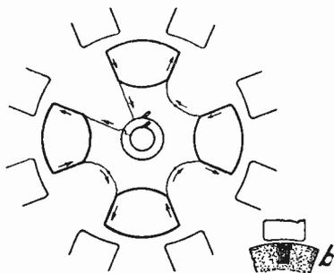
Fig. 114. Concentrated Single-Phase Armature Winding
