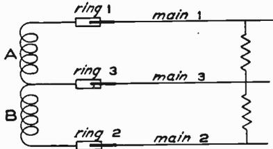
Fig. 92. Diagram of Collector Ring System for Two-Phase Alternator
