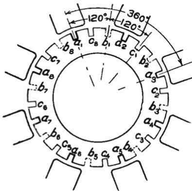
Fig. 95. Arrangement of Slots for Three-Phase Alternator Armature
