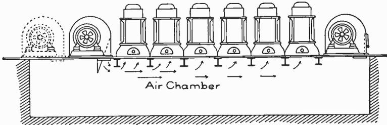
Fig. 264. Bank of Air-Blast Transformers Showing Arrangement of Air Chamber
