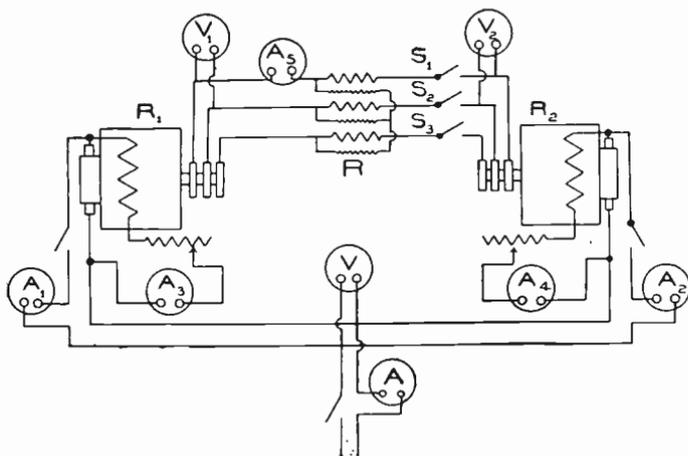
Fig. 314. Wiring Diagram for Motor-Generator Method of Testing Rotary Converters
