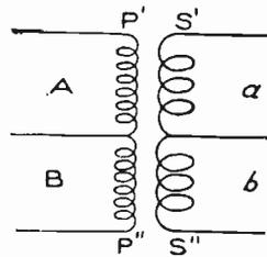
Fig. 211. Transformer Connections on a Three-Wire Two-Phase System
