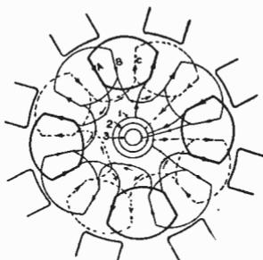
Fig. 119. Three-Phase Concentrated Winding  $\Delta$ -Connected
