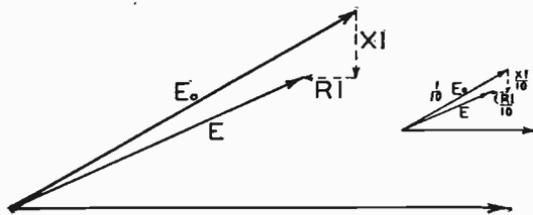
Figs. 398 (left) and 399 (right). Vector Diagrams Showing E.M.F. Relations in the Line and in the Compensator
