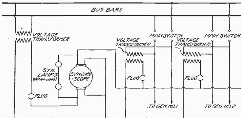
Fig. 379. Wiring Diagram for a Synchroscope for Single-Phase or One Phase of Poly-phase Circuit
