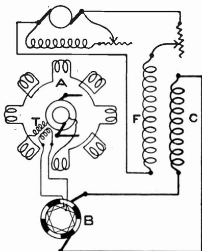
Fig. 83. Diagram Showing Composite Excitation with Transformer
