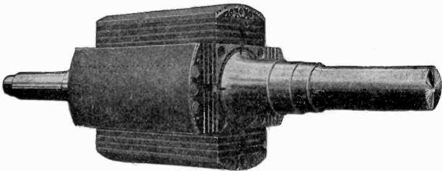
Fig. 152. Four-Pole Rotor for 10,000-Kw. Machine
