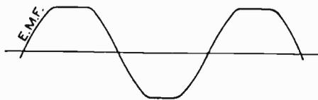
Fig. 16. Typical E. M. F. Curve for Alternator—
