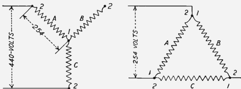
Fig. 360. Typical Delta to Star Connections
