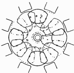
Fig. 118. Three-Phase Concentrated Winding Y-Connected
