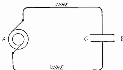
Fig. 12. Alternating Circuit Containing Condenser
