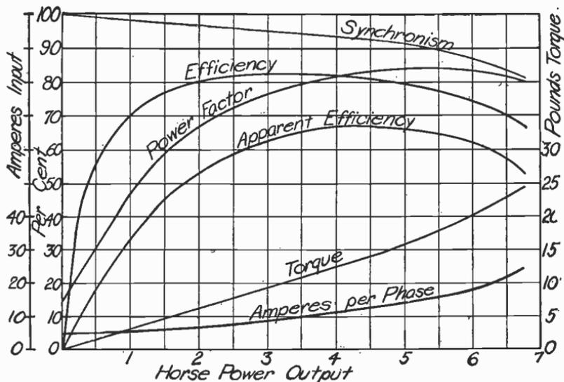
Fig. 358. Performance Curves of 5-Hp. Two-Phase Induction Motor
