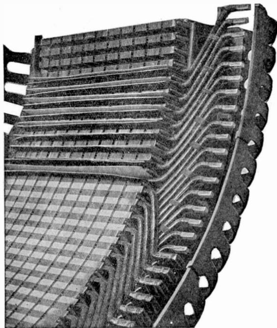
Fig. 134. Armature Coil Support Construction—General Electric Alternator
