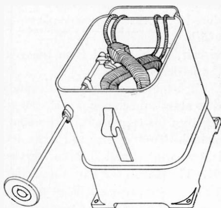
Fig. 393. Magnetic Voltage Regulator in Case with Cover Removed
