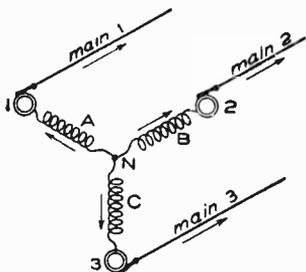
Fig. 98. The "Y" Scheme of Connecting Three Phases in Three-Phase Alternator
