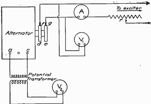
Fig. 160. Diagram of Connections for Saturation Curve Test of Alternator
