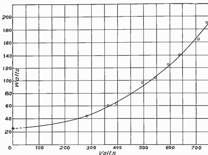
Fig. 353. Curve Showing Watts Input to a 1-H. P. Motor at Different Voltages
