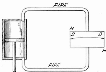
Fig. 13. Water Analogy for Alternating Circuit with Condenser
