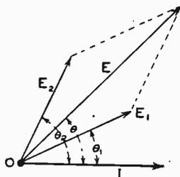
Fig. 65. Diagram of E. M. F. Conditions for Fig. 64
