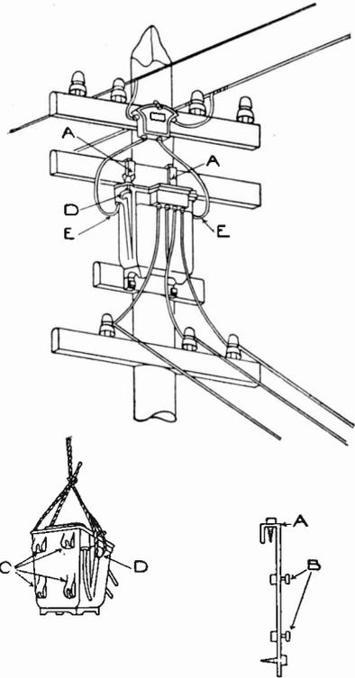
Fig. 275. Sample Mounting for Out-Door Transformers
