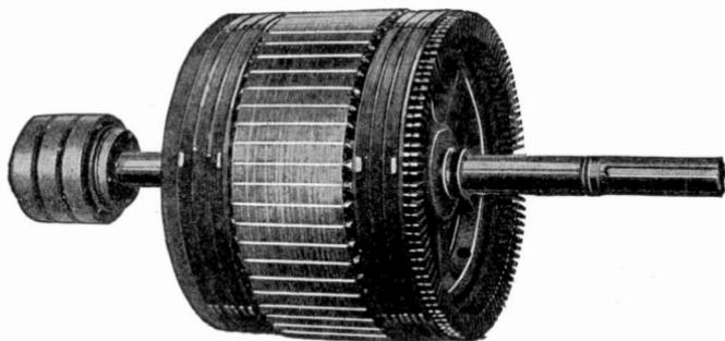
Fig. 336. Rotor with Polar Winding and Collector Rings
