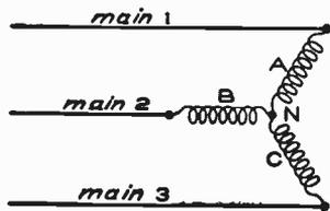
Fig. 102. "Y" Method of Connecting Receiving Circuits
