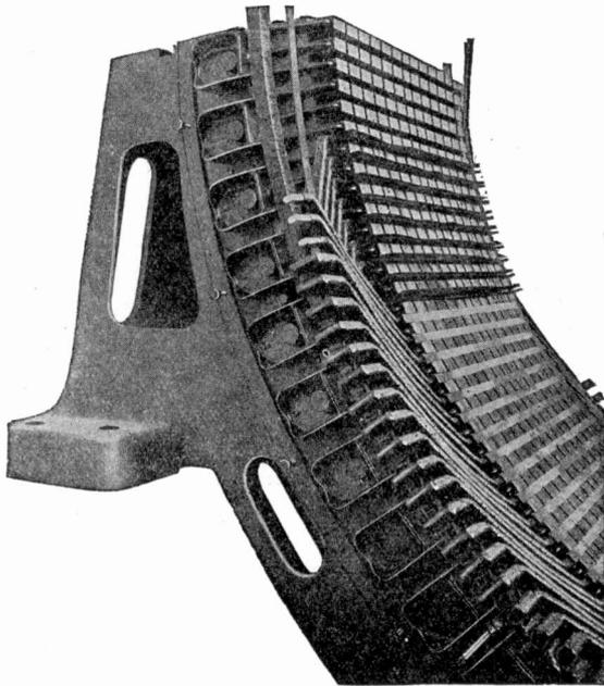
Fig. 135. Armature Coil Support Construction—General Electric Alternator
