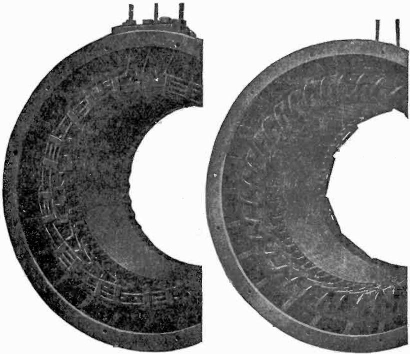
Fig. 155. Two Views of Stationary Armature of Curtis Alternator
