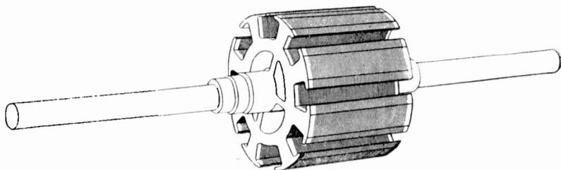
Fig. 124. Westinghouse Single-Phase Uni-Coil Armature Core
