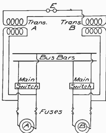
Fig. 411. Wiring Diagram Showing Method of Determining Phase Relation by Synchronizer
