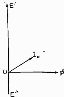
Fig. 194. Clock Diagram for Transformer without Load
