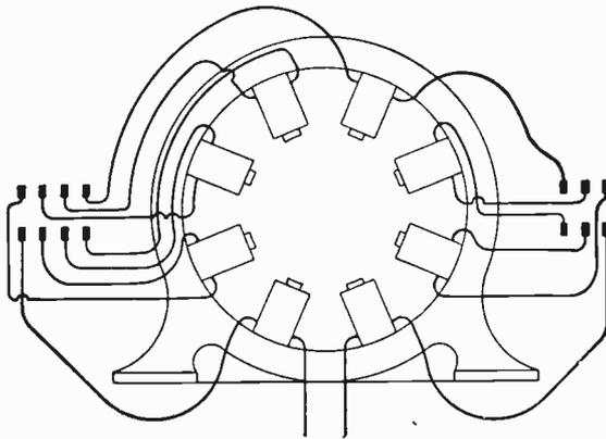
Fig. 184. Diagrammatic View of Stationary Field of a Synchronous Motor
