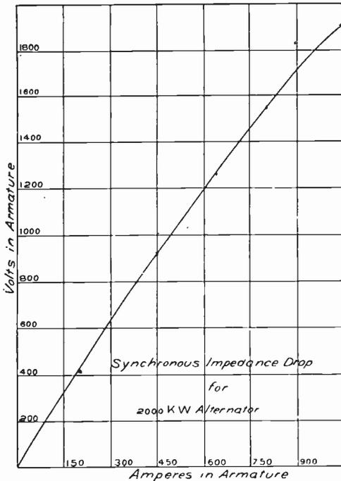
Fig. 163. Curve Showing Synchronous Impedance Drop for 2,000-Kw. Alternator
