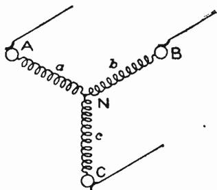
Fig. 164. Diagram for Armature when Y-connected
