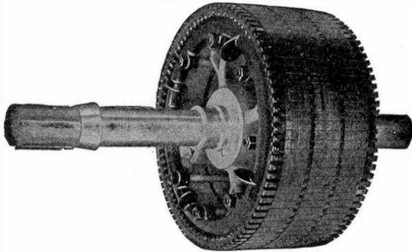
Fig. 334. Squirrel-Cage Type of Rotor
