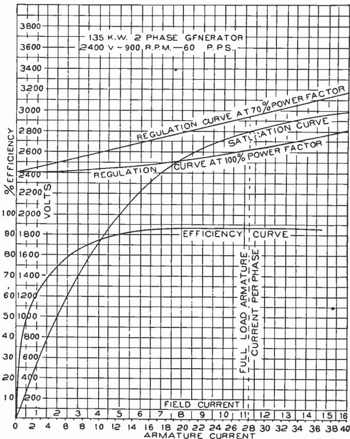
Fig. 162. Set of Curves for Two-Phase 135-Kw. Inductor Alternator
