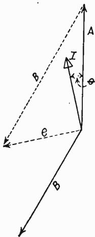
Fig. 185. Effect of Motor Over-Excited, Current Leading
