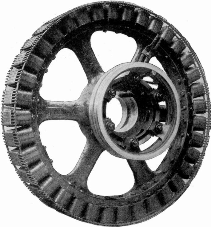
Fig. 182. Rotor of a Synchronous Motor Provided with "Squirrel-Cage" Form of Damper
