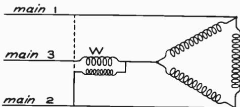
Fig. 105. Diagram of Power Connection for Three-Wire Three-Phase System
