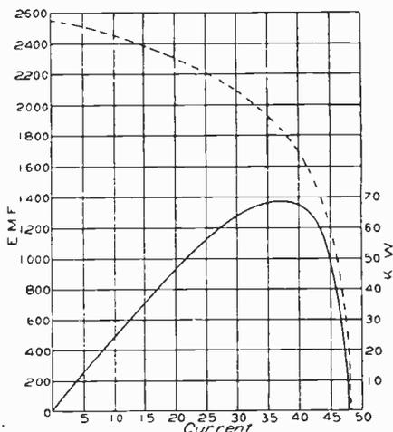
Fig. 157. Characteristic Curves of an Alternator
