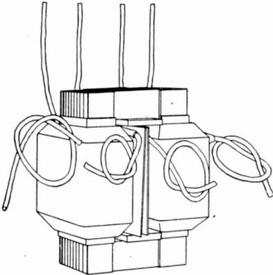
Fig. 227. Core-Type of Transformer
