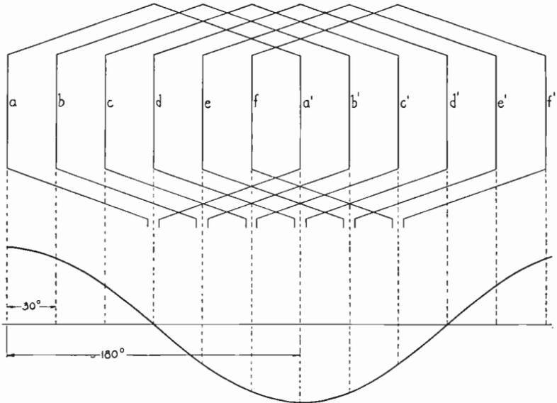
Fig. 361. Phase Relations of Induced Voltages in Pole Coils
