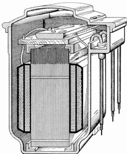
Fig. 232. Section Through Commercial Core-Type of Transformer
