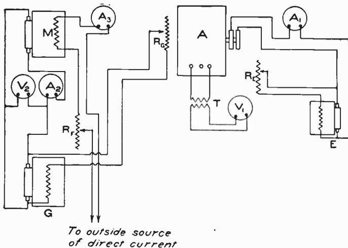
Fig. 175. Diagram of Connections for Core-Loss Test of Alternators
