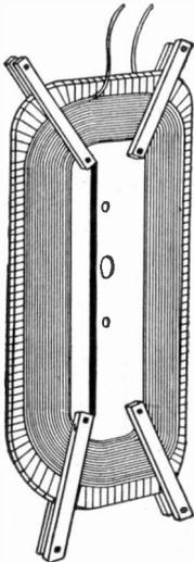
Fig. 250. Pancake Coil for Shell-Type Transformer
