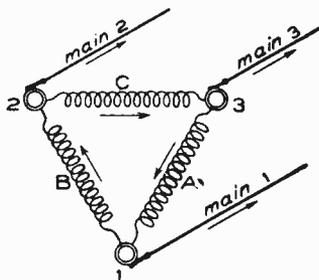
Fig. 99. Diagram of "Δ" Scheme for Connecting Phases in Three-Phase Alternator
