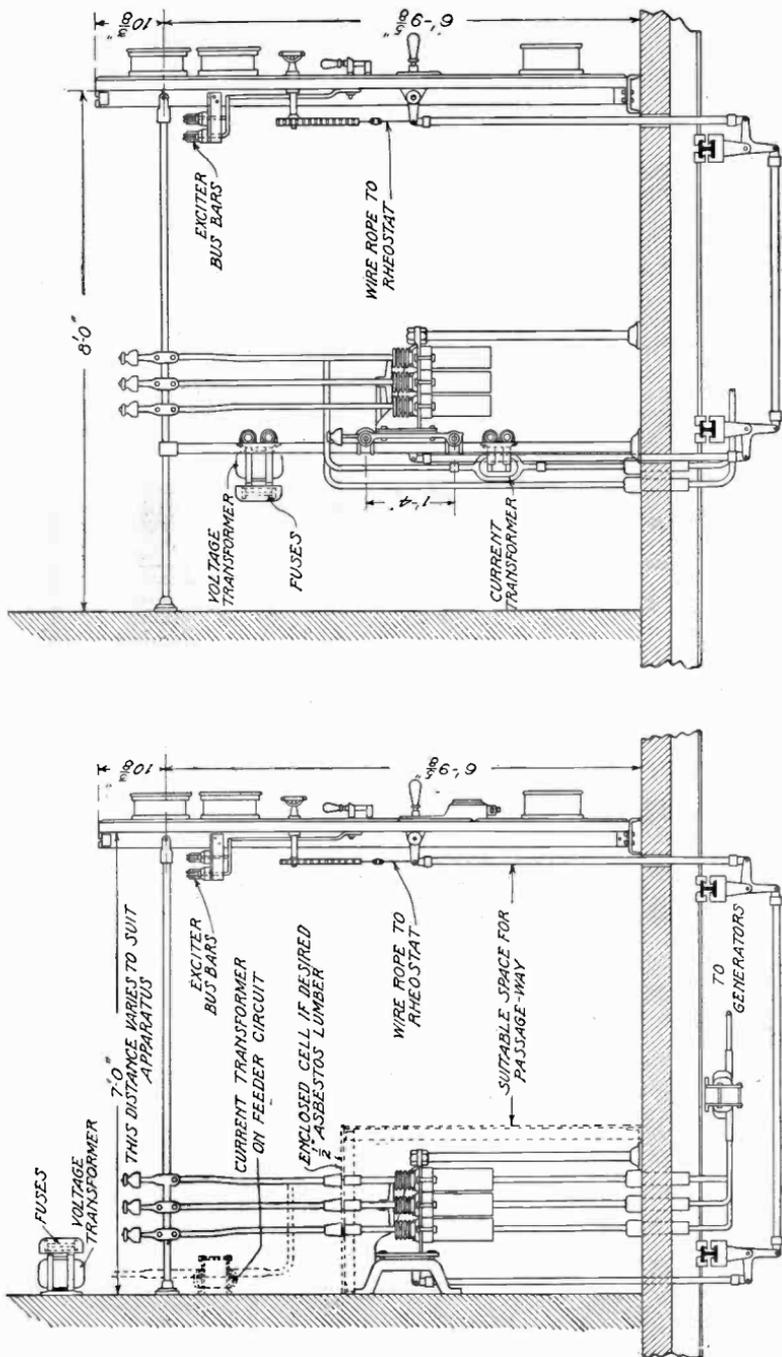
Fig. 377. Diagram of High Voltage Switchboard Showing System of Levers for Operating Switches by "Remote Control"
