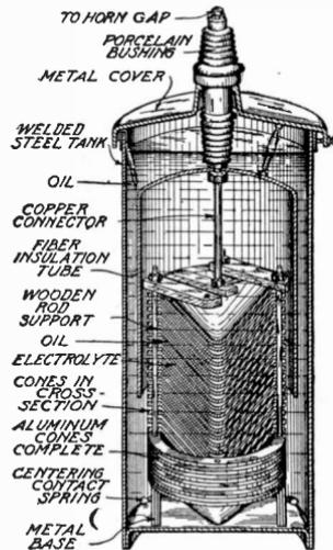
Fig. 407. Cross-Section of Aluminum Cell Lightning Arrester
