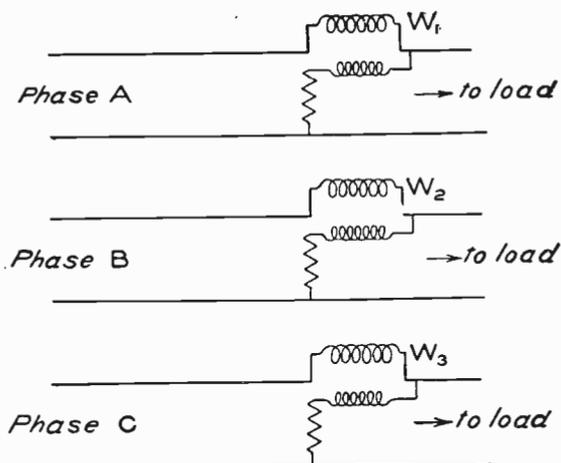
Fig. 108. Diagram of Power Connection for Six-Wire Three-Phase System
