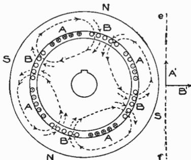
Fig. 325. Instantaneous Effect of Alternating Current for a Given Position of Rotor
