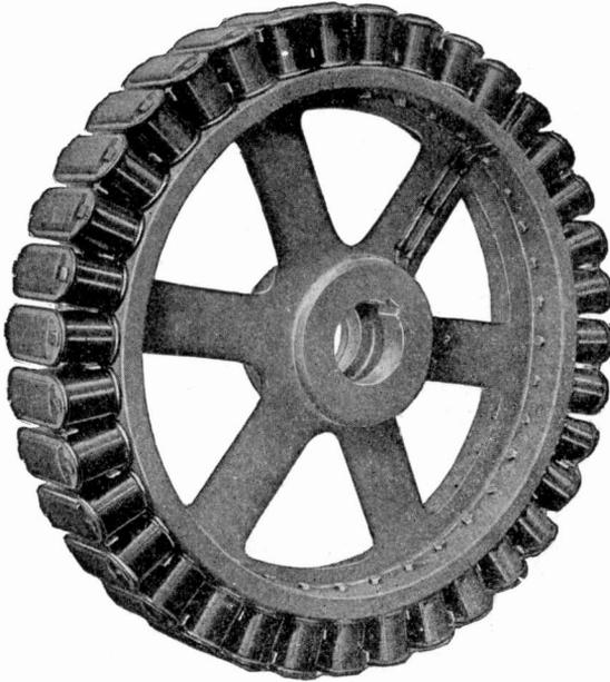
Fig. 143. Rotor Construction with Laminated Pole Pieces Bolted to Cast-Iron or Steel Ring
