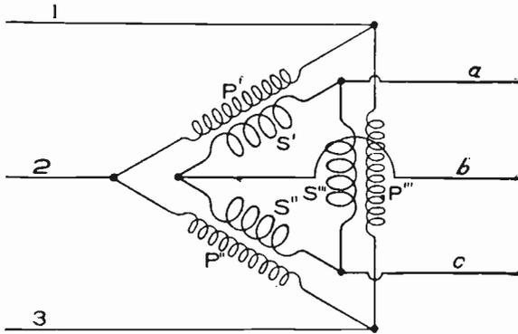
Fig. 212. Connections for Three Transformers with Primaries  $\Delta$ -Connected to Three-Wire Three-Phase Mains
