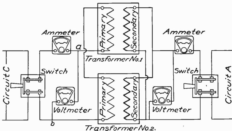
Fig. 278. Connections for Transformer Heat Test
