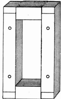
Fig. 228. Standard Form of Laminated Transformer Core
