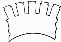
Fig. 110. Portion of Stamping for Twelve-Pole Uni-Tooth Three-Phase Alternator
