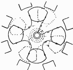
Fig. 116. Two-Phase Concentrated Armature Winding
