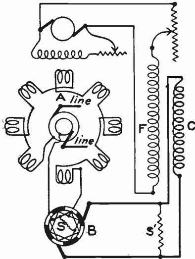
Fig. 82. Diagram Showing Method of Composite Excitation
