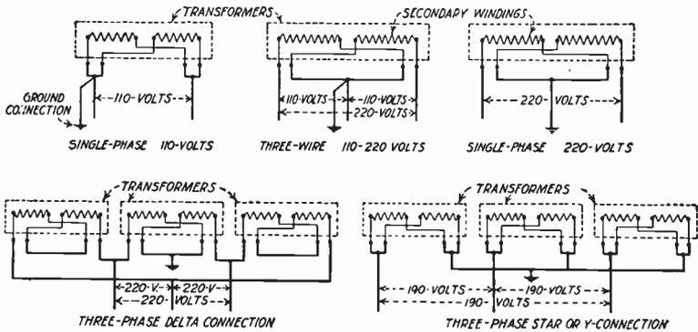
Fig. 277. Ground Connections to Secondaries of Commercial Transformers
