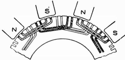
Fig. 96. Portion of Diagram of Windings for Three-Phase Alternator Armature
