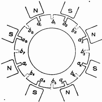
Fig. 90. Diagram Showing Method of Combining Separate Armature Windings on One Core
