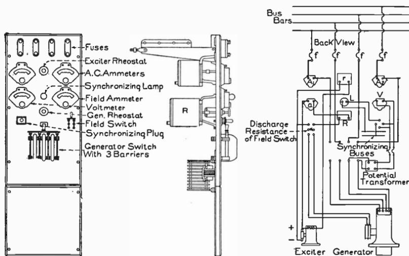
Fig. 371. Front and Side View and Complete Wiring Diagram of Switchboard Panel for Two-Phase Alternator Operated in Parallel with Other Two-Phase Machines
