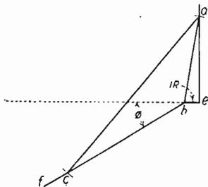
Fig. 167. Terminal Voltage with Reactance
