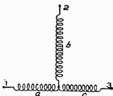
Fig. 223. Y Connections for Three Secondaries of Scott Transformer for Two-Phase System
