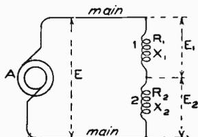
Fig. 64. Two Elements in Series in Alternating Circuit
