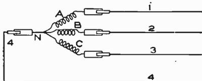
Fig. 97. Collector Ring System for Three-Phase Alternator
