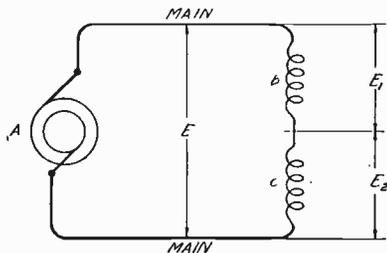
Fig. 8. Alternating Current Through Two Coils in Series
