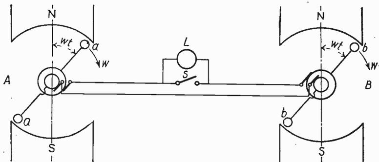
Fig. 176. Diagram Showing Principle of Synchronizing Motor and Generator
