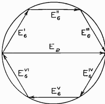
Fig. 297. E.M.F. Relations in a Six-Ring Converter
