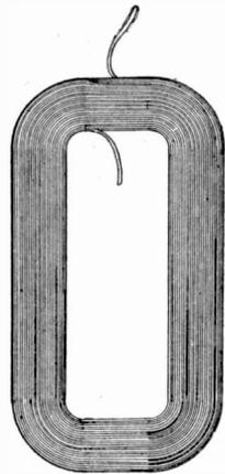
Fig. 252. Pancake Coil Showing Use of Insulated Flat Strips
