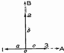
Fig. 220. Vector Diagram of E.M.F. Relations in Three Secondaries of Scott Transformer
