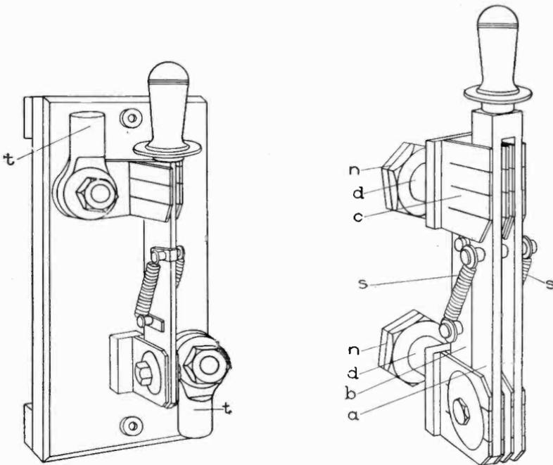
Fig. 380. "Quick Break" Knife Switches
