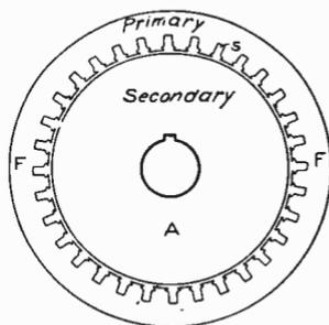
Fig. 319. Diagram Showing Slots in Stator of Induction Motor
