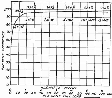
Fig. 225. Graphic Relation between Efficiency and Output for a Core Type Transformer
