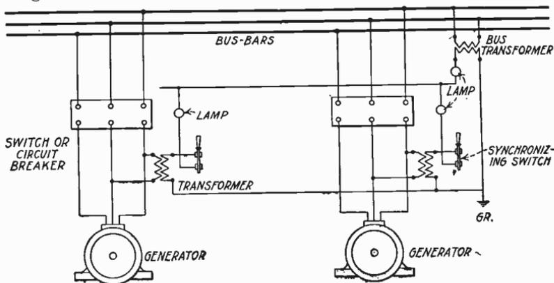
Fig. 413. Connections for Synchronizing Three-Phase Generators
