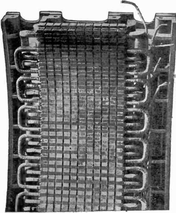
Fig. 136. Portion of General Electric Stationary Armature Showing Method of Connecting Armature Coils
