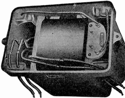
Fig. 258. Top View of Fort Wayne Transformer with Cover Removed Showing Arrangement of Lead Wires
