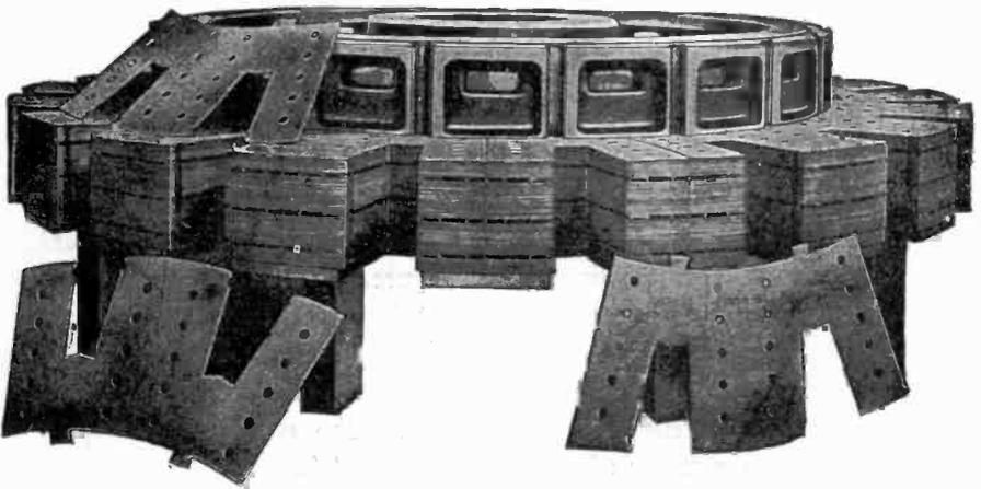
Fig. 137. Method of Constructing Laminated Field Cores
