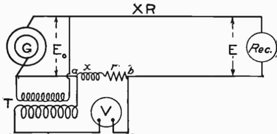
Fig. 397. Diagram of Connections for Voltmeter Compensator
