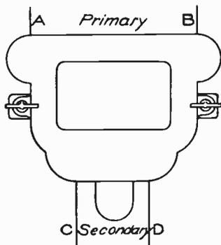
Fig. 281. Transformer Connected for Polarity Test
