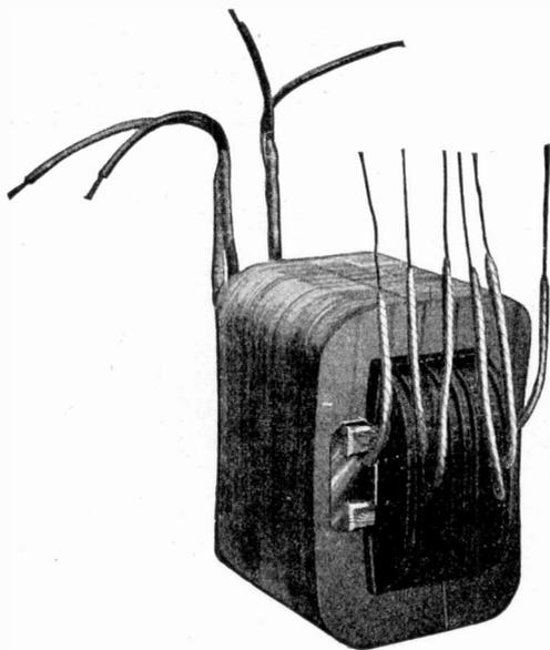
Fig. 257. Assembled Core and Coils for Fort Wayne Transformer
