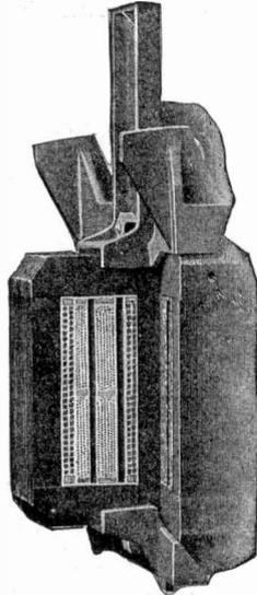
Fig. 249. Part Section through Westinghouse Transformer
