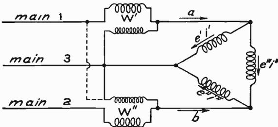
Fig. 109. Diagram of Power Connection for Three-Wire Three-Phase System
