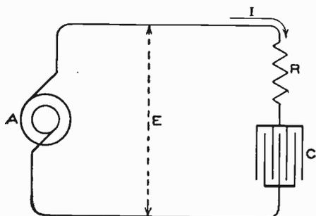
Fig. 53. Circuit Containing Resistance and Capacity
