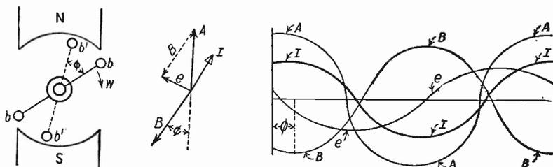
Fig. 178. Voltage Conditions of Motor under Load
