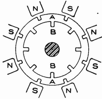
Fig. 89. Diagram of Two-Phase Alternator with Two Separate Armatures
