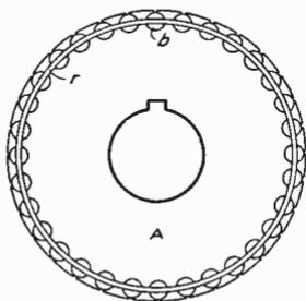
Fig. 318. Diagram of Squirrel-Cage Type of Rotor
