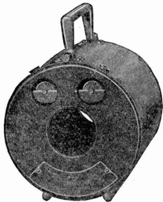
Fig. 267. Portable Current Transformer without Regular Primary Windings
