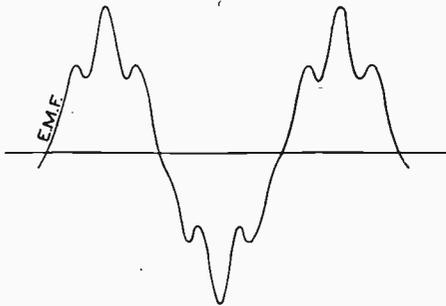
Fig. 15. Typical E. M. F. Curve for Alternator—
