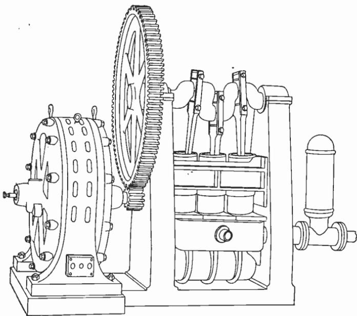
Fig. 347. Induction Motor Driving Triplex Pump
