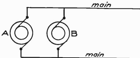
Fig. 35. Two Alternators Running in Synchronism Connected in Parallel
