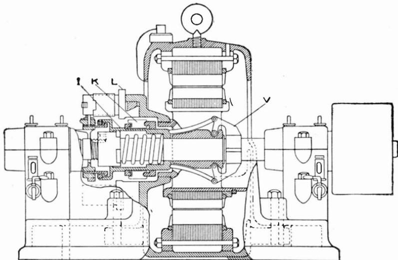
Fig. 251. Part Section of Wagner Single-Phase Induction Motor
