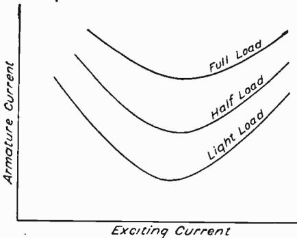
Fig. 188. Curve Showing Variation of Armature Current with Field Excitation
