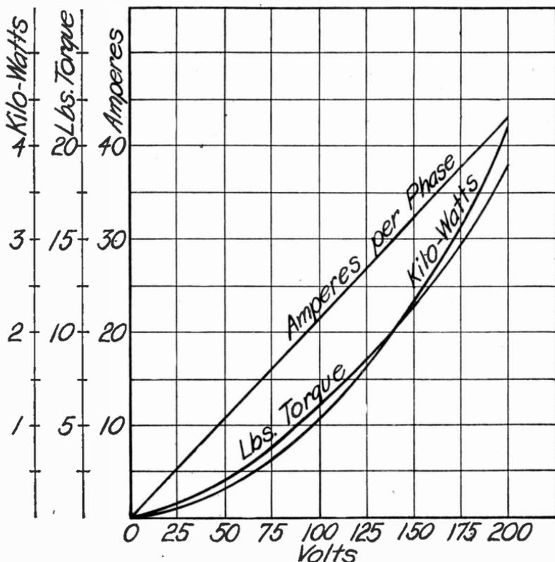
Fig. 357. Locked Saturation Curves
