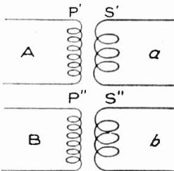
Fig. 210. Transformer Connections on a Two-Phase System
