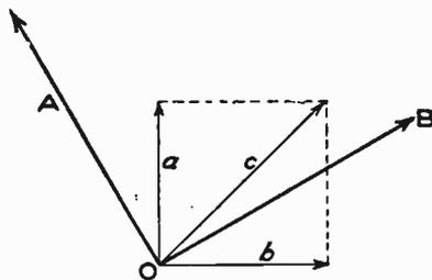
Fig. 93. Clock Diagram of E. M. F.'s and Currents for Two-Phase Alternator
