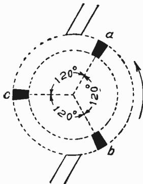
Fig. 290. Brush and Commutator Diagram for Three-Ring Converter
