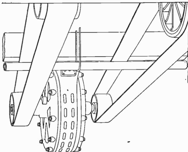
Fig. 348. Induction Motor Suspended from the Ceiling, Driving Shafting by a Belt
