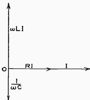
Fig. 46. Vector Diagram of Conditions in Fig. 45
