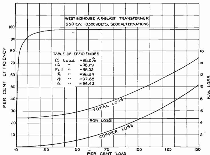
Fig. 226. Efficiency Curves for a Westinghouse Air-Blast Transformer
