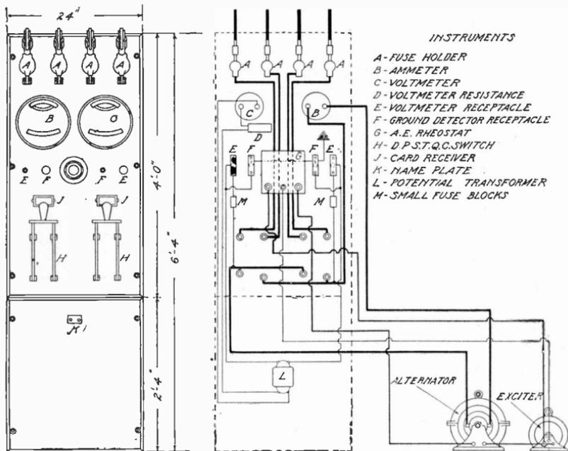
Fig. 367. Front Elevation and Connections for Board Shown in Fig. 366
