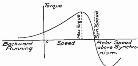
Fig. 329. Graphical Relation of Torque and Speed of Induction Motor
