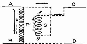
Fig. 208. Connections for Auto Step-Up Transformer
