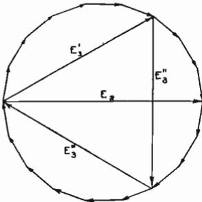
Fig. 295. E.M.F. Relations in Two- and Three-Ring Converter
