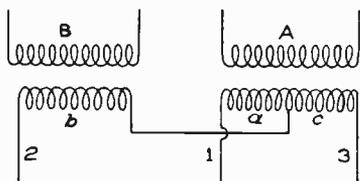
Fig. 224. Complete Connections of Scott Transformer
