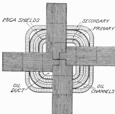
Fig. 245. Plan of Assembled Core and Coils Showing Four Magnetic Circuits in Parallel
