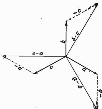
Fig. 101. Clock Diagram for Currents in " $\Delta$ " Connected Three-Phase Armature
