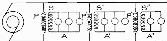
Fig. 198. Diagram of Connections of Constant-Voltage Transformers in Parallel
