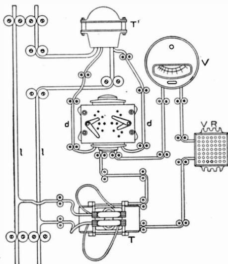
Fig. 401. Diagram of Circuits and Apparatus in Connection with Westinghouse Compensated Voltmeter
