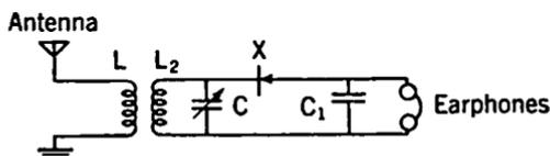
FIG. 13-2. Simple Crystal Receiver.
