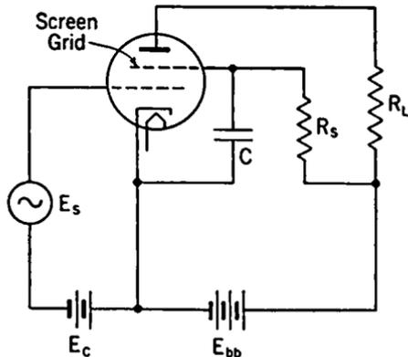
FIG. 4-15. Screen Supply for Tetrode.
