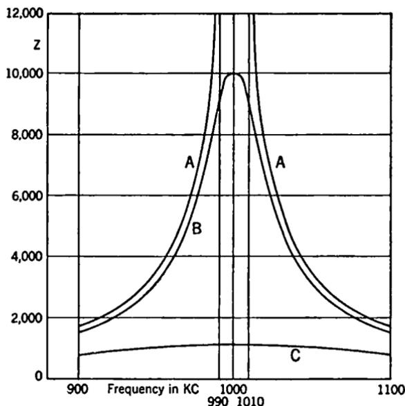
(b) Frequency, impedance characteristic of parallel circuit
