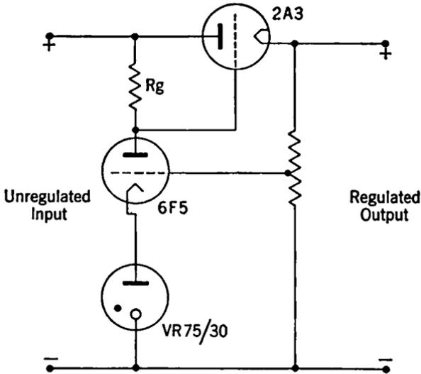
FIG. 5-11. Electronic Voltage Regulator.
