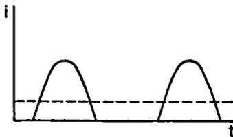
FIG. 5-2. Output of Half-wave Rectifier.
