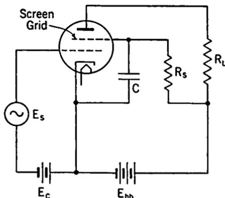
FIG. 4-15. Screen Supply for Tetrode.
