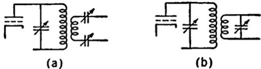
FIG. 16-12. Coupling a Transmitter to a Resonant Line. (a) Series feed for coupling at a low-impedance point. (b) Parallel feed for coupling at a high-impedance point.
