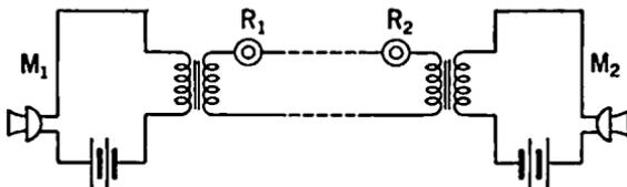
FIG. 6-6. Local-battery Telephone Circuit.
