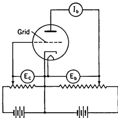
FIG. 4-7. Circuit for Obtaining Triode Characteristics.
