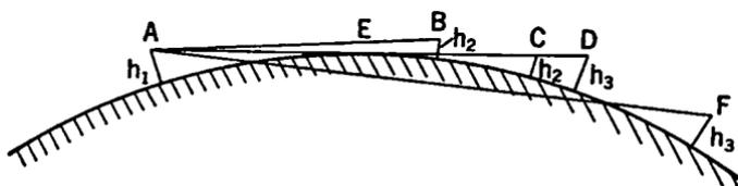
FIG. 15-10. Direct-ray Propagation at the Ultrahigh Frequencies.
