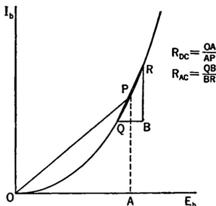
FIG. 4-4. D.C. and A.C. Plate Resistance.
