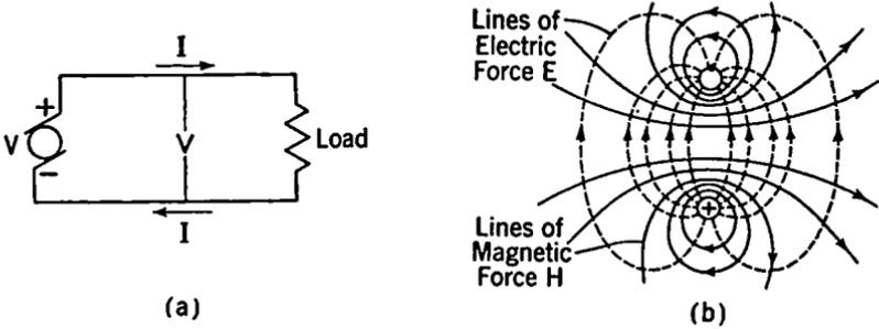
FIG. 9-7. Electric and Magnetic Fields about a Pair of Parallel Wires.
