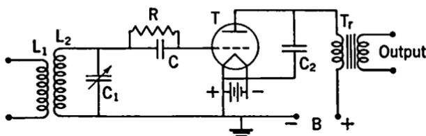
FIG. 11-32. Grid-circuit Detection.
