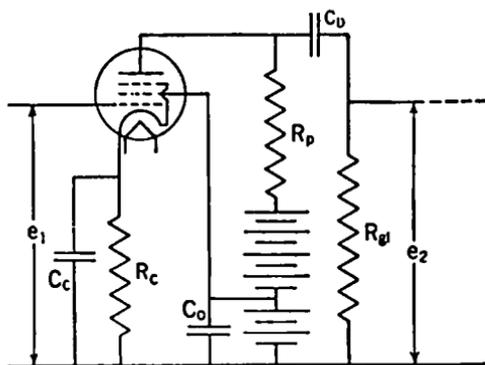
FIG. 7-4. Circuit of a Resistance-coupled Pentode Amplifier.
