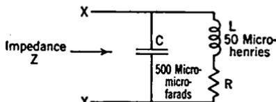
(a) Parallel resonant circuit
