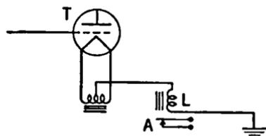
FIG. 12-15. Overload Relay.
