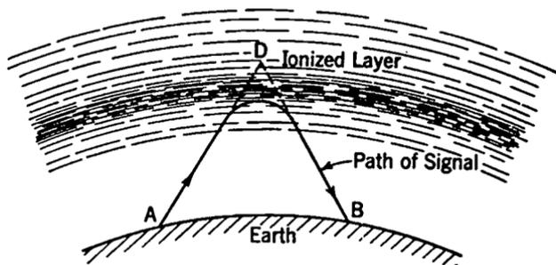
FIG. 15-3. Refraction of the Sky Wave by an Ionized Layer.
