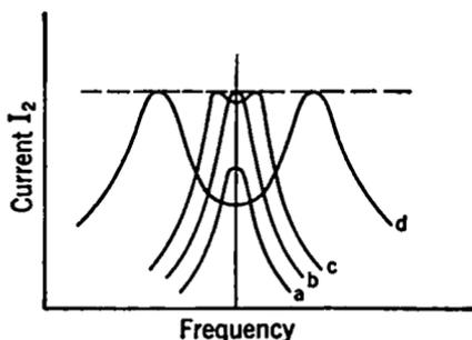
FIG. 3-32. Resonance Curves for Tuned Circuits with Different Amounts of Mutual Coupling.
