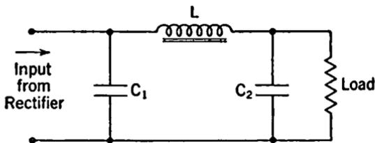
FIG. 5-7. Condenser-input Filter.
