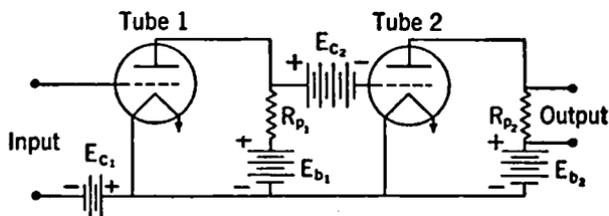
FIG. 7-18. A D.C. Amplifier Circuit.
