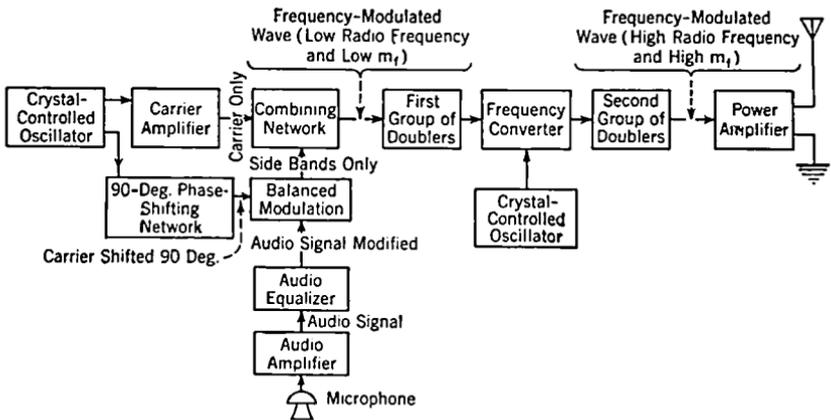
FIG. 14-5. Block Diagram of Armstrong Frequency-modulation Transmitter System.
