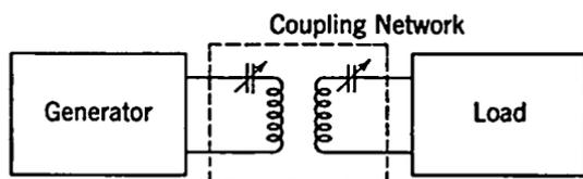
Fig. 16-10. Typical Series-tuned Coupling Network for Connecting a Low-impedance Generator to a Low-impedance Load.
