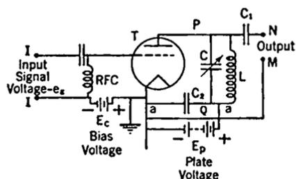
FIG. 11-4. Simple Triode Radio Amplifier.
