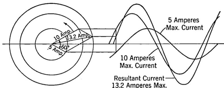
FIG. 3-3. Addition of Alternating Currents.
