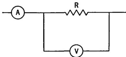
FIG. 2-35. Determination of Resistance by Ammeter and Voltmeter.
