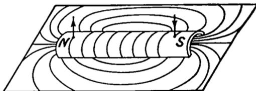
FIG. 2-24. The Magnetic Field about a Coil of Wire Carrying Current.
