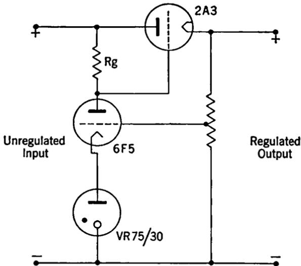
FIG. 5-11. Electronic Voltage Regulator.
