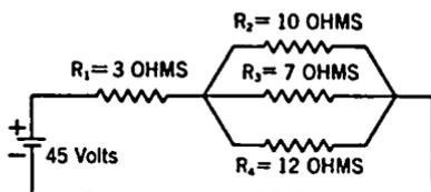
FIG. 2-4. Resistances in Series and Parallel.
