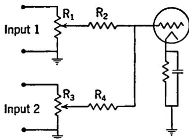
FIG. 7-22. Resistance Mixing Circuit.
