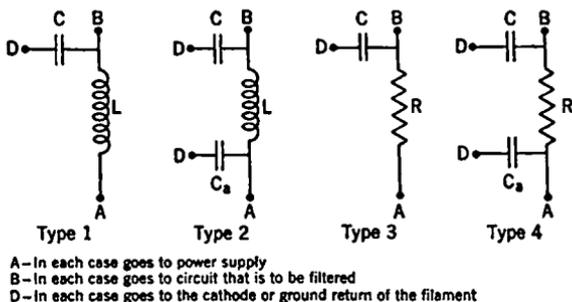
FIG. 11-14. D.C. Power-supply Filters.
