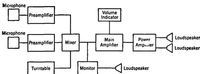
FIG. 7-21. Block Diagram of a Large Public-address System.
