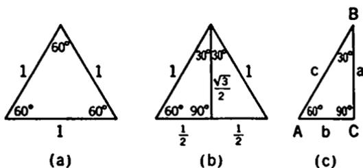
FIG. 1-5. Equilateral Triangle and  $30^\circ$ - $60^\circ$  Triangle.
