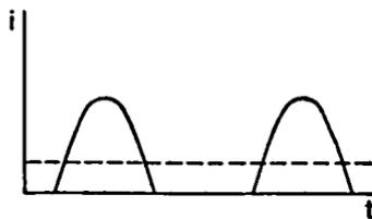
FIG. 5-2. Output of Half-wave Rectifier.
