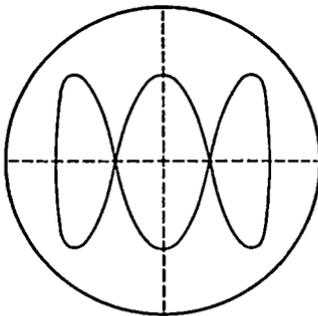
FIG. 8-8. Lissajous Figure, Frequency Ratio 3:1.
