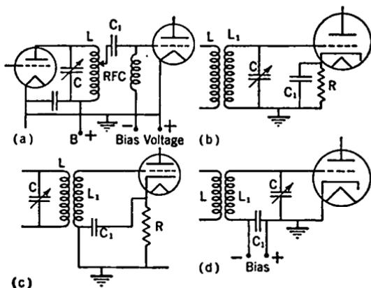
FIG. 11-5. Types of Radio-amplifier Input Circuits.
