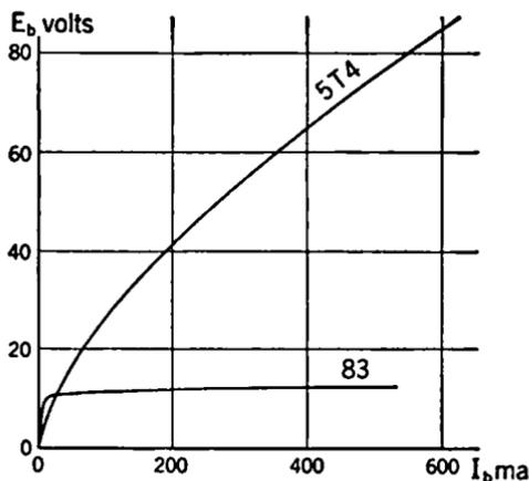
FIG. 5-9. Plate Characteristics of Rectifier Tubes.
