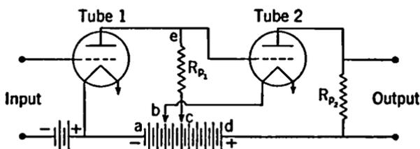
FIG. 7-19. An Alternative Method of Connection for a D.C. Amplifier.
