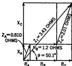
FIG. 3-19. Impedance Diagram; Example pp. 93-94.
