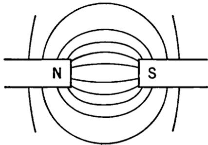
FIG. 2-21. The Magnetic Field about Two Unlike Poles.
