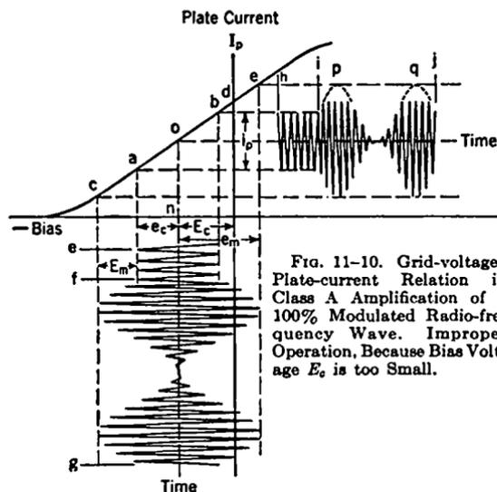
FIG. 11-10. Grid-voltage-Plate-current Relation in Class A Amplification of a 100% Modulated Radio-frequency Wave. Improper Operation, Because Bias Voltage  $E_c$  is too Small.
