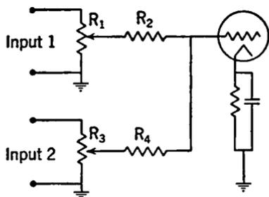
FIG. 7-22. Resistance Mixing Circuit.
