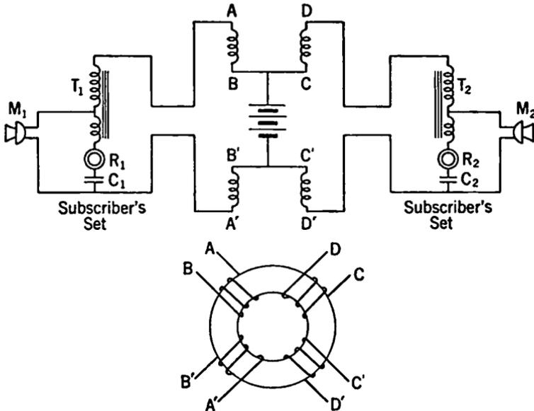
FIG. 6-7. Common-battery Telephone Circuit.
