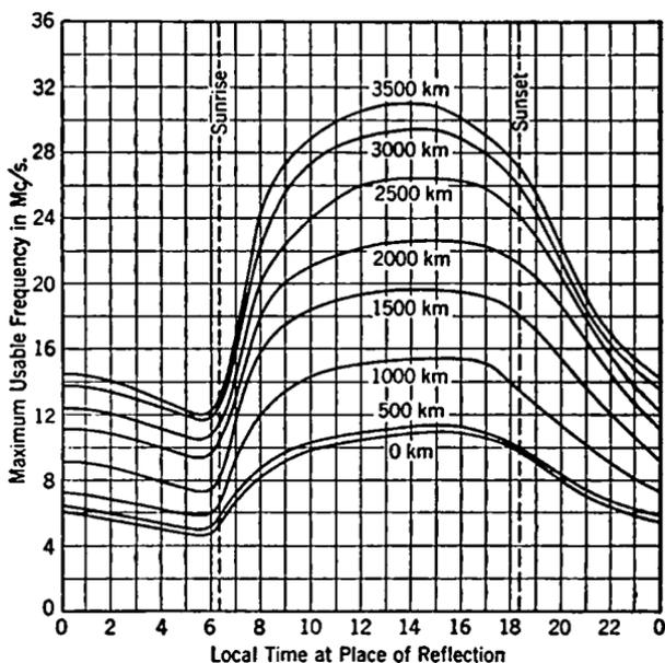
FIG. 15-7. Graph of Maximum Usable Frequency.
