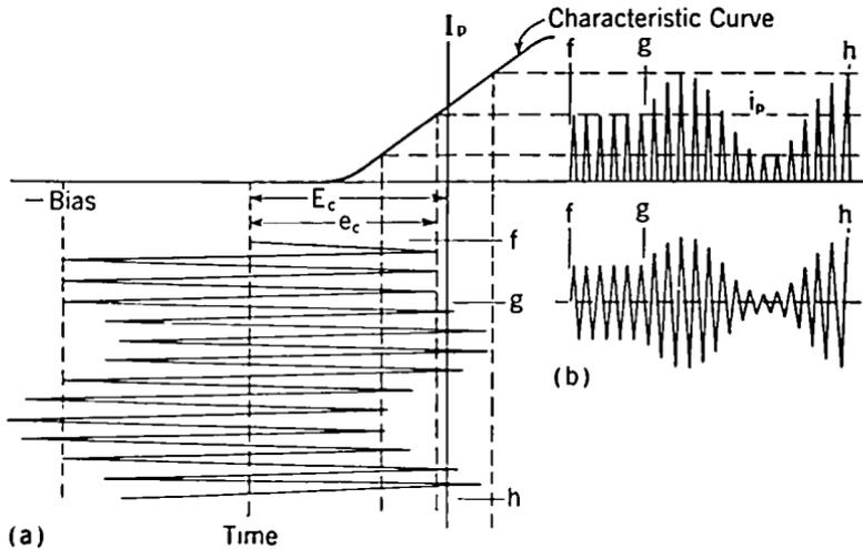
FIG. 12-8. Grid-voltage-Plate-current Relation in Grid Modulation.
