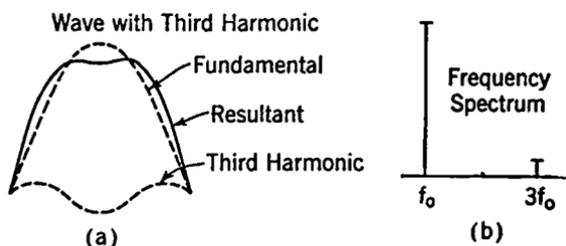
FIG. 14-3. Distorted Wave and Components.
