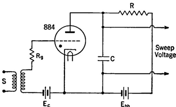
FIG. 8-4. Cathode-ray Sweep Generator.
