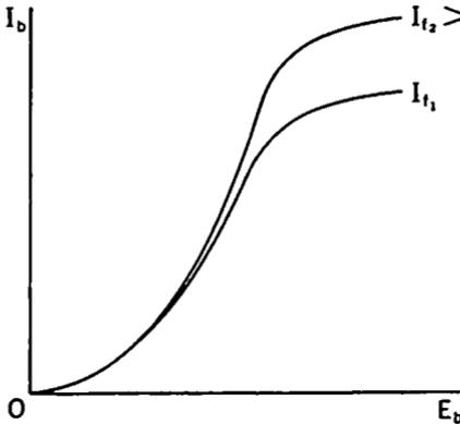
FIG. 4-2. Limitation of Diode Current by Temperature.
