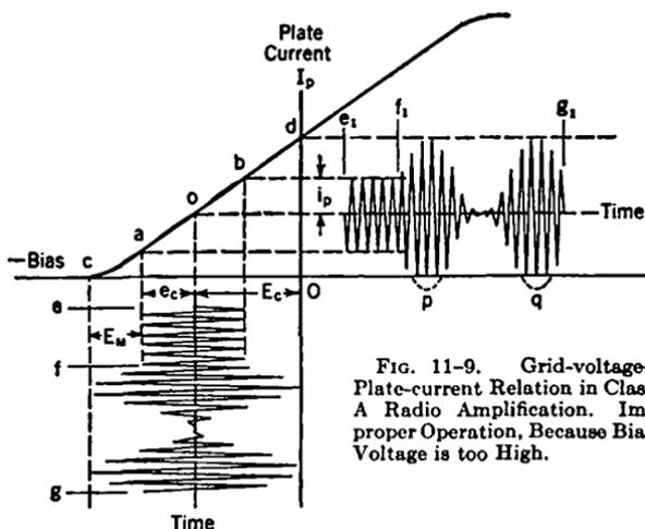
FIG. 11-9. Grid-voltage-Plate-current Relation in Class A Radio Amplification. Improper Operation, Because Bias Voltage is too High.
