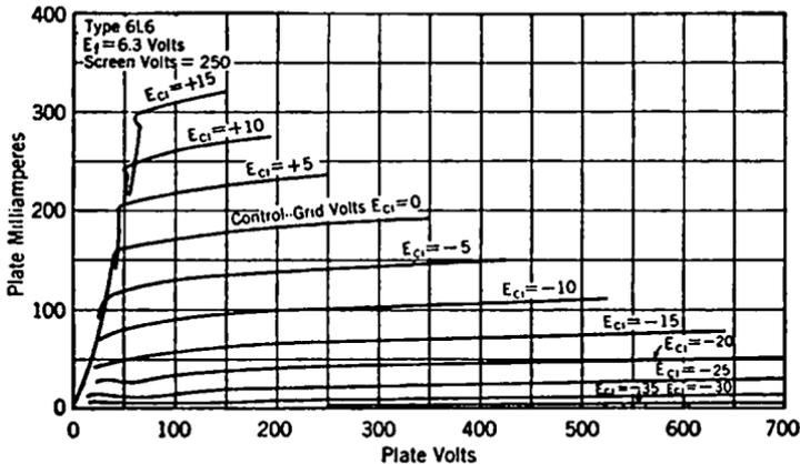
FIG. 4-19. Plate Characteristics of 6L6 Beam Power Tube.
