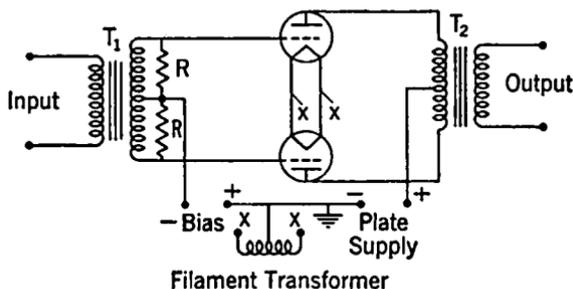
FIG. 11-22. Circuit Diagram of a Push-pull Class B Audio Amplifier.
