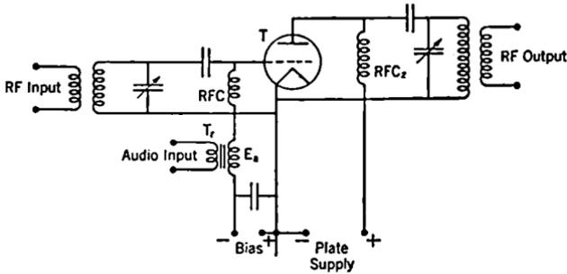
FIG. 12-7. Grid-modulation Circuit.
