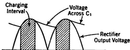
FIG. 5-8. Operation of Condenser-input Filter.
