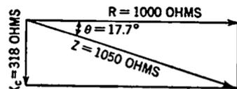
Fig. 3-24. Vector Diagram, Capacitive Circuit.
