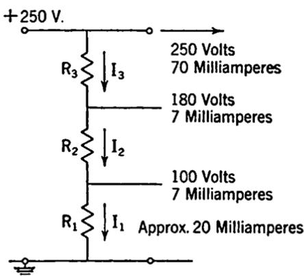
FIG. 2-34. A Voltage Divider.
