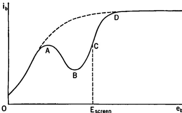
FIG. 4-14. Screen-grid Plate Characteristics.
