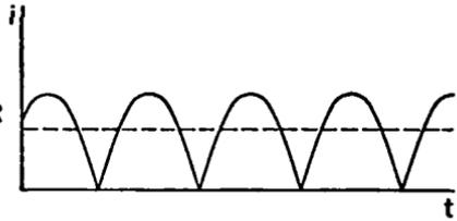
FIG. 5-4. Output of Full-wave Rectifier.
