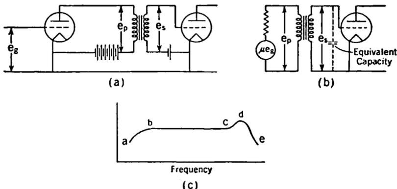
FIG. 7-9. (a) Transformer-coupled Amplifier. (b) Approximate Equivalent Circuit Showing Effect of Capacities. (c) Typical Frequency-response Curve.
