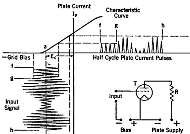
FIG. 11-29. Triode Rectification.
