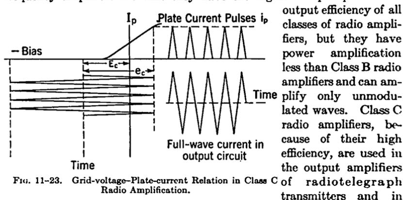
FIG. 11-23. Grid-voltage-Plate-current Relation in Class C of Radiotelegraph Transmitters and in
