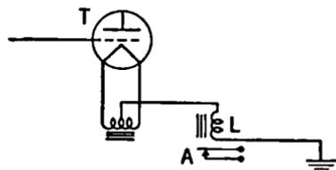
FIG. 12-15. Overload Relay.
