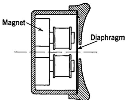
FIG. 6-4. Telephone Receiver.
