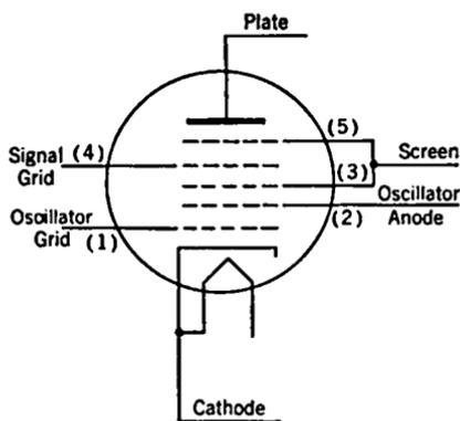
FIG. 4-20. Pentagrid Converter.
