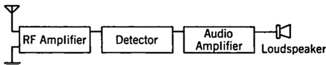
FIG. 13-3. Block Diagram of Simple Tuned Radio-frequency Receiver.
