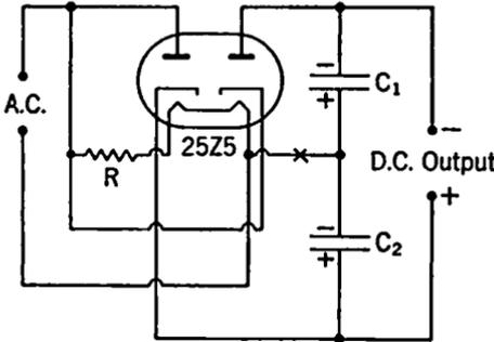
FIG. 5-5. Voltage-doubler Circuit.
