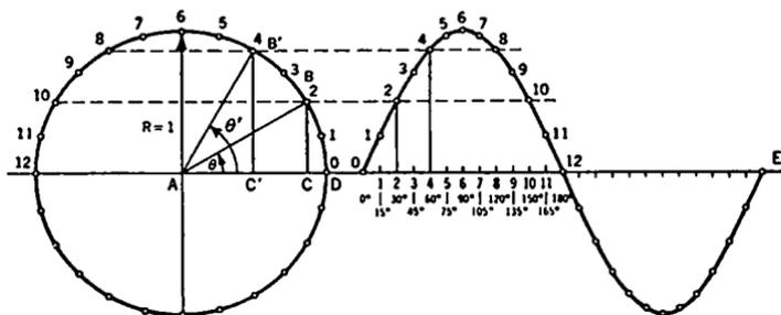
FIG. 1-8. Construction for Sine Curve.
