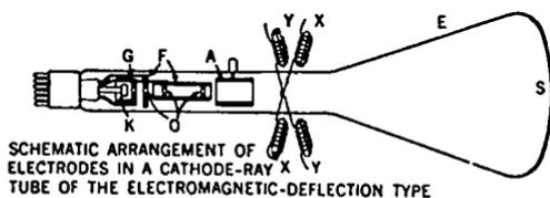
SCHEMATIC ARRANGEMENT OF ELECTRODES IN A CATHODE-RAY X TUBE OF THE ELECTROMAGNETIC-DEFLECTION TYPE
