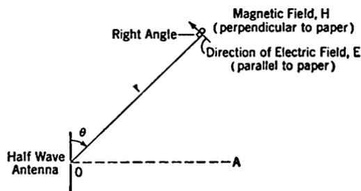
FIG. 9-16. Direction of the Electric Field about an Antenna.
