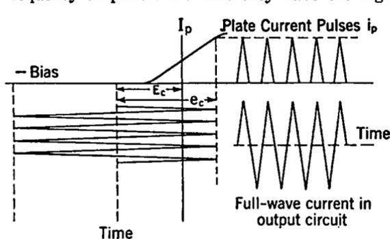
FIG. 11-23. Grid-voltage-Plate-current Relation in Class C of Radiotelegraph Transmitters and in
