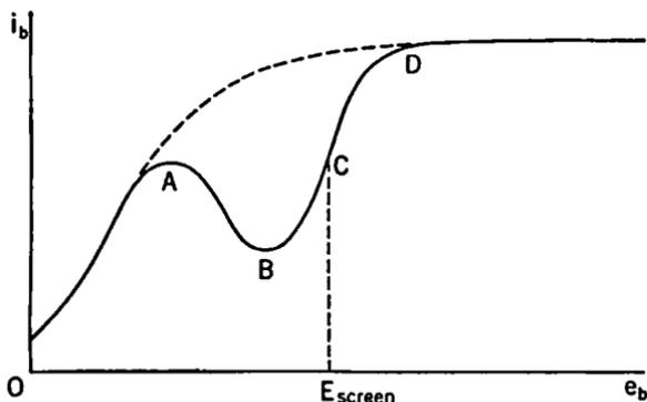
FIG. 4-14. Screen-grid Plate Characteristics.
