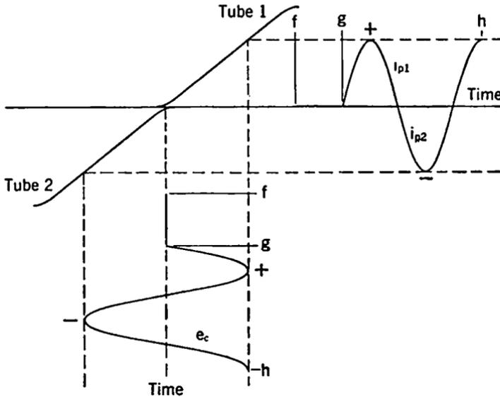
FIG. 12-12. Regulation of Plate Supply for Class B Audio Amplifier.
