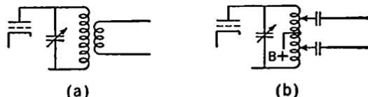
FIG. 16-13. Coupling a Transmitter to a Nonresonant Line. (a) Inductive coupling. (b) Direct coupling.
