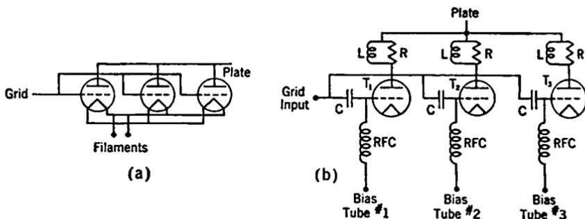
FIG. 11-15. Parallel Operation of Vacuum Tubes.
