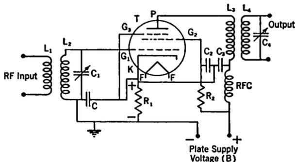
FIG. 11-12. Diagram of Pentode Radio-frequency Amplifier
