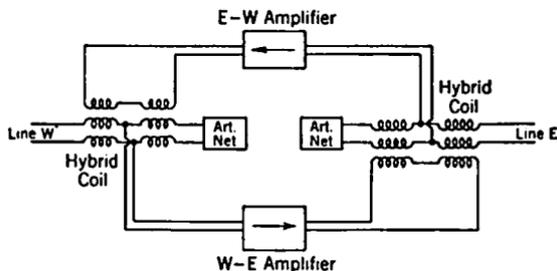
FIG. 6-8. Type 22 Telephone Repeater.
