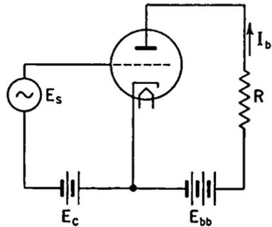
FIG. 4-11. Triode with Resistance Load.
