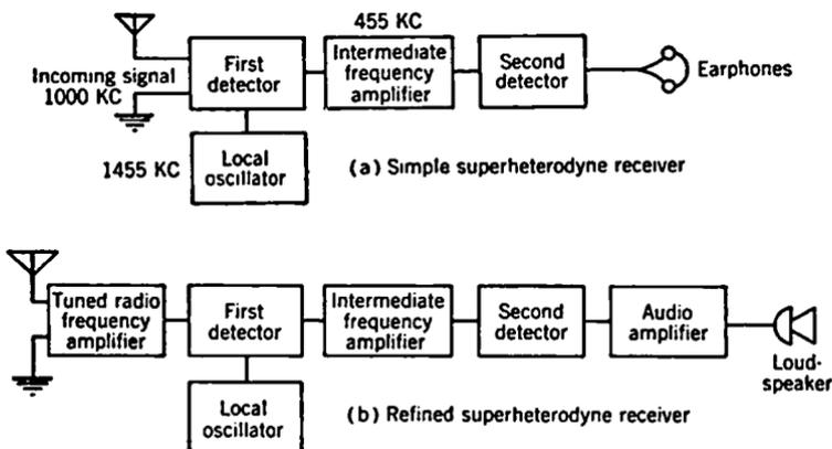
FIG. 10-4. Superheterodyne Receivers.
