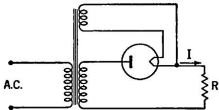
FIG. 5-1. Half-wave Rectifier.
