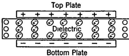
FIG. 3-22. Tension in Dielectric.
