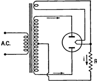
FIG. 5-3. Full-wave Rectifier.
