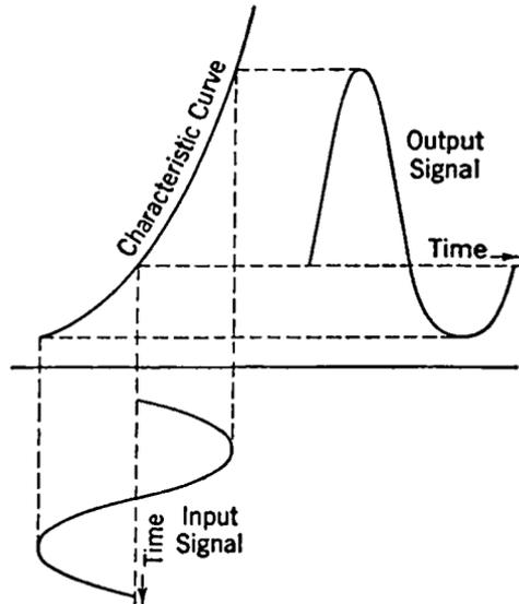
FIG. 6-2. Nonlinear Distortion.
