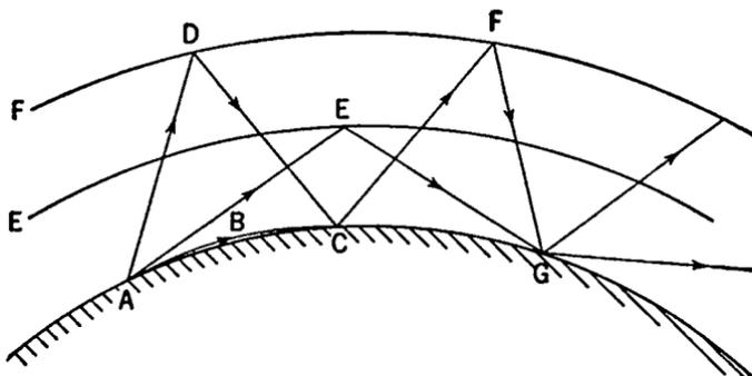
FIG. 15-9. Fading Due to Interference between Waves Which Have Traveled Different Distances.
