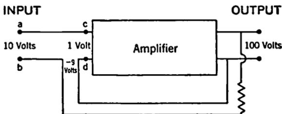
FIG. 7-14. Principle of Inverse Feedback.
