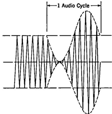
FIG. 14-2. Amplitude-modulated Wave.
