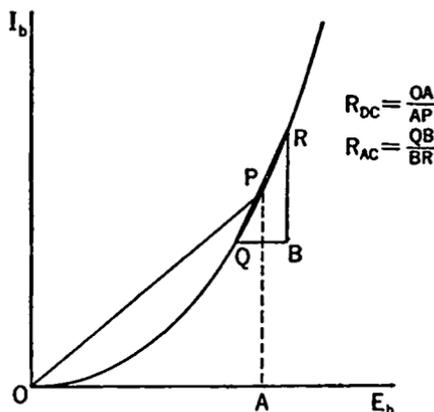
FIG. 4-4. D.C. and A.C. Plate Resistance.
