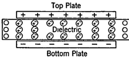
FIG. 3-22. Tension in Dielectric.
