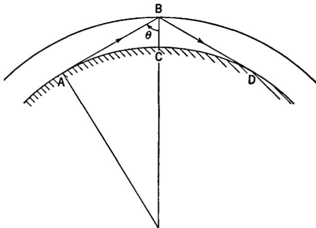
FIG. 15-6. Transmission by Means of Ionosphere Reflection, Showing Angle  $\theta$ .
