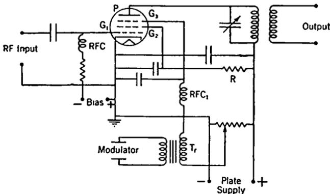
FIG. 12-10. Suppressor-grid Modulation.
