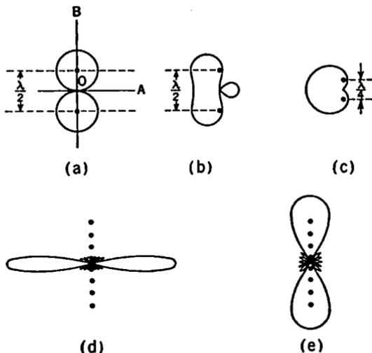
FIG. 16-18. Radiation Patterns for Commonly Used Antenna Arrays. (a) Two antennas spaced one half wave length and with  $180^\circ$  phase difference. (b) Same with  $90^\circ$  phase difference. (c) Two antennas spaced one quarter wave length and fed with  $90^\circ$  phase difference. (d) Broad-side array (currents in-phase). (e) End-fire array (currents  $180^\circ$  out-of-phase).
