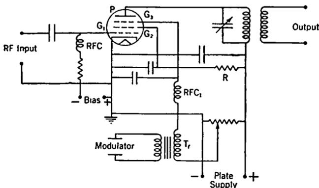
FIG. 12-10. Suppressor-grid Modulation.
