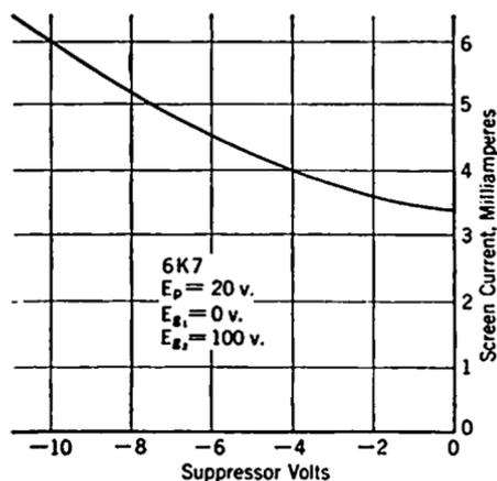
FIG. 8-3. Mutual Characteristic of 6K7 Tube. Suppresser Voltage-Screen Current.
