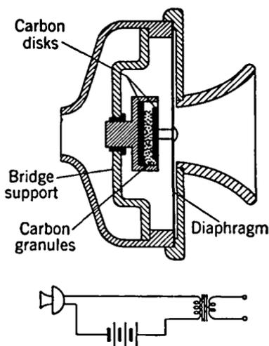
FIG. 6-3. Carbon Microphone.
