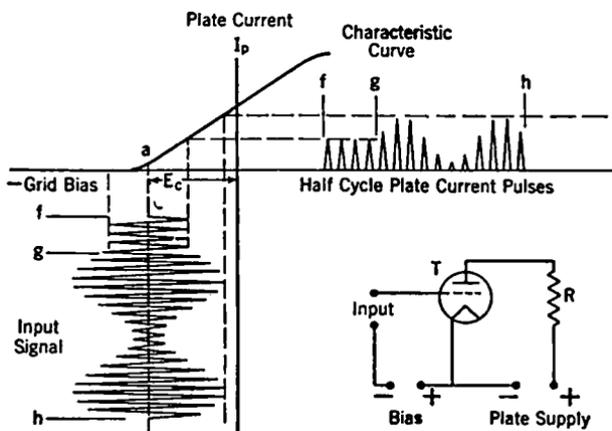
FIG. 11-29. Triode Rectification.
