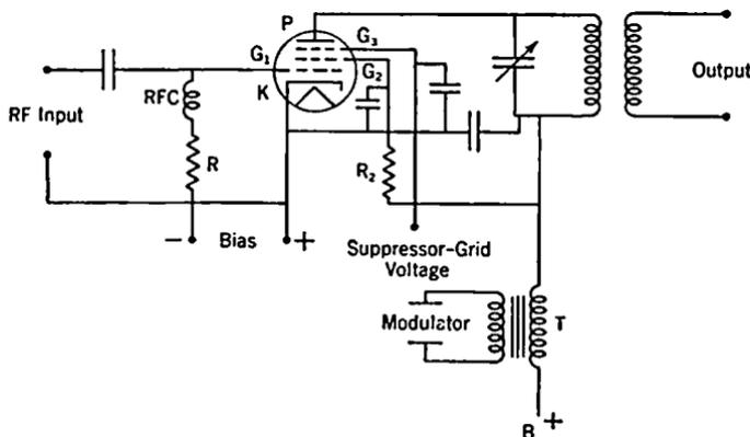
FIG. 12-9. Modulation of Screen-grid Tube.
