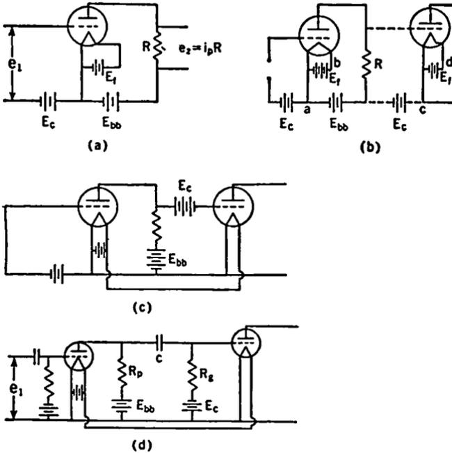
FIG. 7-1. Development of a Resistance-coupled Amplifier Circuit.
