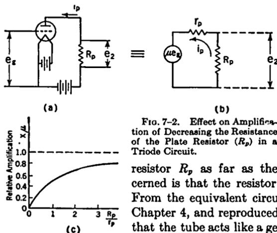
FIG. 7-2. Effect on Amplification of Decreasing the Resistance of the Plate Resistor ( $R_p$ ) in a Triode Circuit.
