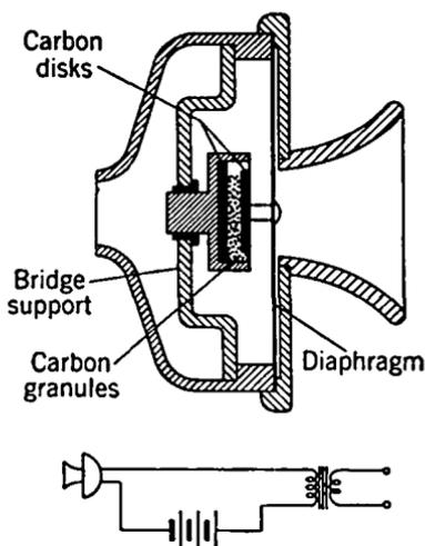
FIG. 6-3. Carbon Microphone.
