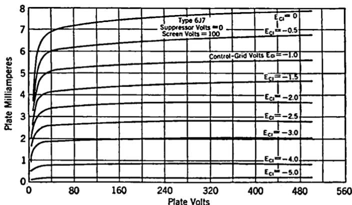
FIG. 4-16. Plate Characteristics of 6J7 Pentode.
