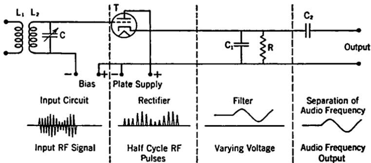
FIG. 11-30. Linear Plate Detector.
