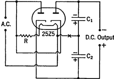
FIG. 5-5. Voltage-doubler Circuit.
