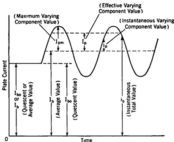
FIG. 4-10. Components of Plate Current.
