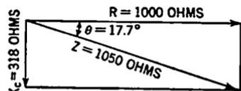
Fig. 3-24. Vector Diagram, Capacitive Circuit.
