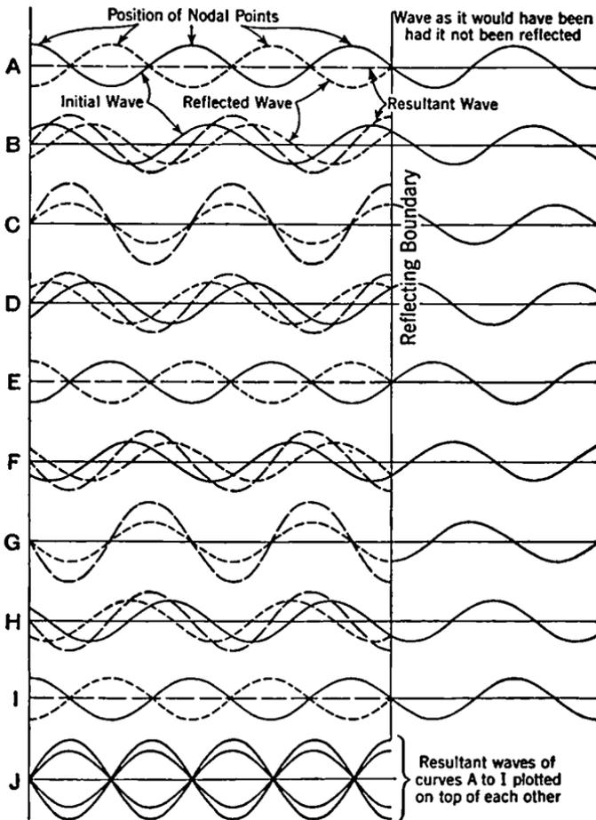
FIG. 9-5. Reflection of a Wave at a Boundary, Showing Addition of Initial and Reflected Waves to Give Standing Waves.
