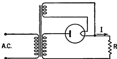
FIG. 5-1. Half-wave Rectifier.
