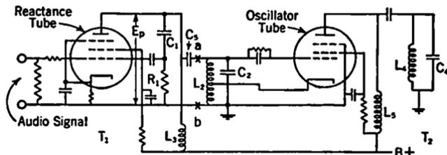
FIG. 14-7. Circuit Diagram of Oscillator and Reactance Tube.
