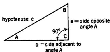
FIG. 1-3. Right Triangle with Parts Labeled.
