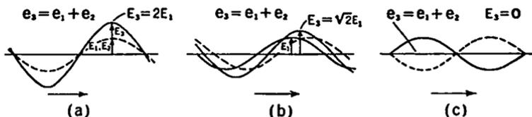
FIG. 9-3. Addition of Sine Waves: (a) in phase, (b)  $90^\circ$  phase difference, (c)  $180^\circ$  phase difference.
