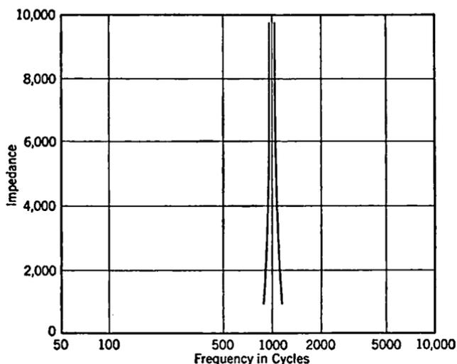
FIG. 11-3. Parallel Resonant Circuit at Audio Frequencies. Electrical Constants Equivalent to (B) of Fig. 11-2.
