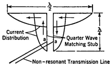
FIG. 16-8. Use of a Quarter-wave Matching Section to Match a High-impedance (500-ohm) Line to a Low-impedance (73-ohm) Antenna.
