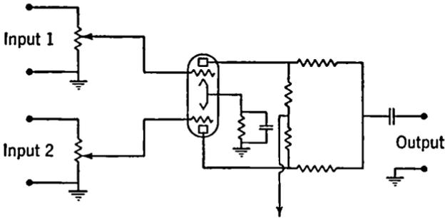
FIG. 7-24. Improved Electronic Mixing Circuit.
