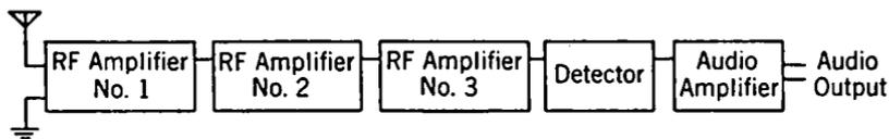
FIG. 13-4. Block Diagram of Multistage Tuned Radio-frequency Receiver.
