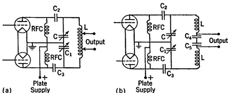
FIG. 11-17. Types of Push-pull Radio-amplifier Output Circuits.
