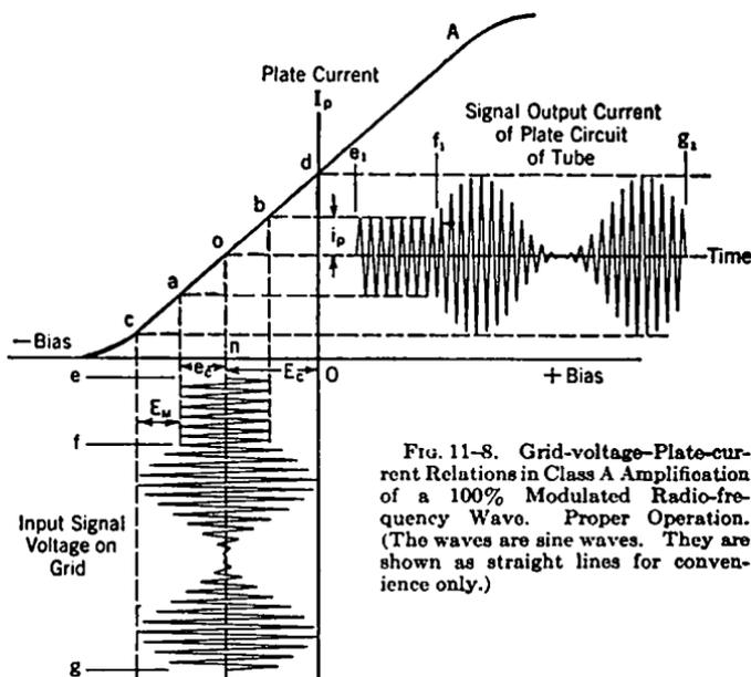
FIG. 11-8. Grid-voltage-Plate-current Relations in Class A Amplification of a 100% Modulated Radio-frequency Wave. Proper Operation. (The waves are sine waves. They are shown as straight lines for convenience only.)
