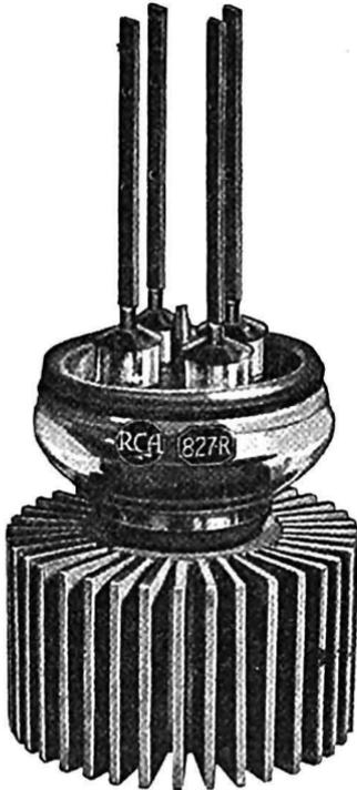
FIG. 4-5. Air-cooled Tube with Radiating Fins.
