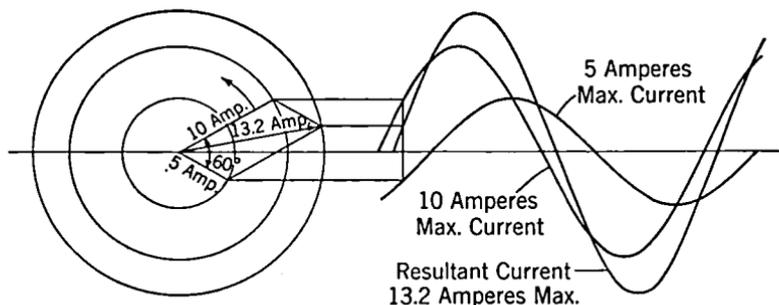
FIG. 3-3. Addition of Alternating Currents.
