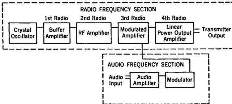
FIG. 12-2. Block Diagram of Crystal-controlled Amplitude-modulated Transmitter (low-level modulation).
