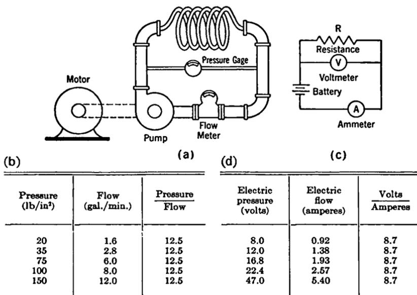
FIG. 2-1. Analogy Between Hydraulic and Electric Circuits.
