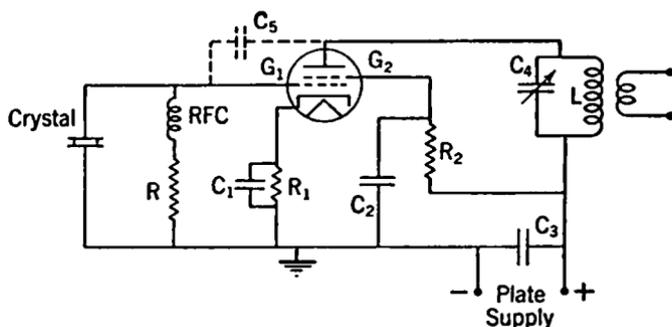
FIG. 12-4. Crystal-controlled Circuit—Tetrode Tube.
