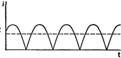
FIG. 5-4. Output of Full-wave Rectifier.
