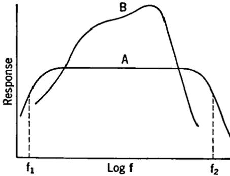
FIG. 6-1. Frequency Distortion.
