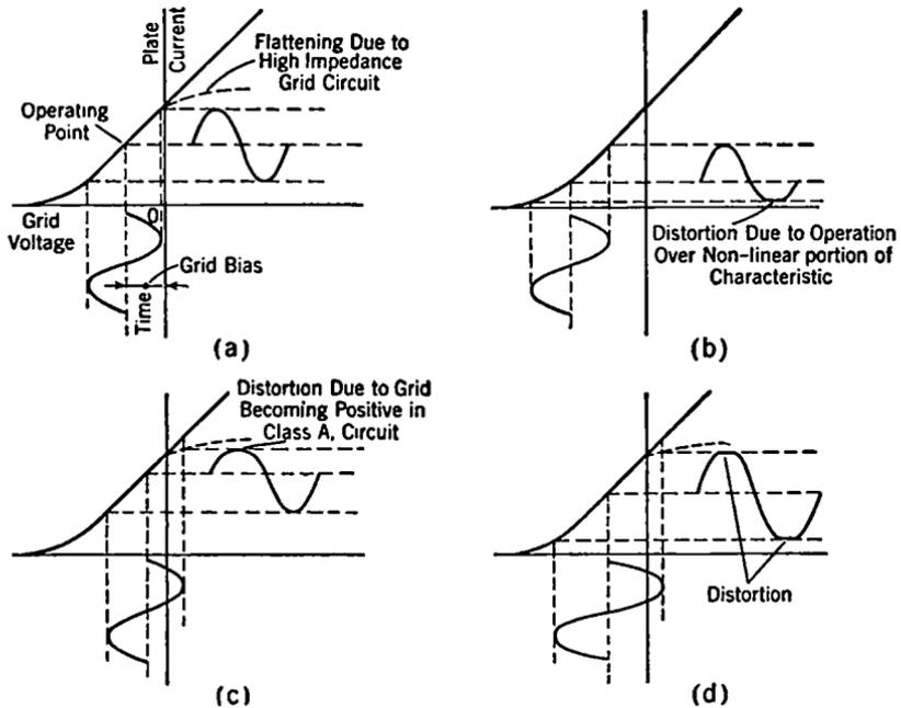
FIG. 7-6. Nonlinear Distortion Produced by Incorrect Operating Conditions. (a) Correct operating condition. (b) Grid bias too large. (c) Grid bias too small. (d) Correct grid bias but grid driving voltage too high.
