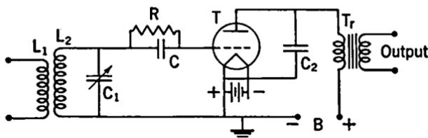
FIG. 11-32. Grid-circuit Detection.
