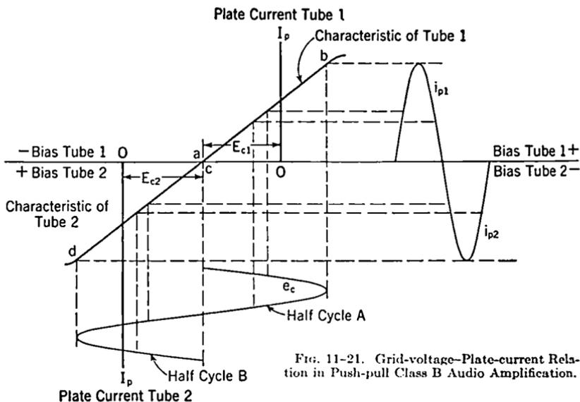
FIG. 11-21. Grid-voltage-Plate-current Relation in Push-pull Class B Audio Amplification.
