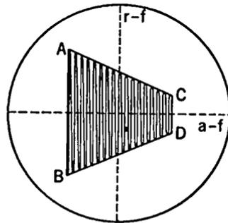
FIG. 8-9. Trapezoid Pattern Showing Modulation.
