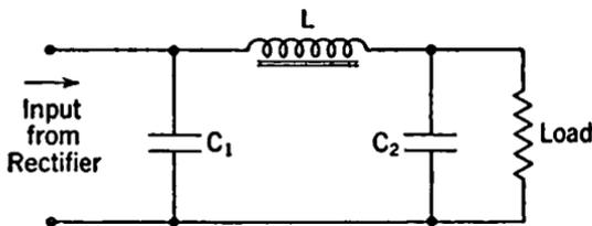
FIG. 5-7. Condenser-input Filter.
