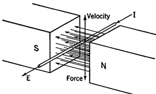
FIG. 2-28. Relation Between (a) Magnetic Field, Motion, and Voltage; (b) Magnetic Field, Current, and Force.
