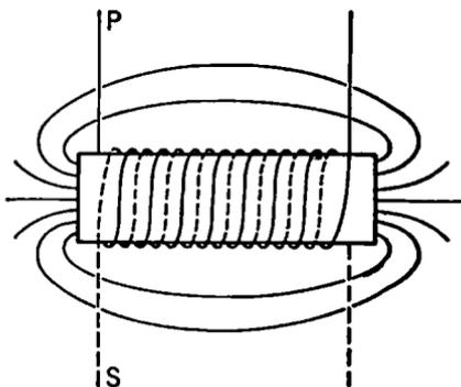
FIG. 3-30. A Mutual-inductance—Air-core Transformer.
