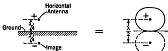
FIG. 16-22. Vertical Radiation Pattern of a Horizontal Antenna One Quarter Wave Length above the Ground, Determined by Considering the Antenna and Its Image.
