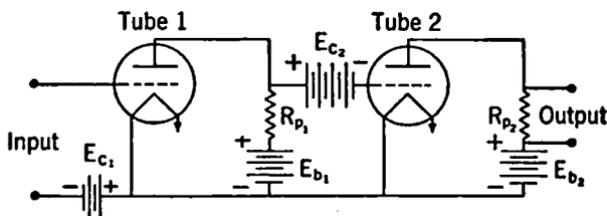
FIG. 7-18. A D.C. Amplifier Circuit.
