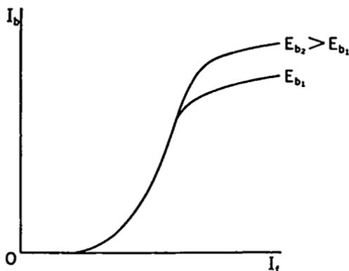
FIG. 4-3. Limitation of Diode Current by Space Charge.
