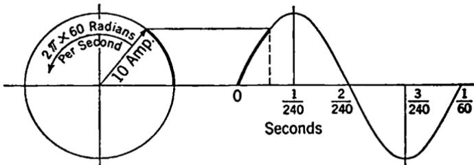
FIG. 3-2. A Rotating Radius Vector and Sine Wave Show the Variation of Current in a Conductor Carrying Alternating Current.
