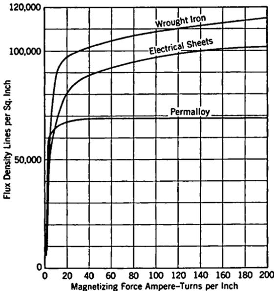
FIG. 2-27. Typical Magnetisation Curves.
