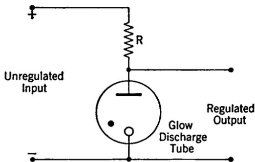
FIG. 5-10. Regulated Voltage Supply.
