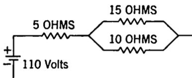
FIG. 2-5. A Series-Parallel Circuit.
