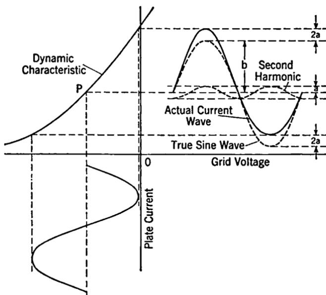
FIG. 7-8. Distortion Introduced by a Nonlinear Dynamic Characteristic.
