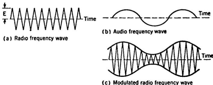
FIG. 10-6. Modulation of a Radio-frequency Wave.
