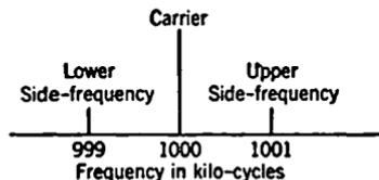
FIG. 10-8. Side Frequencies in Modulation.
