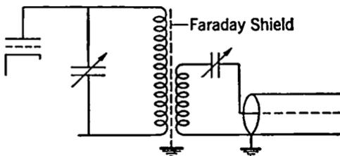
FIG. 16-14. Coupling a Transmitter to an Unbalanced Line.
