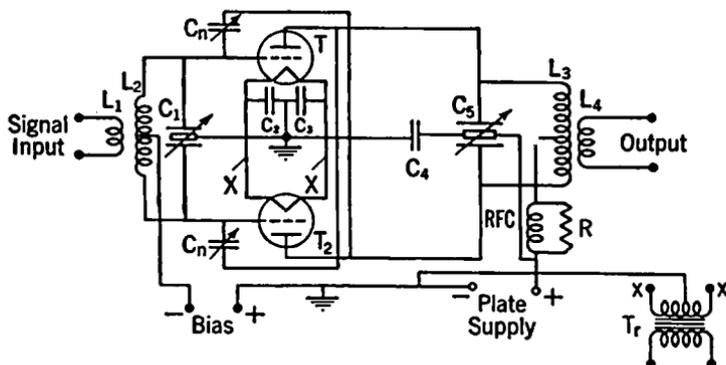
FIG. 11-16. Push-pull Triode Radio-frequency Amplifier.
