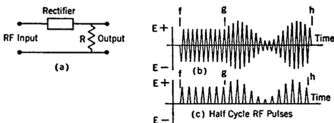
FIG. 11-24. Rectification of Radio-frequency Signal.
