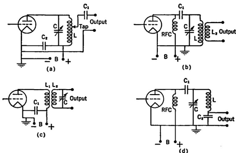
FIG. 11-6. Types of Single-ended Radio-amplifier Output Circuits.
