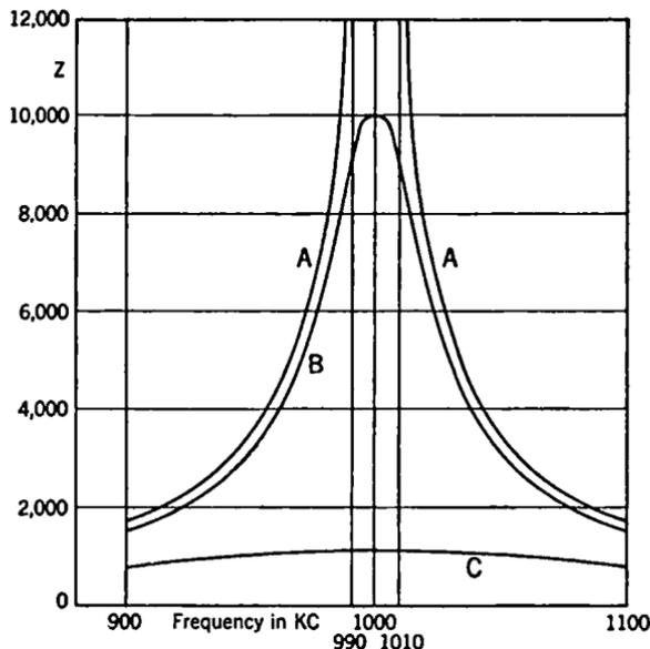
(b) Frequency, impedance characteristic of parallel circuit
