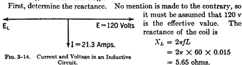
FIG. 3-14. Current and Voltage in an Inductive Circuit.
