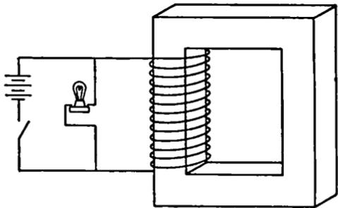
FIG. 3-12. Energy Is Stored in the Magnetic Field of a Transformer.
