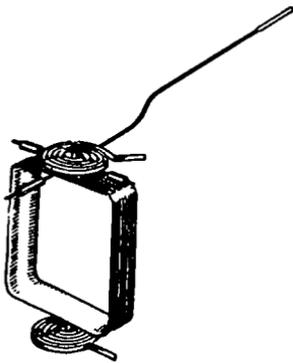
FIG. 2-32. The Moving-coil Assembly.
