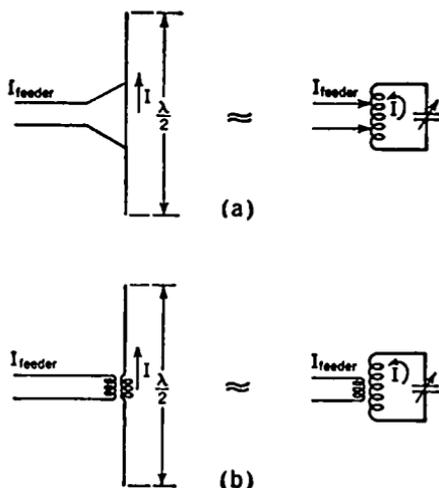
FIG. 16-2. The Half-wave Antenna Compared with a Parallel Resonant Circuit.
