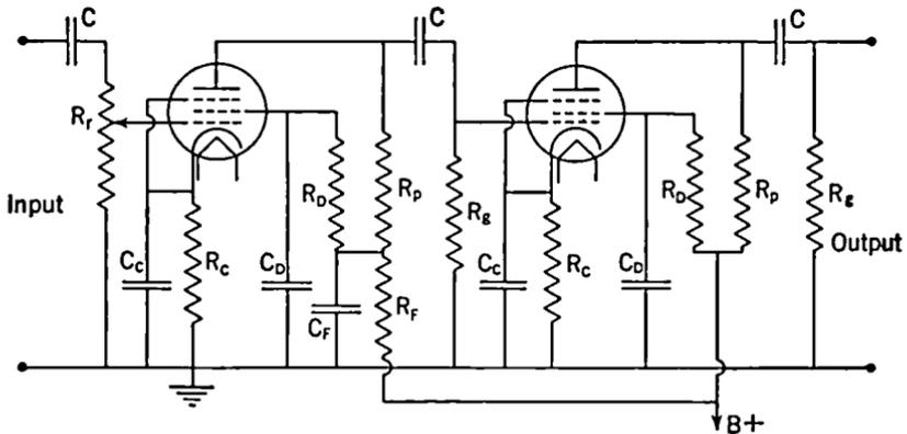
FIG. 7-5. A Two-stage Resistance-coupled Amplifier Using Pentodes.
