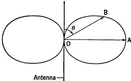
FIG. 16-3. Radiation Characteristic of a Half-wave Antenna.
