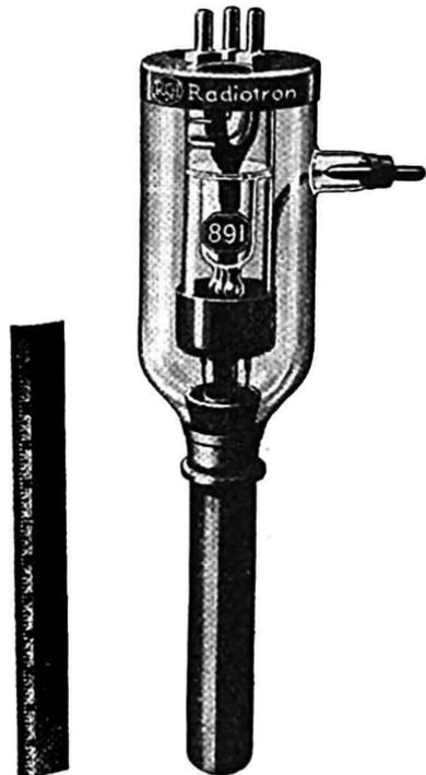
FIG. 4-6. Water-cooled Tube.
