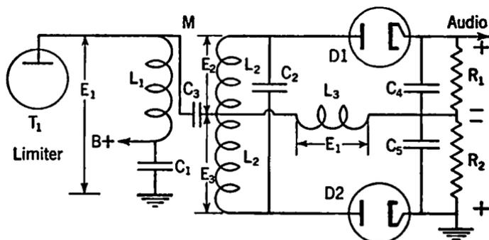
FIG. 14-10. Frequency-modulation Detector or Discriminator.
