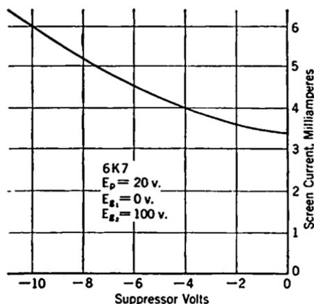
FIG. 8-3. Mutual Characteristic of 6K7 Tube. Suppressor Voltage-Screen Current.
