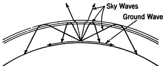
FIG. 15-1. Ground-wave and Sky-wave Radiations.
