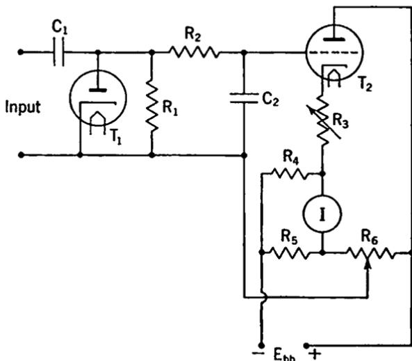
FIG. 8-10. Diode Vacuum-tube Voltmeter with D.C. Amplifier.
