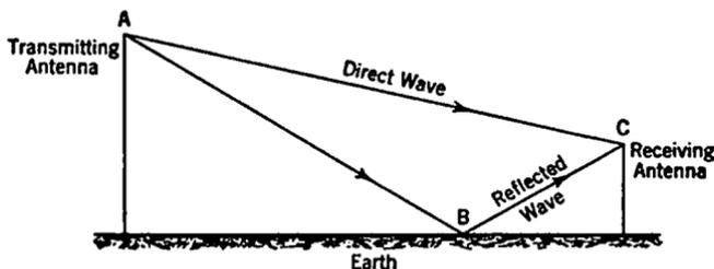
FIG. 15-11. Reception of Direct and Reflected Waves at Ultrahigh Frequencies.
