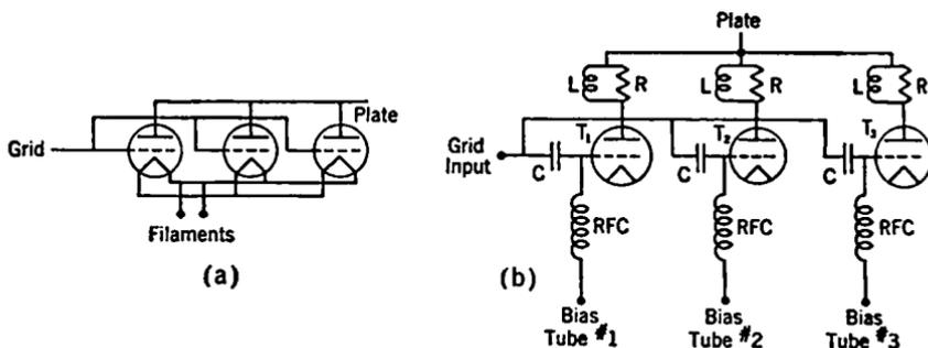
FIG. 11-15. Parallel Operation of Vacuum Tubes.
