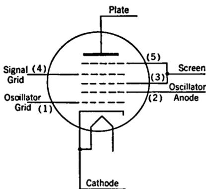
FIG. 4-20. Pentagrid Converter.
