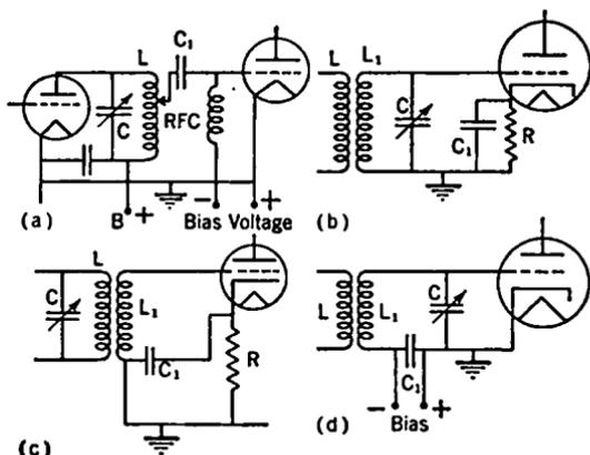
FIG. 11-5. Types of Radio-amplifier Input Circuits.
