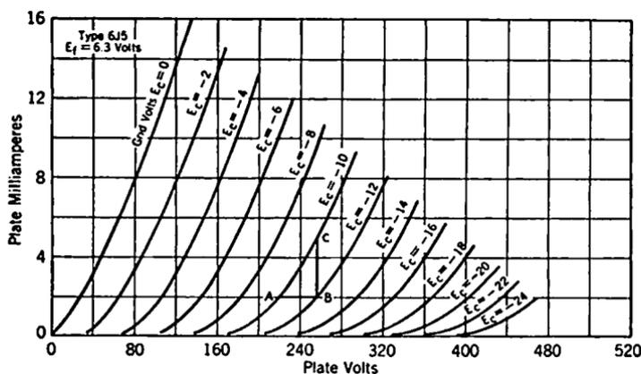
FIG. 4-9. Plate Characteristics of 6J5 Triode.
