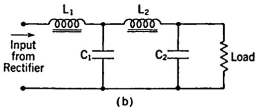
FIG. 5-6. Choke-input Filter Circuits: (a) Single-section, (b) Two-section.
