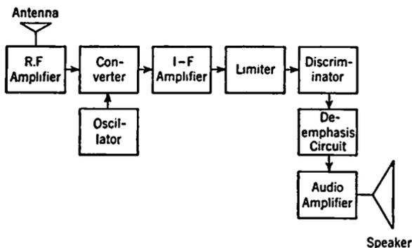
FIG. 14-8. Block Diagram of Typical Frequency-modulation Receiver.
