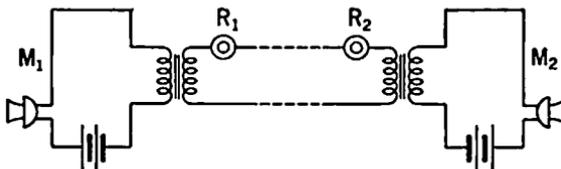
FIG. 6-6. Local-battery Telephone Circuit.
