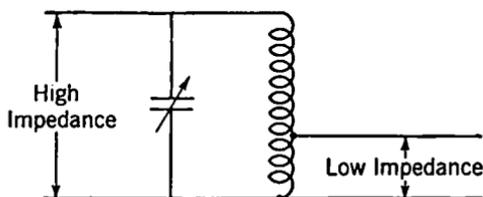
FIG. 3-29. Impedance Matching Using a Parallel Resonant Circuit.
