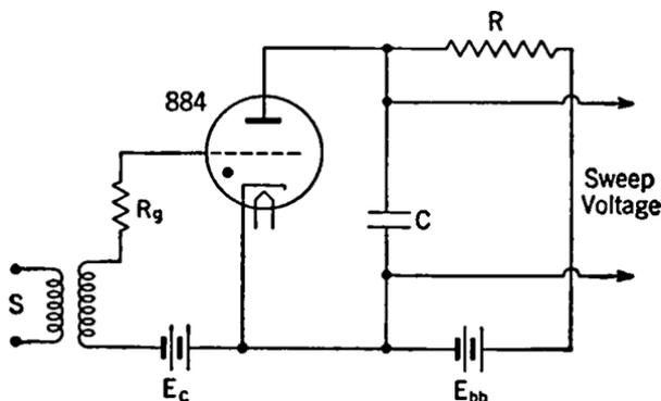
FIG. 8-4. Cathode-ray Sweep Generator.
