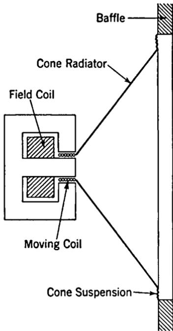
FIG. 6-5. Cone Type of Loudspeaker.
