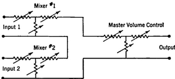
FIG. 7-26. Complete Mixing System.
