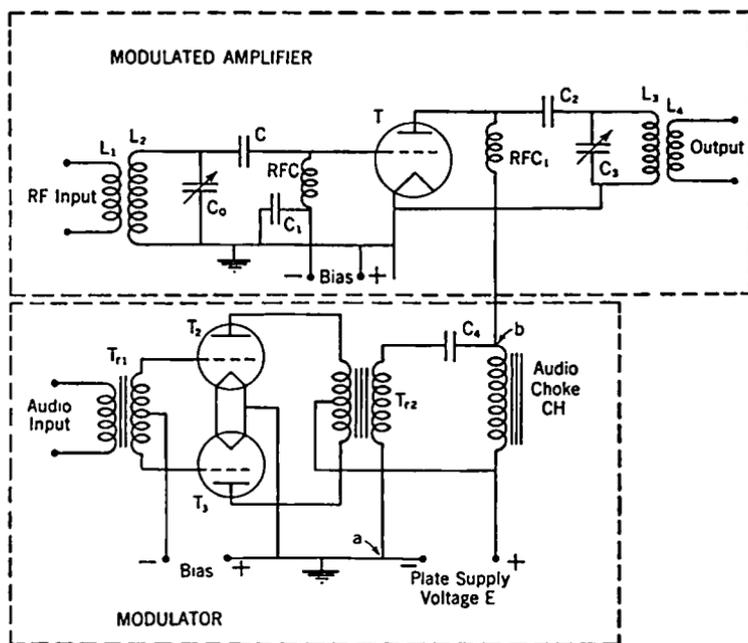
FIG. 12-5. Plate Modulation.
