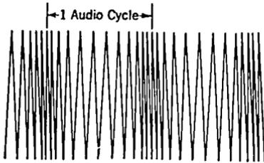
FIG. 14-1. Frequency-modulated Wave.
