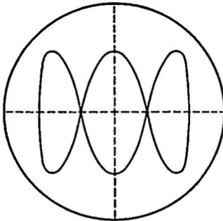
FIG. 8-8. Lissajous Figure, Frequency Ratio 3:1.
