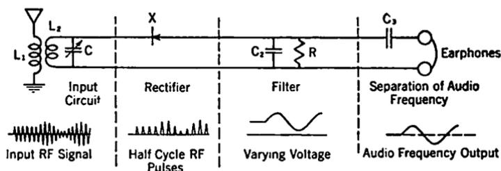
FIG. 11-26. Simple Crystal Detector.
