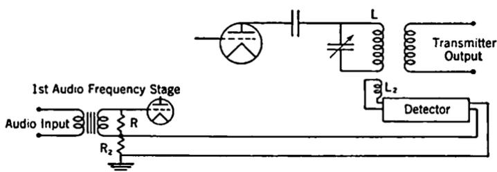
FIG. 12-23. Inverse Feedback Applied to a Modulated Transmitter.
