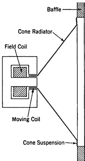
FIG. 6-5. Cone Type of Loudspeaker.
