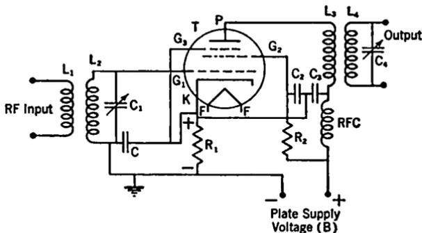
FIG. 11-12. Diagram of Pentode Radio-frequency Amplifier
