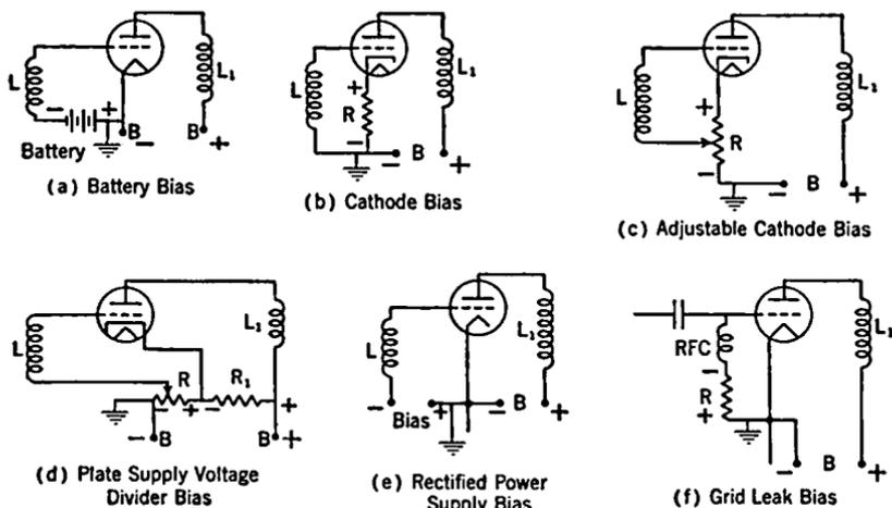
FIG. 11-7. Grid-bias Voltage Supplies.
