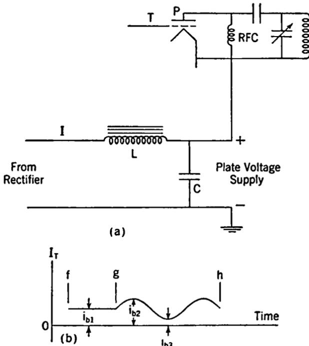
FIG. 12-11. Class B Radio Amplifier Plate-supply Regulation.
