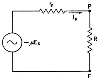
FIG. 4-13. Equivalent Circuit Corresponding to Fig. 4-11.
