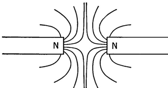
FIG. 2-22. The Magnetic Field about Two Like Poles.
