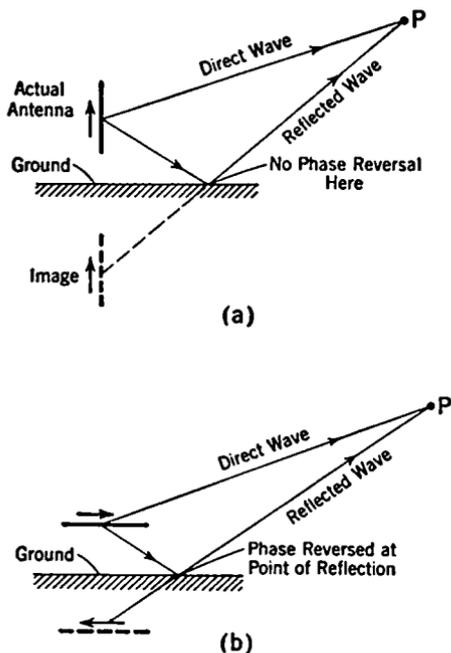
FIG. 16-21. Image Antenna Due to a (Perfectly) Reflecting Ground. (a) Vertical antennas (reflection without phase reversal). (b) Horizontal antennas (phase reversal on reflection).
