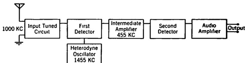
FIG. 13-6. Block Diagram of a Simple Superheterodyne.
