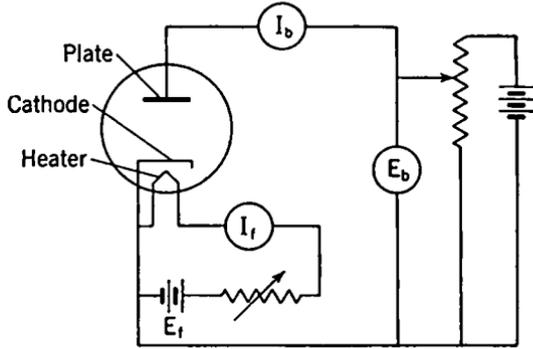
FIG. 4-1. Circuit for Obtaining Diode Characteristics.
