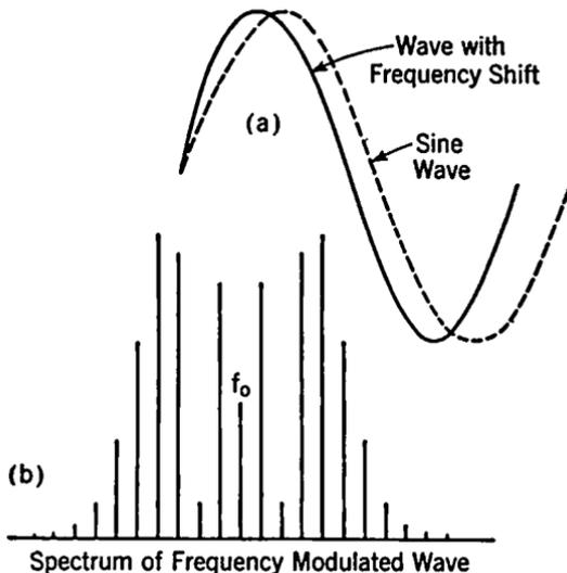
FIG. 14-4. Distorted Wave and Frequency-modulation Spectrum.
