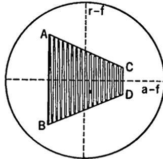
FIG. 8-9. Trapezoid Pattern Showing Modulation.
