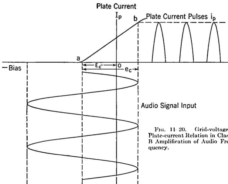
FIG. 11-20. Grid-voltage-Plate-current Relation in Class B Amplification of Audio Frequency.
