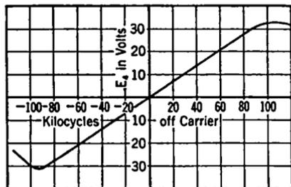
FIG. 14-11. Frequency Variation Plotted against Audio-frequency Output in a Discriminator.
