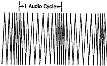
FIG. 14-1. Frequency-modulated Wave.
