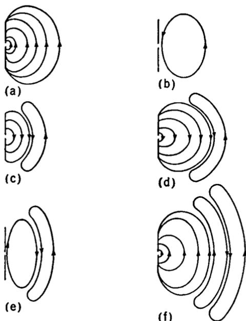
FIG. 9-15. Electric-field Distribution about an Antenna at Successive Instants over a Complete Electrical Cycle.
