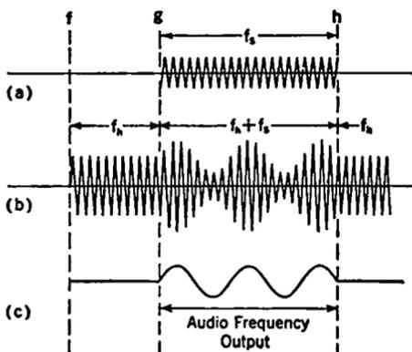
FIG. 11-34. Detection of Keyed Transmitted Continuous Wave.
