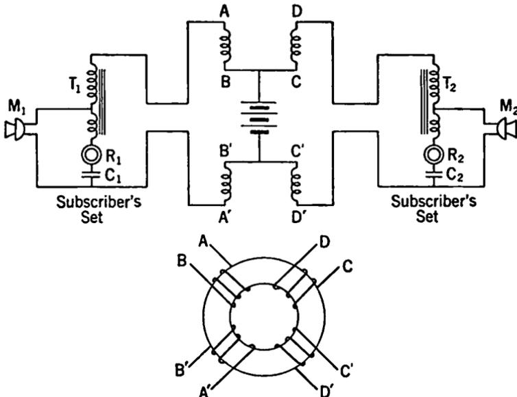
FIG. 6-7. Common-battery Telephone Circuit.
