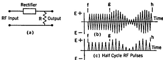
FIG. 11-24. Rectification of Radio-frequency Signal.
