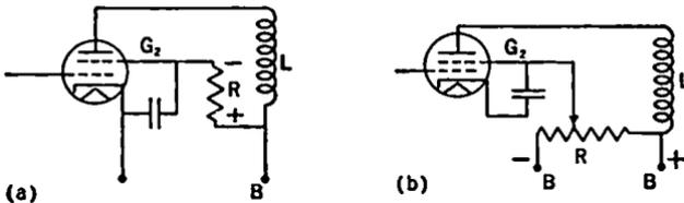
FIG. 11-13. Screen-grid Voltage Supplies.
