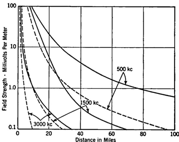
FIG. 15-2. Effect of Frequency and Ground Conductivity upon the Strength of the Ground-wave Signal. Solid lines: fairly good conductivity ( $100 \times 10^{-16}$  e.m.u.). Dashed lines: poor conductivity ( $20 \times 10^{-16}$  e.m.u.).
