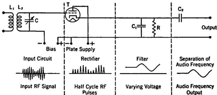
FIG. 11-30. Linear Plate Detector.
