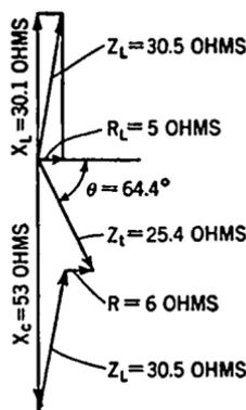
FIG. 3-25. Vector Diagram—Resistance, Inductance, and Capacitance in Series.
