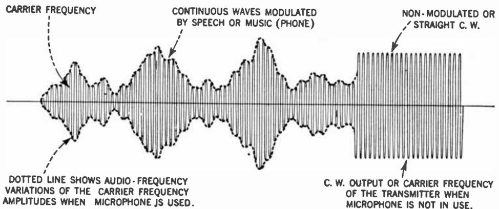
FIG. 26.—Curves illustrating how high-frequency oscillations are modulated according to the characteristics of voice or music.
