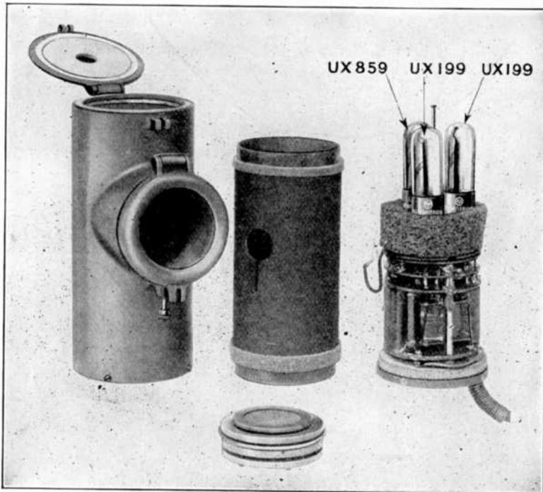
FIG. 39.—A condenser microphone disassembled, showing the microphone (lower center) and compact speech amplifier consisting of three tubes, required to build up the low output level of the microphone to provide proper grid voltages for operating the audio amplifiers.
