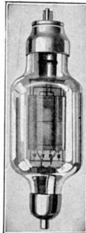
FIG. 49.—A 1000-watt transmitting tube.
