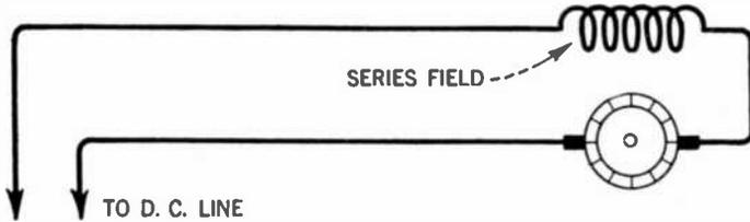
FIG. 74.—Elementary diagram of a series-wound motor.
