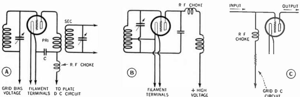
FIG. 35.—Illustrating three ways in which r-f. choke coils may be advantageously used.
