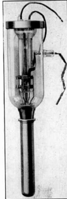
FIG. 51.—A view of a water-cooled tube showing filament leads at the top, grid connection at the right and the cylindrically shaped plate at the bottom. The plate is inserted in the water jacket.
