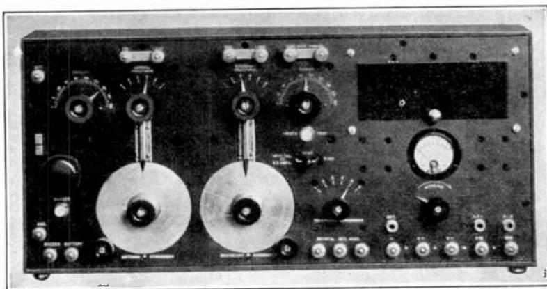
FIG. 67.—Commercial long-short wave receiver, type IP-501A, containing detector and audio-amplifier system.
