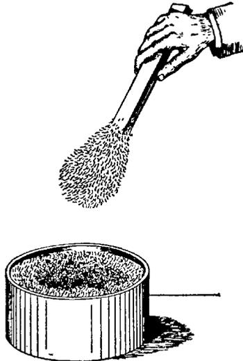
Fig. 7. Iron Filings Clinging to End of a Bar Magnet
