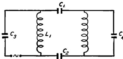
Fig. 68. An Indirect-Capacity Coupled Circuit
