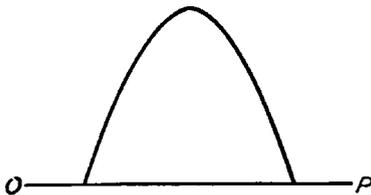
Fig. 44. One Pulsation Caused by Passing a Coil through a Magnetic Field
