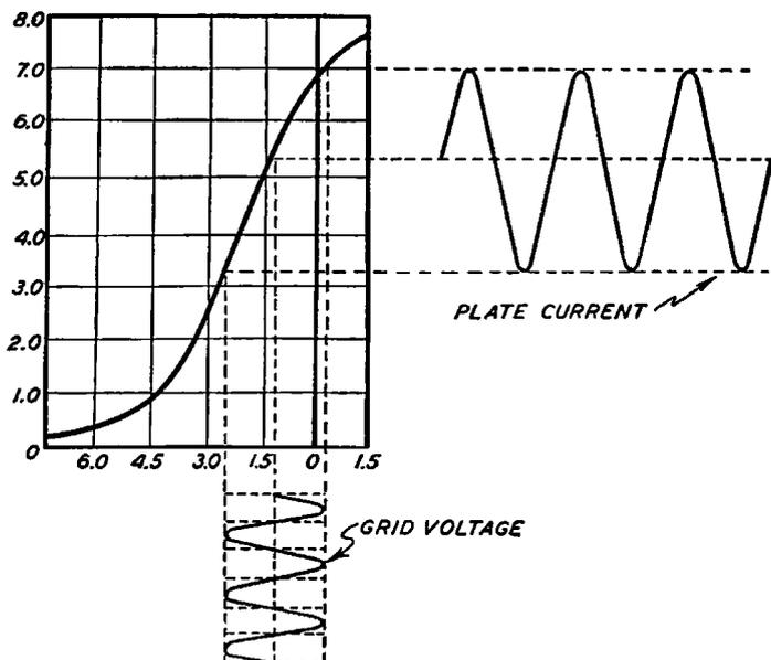
Fig. 80. Result of Operating a Tube Without Enough Negative Grid Bias
