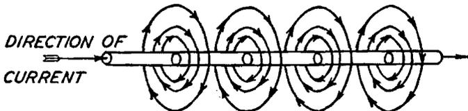
Fig. 16. Diagram Showing Lines of Force Around a Wire
