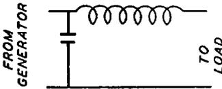
Fig. 74. A Filter Which Passes Low Frequencies
