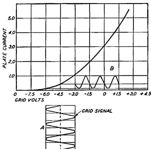
Fig. 55. Characteristic Curve of a Vacuum Tube Showing Result of Operating the Grid Signal Voltage on the Bend of the Curve
