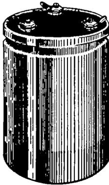
Fig. 34. Typical Electrolytic Condenser Having Multiple Electrodes
