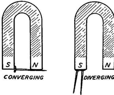
Fig. 10. Diagram Illustrating Laws of Attraction and Repulsion
