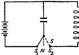
Fig. 63. Method of Charging and Discharging Condenser
