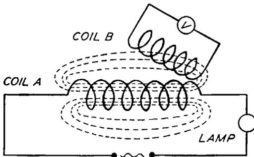
Fig. 49. Method of Exploring a Magnetic Field Around a Coil
