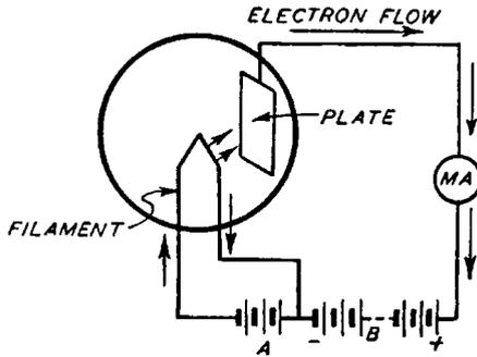
Fig. 50. Direction of Electron Flow in a Vacuum Tube Circuit
