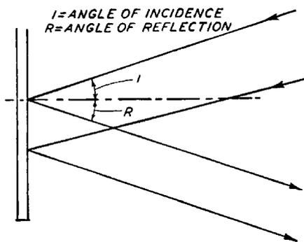
Fig. 3. Reflection of Sound Waves from a Hard Smooth Plane Surface
