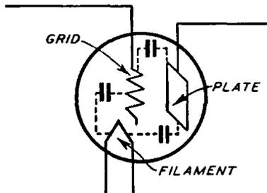
Fig. 60. Capacity Effect Between the Different Tube Elements
