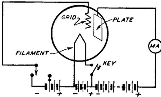
Fig. 51. A Radio Tube Circuit
