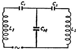
Fig. 65. A Direct-Capacity Coupled Circuit
