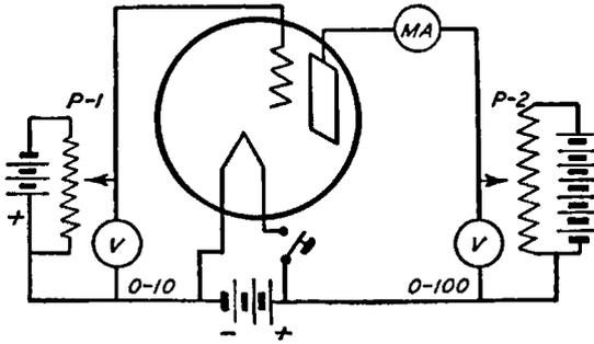
Fig. 52. A Radio Tube Test Circuit
