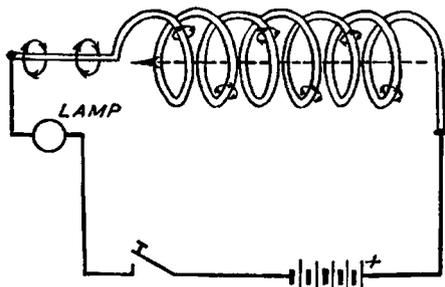
Fig. 23. Magnetic Fields Around a Conductor and Coil
