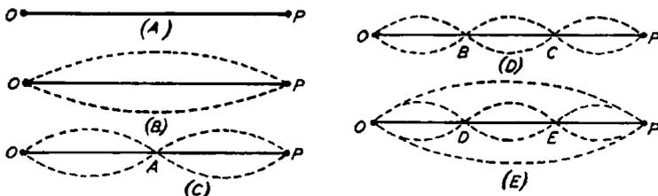
Fig. 5. Diagram Showing How First and Second Harmonics and Overtones Are Produced
