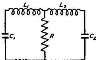
Fig. 66. A Direct Resistance Coupled Circuit
