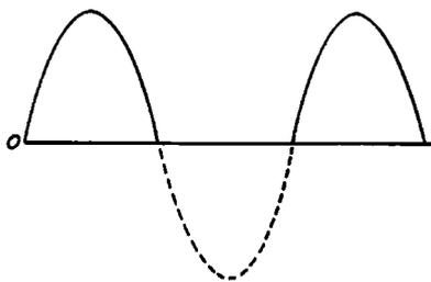
Fig. 57. Diagram Showing How a Pulsating Direct Current Is Obtained from Alternating Current
