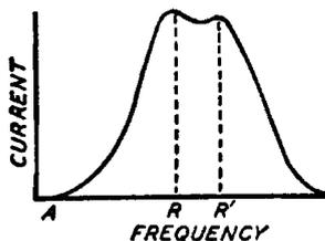
Fig. 70. Curve Showing How Mutual Inductance Effects the Resonance Frequency
