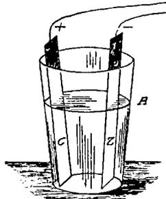
Fig. 14. A Simple Voltaic Cell
