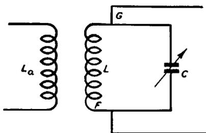
Fig. 89. Antenna Tuning Circuit
