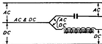
Fig. 71. A Simple Filter Circuit
