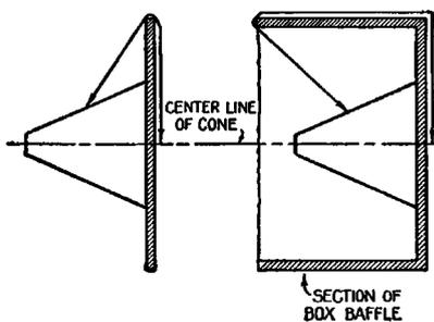
Fig. 99. Flat and Box Type Baffles
