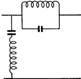
Fig. 76. A Filter Circuit Designed to Reject a Particular Frequency
