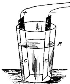
Fig. 14. A Simple Voltaic Cell
