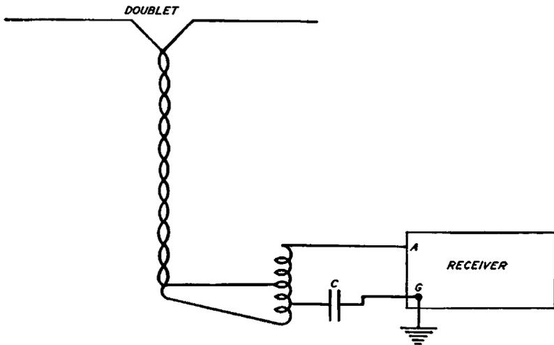
Fig. 103D. Antenna System Providing Noise Reduction Only on Short-Wave Bands
