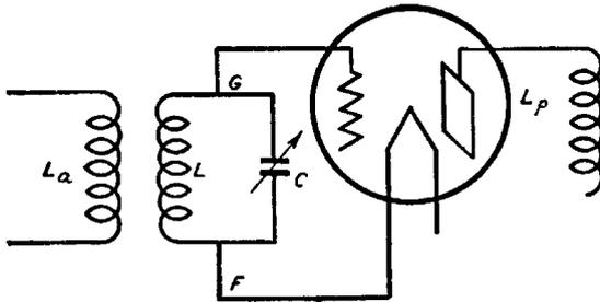
Fig. 90. A Stage of Radio Frequency
