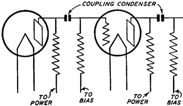
Fig. 85. A Resistance Coupled Amplifier
