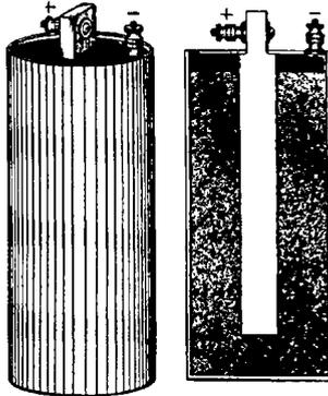
Fig. 15. Cross Section of a Dry Cell
