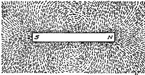
Fig. 12. Magnetic Field of a Bar Magnet
