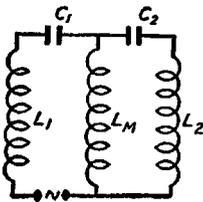
Fig. 64. A Direct-Inductively Coupled Circuit
