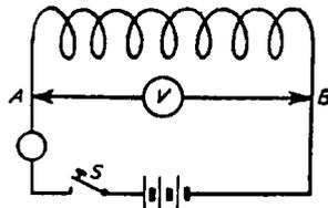
Fig. 39. Experiment Illustrating Counter Electromotive Force of a Coil
