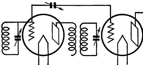
Fig. 91. The Neutrodyne Method of Controlling Regeneration
