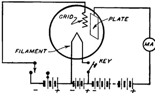
Fig. 51. A Radio Tube Circuit
