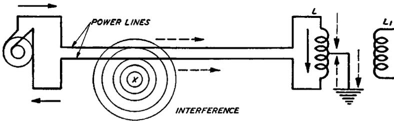
Fig. 103C. Desired Current, Indicated by Full Arrows, Flows around Complete Circuit Setting up Magnetic Field around Coil *L*. Interference Current Flows through Coil *L* in Phase Opposition, Preventing the Setting up of a Magnetic Field. Energy Appearing in *L*<sub>1</sub> Will Be Due Only to the Desired Current Flow in *L*
