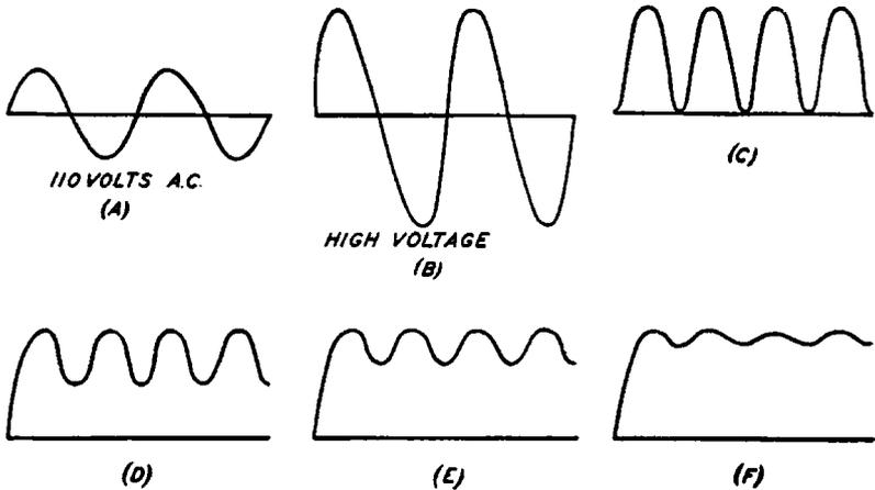
Fig. 105. Curves Showing the Result of Passing Alternating Current (A) through a Transformer (B), Rectifier Tube (C), and Filters (D, E and F)
