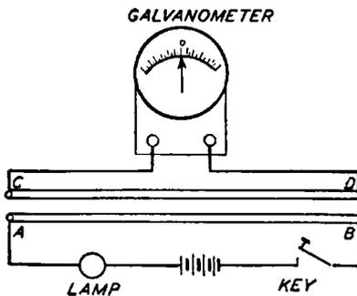
Fig. 21. Electromagnetic Induction Experiment
