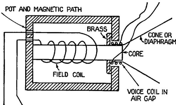
Fig. 98. Diagram of Construction of Dynamic Speaker Field
