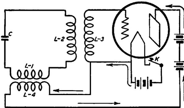
Fig. 87. Diagram of an Oscillator Circuit
