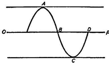
Fig. 45. Diagram Showing One Cycle of Alternating Current
