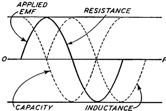
Fig. 46. Diagram Showing Effect of Capacity and Inductance on the Flow of Current
