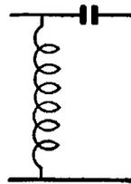
Fig. 75. A Filter Which Passes High Frequencies
