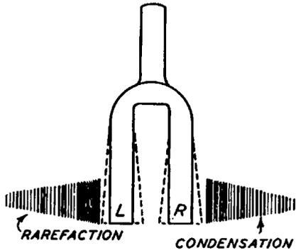
Fig. 2. Sound Waves from a Tuning Fork
