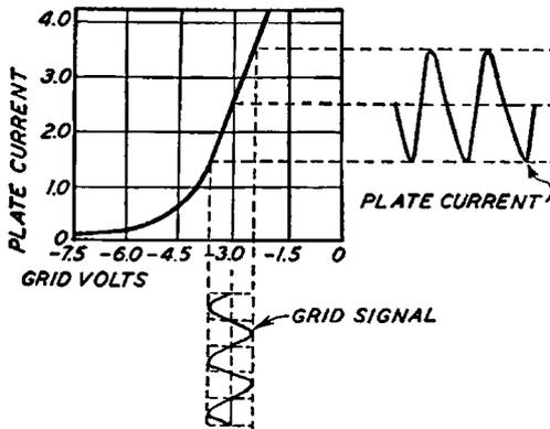
Fig. 78. Showing Type of Signal Produced When Tube Is Operated on Straight Portion of Characteristic Curve
