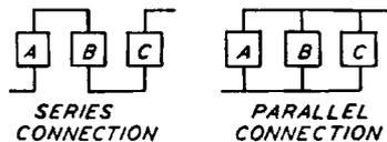
Fig. 25. Diagram Showing Difference between Series and Parallel Circuits
