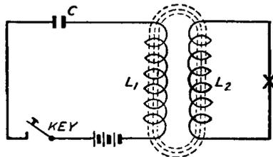
Fig. 67. An Indirect-Inductively Coupled Circuit
