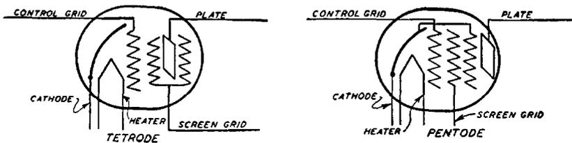
Fig. 61. Diagram Showing the Elements in a Tetrode and Pentode Tube
