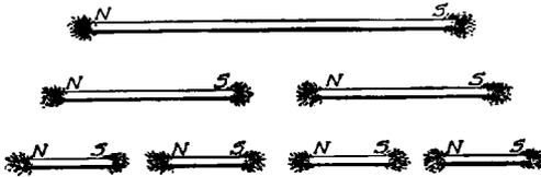
Fig. 8. Results of Breaking a Bar Magnet
