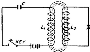
Fig. 67. An Indirect-Inductively Coupled Circuit
