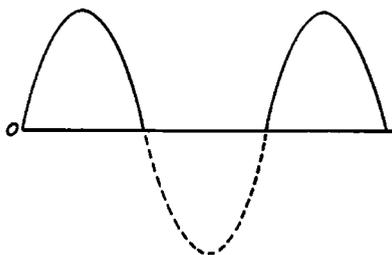
Fig. 57. Diagram Showing How a Pulsating Direct Current Is Obtained from Alternating Current
