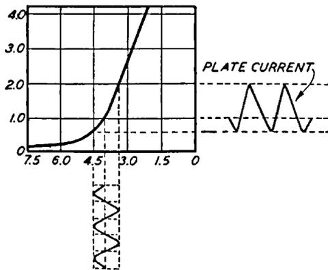
Fig. 79. Curves Showing Result of Charging the Grid Bias
