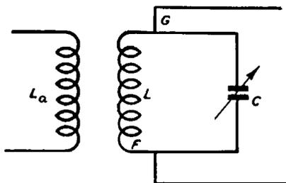
Fig. 89. Antenna Tuning Circuit
