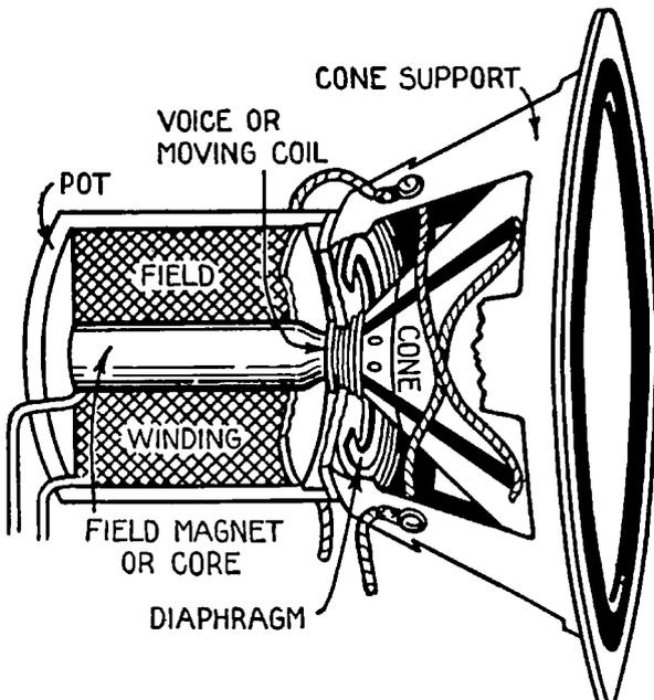
Fig. 97. A Cutaway View of a Dynamic Speaker Unit
