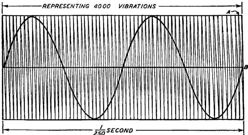
Fig. 92. A Carrier Wave and Two Cycles of 500 Cycle Note
