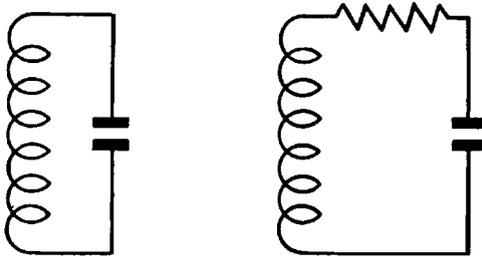
Fig. 62. Oscillatory Circuits
