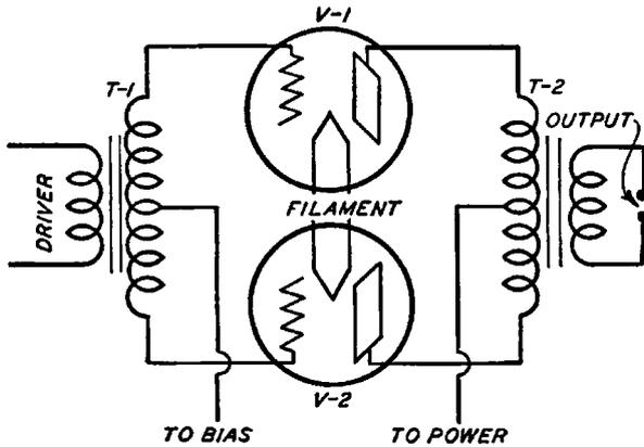
Fig. 82. A Push-Pull Amplifier Stage
