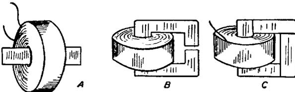
Fig. 43. Construction of Iron-Core Inductance or Choke Coil
