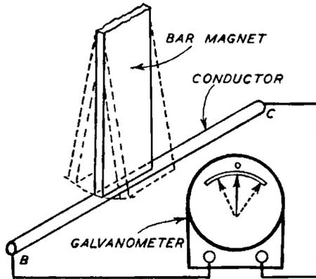
Fig. 20. Electric Circuit Produced by a Moving Magnetic Field
