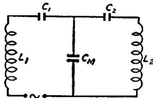
Fig. 65. A Direct-Capacity Coupled Circuit
