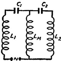
Fig. 64. A Direct-Inductively Coupled Circuit
