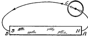
Fig. 13. Diagram Showing Method of Plotting Lines of Force in a Magnetic Field
