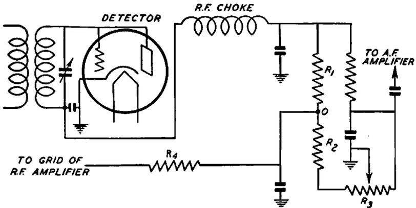
Fig. 94 (B). Automatic Volume Control Circuit
