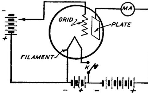
Fig. 53. Circuit Connections for Determining the Amplification Factor of Tube Circuit Connections Arranged for Varying the Grid Voltage
