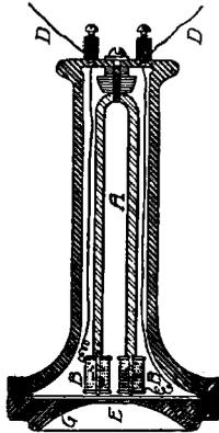
Fig. 95. A Telephone Receiver
