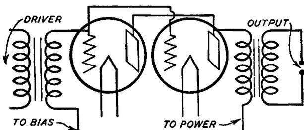
Fig. 81. A Plate Circuit Using Two Power Tubes in Parallel
