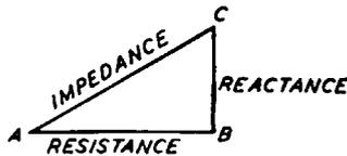
Fig. 47. Diagram Showing the Effect of Resistance and Reactance
