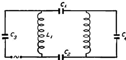
Fig. 68. An Indirect-Capacity Coupled Circuit
