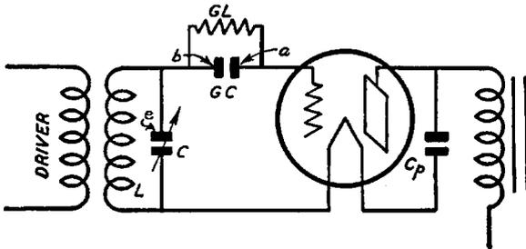
Fig. 94 (A). Diagram of a Detector Circuit
