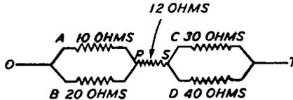
Fig. 32. Resistance Connected in Series-Parallel Circuit
