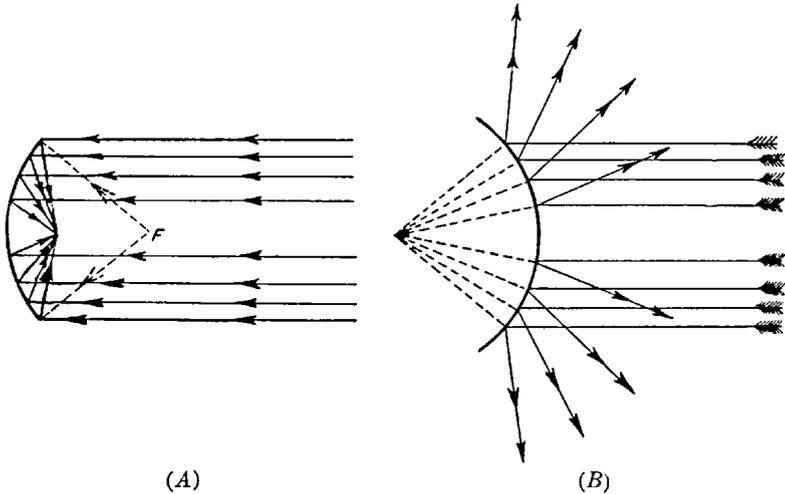
Fig. 4. Reflection of Sound Waves from Curved Surfaces
