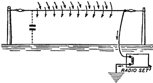
Fig. 102. Action of Radio Waves on Antenna
