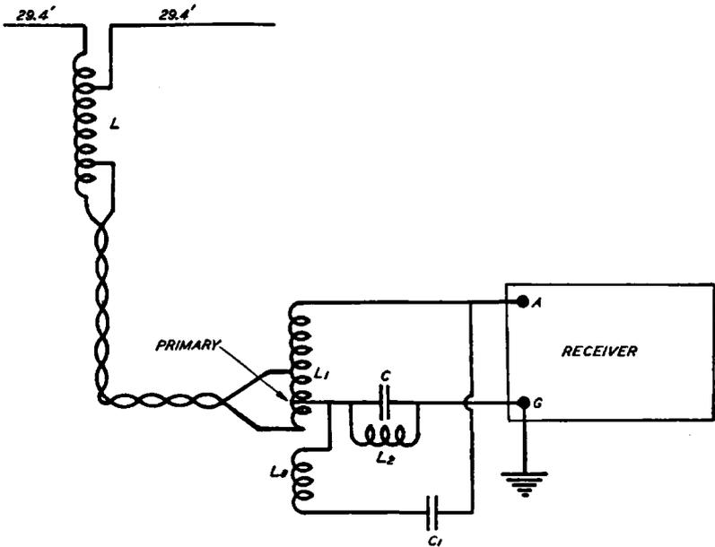
Fig. 103E. Antenna System Providing Noise Reduction in Broadcast and Short-Wave Bands
