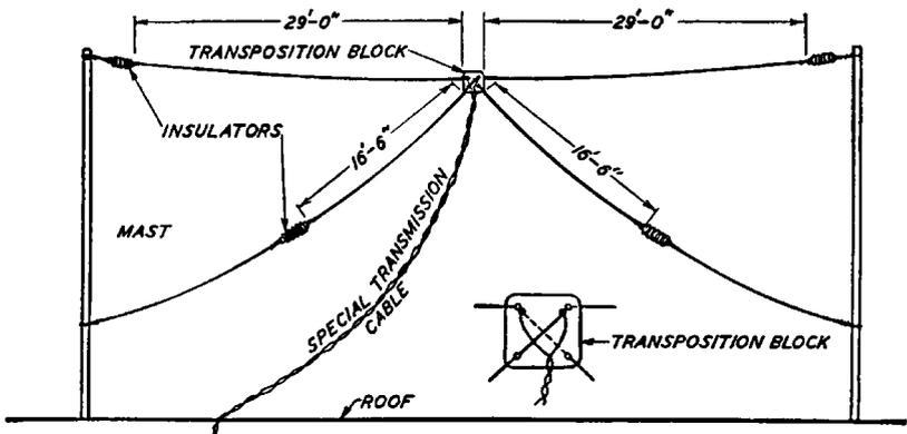
Fig. 103A. The Double-Doublet Type of Antenna
