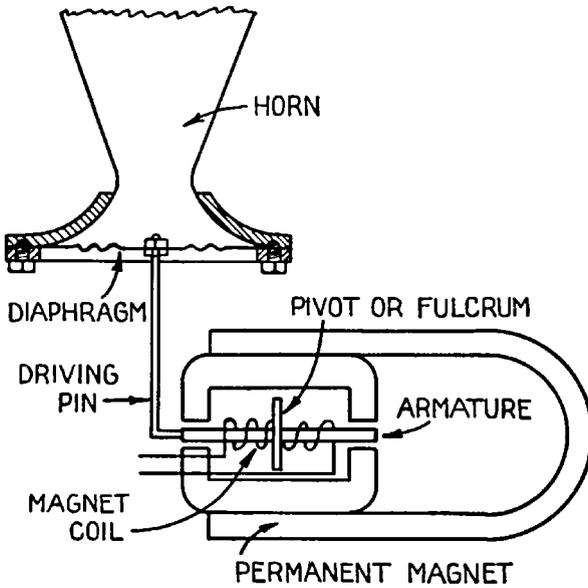
Fig. 96. The Balanced Armature Type of Speaker
