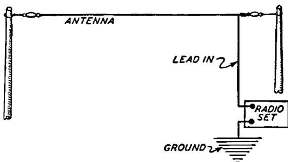
Fig. 100. A Simple Antenna System
