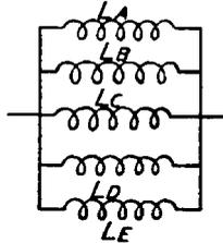
Fig. 41. Inductance Coils Connected in Parallel
