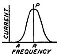
Fig. 69. Curve Showing Increase of Current as Resonant Frequency Is Increased
