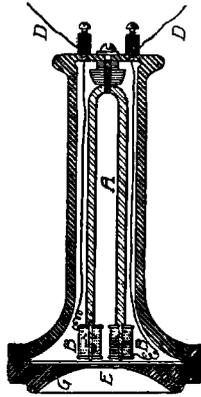
Fig. 95. A Telephone Receiver
