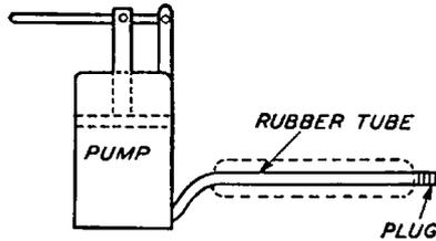
Fig. 19. Diagram Illustrating Effect of Applying Pressure to a Soft Rubber Tube
