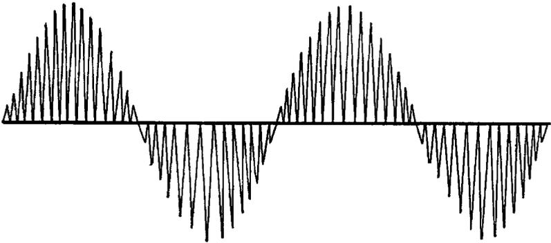
Fig. 93. The Result of Combining a 1000 Kilo Cycle and 500 Cycle Wave
