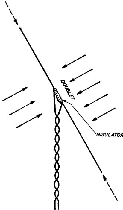
Fig. 103. Solid Arrows Indicate Plane of Maximum Doublet Pick-up, while Dotted Arrows Show Plane of Minimum Pick-up. Proper Orientation May Be Used to Reduce the Pick-up of Noise Interference
