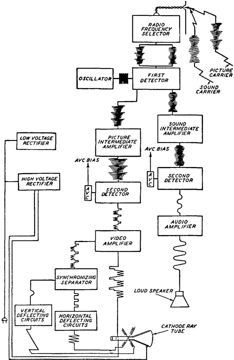
loud speaker. Some television receivers are designed with the audio section as a conventional all-wave receiver, tuned to an intermediate frequency, the television receiver serving as an ultra-high frequency converter.
