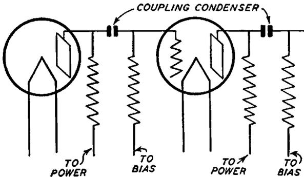
Fig. 85. A Resistance Coupled Amplifier
