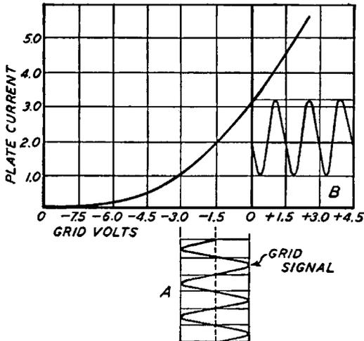
Fig. 54. Graph Showing Characteristic Curve of a Vacuum Tube
