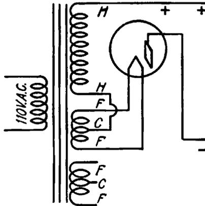
Fig. 56. Transformer Connections to Half-Wave Rectifier Tube
