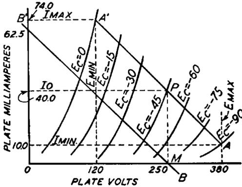
Fig. 83. A Group of Plate-Voltage Plate-Current Curves Obtained with Different Grid-Bias Voltages
