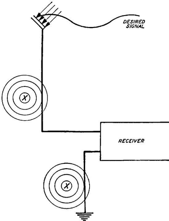
Fig. 103B. Electrical Disturbances at Points Marked "X" Enter the Receiver with the Desired Signal and Issue from the Speaker as Annoying Interference
