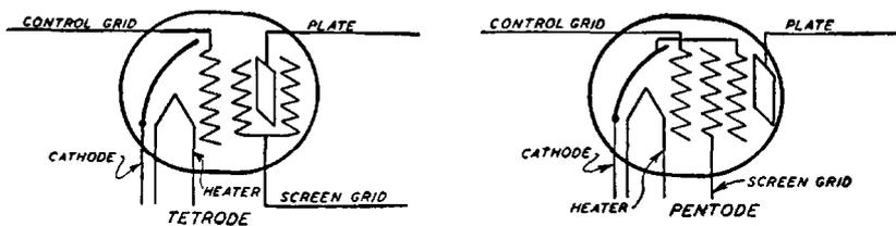
Fig. 61. Diagram Showing the Elements in a Tetrode and Pentode Tube
