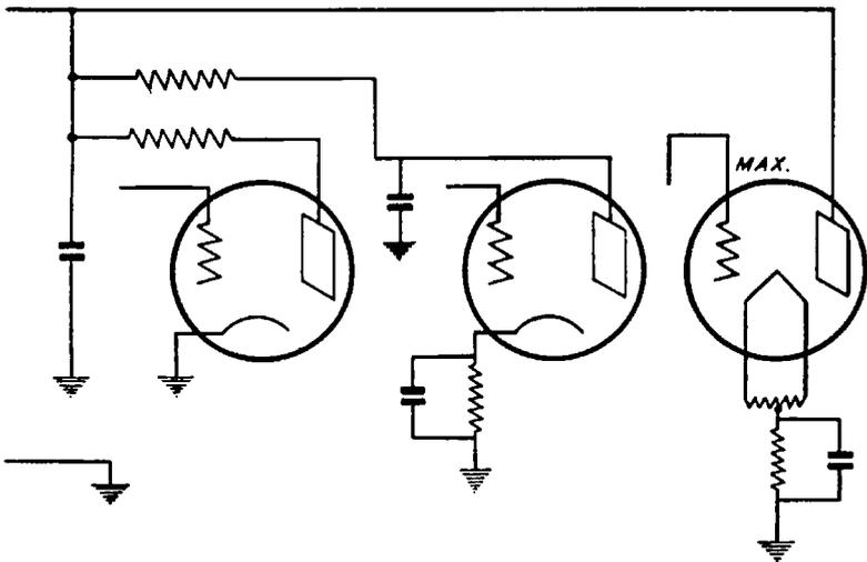
Fig. 106. A Voltage Divider Using Individual Resistance Units
