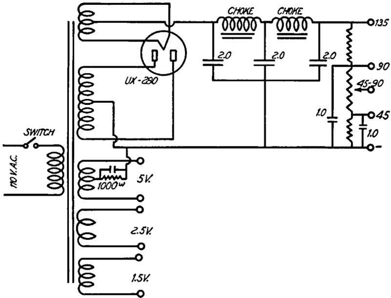
Fig. 104. Arrangement of Choke Coils, Condensers, and Resistances in a Power Supply Unit
