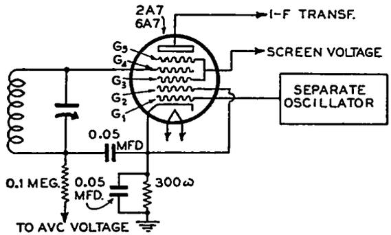
and  $G_2$  is reduced to a small value, and the frequency of oscillation cannot change materially because it is determined by a separate tube in which the grid  $G_1$  of the converter tube plays a small part.  $G_1$ , therefore, is nothing but a means of coupling the oscillator voltage to the mixer tube (first detector).
