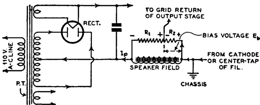
FIG. 20-10.—This output stage grid-bias arrangement is the same as that shown in Fig. 20-9, with the exception that resistors  $R_1$ — $R_2$  serve to proportion the voltage drop across the speaker field winding so that the output tubes get the proper *C* bias voltage. No tap is required on the speaker field.
