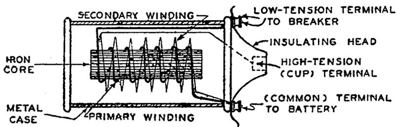
FIG. 27-30.—Interior of a typical automobile ignition coil. Several external connection arrangements which are employed are shown in Fig. 27-31 to 27-35 inclusive.
