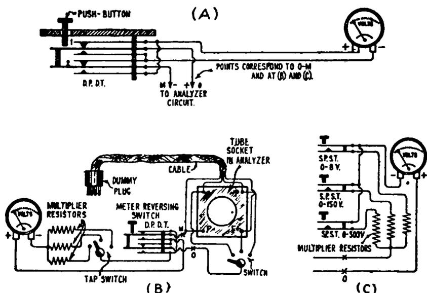
FIG. 11-18.—Progressive study of the voltage-current analyzer and the switching arrangements.
