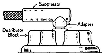
each end. The high tension lead is cut near the distributor cover and the suppressor is screwed firmly into the wires of the two cut ends as shown. There are several cars which require an "elbow" type suppressor in the distributor lead. The method of installing a suppressor of this type is illustrated in Fig. 27-53. In those cars which employ two ignition coils (see Figs. 27-34
