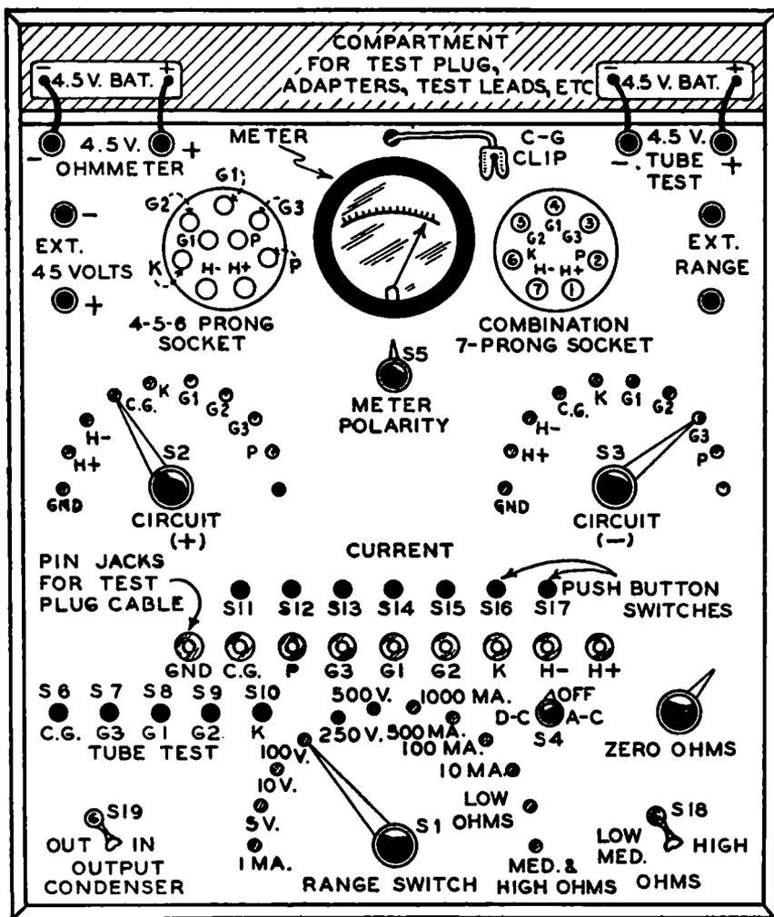
FIG. 13-3.—A suggested panel layout for the analyzer of Fig. 13-1. The labeling of the various parts shown here corresponds to that in Fig. 13-1. The compartment at the top contains the two 4½-volt dry cell batteries and also serves as storage space for the test plug and cable, adapters, etc.
