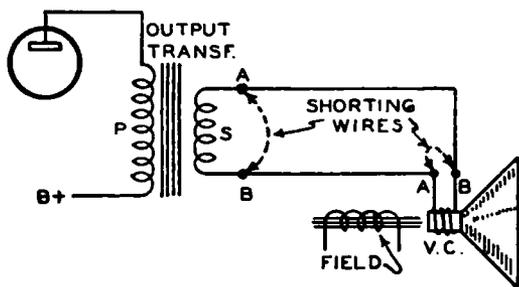
FIG. 23-14. — How the output transformer secondary, or voice coil, should be shorted across points A-B to test for hum in the loud speaker.
