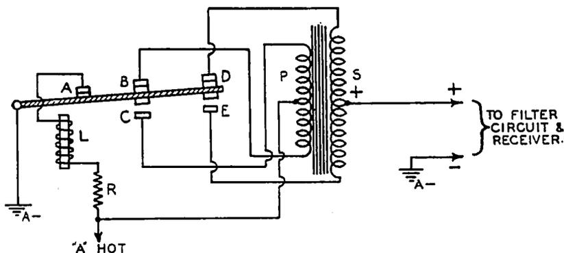
FIG. 27-63.—A “synchronous” auto-radio vibrator circuit arrangement in which full-wave rectification is accomplished by the use of synchronous contacts *D* and *E*. No rectifier tube is necessary in this system.
