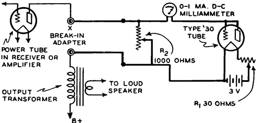
FIG. 7-17.—A tube rectifier type output meter connected into the plate circuit of one of the output tubes of a receiver or amplifier by means of a break-in adapter.
