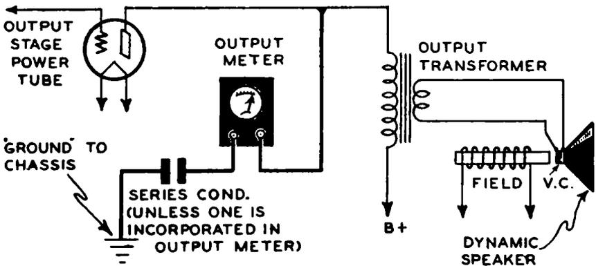
FIG. 7-8.—How an output meter may be connected to a receiver which employs a single-tube power output stage and a dynamic loud speaker.
