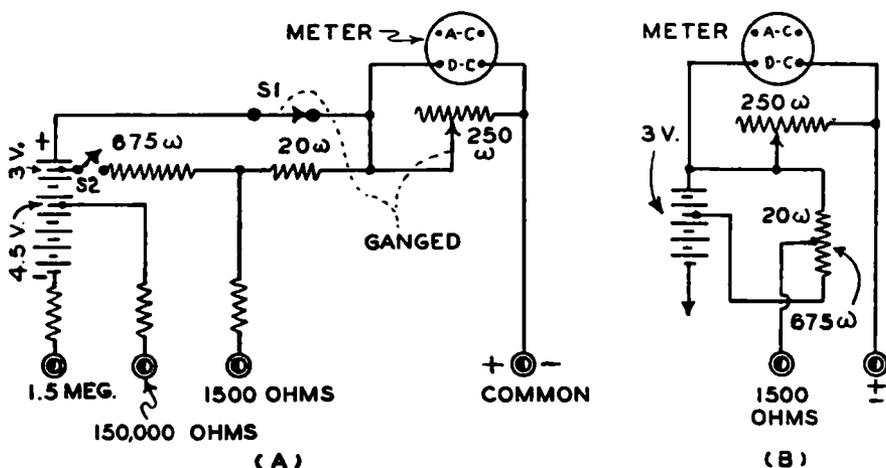
FIG. 5-21.—A “breakdown” circuit diagram of the ohmmeter portion of the tester shown in Fig. 5-20.
