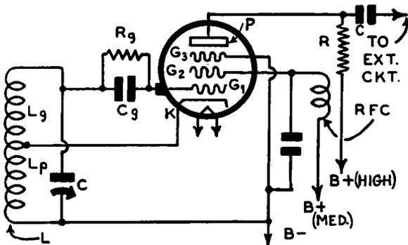
FIG. 15-21.—A typical electron-coupled oscillator circuit. A Hartley oscillator arrangement is used. The oscillator is electron-coupled to the plate, *P*, and the *external circuit* via the electron stream in the tube.
