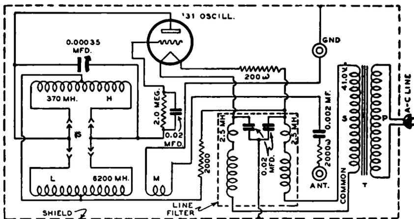
FIG. 17-16.—Schematic circuit diagram of the test oscillator illustrated in Fig. 17-15. A single tube is employed, and its output is modulated by the a-c line. A fundamental frequency range of 95 kc to 220 kc, and from 1.5 to 3.3 mc is provided.
