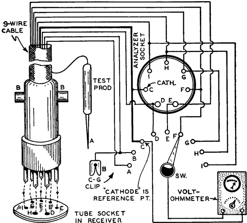
FIG. 12-7.—Circuit arrangement of a point-to-point analyzer capable of checking both resistance and voltage. Here the analyzer is provided with a tube socket in which the tube removed from the receiver socket under test is inserted. The switch enables the volt-ohmmeter to be connected between the "cathode" (which is the reference point) and any other terminal of the tube socket.
