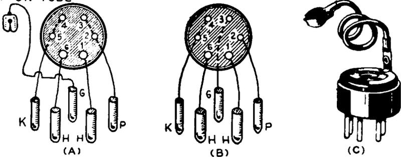
FIG. 8-19.—(A) Wiring of an adapter for testing the 57, 58, 77, 78, 6C6, 6D6, etc. tubes in the '27 or '37 sockets of tube checkers. (B) Adapter for testing the 57, 58, 6C6, 6D6, etc., in the '24 or '36 sockets. (C) A commercial adapter of this type. Notice the flexible lead and clip for connecting to the control-grid cap on the tube.
