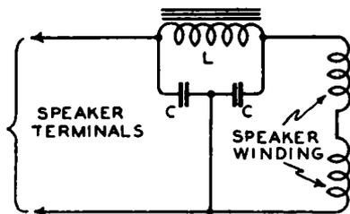
FIG. 23-34.—A typical filter for a magnetic speaker. This prevents fringe howl.
