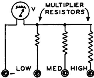
FIG. 2-21.—A d-c voltmeter employing individual multiplier resistors and individual terminals for each range. This arrangement is used in the voltmeter illustrated in Fig. 2-18 (Left).
