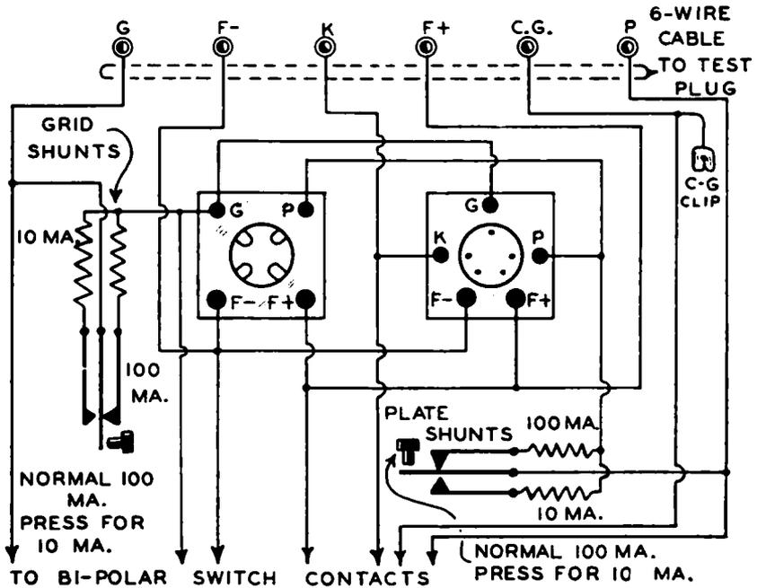
FIG. 11-20.—A double-shunt switching system which makes use of two S.P.D.T. switches for providing two current ranges for grid current and screen current measurement.
