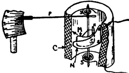
FIG. 2-29.—The movable-iron type movement used in some a-c instruments. The repulsion between the magnetized iron vanes *M* and *N* causes the pointer to move over the scale. A portion of the coil *C* has been cut away in this view to show the interior arrangement of the parts.
