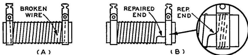
FIG. 26-1.—Method of repairing a wire-wound fixed resistor in which the resistance wire has broken near one of the end terminal clamps.
