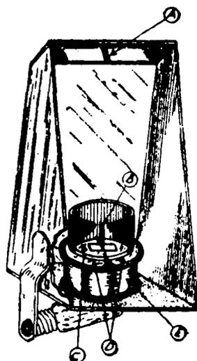
FIG. 19-26. — Construction of the Shadowgraph tuning indicator. A detailed view of the permanent magnet *D*, iron disc *C* and deflecting "shadow"-vane *B*, is shown at the left. The entire unit assembled in its box, is shown at the right. The pilot lamp is at the bottom.
