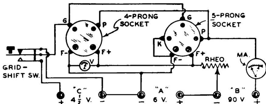
FIG. 8-11.—Here, a 5-prong socket has been added to the tester of Fig. 8-10. This makes it possible to test both 3- and 4-electrode tubes.
