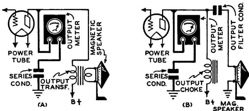
FIG. 7-12.—(A). How an output meter should be connected in a receiver having a single output tube feeding into a magnetic speaker through an output transformer.
