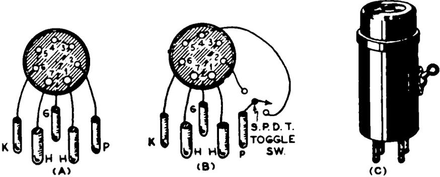
FIG. 8-20.—(A) Wiring of an adapter suitable for testing the 2A7, 6A7, 6D7, 6E7, etc., tubes in a '24 or '36 socket of a tube checker. (B) Wiring of an adapter for testing the 2B7 and 6B7 tubes in a '24 or '36 socket. (C) A typical commercial adapter of this general type. Notice the toggle switch at the side.
