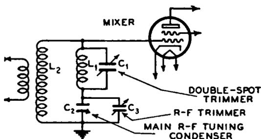
**FIG. 25-11.**—Double-spot tuning circuit which has been used in Atwater Kent receivers for the prevention of image-frequency interference and double-spot tuning. The main tuning circuit and the double-spot circuit are tuned simultaneously to two different frequencies.
