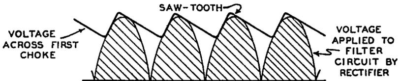
FIG. 25-39.—How a saw-tooth voltage may be obtained from the output of a full-wave rectifier-filter system.
