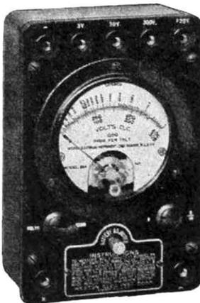
FIG. 5-13.—A volt-ohmmeter which provides two resistance ranges and four d-c voltage ranges at 1,000 ohms-per-volt. All voltage ranges are brought out at the upper pin jacks. The schematic circuit diagram is shown in Fig. 5-14. (Weston Model 564.)
