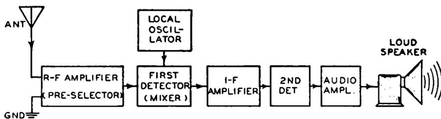
FIG. 25-1.—Block diagram showing the main parts and their sequence in a typical superheterodyne receiver.
