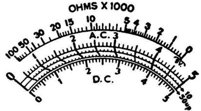
reading by scale factor); 25-50,000-500,000-5,000,000 ohms resistance (multiply reading by scale factor). The schematic circuit of the instrument is shown in Fig. 2-48.
