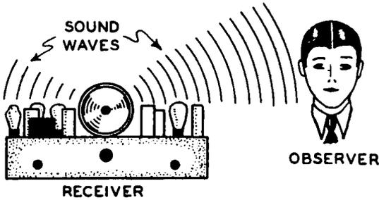
FIG. 7-1.—The "ear" method of judging the intensity of the output of a radio receiver or amplifier. This is an inaccurate method, for the human ear is relatively insensitive to small changes in the loudness of a sound.
