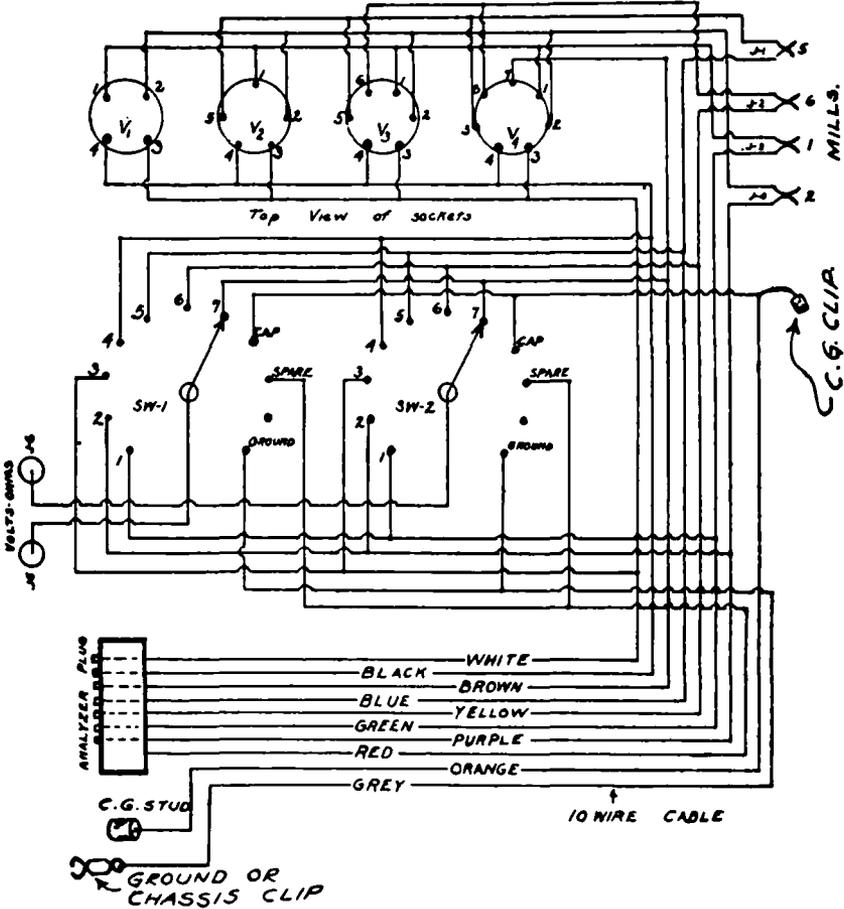
FIG. 14-2.—Schematic circuit diagram of the analyzer-adapter unit illustrated in Fig. 14-1.
