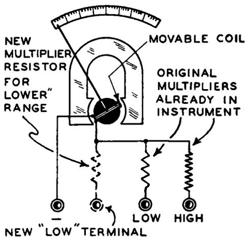
voltmeter by connecting suitable multiplier resistors to it (see Figs. 2-19, 20, 21, 22). Of course, a meter having a full-scale reading of 1 milliampere or less, is preferable to start with, for then it will make a high-resistance voltmeter (see Arts. 2-19 and 2-20).
