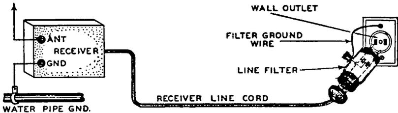
FIG. 30-21.—Correct method of connecting a line filter unit directly at the power line outlet so that no interference will enter the receiver line cord and be radiated to the receiver wiring or antenna system from it. The “ground” terminal of the filter unit should be grounded to the conduit of the line—not to the receiver ground. It is preferable to locate the filter unit at the main service switch of the building if it is possible (see text).
