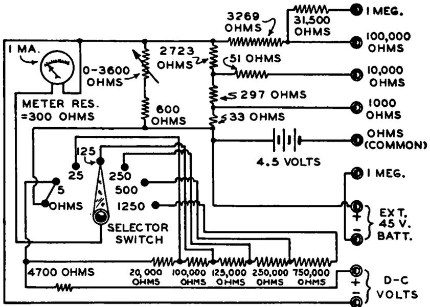
FIG. 5-11.—Schematic circuit diagram of the volt-ohmmeter shown in Fig. 5-10. The ohmmeter section has been redrawn separately in Fig. 5-12.
