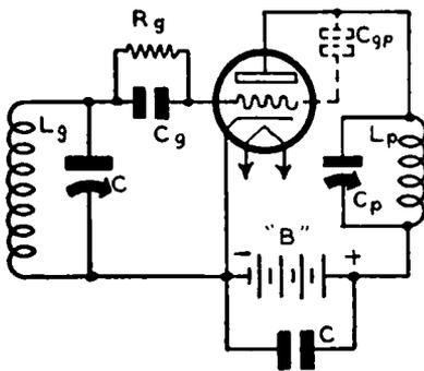
FIG. 15-9.—Tuned grid—tuned plate oscillator circuit.
