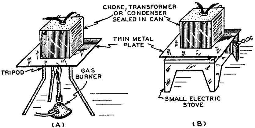
FIG. 26-4.—Two convenient methods of heating the compound in a sealed choke, transformer, or condenser unit so that it may be melted out. At (A) a gas burner is used; at (B) an electric "hot plate" or stove is employed.
