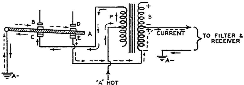
FIG. 27-65.—Simplified diagram showing the circuit conditions when the vibrator reed is “down”.
