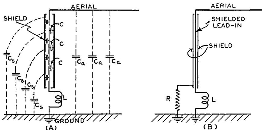
FIG. 30-28.—(A) The various capacitances which exist between the aerial, ground, lead-in and shield in a shielded lead-in antenna system. (B) How the lower end of the shield may be connected to ground through a resistance (or choke) to reduce local oscillations of noise current in the shield circuit.
