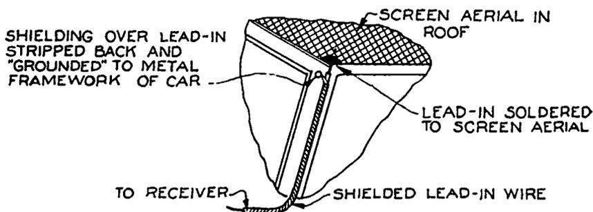
FIG. 27-16.—How the shielded lead-in may be connected to the aerial and run down the side of a front post of the car.
