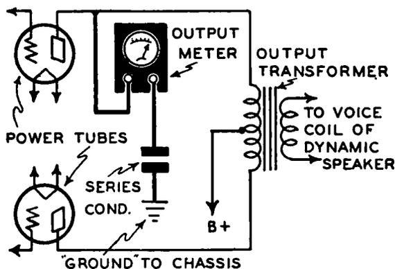
FIG. 7-10.—Preferable way of connecting an output meter when the receiver employs a push-pull output stage.
