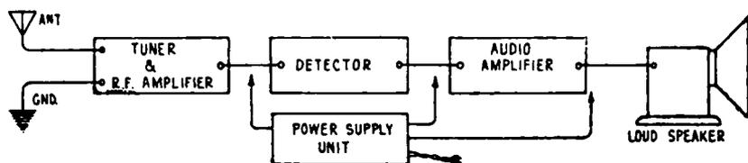
FIG. 18-4.—The main units of a t-r-f receiver shown in proper sequence, from left to right, as the radio signal passes through them.
