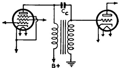
phones, phonograph pickups or talking motion picture equipment, a number of commercial radio receivers also employ this system of amplification because of its high gain and wide audio-frequency response.
