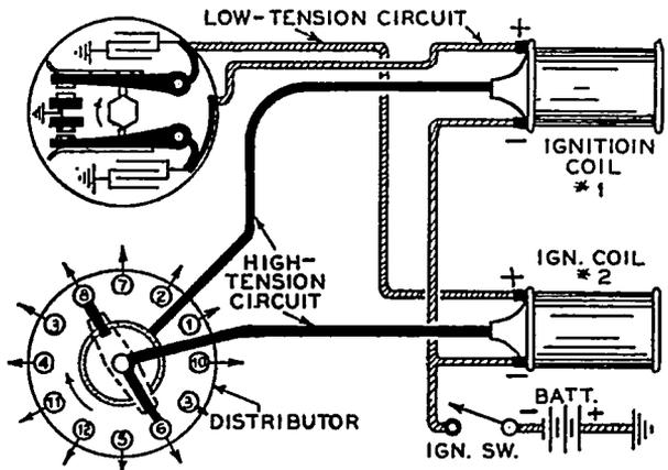
cylinders in the engine. The arrangement shown here is that for a 12-cylinder engine.
