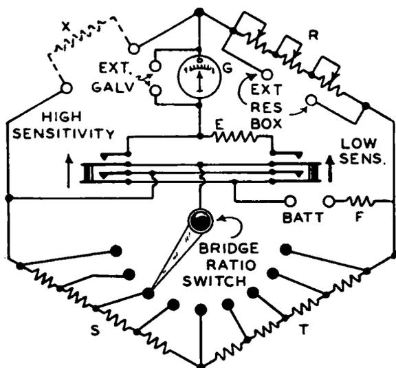
FIG. 3-6. — Schematic circuit diagram of the typical commercial form of Wheatstone bridge shown in Fig. 3-7.
