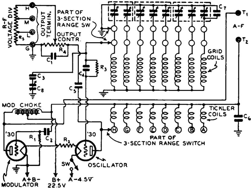
FIG. 17-2.—Schematic circuit diagram of the all-wave test oscillator illustrated in Fig. 17-1. A separate oscillator and modulator tube are used, and a 3-section range switch is employed with 8 grid and tickler coils to cover the entire frequency range from 90 kc to 25 mc. Only fundamental frequencies of the oscillator are employed.
