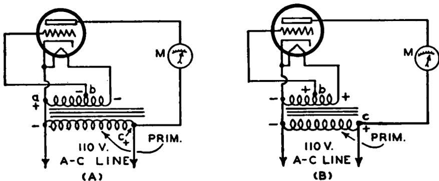
FIG. 8-8.—(A) Incorrect transformer connections for grid shift test method of Fig. 8-7. The instantaneous polarities of the grid and plate are opposite, so they oppose each other's action on the plate current.
