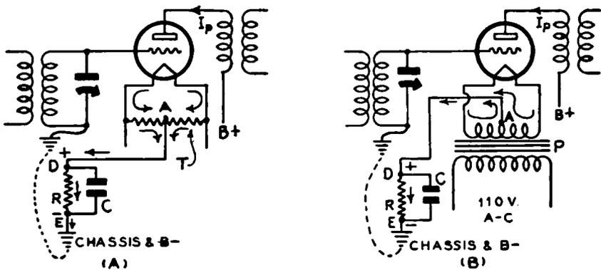
FIG. 20-5.—(A) A circuit arrangement used for obtaining *C* bias voltage in many old electric receivers. The plate current of the tube is made to flow through a *C* bias resistor *R*. The voltage drop produced in this resistor is utilized as the negative *C* bias voltage.
