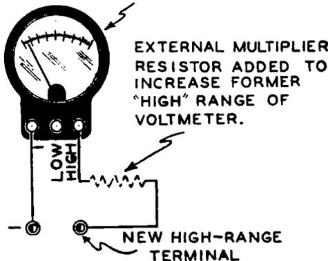
FIG. 2-23.—A suitable external multiplier resistance may be connected to the "HIGH" range terminal of a voltmeter in order to increase its range.
