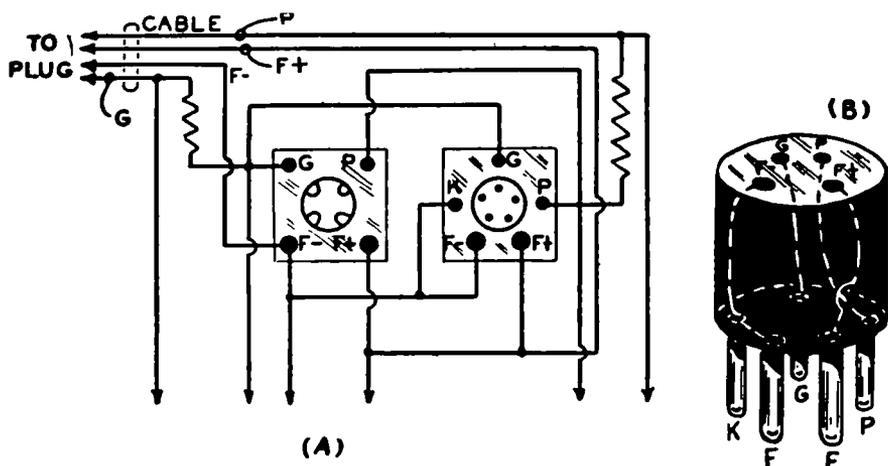
FIG. 11-17.—(A) How a 5-prong socket is added to our analyzer to make it possible to analyze the circuits leading to 5-prong tubes in receivers.
