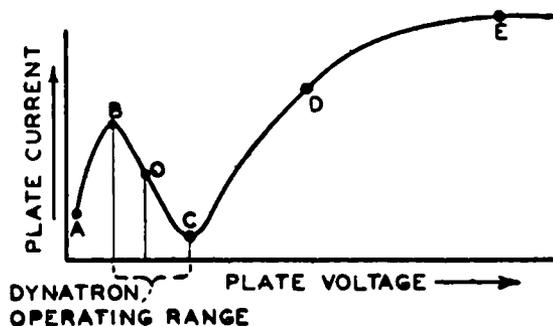
FIG. 15-14.—Fundamental dynatron characteristic of a screen grid tube. Over region B-C an increase in plate voltage results in a decrease in plate current i.e., the tube exhibits a *negative resistance* characteristic.
