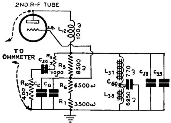
FIG. 21-13.—Equivalent simplified circuit diagram of the plate-to-ground and the screen-grid-to-ground circuits in the second r-f stage of the all-wave receiver whose circuit diagram is shown in Fig. 21-12.
