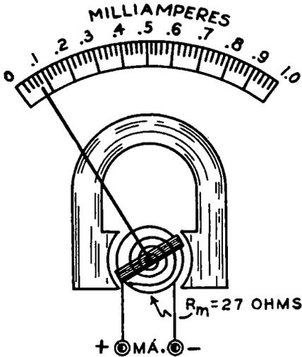
FIG. 2-15.—The internal arrangement of our 1-ma. range milliammeter before converting it into the voltmeter of Fig. 2-16. The resistance  $R_m$  of the movable coil, is 27 ohms. The scale is calibrated to read “milliamperes”—up to 1 ma.
