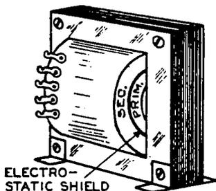
FIG. 30-22.—How the electrostatic shield is placed between the primary and secondary windings of a power transformer.
