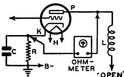
FIG. 12-2.—Checking the resistance between the plate and cathode in a simple radio circuit by means of an ohmmeter.
