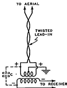
FIG. 30-38.—How noise voltage appearing across the primary of the receiver impedance-matching transformer may induce noise voltage in the secondary winding if appreciable capacity,  $C$ , exists between them.
