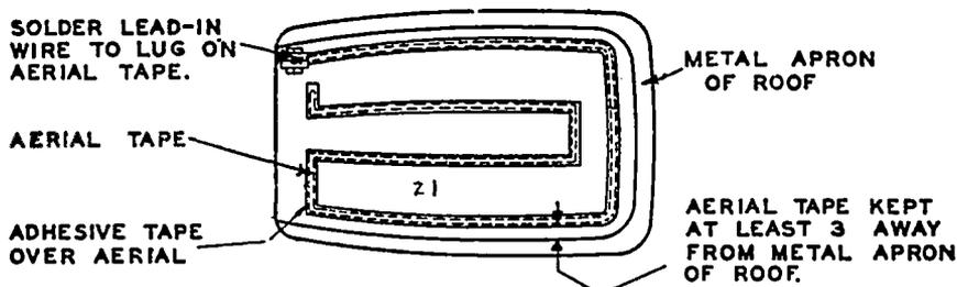
FIG. 27-21.—Method of laying the tape aerial on the roof of the car. The lead-in is brought up through a small hole in the roof, as shown in Fig. 27-20. The hole should be filled and sealed with ordinary plastic roofing cement to prevent water leakage.
