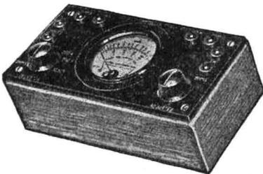
FIG. 5-10.—A volt-ohmmeter which provides for a wide range of voltage and resistance measurements. Its circuit diagram is shown in Fig. 5-11. (Supreme Model 111.)
