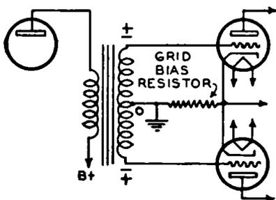
FIG. 23-20.—Input circuit of a transformer-coupled push-pull amplifier.
