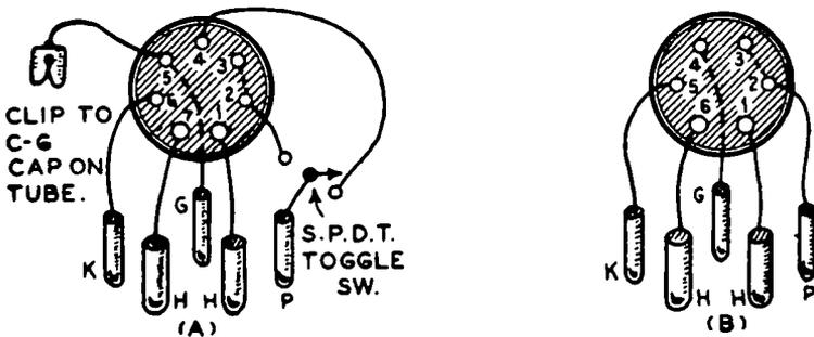
FIG. 8-25.—(A) Wiring of an adapter for testing the 6F7 tube in the '37 socket of a tube checker. (B) Adapter for testing the 41 and 42 tubes in the '37 socket.
