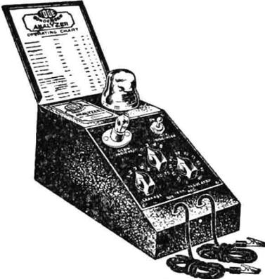
FIG. 6-2. — The relaxation oscillator type condenser analyzer whose circuit diagram is shown in Fig. 6-1.
