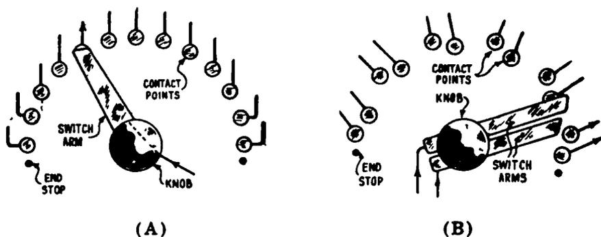
FIG. 11-9.—(A) A single-arm tap switch with 13 contact points.
