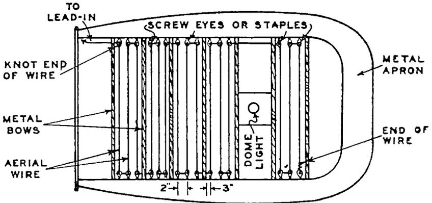
FIG. 27-19.—A "strung" wire aerial suitable for use in closed cars having all-metal bows in their tops. The insulated wire is strung back and forth across the top of the car through screw eyes or insulated staples fastened to the wooden top frame.
