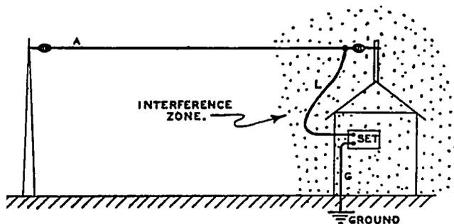
“ground” should be given some attention when noisy reception is experienced. In rural districts, perhaps the best ground is one that is buried outside the house where it is definitely away from all electric light wiring. Obviously, nothing will be gained by sinking a ground close to the point of exit of the electric light circuit, or even the water and gas pipes. A position at least 6
