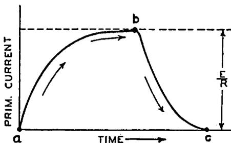
FIG. 27-44. — How the primary current of the ignition coil increases ( $a$  to  $b$ ) when the breaker points close (at  $a$ ), and falls ( $b$  to  $c$ ) when they open (at  $c$ ).
