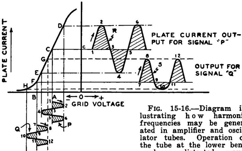
FIG. 15-16.—Diagram illustrating how harmonic frequencies may be generated in amplifier and oscillator tubes. Operation of the tube at the lower bend produces distorted waveform S which represents a condition where harmonic frequencies are present.
