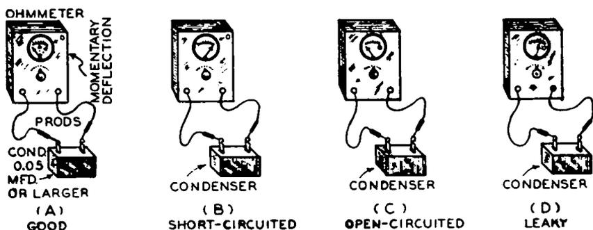
FIG. 22-12.—Sketches showing the four possible pointer indications of an ohmmeter when it is used for testing a condenser having a capacity larger than about 0.05 mfd.
