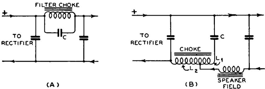
FIG. 23-13.—Two filter choke arrangements employed in the  $B$  supply portions of a-c electric receivers. That at (A) uses a condenser  $C$  to tune the choke. That at (B) uses a tapped choke. Causes of hum in these circuits are discussed in the text.
