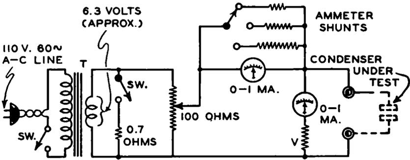
FIG. 6-6.—Schematic circuit diagram of a capacity meter designed especially to measure the capacity of electrolytic condensers. The design of this meter is such that it may be constructed easily by radio service men.
