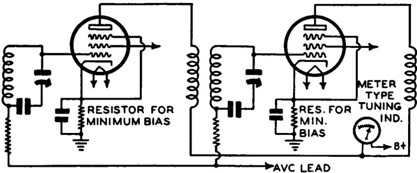
FIG. 19-25.—How a “meter” type tuning indicator is connected in the plate circuits of the avc-controlled tubes in a receiver.
