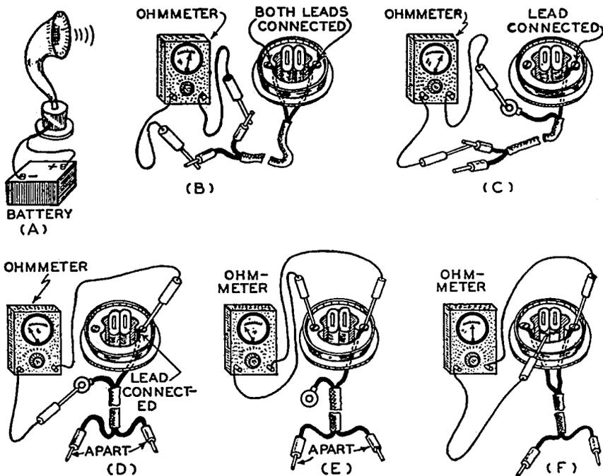
FIG. 26-8.—Various electrical tests which should be made on a magnetic loud speaker of either the *iron-diaphragm* or *balanced armature* type in order to locate electrical trouble in either the speaker cord or the coils. These tests are described in detail in the accompanying text.
