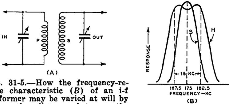
FIG. 31-5.—How the frequency-response characteristic (B) of an i-f transformer may be varied at will by varying the distance between the primary and secondary windings shown at (A). Two extremes of coupling desirable in an i-f transformer suitable for use in a high-fidelity receiver are shown at (B). The tuning characteristic labeled *S* provides high selectivity but poor high-note reproduction; that labeled *H* provides less adjacent channel selectivity but better audio fidelity.
