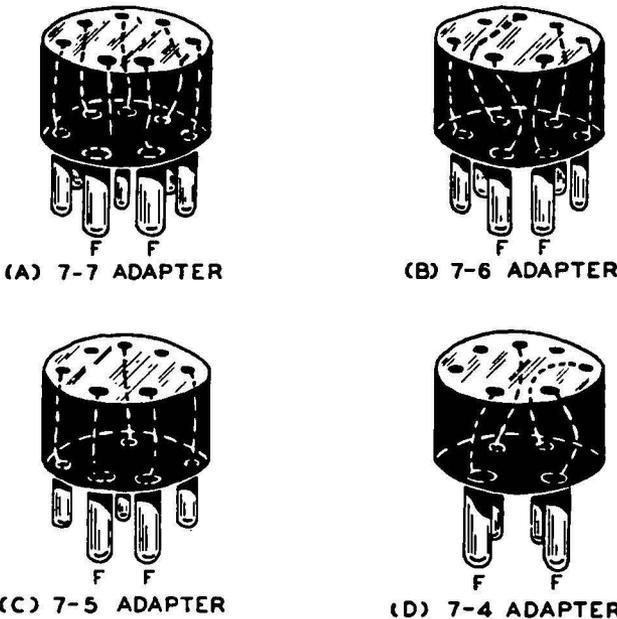
FIG. 11-24.—Internal wiring of the four analyzer adapters illustrated in Fig. 11-23.
