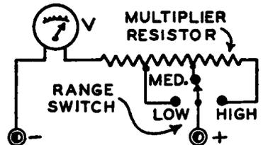
FIG. 2-20.—A d-c voltmeter employing a tapped multiplier resistor and a range-switch for switching from one range to another quickly.
