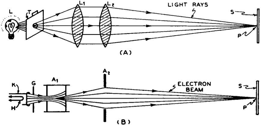
FIG. 25-17.—(A) How light rays may be focussed to a small point by means of glass lenses.
