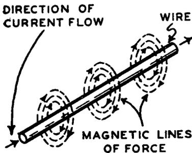
FIG. 2-1.—The magnetic field around the straight current-carrying wire is circular in shape and is represented by the dotted circles. These are called “magnetic whirls”. The arrows show their direction.
