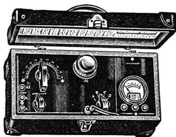
FIG. 17-13.—Exterior view of the battery operated test oscillator whose circuit diagram is shown in Fig. 17-14. The oscillator is shown here in its carrying case, with an output meter at the right. (Model 553)
