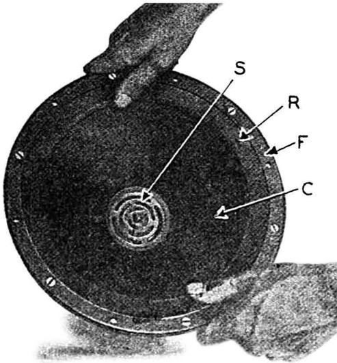
**FIG. 26-19.**—Correct method of holding the speaker frame and cone to determine if the voice coil scrapes against the pole pieces. The cone is gently moved straight in and out with the thumbs of both hands. If a dull scraping sound is heard when this is done, it indicates that the voice coil is not properly centered and is rubbing against the metal pole piece. The main parts of the cone assembly are labeled.
