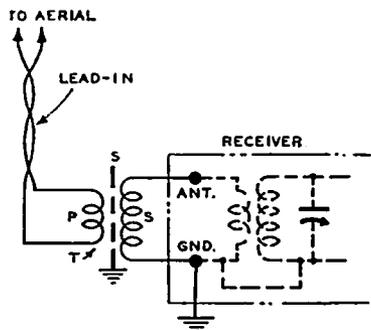
FIG. 30-42.—How the twisted-wire (or transposed-wire) lead-in is connected to the type of receiver input shown at (A) of Fig. 30-41 when an impedance-matching transformer, *T*, is to be used between the lead-in and the radio receiver.
