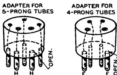
FIG. 24-10.—A neutralizing adapter for 5-prong tubes (*left*) and one for 4-prong tubes (*right*). In each, one leg of the filament circuit is left *open*.
