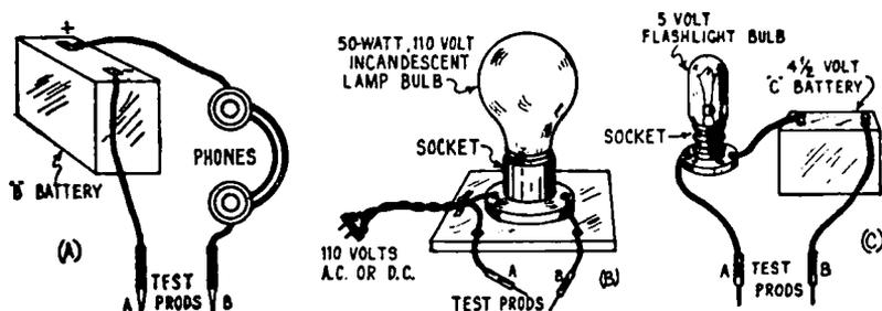
FIG. 22-2.—Three simple continuity testers which may be used when an ohmmeter is not available.
