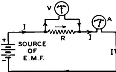
FIG. 3-1.—Preferable circuit arrangement for measuring “low” resistances by the ammeter-voltmeter method. (See also, Fig. 3-2.)
