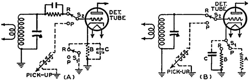
FIG. 26-22.—(A) Method of connecting a phonograph pickup to the detector input circuit of a receiver employing grid-leak detection. (B) Method of connection when the receiver employs grid-bias detection. In each case, the additional pickup and other wiring is shown dotted.
