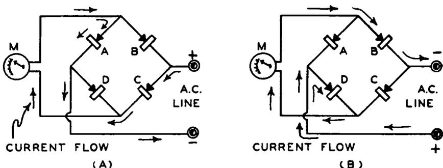
FIG. 2-35.—How a full-wave rectifier operates.
