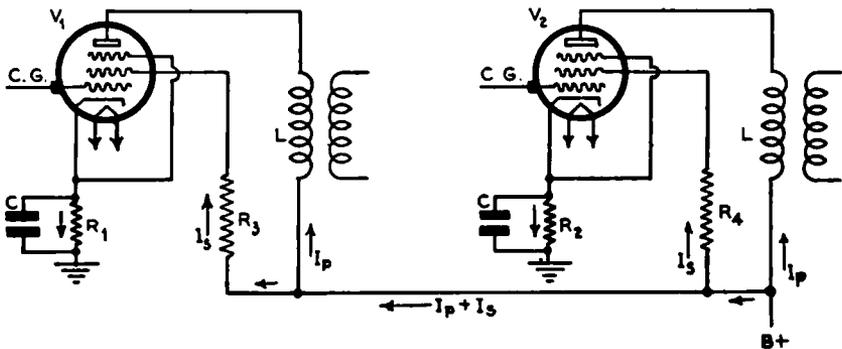
FIG. 20-17.—Typical amplifier stages of the type having individual series-connected voltage-dropping resistors in the screen circuits.
