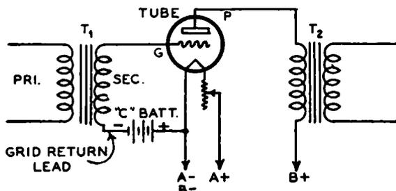
FIG. 20-3.—In most battery-operated receivers, the *C* bias voltages for the amplifier tubes are supplied by one or more dry-cell *C* batteries connected in the grid-return circuit as shown here.
