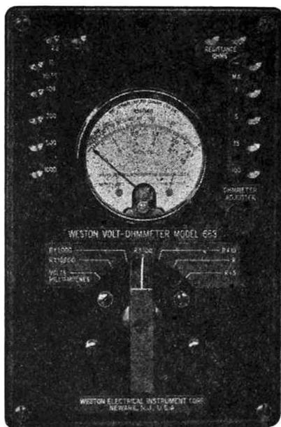
FIG. 5-15. — A volt-ohm-milliammeter which provides four current ranges, six voltage ranges, and six resistance ranges. All ranges are selected by the selector switch at the bottom. Its schematic circuit diagram is shown in Fig. 5-17. A facsimile reproduction of its scale is shown in Fig. 5-16.
