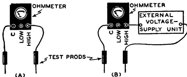
FIG. 4-4.—The high-resistance range of a series-type ohmmeter (A), may be increased by connecting a suitable external voltage source (including the proper resistor) to it as shown at (B).
