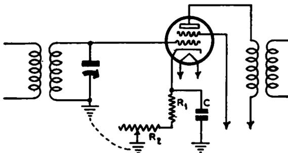
FIG. 20-8. — Grid bias voltage is obtained here by the combination of a fixed and a variable resistor in the cathode circuit. The variable resistor is used for the purpose of varying the bias voltage in order to control the volume.
