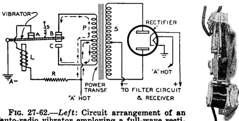
**FIG. 27-62.**—*Left:* Circuit arrangement of an auto-radio vibrator employing a full-wave rectifier tube.
