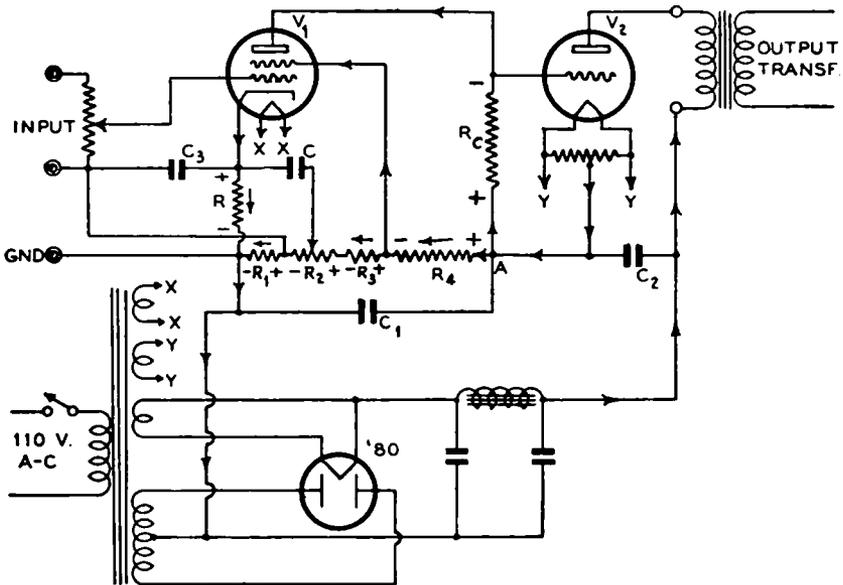
FIG. 23-24.—A typical direct-coupled a-f amplifier. Resistor  $R_o$  couples the two tubes together.
