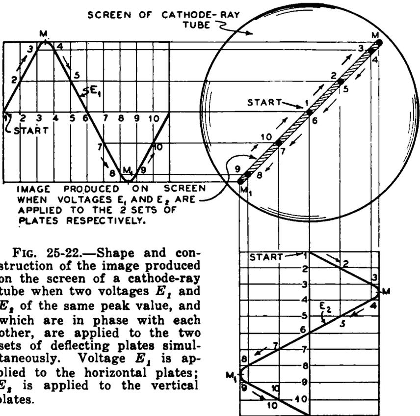
IMAGE PRODUCED ON SCREEN WHEN VOLTAGES  $E_1$  AND  $E_2$  ARE APPLIED TO THE 2 SETS OF PLATES RESPECTIVELY.
