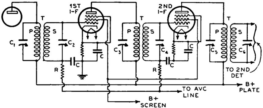
FIG. 25-6.—A typical i-f amplifier for a very sensitive superheterodyne receiver. Two stages of i-f amplification are used. Each i-f transformer winding is tuned by an adjustable tuning condenser  $C_1$ ,  $C_2$ , etc. Most "midget" superheterodyne receivers employ only one such stage.
