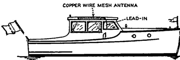
able shielding of wires is necessary in some boats, especially in short ones. In some cases, the entire engine compartment must be completely shielded internally with grounded *sheet* copper or brass in order to reduce the interference to a permissible level. All connections should be well soldered, and all wires should be fastened securely, for considerable vibration and "weaving" exists in these craft.
