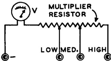
FIG. 2-19.—A d-c voltmeter employing a tapped multiplier resistor, and individual terminals for each range.
