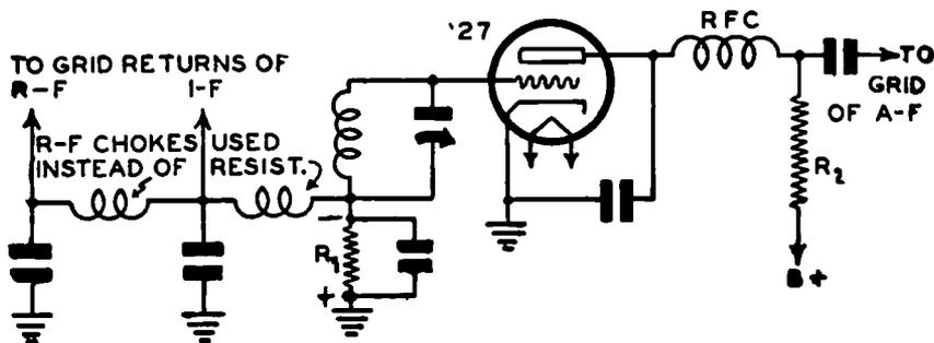
FIG. 19-6.—An avc system in which a single triode is used as both a detector and avc tube. The avc voltage developed across resistor  $R_1$  controls the grid bias on the r-f and i-f tubes.
