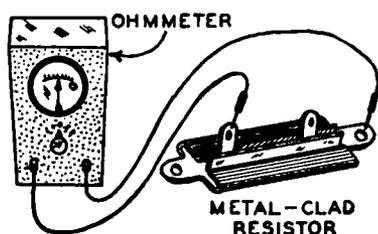
FIG. 22-3.—How a metal-clad resistor should be tested for possible grounds between the resistor element and the metal shield. The test is made between the shield mounting lug and one terminal of the resistor.
