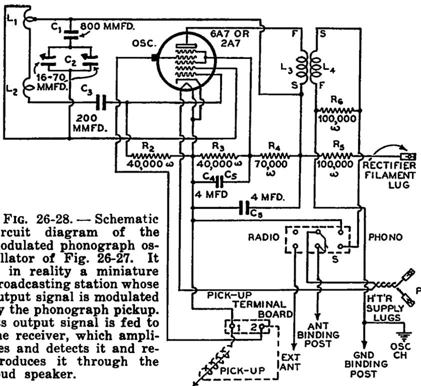
FIG. 26-28. — Schematic circuit diagram of the modulated phonograph oscillator of Fig. 26-27. It is in reality a miniature broadcasting station whose output signal is modulated by the phonograph pickup. Its output signal is fed to the receiver, which amplifies and detects it and reproduces it through the loud speaker.
