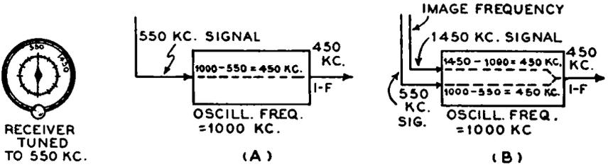
FIG. 23-8.—The receiver is tuned to 550 kc for the reception of a 550-kc station. At (A) the signal of this 550-kc station beats with the 1,000-kc set-oscillator frequency to produce an i-f of 450 kc. At (B) is shown how an “image-frequency” signal of 1,450 kc can also beat with the 1,000-kc oscillator frequency to produce an i-f of 450 kc which will interfere with the first (desired) signal. This is a typical example of “image-frequency” interference.
