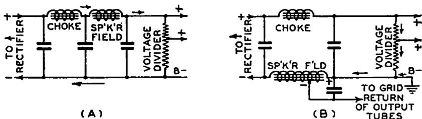
FIG. 26-17.—Two circuit arrangements which are employed in radio receivers for energizing the dynamic speaker field with current from the *B* power supply unit. At (A) the speaker field acts simply as a choke; at (B) the speaker field is tapped so that it not only acts as a choke but also supplies the negative grid bias for the output stage of the receiver.
