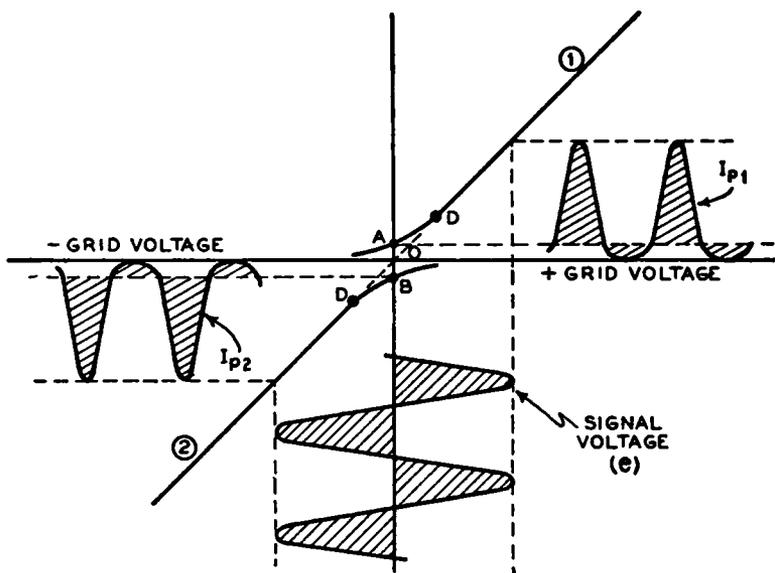
FIG. 23-26.—Graphs illustrating the wave form of the plate current existing in each tube of a push-pull Class B amplifier stage when a signal voltage  $e$  having the wave form shown is applied to the stage. The graphs are plotted with plate current as ordinates (vertical scale) and grid voltage as abscissae (horizontal scale).
