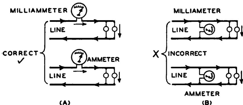
FIG. 2-9.—(A): Correct way to connect (in series) a milliammeter, or an ammeter, in a circuit to measure the current. The total current to be measured should flow *through* the meter and its shunt. (B): Incorrect way to connect a milliammeter or ammeter.
