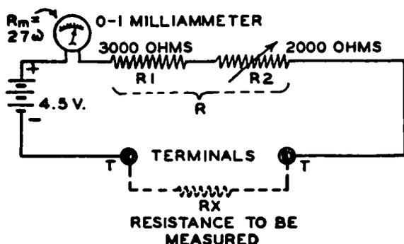
FIG. 4-1.—Circuit diagram of a simple series-type ohmmeter whose design and construction are considered here. A reduced facsimile reproduction of the scale for this meter is shown in Fig. 4-2.
