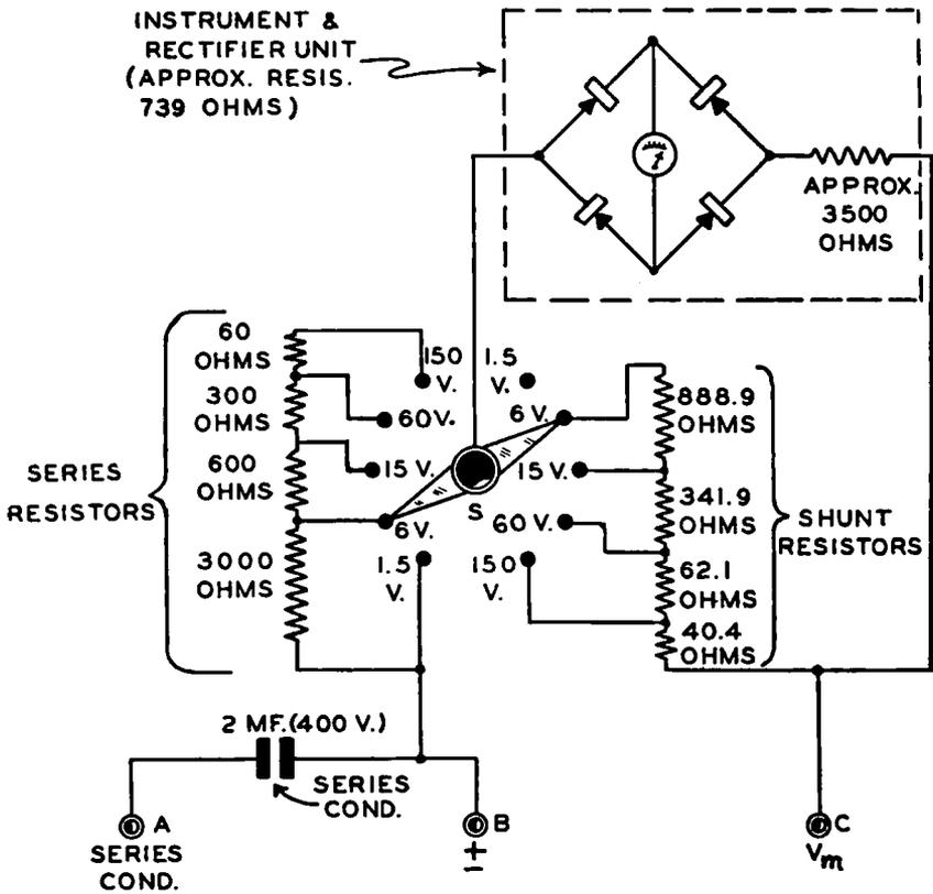
FIG. 7-4.—The schematic circuit diagram of the output meter illustrated in Fig. 7-3. Five voltage ranges may be selected by the knob which controls the selector switch *S*. The impedance remains constant at 4,000 ohms.
