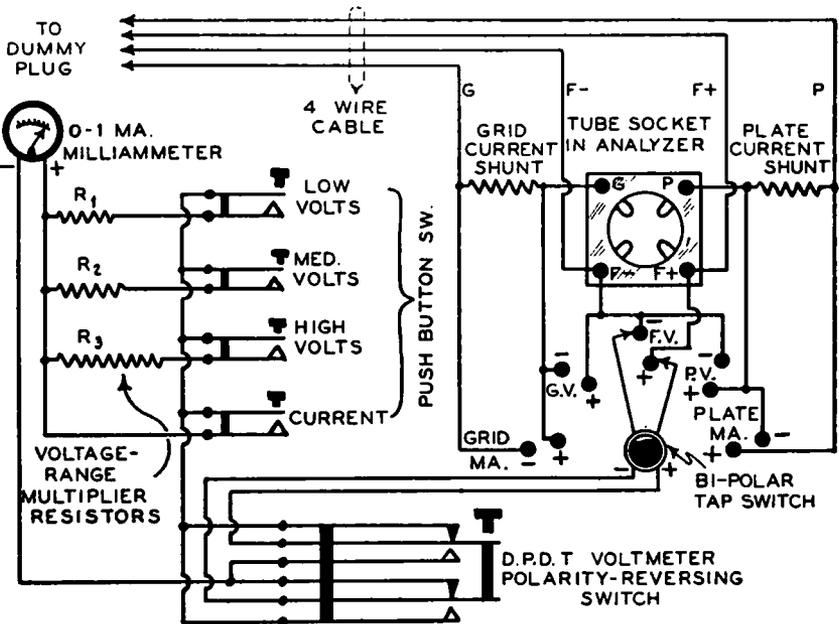
FIG. 11-14.—The circuit arrangement of (B) in Fig. 11-13, altered with a bi-polar tap switch employed to connect the meter to the different circuits of the tube. The meter is provided with shunts and a current switch for checking the plate and grid currents. The voltmeter range multiplier resistances are  $R_1$ ,  $R_2$  and  $R_3$ .
