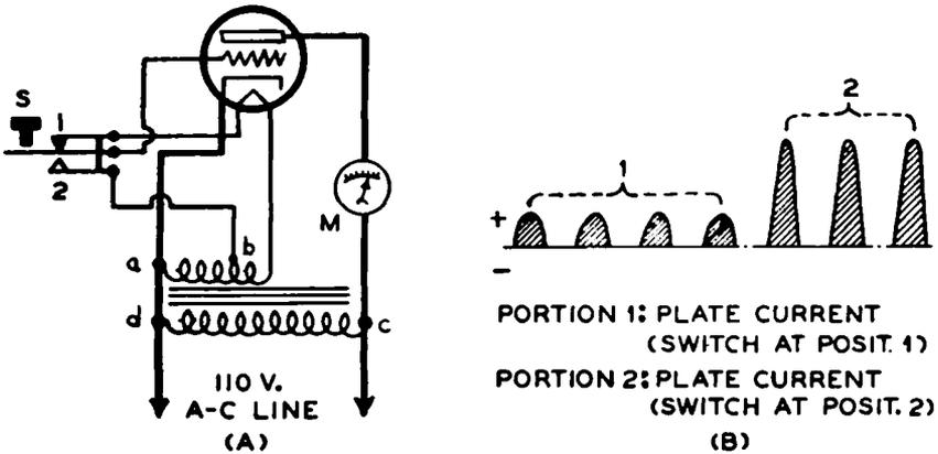
**FIG. 8-7.**—(A) Another method of shifting the grid bias in a tube tester. The bias is shifted by employing either “zero” bias (switch on Contact 1), or the voltage between *a-b* as a grid bias voltage. Point *d* may be considered as *B* minus, and point *c* as *B* plus. Contact 1 is connected to both the cathode and the filament.
