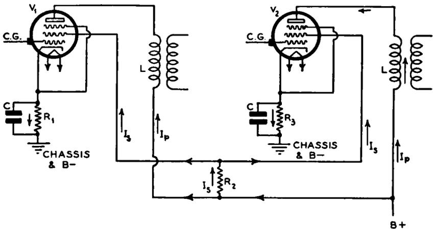
FIG. 20-16.—Typical amplifier stages having a common series-connected voltage-dropping resistor  $R_2$  in the common screen circuit. The total screen current  $I_s$  flows through this resistor, producing a voltage drop in it.
