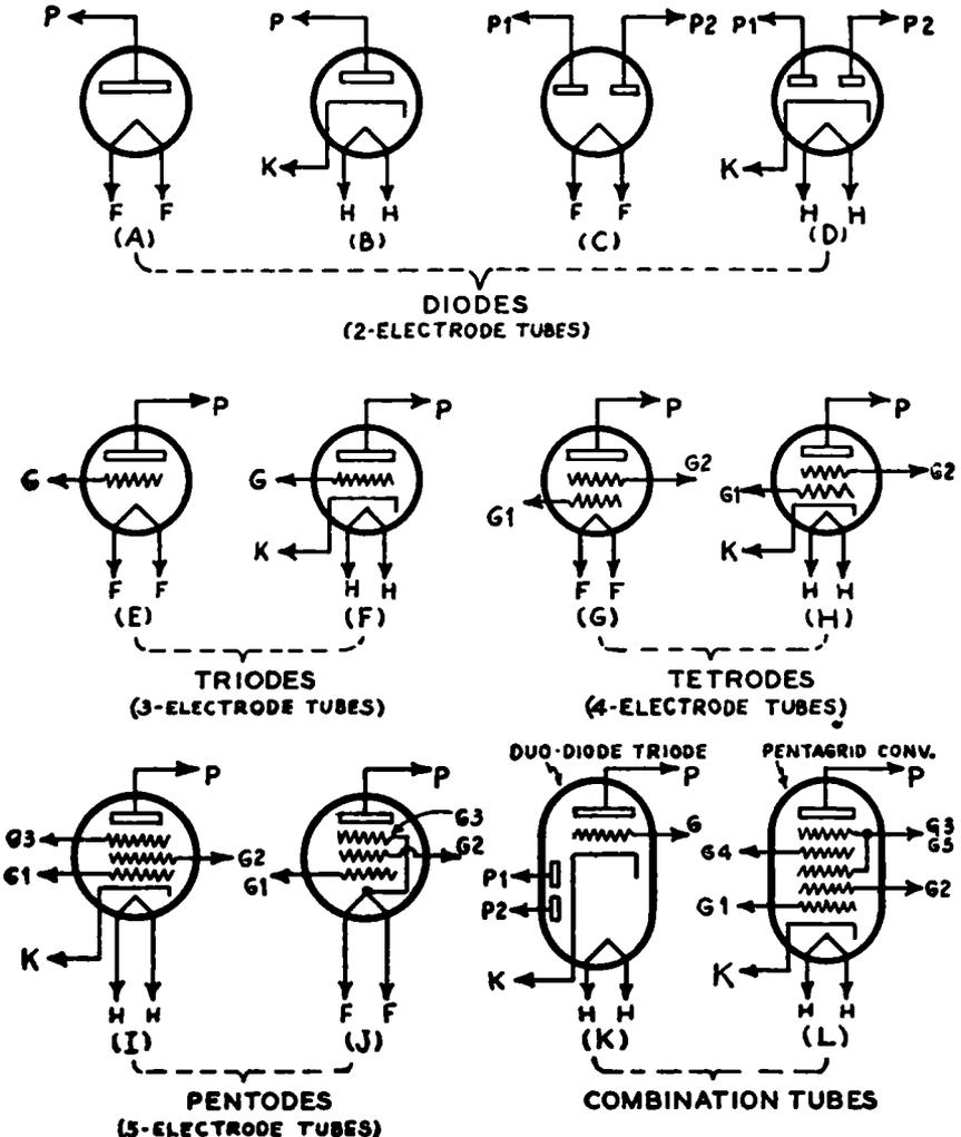
FIG. 8-1.—Some of the electrode arrangements employed in modern radio tubes, starting with the simple diode (2-electrode) tube at (A), progressing to the pentode (5-electrode) tubes at (I) and (J) and the combination tubes at (K) and (L).
