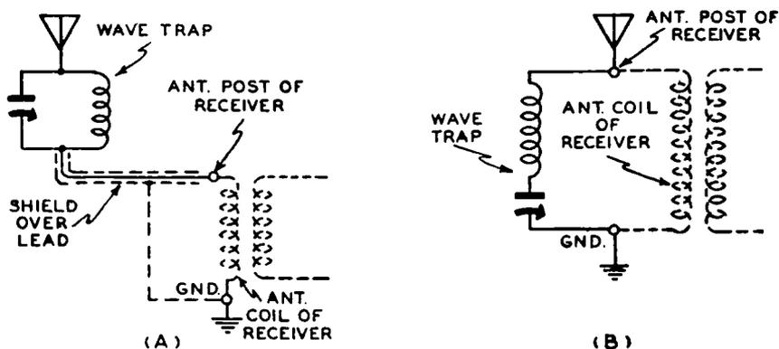
FIG. 23-11.—(A) A wave trap connected in the antenna circuit of a superheterodyne which is troubled by code interference at the low-frequency end of the broadcast scale.
