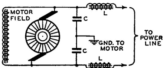
wound with wire of sufficiently large size to safely carry the full load current of the device continuously without overheating. Choke coils having an inductance of about 2 millihenries are commonly used in the filters for those small and medium sized electrical devices which require them.
