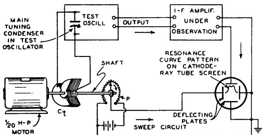
FIG. 25-30.—Arrangement of a motor-driven sweep circuit and frequency-wobbler system for taking visual resonance curves on an i-f amplifier. An electric motor drives the frequency-wobbler condenser  $C_t$  and the sweep-circuit potentiometer  $P$ .
