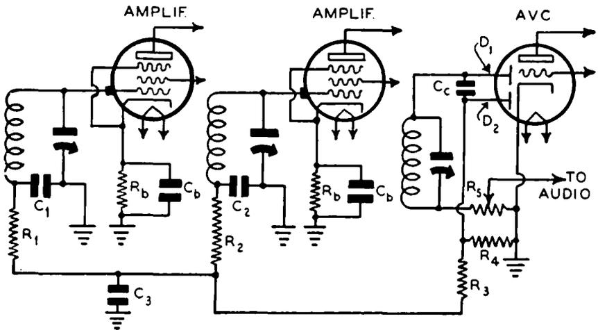
FIG. 19-3.—Controlling the grid bias of amplifier tubes by avc action obtained from the triode section of a duo-diode triode tube in the receiver. This circuit is shown in simplified form in Fig. 19-4.
