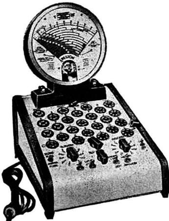
FIG. 10-15. — Weston Model 681 counter type tube checker. Notice the unusually large direct reading meter, the clear and simple layout of its scale.
