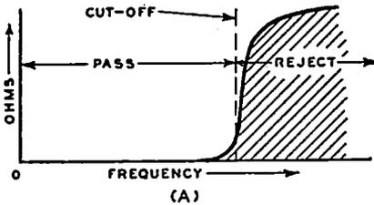
suitable low-pass filter which cuts off sharply at around 7,500 or 8,000 cycles. This filter is located in the audio amplifier.
