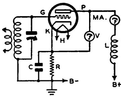
FIG. 12-1.—Checking the resistance between the plate and cathode in a simple radio circuit by means of a milliammeter and a voltmeter.
