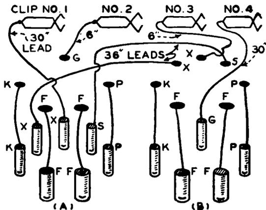
FIG. 11-32.—Two-part adapter for analyzing the circuits of 2A7, 2B7, 6D7, 6E7 and '59, 57B types of tubes when the analyzer is equipped with a 5-prong test plug and a 5-wire cable.
