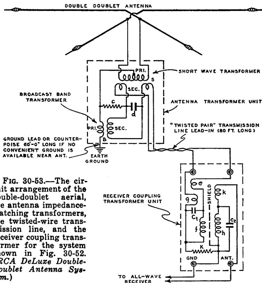
FIG. 30-53.—The circuit arrangement of the double-doublet aerial, the antenna impedance-matching transformers, the twisted-wire transmission line, and the receiver coupling transformer for the system shown in Fig. 30-52. (RCA DeLuxe Double-Doublet Antenna System.)
