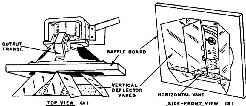
**FIG. 31-14.**—Top and front-side views of a single-unit high-fidelity loud speaker employed in a commercial high-fidelity receiver (Philco). Notice the four vertical and one horizontal deflecting vanes mounted in front of the cone. These “spread” the high-frequency sound waves (see Fig. 31-15) which would otherwise be projected forward in the form of a narrow sound beam.
