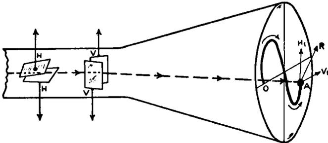
FIG. 25-25.—How the cathode-ray beam traces a wave-form pattern when acted upon by a sinusoidal voltage applied to the horizontal pair of plates,  $H-H$ , and a saw-tooth sweep voltage applied to the vertical pair of plates,  $V-V$ . At the instant pictured here, the beam is acted upon by force  $H_1$  tending to move it vertically in direction  $H_1$ , and by force  $V_1$  tending to move it horizontally in direction  $V_1$ . It actually moves along the direction of the resultant force  $R$ .
