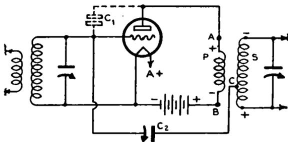
FIG. 24-9. — Another neutralizing circuit similar to that of Fig. 24-8 excepting that here the neutralizing condenser  $C_2$  is excited from the induced e.m.f. in the secondary coil  $S$ . This coil is tapped at  $C$ . This is also a form of *neutrodyne* circuit.
