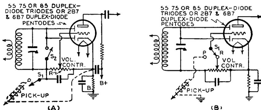
FIG. 26-23.—Two methods of connecting a phono pickup to receivers employing a duplex-diode triode (or duplex-diode pentode) tube. The pickup is connected to the input of the audio triode (or pentode) amplifier section of the tube.
