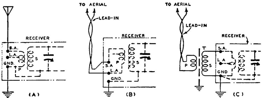
FIG. 30-43.—(A) Arrangement of the antenna coil in a receiver provided with L.A. and S.A. antenna posts.
