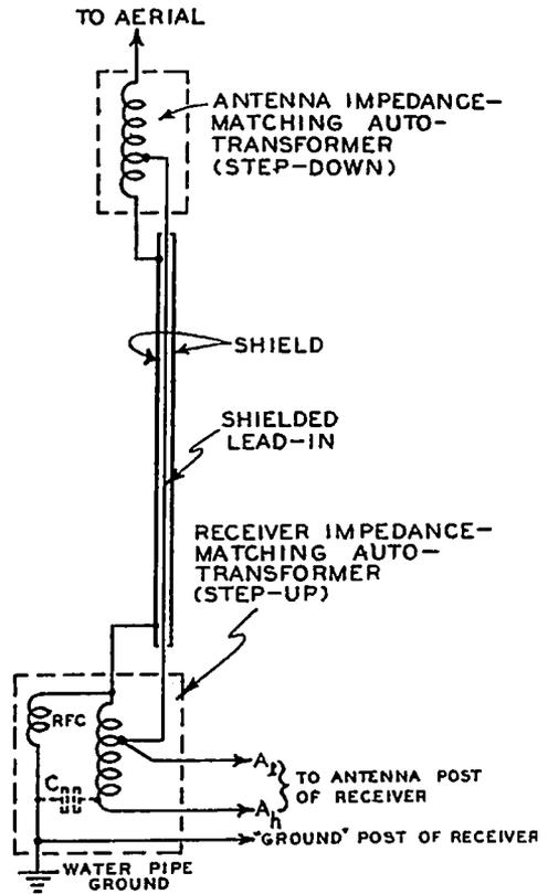
FIG. 30-30.—How impedance-matching transformers are connected at both the aerial and the receiver end of the shielded lead-in.
