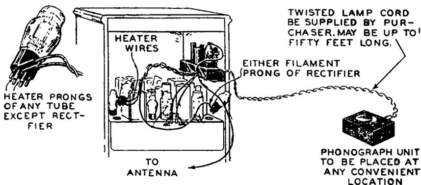
FIG. 26-29.—Typical installation of the phonograph oscillator unit of Figs. 26-27 and 26-28. The method of slipping the lugs over the heater prongs of a tube in the receiver for filament current supply is shown at the left.
