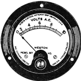
FIG. 2-31.—Exterior view of a small 2-inch diameter a-c voltmeter of the movable-iron type shown in Fig. 2-29. Note the non-uniform scale divisions—crowded at the lower end. (Weston Model 517.)
