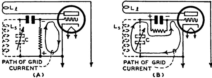
FIG. 15-6.—Direction of the grid current flow in the grid-leak and condenser circuits of Fig. 15-5.
