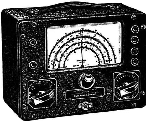
FIG. 17-1. — Exterior view of the all-wave battery-operated test oscillator whose schematic circuit diagram is illustrated in Fig. 17-2. The large dial face with the scales for the various frequency ranges can be seen plainly. The frequency range switch is at the lower left and the attenuator control is at the right. (Model 10.)
