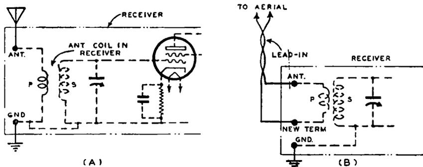
**FIG. 30-41.**—(A) How the antenna coil circuit of most ordinary receivers is arranged.
