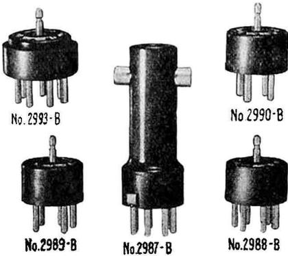
FIG. 11-23. — Seven-prong analyzer dummy plug and four adapters for adapting it to 6-, 5-, 4- and 7 (large base)-hole sockets. See Fig. 11-24 for the internal wiring of these adapters. Notice the control-grid studs on the dummy plug.
