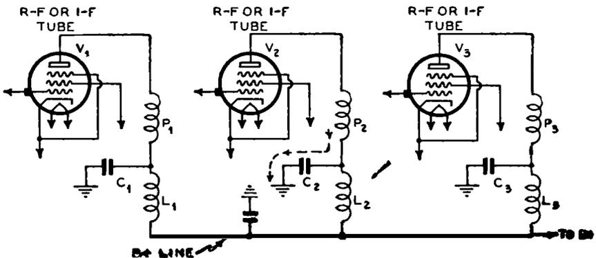
FIG. 23-5.—A typical arrangement for by-passing the plate circuits of a receiver. Chokes are shown inserted in the plate circuits to assist the by-passing action of the by-pass condensers.
