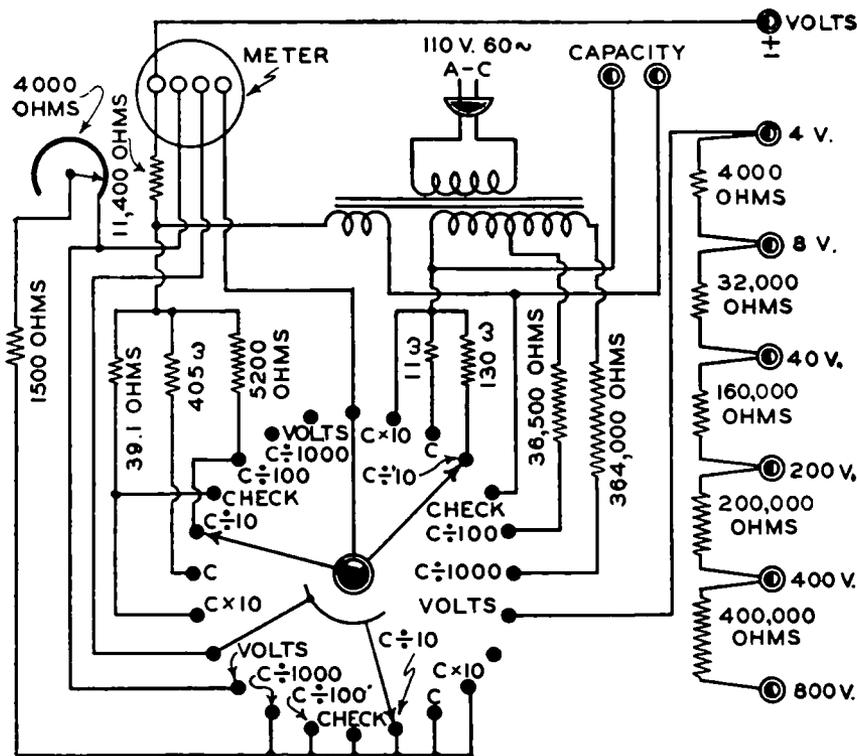
FIG. 6-11.—The schematic circuit diagram of the capacity meter illustrated in Fig. 6-10. Notice the terminals at the right for voltage measurements. Its scale is shown in Fig. 6-12.
