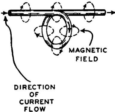
FIG. 2-3. — How the magnetic lines of force arrange themselves around a single-turn loop of wire carrying a current. Notice that they still encircle the wire, but in doing so, they also thread through the inside of the loop.
