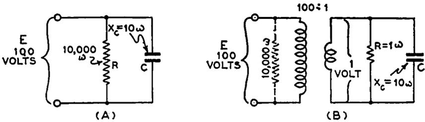
FIG. 30-32.—Equivalent electrical diagrams showing the effect of the impedance-matching transformer on the by-passing action of the lead-in-to-shield capacity of the shielded lead-in.
