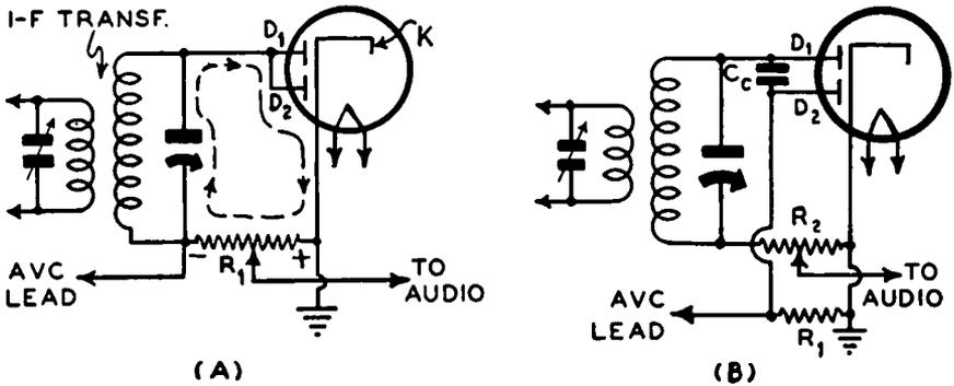
FIG. 19-2.—Two diode detector and avc circuits. In that at (A) the detection and avc action occur in the same circuit. At (B), the detection and avc action take place in two separate circuits.
