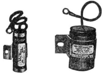
current ripple of the generator may be effectively suppressed by by-passing the live lead which comes from the cut-out, directly to the generator housing by means of a 1/2-mfd. or 1-mfd. condenser. (This is condenser C in Fig. 27-38.) Condensers sealed in metal cans, with one terminal grounded to the can and the other terminal brought out by a flexible lead terminating in a
