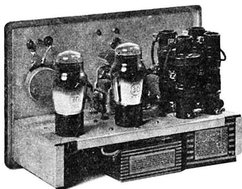
FIG. 17-11.—Interior view showing the construction of the test oscillator above. The two tubes, tuning condenser, coils, and filament and plate batteries are plainly visible.
