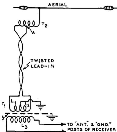
FIG. 30-37. — Circuit arrangement of an antenna system having a twisted-wire lead-in. The method of connecting the two impedance-matching transformers  $T_1$  and  $T_2$ , and the electrostatic shield  $S$  is shown.
