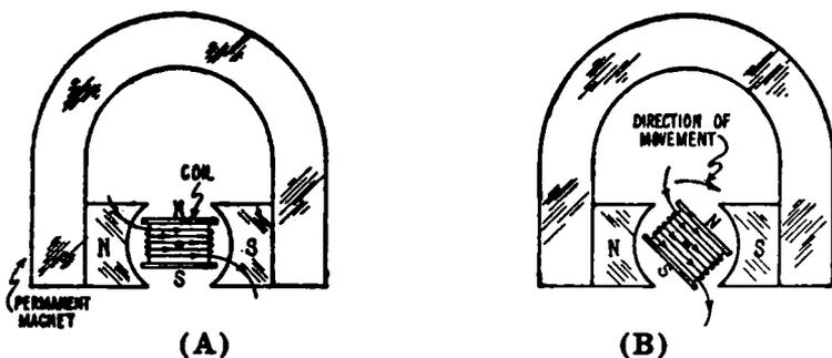
FIG. 2-5.—(A): Arrangement of all of the magnetic poles when a current-carrying coil of wire is placed between the poles of a permanent horseshoe magnet.
