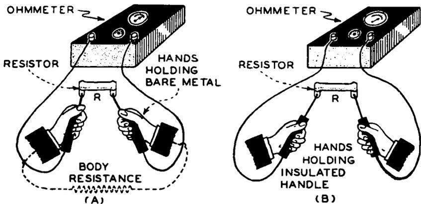
**FIG. 3-15.—(A):** Incorrect way to hold the test prods when using an ohmmeter. The fingers are touching the bare metal of the test prods, thereby shunting the resistance of the body across them.
