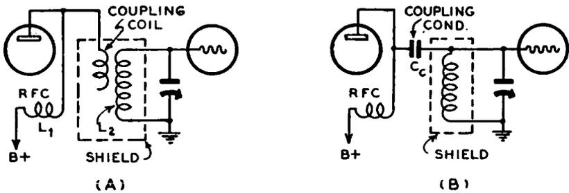
FIG. 23-1.—An open circuit in either the coupling-coil circuit shown in (A), or in the coupling-condenser circuit shown in (B) will cause lack of sensitivity in an r-f or i-f amplifier which employ them. These obscure troubles would not be revealed by the usual voltage-current analysis of the receiver.
