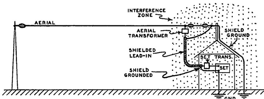
FIG. 30-31.—Method of installing a shielded lead-in for broadcast-band reception only. Impedance-matching transformers are connected at both the aerial and receiver ends of the shielded lead-in wire. The shield is grounded at each end. The ground to the upper end may be conveniently made to a metal roof gutter or leader in many cases.
