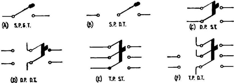
FIG. 11-6.—The common knife switches used extensively in electrical work. These contact arrangements can also be obtained in push-button type switches (see Fig. 11-8).
