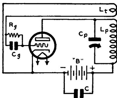
FIG. 15-8.—Reversed feedback oscillator circuit.
