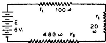
FIG. 21-1.—Three resistances connected in series with each other across a source of voltage,  $E$ . All of the current flows through each resistor. Each resistor has a different voltage drop across it.
