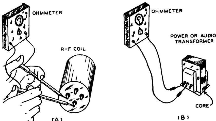
FIG. 22-10.—How an ohmmeter is used to test coil windings for continuity.
