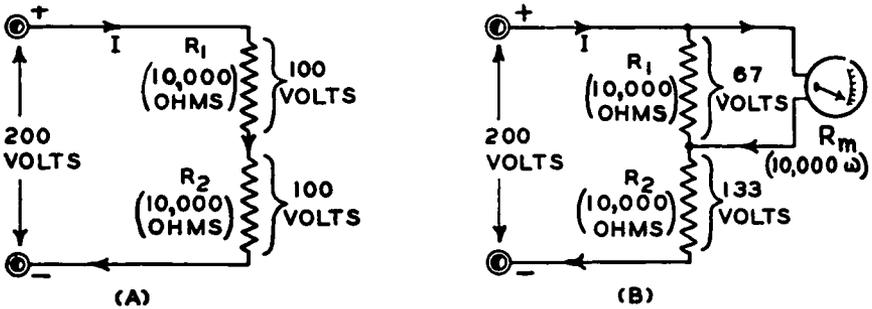
FIG. 2-17.—(A): A typical circuit showing all resistances and voltages before a voltmeter is connected.
