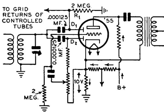
FIG. 19-15. — Another version of the delayed *avc* circuit of Fig. 19-14. Here the diode plates are coupled to the i-f transformer by condensers. (This circuit is employed in the Atwater Kent 711 receiver.)
