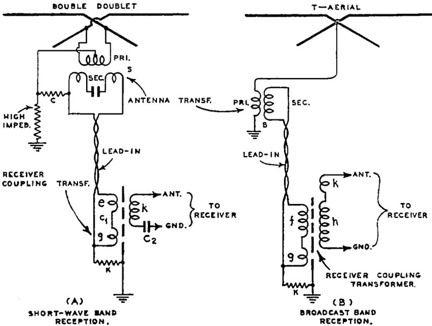
FIG. 30-54.—(A) The essential circuit arrangement which exists when short-wave signals are being received by the double-doublet antenna circuit of Fig. 30-53.
