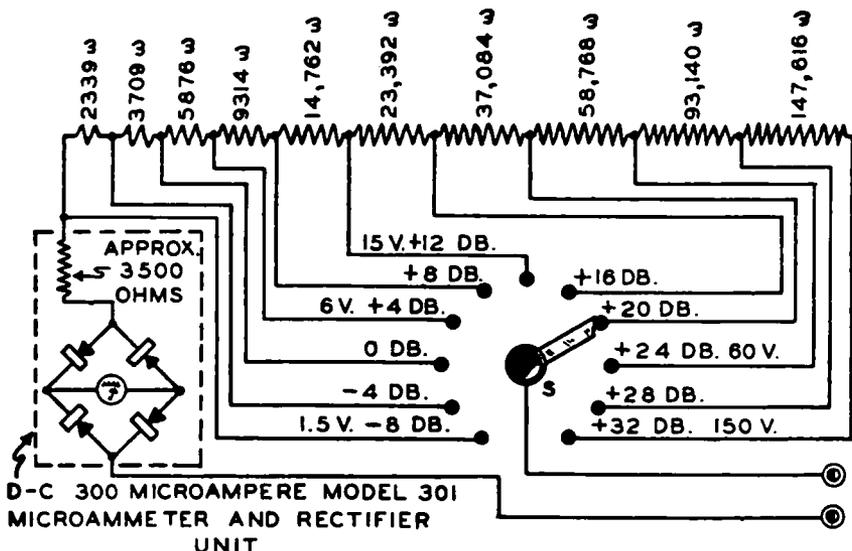
FIG. 7-7.—The schematic circuit diagram of the power level meter illustrated in Fig. 7-7.
