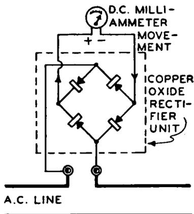
FIG. 2-40 — Conventional circuit diagram for the rectifier type a-c milliammeter arrangement shown in Fig. 2-39. Notice that the *complete* instrument is connected in series with one side of the a-c line.
