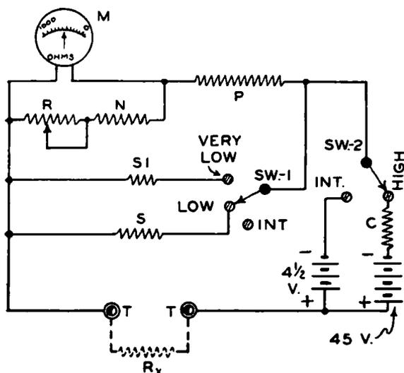
FIG. 3-11. — The series ohmmeter of Fig. 3-10 with two shunt resistors  $S$  and  $S1$  added. These provide two additional ranges. For high resistances, the 45-volt battery and current-limiting resistor  $C$  are put in series with the circuit by switch  $SW-2$ . This results in an ohmmeter with four ranges.
