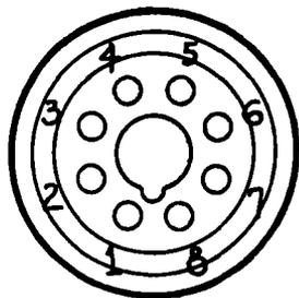
An 8-pin "Octal" tube base (viewed from the bottom) showing the eight pins, their numbers, and the guiding lug at the center.
