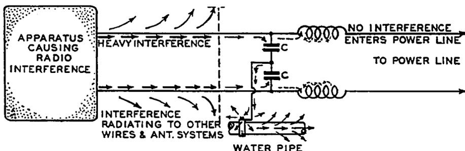
FIG. 30-14.—Schematic circuit showing how the ground pipe may radiate interference, and how the leads which connect the filter to the interfering device may also radiate interference impulses to the part of the line beyond the filter unit, and possibly to the antenna system of the receiver, if it is near enough. The filter should therefore be mounted close to the interfering device and the leads to it should be kept as short as is possible in order to prevent this.
