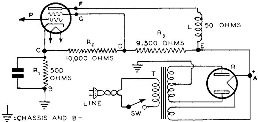
**FIG. 12-3.**—A typical circuit associated with a tube in a radio receiver. This may be analyzed easily by point-to-point resistance measurements made between the reference points indicated by the heavy dots.
