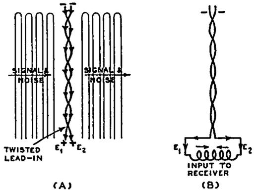
FIG. 30-34.—How a vertical twisted-pair wire lead-in cancels any voltage induced in it by any kind of a signal (including noise) provided it is terminated in a transformer winding in which the induced voltages  $E_1$  and  $E_2$  can balance each other out.
