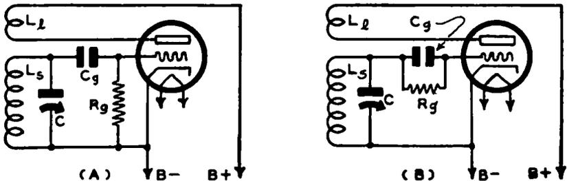
FIG. 15-5.—Two possible ways to connect the grid leak  $R_g$ , and grid condenser  $C_g$ , in the grid circuit of an oscillator tube.
