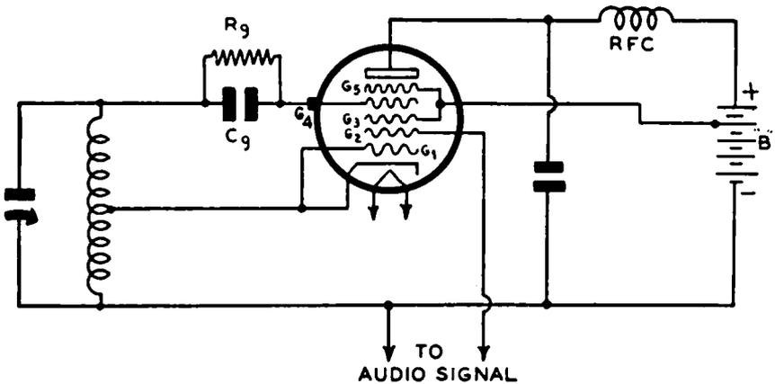
FIG. 15-20.—An electron modulator system. Modulating grid  $G_2$  controls the flow of the stream of electrons between the cathode and plate and modulates it in accordance with the modulating signal impressed upon it.
