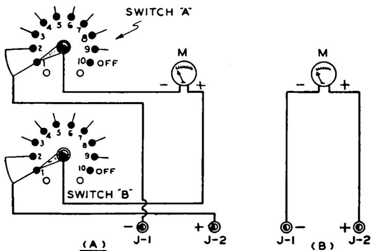
FIG. 5-3.—“Breakdown” of the circuit of Fig. 5-2 when the selector switch *A-B-C* is on contact No. 1. The actual circuit through the switches *A* & *B* (switch *C* is out of the circuit) is shown at (A). The simplified circuit is shown at (B). This places the meter directly across the output terminals, providing the 500-microampere range.
