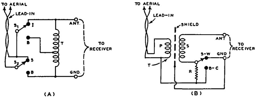
FIG. 30-44.—Two typical switching systems for use with transmission-line aerial systems when they are applied to all-wave receivers. In each case, *T* is the impedance-matching transformer connected between the lead-in and the receiver.
