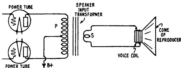
FIG. 23-36.—The same speaker circuit arrangement as that of Fig. 23-35—for two power tubes in push-pull.
