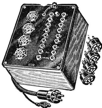
FIG. 14-15.—Another simple analyzer-adapter unit designed to be used in conjunction with an external volt-ohm-milliammeter for point-to-point set analysis. The four adapters provided are shown at the right. Additional "standard" adapters may be used for "octal base" all-metal tubes. (Triplett Model 1220)
