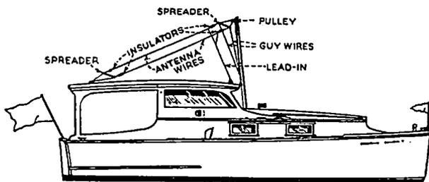
FIG. 29-3.—Method of installing a single or two-wire antenna supported by the mast on a small cabin cruiser.
