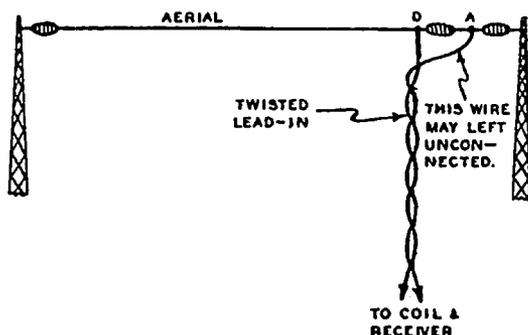
ordinary inverted-L (or T) type used by so many millions of radio owners. With the second section of the lead-in present, any noise voltage picked up by the lead-in is cancelled in the coil connected to the bottom end, and if the horizontal aerial section of the antenna is in a noise-free zone, reception will be comparatively free from noise disturbances (provided the cir-
