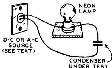
FIG. 22-15.—A simple method for testing solid-dielectric condensers for open-circuits, short-circuits, or leakage, by means of a neon lamp and a 110-volt a-c or d-c voltage source.
