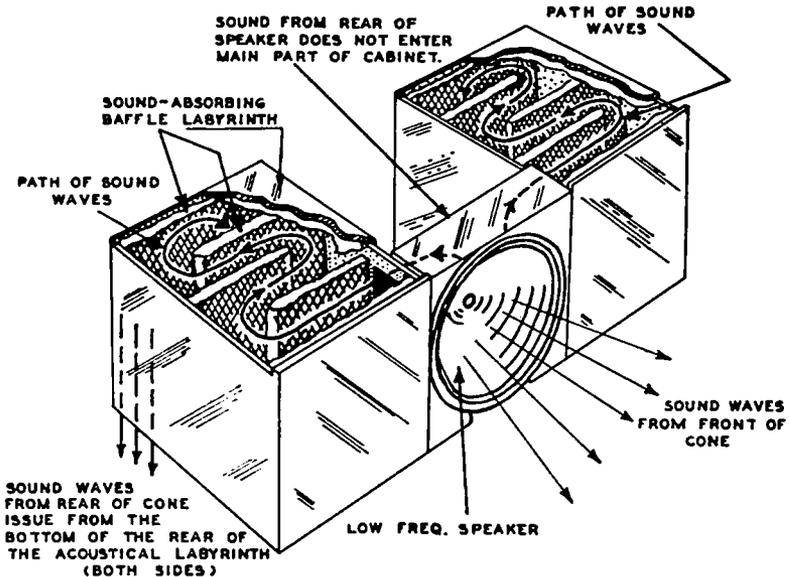
FIG. 31-20.—An acoustical labyrinth type of low-frequency baffle which makes the sound waves from the rear of the speaker cone take a long winding path through the labyrinth before they emerge from the bottom of the receiver cabinet.
