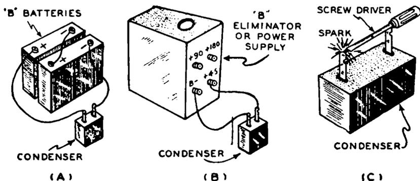
FIG. 22-14.—Testing a large solid-dielectric condenser by means of the charge and discharge method. If the condenser is normal, a spark will be produced on discharge.
