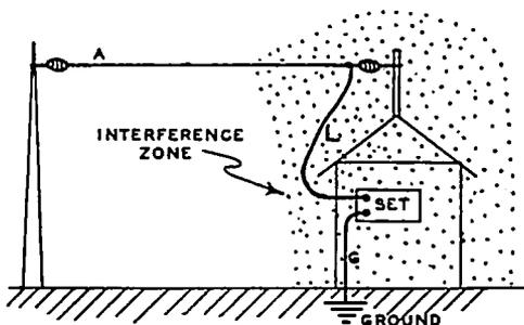
certainly be discontinued, for this connects the ground lead of the set directly to the conduit in which the electric light circuit, alive with interference, runs. The set is really then using the main source of the interference as a ground lead—which is certainly not a pleasant condition to picture!
