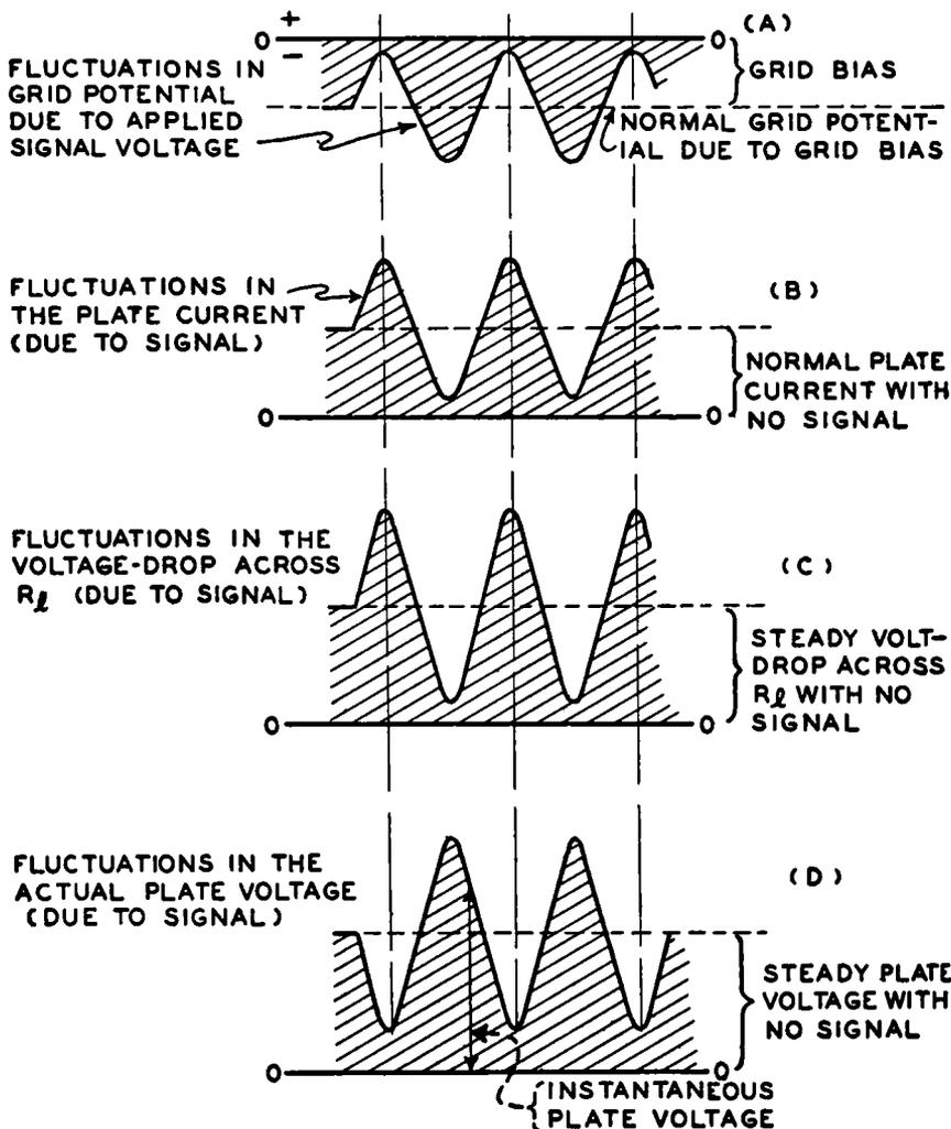
FIG. 15-2.—Graphs showing the simultaneous effects on the grid potential, plate current, voltage drop across the plate load and actual plate voltage, when a sine-wave signal voltage is applied to the grid input circuit of a vacuum tube amplifier or oscillator.
