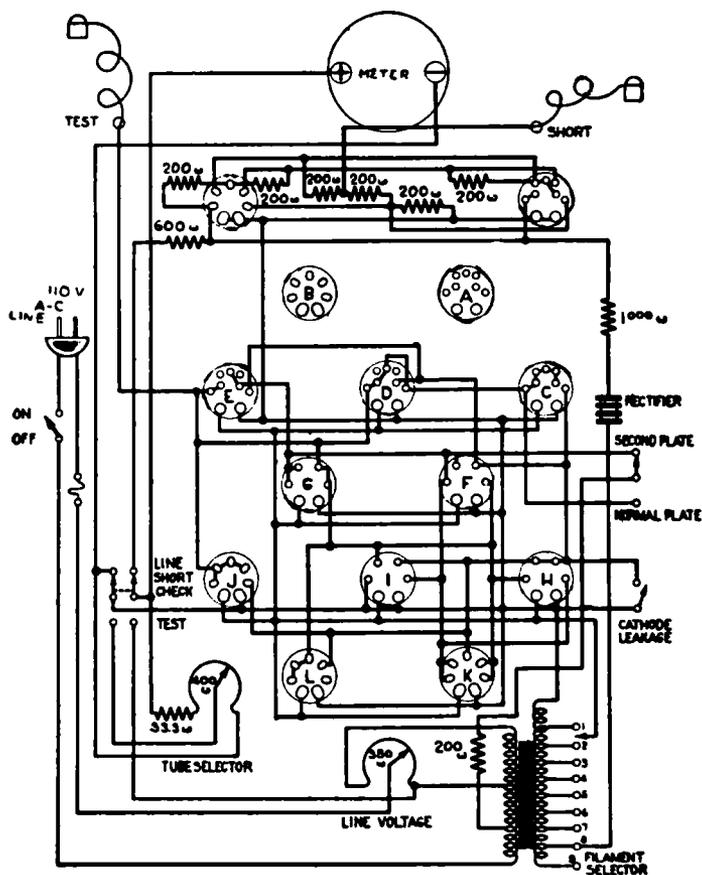
FIG. 10-18.—Schematic circuit diagram of the "emission" type tube checker illustrated in Fig. 10-17.
