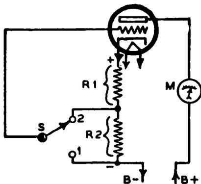
FIG. 8-6. — One method of shifting the grid bias in a tube tester. The switch enables either the voltage drop across  $R1$ , or that across both  $R1$  and  $R2$ , to be applied to the grid of the tube at will.
