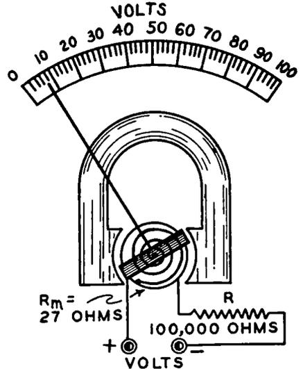
FIG. 2-16.—The general arrangement of the instrument of Fig. 2-15 after a multiplier resistor  $R$  has been connected in series with its movable coil. This multiplier determines the range of the meter. The scale is now calibrated to read “volts”—up to 100 volts.
