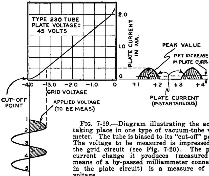
FIG. 7-19.—Diagram illustrating the action taking place in one type of vacuum-tube voltmeter. The tube is biased to its “cut-off” point. The voltage to be measured is impressed on the grid circuit (see Fig. 7-20). The plate current change it produces (measured by means of a by-passed milliammeter connected in the plate circuit) is a measure of this voltage.
