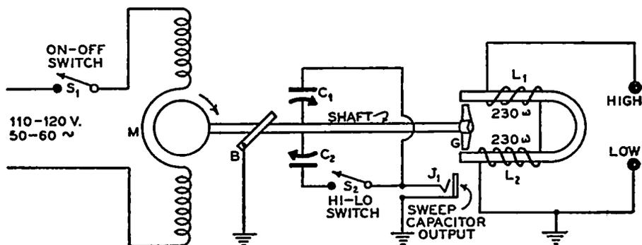
FIG. 25-36.—Schematic circuit arrangement of the motor-driven “frequency-wobler” and saw-tooth voltage synchronizing unit illustrated in Fig. 25-35.
