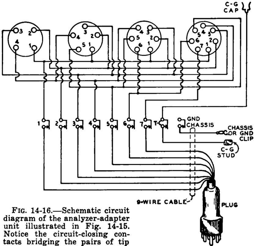
FIG. 14-16.—Schematic circuit diagram of the analyzer-adaptor unit illustrated in Fig. 14-15. Notice the circuit-closing contacts bridging the pairs of tip jacks.
