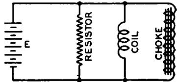
FIG. 21-4.—A choke, a coil and a resistor are shown here connected in parallel. The respective *resistances* of these devices might be represented as shown in Fig. 21-3.
