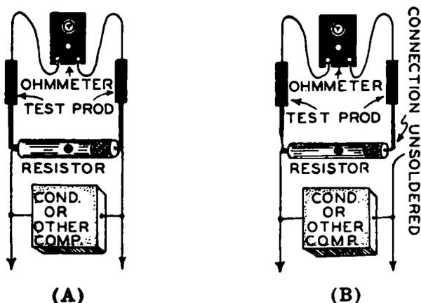
FIG. 3-16.—(A): Incorrect method of checking resistance with an ohmmeter. A leaky condenser (or other component) has been left connected across the resistor whose value is to be measured, thus shunting it and causing the ohmmeter to indicate a lower resistance than the true value.
