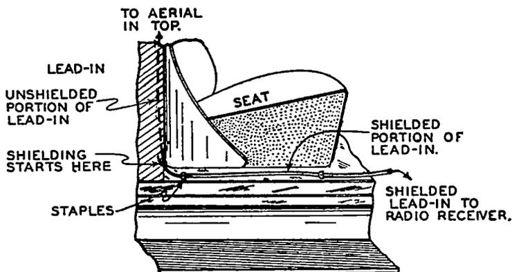
FIG. 27-23.—How the partly-shielded lead-in is run down along the side of the seat and along the floor of the car when a wire aerial is installed in a car having a folding top.
