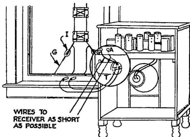
**FIG. 30-49.**—How the leads of a transposed lead-in may be brought in through the window to the impedance - matching transformer *T* at the receiver, when the receiver is near the window. The wires to the receiver may be twisted if the distance is short.
