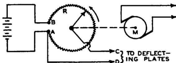
FIG. 25-28.—A saw-tooth sweep voltage may be generated by arranging a motor  $M$  to drive a potentiometer  $R$  connected across a source of potential.
