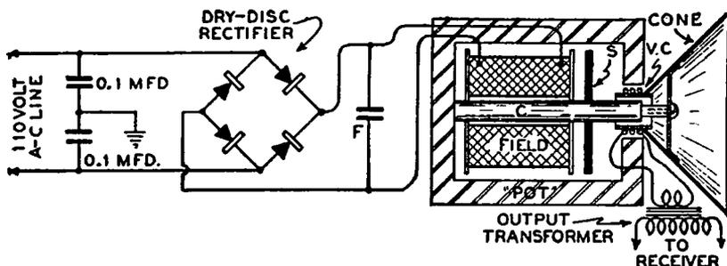
FIG. 26-15.—A high-voltage type dry-disc rectifier arrangement for rectifying the a-c voltage from the line so that d-c may be supplied to the speaker field. A "shading" ring *S* is used to prevent line hum.
