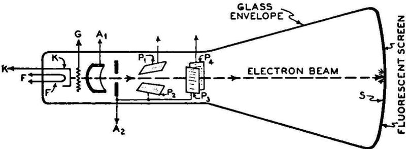
FIG. 25-16.—Internal construction of a typical cathode-ray tube. The electron beam is projected along the length of the tube to the fluorescent screen upon which it impinges and produces a spot of visible light.
