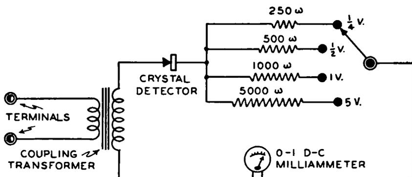
FIG. 7-15.—A crystal detector type output meter in which a 0-1 d-c milliammeter is employed as a low-range d-c voltmeter.
