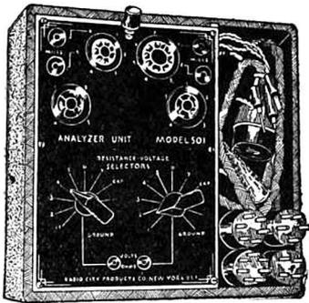
FIG. 14-1. — An analyzer-adapter unit designed to operate in conjunction with an external volt-ohm-milliammeter for point-to-point set analysis. Its circuit diagram is shown in Fig. 14-2. (Dependable Model 501.)
