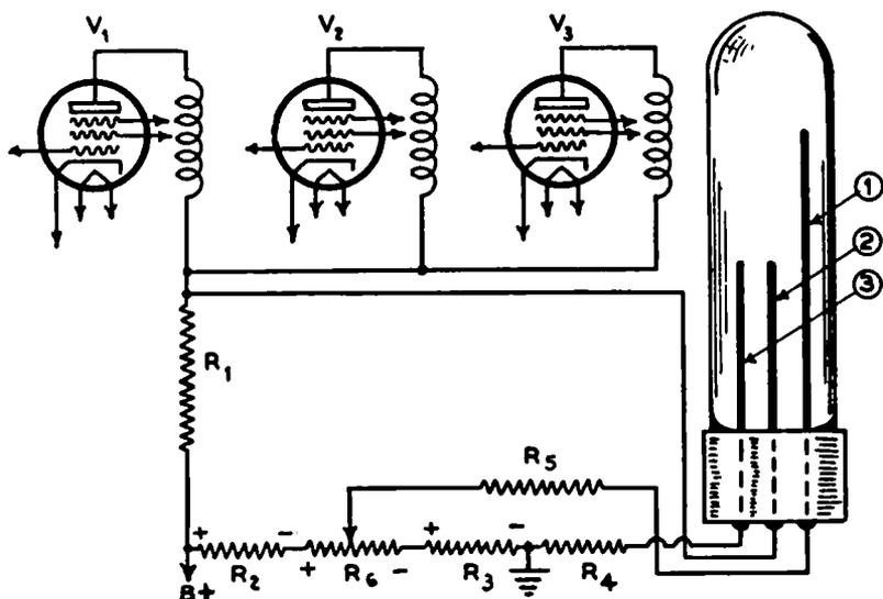
FIG. 19-29.—Connection of the 3-element Flashograph to the r-f or i-f amplifier tube circuits.
