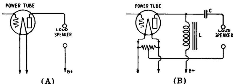
FIG. 23-33.—(A) Connecting the loud speaker winding directly into the plate circuit of the power tube.
