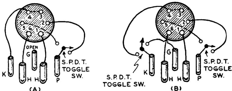
FIG. 8-24.—(A) Wiring of an adapter for testing 25Z5 tubes in the '27 socket of a tube tester able to supply 25 volts to the filament. (B) A single adapter for testing both the '19 and 25Z5 tubes. Two switches are employed.
