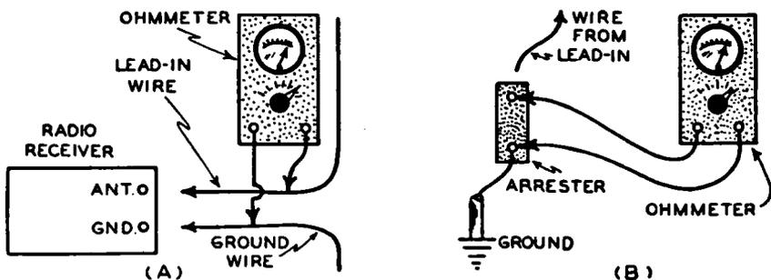
FIG. 18-2.—(A): Testing the aerial and lead-in circuit for grounds or high-resistance leaks, using an ohmmeter. (B): Checking the lightning arrester for leakage and short circuit, using an ohmmeter.
