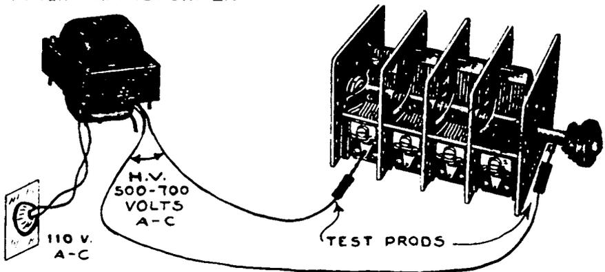
FIG. 26-7.—Circuit arrangement for burning out dust, or metal peelings, from the plates of a tuning condenser by using the high voltage from an ordinary radio receiver power transformer.
