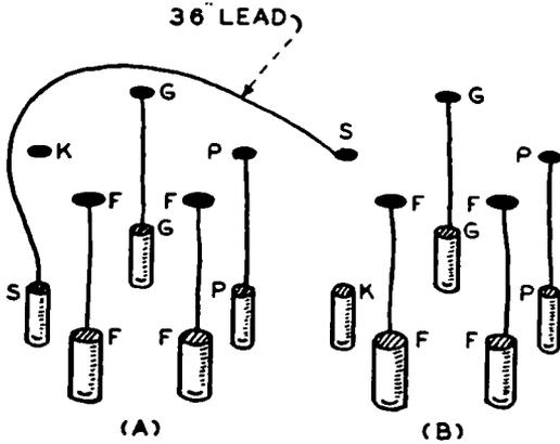
FIG. 11-30.—Two-part adapter for analyzing the circuits to '33, '46, '47, '49, etc., tubes when the analyzer is equipped with a 5-prong test plug and a 5-wire cable.
