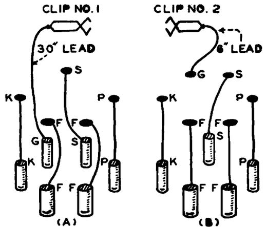
FIG. 11-33.—Adapter for analyzing the circuits to '55, '57, '58, '75, '77, '78, etc., tubes, and to '18, '41, '42, '43, '48, PZH, etc., tubes when the analyzer is equipped with a 5-prong plug and 6-wire cable.
