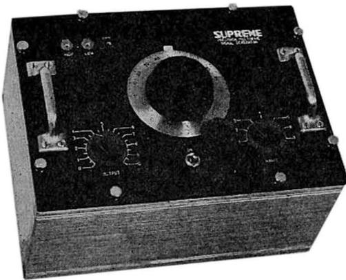
FIG. 17-17.— The battery-operated, two-tube, all-wave test oscillator whose schematic circuit diagram is shown in Fig. 17-18. (Model 180)
