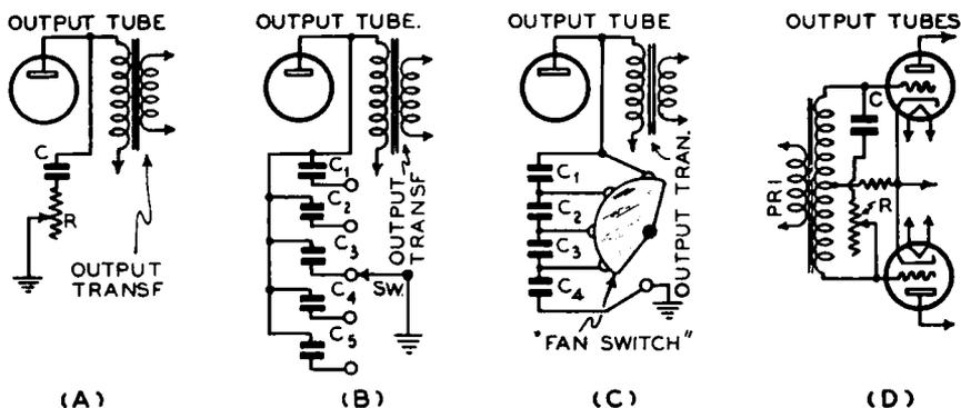
FIG. 23-30.—Several common tone-control circuit arrangements.
