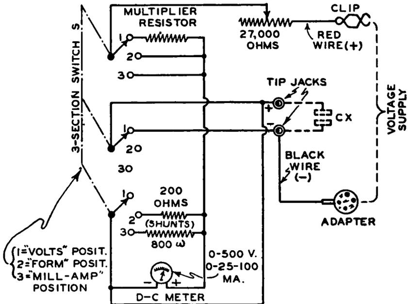
FIG. 6-9.—Schematic circuit diagram of the portion of the capacity meter of Fig. 6-7 which is used for testing electrolytic condensers by measuring their leakage current.
