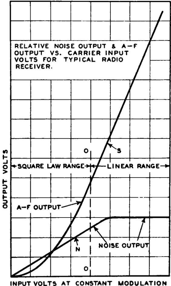
carrier of the strong one remains, and since an r-f carrier cannot be amplified in an audio amplifier, the weak station cannot be heard. The curves of Fig. 31-11 illustrate the idea of demodulation of noise by a strong carrier in a linear detector. Notice that the noise output curve *N* flattens out soon after a signal input which makes the detector operate linearly is applied.
