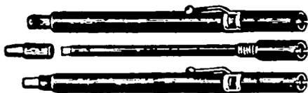
FIG. 25-13.—Three views of a combination fountain-pen size neutralizing tool made of fibre. By screwing the various sections together in different combinations 1/4- and 5/16-inch nut wrenches, a miniature blade screw driver for neutralizing and aligning, and a full-size general-purpose screw driver with insulated handle are provided.
