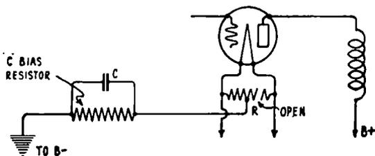
FIG. 23-12.—How a center-tapped filament resistor may become “open” thus upsetting the electrically-neutral condition of the center-tap and causing hum.
