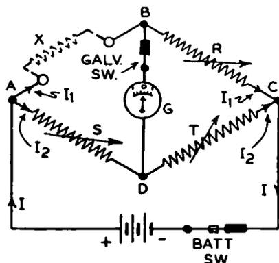
cating meter  $G$  is connected across points  $B$ - $D$ . A low-voltage battery connected, as shown, to points  $A$  and  $C$  causes current to flow through the two branches of resistors, in the directions shown by the arrows, when the battery switch is closed.
