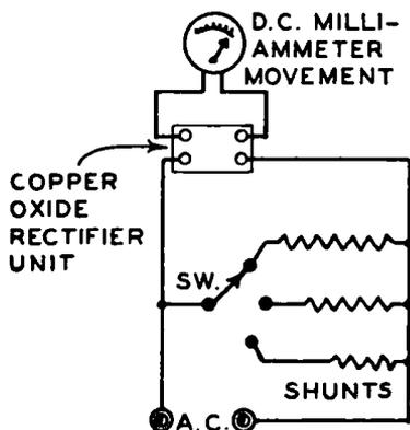
FIG. 2-41.—How a d-c milliammeter movement, a meter rectifier and shunts may be connected together to make a multi-range rectifier type a-c milliammeter.
