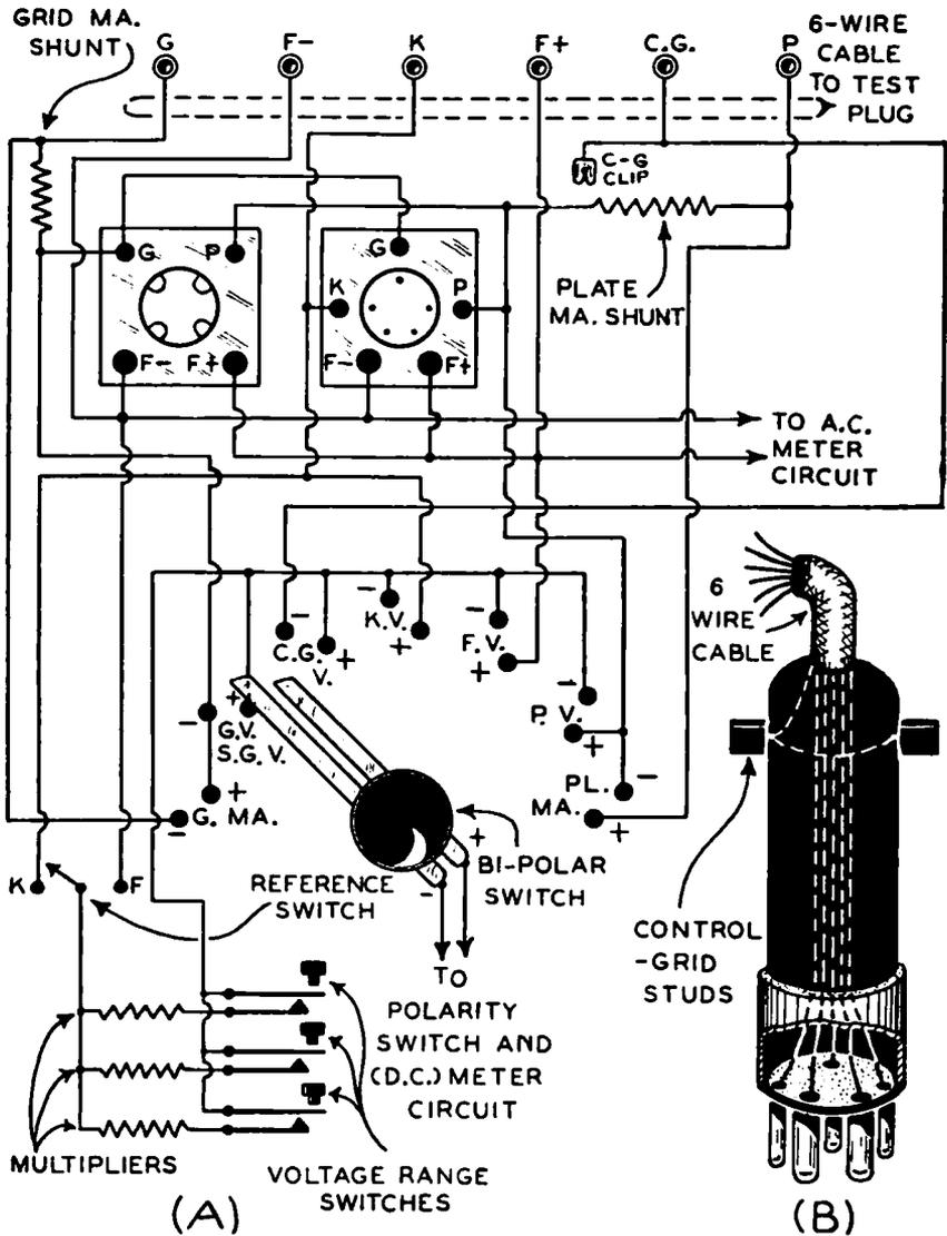
FIG. 11-19.—(A) Analyzer circuit after provisions have been made for measuring the control-grid voltage of screen grid tubes.
