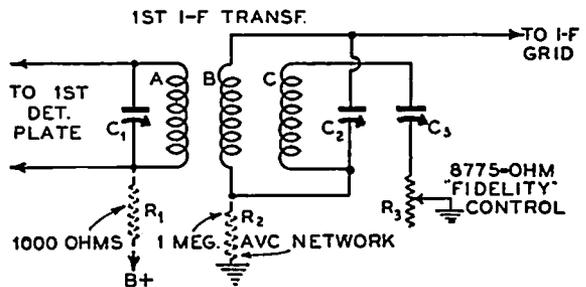
on the first detector (by means of resistor  $R$  in Fig. 31-4) and first i-f stages is reduced to raise the gain to that obtainable, when the receiver is adjusted to provide sharp tuning (a total band width of about 4,000 cycles).
