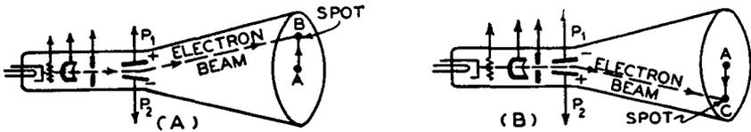
FIG. 25-18.—How the electron beam is “bent” or “deflected” by the electric charges applied to the deflecting plates. Only one pair of deflecting plates is shown here for simplicity.
