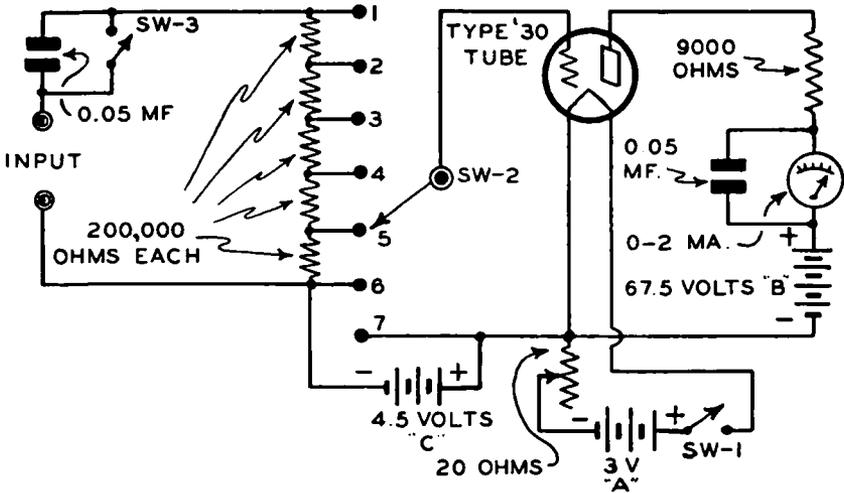
FIG. 7-21.—Schematic circuit diagram of an easily constructed V.T. voltmeter for use by radio service men.
