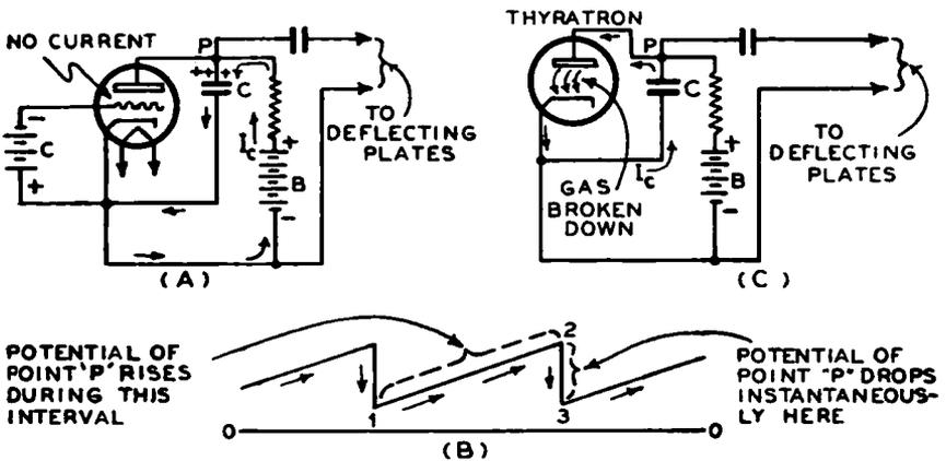
FIG. 25-27.—A simplified analysis of the “trigger” action which takes place in the sweep circuit of Fig. 25-26 is shown at (A) and (C). The saw-tooth voltage shown at (B) exists across condenser  $C$  and is applied to one pair of plates of the cathode-ray tube (not shown here).
