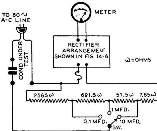
FIG. 14-9. — Circuit arrangement employed for capacity measurements in the set analyzer of Fig. 14-5. The meter rectifier enables the d-c meter to be used to measure the a-c flowing through the condenser under test. The meter shunts are selected by the switch.
