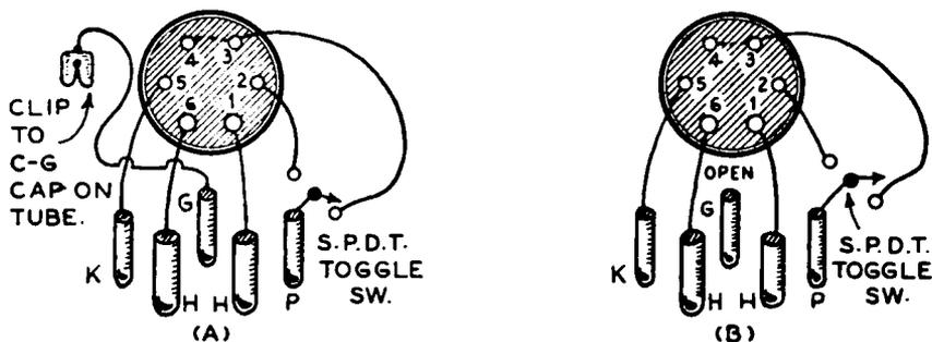
FIG. 8-21.—(A) Wiring of an adapter for testing the 55, 75, 85, and 2A6 tubes in the '27 or '37 socket of a tube checker. (B) Wiring of an adapter for testing the 55, 75, 85, and 2A6 tubes in a '24 or '36 socket of a tube checker.
