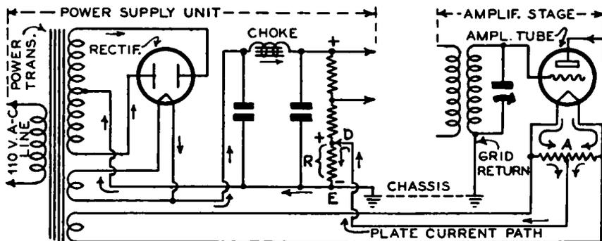
FIG. 20-4.—One of the two circuit arrangements used for obtaining the required *C* bias voltages in many old electric receivers which employed direct-heater type tubes. Resistor *R*, which forms part of the voltage-divider resistor, is the grid-bias resistor. The arrows show the complete path of the plate current of the amplifier tube.
