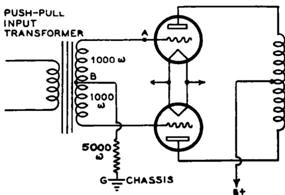
FIG. 21-9.—A typical push-pull output stage of a receiver. The resistance of each half of the input transformer secondary is considered to be 1,000 ohms.
