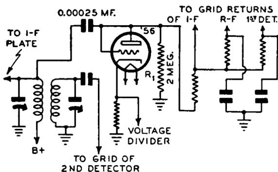
**FIG. 19-13.**— Here, a triode, connected as a diode, acts as the avc tube. Signal voltage from the i-f plate circuit feeds the avc diode. The variations in diode plate current vary the avc voltage-drop across  $R_1$ . (Used in Atwater Kent 310 receiver.)
