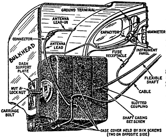
FIG. 27-8.—Detail showing how a typical single-bolt mounting auto-radio receiver is fastened to the driver's side of the bulkhead between the engine compartment and the passenger portion of the car. This view is drawn looking from the engine side of the bulkhead back toward the driver's compartment.
