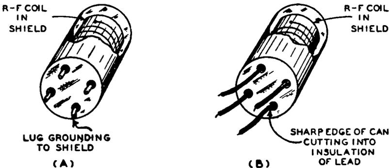
FIG. 22-6.—Two possible ways in which the terminals of a coil or transformer may ground to the metal shield which encloses it. At (A) the coil has metal terminal lugs; at (B) the coil has flexible-lead terminals.
