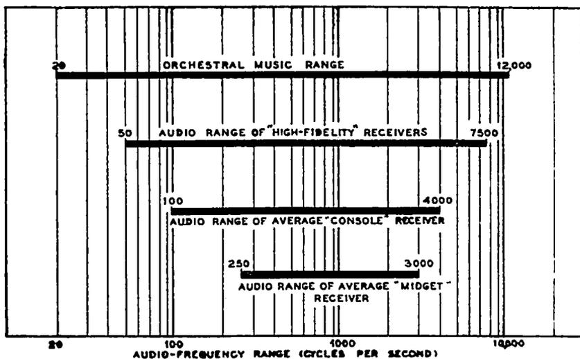
FIG. 31-1.—The average audio reproduction ranges of various classes of radio receivers are shown here. They are arranged so they may be compared to the full frequency range of orchestral music.
