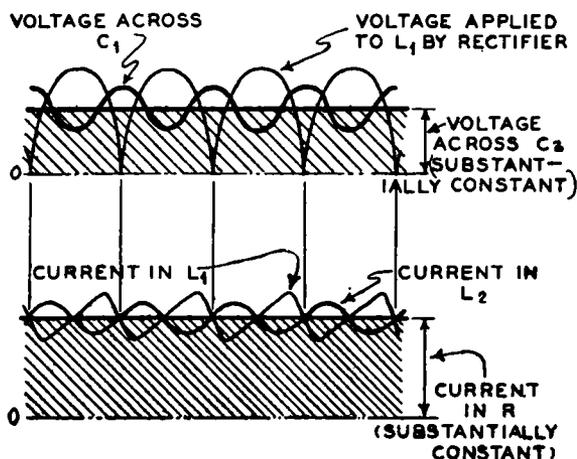
FIG. 20-22.—Graphs showing the waveforms of the currents and voltages in a choke-input type filter (see (A) of Fig. 20-21).
