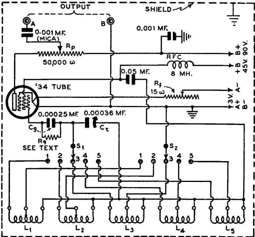
FIG. 16-1.—Schematic circuit diagram of an all-wave, battery-operated electron-coupled test oscillator. Instructions for constructing and operating it will be found in the accompanying text. The same oscillator, arranged for line operation, is shown in Fig. 16-3.
