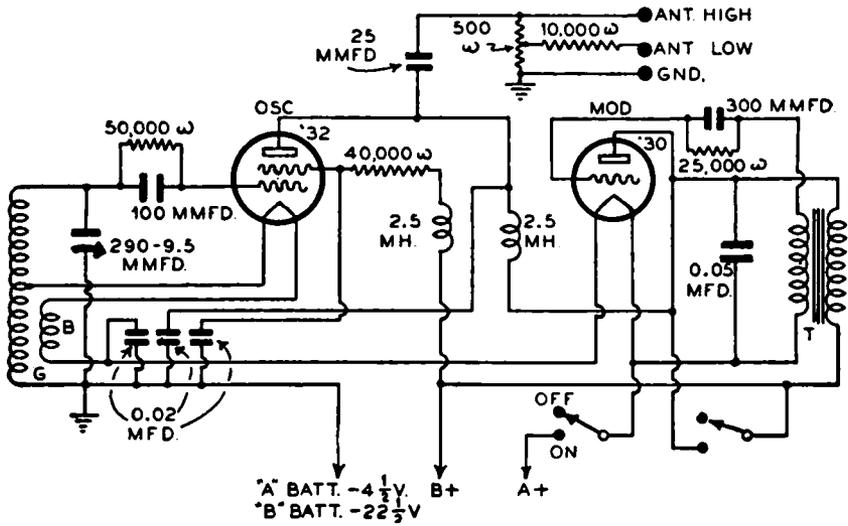
FIG. 17-18.—Schematic circuit diagram of the test oscillator illustrated in Fig. 17-7. This is a 2-tube, separately modulated, oscillator of the electron-coupled type.
