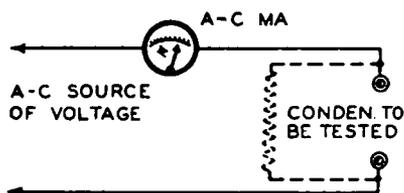
a known voltage of known frequency to the condenser to be tested and measuring the amount of current flow by means of an a-c current-indicating device, as shown in Fig. 22-16.
