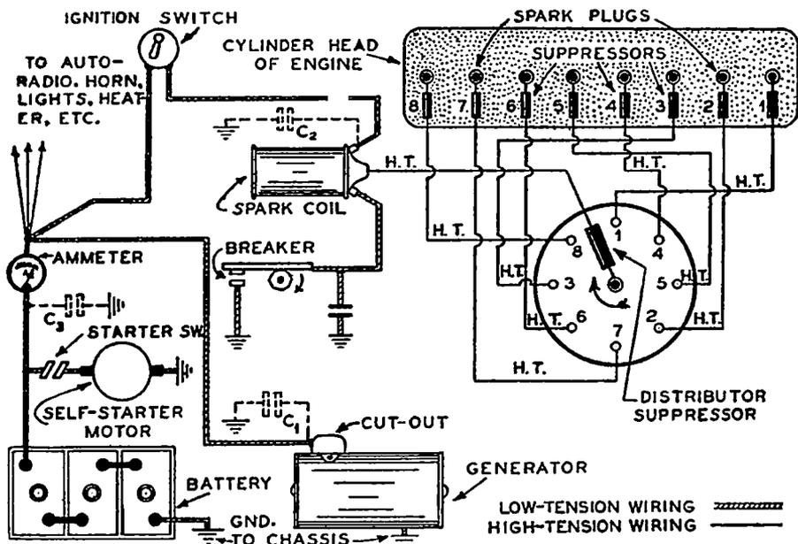
FIG. 27-57.—Complete schematic wiring diagram of the ignition wiring on a typical 8-cylinder automobile.  $C_1$ ,  $C_2$  and  $C_3$  are the added generator, coil and ammeter by-pass condensers respectively. The distributor and spark plug suppressors are shown installed in place. This represents the "standard" suppression measures which are sufficient for interference suppression on about half of the cars encountered. Additional measures must be taken in the others.
