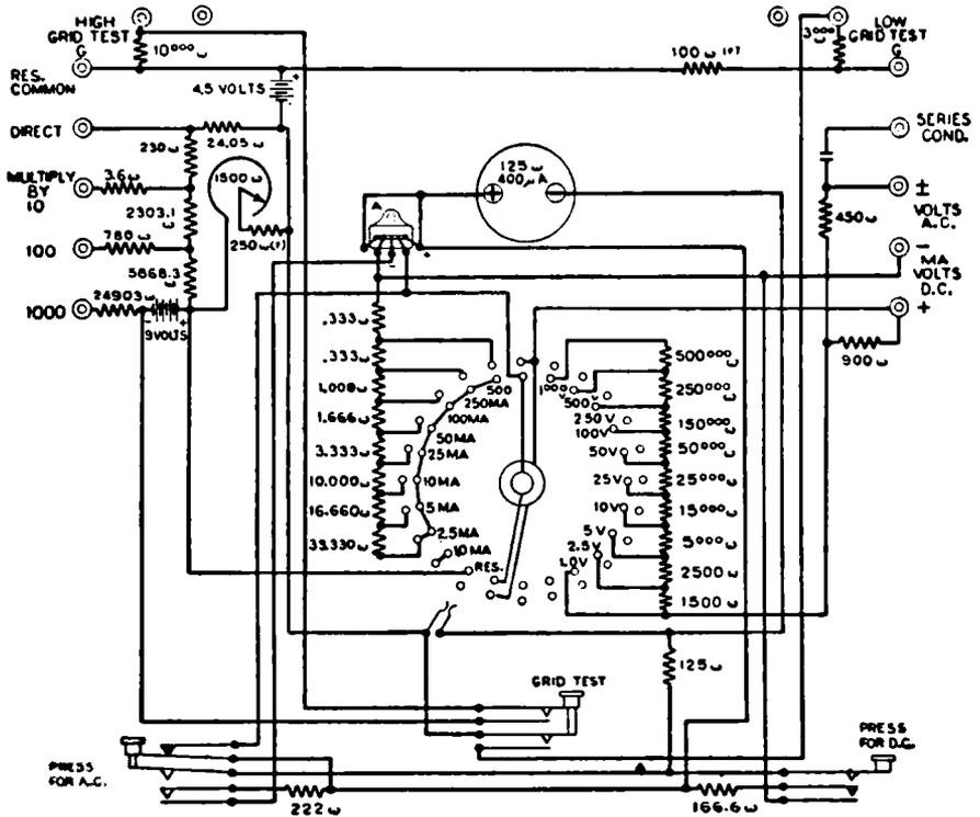
FIG. 14-19.—Schematic circuit diagram of the Selective Set Analyzer Unit illustrated in Fig. 14-17. The circuit shown here is for the Type 1 instrument, which is provided with a selector switch for switching the various circuits.
