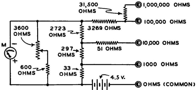
FIG. 5-12.—“Breakdown” of the circuit of the volt-ohmmeter shown in Figs. 5-10 and 5-11 when it is used as an ohmmeter.
