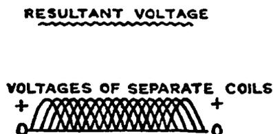
FIG. 27-37. — The “resultant voltage” graph shows the “ripply” nature of the output current of a d-c generator due to the fact that this current is really the sum of the various rectified sine-wave currents of the individual coils on the armature as shown below.
