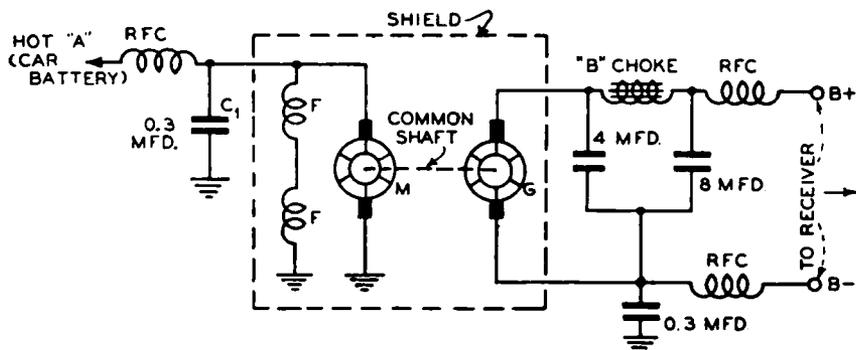
FIG. 27-68.—The circuit arrangement of the "generator" type auto-radio *B* power unit illustrated above. Both the r-f choke and *B*-filter systems are built into the unit.
