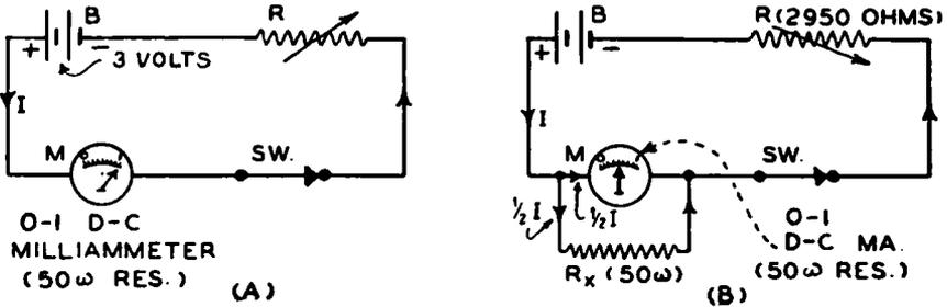
FIG. 3-12.—(A): Simple series-type ohmmeter circuit with a 50-ohm 1-ma. meter.
