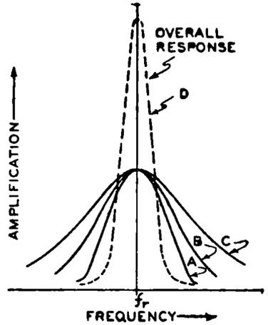
FIG. 25-3. — Amplification curves of the individual i-f amplifier stages A, B and C of a superheterodyne. D is the overall response curve. The resonant frequency is  $f_r$ .
