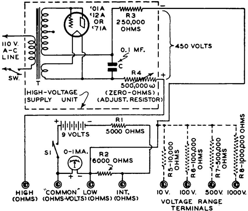
FIG. 4-5.—Circuit diagram of a high-voltage supply unit (within the dotted line rectangle) capable of delivering 450 volts, and an ohmmeter circuit capable of measuring from ½-ohm to 10 megohms in 4 ranges. If the resistors shown at the right (drawn dotted) are employed, the meter can also be used as a 4-range d-c voltmeter.
