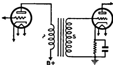
FIG. 23-17.—A typical transformer-coupled audio amplifier stage.
