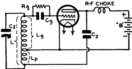
FIG. 15-12.—Parallel feed Hartley oscillator circuit. The feedback coil  $L_g$  and condenser  $C_2$  form a parallel circuit with that of the plate.
