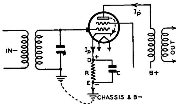
FIG. 20-6. — The most common method for obtaining the negative grid bias for an indirect-heater type tube by making its plate current flow through resistor *R*. This makes point *E* (and the control grid) *negative* with respect to point *D* (and the cathode).
