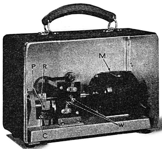
FIG. 25-35.—A portable motor-driven "frequency-wobbler" and saw-tooth voltage synchronizing unit for use with a cathode-ray oscilloscope when aligning tuned circuits. (Model TMV-128-A)
