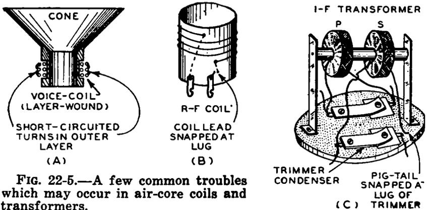
FIG. 22-5.—A few common troubles which may occur in air-core coils and transformers.
