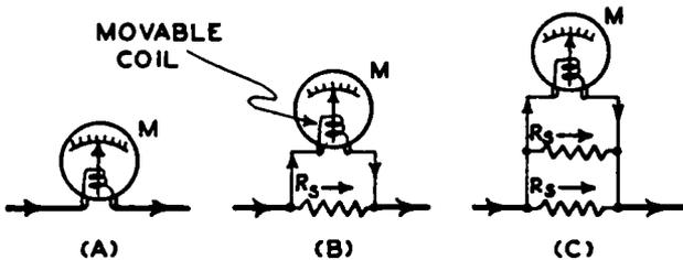
FIG. 2-8.—How shunts are connected in *parallel* with the movable coil of the meter. The shunts carry a definite fraction of the total current to be measured, permitting the use of an ordinary milliammeter movement as an ammeter to measure larger currents than the movable coil is able to carry safely.
