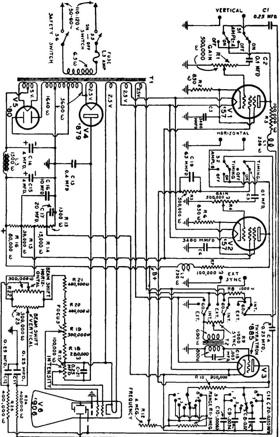
FIG. 25-34.—Schematic circuit diagram of the complete oscilloscope illustrated in Figs. 25-32 and 25-33. (Courtesy R.O.A. Mfg. Co.)
