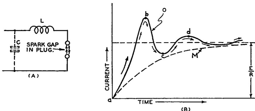
FIG. 27-45.—(A) The oscillatory circuit which is formed by the spark plug circuit.
