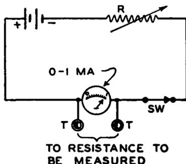
of resistance being measured. When a shunt resistor  $R_s$  is employed, resistor  $R$  is first adjusted (with terminals  $T-T$  open) so that the meter reads full-scale with this shunt connected.
