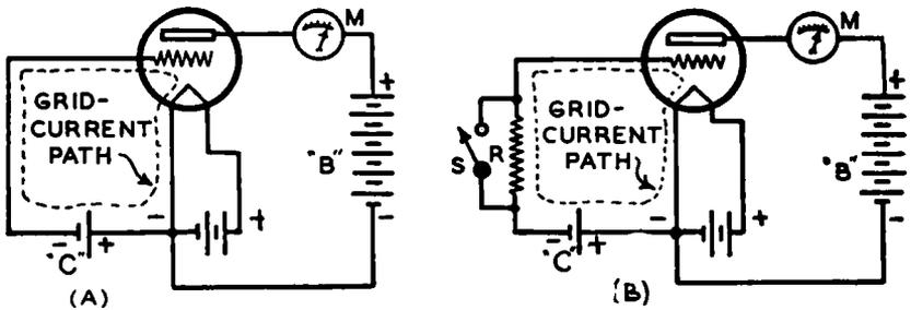
FIG. 8-4.—Action of the circuit arrangement employed to make a "gas" test on a vacuum tube.
