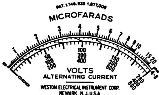
FIG. 6-12.—Reduced facsimile reproduction of the scale of the capacity meter shown in Figs. 6-10 and 6-11. Notice the fairly uniform division spacings.
