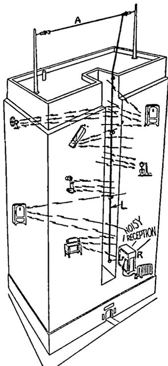
FIG. 30-7. — How various electrical appliances in an apartment house or hotel will cause disturbances not only through the power supply line (see Fig. 30-4) but also by direct radiation and re-radiation to the lead-in (and possibly the aerial) due to their close proximity to it.
