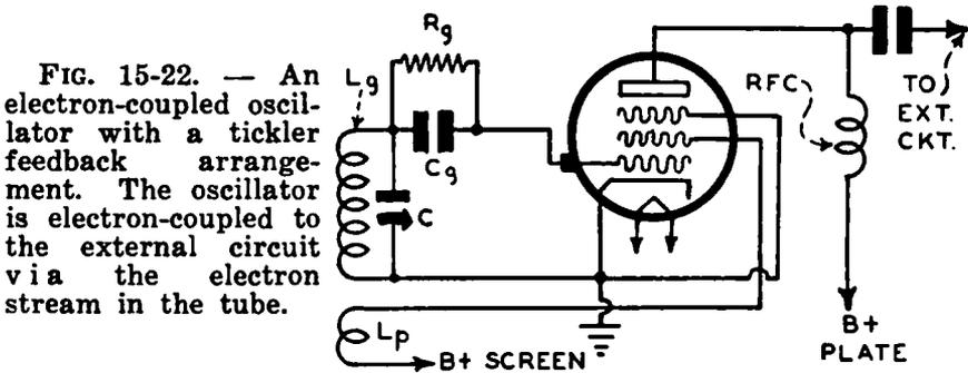
FIG. 15-22. — An electron-coupled oscillator with a tickler feedback arrangement. The oscillator is electron-coupled to the external circuit via the electron stream in the tube.
