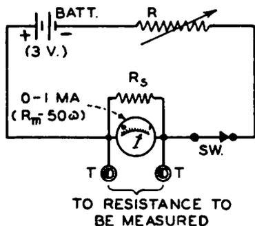
FIG. 3-14.—Here the meter is shunted by shunt resistor  $R_s$  in order to make it possible to measure lower values of resistance.
