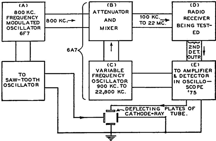
FIG. 25-38.—Block diagram showing the main parts of the visual resonance oscilloscope illustrated in Fig. 25-37. Their relation to each other is indicated by the circuit lines. The frequency of oscillator (A) is indicated as 800 kc. here. This is actually the *average* frequency between 789 and 811 kc., as is explained on Page 787.
