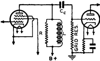
FIG. 23-22. — Resistance-impedance audio-frequency coupling system.
