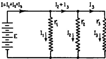
FIG. 21-3. — Three resistances connected in parallel with each other and across a source of voltage,  $E$ . The total current,  $I$ , divides, part of it flowing through the path presented by each resistor.
