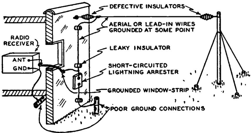
FIG. 18-1.—Places in a typical outdoor antenna system where trouble is likely to occur.
