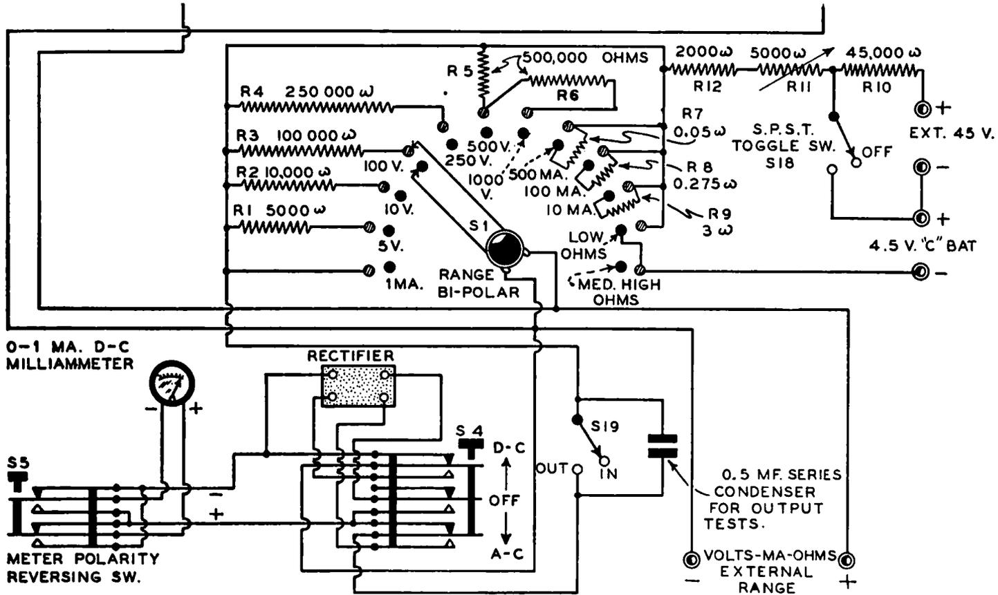
FIG. 13-1.—Schematic circuit diagram (in two parts) of the complete set analyzer described in this chapter.
