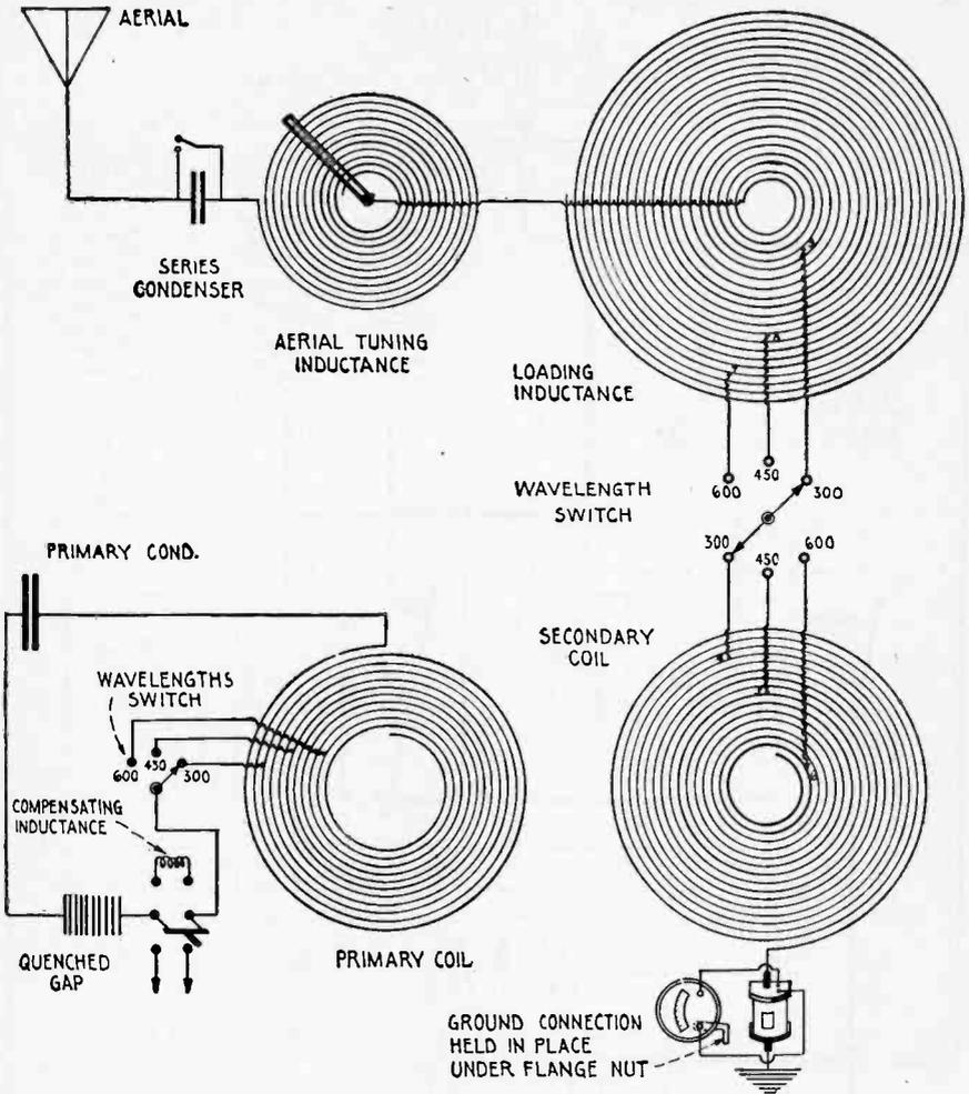
Fig. 256—Radio Frequency Circuits of the 1/2 K. W. 500 Cycle Transmitter.
