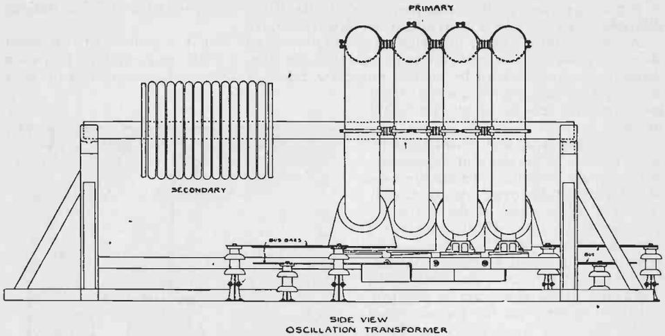
Fig. 316—Side View of 300 Kilowatt Oscillation Transformer.
