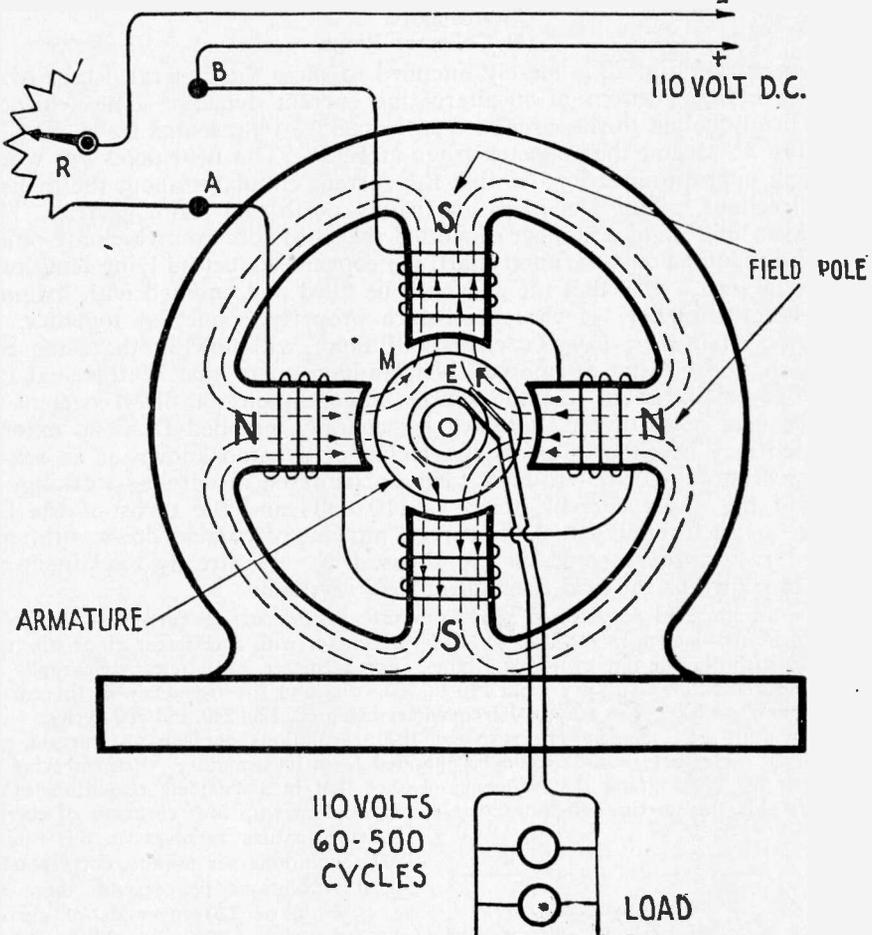
Fig. 23—Fundamental Diagram of 4 Pole A. C. Generator.
