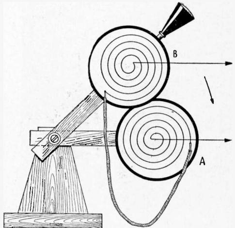
Fig. 123—Showing Fundamental Principle of the Variometer.
