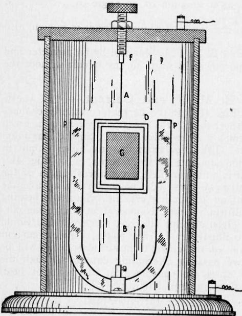
Fig. 46—Simple Galvanometer.
