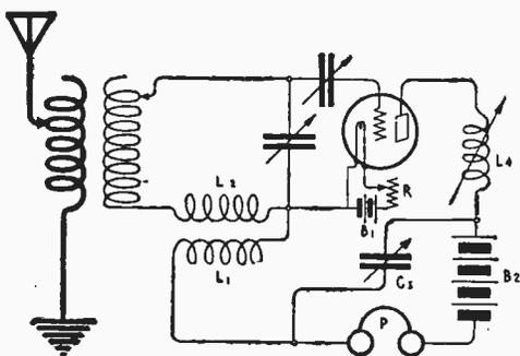
Fig. 182—Audio-Frequency Repeater Circuit. Fig. 183—Tuned Regenerative Vacuum Valve Circuit.
