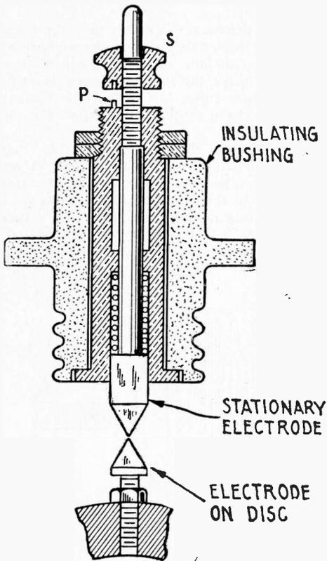
Fig. 252—Showing How the Stationary Electrodes of the Marconi Synchronous Gap are Adjusted.
