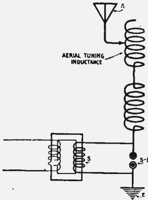
Fig. 327—Method for Determining Leakage in Aerial Insulators.
