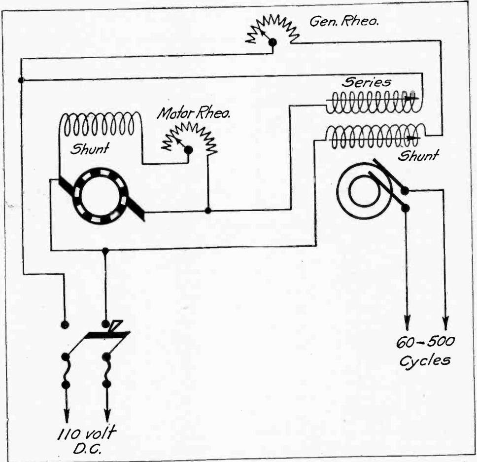
Fig. 65—Motor Generator with Compound Generator Field Winding.
