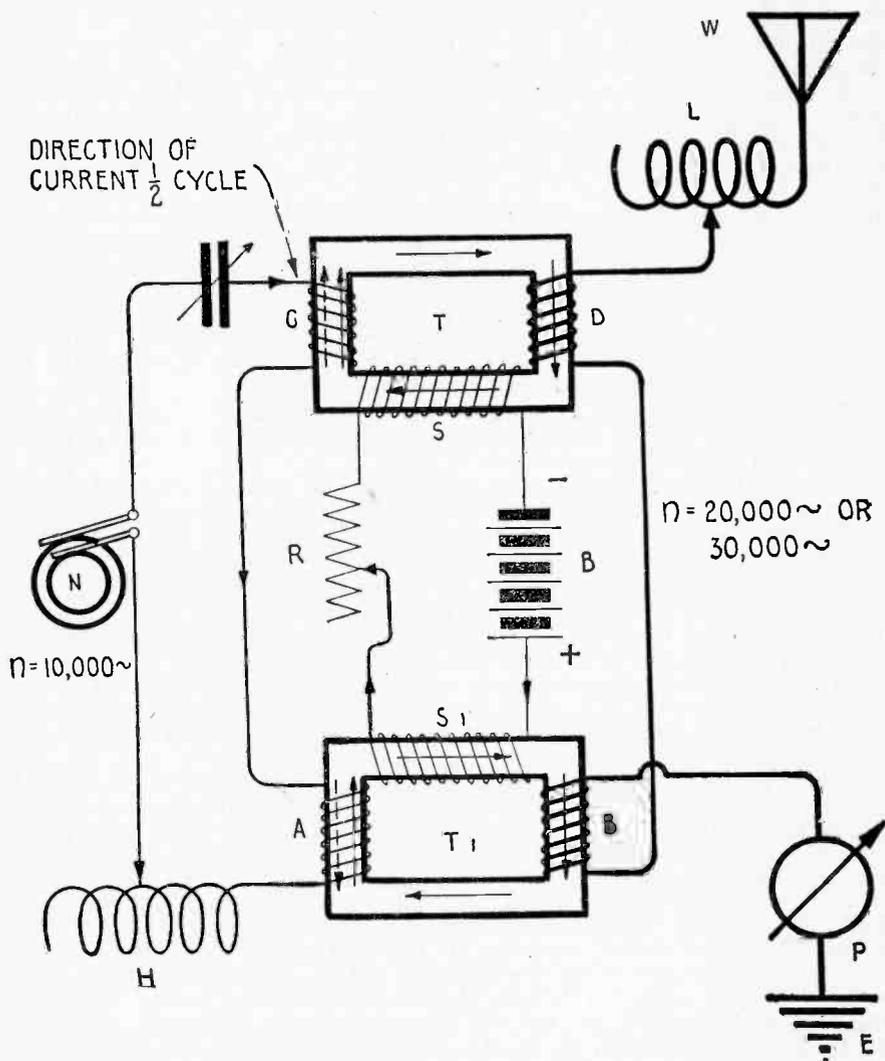
Fig. 284—The Joly-Arc Undamped Wave Transmitter.
