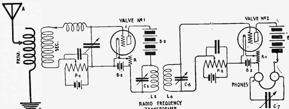
Fig. 187—Circuit for Cascade Amplification of Radio Frequencies.
