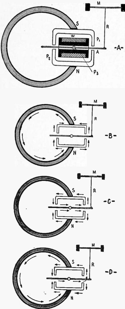
or isinglass diaphragm M which is screwed under the receiver cap as in the ordinary telephone. During the passage of a fluctuating current through the winding W the soft iron armature A is thrown into vibratory motion and the vibrations transferred to M. *A prominent feature of this receiver is the fact that the armature A is under no magnetic strain until a fluctuating current flows through the winding W.*
