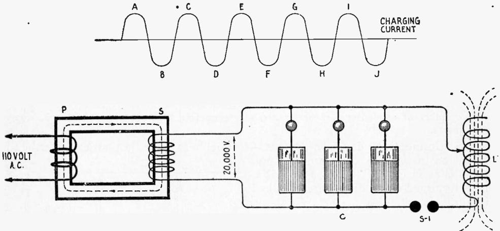
Fig. 93.—Apparatus for Production of Radio Frequency Oscillations.
