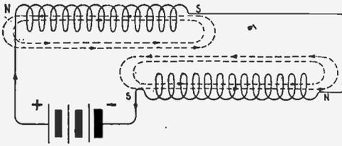
Fig. 18—Variation of Magnetic Field by Opposing Coils.
