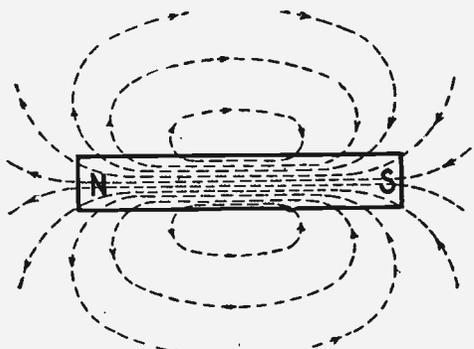
Fig. 1.—Field of a Simple Bar Magnet.
