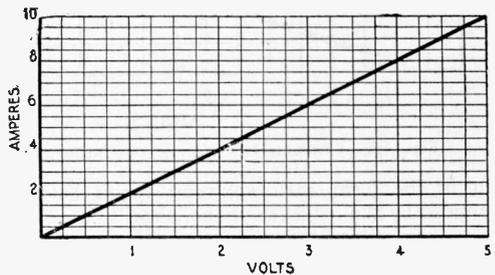
Fig. 155—Characteristic Curve of Ordinary Resistance.
