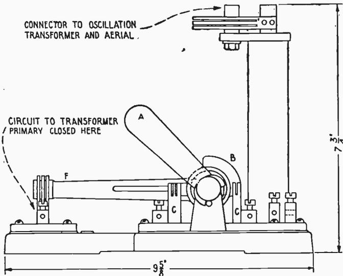
Fig. 200b—Elevation of Type I Aerial Changeover Switch.
