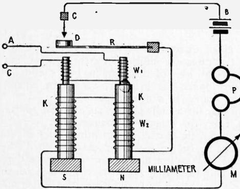
Fig. 197a—Brown Amplification Relay for Increasing Radio Signals.
