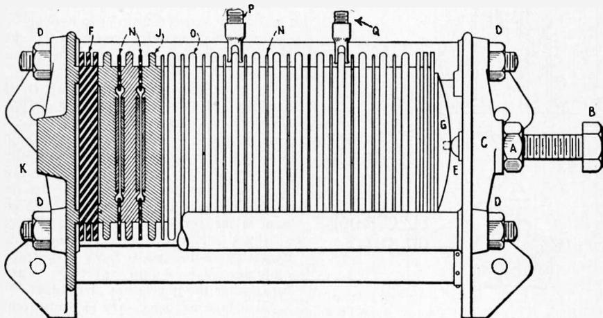
Fig. 253—Detailed Sketch of Marconi Quenched Spark Gap.
