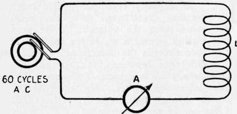
Fig. 43—Alternating Current Circuit with Concentrated Inductance.
