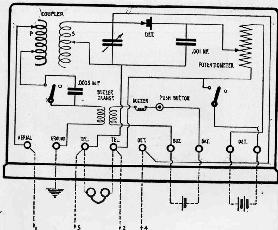
WIRES 1,2,4,5 CONNECT TO TYPE I AERIAL SWITCH
