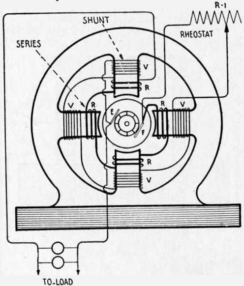
Fig. 27—Circuit of Compound Wound D. C. Generator.
