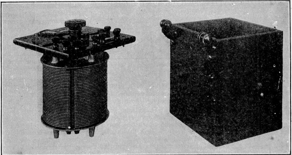
Fig. 147a—Variable Condenser for Receiver Circuits.
