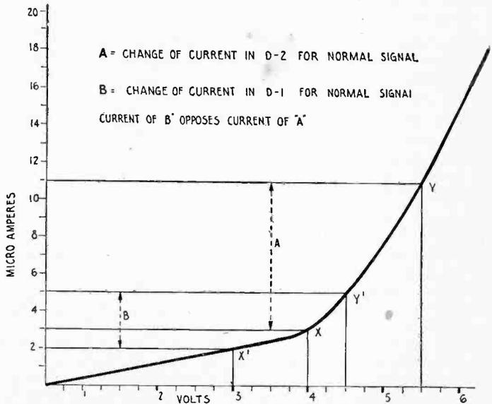
Fig. 199—Curve Showing Principle of Balanced Crystal Receiver.
