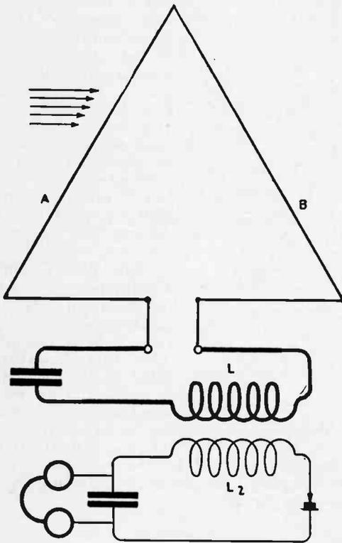
Fig. 274—Receiver Connected to a Single Loop Aerial.
