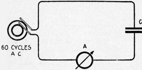
Fig. 44—Alternating Current Circuit with Condenser in Series.
