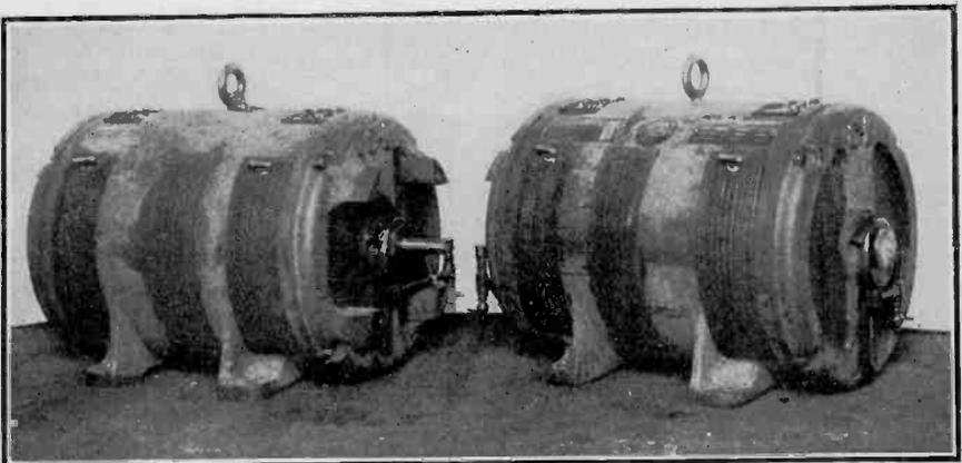
Fig. 67b—2 K. W. Crocker-Wheeler Motor Generator Assembled.
