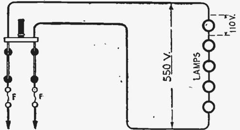
Fig. 61.—Lamps in Series on 550 Volts Circuit.
