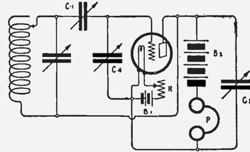
Fig. 184—Simple Regenerative Circuit.
