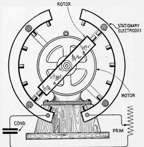
Fig. 114—Another Type of Non-synchronous Discharger.
