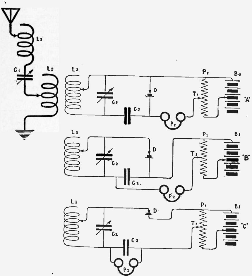
Fig. 153a, b, c—Complete Circuit for the Carboredum Rectifier and Receiving Tuner.
