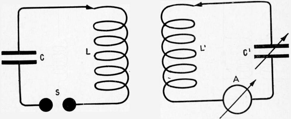
Fig. 96—Circuits for Demonstrating the Phenomenon of Resonance.
