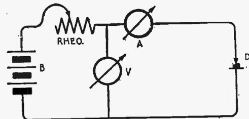
Fig. 156—Apparatus for Determining Volt-ampere Characteristic of Carborundum Rectifier\*
