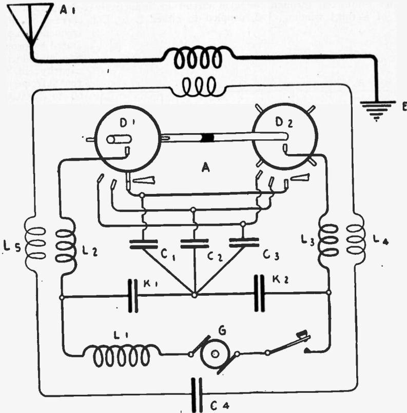
Fig. 287—One Type of Marconi Continuous Wave Generator.
