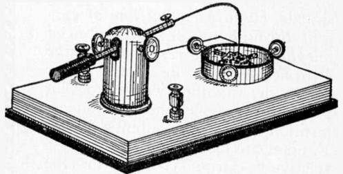
Fig. 160—Detector Holder for Galena and Silicon Crystals.
