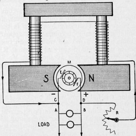
Fig. 25—Circuit of Shunt Wound D. C. Generator.
