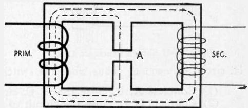
Fig. 133—Closed Core Transformer with Magnetic Leakage Gap.
