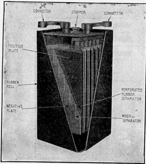
Fig. 86a—Detail of Exide 11 M. V. Storage Cell.
