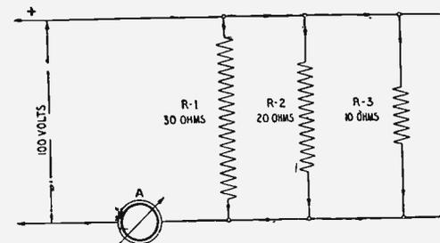
The current in the branches of the divided circuit, Fig. 10, can be determined by finding the voltage across the terminals of each branch, and dividing the result by the resistance of each branch.
