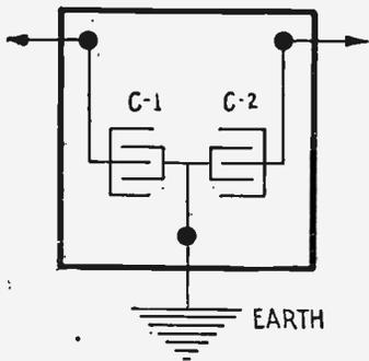
Fig. 77—Protective Condensers.
