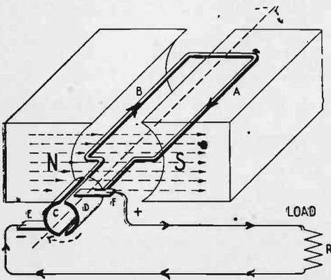
Fig. 24.—Showing the Function of a Simple Commutator.
