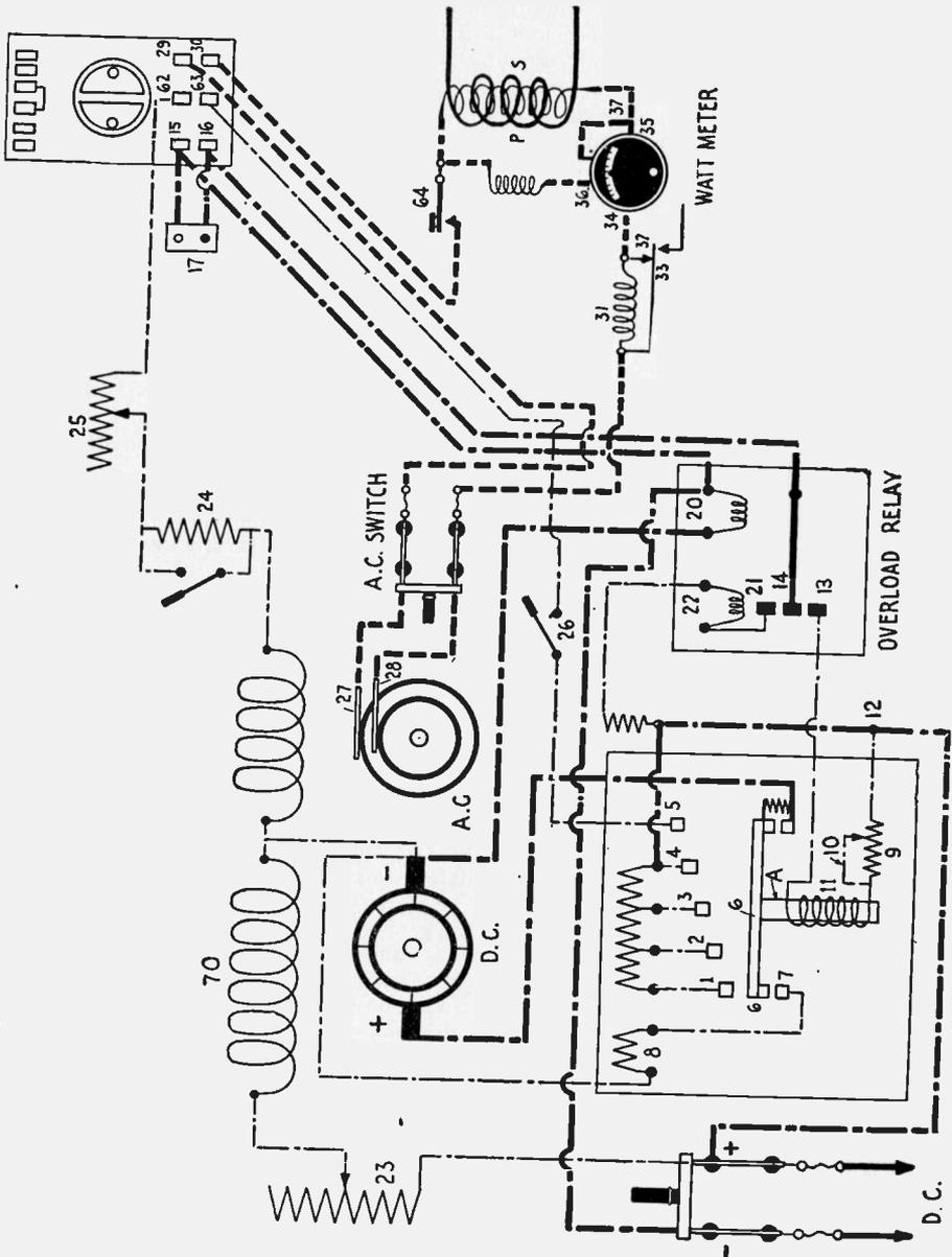
Fig. 75a—Complete Circuit Diagram of Automatic Starter and Motor Generator of the Marconi 2 K. W. 500 Cycle Set.
