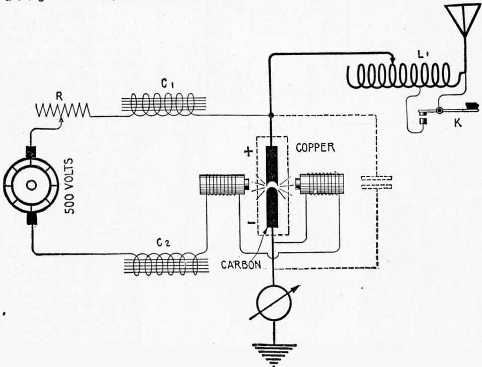
Fig. 279—Complete Circuits of a Modern Arc Transmitter.
