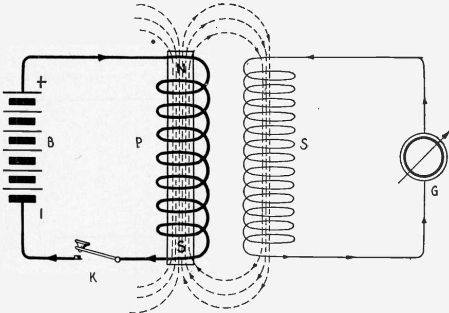
Fig. 19—Diagram Illustrating the Principle of Electromagnetic Induction.
