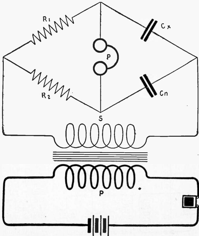
Fig. 227—Diagram for the Measurement of Electrostatic Capacity.
