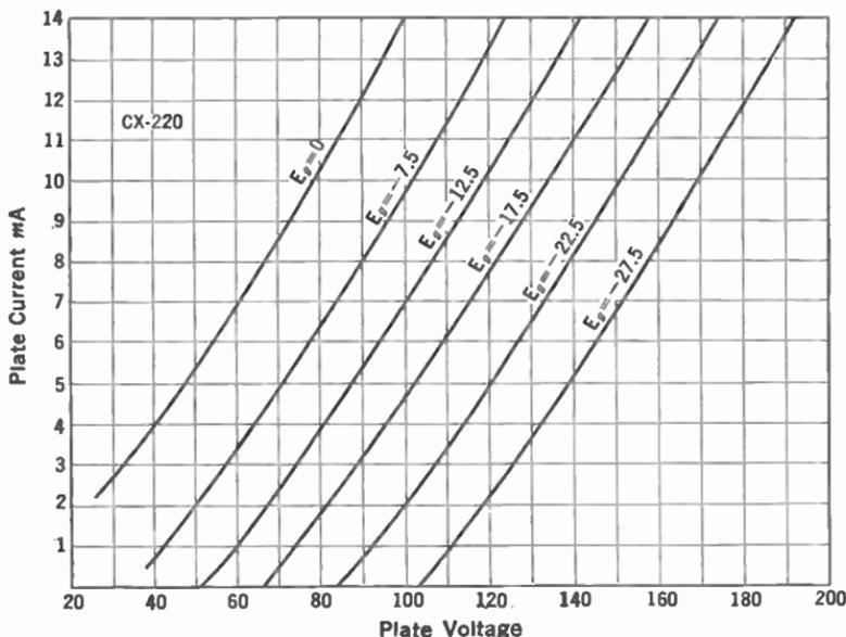
Fig. 120.—Plate current—plate voltage curves.
