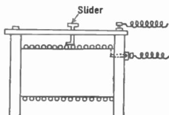
FIG. 58.—An early form of variable inductance for radio purposes called a "single slide tuning coil."
