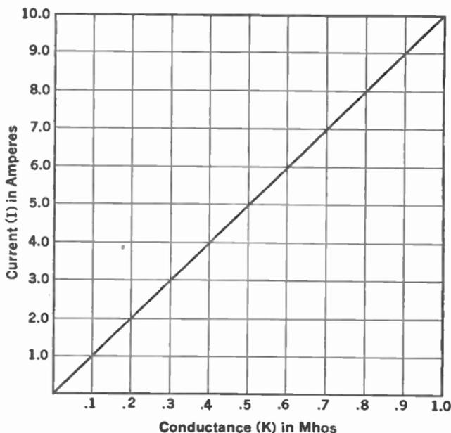
FIG. 15.—Conductance  $\left(\frac{1}{R}\right)$  plotted against current.
