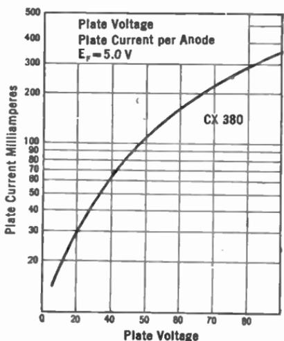
FIG. 242.—Characteristic of double wave rectifier tube.
