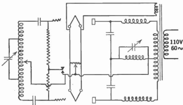
FIG. 288.—Full-wave self-rectified oscillator operated entirely from a.c.
