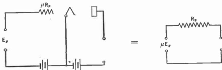
Fig. 122.—The tube and its equivalent circuit; a voltage  $\mu E_p$  in series with  $R_p$  and the load.
