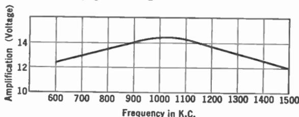
FIG. 215.—Amplification-frequency characteristic of r-f. amplifier in Radiola 60—gain per stage
