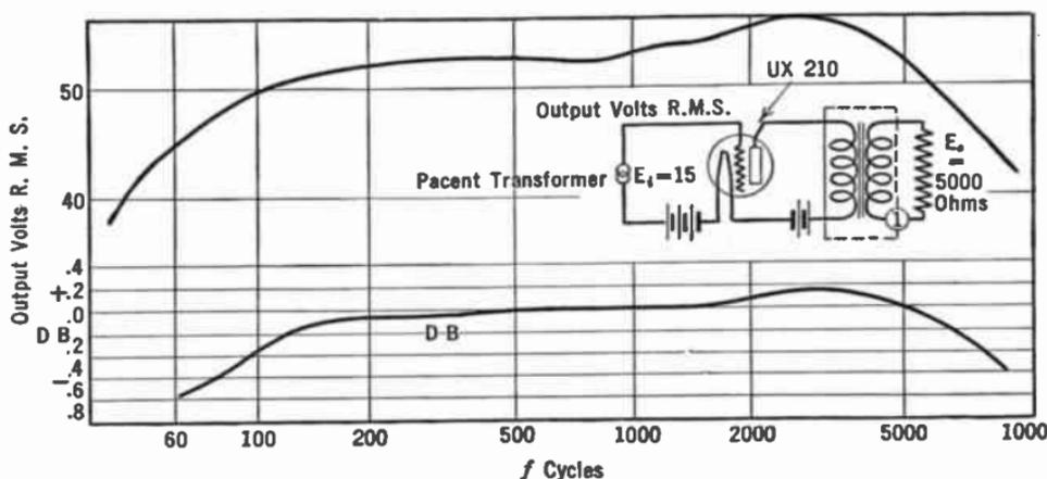
FIG. 169.—Transmission characteristic of output transformer.
