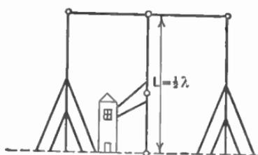
FIG. 301.—Half-wave vertical antenna.
