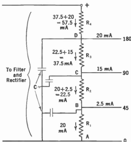
FIG. 261.—Designing the voltage divider.
