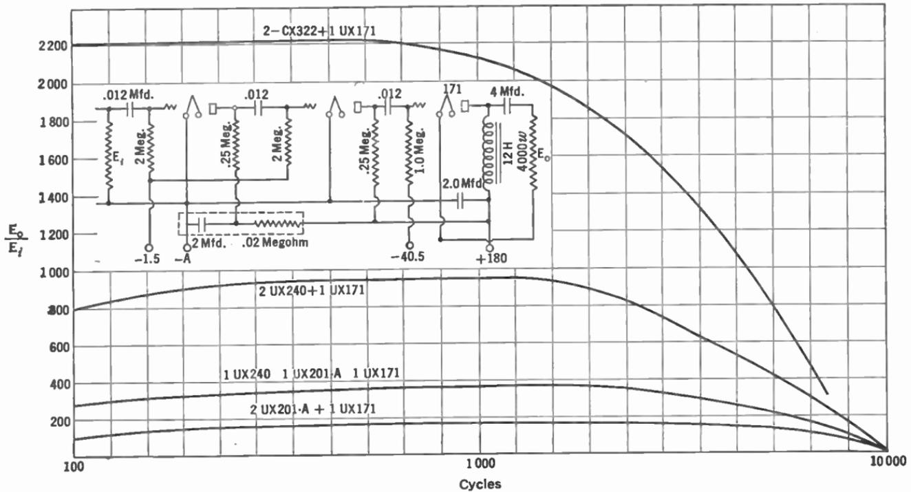
FIG. 180.—Circuit and characteristic of resistance coupled amplifier. The dotted part of the circuit is an "anti-motor-boating" device.
