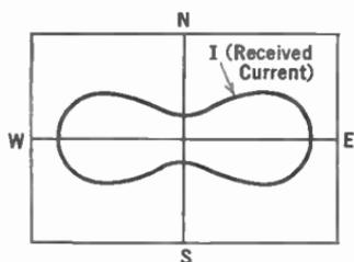
FIG. 303.—Directional effect of reception on a loop.
