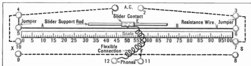
FIG. 33.—A single slide wire bridge.
