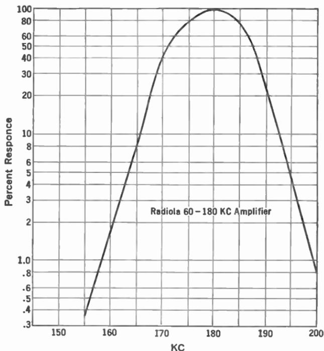
FIG. 216.—Response of intermediate frequency amplifier of Radiola 60.
