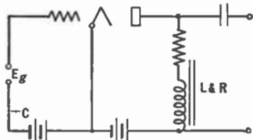
FIG. 154.—Inductance-capacity or "impedance" coupled amplifier.
