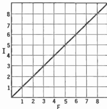
FIG. 13.—In an Ohm's law circuit plotting current against voltage results in a straight line.
