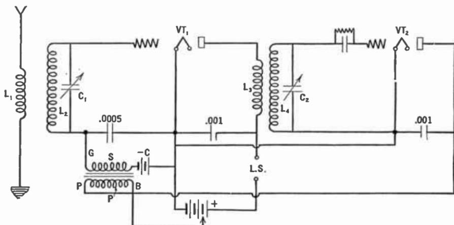
FIG. 160.—A reflex circuit.  $VT_1$  amplifies both at low and high frequencies.
