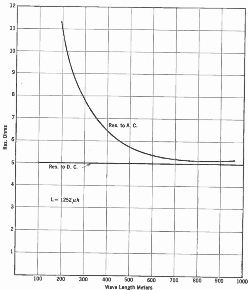
Fig. 102.—High-frequency resistance of a coil.
