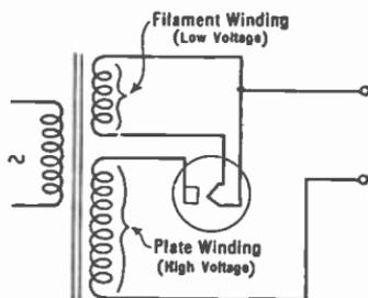
FIG. 238.—Operating rectifier filament from a. c.
