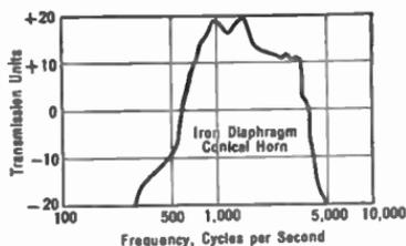
FIG. 234.—Limited response of horn speaker.
