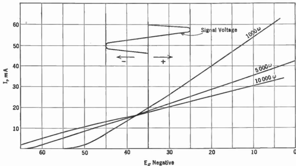
FIG. 164.—Flattening effect of increasing load resistance.
