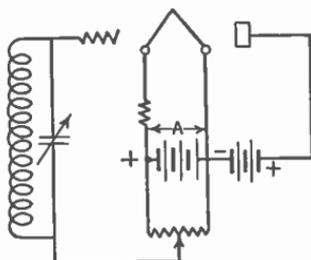
FIG. 194.—Potentiometer method of controlling oscillations.
