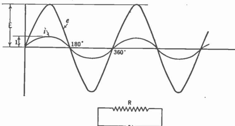
FIG. 74.—Current and voltage in phase.
