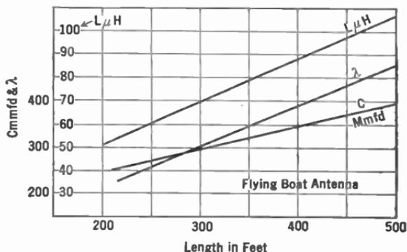
FIG. 305.—Characteristics of airplane antenna.
