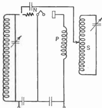
FIG. 197.—Hazeltine neutralized circuit.
