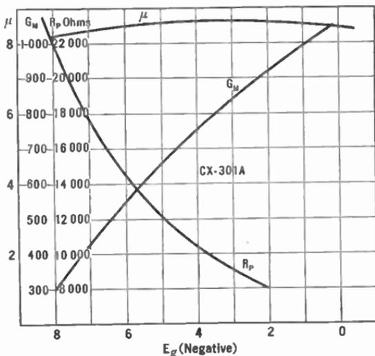
Fig. 124.—Effect of grid voltage on tube characteristics.
