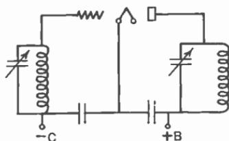
FIG. 192.—Tuned plate-tuned grid circuit.
