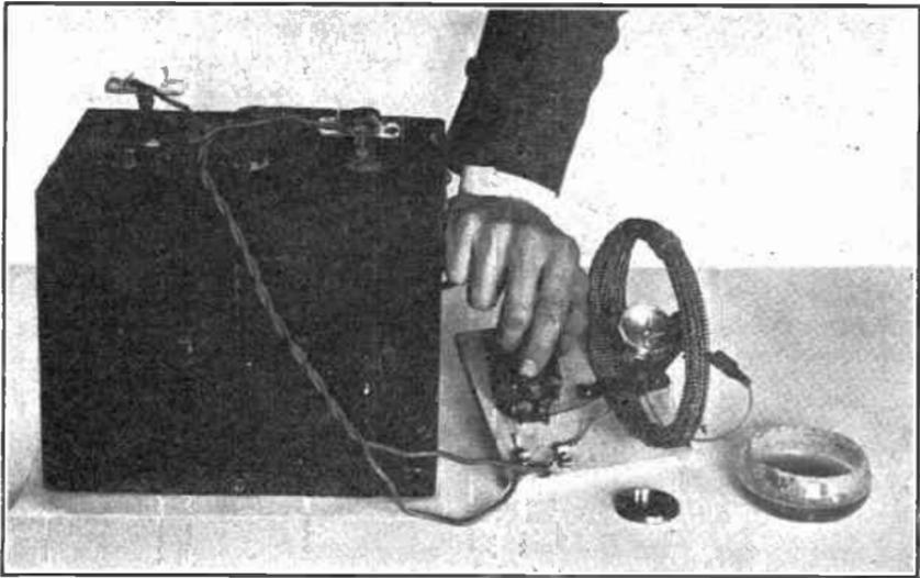
FIG. 26(a).—A simple form of galvanometer. When a current flows through the coil of about 25 turns, a magnetic field is created which effects the position of the needle.
