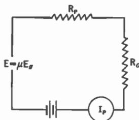
Fig. 143.—Equivalent circuit of amplifier tube.
