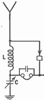
FIG. 104.—A simple radio receiver.
