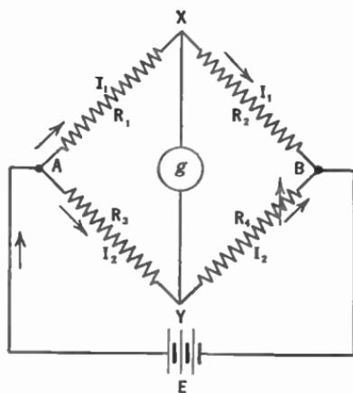
FIG. 32.—Wheatstone bridge for measuring resistance.
