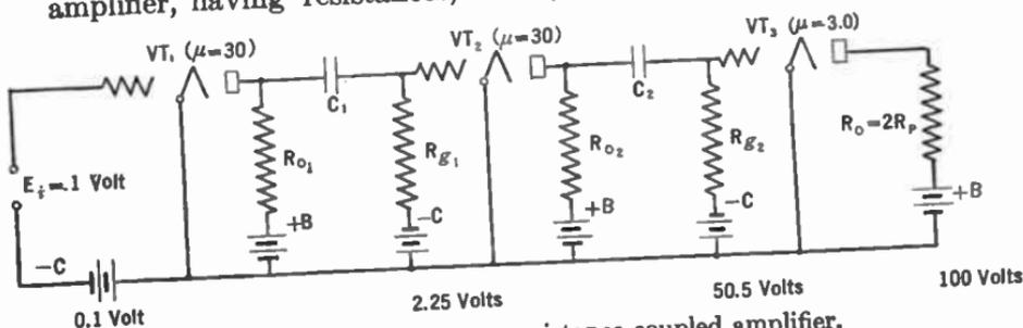
FIG. 153.—Three stage resistance coupled amplifier.
