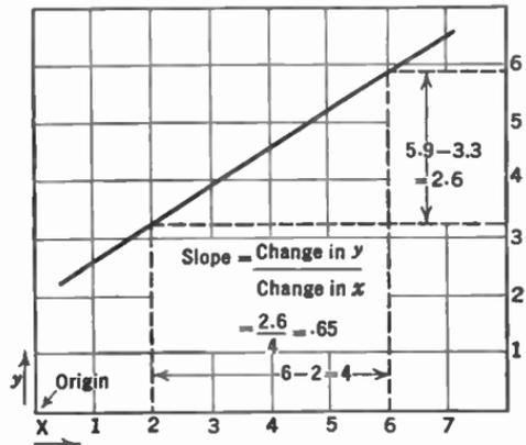
FIG. 6.—How to calculate the shape of a curve.
