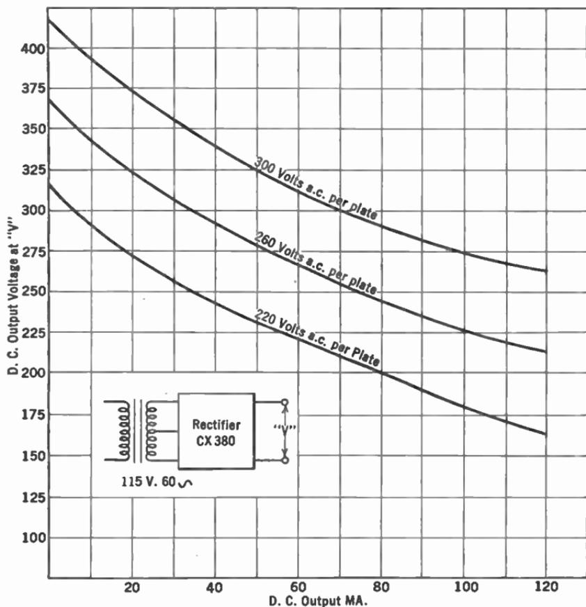
FIG. 7.—A "B eliminator" regulation curve.
