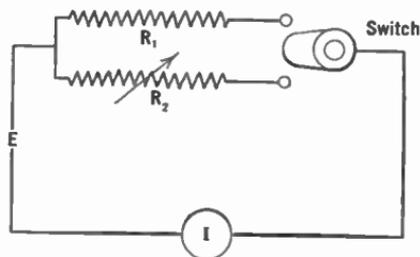
FIG. 31.—Measuring resistance by comparison.
