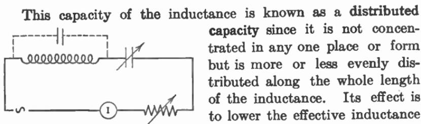
FIG. 103.—When the dotted capacity across the coil tunes it to the frequency of the generator, the series impedance of the circuit becomes very high.
