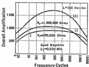
FIG. 157.—Frequency characteristic of resistance- and inductance-coupled amplifiers.
