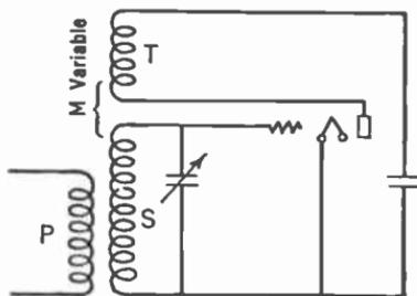
FIG. 191.—A simple regenerative circuit.
