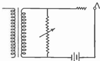
FIG. 167.—Shunt resistance volume control.
