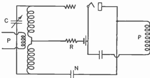
FIG. 195.—Rice neutralized circuit.
