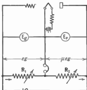
Fig. 125.—Bridge for determining amplification factor.
