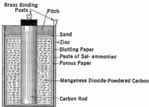
FIG. 36.—Construction of dry cell.
