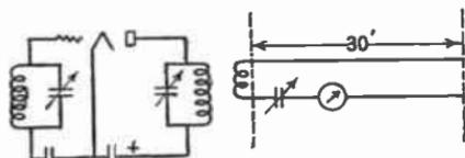
FIG. 299.—Experimental diagram to demonstrate existence of radiation resistance.
