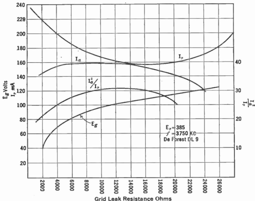
FIG. 281.—Effect of varying grid leak resistance.
