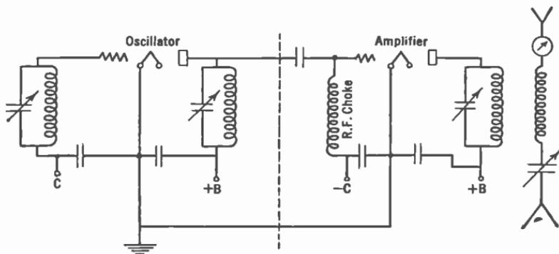
FIG. 283.—Master oscillator-power amplifier transmitting circuit.
