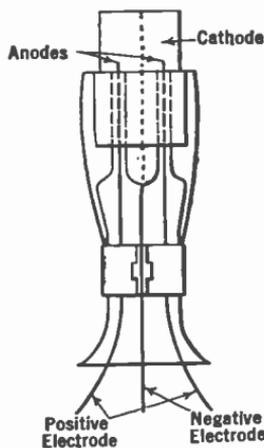
FIG. 247.—Raytheon tube construction.
