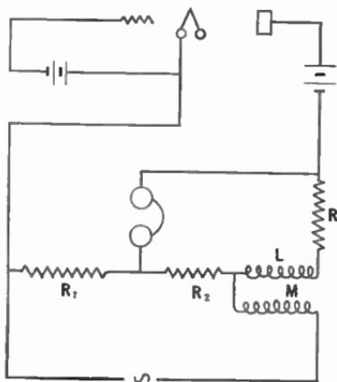
Fig. 127.—A bridge for measuring  $R_p$ .
