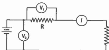
FIG. 29.—Ammeter-voltmeter method of measuring resistance.
