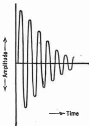
FIG. 264.—Highly damped series of waves.
