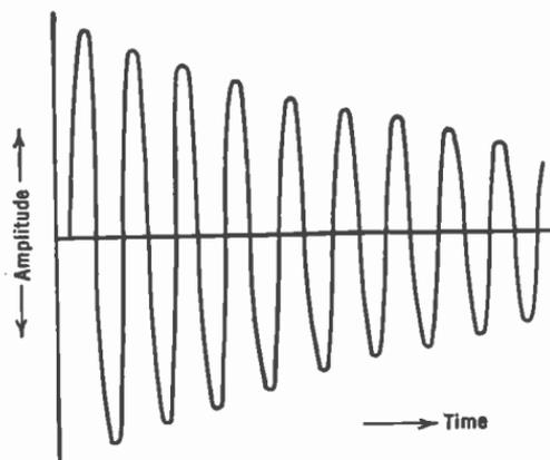
FIG. 265.—Slightly damped (low resistance circuit) waves.
