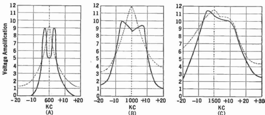
FIG. 225.—Quantitative data on band pass amplifier-tube and tuned coils. The dotted curves are of a single coil properly tuned.
