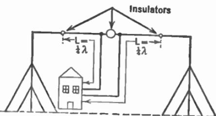
FIG. 302.—Folded half-wave antenna.
