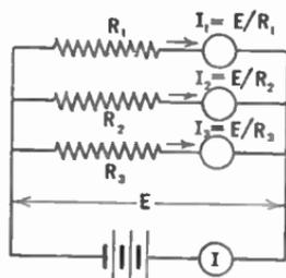
FIG. 21.—A parallel circuit.
