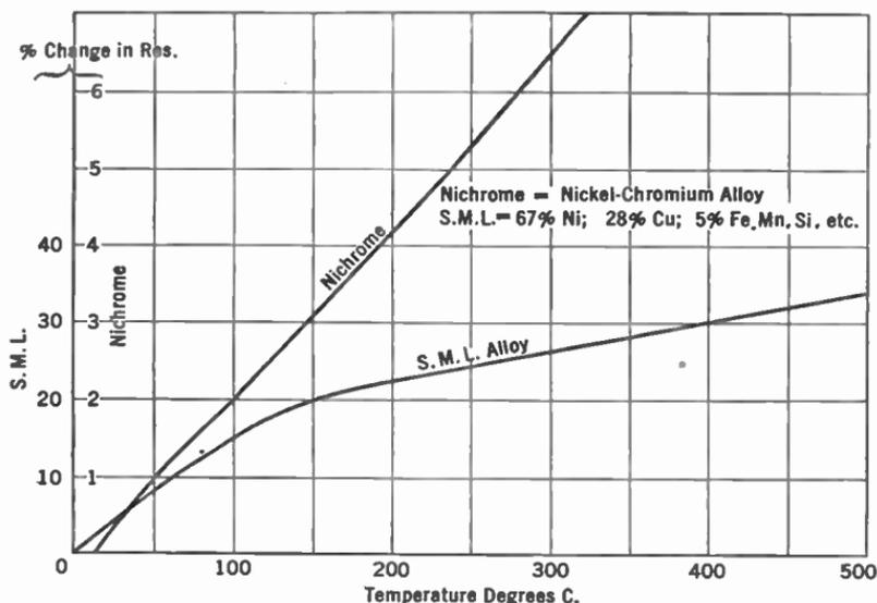
FIG. 3.—Effect of temperature on resistance.
