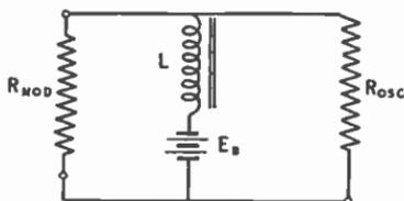
FIG. 294.—Equivalent of Heising modulation system
