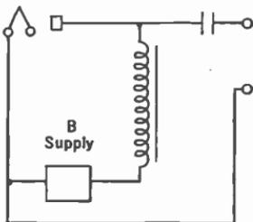
FIG. 171.—In this output connection, loud-speaker currents return to the filament directly.
