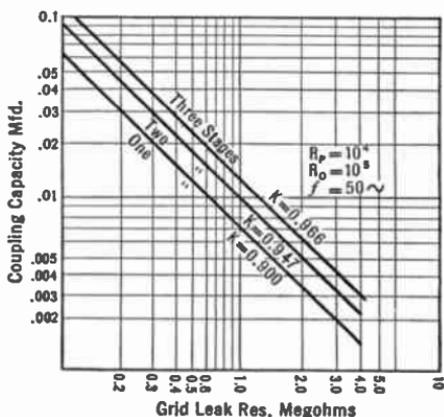
FIG. 152.—Relation between grid leak resistance, coupling capacity and efficiency ( $K$  or  $N$ ).
