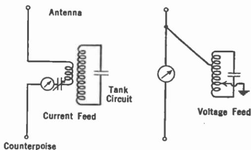
FIG. 292.—Current feed and voltage feed antenna circuits.
