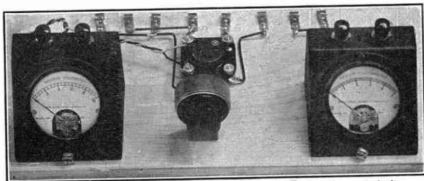
Fig. 115.—An experimental set-up for measuring tube characteristics.
