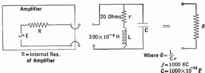
FIG. 97.—A high impedance is desired for the amplifier to work into. A tuned circuit does the trick. Numerically it is equal to  $Z$ .
