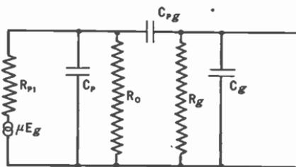
FIG. 155.—Equivalent circuit at high frequencies of resistance-capacity coupled tubes.
