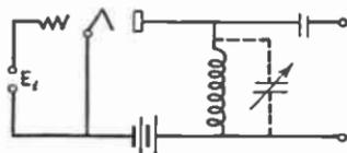
FIG. 158.—Tuned inductance output.
