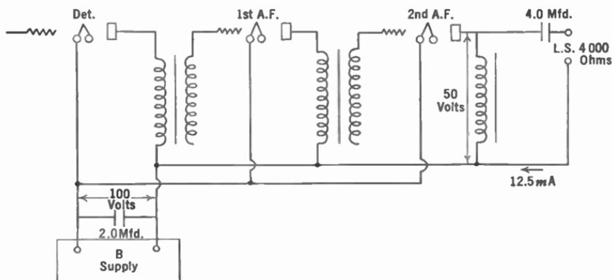
FIG. 175.—Regeneration in audio amplifiers is caused by forcing a.-c. currents through the impedance of the B supply.
