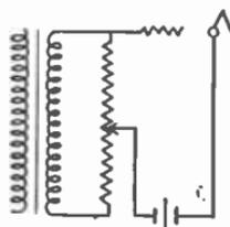
Fig. 168.—Potentiometer gain or volume control.
