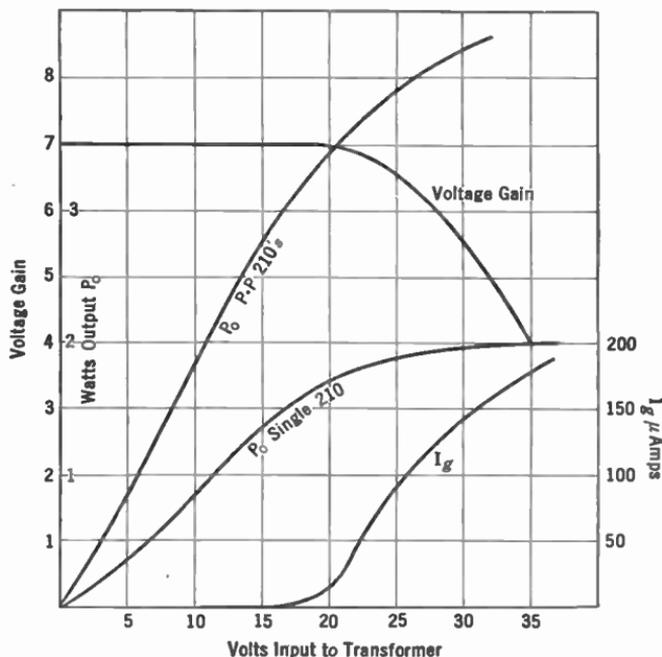
FIG. 179.—Comparison of single and pushpull tube amplifiers.
