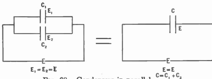
FIG. 68.—Condensers in parallel.
