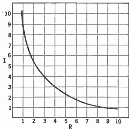
FIG. 14.—The result of plotting current against resistance.
