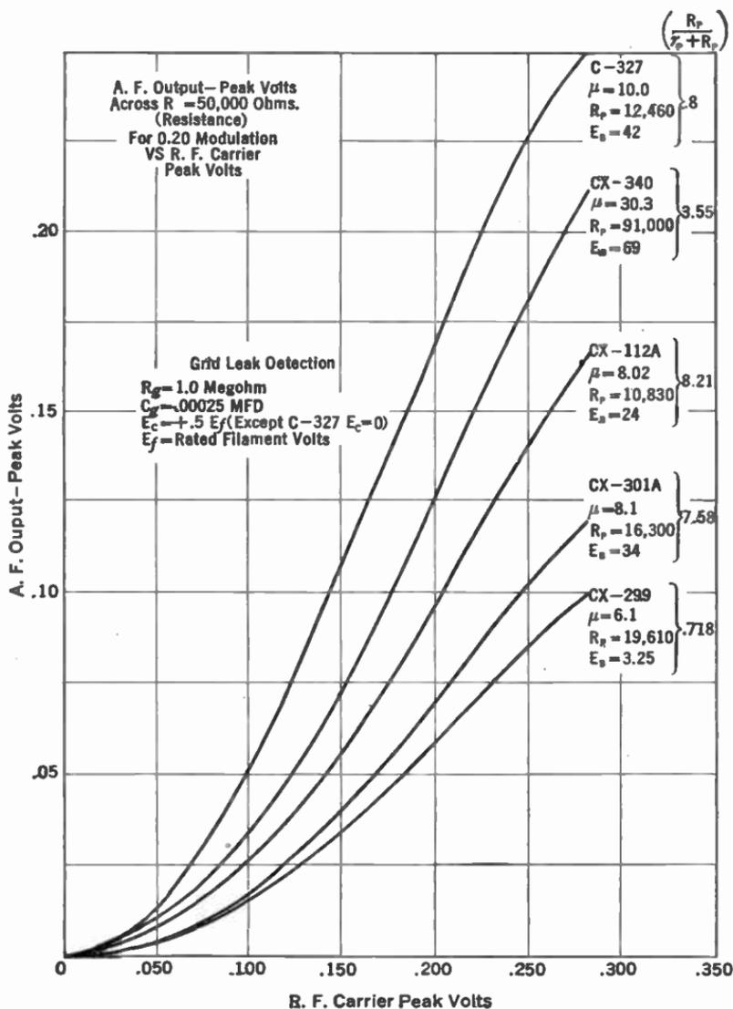
FIG. 211.—Comparison of various tubes as grid leak detectors.
