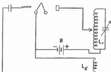
FIG. 289.—Maximum power is obtained by adjusting tap until tube works into its own impedance.
