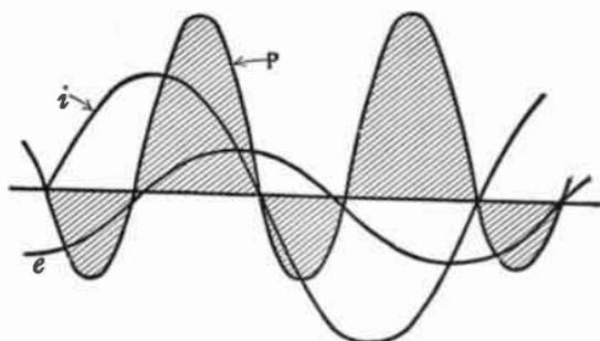
FIG. 87.—Power in a capacitive circuit.
