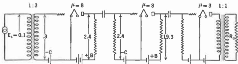
FIG. 163.—A combination transformer and resistance coupled amplifier.
