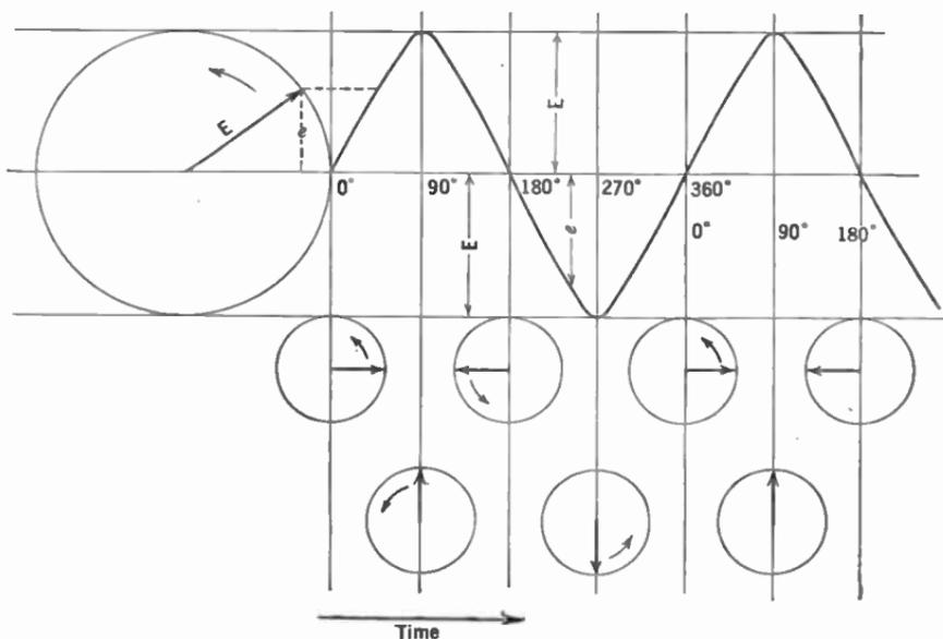
FIG. 70.—As the vector  $E$  rotates, the circle moves to the right. A piece of crayon attached to the end of the vector would trace out a curve similar to the wavy line. When the vector has the position as shown in the first small circle, the instantaneous value  $e$  is zero. At other times the instantaneous voltage has some other value.
