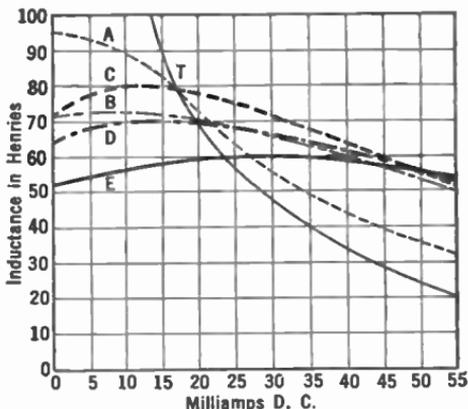
FIG. 62.—Variation of inductance with air gap.
