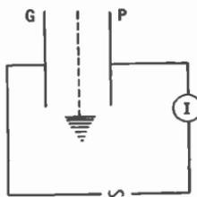
Fig. 136.—Capacity current from grid to plate is nullified by grounded shield or screen.
