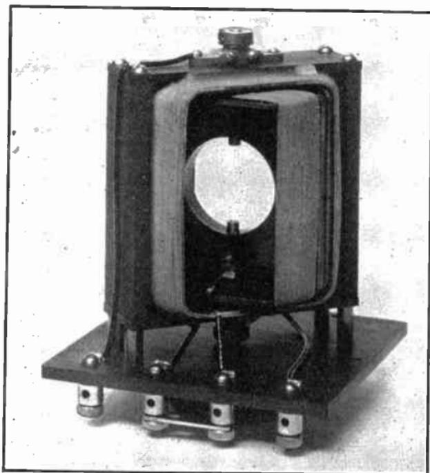
FIG. 59.—General Radio Company variable inductance.
