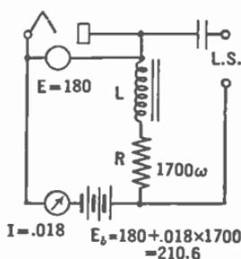
FIG. 10.—A choke-condenser coupling circuit.
