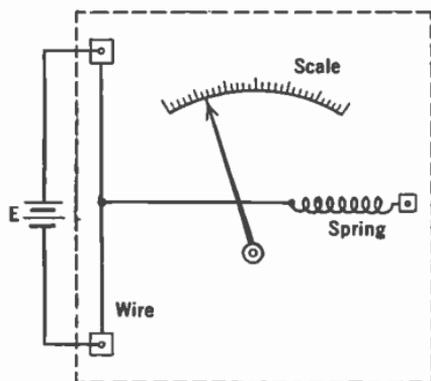
FIG. 25.—Hot wire ammeter.
