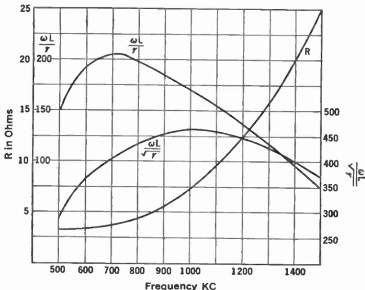
FIG. 186.—How resistance and figure of merit “ $Q$ ”  $\left(\frac{\omega L}{r}\right)$  of a coil vary with frequency.
