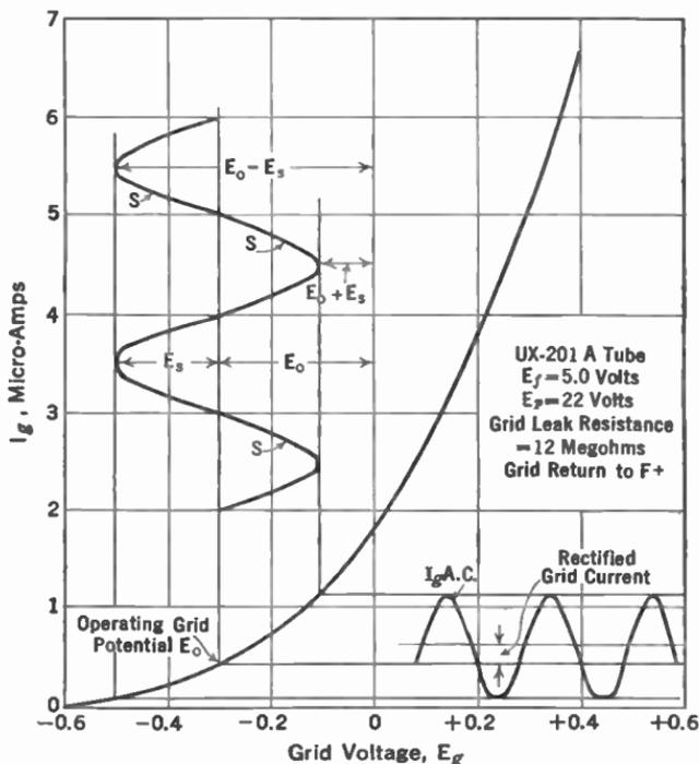
FIG. 208.—Rectification on the grid voltage-grid current curve.
