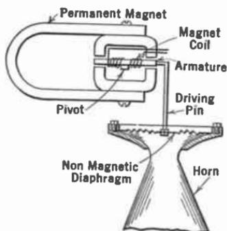
FIG. 231.—Horn type speaker mechanism.
