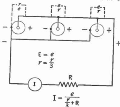
FIG. 39.—Cells in parallel.
