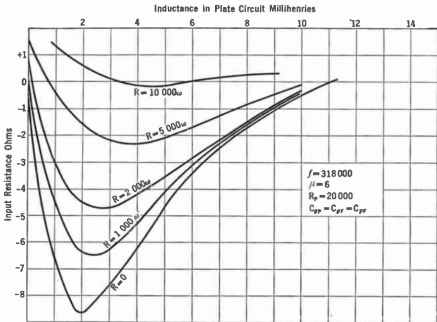
FIG. 184.—Dependence of input resistance upon inductive load.
