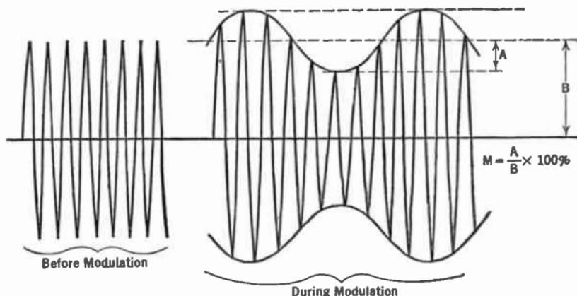
FIG. 201.—Unmodulated and modulated wave.
