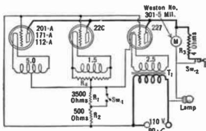
Fig. 129.—An a.-c. tube-tester.
