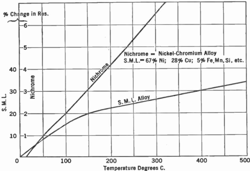
FIG. 3.—Effect of temperature on resistance.
