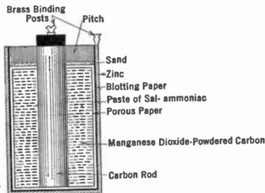
FIG. 36.—Construction of dry cell.
