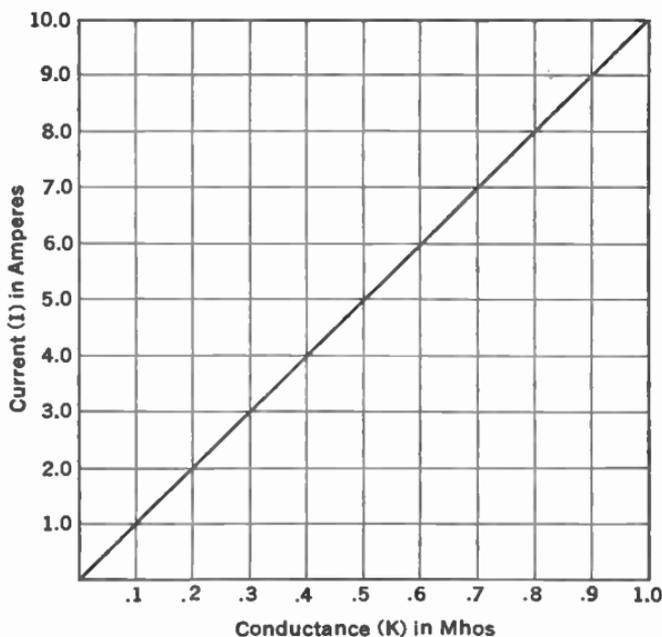
FIG. 15.—Conductance  $\left(\frac{1}{R}\right)$  plotted against current.
