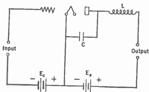
FIG. 204.—To keep radio-frequency currents from the output, a low impedance path ( $C$ ) and a high series impedance ( $L$ ) are used.
