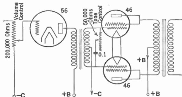
FIG. 224.—Tone control across input to power amplifier.
