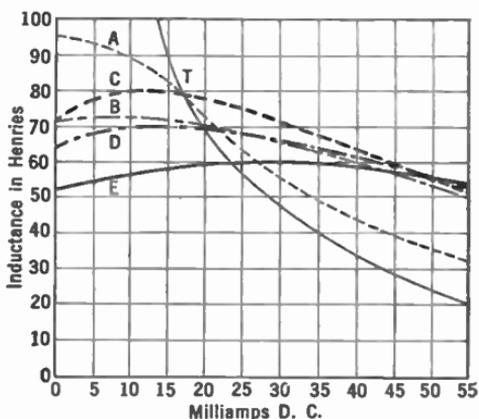
FIG. 62.—Variation of inductance with air gap.
