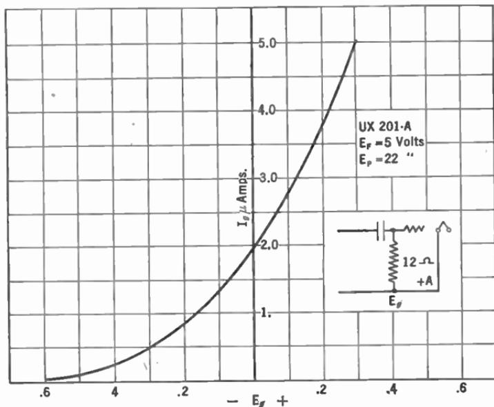
FIG. 119.—Grid current curve of a three-element tube.
