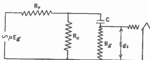
FIG. 151.—Equivalent circuit of Fig. 150.
