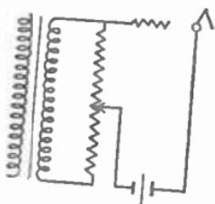
FIG. 167.—Potentiometer gain or volume control.
