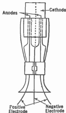
FIG. 247.—Raytheon tube construction.
