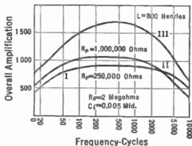
FIG. 157.—Frequency characteristic of resistance- and inductance-coupled amplifiers.
