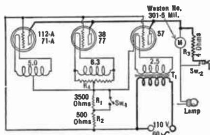
Fig. 129.—An a.-c. tube-tester.
