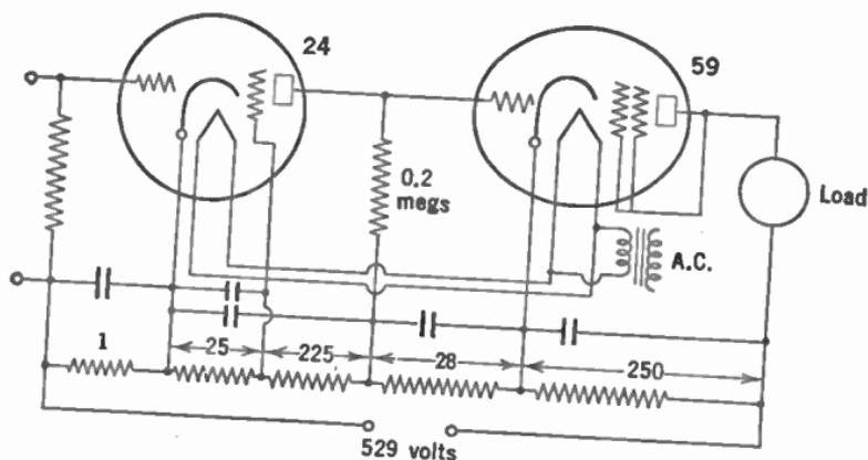
FIG. 180a.—Simple direct-coupled amplifier.
