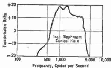
FIG. 234.—Limited response of horn speaker.
