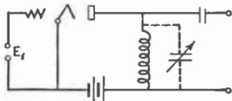
FIG. 158.—Tuned inductance output.
