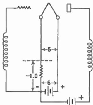
Fig. 133.—Obtaining grid bias by means of filament-current flowing through a resistance.
