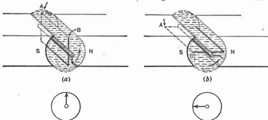
FIG. 45.—In (a) the conductor *AB* is moving parallel or along the lines of force. In (b) the conductor is moving across or at right angles to the lines. At (a) the generated voltage is zero; at (b) it is a maximum.
