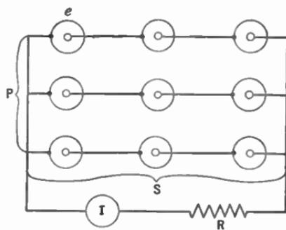
FIG. 40.—Cells in series-parallel.
