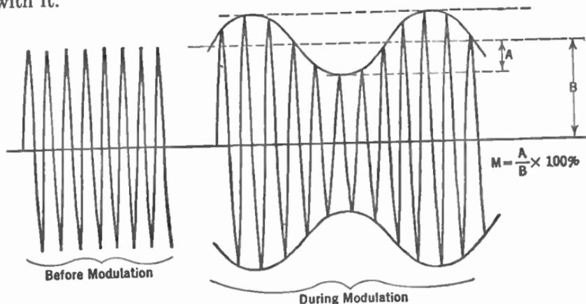
FIG. 201.—Unmodulated and modulated wave.
