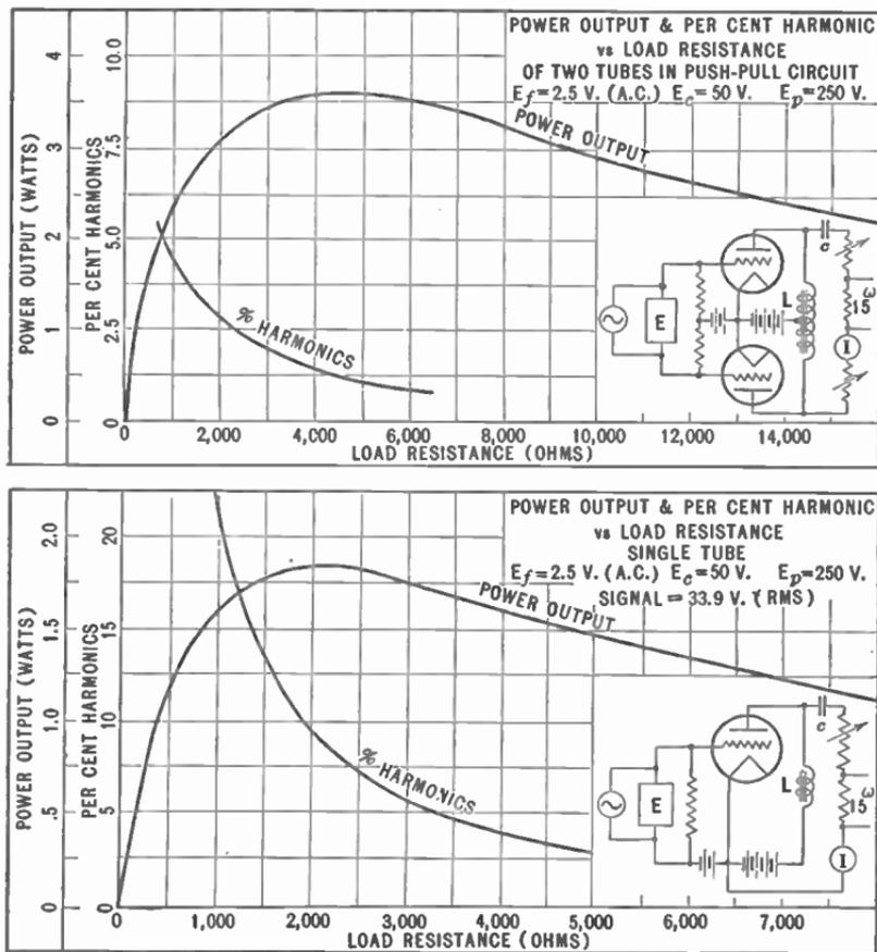
Fig. 178.—Demonstration of advantages of push-pull tubes.
