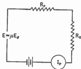
Fig. 143.—Equivalent circuit of amplifier tube.
