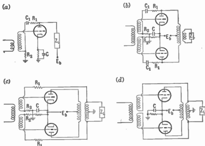
FIG. 179.—Negative feedback circuits.
