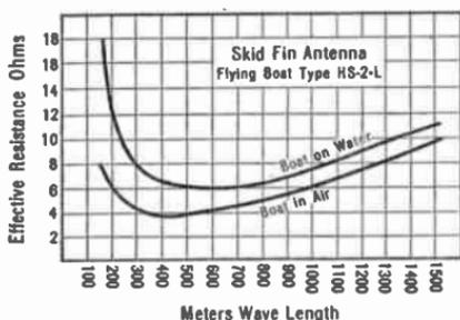
FIG. 300.—Antenna resistance.
