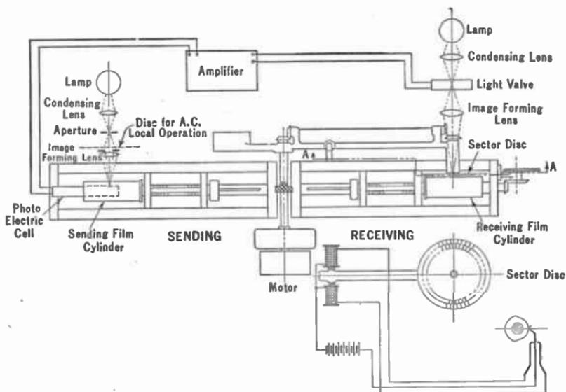
FIG. 308.—Bell system of photograph transmission.
