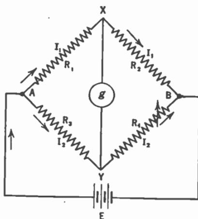
FIG. 32.—Wheatstone bridge for measuring resistance.
