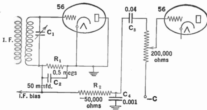
FIG. 211.—Typical diode detector circuit.
