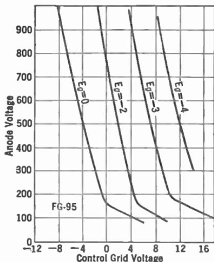
FIG. 262.—Characteristics of shield-grid thyratron. Note that various starting voltages are possible, dependent upon voltage of shield grid.
