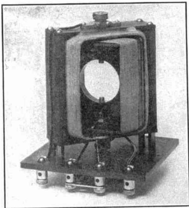
FIG. 59.—General Radio Company variable inductance.
