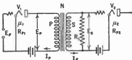
FIG. 159.—Transformer coupled amplifier
