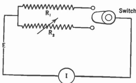
FIG. 31.—Measuring resistance by comparison.
