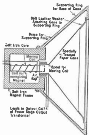
Fig. 233.—Modern "dynamic" or moving coil loud speaker.
