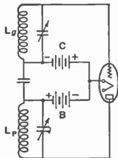
FIG. 276.—Practical Colpitts circuit.
