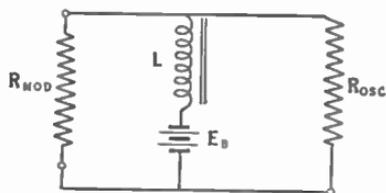
FIG. 294.—Equivalent of Heising modulation system.
