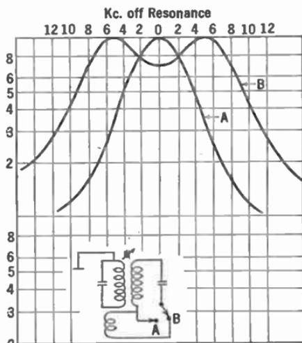
FIG. 227.—Selectivity curve for two-position i.-f. transformer (RCA).
