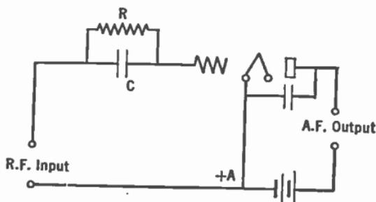
FIG. 207.—Grid leak-grid condenser detector.
