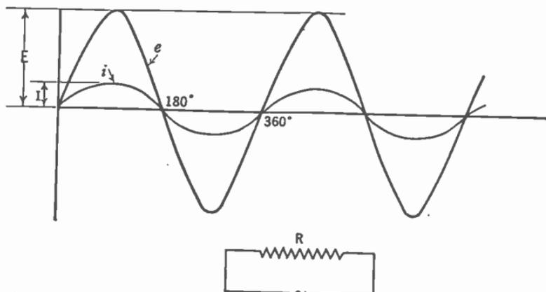
FIG. 74.—Current and voltage in phase.
