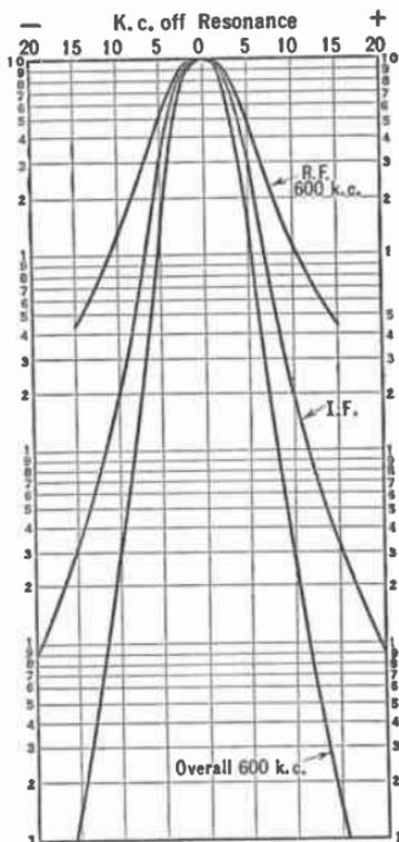
FIG. 216.—Response of modern superheterodyne.
