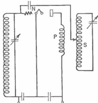
FIG. 196.—Hazeltine neutralized circuit.
