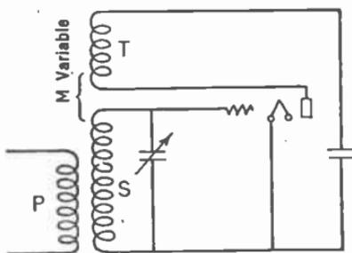
FIG. 192.—A simple regenerative circuit.
