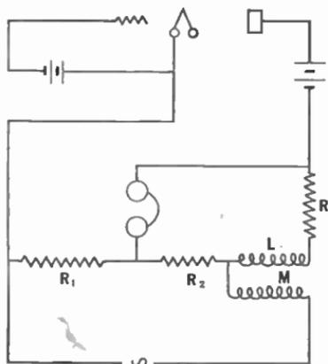
Fig. 127.—A bridge for measuring  $R_p$ .
