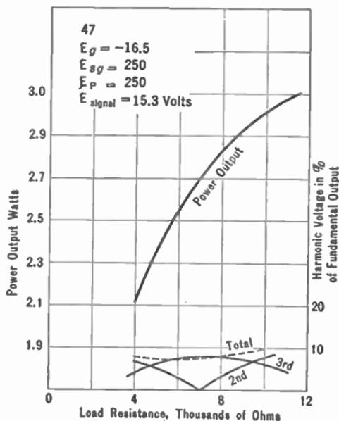
FIG. 149.—Pentode output characteristics.
