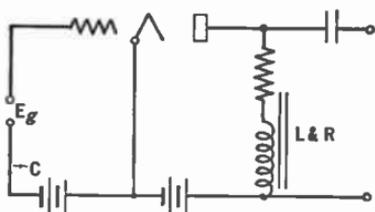
FIG. 154.—Inductance-capacity or "impedance" coupled amplifier.
