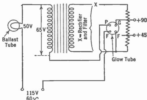
FIG. 260.— Ballast tube to maintain constant a.-c. voltage input to power transformer.
