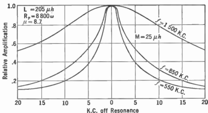
FIG. 188.—Curves showing how selectivity of tuned r.-f. circuit upon frequency.
