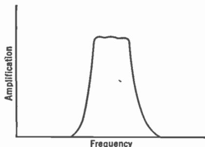
Fig. 191.—Overall response produced by amplifier of Fig. 190.
