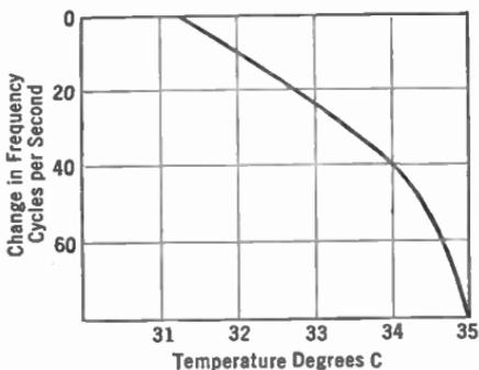
FIG. 285.—Effect of temperature on frequency.
