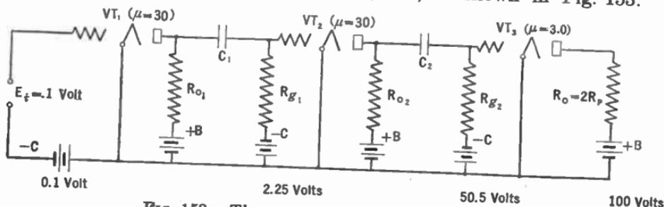
Fig. 153.—Three stage resistance coupled amplifier.
