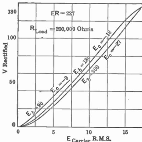
FIG. 210.—Plate rectification "power" detector characteristic.
