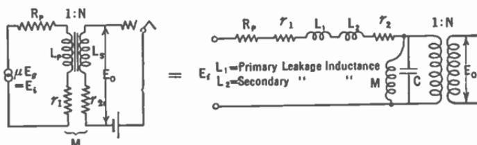
FIG. 177.—Equivalent circuit of transformer.
