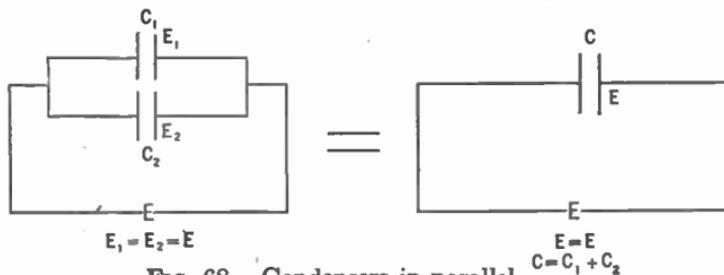
FIG. 68.—Condensers in parallel.
