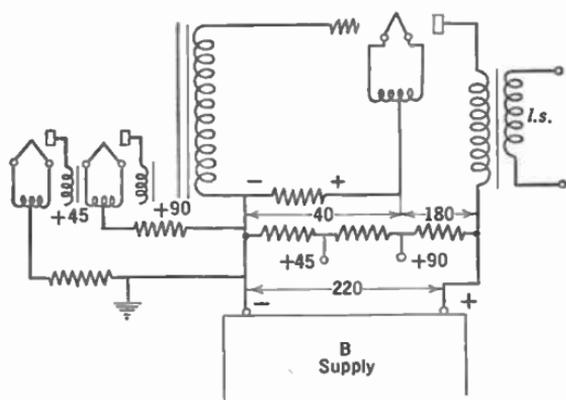
FIG. 256.—How the voltage divider originates.
