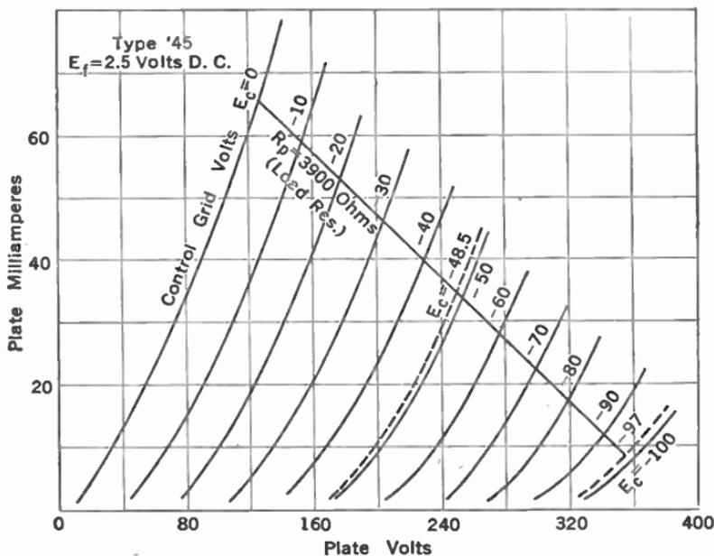
FIG. 120.—Plate current—plate voltage curves.
