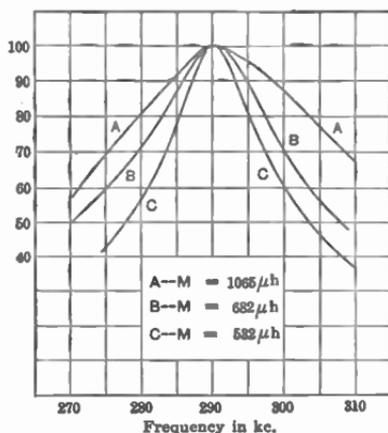
FIG. 187.—Relation between coupling and selectivity.
