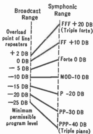
FIG. 171.—Compression of dynamic range in broadcasting system.
