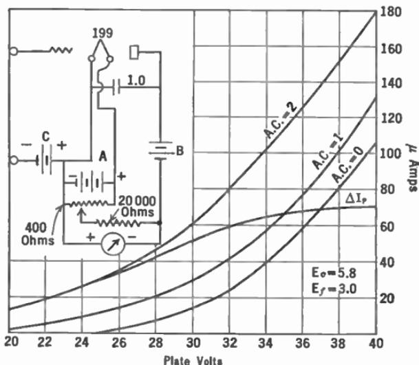
FIG. 205.—Calibration and circuit of vacuum tube voltmeter
