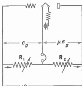
Fig. 125.—Bridge for determining amplification factor.
