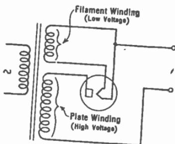
FIG. 238.—Operating rectifier filament from a. c.
