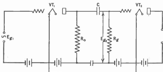
Fig. 150.—Two tubes coupled by a resistance-capacity unit.
