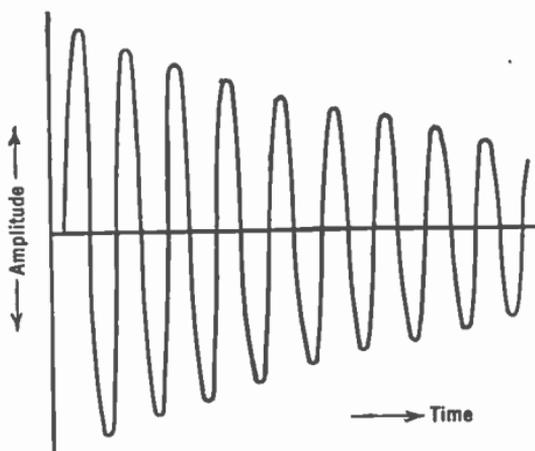
FIG. 265.—Slightly damped (low resistance circuit) waves.
