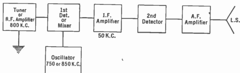
FIG. 214.—Symbolic diagram of superheterodyne.
