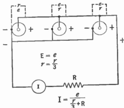
FIG. 39.—Cells in parallel.
