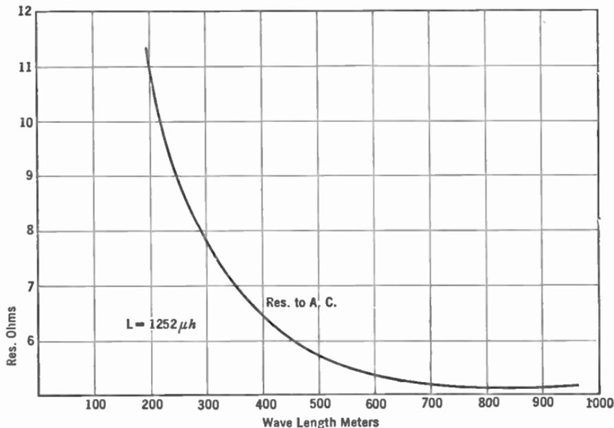
FIG. 101—High-frequency resistance of a coil.
