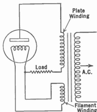
FIG. 249.—Tungar rectifier circuit.
