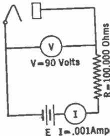
FIG. 20.—A problem in a resistance-coupled amplifier. What is the value of  $E$ ?
