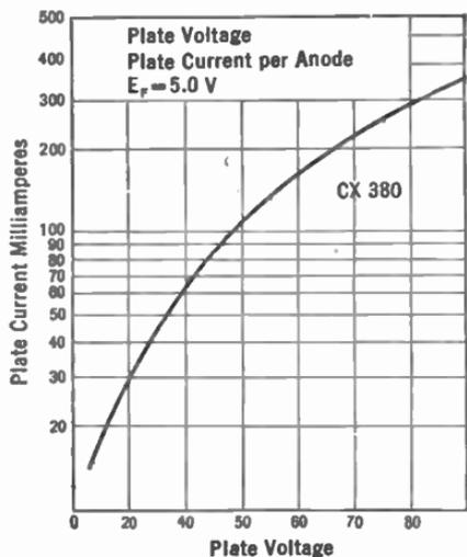
FIG. 242.—Characteristic of double wave rectifier tube.
