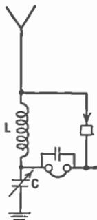
FIG. 104.—A simple radio receiver.
