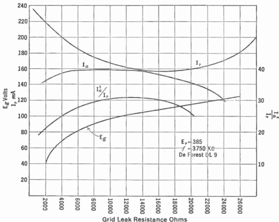
FIG. 281.—Effect of varying grid leak resistance.
