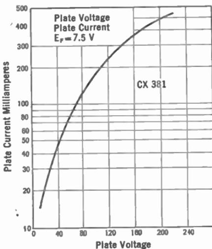
FIG. 243.—Single wave rectifier tube characteristic.
