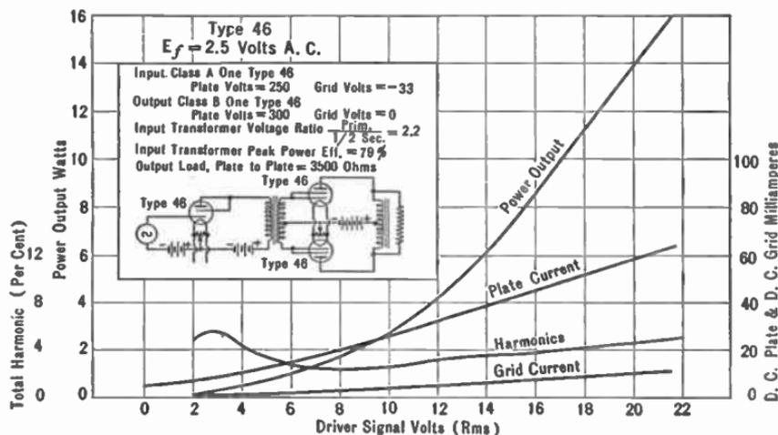
FIG. 164.—Characteristics of Class B Amplification.
