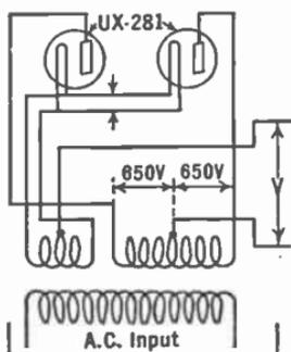
FIG. 240.—Connections of a full wave rectifier.
