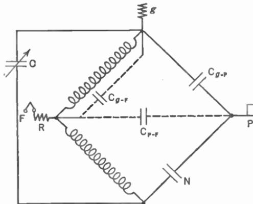
FIG. 195.—Equivalent bridge circuit of Fig. 194.
