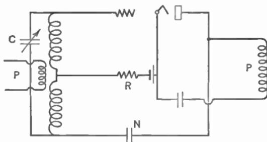
FIG. 194.—Rice neutralized circuit.
