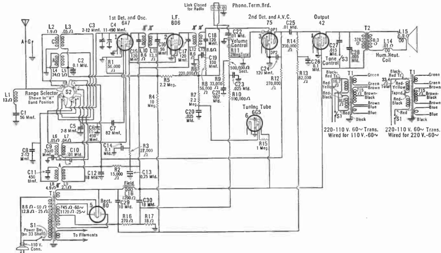
Fig. 130.—Circuit diagram of 1937 superheterodyne with coils in input and oscillator for multi-band reception.
