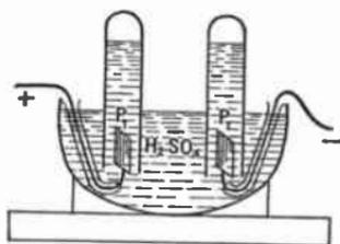
FIG. 35.—An experiment in electrolysis.
