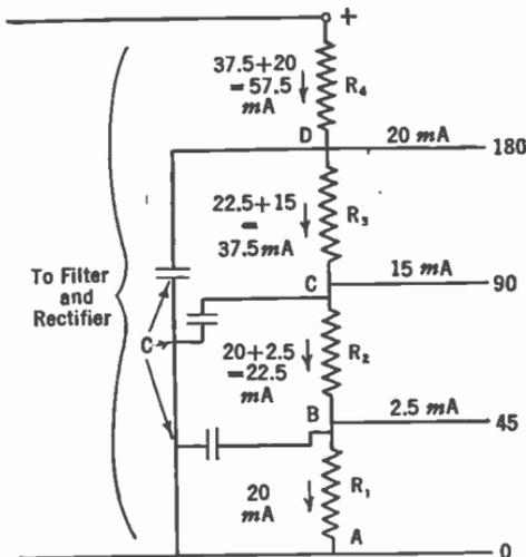
FIG. 258.—Designing the voltage divider.
