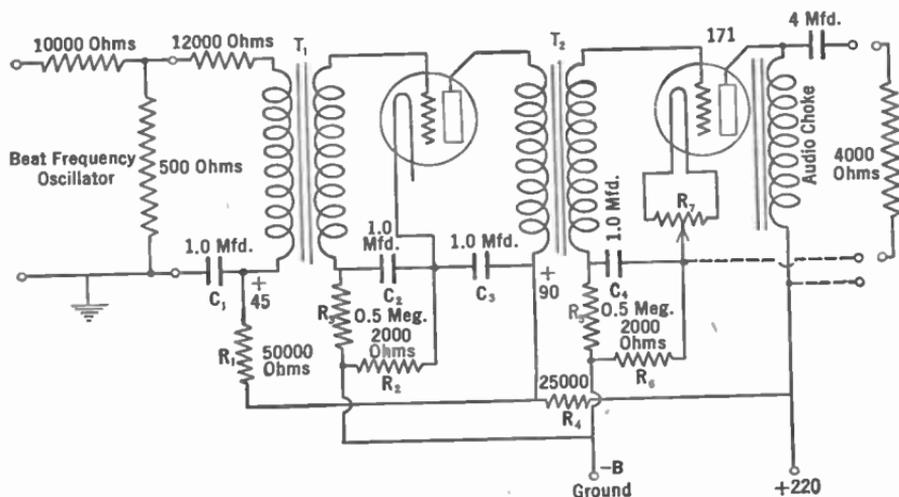
FIG. 176.—A high quality, well-filtered audio amplifier.
