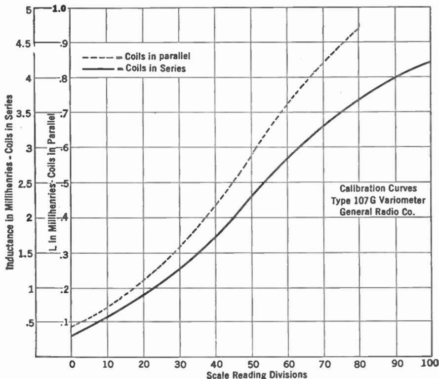
FIG. 60.—Calibration of a standard variable inductance.
