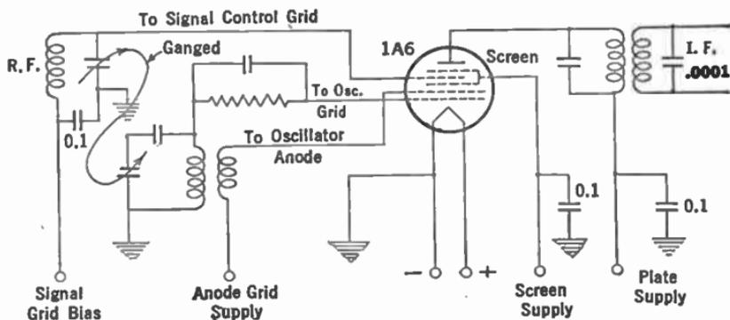
FIG. 217.—Circuit of electron-coupled oscillator combining both the of oscillation and mixing in the same tube and using the same electron stream
