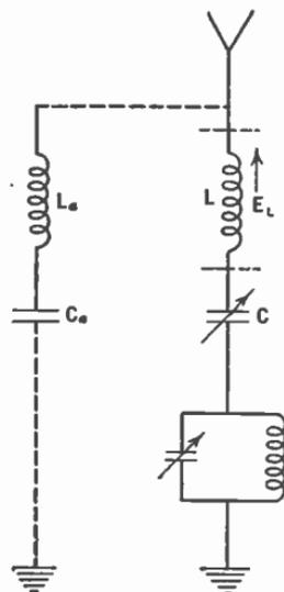
7 FIG. 96.—The anti-resonant circuit in series with the antenna rejects undesired signals by making the series impedance to them very high.
