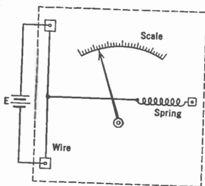
FIG. 25.—Hot wire ammeter.
