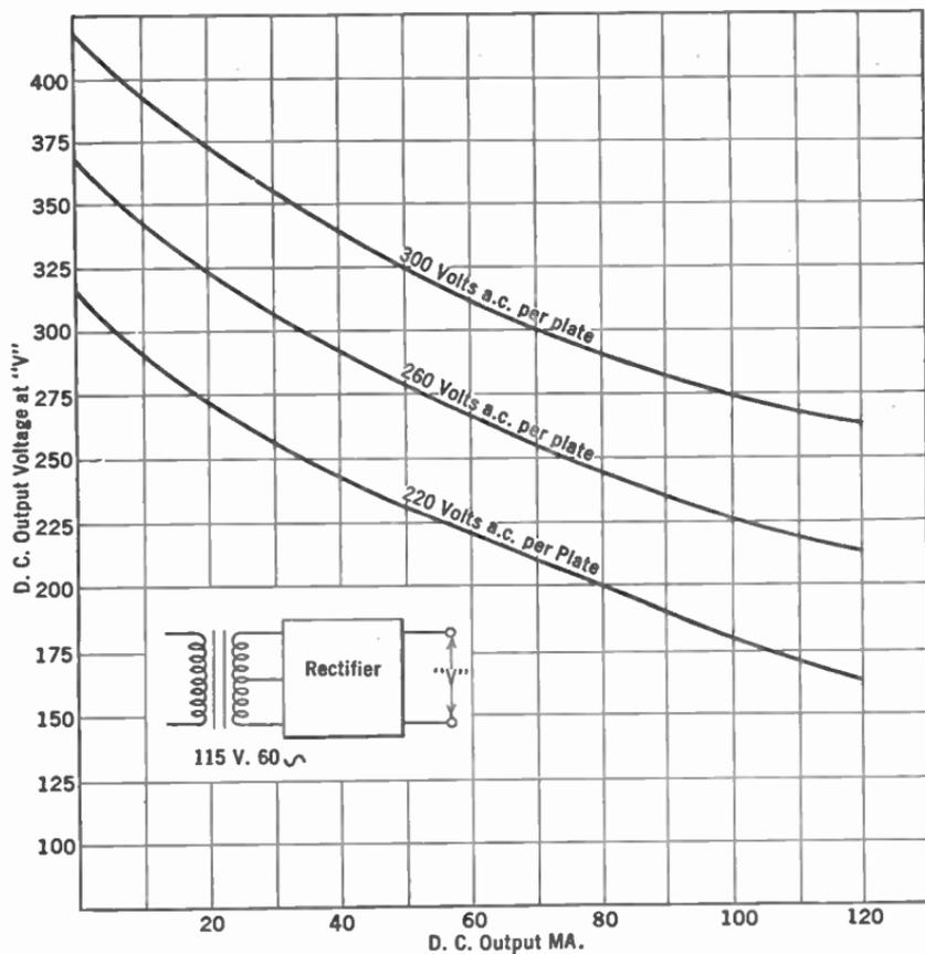
FIG. 7.—A power supply device regulation curve.
