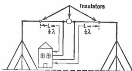
FIG. 302.—Folded half-wave antenna.
