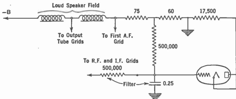
FIG. 259.—Circuit supplying bias voltages including a.v.c. bias.
