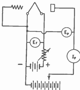
Fig. 116.—Circuit for apparatus of Fig. 115.
