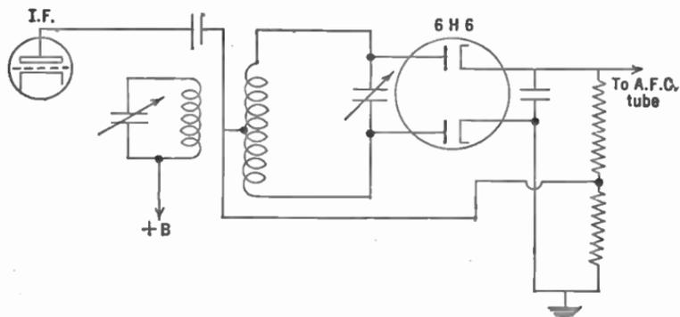
Fig. 230.—Discriminator Circuit for a.f.c.
