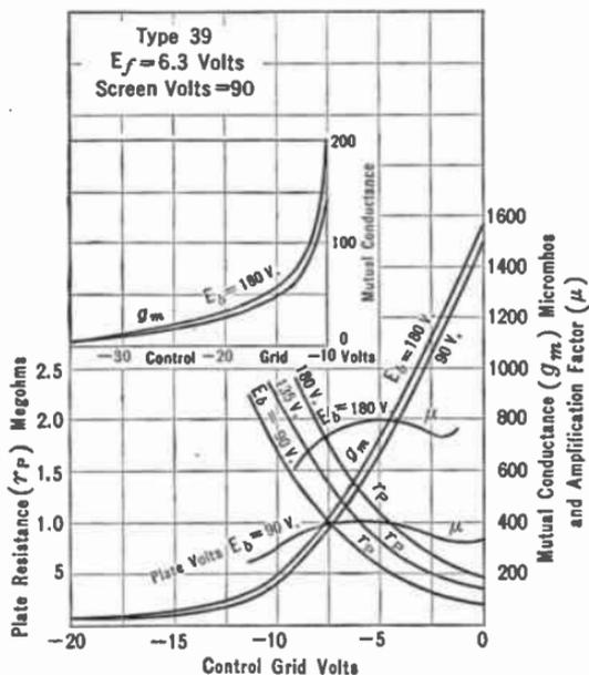
FIG. 137.—Characteristic of variable- $\mu$  tube.
