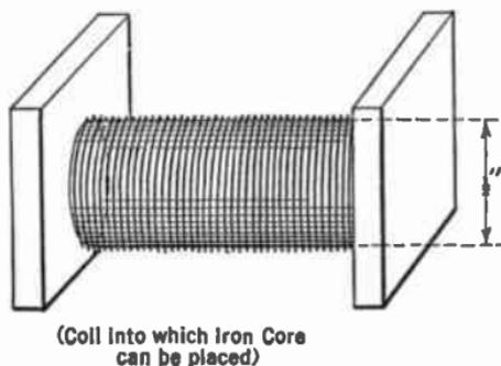
(Coil into which Iron Core can be placed)
