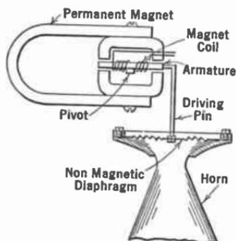
Fig. 231.—Horn type speaker mechanism.
