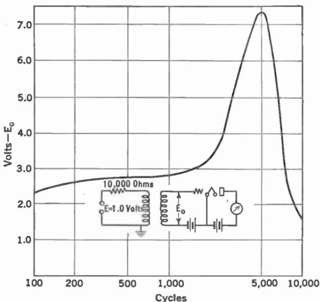
FIG. 160.—Characteristic of single audio transformer.
