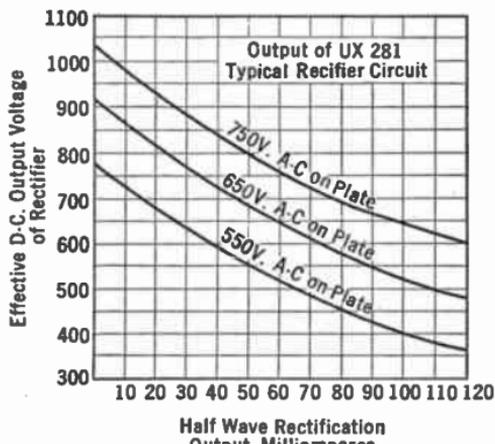
FIG. 252.—Output of modern rectifier.
