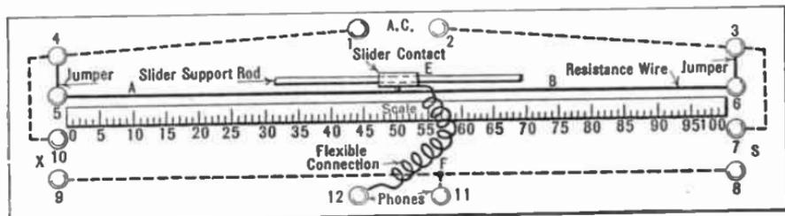
FIG. 33.—A single slide wire bridge.
