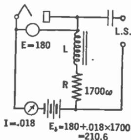
FIG. 10.—A choke-condenser coupling circuit.
