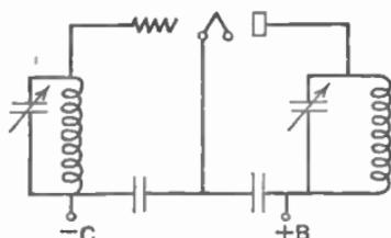
FIG. 193.—Tuned plate-tuned grid circuit.
