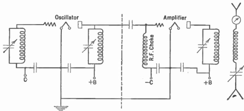
FIG. 283.—Master oscillator-power amplifier transmitting circuit.
