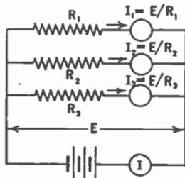
FIG. 21.—A parallel circuit.
