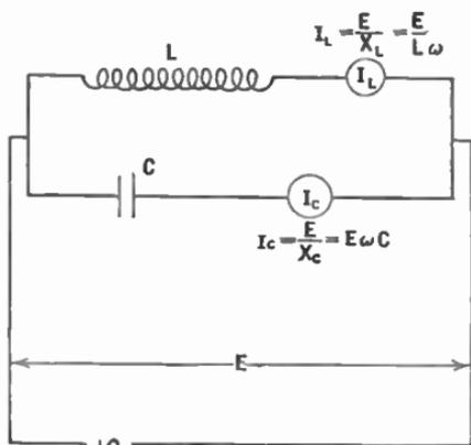
FIG. 95.—An anti-resonant circuit.
