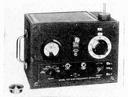
Fig. 306A.—External appearance of u-h-f signal generator, suitable use in method shown in Fig. 305.
