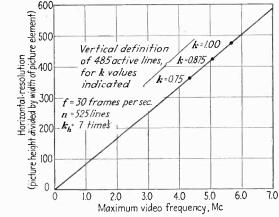
Fig. 304.—Relationship between maximum video frequency and horizontal definition, useful in determining frequency limits in terms of resolution observed in test charts.
