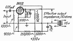
Fig. 136B.—Practical arrangement of a cathode-coupled stage displaying an output impedance of 110 ohms.
