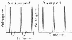
Fig. 86.—Resonance oscillations (left) at base of scanning waveform caused by reaction of deflection coil inductance and distributed capacitance. A damping circuit removes the oscillations, as shown at the right.
