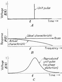
Fig. 110.—Response to a unit pulse of a transmission system having amplitude distortion but no phase distortion: A, the applied pulse, of unit area; B, the ideal amplitude-response characteristic required to reproduce the pulse exactly and a typical actual characteristic; and C, the pulse reproduced by the system displaying the nonideal characteristic, in the absence of phase distortion.
