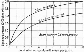
Fig. 59.—Iconoscope output vs. illumination curves showing increased sensitivity due to silver sensitizing. The silver-sensitizing technique also improves the color response of the camera tube.
