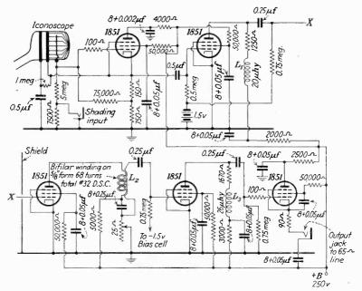
Fig. 242.—Complete diagram of iconoscope preamplifier.
