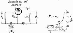
Fig. 137.—Typical distorting amplifier circuit used for obtained nonlinear reproduction ("gamma-control" amplifier). By adjusting the bias voltage  $E_c$  different portions of the  $i_p$ - $e_q$  operating characteristic may be chosen.
