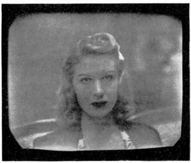
Fig. 55.—Appearance of televised image when subject is insufficiently illuminated.
