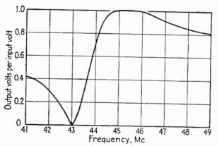
Fig. 266B.—Response characteristic of the filter structure shown in Fig. 266A. are of the high-level modulation type, modulating either in the final stage or in the next-to-final stage.
