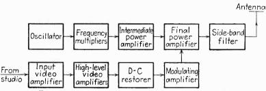
Fig. 155.—Essential elements of a television transmitter employing high-level modulation.
