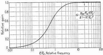
Fig. 123.—Amplitude-frequency response curve of uncompensated amplifier at low frequencies, in terms of the reference frequency fe determined by the coupling capacitor and grid resistor.
