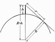
Fig. 149.—Geometrical relationship of antenna height to the horizon distance.
