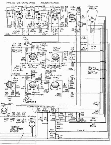
5-in. picture-tube receiver shown in Fig. 278.
