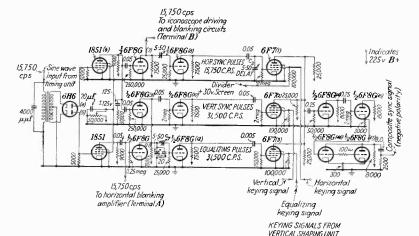
Fig. 254.—Horizontal shaping units of the sync signal generator. This unit accepts 15,750-e.p.s. timing pulses from the timing unit (Fig. 251), and 60-c.p.s. keying signals from the vertical shaping unit (Fig. 255), and derives from them the composite sync signal with horizontal, equalizing, and serrated-vertical pulses. It produces also 15,750-c.p.s blanking signals for the iconoscope and picture tube.
