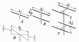
Fig. 174.—Elementary forms of television antennas available commercially: A, the simple dipole; B, the stacked double dipole; C, stacked dipoles with reflectors; D, double-V dipole.
