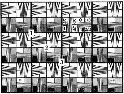
Fig. 27.—The "12-square" test chart used in production testing of camera tubes, picture tubes, and overall system performance. The fractions indicate the degree of shading, while the numbers 1, 2, and 3, indicate resolutions of 100, 200, and 300 lines in the wedges.
