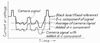
Fig. 101.—The d-c component of the video signal. The waveform retains its shape, but is displaced upward or downward as the picture becomes darker or brighter, respectively.
