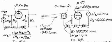
Fig. 42A.—Basic phototube amplifier circuit. The photoelectric current  $\Delta i_{pl}$  passes through the grid resistor  $R_g$ , producing a voltage  $\Delta e_g$  which is amplified to the value  $\Delta e_g$ .
