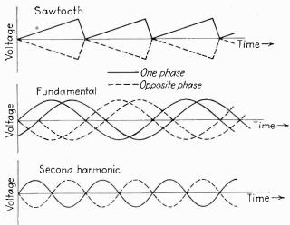
Fig. 257.—Wave shapes produced by the shading correction generator (Fig. 256). The saw-tooth, sine wave and double-frequency sine wave are available at vertical and horizontal seanning rates, with controllable amplitude, phase, and polarity.
