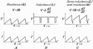
Fig. 81.—Saw-tooth waves of current produced by voltage waves in a resistive circuit (A), an inductive circuit (B), and a combination resistive-inductive circuit (C). The voltage waveform (C) is that commonly applied to the deflecting coils in magnetic deflection systems.
