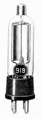
Fig. 41.—Typical commercial phototube. The hemicylindrical cathode, when illuminated, releases electrons which are collected by the central wire anode.
