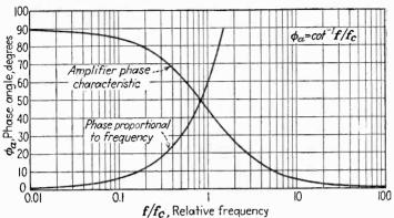
Fig. 124.—Phase-frequency characteristic of the uncompensated amplifier.
