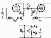
Fig. 122.—Uncompensated amplifier with equivalent low-frequency circuit.
