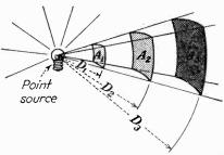
Fig. 28.—Light flux radiating from a point source. As the illuminated areas  $A_1$ ,  $A_2$ , and  $A_3$  are removed from the source, the light flux available in the given solid angle is spread over larger and larger areas, with resulting decrease in illumination.
