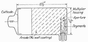
Fig. 484.—The Farnsworth image dissector, a practical television camera tube which employs instantaneous electronic scanning. An electron image, formed at the cathode by the optical image, is conveyed down the tube and moved bodily past a small aperture. The electrons entering the aperture, after multiplication, constitute the output signal of the tube.
