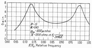
Fig. 181.—Band-pass response curve of circuit shown in Fig. 180A. The gain is directly proportional to the  $y_m$  of the tube and the value of X (after Seeley and Barden).
