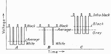
Fig. 261.—Variation of the average of the video signal: A, white image with narrow black bar; B, black image with narrow white bar, with blanking level held same as in A; C, white image with narrow black bar, as in A, but with average coinciding with average in B. Most of the signal in C is lost above the black level, due to the upward displacement of the average.
