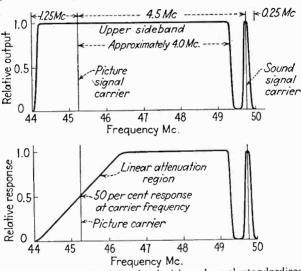
Fig. 148.—The vestigial sideband television channel standardized by the R.M.A. Television Committee and now used as the basis of transmissions in the United States. The upper diagram is the transmitter output curve, the lower the receiver response curve which equalizes the percentage modulation of sideband components near the carrier to that of components far removed.
