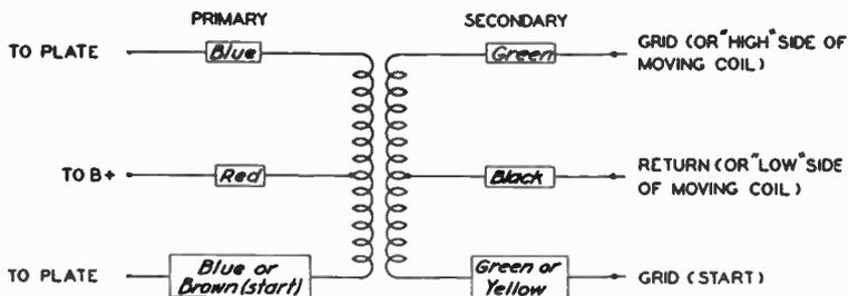
Standard RMA Color Code for the leads of audio-frequency transformers. (See accompanying text for explanation).
