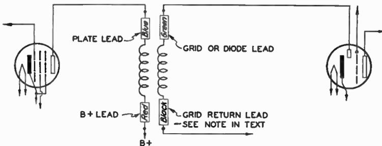
Standard RMA Color Code for the leads of intermediate-frequency transformers. (See accompanying text for explanation).
