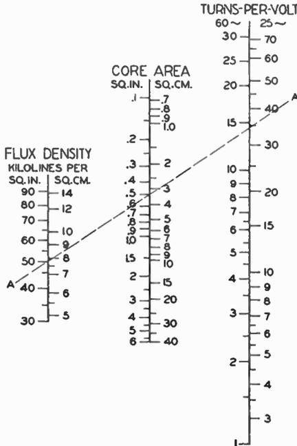
**TRANSFORMER TURNS-PER-VOLT CHART:** Knowing the flux density and the core area, the turns-per-volt for either a primary or a secondary winding may be determined by merely drawing the straight line (A-A) from the proper point on the "FLUX DENSITY" line through the proper point on the "CORE AREA" line—the extension of this line intersects the "TURNS-PER-VOLT" line at the point which represents the turns-per-volt of the transformer.
