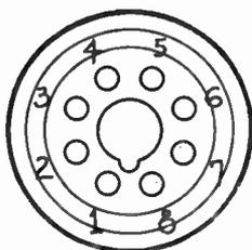
An 8-pin "Octal"-type tube base (viewed from the bottom) showing the eight pins, their numbers, and the guiding lug at the center.
