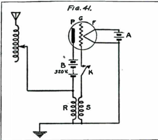
The oscillations are generated as long as the key is closed. It is to be noted that the oscillations have energy from the battery, B, added. Hence, they are undamped oscillations. The circuit containing the antenna determines the frequency of the oscillations. The coupling between R and S must be close enough to cause the voltage of the grid to vary over a range sufficient to keep the oscillations flowing in the circuit.
