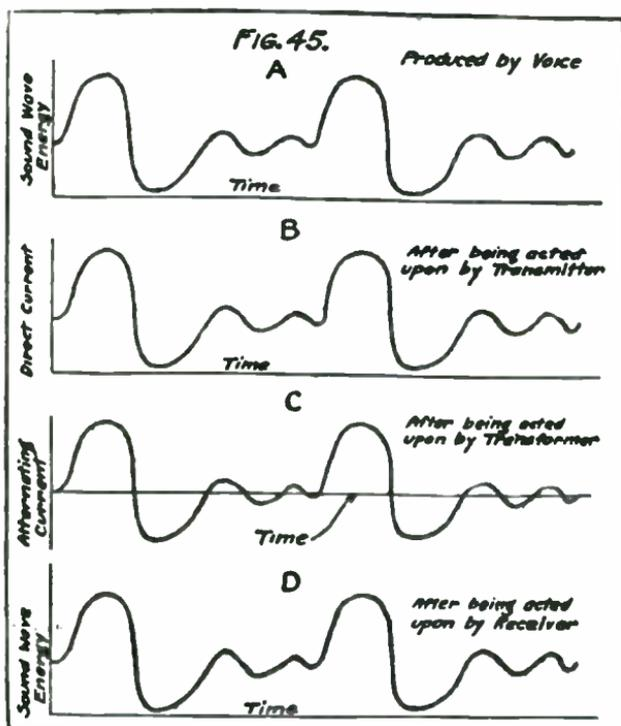
variation in pressure between the carbon granules varies the resistance of the granules. A direct current which is flowing through the granules is varied by this varying resistance. This varying direct current is changed into a varying alternating current by means of a step-up transformer. The alternating current acts upon the receiver. This receiver consists of an electromagnet
