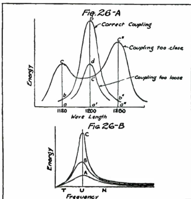
amount of energy. The explanation of this lies in the fact that an oscillating circuit coupled to another oscillating circuit is affected by the circuit to which it is coupled. It has two frequencies at which it will oscillate well. One of these frequencies is slightly higher and the other slightly lower than its natural frequency when oscillating alone. The closer the coupling the farther apart are these two
