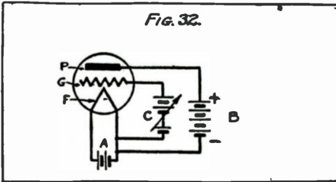
nected to the plate or not built in the tube) may be used as a detector in place of the galena crystal. Such a tube may also be used as a rectifier of alternating currents, because it allows current to pass only in one direction. The use of the grid greatly improves the action of the tube and will be explained before taking up the action of a vacuum tube used as a detector.
