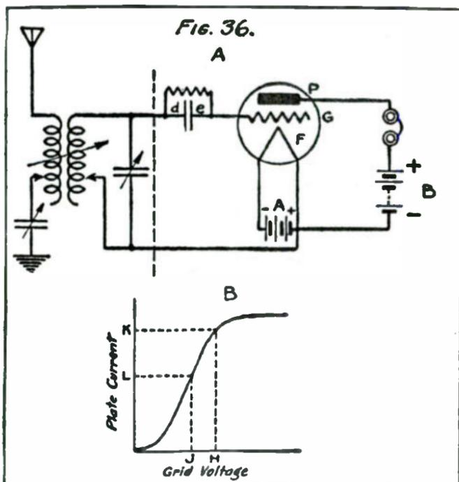
The result of reducing the potential of the grid is to reduce the plate current flowing in the valve. In figure 36 B, the steady potential (with no oscillations) is represented at H. This gives a steady value of the current represented by the point K. The wave train reduces the grid potential to J which reduces the plate current and there-
