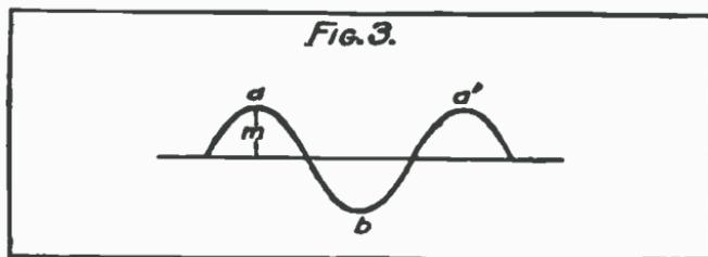
and the other part of the wave disturbance is on the opposite side of the usual (waveless) condition. This is true of the radio waves. Look at figure 2 and note that the arrows show that the electrostatic lines of force are directed upward in one part of the wave and downward in another part. This is also true of the electromagnetic lines of force. The open circles represent those that are directed toward you; the solid circles represent those that are directed away from you.
