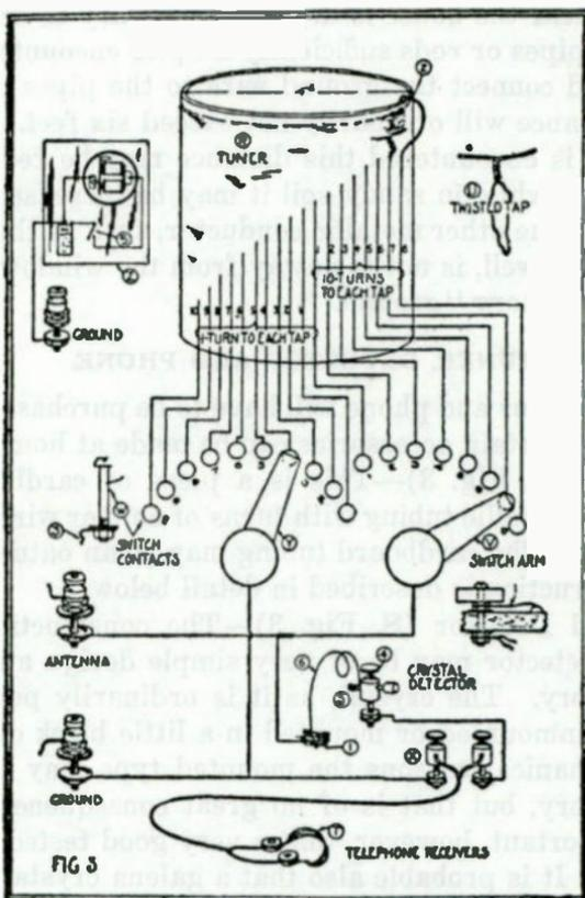
Phone (T, Fig. 3)—It is desirable to use a pair of telephone receivers connected by a head band, usually called a double telephone headset. The telephone receivers may be any of the standard commercial makes having a resistance of between 2,000 and 3,000 ohms,
