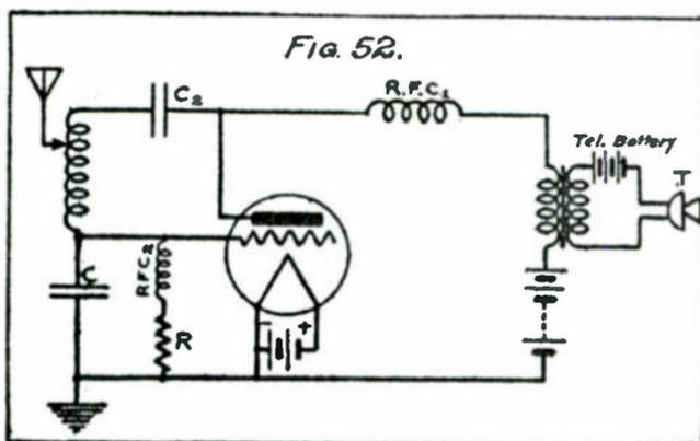
proper negative potential at which it works efficiently. The choke coil in this circuit forces the oscillations to pass through the condenser, C, to which the filament is also connected. The condenser, C, assures the proper oscillating voltage between the filament and the grid. The condenser  $C_2$ , prevents the positive potential of the plate battery from reaching the grid through the coils of the autotransformer which couples the grid and the plate circuits.
