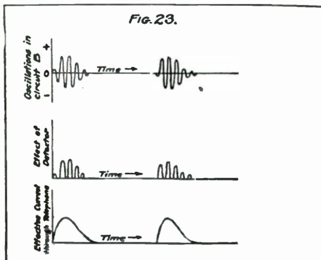
current flowing in circuit C. The pulsations occur at the radio frequency of the oscillation in circuit B.
