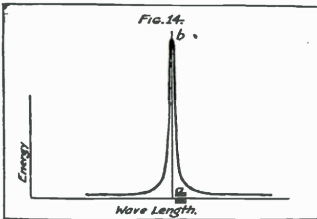
represented by the length of the line *ab*; but in addition to that wave, there is a continuous band of waves having all possible wave lengths near the wave length of 300. Thus the wave whose length is 200 is radiated with an energy represented by the length of the line *cd*. Now, as only the energy represented by a very narrow band of wave lengths (shaded area around *ab*) can be received, all the other energy is wasted.
