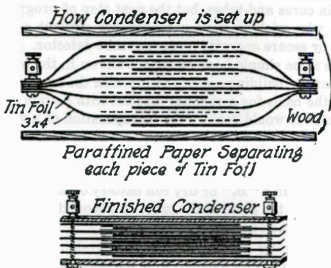
signed, but the simplest is built up of alternate layers of tin foil and paraffined paper cut in strips. There should be ten strips of foil about four inches long by three wide, arranged as shown in the accompanying diagram. The strips of paraffined paper between should be slightly wider than the foil sheets. When arranged as shown, the paper and foil strips are pressed tightly together with pieces of cigar box wood on either side to hold them firmly. The diagrams are self explanatory.
