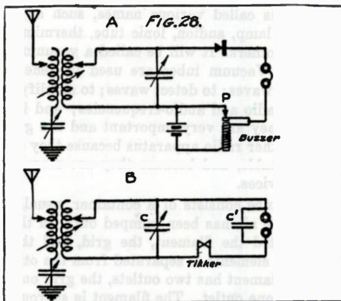
into the condenser C', thus charging it. When the tikker opens the circuit, the charge condenser discharges through the telephone. As the condenser has a large capacity, the discharge gives a current large enough to actuate the telephone diaphragm. A discharge occurs each time the tikker interrupts the circuit. This is at audio-frequency, so that a note is heard in the receiver. Other methods of receiving undamped waves will be discussed under vacuum tubes.
