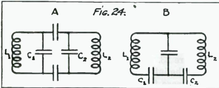
and the other set of plates of the same condenser is in the other circuit. Figure 24 shows two methods of electrostatic coupling. The inductance and capacity of each circuit is marked; the unmarked condensers are the condensers used in coupling the circuit. There are various other methods besides those shown. Electrostatic coupling takes the place of an oscillation transformer. Such an arrangement of circuits may be called an electrostatic transformer.
