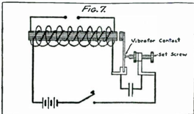
sudden stopping of the current in the primary produces a surge of high voltage in the secondary, thus charging the condenser. Figure 8 shows the relations of current and voltage in the primary and secondary.
