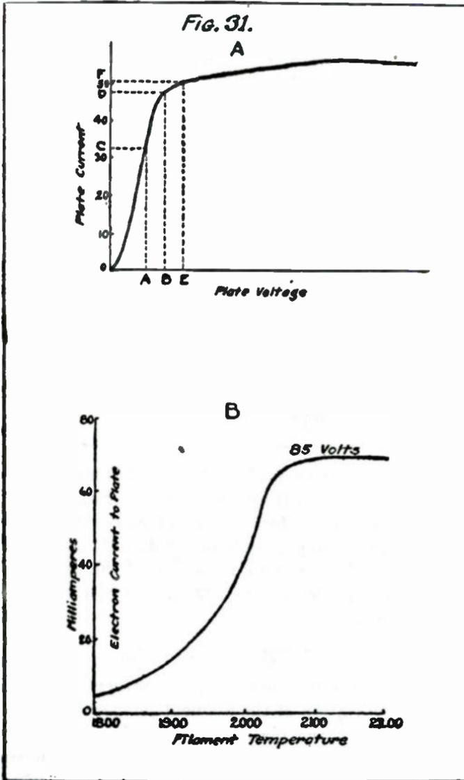
A current flows in the tube because the filament emits electrons. The electrons pass from the filament to the plate and grid. Neither the plate nor grid can emit electrons as they are not heated. This means that the electrons can pass only one way through the tube and hence an electric current can pass *only one way* through the tube. This is exactly what the galena crystal does. A vacuum tube with only a filament and plate (grid con-
