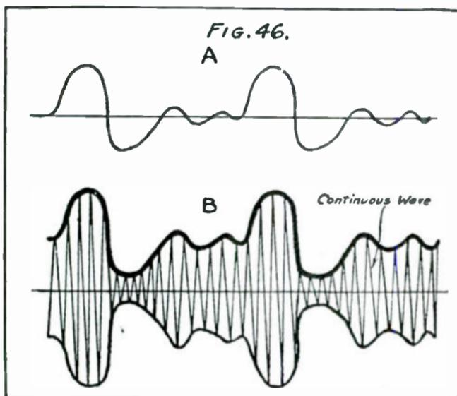
wave, that is, a wave similar in character to that of figure 45. It has been possible to do this by varying the amplitude of the radiated high-frequency waves so that this variation in amplitude follows in detail the wave variation produced by the sound. In figure 46, curve A represents a simple sound wave. By means of methods to be described later, the amplitude of a *continuous* radio wave
