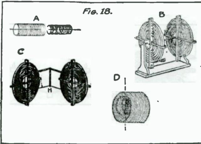
able. The smaller one can be slid into the larger one. It is commonly termed a loose coupler. B shows a flat, spiral type whose coils can be made to approach each other. C shows an arrangement for mounting the flat spirals and moving them on a hinge at H. D shows two coils, the small one mounted inside the other. The inside one can be rotated around an axis, so that it can be made to be at any angle with the outside one.
