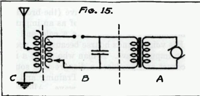
is the power circuit. Circuit B is the spark-gap circuit. Circuit C is the radiating circuit.
