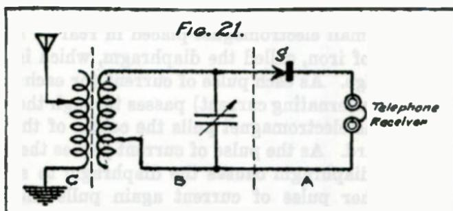
tion induced in the receiving antenna is caused by electromagnetic induction. This is the same phenomena that occurs in the induction coil, the transformer, and various other instruments.
