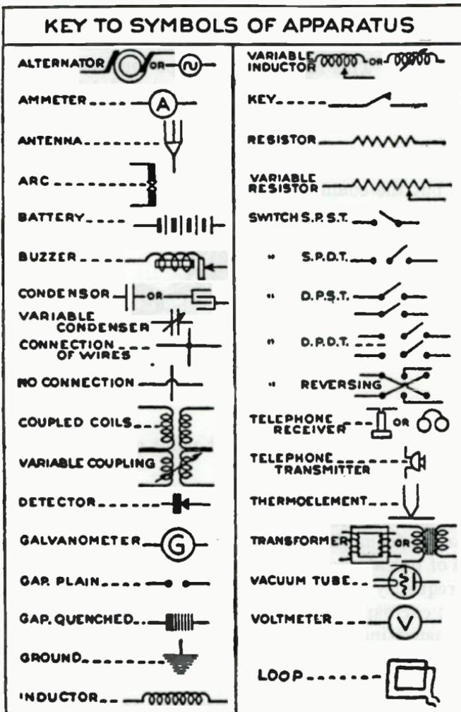
THESE SYMBOLS ARE USED IN DIAGRAMS TO INDICATE THE VARIOUS PARTS OF RADIO APPARATUS.
