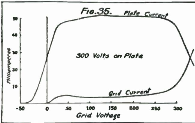
to neutralize the effect of the pump B. The blower action would not have to be very strong to completely overcome the effect of the pump B. In the actual tube, giving the grid a negative potential has the same effect as making the pump, C, a blower.
