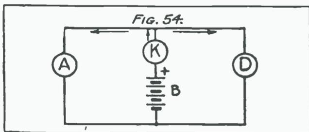
rent passing through K does not split 50-50, but, say, 80-20, the larger part going through the D circuit. When the resistance of D is increased the reverse of this takes place, the larger current passing through A. A and D represent the tubes and K represents the low-frequency choke coil of figure 52. The varying potential on the grid of tube II has the effect of changing the resistance of that tube.
