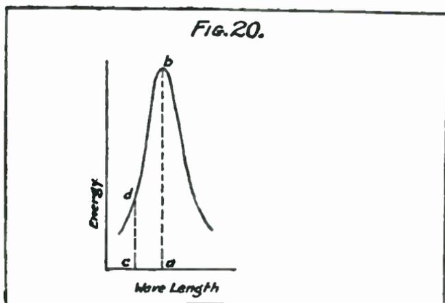
quencies are the same. This condition of resonance must exist between circuits coupled together in any way if there is to be an efficient transfer of energy.
