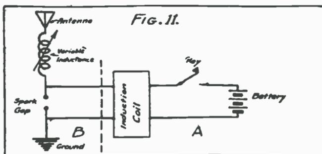
but it is usual to add variable inductance in the form of a coil so as to be able to control the wave length.
