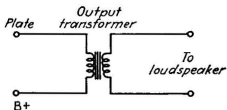
FIG. 255.—Coupling circuit of transformer type for power-output tube.
