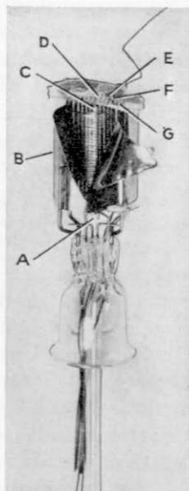
FIG. 93.—Pentagrid converter.
