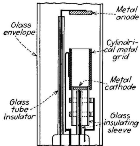
FIG. 169.—Reich and Hesselberth's cold-electrode glow-discharge tube.
