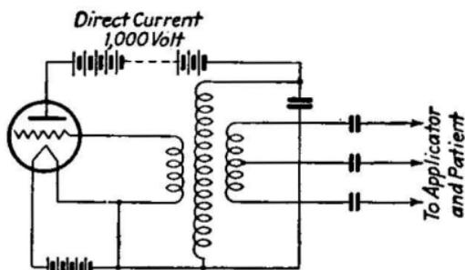
FIG. 479.—Circuit for radio surgical needle.
