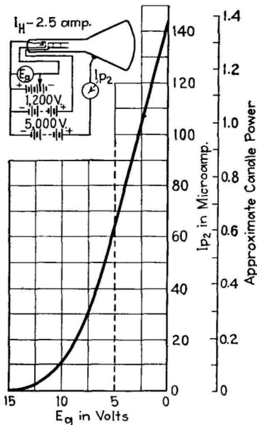
FIG. 441.—Characteristic curve of kinescope.
