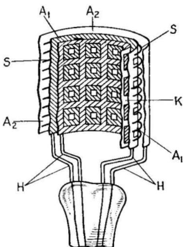
FIG. 166.—Cold-electrode tube with cylindrical electrodes.
