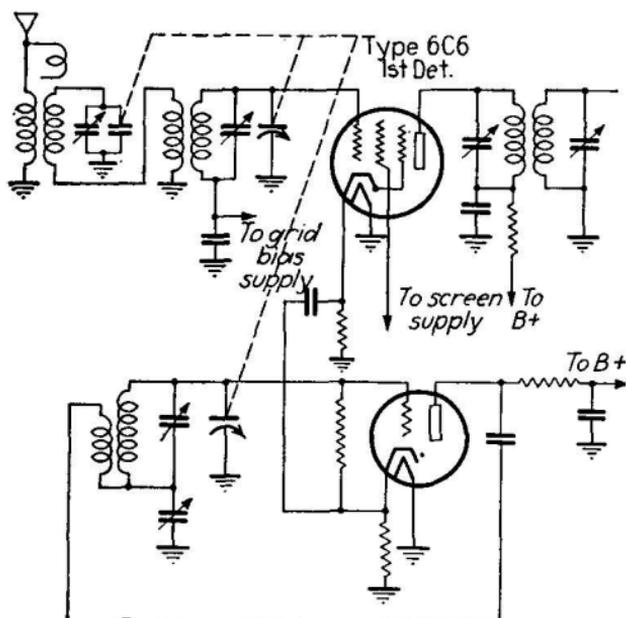
FIG. 407.—Typical all-wave superheterodyne oscillator circuit.
