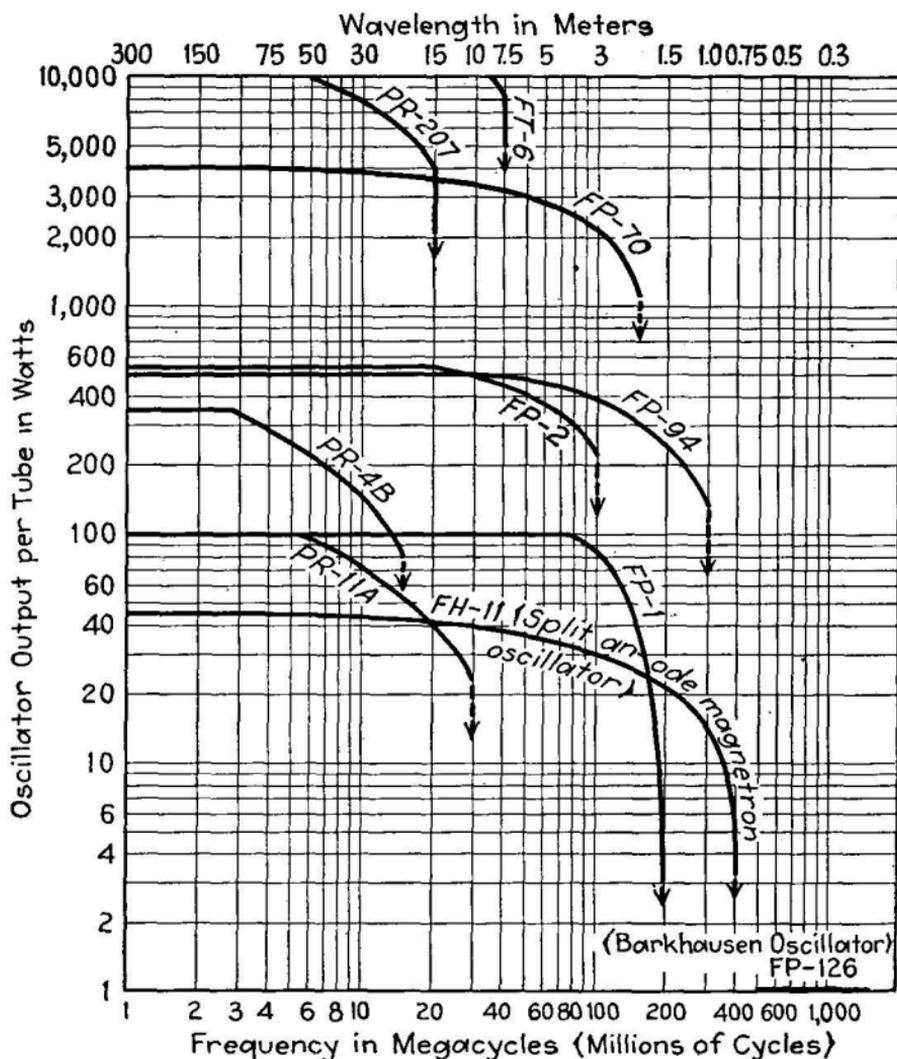
FIG. 414.—Frequency and power-output capacities of typical vacuum tubes
