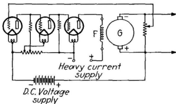
FIG. 377.—Direct-coupled amplifier for slow-voltage variations with generator-field adjustments.
