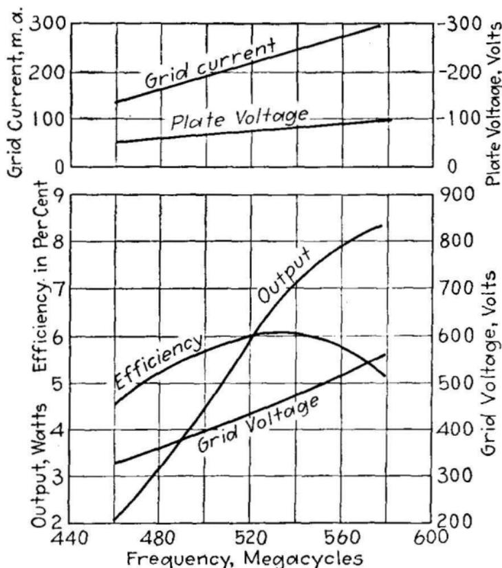
FIG. 425.—Output and efficiency curves for positive-grid oscillator tube in Fig. 423.
