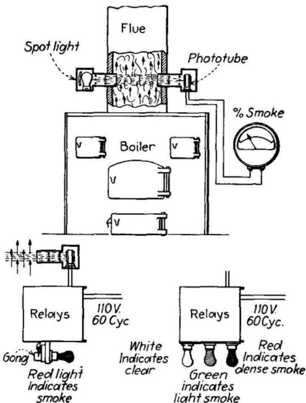
FIG. 468.—Photoelectric tube mounted in flue in boiler for smoke indication.
