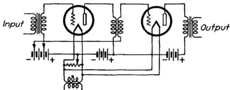
FIG. 375.—Transformer-coupled amplifier.
