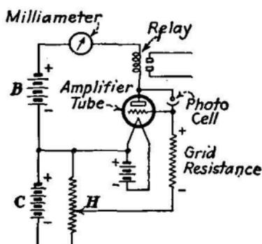
FIG. 378.—Typical direct-current forward circuit.
