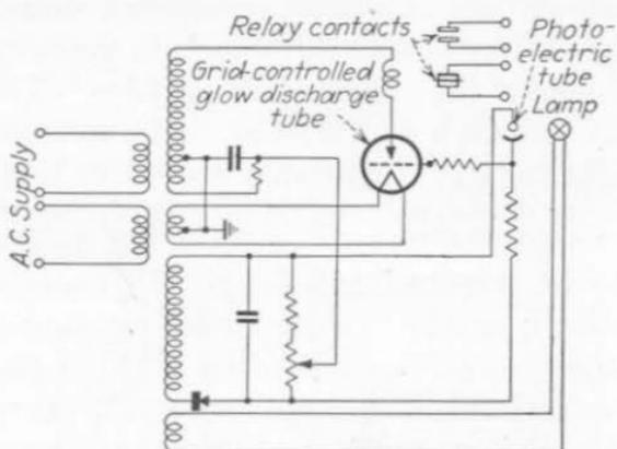
FIG. 448.—Circuit of photoelectric controller.
