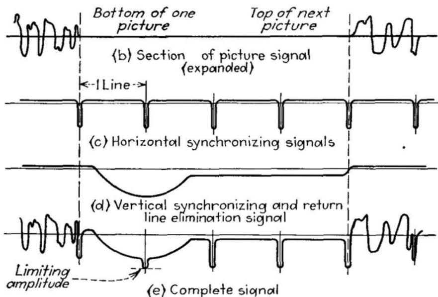
FIG. 445.—Diagram of synchronizing signals in iconoscope.
