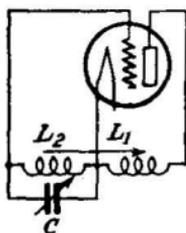
FIG. 400.—Tuned-grid oscillating circuit.
