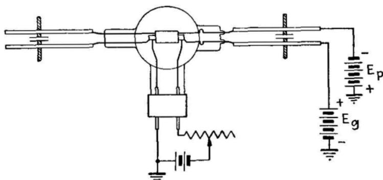
FIG. 424.—Typical positive-grid oscillator circuit.
