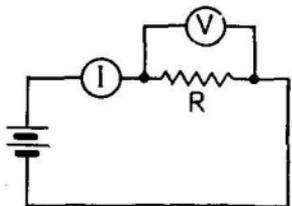
FIG. 213.—Arrangement of voltmeter in circuit of Fig. 211 when the resistance to be measured is low.
