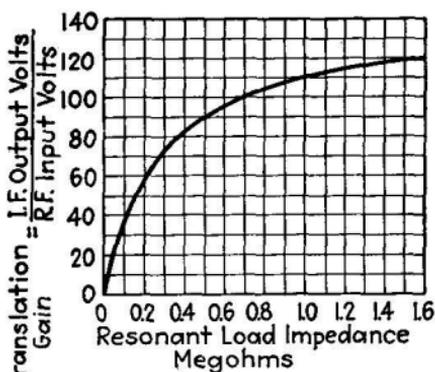
FIG. 96.—Translation gain curve for pentagrid converter (type 6A7).
