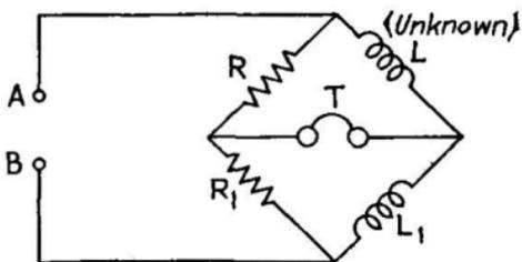
FIG. 214.—Circuit diagram for inductance measurement with a Wheatstone bridge.
