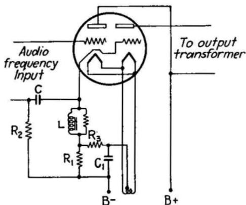
FIG. 80.—Conventional circuit for triple-twin tube.
