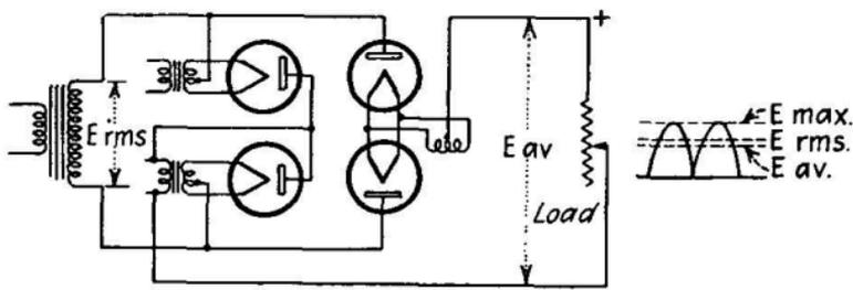
FIG. 307.—Method of rectifying both halves of a cycle with the use of four tubes to obtain twice the output voltage obtained from the circuit shown in Fig. 306.
