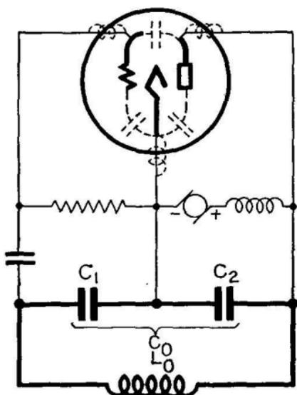
FIG. 417.—Modified Colpitts oscillator circuit.
