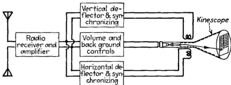
FIG. 439.—Iconoscope receiving equipment.
