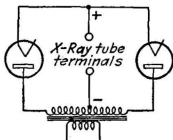
FIG. 322.—Full-wave rectification circuit.
