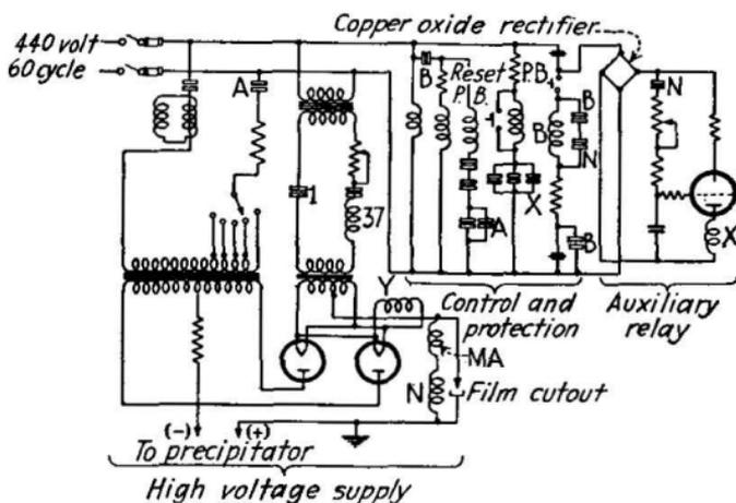
FIG. 458.—Circuit diagram of precipitation apparatus.
