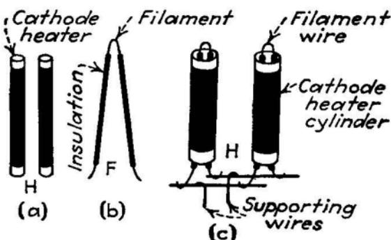
FIG. 10.—Construction of cathode heaters.
