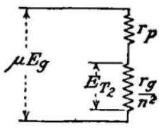
FIG. 348.—Equivalent of plate circuit of tube  $A$  in Fig. 347.
