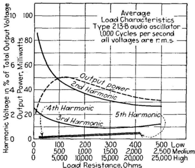
FIG. 210.—Load characteristics of audio-frequency oscillator.
