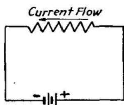
FIG. 17.—Electron flow opposite in direction to current flow.
