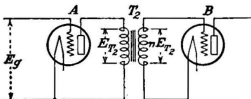
FIG. 347.—Circuit of transformer-coupled amplifier unit.
