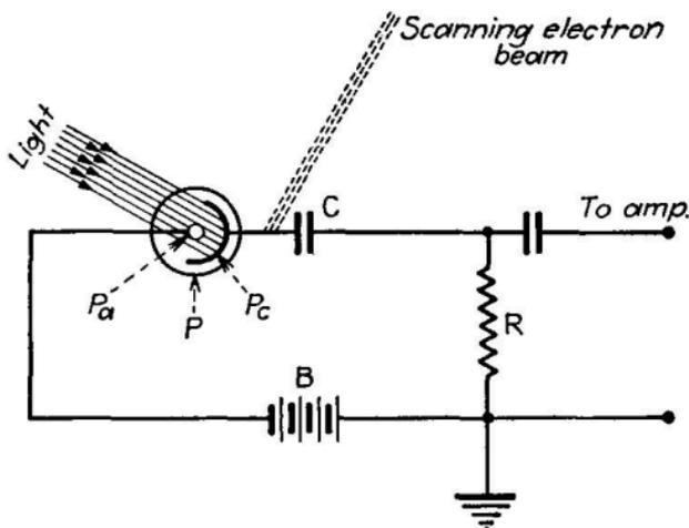
FIG. 429.—Circuit of photoelectric elements in iconoscope.
