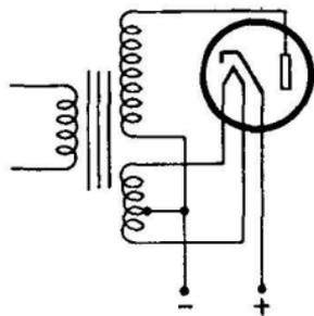
FIG. 288.—Circuit for half-wave rectifier with heater cathode.
