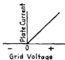
FIG. 258.—Relation between plate current and grid voltage in true detector.
