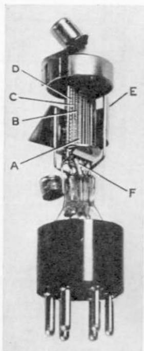
FIG. 72.—Section of typical triple-grid tube (type 58).
