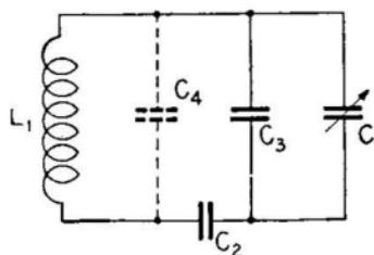
FIG. 412.—Typical oscillator circuit in super-heterodyne receiver.
