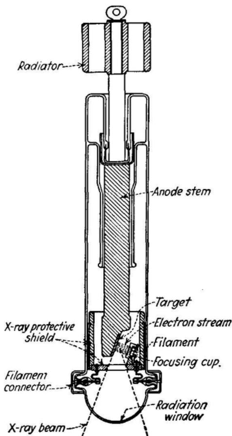
FIG. 184.—Construction details of typical radiographic x-ray tube.
