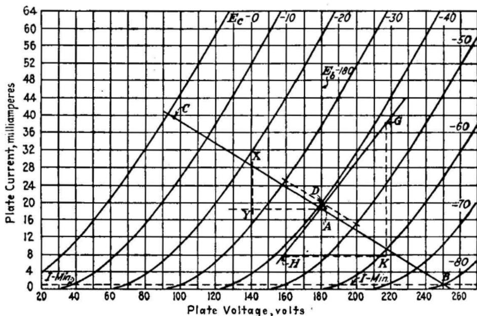
FIG. 332.—Curves showing distortion effects in power tubes.
