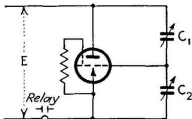
FIG. 142.—Circuit for cold-cathode gaseous tube with condenser-potentiometer units for control.
