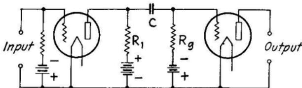
FIG. 343.—Resistance-coupled audio-frequency amplifier.
