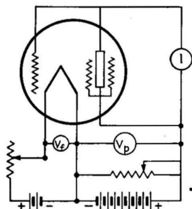
FIG. 215.—Typical circuit for emission testing.
