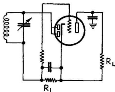
FIG. 278.—Typical detection circuit for duplex-diode-triode tubes.
