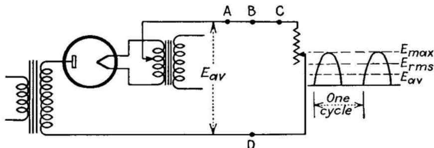
FIG. 292.—Typical rectified power-supply system.
