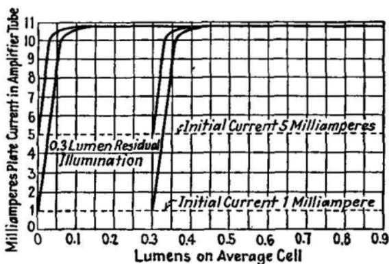
FIG. 380.—Response curve for forward circuit.
