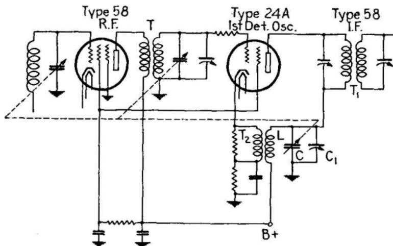
FIG. 406.—Autodyne frequency converter.
