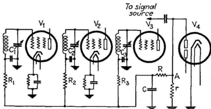
FIG. 355.—Automatic-volume-control circuit with filters.
