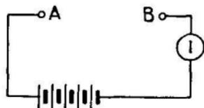
FIG. 211.—Simple circuit for resistance measurements.
