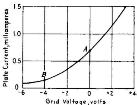
FIG. 267.—Characteristic curve of typical triode vacuum tube.
