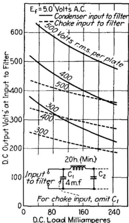
FIG. 302.—Characteristic curves of typical heavy-duty rectifier tube.
