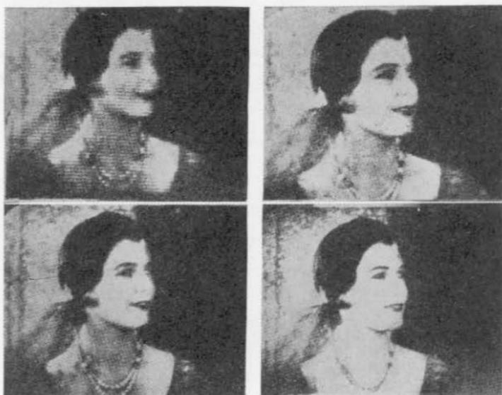
FIG. 427.—Television pictures made with 60, 120, 180, and 240 lines.
