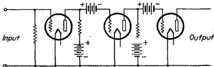
FIG. 370.—Typical direct-coupled amplifier.
