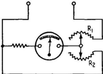
FIG. 203.—Wiring of Weston output meter.
