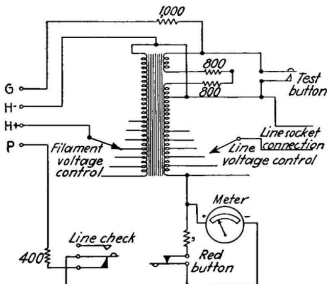
FIG. 240.—Simplified circuit diagram showing connections to socket A in Weston Model 661 tube tester.
