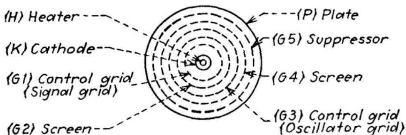
FIG. 108a.—Electrodes in type 6L7 tube.
