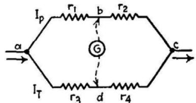
FIG. 204.—Typical Wheatstone-bridge circuit.
