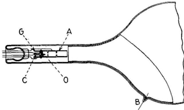
FIG. 434.—Electron gun of iconoscope.
