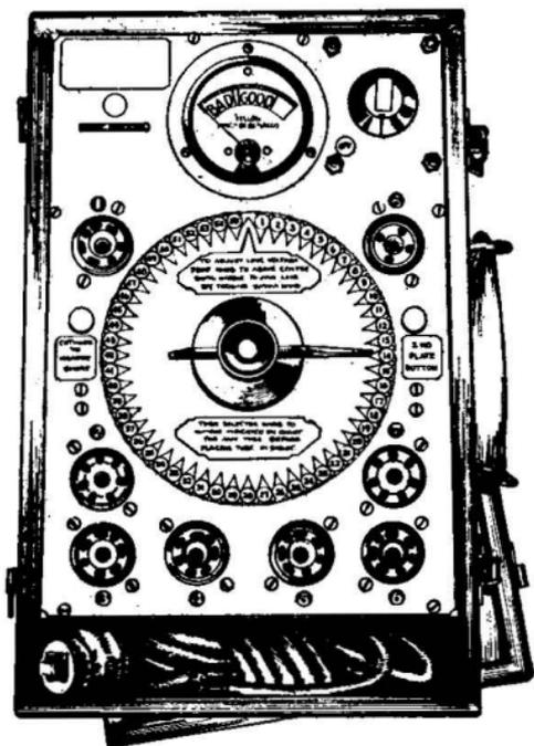
FIG. 227.—Panel of "Confidence" No. 6 tube tester.
