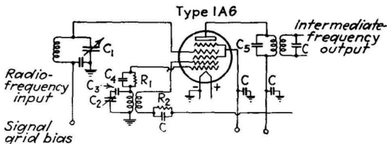
FIG. 95.—Diagram of typical pentagrid converter circuit for filament type of tube.
