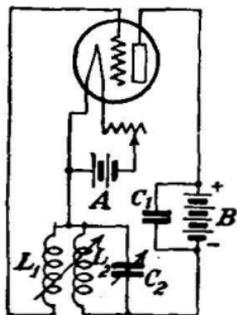
FIG. 397.—Simple oscillator for producing alternating current.
