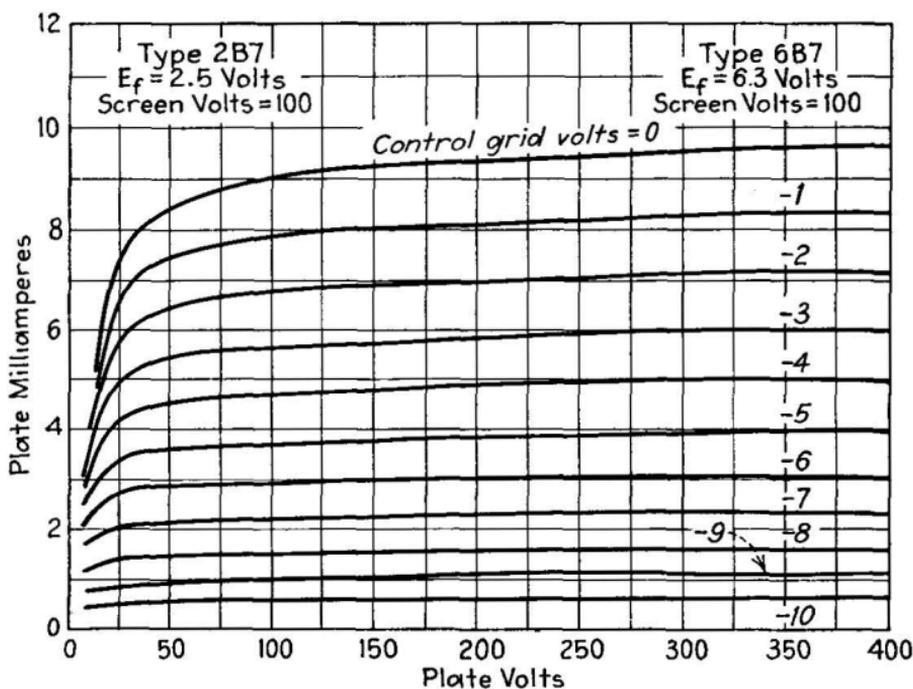
FIG. 88.—Average characteristics of duplex-diode pentode (type 6B7).
