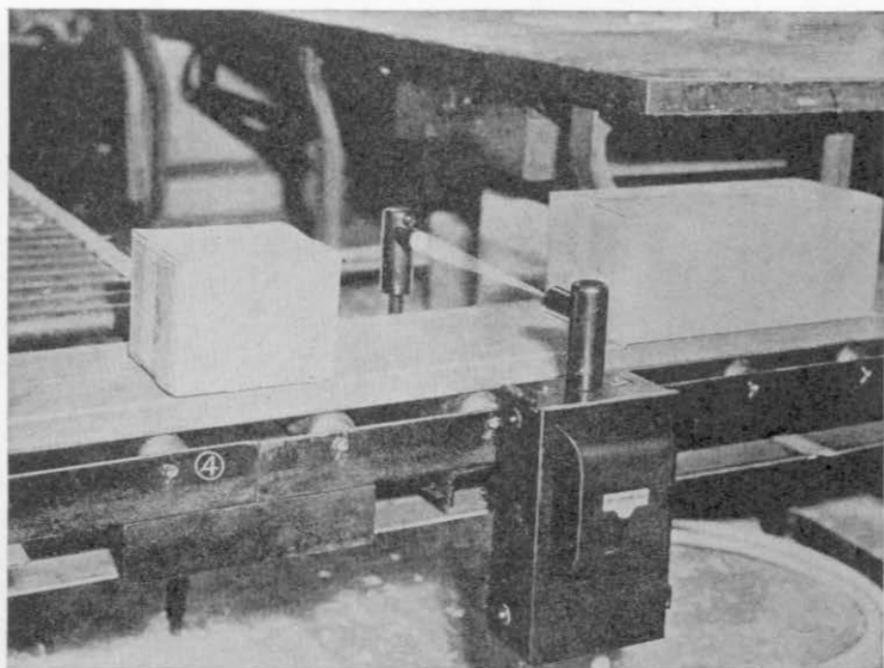
FIG. 449.—Photoelectric tube used for automatic counting and destination of parcels.
