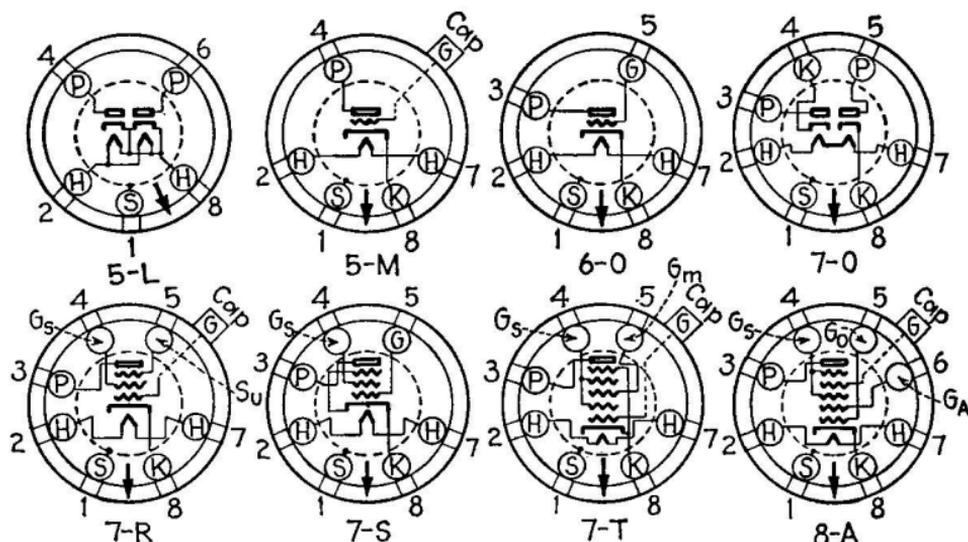
FIG. 243d.—Bottom views of bases for metal tubes.
