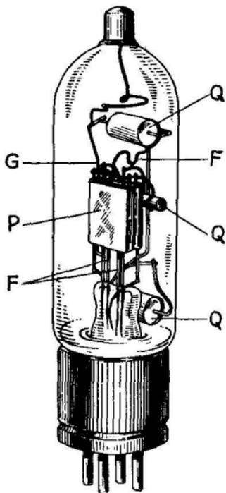
FIG. 109.—Piotron detector tube (FP-54).
