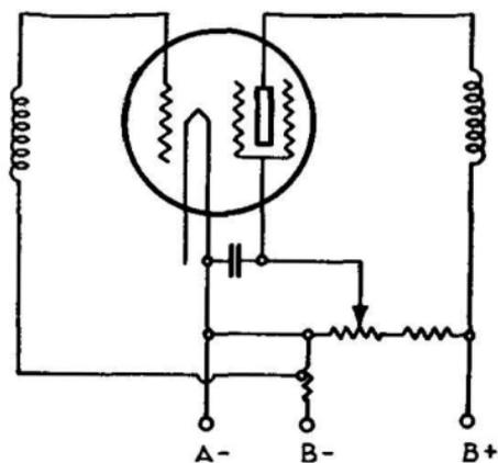
FIG. 253.—Volume-control arrangement using screen-grid voltage variation.
