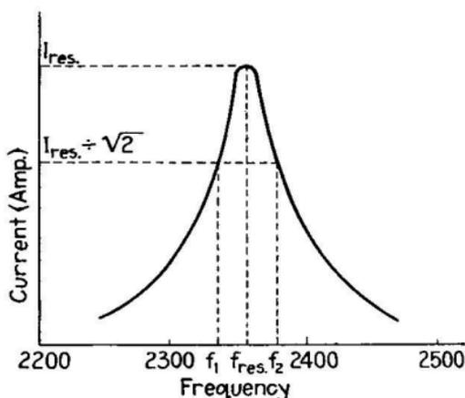
FIG. 35.—Typical resonance curve.
