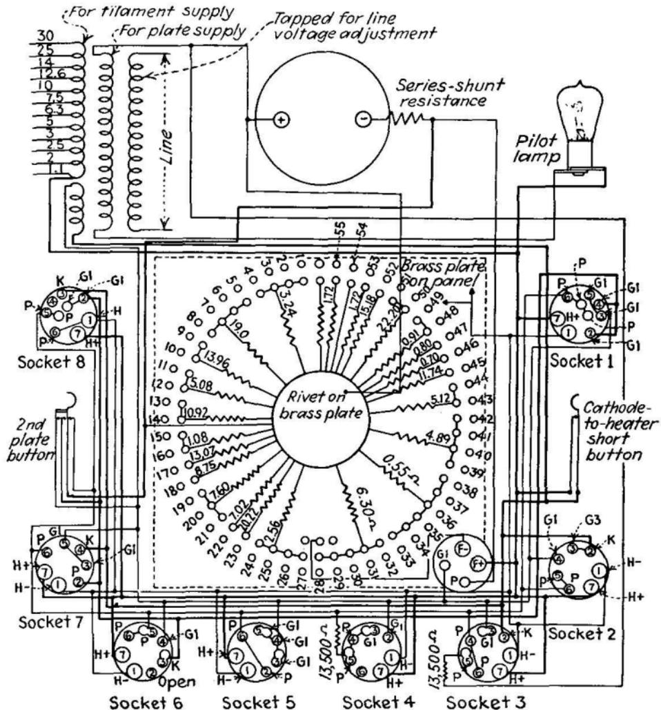
Fig. 228.—Wiring diagram of "Confidence" No. 6 tube tester.
