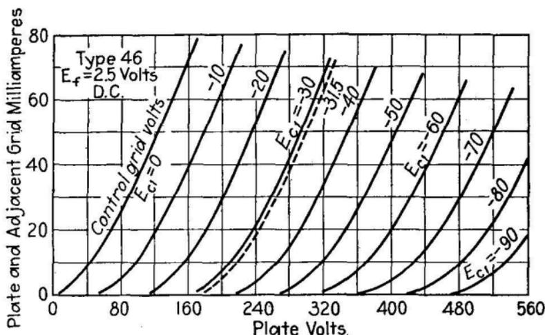
FIG. 67.—Average plate characteristics of type 46 tube used as class A amplifier.
