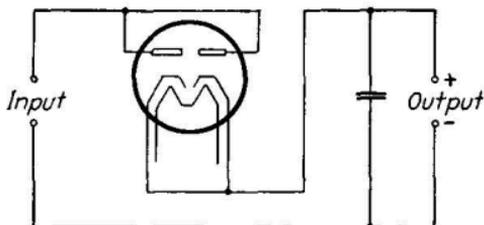
FIG. 304.—Half-wave rectifier using 25Z5 tube.
