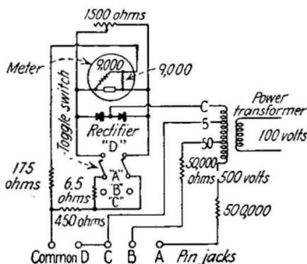
FIG. 206.—Circuit of Hickok capacity meter.
