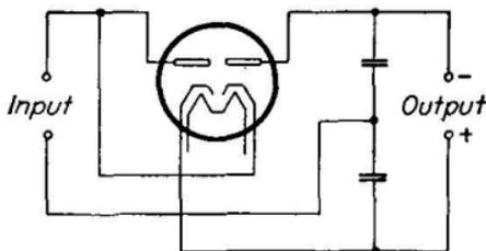
FIG. 305.—Voltage-doubling rectifier using 25Z5 tube.
