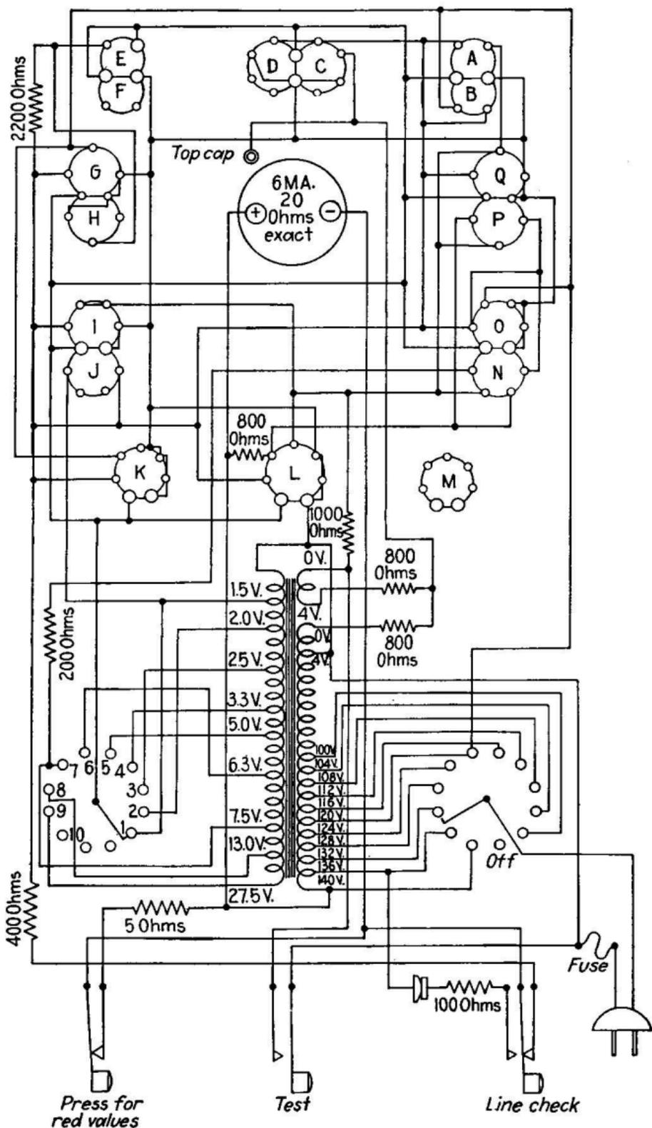
FIG. 238.—Wiring diagram of Weston Model 661 tube tester.
