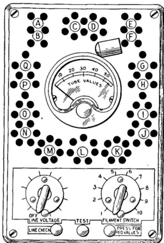
FIG. 237.—Panel of Weston Model 661 tube tester.
