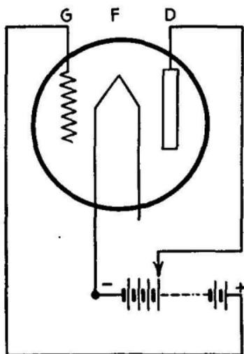
FIG. 185.—Dynatron connection for a three-element tube.
