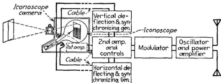
FIG. 438.—Iconoscope transmitting equipment.
