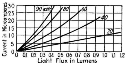
FIG. 175.—Operating characteristics of gas-filled photoelectric tube (type SK-60).
