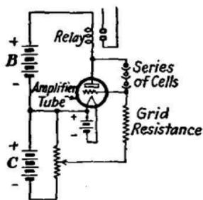
FIG. 387.—Photoelectric tubes in series.
