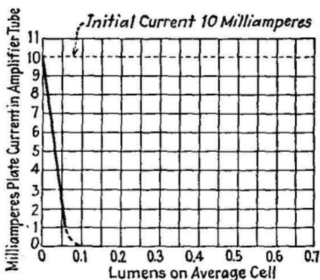
FIG. 382.—Response curve of reverse circuit.
