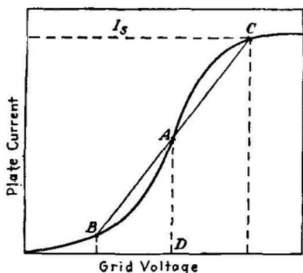
FIG. 404.—Variation of oscillation with grid voltage.
