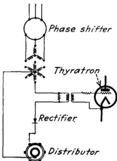
FIG. 474.—Circuit connections of thyatron motor with grid circuit.
