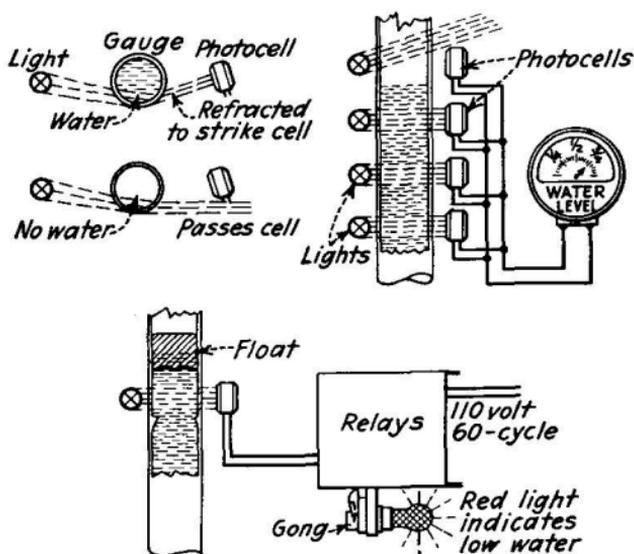
FIG. 469.—Photoelectric water-level indicator.
