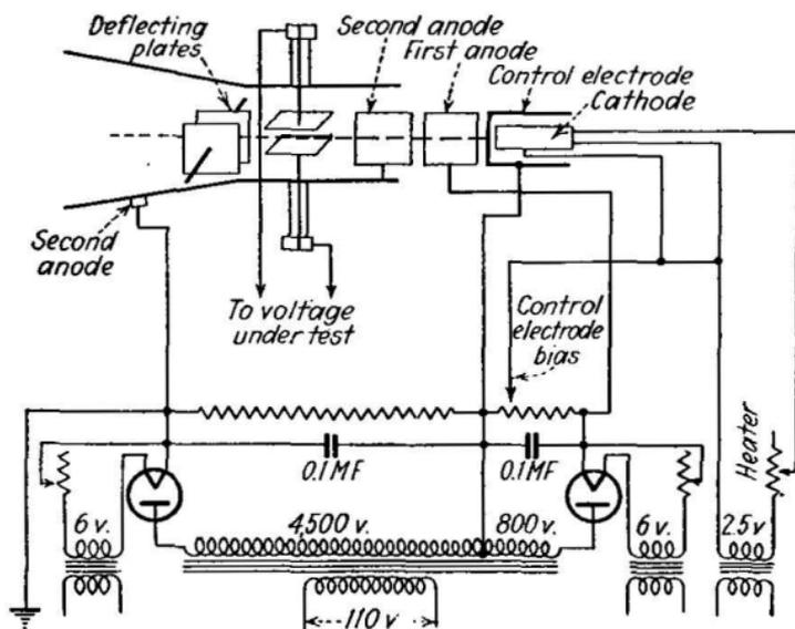
FIG. 320.—Rectifier supplying focusing and accelerating voltages to cathode-ray tube.
