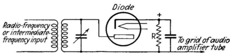
FIG. 259.—Half-wave rectification with diode.
