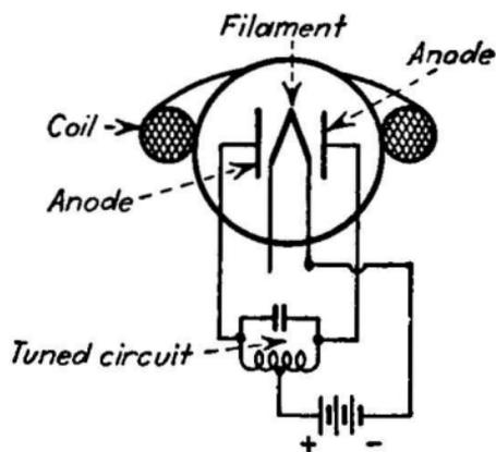
FIG. 189.—Magnetron for generation of high-frequency power.
