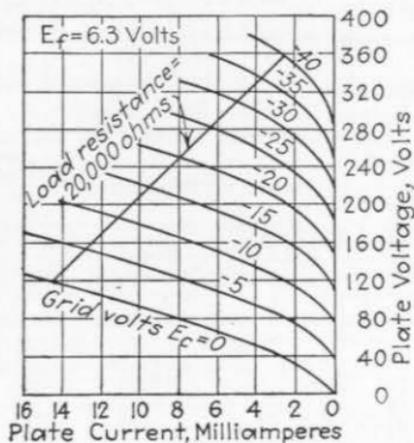
FIG. 86.—Plate characteristics of triode unit (tube type 85).
