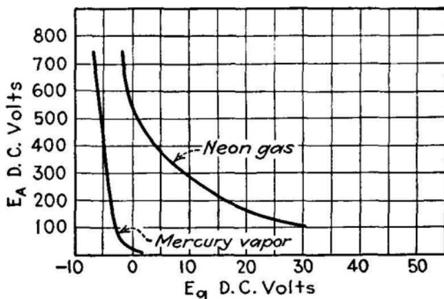
FIG. 144.—Comparison of operating characteristics of neon-filled tube and mercury-vapor tube.
