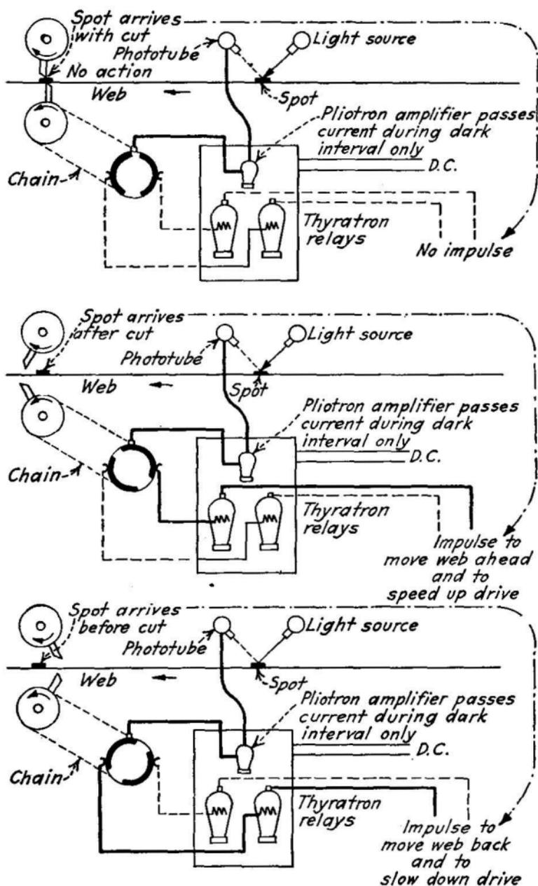
Fig. 463b.—Arrangement of apparatus for register control.
