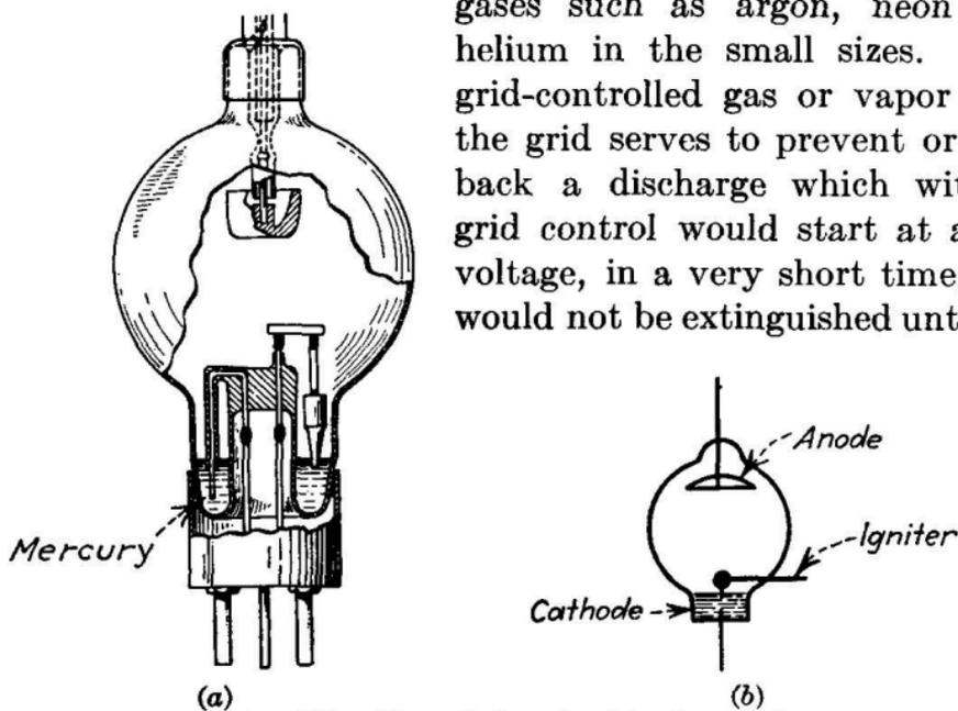
FIG. 155.—Essential parts of ignitron tube.
