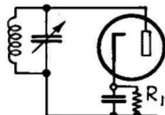
FIG. 276.—Typical two-element tube circuit for detection.
