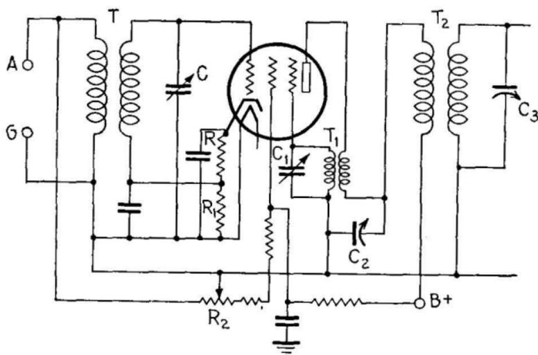
FIG. 409.—Triple-grid tube in oscillator-mixer circuit.
