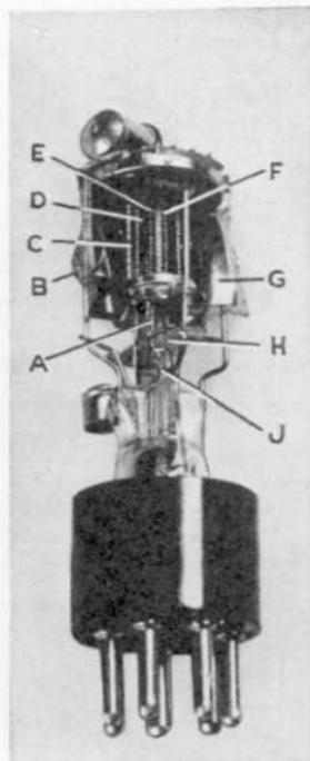
FIG. 99.—Triode-pentode tube.
