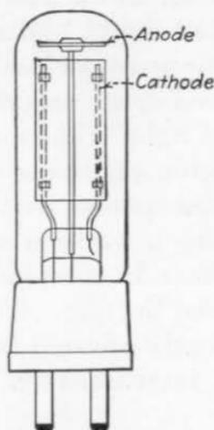
FIG. 172.—Elements of photoelectric tube.
