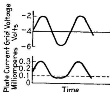
FIG. 269.—Relation of plate current to grid voltage at  $B$  in Fig. 267.
