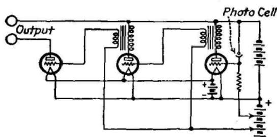
FIG. 390.—Transformer-coupled amplifier including photoelectric tube.
