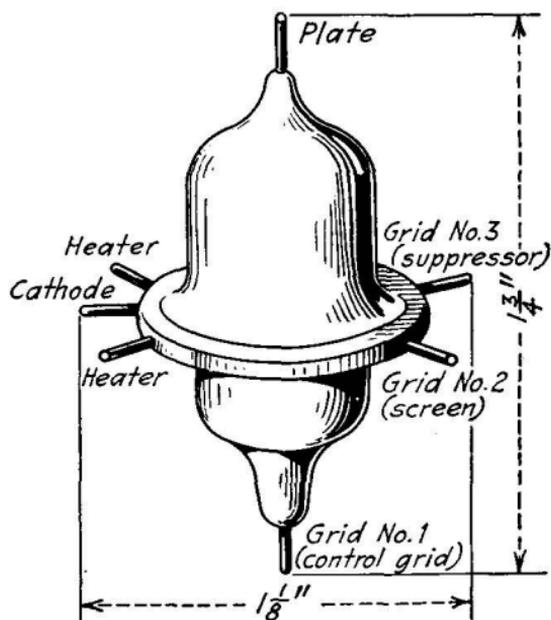
FIG. 128.—Midget pentode tube (type 954).
