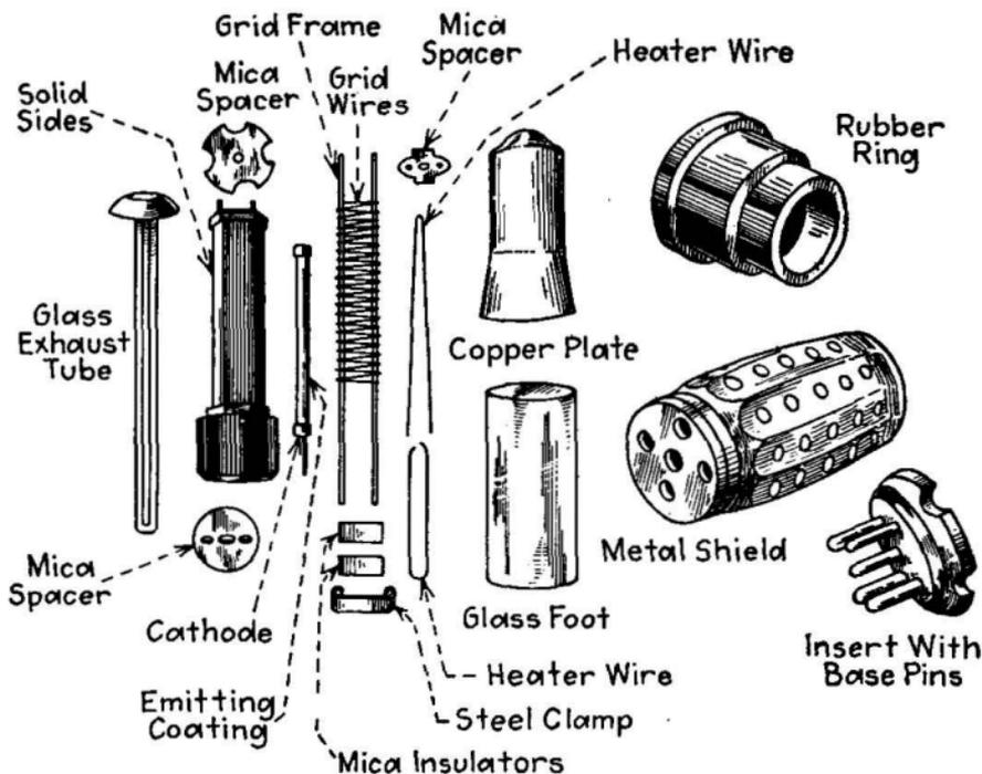
FIG. 107.—Parts of Catkin metal screen-grid tube.
