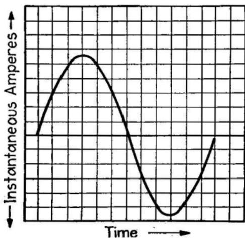
FIG. 22.—Typical sine wave of alternating current.
