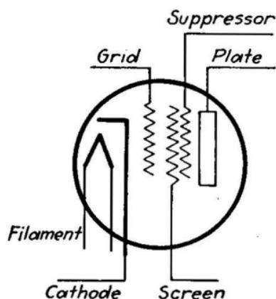
FIG. 63.—Conventional representation of pentode.
