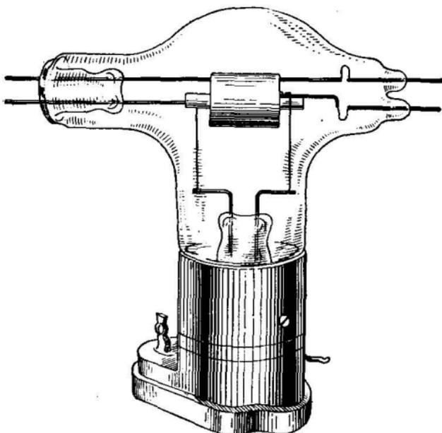
FIG. 423.—Typical positive-grid oscillator tube.
