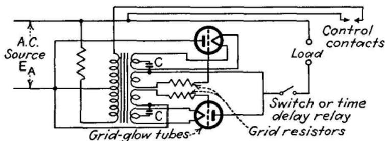
FIG. 152.—Circuit including contact-control tubes for relay action for spot welding.
