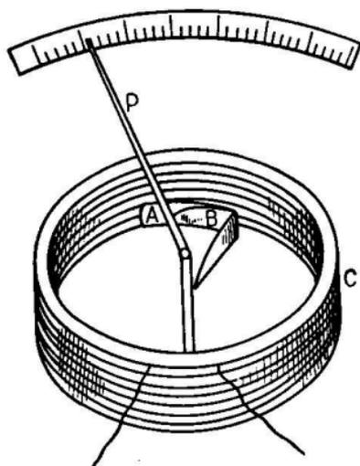
FIG. 195.—Alternating-current voltmeter.
