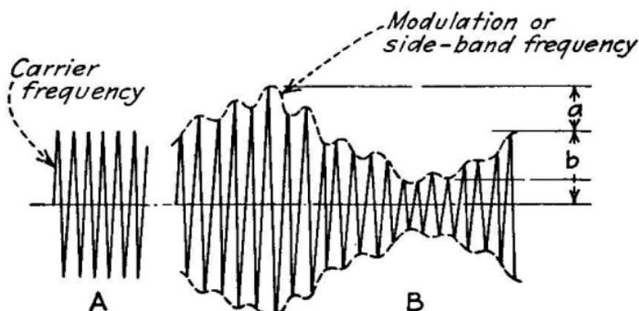
FIG. 257.—Carrier and modulation frequencies.
