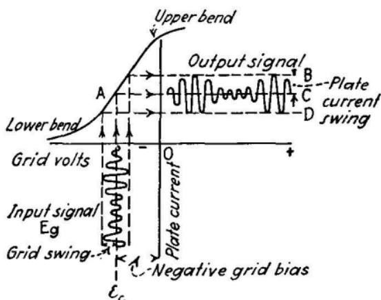
FIG. 325.—Static characteristic curve of simple amplifier.
