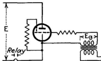
FIG. 143.—Circuit for cold-cathode gaseous tube with external source of grid-bias voltage for control.
