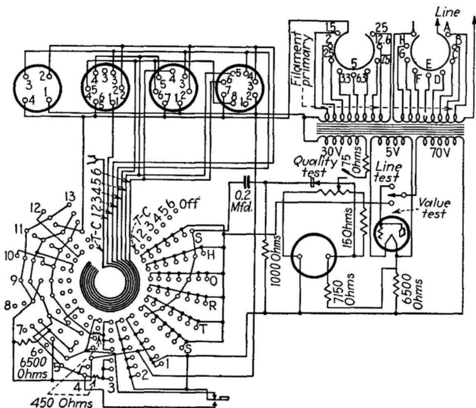
FIG. 242b.—Wiring of Triplett tube tester.
