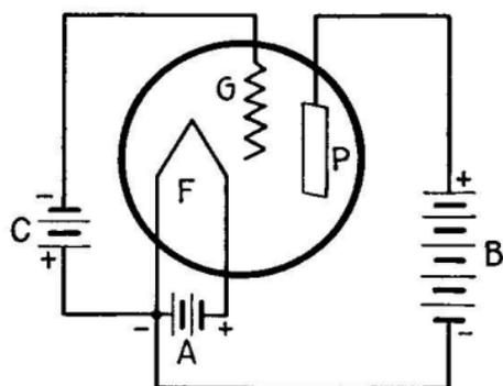
FIG. 44.—Conventional representation of three-element tube.
