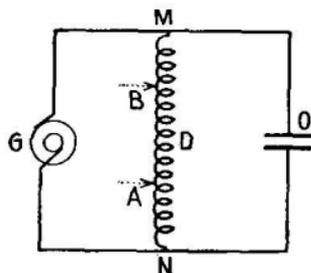
FIG. 38.—Resonance frequency impressed at points of circuit that are varying distances apart.
