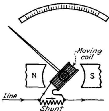
FIG. 194.—Direct-current ammeter with shunt connection.
