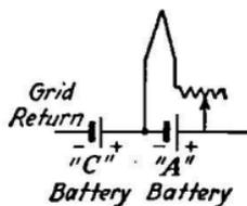
FIG. 271.—Part of circuit in Fig. 270 changed by adding "C" battery and putting rheostat in positive leg of filament.
