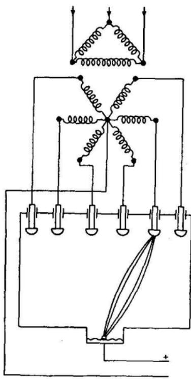
FIG. 319.—Simple method of connecting a mercury-arc rectifier to transformer.
