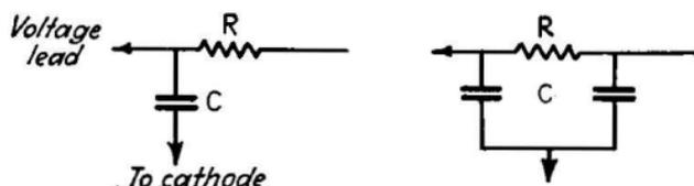
FIG. 254.—Electric filters for voltage-supply wires.
