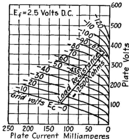
FIG. 337.—Power-output of twin triode used as class A amplifier.
