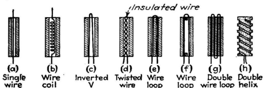
FIG. 5.—Tungsten heating elements.
