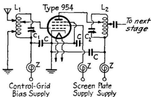
FIG. 131.—Circuit of radio-frequency amplifier using midget pentode tube (type 954).
