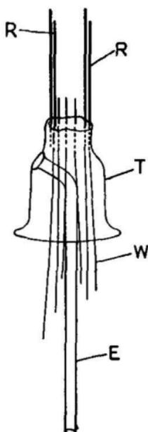
FIG. 8.—Method of fusing capillary tube into flanged glass bell.
