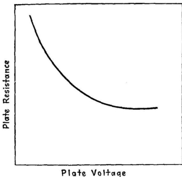
FIG. 49.—Relation of plate resistance to plate voltage at zero grid voltage.
