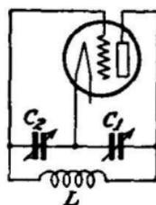
FIG. 402.—Colpitts oscillating circuit.
