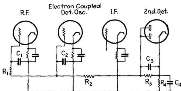
FIG. 360.—Circuit providing grid-bias voltage to detector unit of pentagrid converter for automatic volume control.
