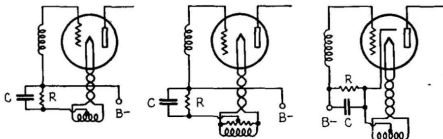
FIG. 244.—Self-biasing method of obtaining grid-bias voltage.
