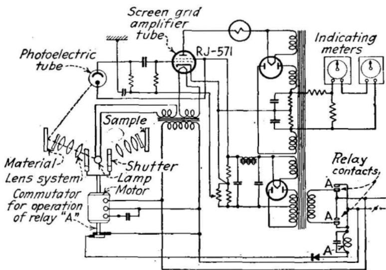
FIG. 455.—Circuit diagram of concentration indicator.
