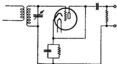
FIG. 266.—Simple diode-detector circuit.
