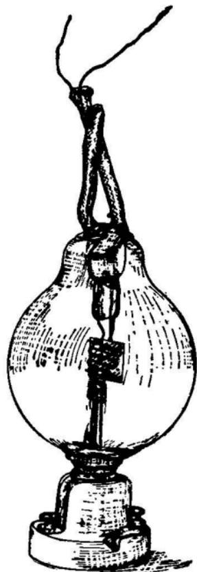
FIG. 3.—Three-element vacuum tube as constructed by deForest.
