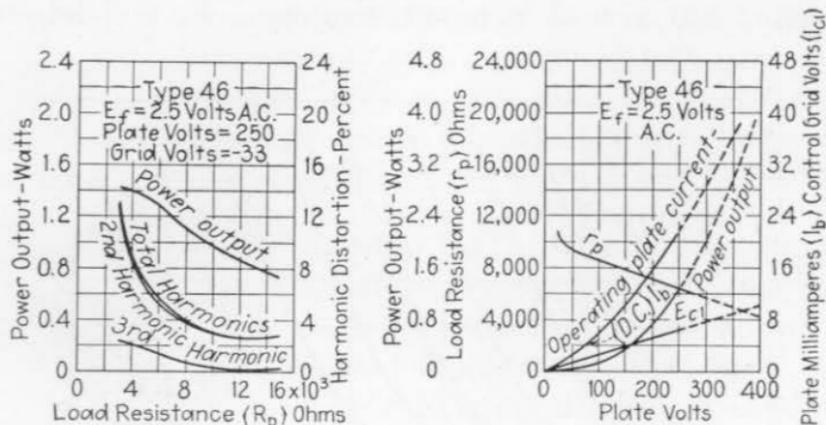
FIG. 69.—Operation characteristics of type 46 tube.
