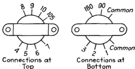
FIG. 226.—Power-transformer connections for Model 304 tube tester.
