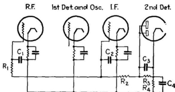
FIG. 359.—Circuit details for automatic volume control.
