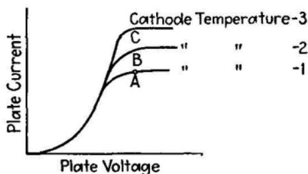
FIG. 42.—Relation of plate current to cathode temperature.
