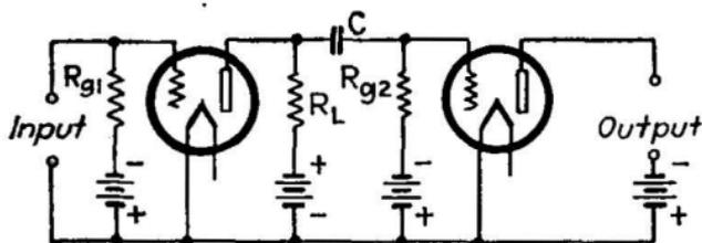
FIG. 374.—Resistance-coupled amplifier.
