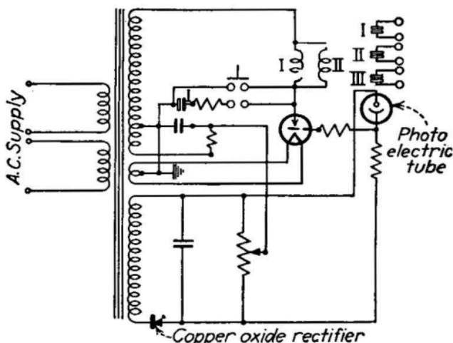
FIG. 454.—Circuit diagram for heater control.
