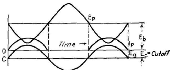
FIG. 330.—Average characteristics of ideal class *B* amplifier.
