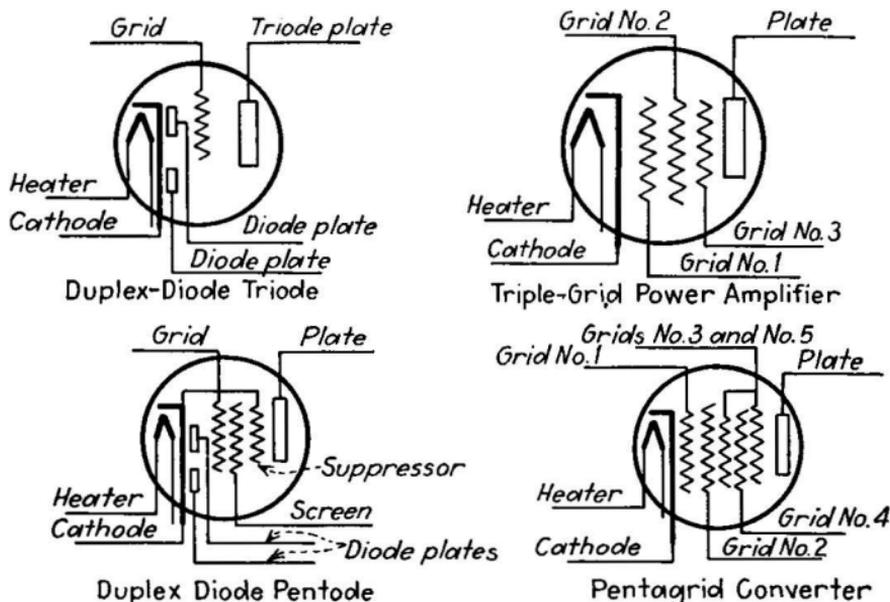
FIG. 65.—Usual representations of multi-electrode and multi-unit tubes.
