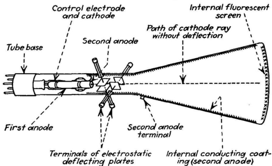
FIG. 183.—Typical cathode-ray tube.
