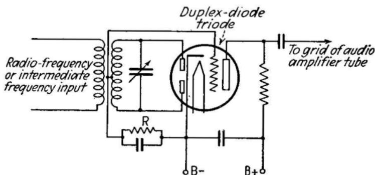
FIG. 260.—Full-wave rectification with duplex-diode triode.
