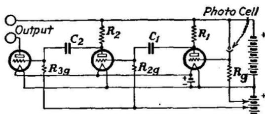
FIG. 389.—Condenser-coupled amplifier including photoelectric tube.
