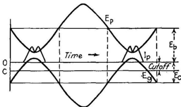
FIG. 331.—Average characteristics of ideal class *C* amplifier.
