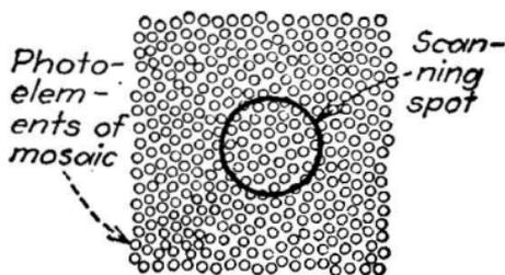
FIG. 432.—Scanning spot on photoelectric elements.
