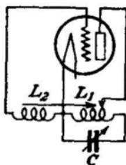
FIG. 401.—Tuned-plate oscillating circuit.
