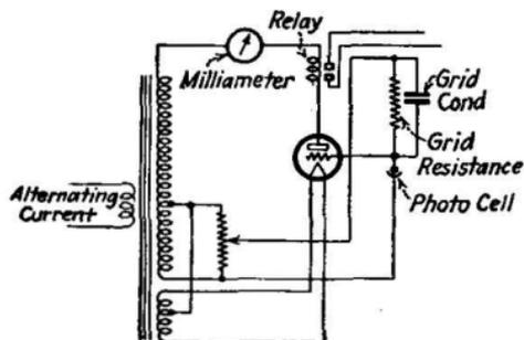
FIG. 385.—Reverse circuit for alternating-current operation
