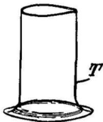
FIG. 6.—Glass support for vacuum tube.
