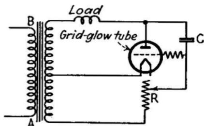
FIG. 147.—Circuit of half-wave rectifier using hot-cathode gaseous power tube.
