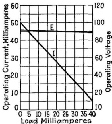
FIG. 164.—Operation characteristics of UX-874 tube.
