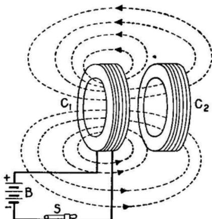
FIG. 31.—Mutual induction between two coupled coils.
