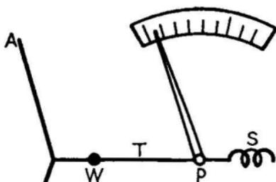
FIG. 197.—Hot-wire ammeter.
