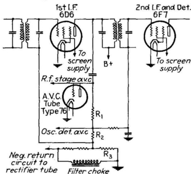
FIG. 358.—Retroactive circuit for automatic volume control.
