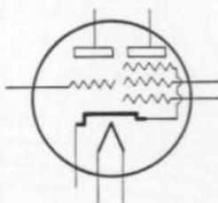
FIG. 100.—Conventional representation of triode-pentode tube (type 6F7).
