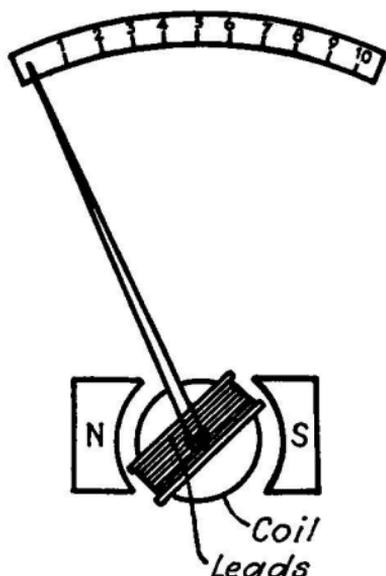
FIG. 190.—Direct-current voltmeter.
