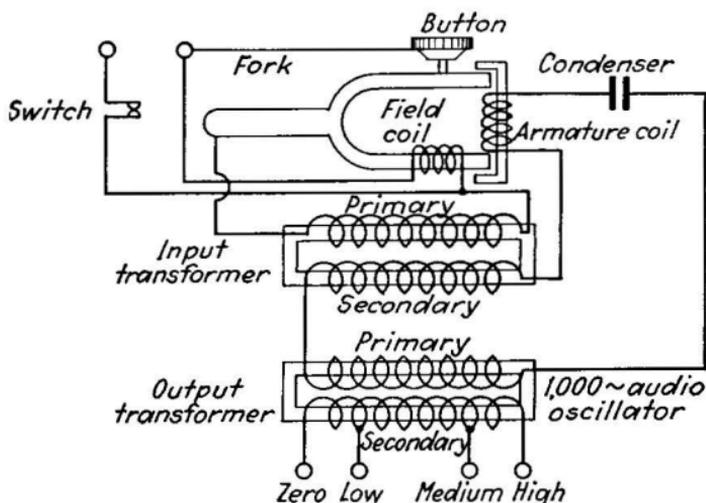
FIG. 209.—Circuit of audio-frequency oscillator.
