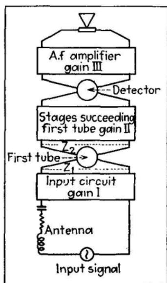
FIG. 394.—Diagrammatic representation of typical radio receiver.
