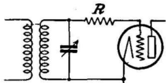
FIG. 364.—Method of stabilizing circuits by use of grid resistance to prevent oscillation.
