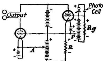
FIG. 388.—Resistance-coupled amplifier including photoelectric tube.
