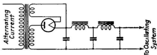
FIG. 480.—Circuit to provide direct current for surgical needle from alternating-current supply.
