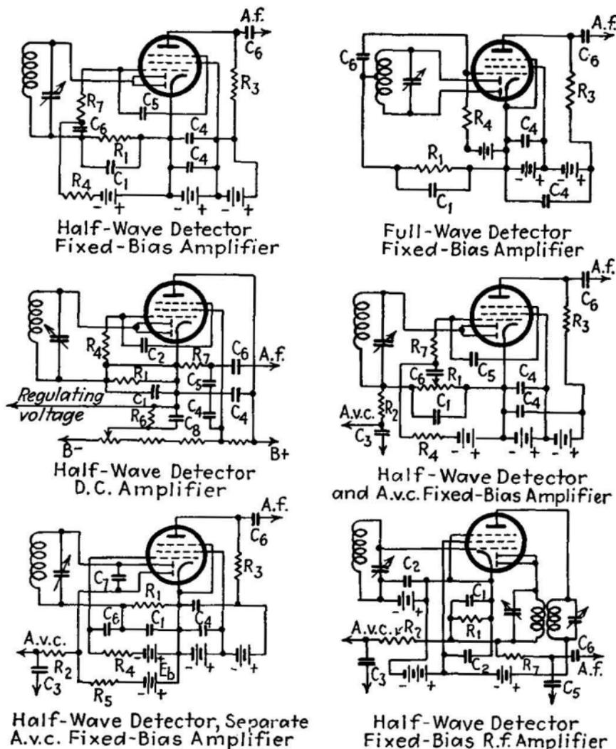
FIG. 89.—Typical circuit diagrams of duplex-diode pentode.
