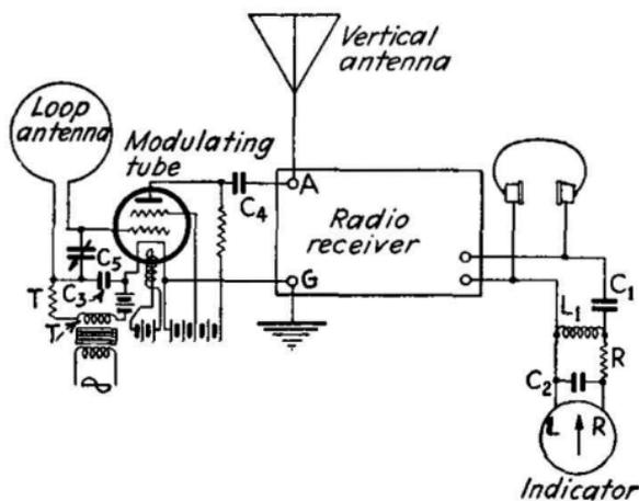
FIG. 483.—Circuit of radio compass for air navigation.
