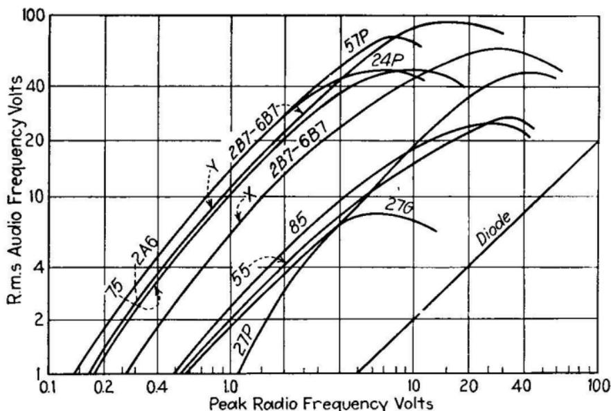
FIG. 275.—Average performance of typical detector tubes.
