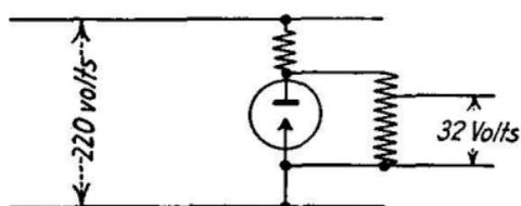
FIG. 161.—Glow lamp used for constant low-voltage supply from higher voltage source.
