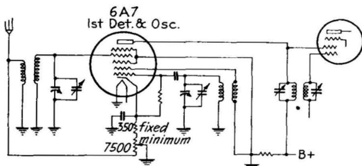
FIG. 350.—Circuit for manual volume control.
