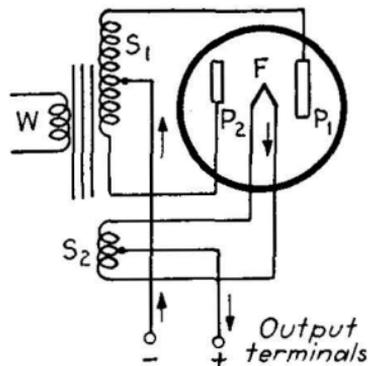
FIG. 289.—Rectifier circuit for full-wave rectification.
