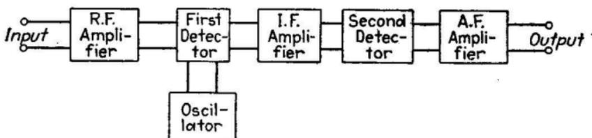
FIG. 368.—Typical superheterodyne receiving set
