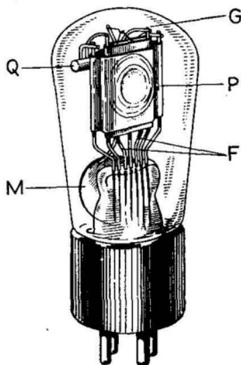
FIG. 110.—Low-noise Pliotron tube for measuring small voltages.
