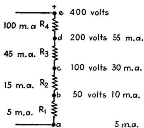
FIG. 312.—Conventional voltage divider.
