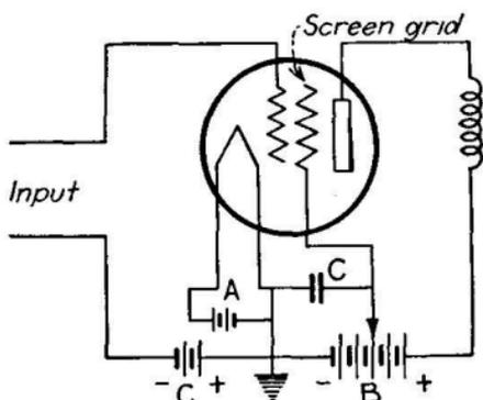
FIG. 54.—Connection of electrodes of screen-grid tube.
