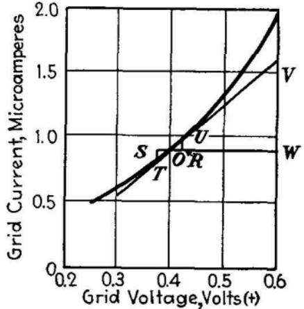
FIG. 223.—Method of obtaining input conductance from slope of curve showing relation between grid current and grid voltage.
