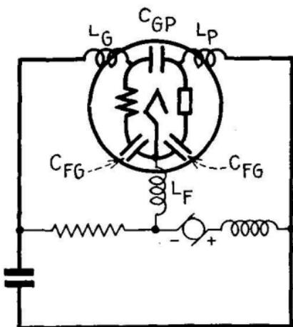
FIG. 418.—Limiting circuit of Colpitts oscillator.
