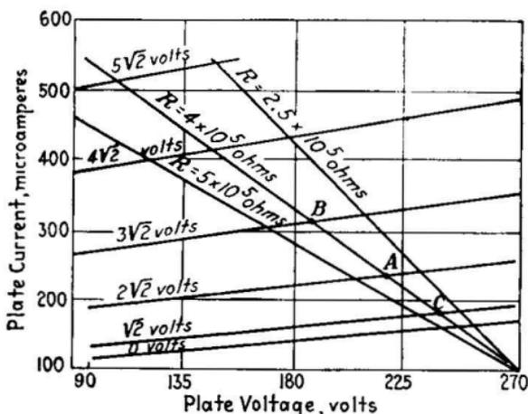
FIG. 283.—Relation of plate current to plate voltage in UX-222 tube for various input voltages and loads.
