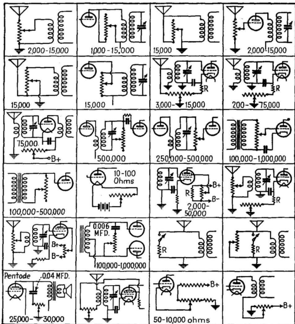
FIG. 349.—Typical volume-control arrangements.
