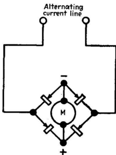
FIG. 196.—Combination of four copper-oxide rectifiers with ammeter.
