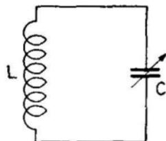
FIG. 411.—Typical radio-frequency circuit in superheterodyne receiver.
