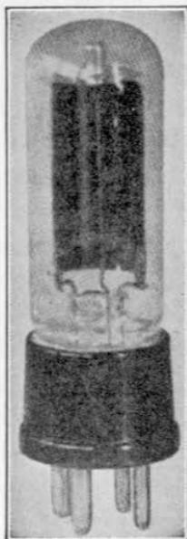
FIG. 171.—Typical photoelectric tube.
