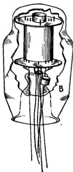
FIG. 14.—Glass bulb used to cover assembled unit.
