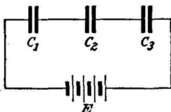
FIG. 25.—Condensers in parallel.      FIG. 26.—Condensers in series.
