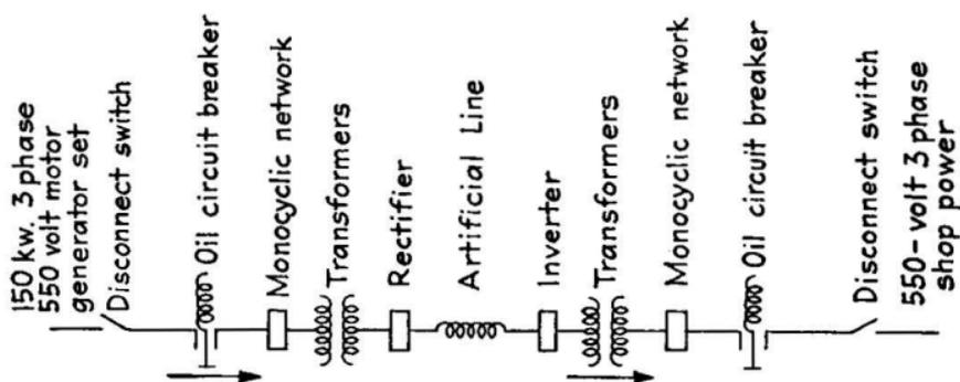
FIG. 471.—Direct-current constant-current transmission system.
