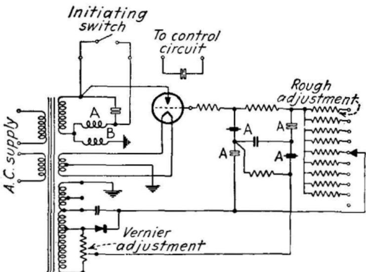
FIG. 457.—Circuit diagram of electronic timer.
