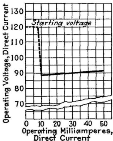
FIG. 163.—Regulation characteristics of UX-874 tube.
