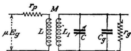
FIG. 362.—Equivalent circuit of tuned radio-frequency stage.
