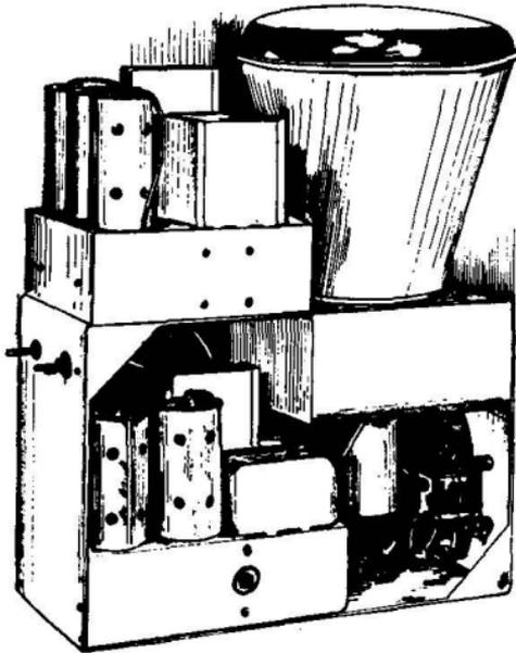
FIG. 446.—Deflecting unit of iconoscope.
