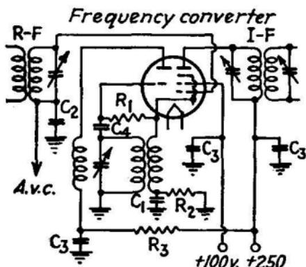
FIG. 103.—Circuit using triode-pentode (type 6F7) as frequency converter in superheterodyne receiver.
