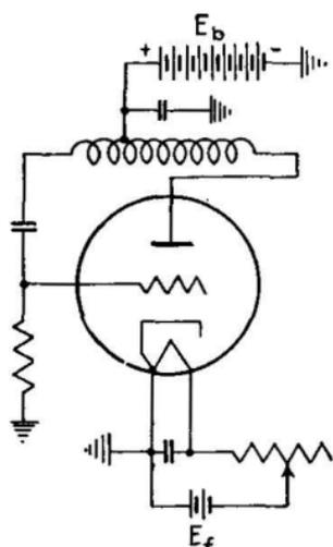
FIG. 119.—Circuit of small triode oscillator.
