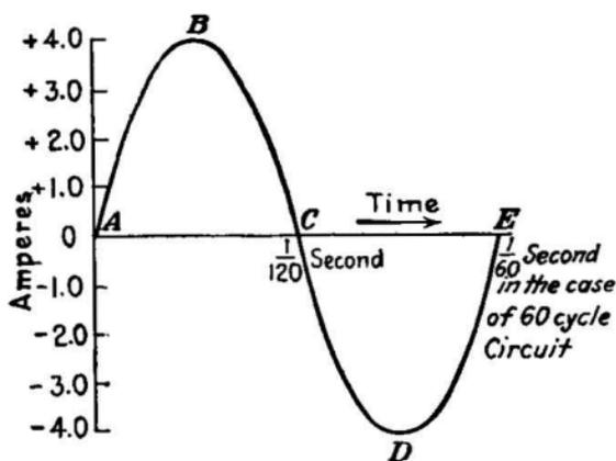
FIG. 21.—Diagram showing variations of alternating current with time (one cycle).
