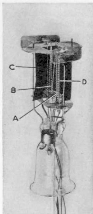
FIG. 66.—Typical dual-grid power amplifier.
