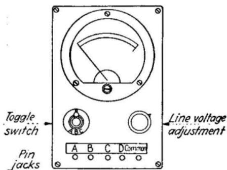
FIG. 205.—Hickok capacity meter.
