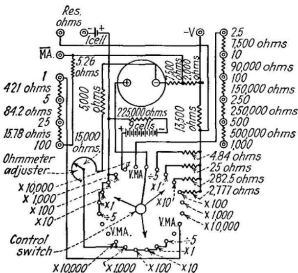
FIG. 201.—Wiring diagram of Weston ohmmeter.
