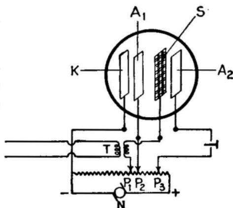
FIG. 167.—Typical circuit for application of cold-electrode tube.
