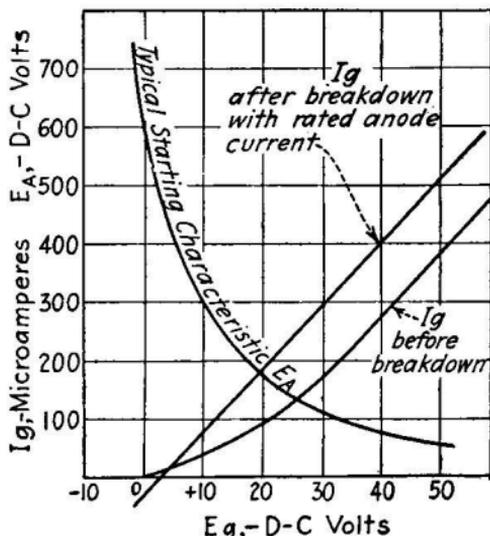
FIG. 137.—Direct-current characteristics of gaseous tube (type KU-610).
