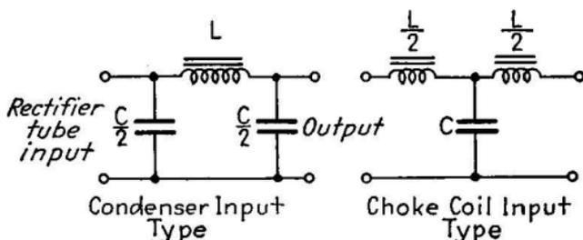
FIG. 294.—Two types of filter sections.
