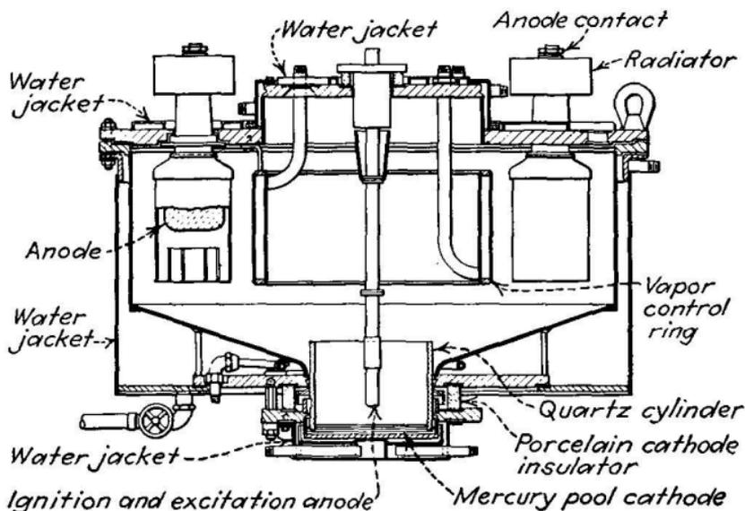
FIG. 154.—Construction details of typical Westinghouse mercury-arc rectifier.
