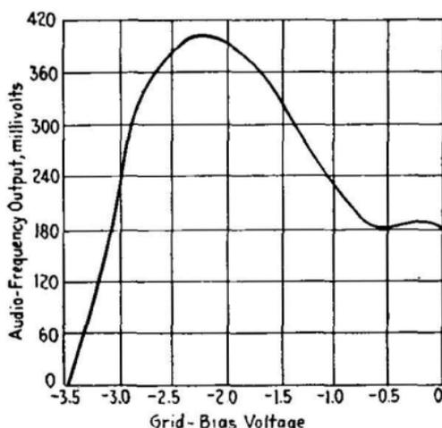
FIG. 281.—Variation of audio-frequency output with changes of grid-bias voltage for UX-200A tube.
