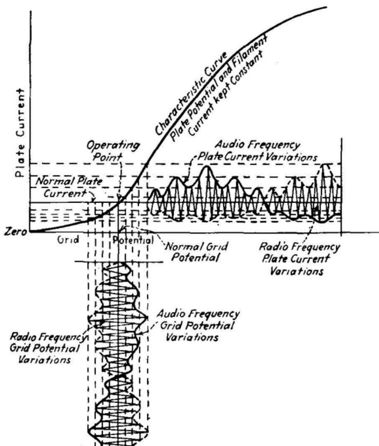
FIG. 272.—Detection of continuous oscillations as modified by the voice.
