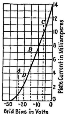
FIG. 379.—Characteristics of typical amplifier tube.
