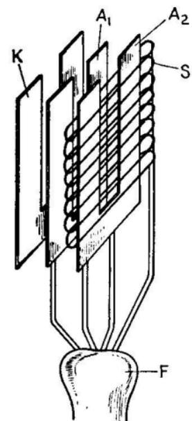
FIG. 168.—Construction details of typical cold-electrode tube.
