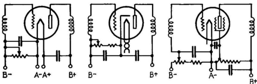
FIG. 251.—Grid-bias voltage variation for volume control.
