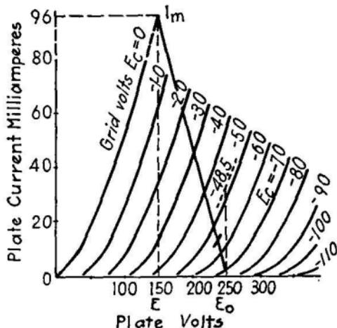
FIG. 335.—Diagram for calculating plate-to-plate load for two triodes in push-pull circuit operated as class A power amplifier.
