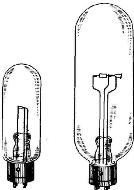
FIG. 476.—Typical arc-oscillator tubes.
