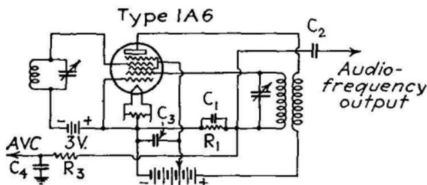
FIG. 98.—Circuit of diode tetrode for half-wave detection, automatic volume control, and radio-frequency amplification.
