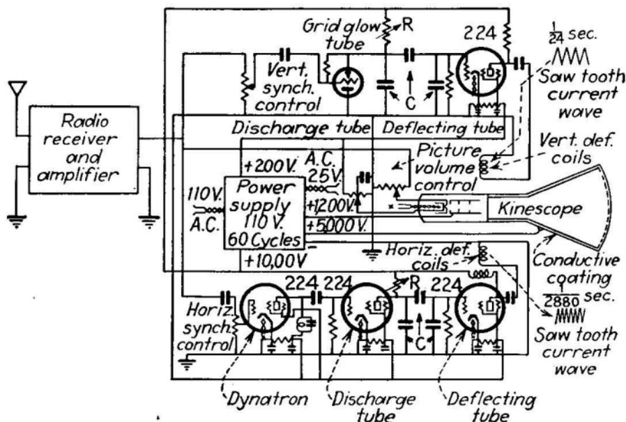
FIG. 444.—Generator for "saw-tooth" deflection current.
