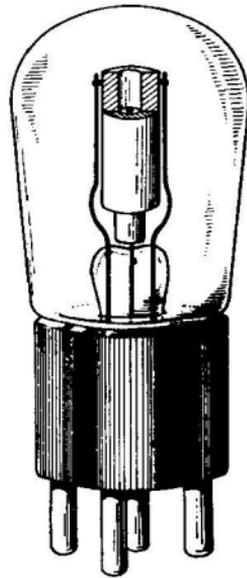
FIG. 157.—Glow lamp with crater type of cathode.
