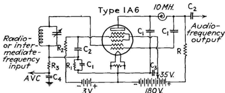
FIG. 97.—Circuit of diode tetrode for half-wave detection, automatic volume control, and fixed grid-biased audio-frequency amplification.
