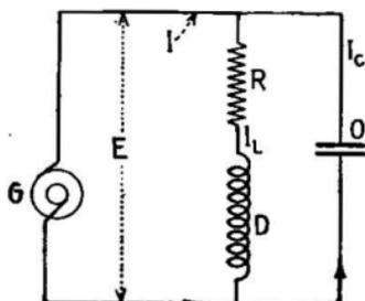
FIG. 36.—Parallel resonance of inductance and condenser.
