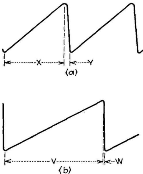
FIG. 443.—Intensity of magnetic fields for unidirectional scanning.
