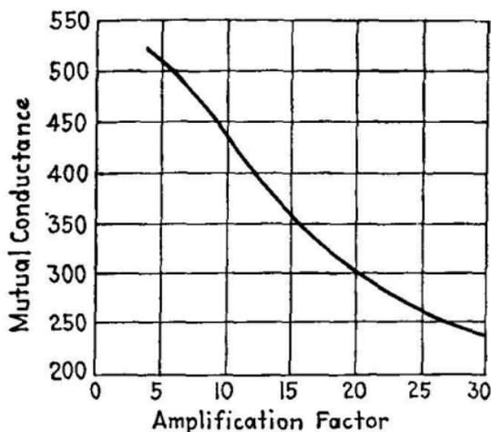
FIG. 50.—Relation of mutual conductance to amplification factor.
