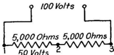
FIG. 191.—Simple electric circuit including two equal resistances.
