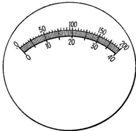
FIG. 233.—Dial of plate milliammeter in Hickok Model AC-47 tube tester.
