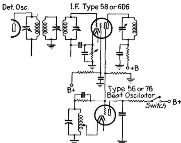
FIG. 413.—Beat-frequency oscillator circuit.
