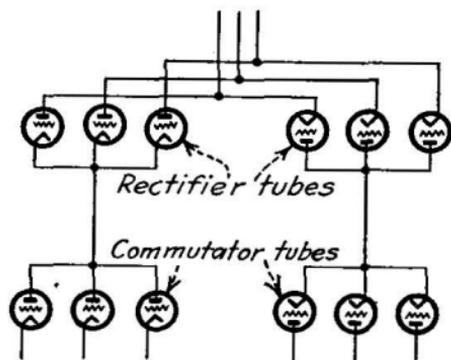
FIG. 475.—Arrangement of commutator tubes and rectifier tubes for grid control in thyatron motor.
