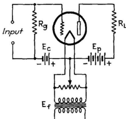
FIG. 372.—Simple amplifier circuit.
