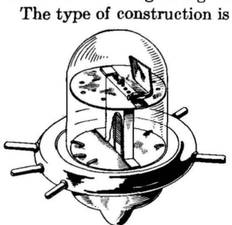
FIG. 123.—Midget triode tube (type 955).
