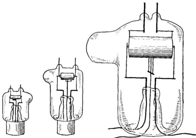
FIG. 426.—Three positive-grid oscillator tubes of spiral-grid type.
