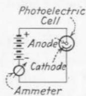
FIG. 173.—Simple photoelectric circuit.
