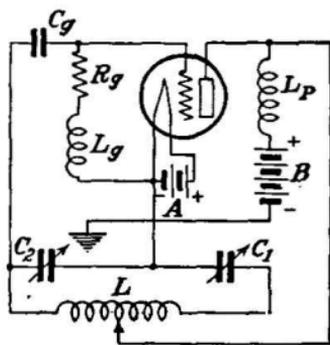
FIG. 405.—Colpitts oscillating circuit arranged for practical operation.
