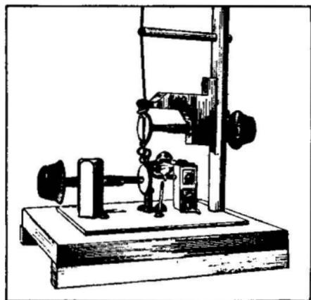
FIG. 120.—Oscillator for 100-centimeter wave lengths.
