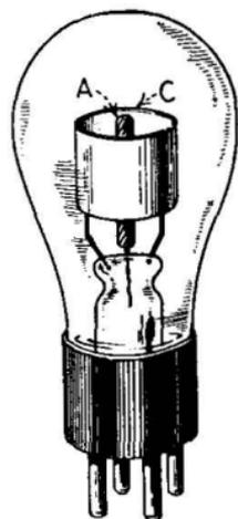
FIG. 162.—Cold-electrode gas-filled, voltage-limiting tube.
