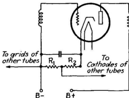
grid-bias voltage for the other tubes is the voltage drop across the resistance  $R_1$ , for the reason that the reference point for those tubes is the junction point of the resistances  $R_1$  and  $R_2$ .
