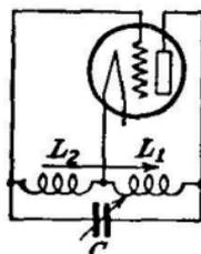
FIG. 399.—Hartley oscillating circuit.
