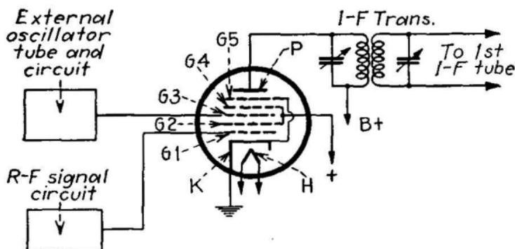
FIG. 108b.—Circuit diagram for type 6L7 tube.
