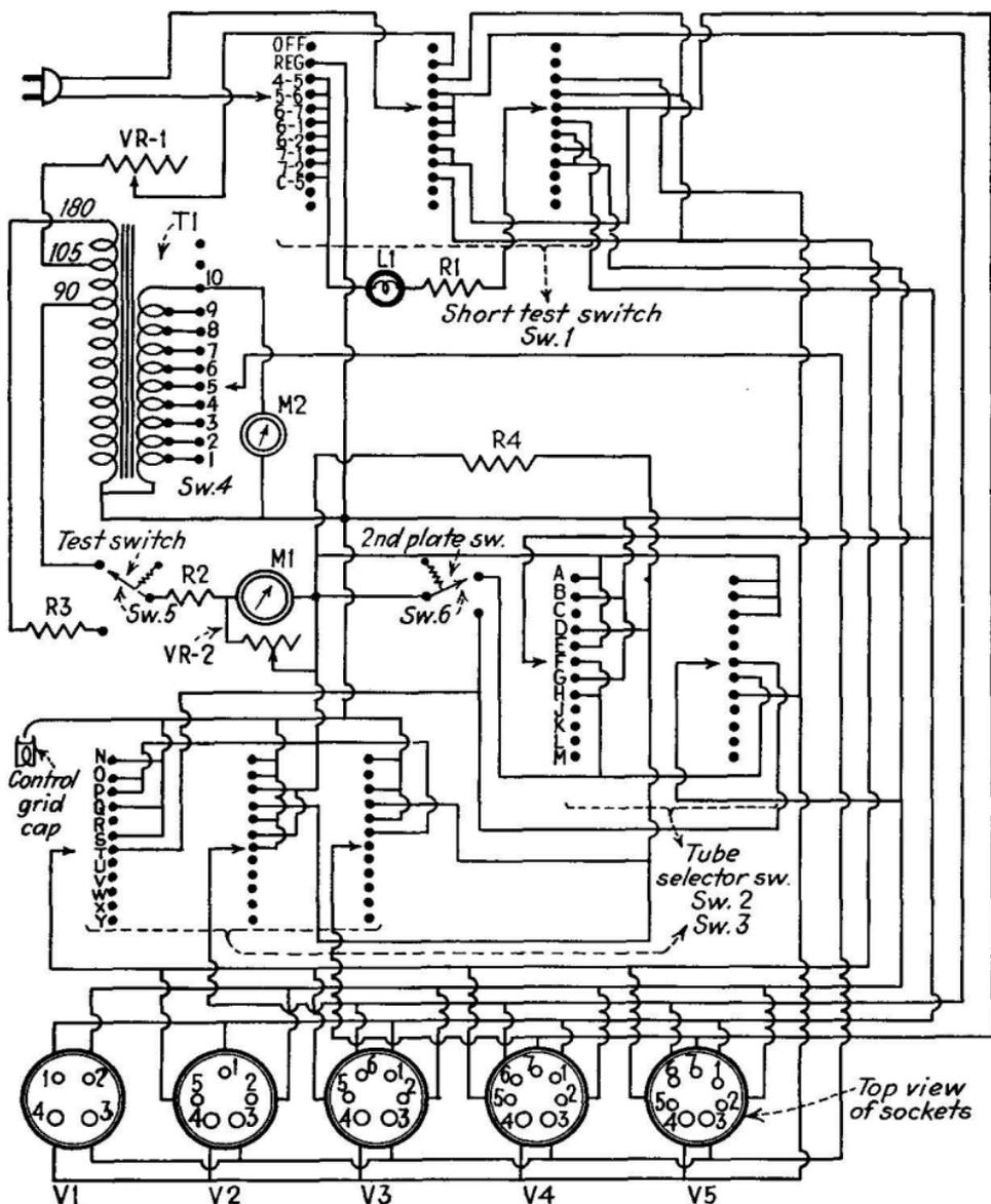
FIG. 225.—Wiring diagram of Model 304 tube tester.
