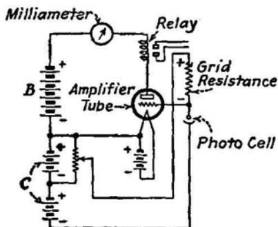
FIG. 381.—Typical direct-current reverse circuit.
