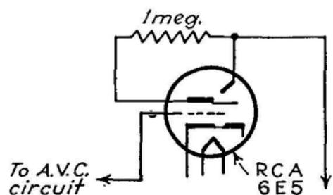
FIG. 367c.—Circuit for tuning indicator.
