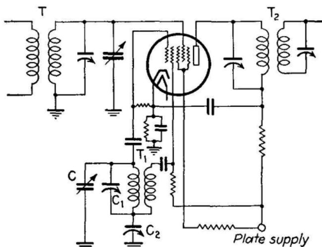
FIG. 410.—Pentagrid-converter tube in oscillator-mixer circuit.
