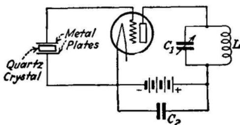
FIG. 403.—Device for frequency control with quartz crystal.
