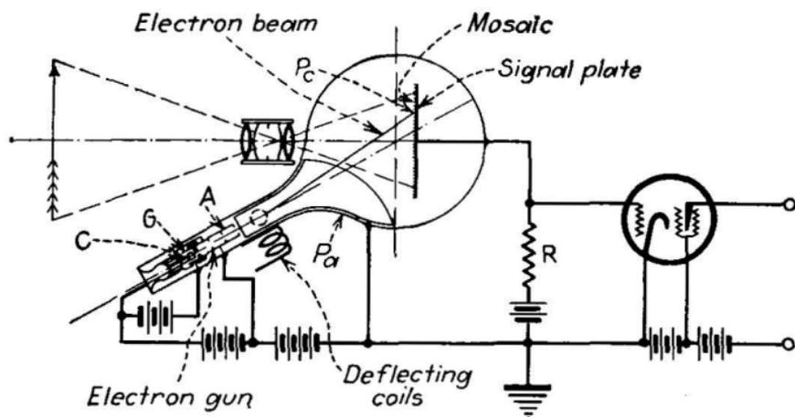
FIG. 428.—Iconoscope circuit.
