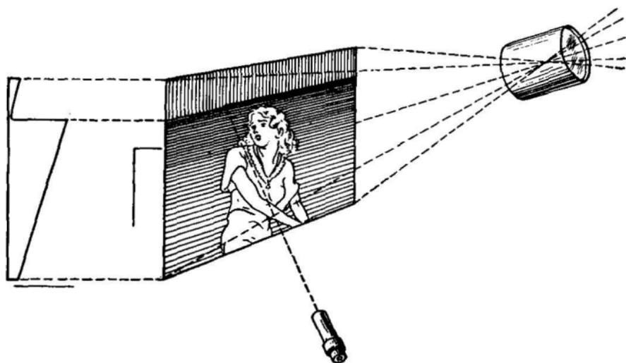
FIG. 431.—Charging conditions on photoelectric surface of iconoscope.
