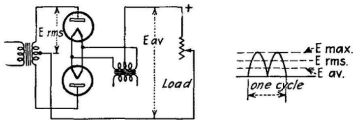
FIG. 306.—Method of rectifying both halves of a cycle with the use of two tubes.
