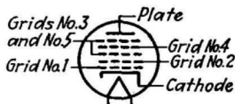
FIG. 94.—Diagram of electrodes in pentagrid converter.
