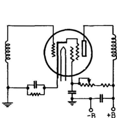
FIG. 252.—Arrangement for obtaining screen-grid voltage.
