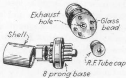
FIG. 106.—Parts of all-metal radio receiving tube.
