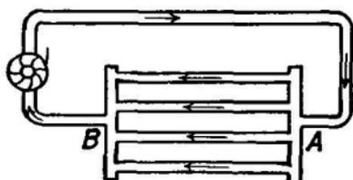
FIG. 19.—Water pipes connected in parallel.
