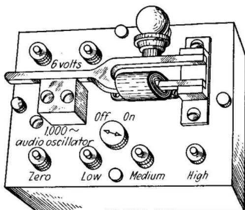
FIG. 208.—Audio-frequency oscillator. (*General Radio.*)
