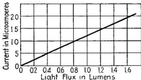
FIG. 174.—High-vacuum photoelectric tube (type SR-50).
