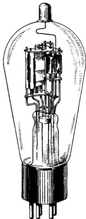
FIG. 79.—Triple-twin tube.
