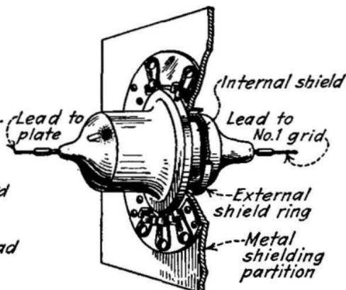
FIG. 130.—Method of shielding midget pentode tube (type 954).
