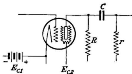
FIG. 284.—Typical circuit using UX-222 tube as detector.
