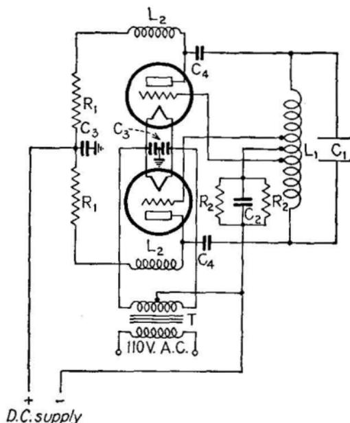
FIG. 415.—Oscillating push-pull circuit for three-electrode tubes.
