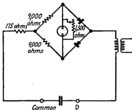
FIG. 207.—Simplified circuit of typical capacity meter.
