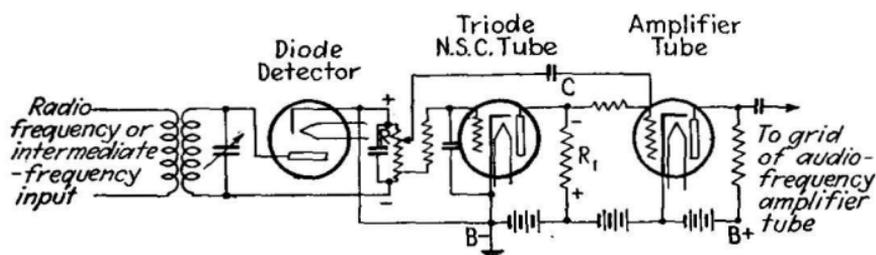
FIG. 353.—Simple circuit for automatic noise suppression.
