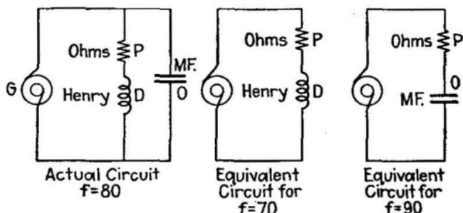
FIG. 37.—Inductance and condenser in parallel: (1) for frequency of resonance; (2) for frequency below resonance; (3) for frequency above resonance.
