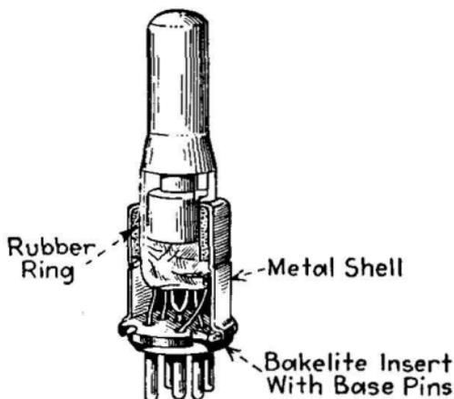
FIG. 108.—Method of attaching to the tube the base of Catkin metal vacuum tube.
