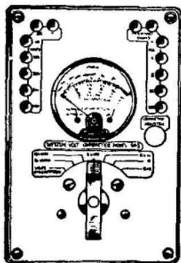
FIG. 200.—Weston volt-ohmmeter.
