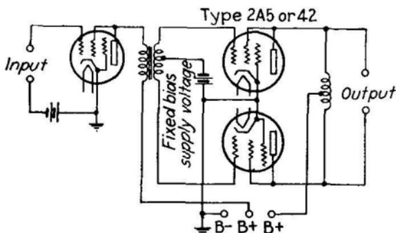
FIG. 247.—Fixed grid-bias arrangement using battery-supply current.
