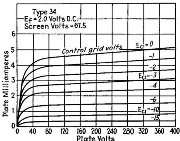
FIG. 61.—Average plate characteristics for type 34 tube.
