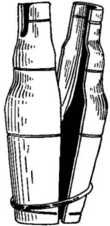
FIG. 485.—Metal shield for radio tubes made in halves.
