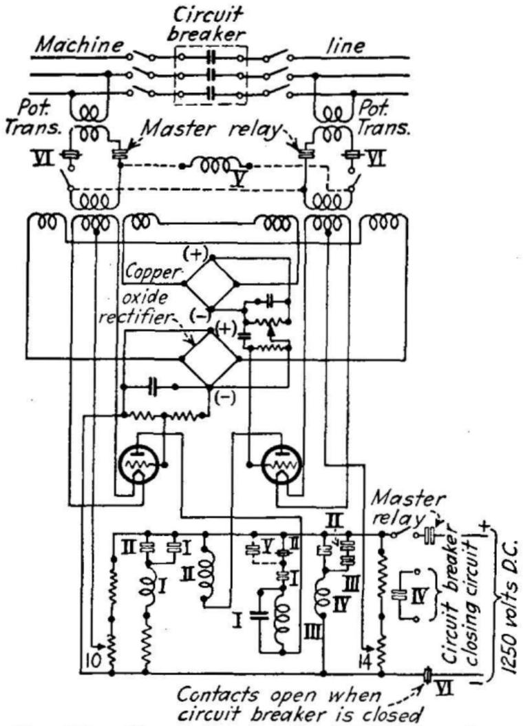
FIG. 456.—Circuit diagram of synchronizing relay.
