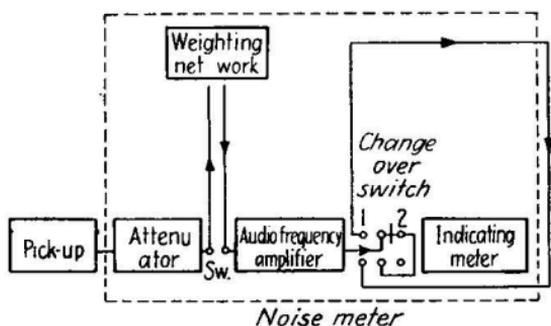
FIG. 482.—Acoustic noise meter.
