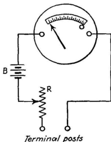
FIG. 199.—Simple ohmmeter.
