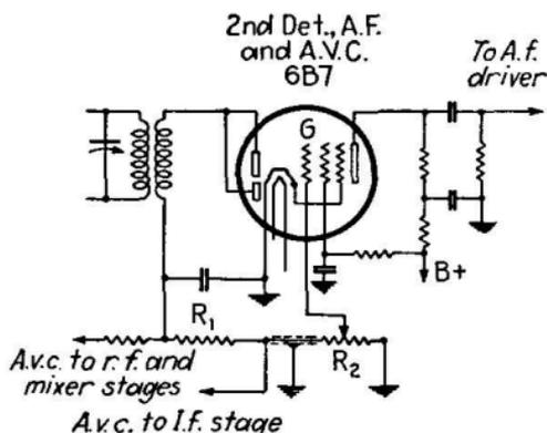
FIG. 357.—Automatic volume control on audio-frequency section of tube.
