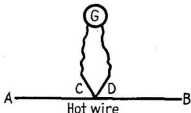
FIG. 98.—Thermocouple ammeter.
