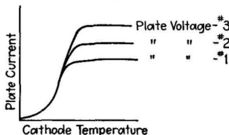
FIG. 43.—Relation of plate voltage to cathode temperature.
