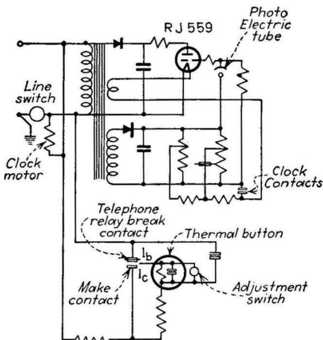
FIG. 452.—Circuit diagram for lighting control.
