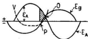
FIG. 146.—Instantaneous values of grid-bias voltage at which hot-cathode gaseous power tube breaks down.
