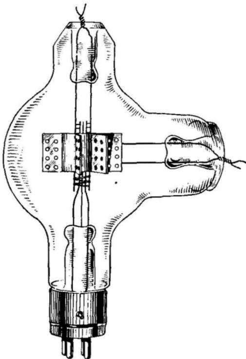
FIG. 419.—Typical air-cooled high-frequency oscillator.
