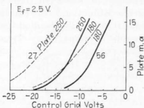
FIG. 81.—Relation of plate current to control-grid voltage in typical triode tube (types 27 and 56).
