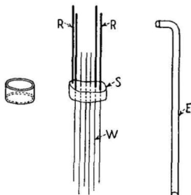
FIG. 7.—Construction of supporting posts and lead-in wires.
