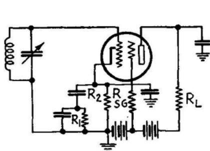
FIG. 277.—Typical detection circuit for four-element tubes.
