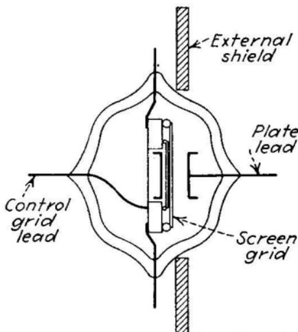
FIG. 114.—Bulb and shield for midgrid tetrode tube.
