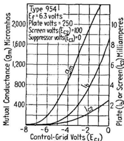
FIG. 133.—Average characteristics of midget pentode tube (type 954).
