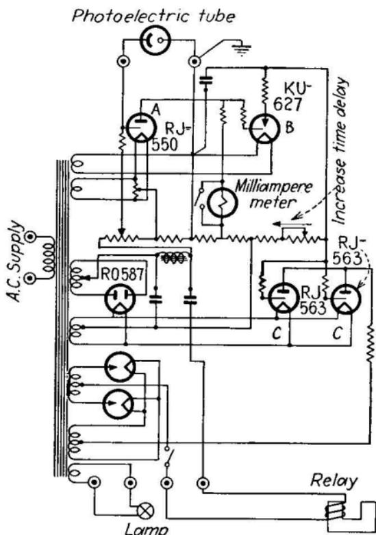
FIG. 451.—Photoelectric controller with time delay.
