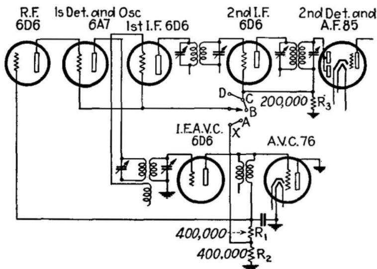
FIG. 356.—Circuit for double-automatic-volume control.
