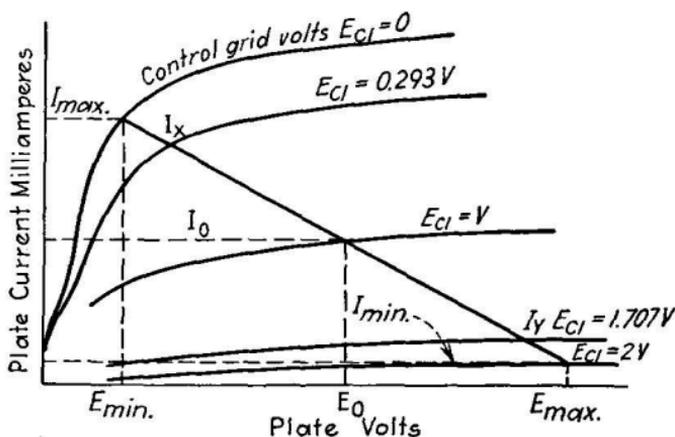
FIG. 336.—Average characteristics of pentode used as class A amplifier.
