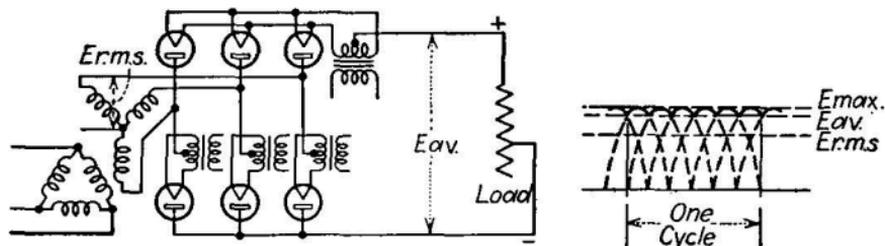
FIG. 310.—Three-phase rectifier circuit using six tubes with full-wave rectification.
