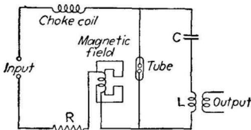
FIG. 477.—General purpose arc-tube circuit.
