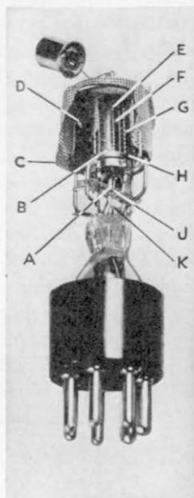
FIG. 87.—Duplex-diode pentode.
