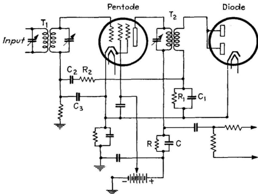
FIG. 369.—Reflex circuit including pentode and diode for amplifier.
