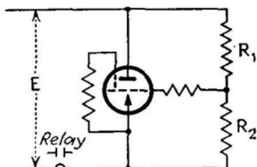
FIG. 141.—Circuit for cold-cathode gaseous tube with resistance-potentiometer units for control.
