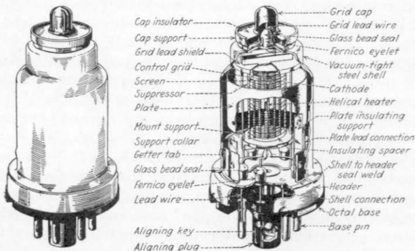
FIG. 105.—Triple-grid super-control device.
