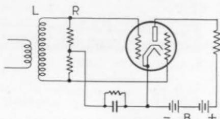
FIG. 71.—Detector circuit for Wunderlich tube.
