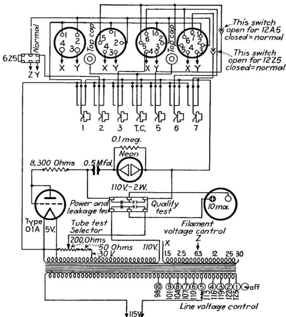
FIG. 231.—Wiring diagram of "Supreme" Model 85 tube tester.
