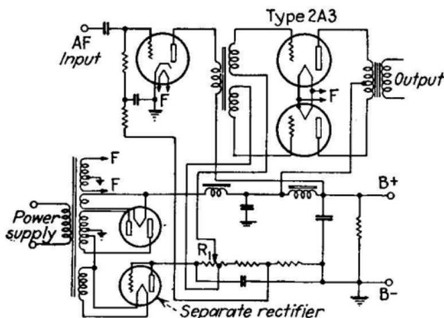
FIG. 248.—Circuit arrangement for obtaining grid-bias voltage from separate rectifier for circuit with type 2A3 tubes.
