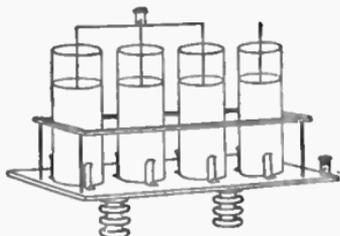
FIG. 99.—A TRANSMITTING CONDENSER MADE UP OF JARS.
