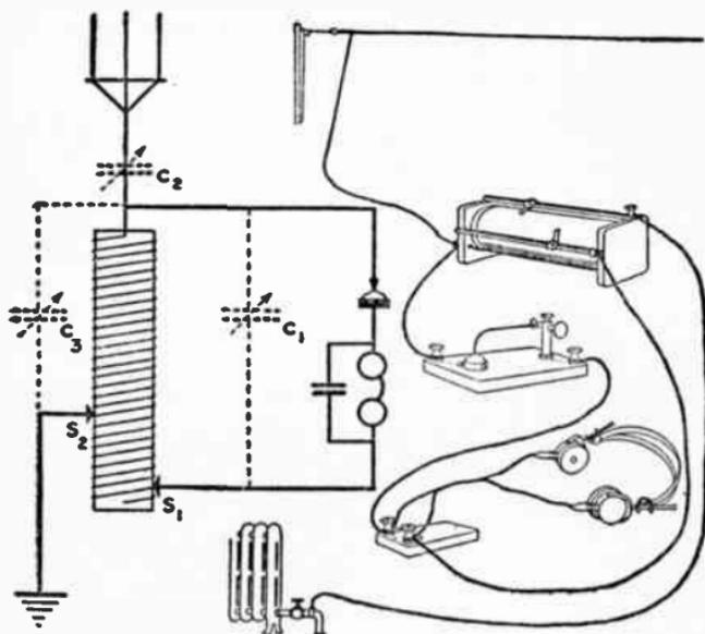
FIG. 31.—HOOK-UP FOR A DOUBLE SLIDE TUNING COIL.
