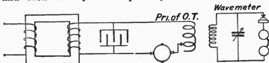
FIG. 102.—METHOD OF COUPLING THE WAVE METER TO THE PRIMARY OF THE OSCILLATION TRANSFORMER.
