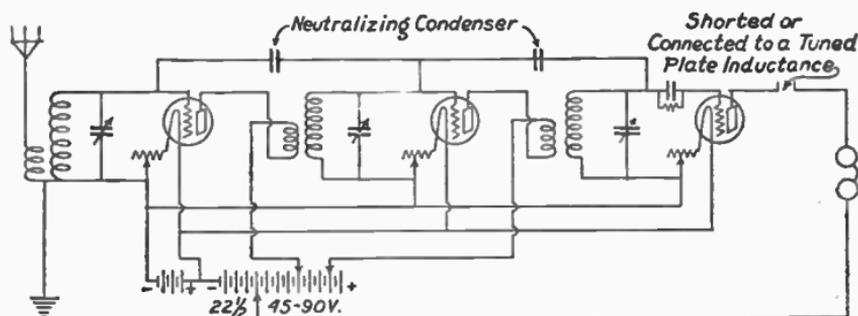
Fig. 90.—HOOK-UP FOR A THREE-TUBE NEUTRODYNE RECEIVER.
