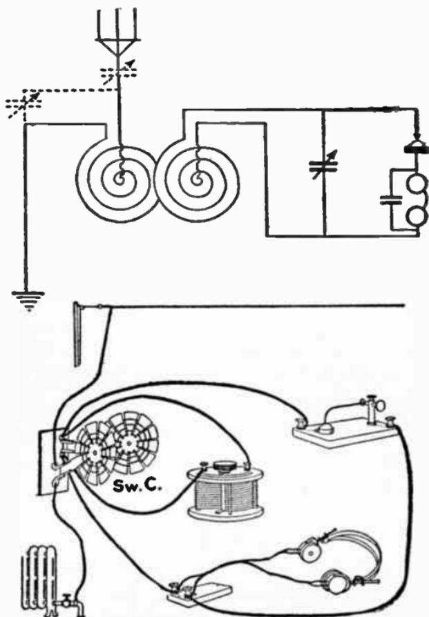
FIG. 44.—HOOK-UP FOR A CRYSTAL DETECTOR SET WITH TWO SPIDERWEB COILS.
