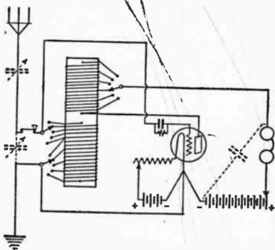
FIG. 103.—THE REGENERATIVE RECEIVING SET HOOKED UP AS A TRANSMITTER.
