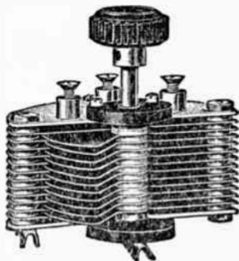
FIG. 24.—A 23-PLATE VARIABLE CONDENSER.
