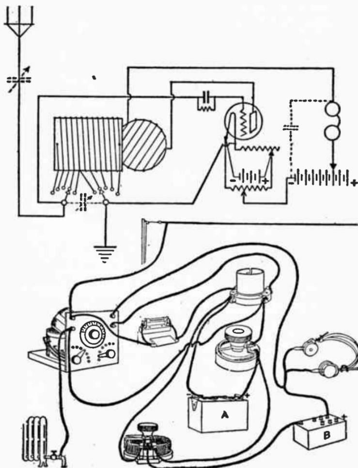
FIG. 62.—HOOK-UP FOR A VARIOCOUPLER IN A REGENERATIVE SET.
