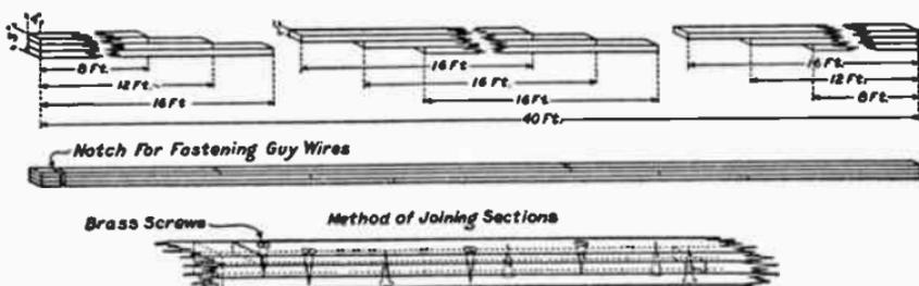
FIG. 7.—METHOD OF CONSTRUCTING A 40-FOOT LAMINATED MAST.
