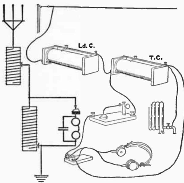
FIG. 23.—A LOADING COIL IN THE AERIAL CIRCUIT.
