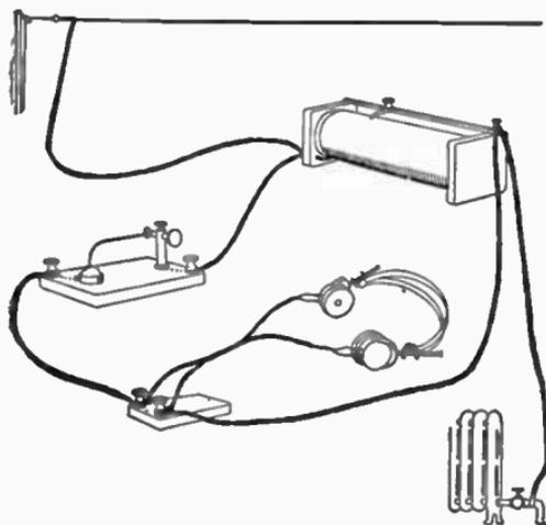
FIG. 21.—CIRCUITS OF THE CRYSTAL DETECTOR HOOK-UP. A. PRIMARY IN HEAVY LINES. B. SECONDARY IN HEAVY LINES.
