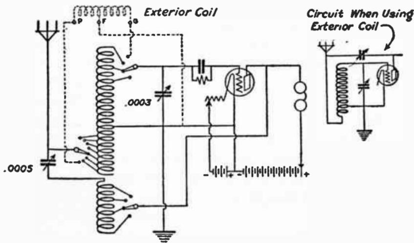
FIG. 74.—HOOK-UP FOR THE REINARTZ TUNER WITH DETECTOR.
