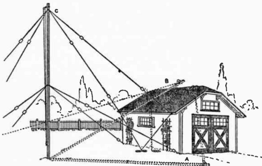
FIG. 10.—A SIMPLE METHOD OF ERECTING A MAST.
