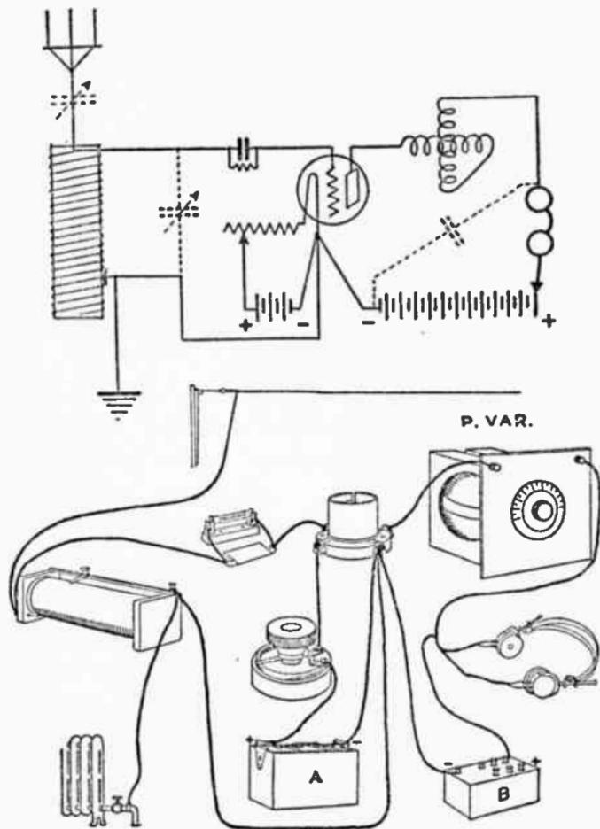
FIG. 67.—HOOK-UP FOR A SINGLE SLIDE TUNING COIL IN A TUNED PLATE REGENERATIVE SET.
