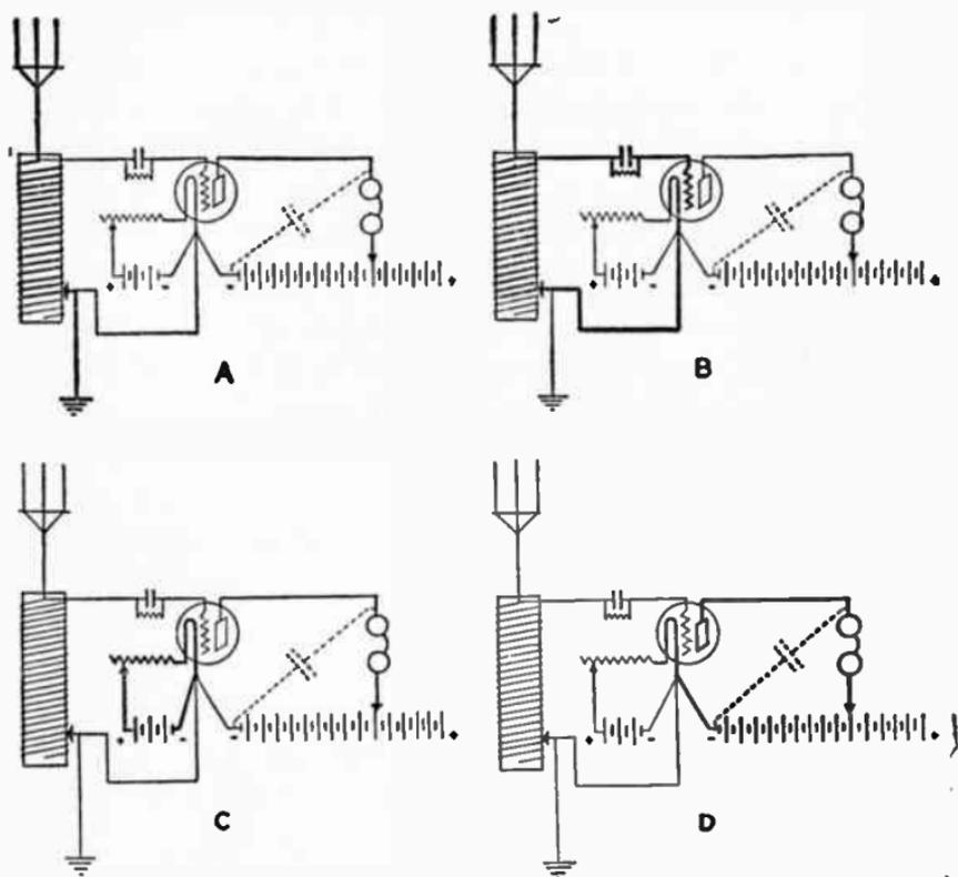
FIG. 49.—FOUR ILLUSTRATIONS OF THE HOOK-UP SHOWN IN FIG. 48. A SHOWS THE AERIAL CIRCUIT IN HEAVY LINES; B, THE SECONDARY OR GRID CIRCUIT IN HEAVY LINES; C, THE FILAMENT CIRCUIT IN HEAVY LINES; AND D, THE PLATE CIRCUIT IN HEAVY LINES
