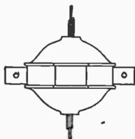
FIG. 12.—AN APPROVED WEATHERPROOF LIGHTNING ARRESTER.
