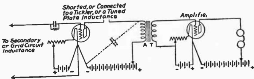
FIG. 75.—DIAGRAM SHOWING A VACUUM TUBE DETECTOR AND ONE STAGE OF AUDIO-FREQUENCY AMPLIFICATION.
