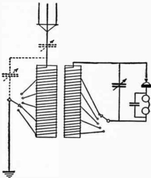
FIG. 38.—HOOK-UP FOR A CRYSTAL DETECTOR SET WITH A TAPPED LOOSE COUPLER.
