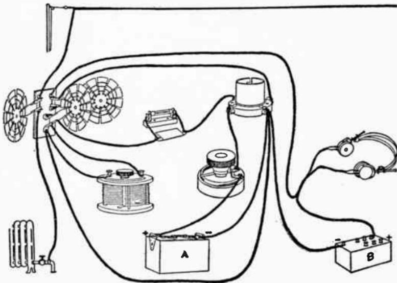
FIG. 66.—HOOK-UP FOR THREE SPIDERWEB COILS IN A REGENERATIVE SET.
