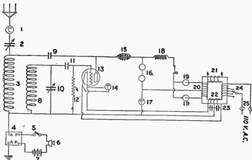
FIG. 105.—COMPLETE HOOK-UP FOR A VACUUM TUBE TRANSMITTER.
