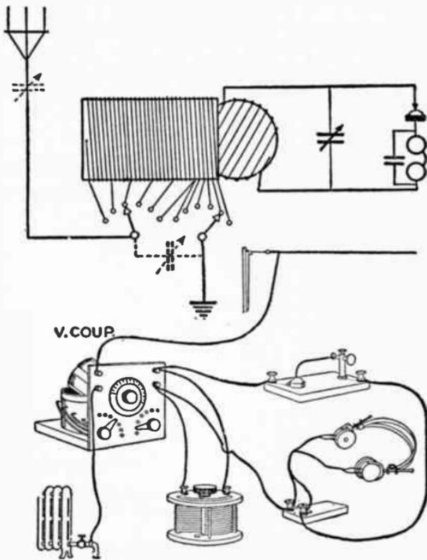
FIG. 37.—HOOK-UP FOR A VARIOCOUPLER IN A CRYSTAL DETECTOR SET.
