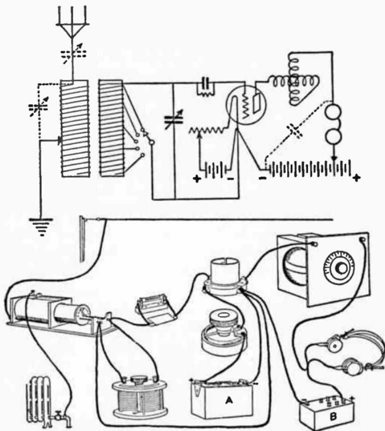
FIG. 68.—HOOK-UP FOR A LOOSE COUPLER IN A TUNED PLATE REGENERATIVE SET.
