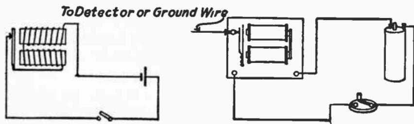
FIG. 22.—HOOK-UP FOR THE TEST BUZZER.
