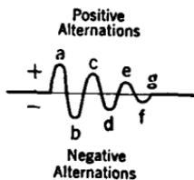
FIG. 156a.—Showing a group of decaying oscillations in a damped wave.
