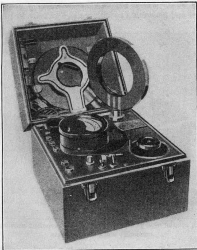
FIG. 304a.—The type D Kolster decrometer. One of the exploring coils is shown mounted in position.
