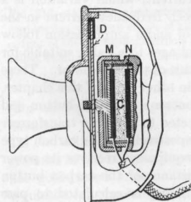
FIG. 312.—Cross-sectional view of a carbon button type transmitter, usually referred to as a microphone.
