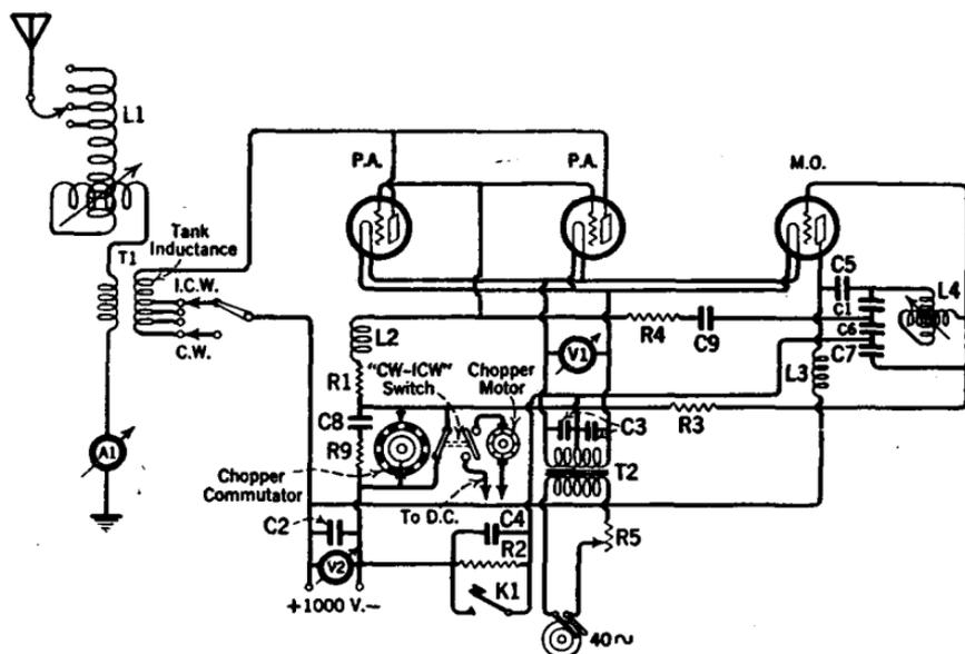
FIG. 360.—Schematic diagram of connections in the 200-watt ET-3627 tube transmitter.
