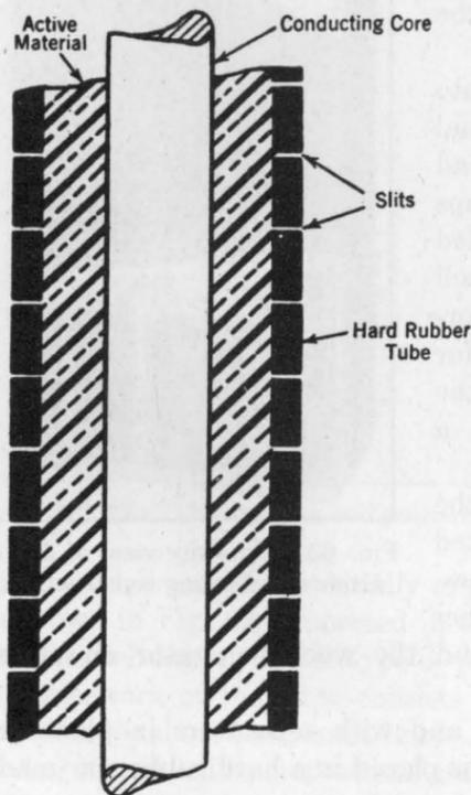
FIG. 65a.—A cross-sectional sketch of an Exide ironclad positive plate. Each individual section is known as a "pencil."
