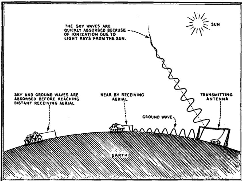
FIG. 286.—Another graphical explanation of the Heaviside-Kennelly theory of radio wave propagation showing how the sun's rays act to absorb the energy in a transmitted signal. This accounts for the reduction in transmission range during daylight hours.
