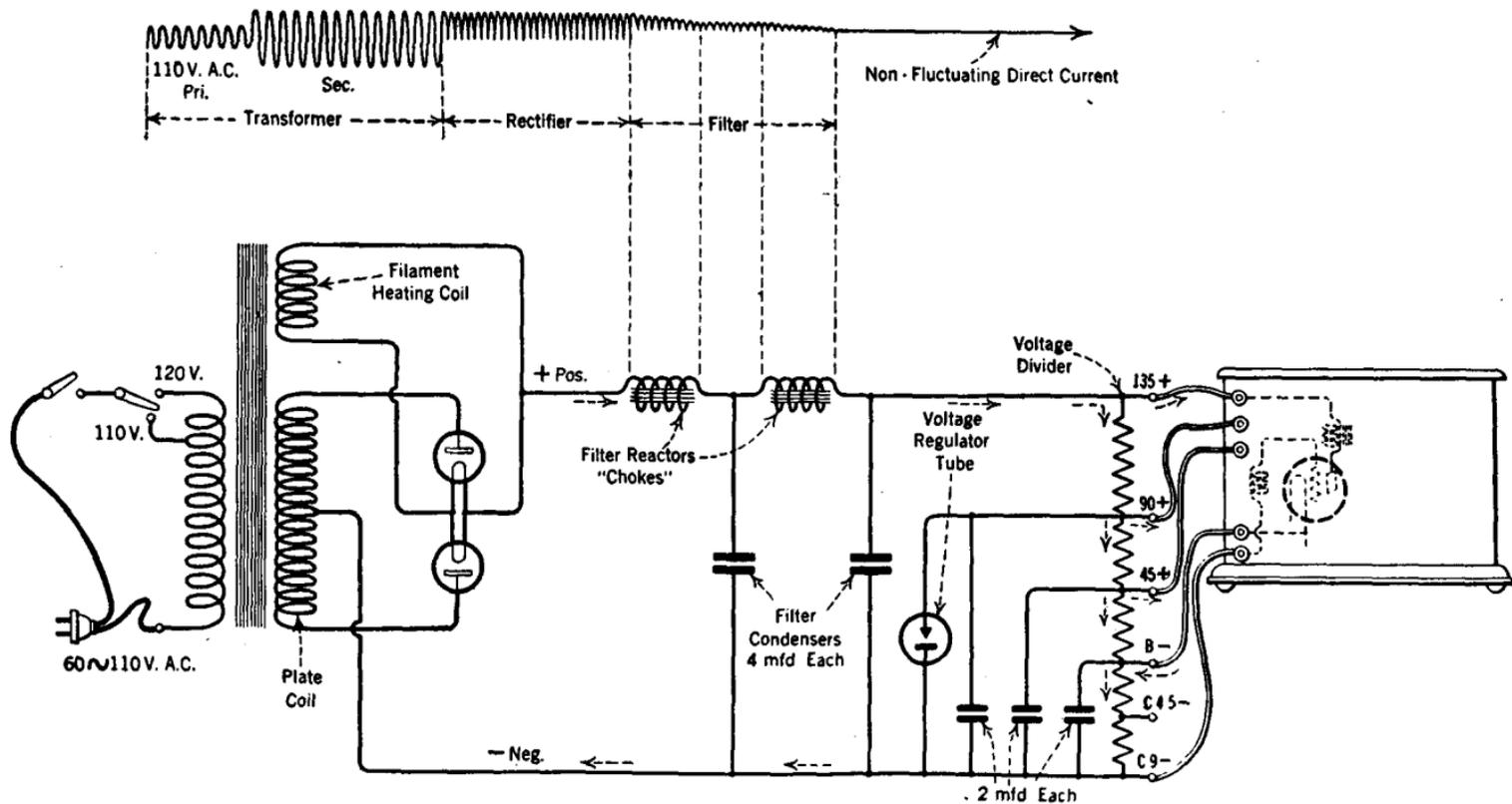
FIG. 243.—Illustrating the essential parts of a full-wave rectifier unit, namely, the power transformer, two half-wave rectifier tubes of the filament (thermionic) type, filter system and voltage divider. The principles are explained by the curves.
