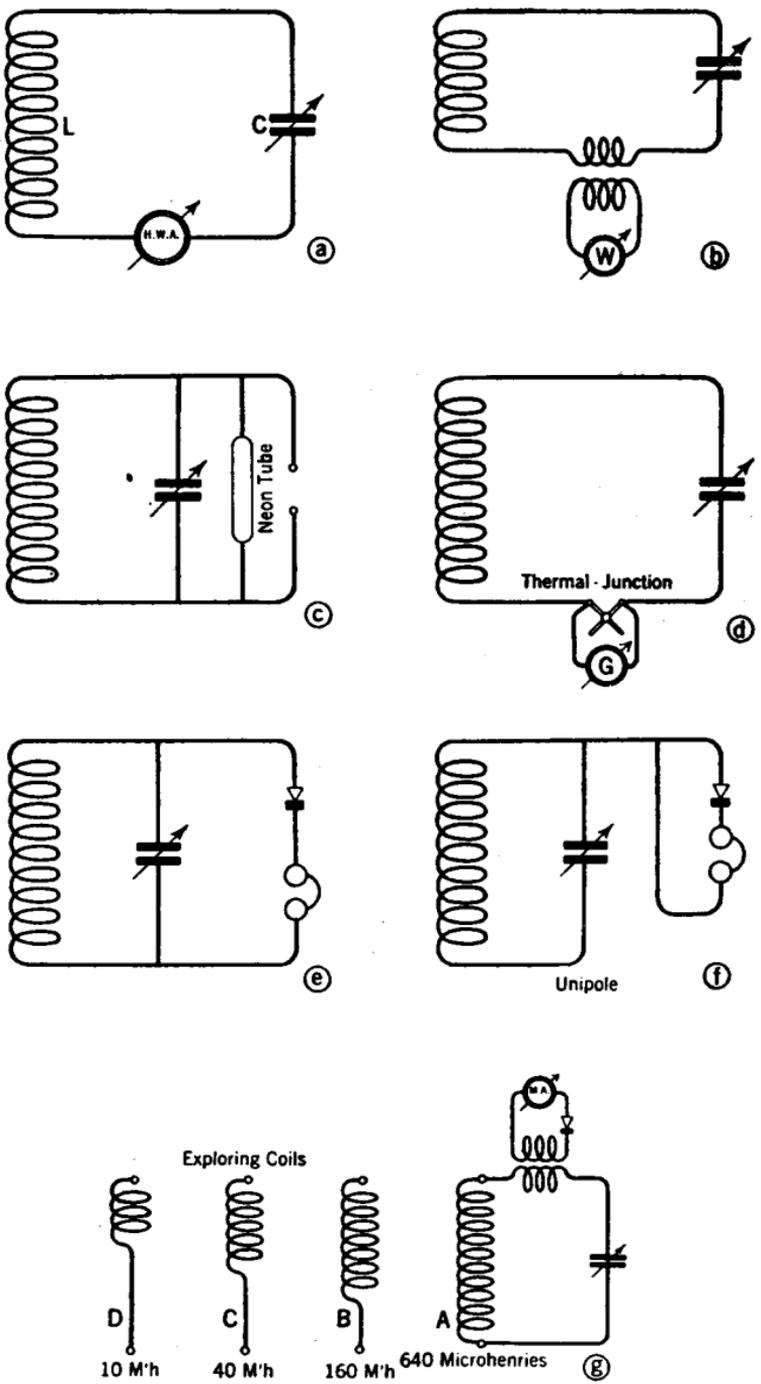
FIG. 290.—Fundamental diagrams of various wavemeter circuits.
