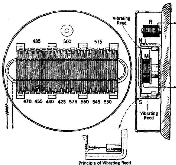
FIG. 86.—Magnetic reed type frequency meter.
