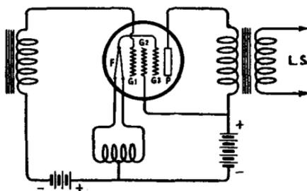
FIG. 226d. Another way of representing the arrangements of the electrodes in a pentode tube. *F* is the filament, it being heated by a-c. from the power transformer to which it is connected, *G1* the control grid, *G2* the screen grid, *G3* the cathode grid, and *P* the plate. This is a fundamental diagram showing the relation of the tube's external circuits.
