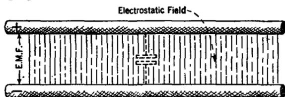
FIG. 130.—An electrostatic field is always present between conductors having a difference of potential.
