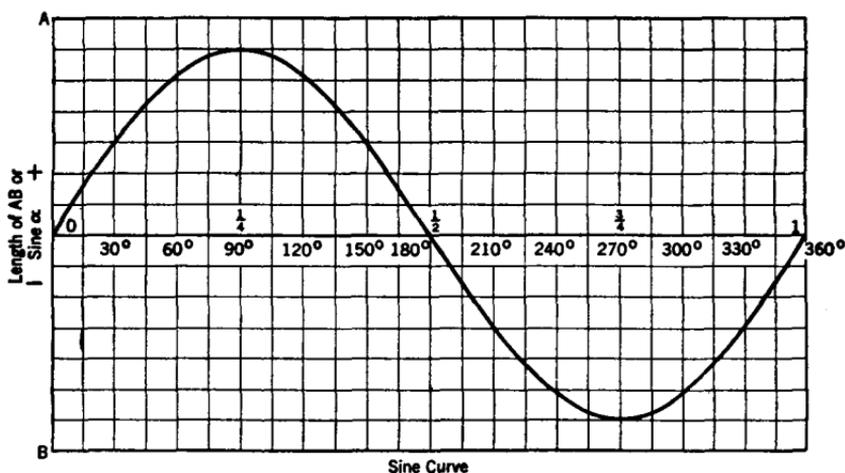
FIG. 61.—One complete cycle of a-c. represented by a sine curve. The height of the amplitude above or below zero axis, or for distances along  $OA$  and  $OB$  is determined by the sine  $\alpha$ . Refer to Fig. 60.
