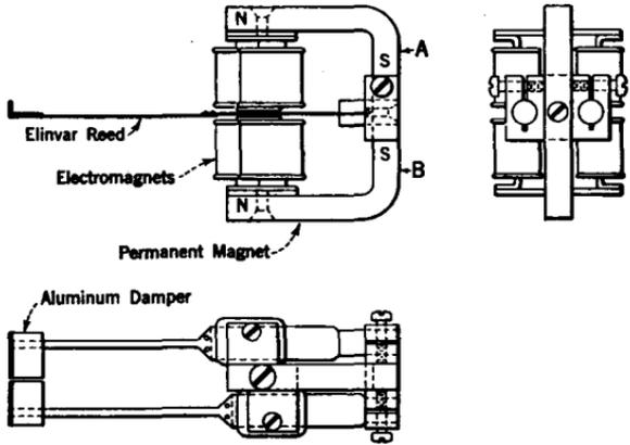
FIG. 432.—Sketches of reed indicator construction.
