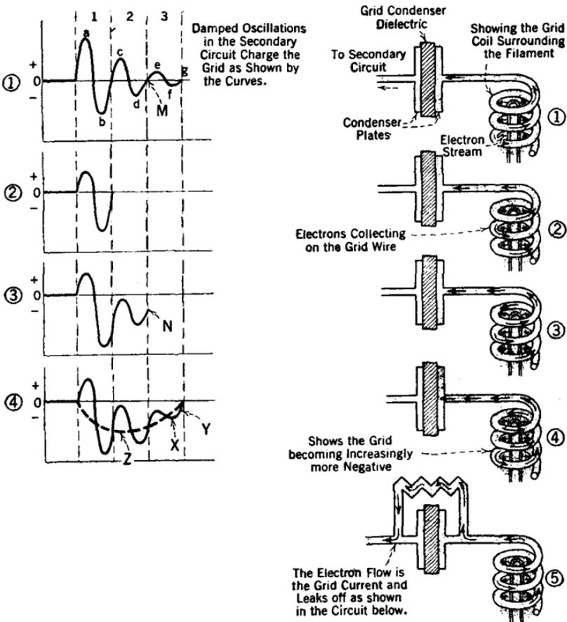
(The above Views show how the Grid Accumulates Electrons when the Fluctuating Signal Voltage is Impressed upon it and also how the Excess Electrons Leak off the Grid through the Resistance at a Predetermined Rate to Restore the Grid to its Normal Potential. This Rate is known as the "Time Constant." The Signal Voltages Readily Pass through the Grid Condenser and Charge the Grid as shown by the Curves in the Upper Left)
