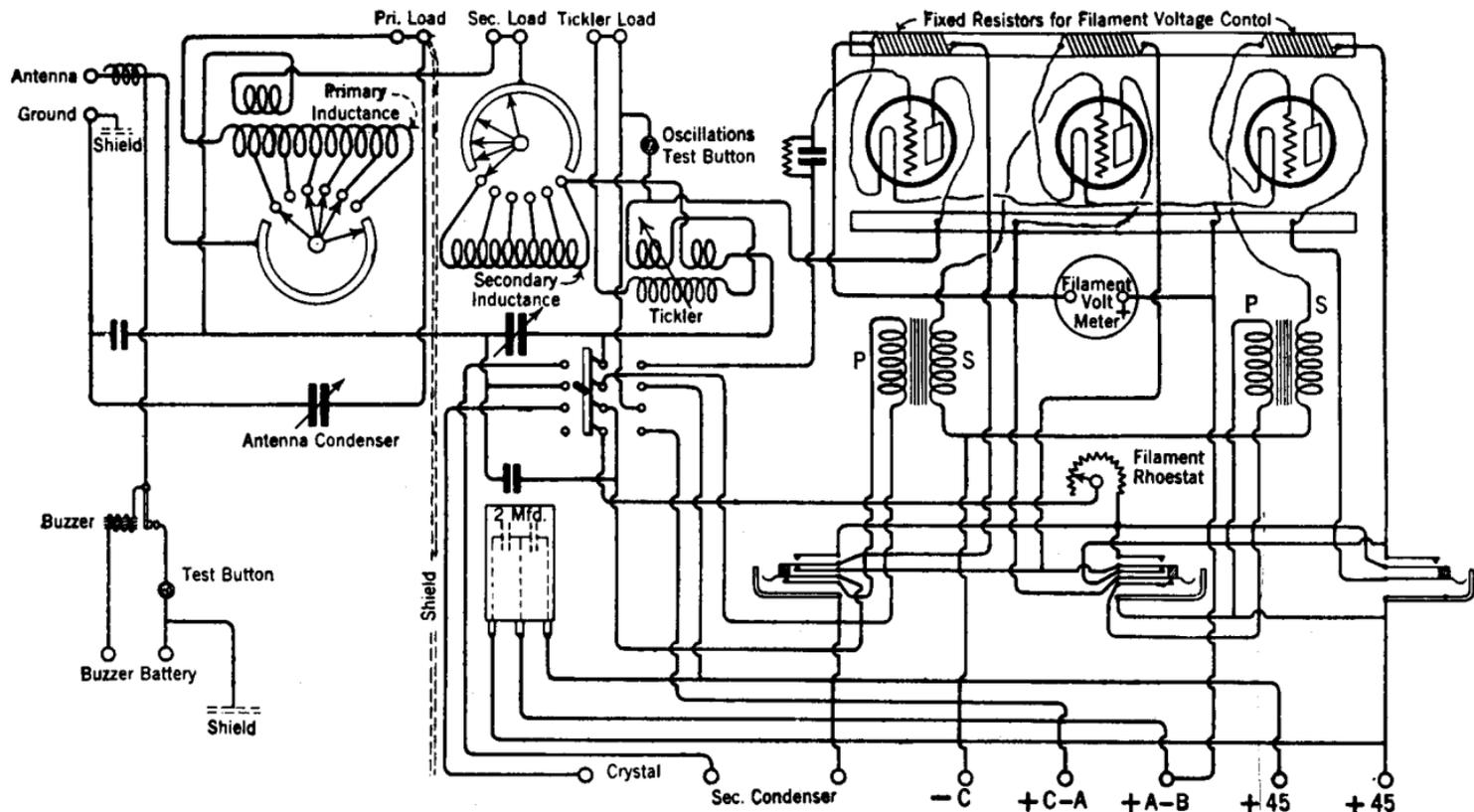
FIG. 239a.—Wiring diagram of the type IP-501-A commercial radio receiver.
