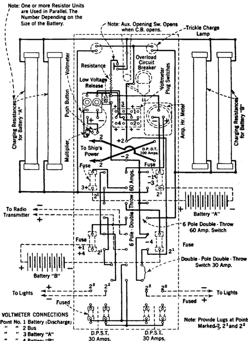
FIG. 70.—Switchboard wiring diagram of the Exide marine type charging panel.
