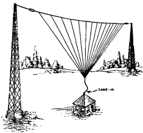
FIG. 275.—A vertical "fan" type antenna.
