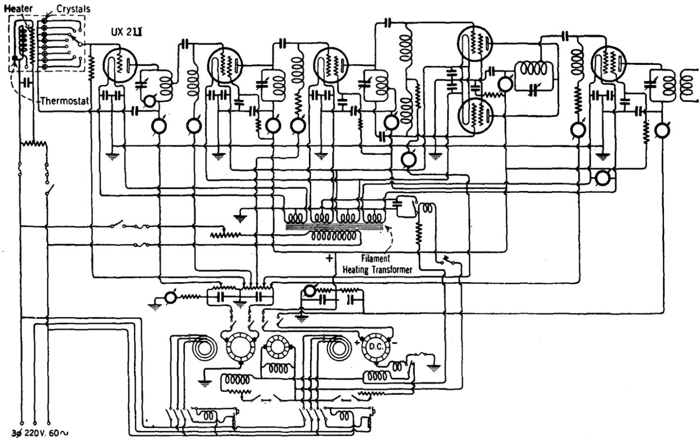
FIG. 386.—The schematic wiring diagram of Model ET-3656 one kw. high frequency (short wave) crystal-controlled tube transmitter. This set employs the screen grid type tubes in the amplifier circuits.
