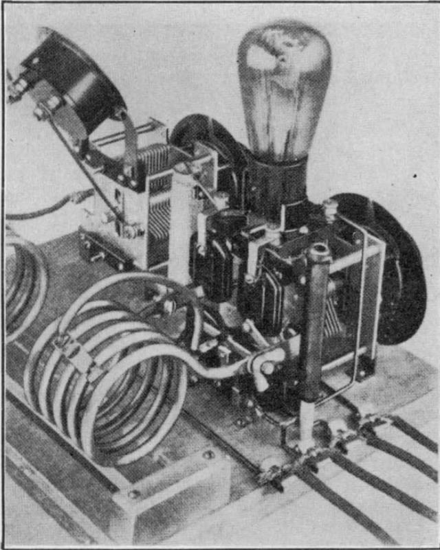
FIG. 374d.—A close-up view of a short wave amateur transmitter, showing the heavy leads and strong mechanical construction.—*Courtesy American Radio Relay League.*
