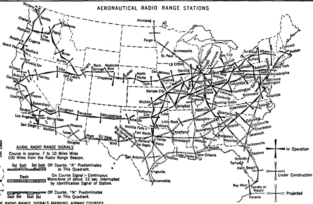
FIG. 428.—Map showing radio range beacon stations in operation, under construction or projected. Courtesy U. S. Dept. of Commerce.
