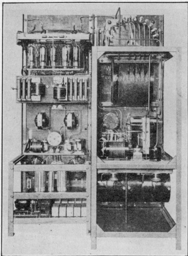
FIG. 364.—Rear view of type ET-3638—2-kw. telegraph transmitter.
