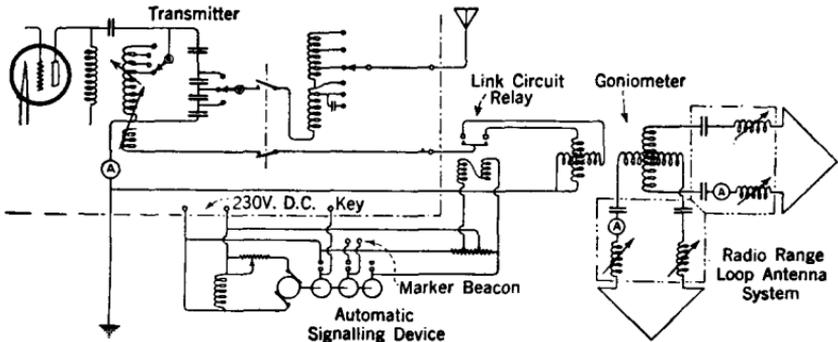
FIG. 429. Schematic diagram of a radio beacon transmitter.
