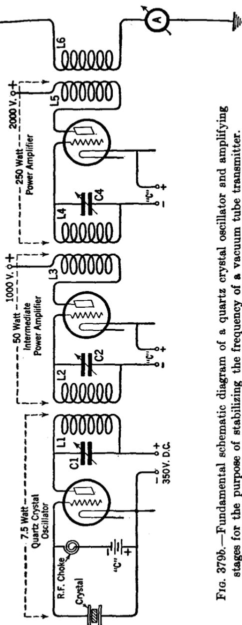
FIG. 379b.—Fundamental schematic diagram of a quartz crystal oscillator and amplifying stages for the purpose of stabilizing the frequency of a vacuum tube transmitter.
