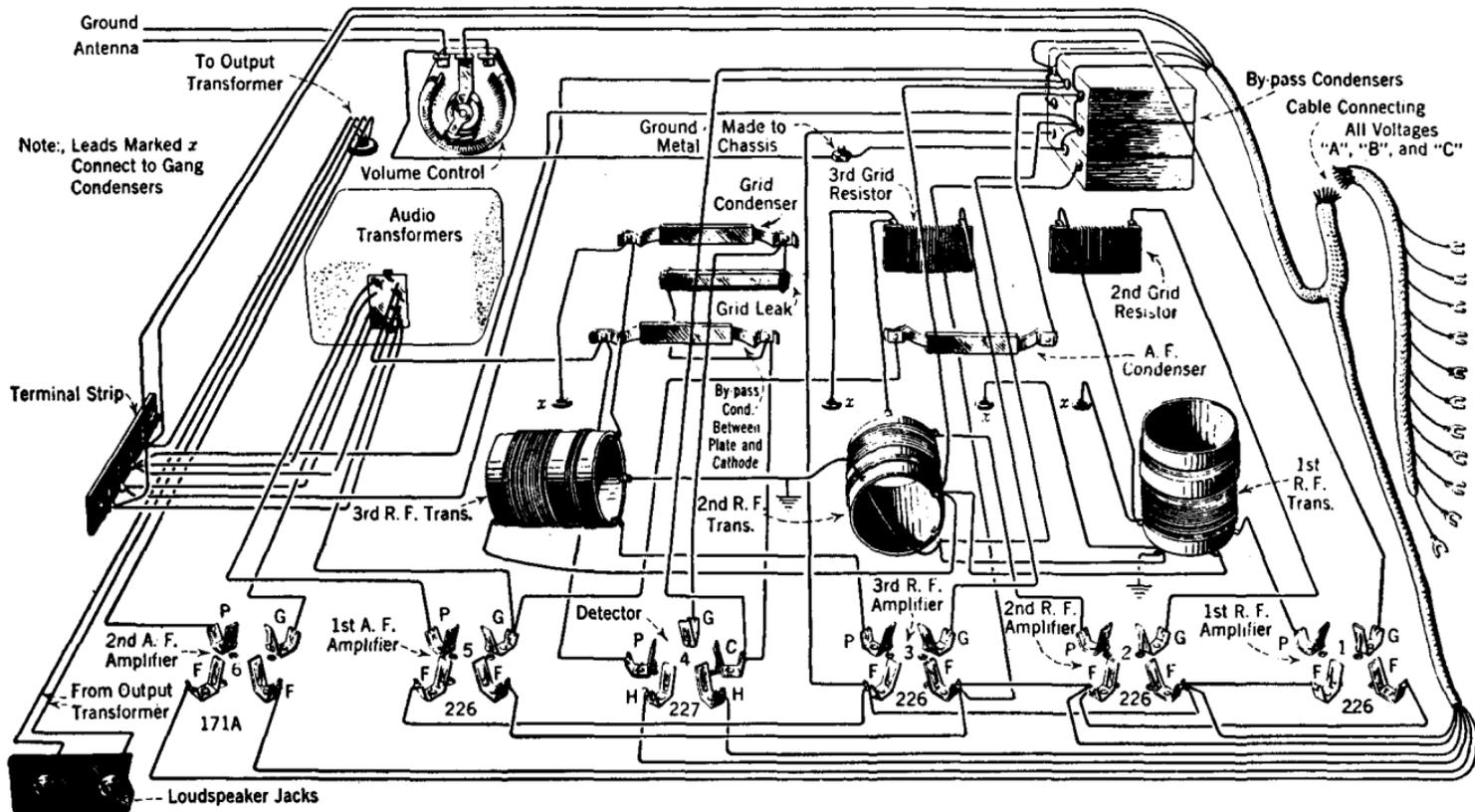
FIG. 211a.—The sub-chassis of a six-tube A.C. operated receiver with the r.f. transformers mounted with their center axes at 90° to each other.
