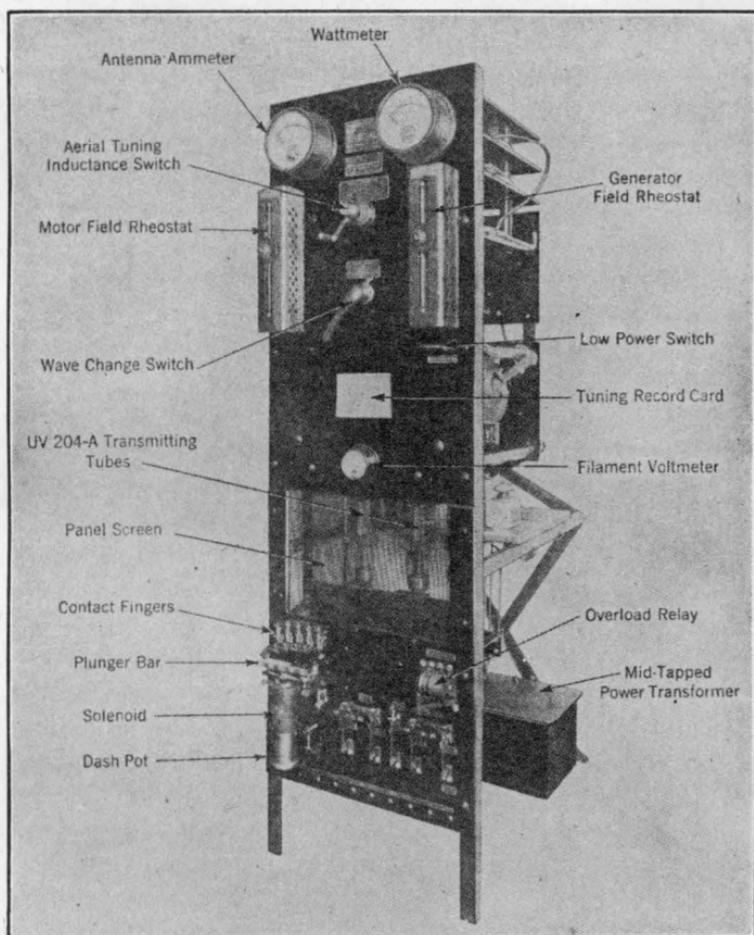
FIG. 342.—Front panel view of P-8 converted tube transmitter, type ET-3628.
