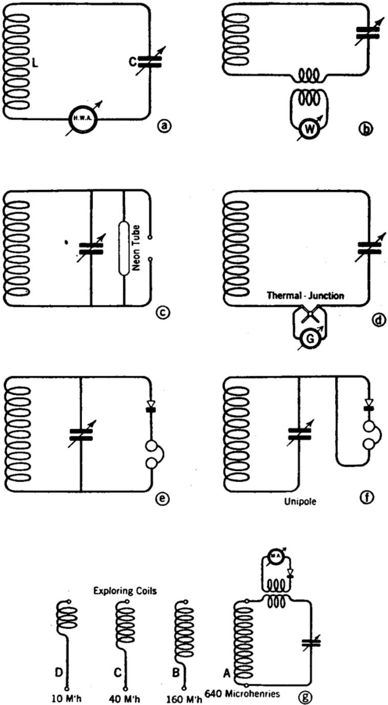
FIG. 290.—Fundamental diagrams of various wavemeter circuits.
