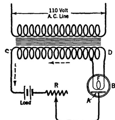
FIG. 77.—Half-wave rectifier and transformer for battery charging.
