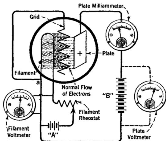
FIG. 145.—A fundamental three-element vacuum-tube circuit.
