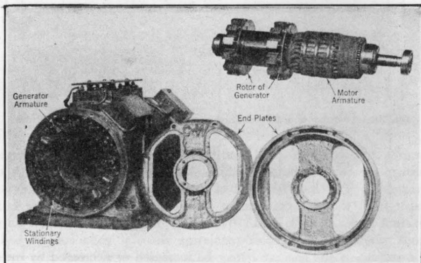
FIG. 41.—The  $\frac{1}{2}$ -k.w. 500-cycle Crocker-Wheeler motor-generator.
