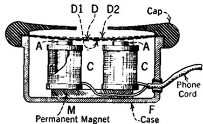
FIG. 227.—An exposed view of the bi-polar type receiver illustrating the operating principles.
