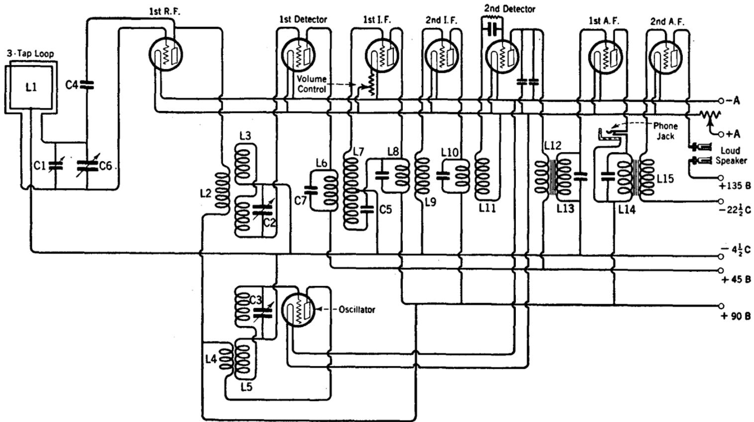
FIG. 204.—Schematic diagram of an eight-tube super-heterodyne receiving circuit.
