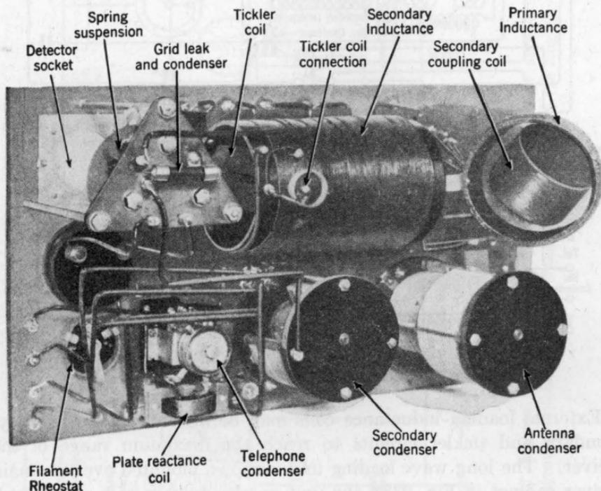
FIG. 235.—Rear view of the IP-501 receiver.
