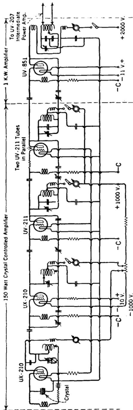
Fig. 323.—A crystal controlled oscillator with its accompanying intermediate and power amplifier circuits.
