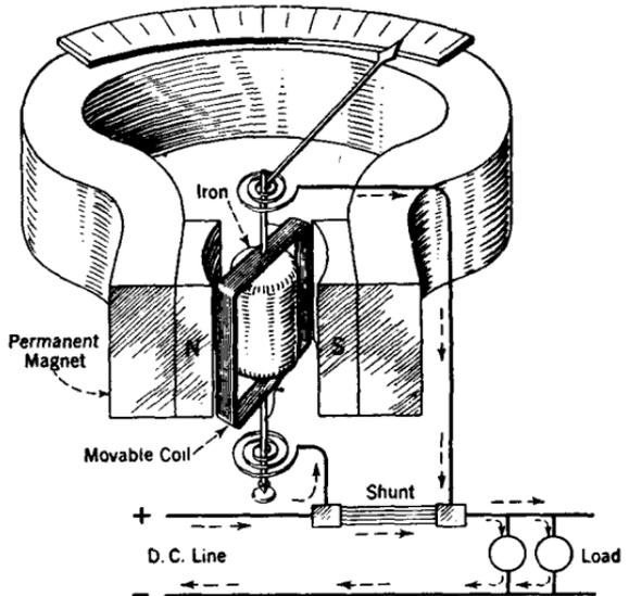
FIG. 83.—Showing the general construction of a d-c. ammeter used with a shunt resistance.
