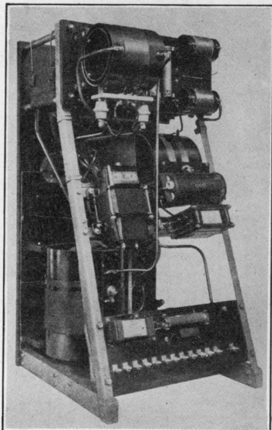
FIG. 358.—Type ET-3627 200-watt transmitter.
