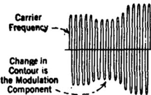
Shows the Carrier Frequency with the Modulation Superimposed upon it
