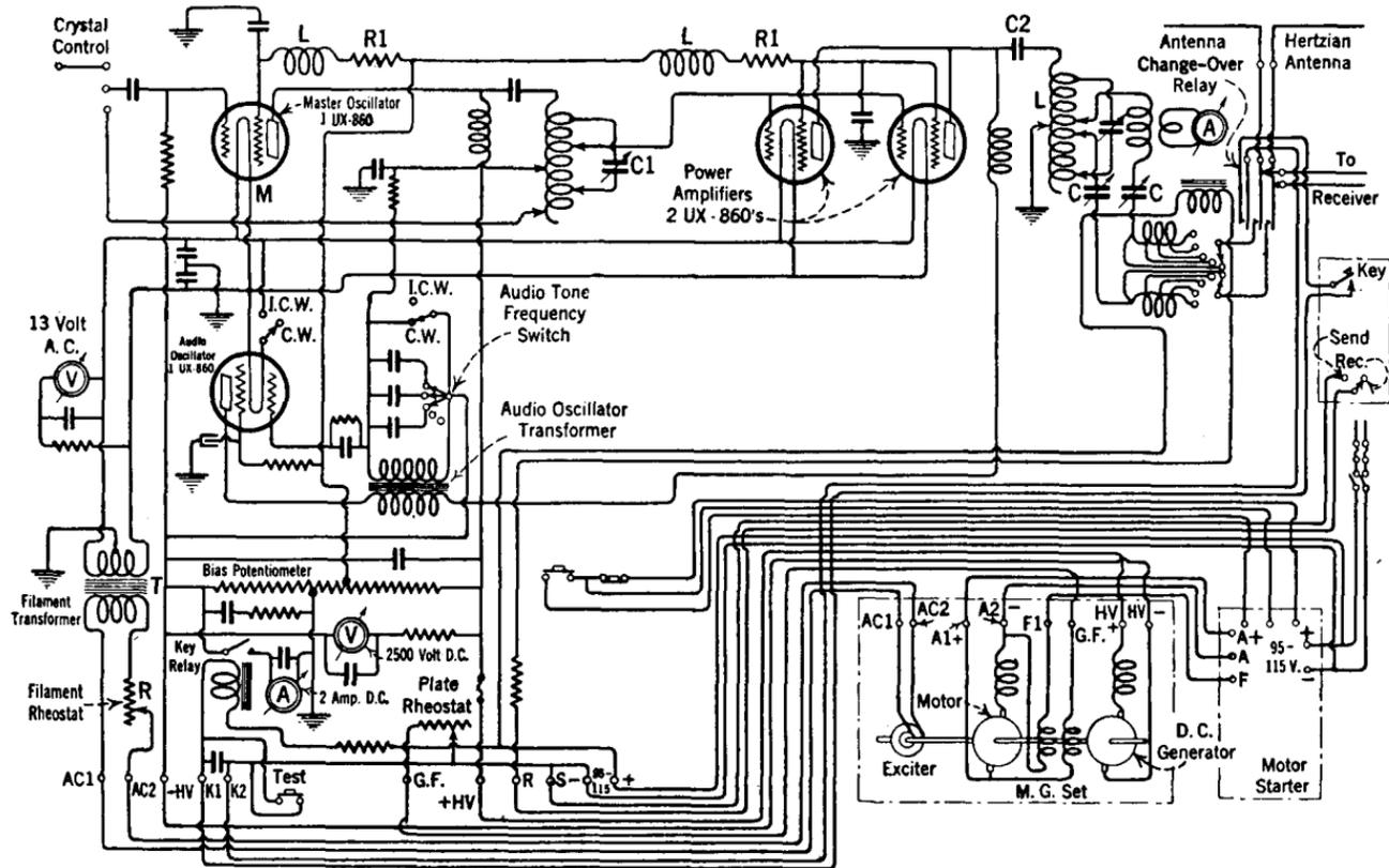
FIG. 387.—Complete schematic wiring diagram of the 200-watt short wave transmitter Model ET-3655. This transmitter employs screen grid tubes and a Hertzian type antenna. It has a wavelength range from 26 to 150 meters. Crystal control may be used to stabilize the transmitted frequency if desired.
