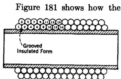
Figure 181 shows how the bank-wound coil of two layers is constructed, the turns being indicated by numbers 1, 3, 2, 5, etc. The maximum difference in potential across three turns corresponds to the e.m.f. between adjacent turns. A threaded or grooved cylindrical insulated form is used to prevent the wire from slipping during the process of winding. It can be seen that by this method of winding the first and last turns are separated by
