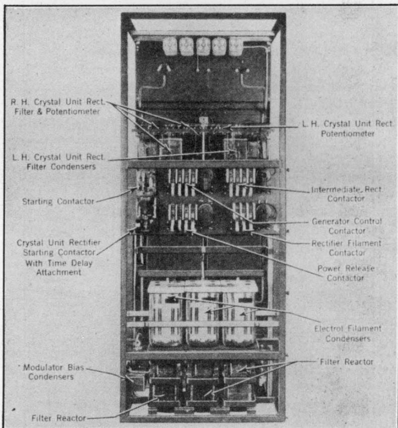
FIG. 497.—Rear view of the low-power rectifier and automatic control unit of the 50-kw. transmitter.
