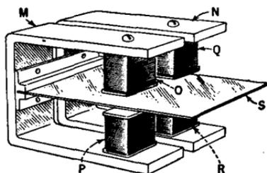
FIG. 436.—Construction of a reed converter.
