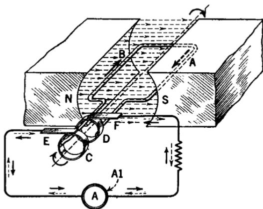
FIG. 28.—Showing the armature coil connected to collector rings to obtain a reversal of current in the external or load circuit of an a-c. generator when armature coil *A, B*, rotates through the magnetic field.
