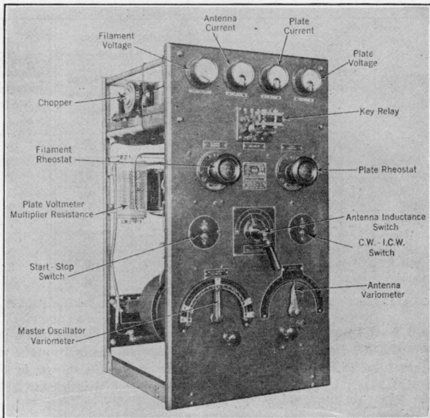
FIG. 361*a*.—Front panel view of the 200-watt tube transmitter type ET-3627-A.
