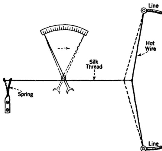
FIG. 85.—Hot-wire ammeter. (Radio-frequency ammeter.)
