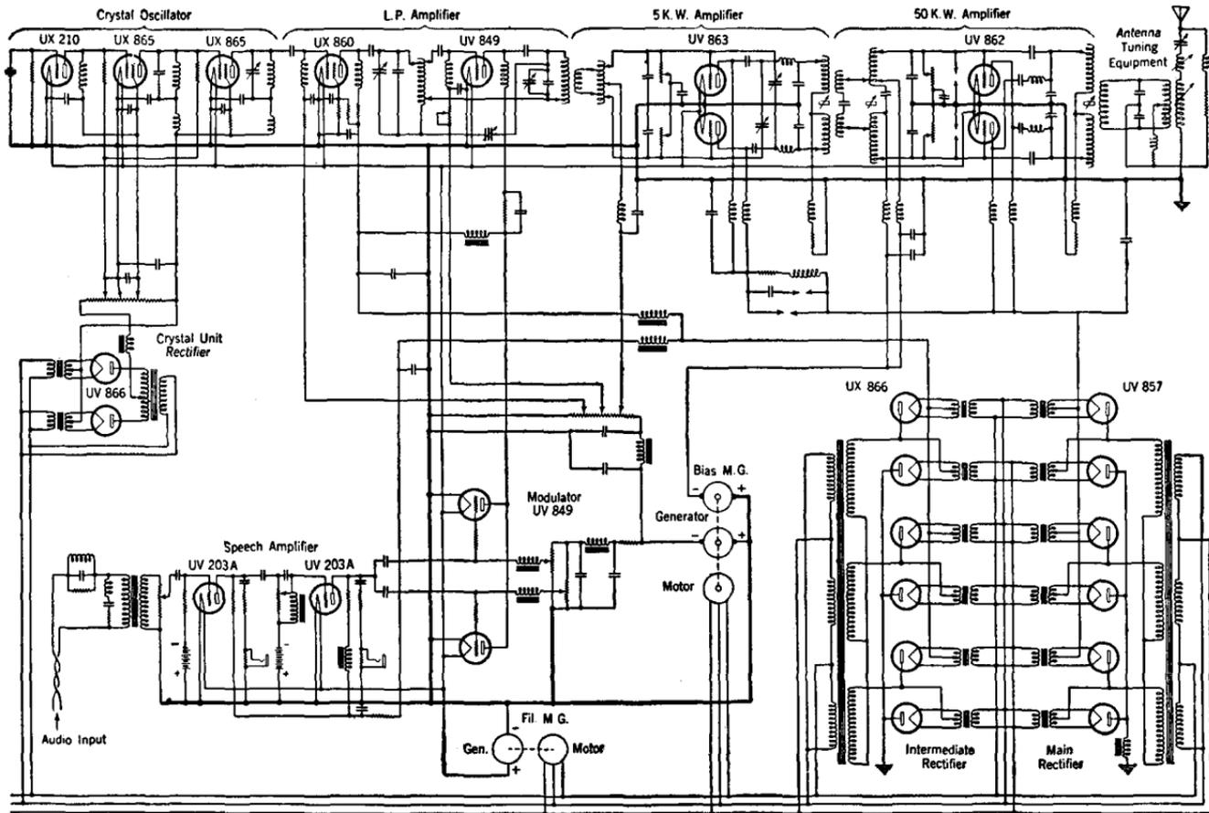
FIG. 491.—Schematic diagram of the RCA 50-kw. broadcast transmitter.
