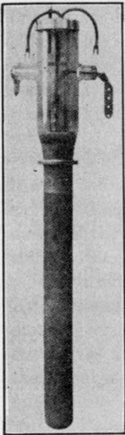
FIG. 509.—Type UV-862 water-cooled tube.
