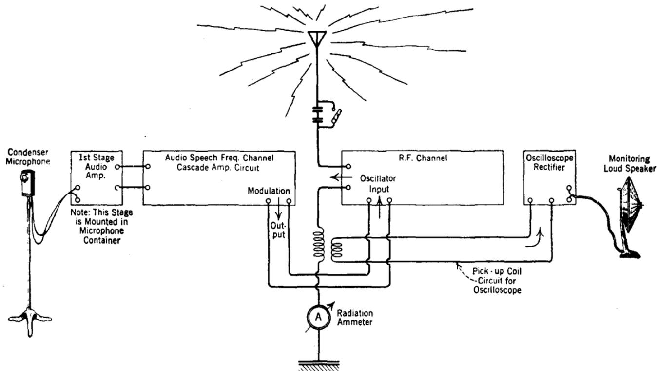
FIG. 320.—A block diagram of a 1-kw. broadcast transmitter. The oscilloscope rectifier is inductively coupled to the antenna as an effective means of checking the modulation of the broadcasted wave. See diagram in Fig. 319.
