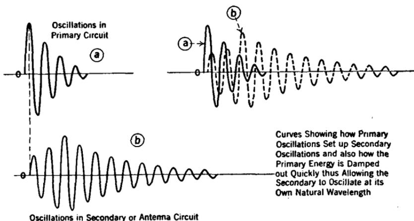
FIG. 401.—The two curves on the left show how the antenna system of a spark transmitter derives its radio-frequency power from the rapidly damped oscillations in the primary circuit. The illustration at the right shows the two curves superimposed on each other.
