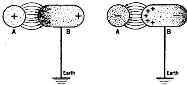
FIG. 125.—Illustrating the effect of a “bound” charge on the surface of a dielectric material when placed within the influence of another charged body.
