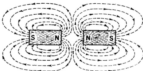
FIG. 2b.—Like magnetic poles repel.
