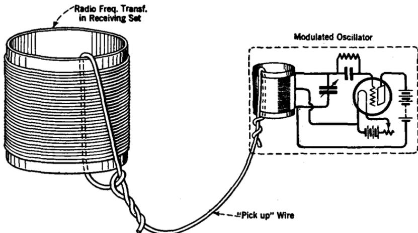
FIG. 217.—One of the uses of a modulated oscillator. The pick-up wire delivers the test signal to the radio-frequency coil.
