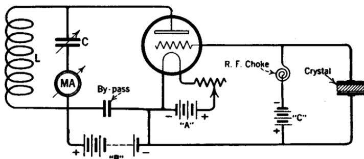
FIG. 379a.—One of several methods of utilizing a quartz crystal to control the frequency allocated to a transmitter.
