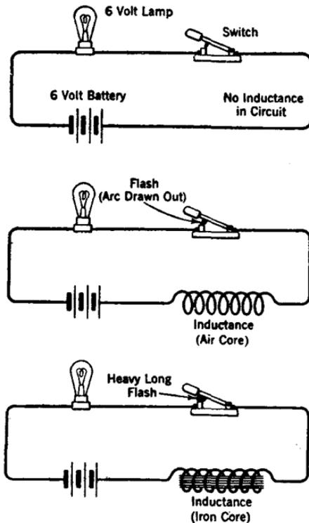
FIG. 101.—Illustrating the principle of self-inductance.
