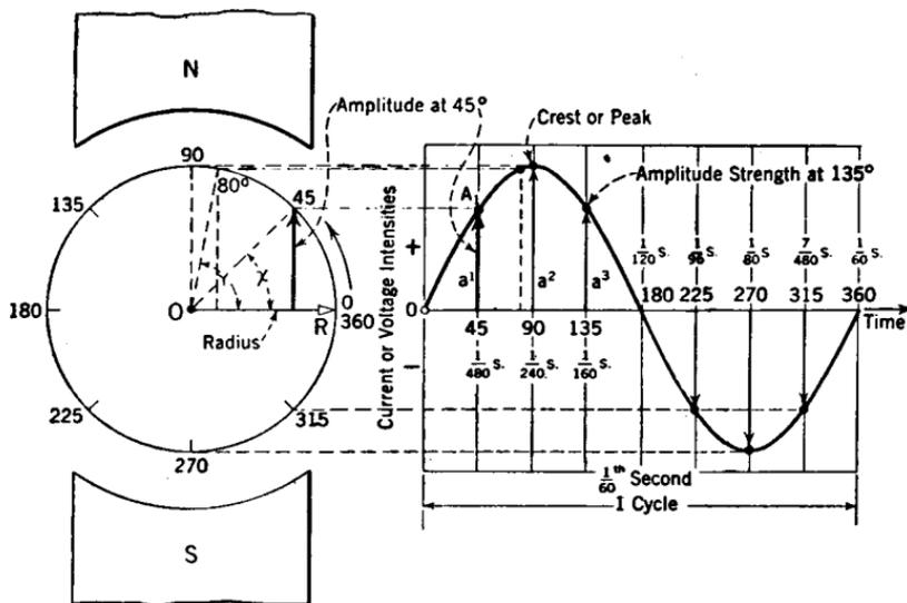
FIG. 92.—Sine curve depicting one cycle of 60 ~ a-c.
