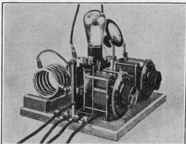
FIG. 374a.—Short wave amateur transmitter incorporating the Hartley circuit.—
