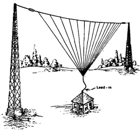
FIG. 275.—A vertical "fan" type antenna.
