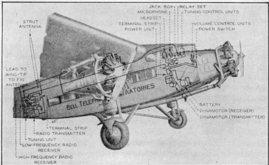
FIG. 452.—Phantom view showing the arrangement of a typical aircraft radio installation which provides for two-way communication. *Courtesy Western Electric Company.*
