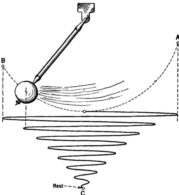
FIG. 91.—Illustrating the phenomenon of inertia.
