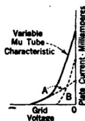
FIG. 226e.—Curve A is a low- $\mu$  tube characteristic and curve B a high- $\mu$  characteristic. The long curve in solid line is a variable- $\mu$  tube characteristic and is a combination of the A and B characteristics.
