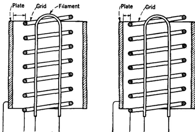
FIG. 146.—Sketches showing the relative position of the elements in a three-electrode vacuum tube.
