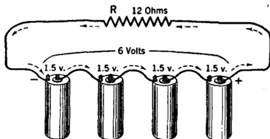
FIG. 12.—Four dry cells connected in series.
