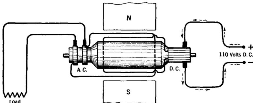
FIG. 44.—An elementary diagram of a dynamotor. In commercial practice the dynamotor is often employed in d.-c. circuits to step-up d.-c. voltage. The machine is then usually equipped with two commutators.
