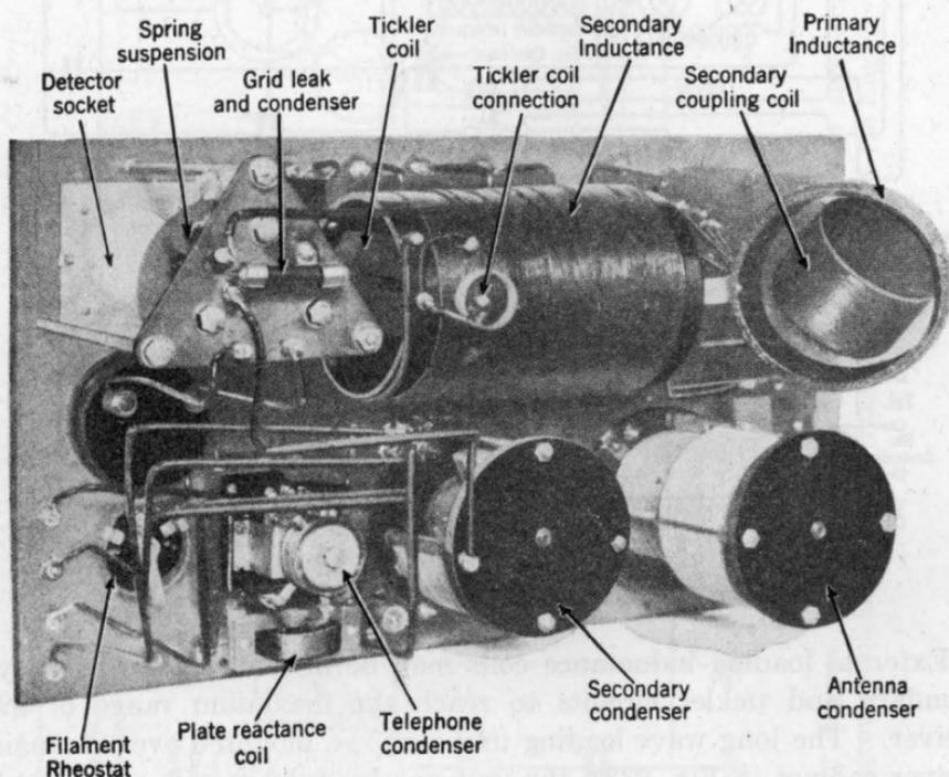
FIG. 235.—Rear view of the IP-501 receiver.
