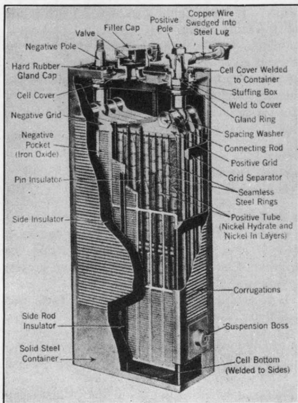
FIG. 73.—Cross-sectional view of the Edison storage cell.
