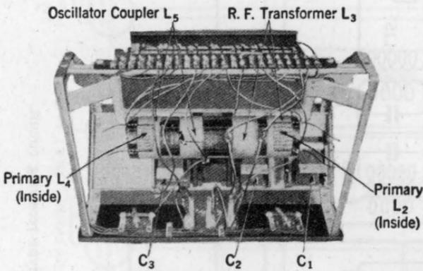
FIG. 204a.—Interior view of eight-tube super-heterodyne receiver.
