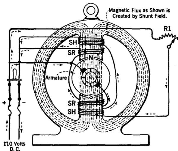
FIG. 36.—Differentially wound d-c generator.
