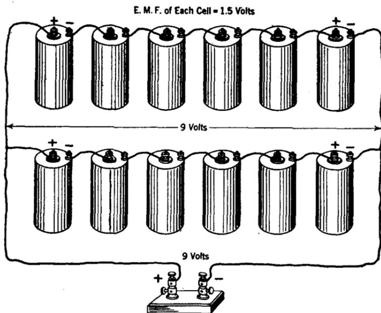
FIG. 16.—Dry cells connected in series-parallel.
