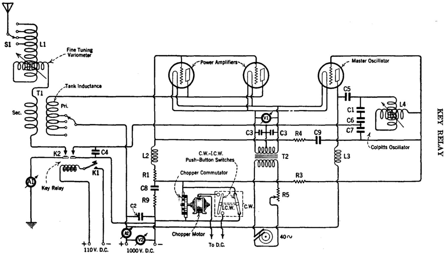
FIG. 362a.—Schematic diagram of the ET-3627-A 200-watt tube transmitter utilizing the break-in system.
