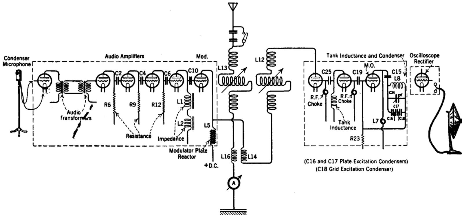
FIG. 321.—A 1-kw. broadcast transmitter. Only portions of the circuits are shown for the purpose of indicating how various kinds of coupling are employed between the vacuum tubes. The complete circuit of this broadcast transmitter is shown in Fig. 319.
