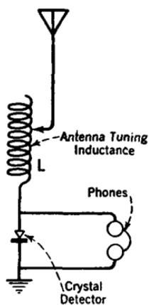
FIG. 184.—A simple radio receiving circuit.
