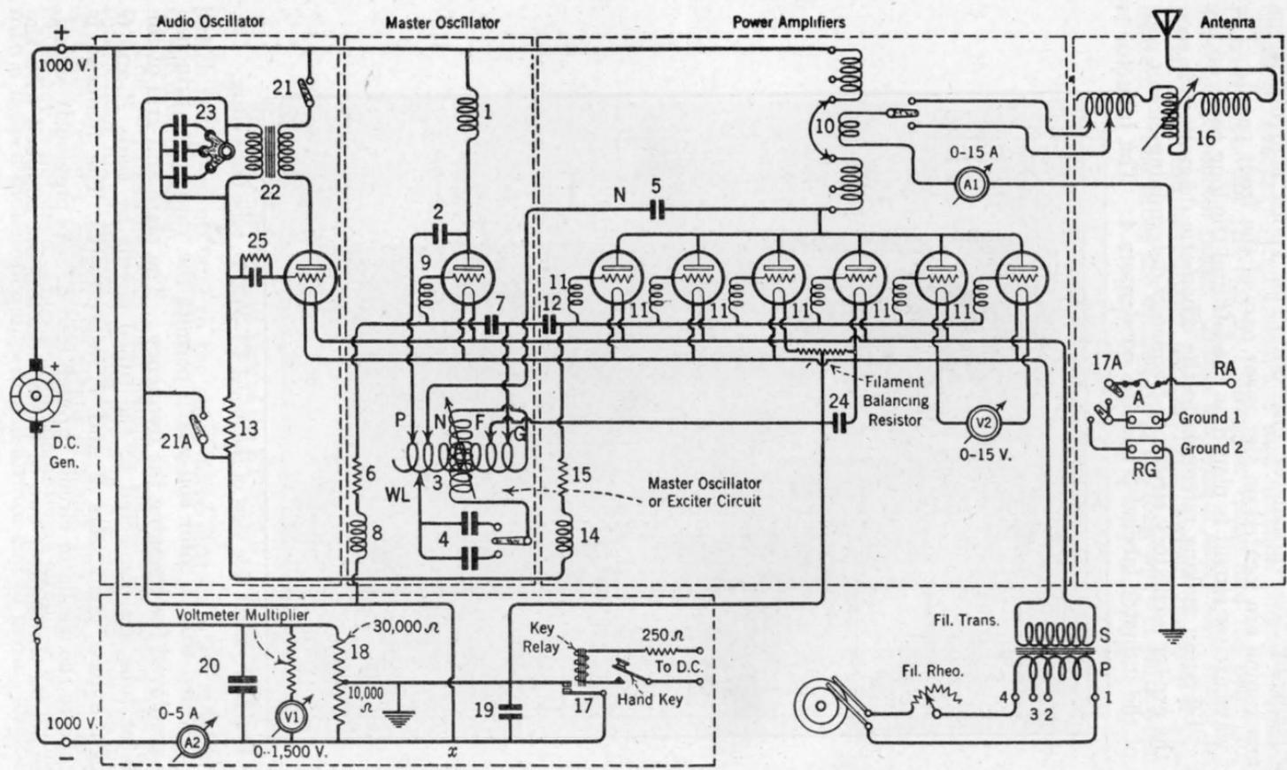
FIG. 355.—Schematic circuit diagram of the ET-3626-B tube transmitter.
