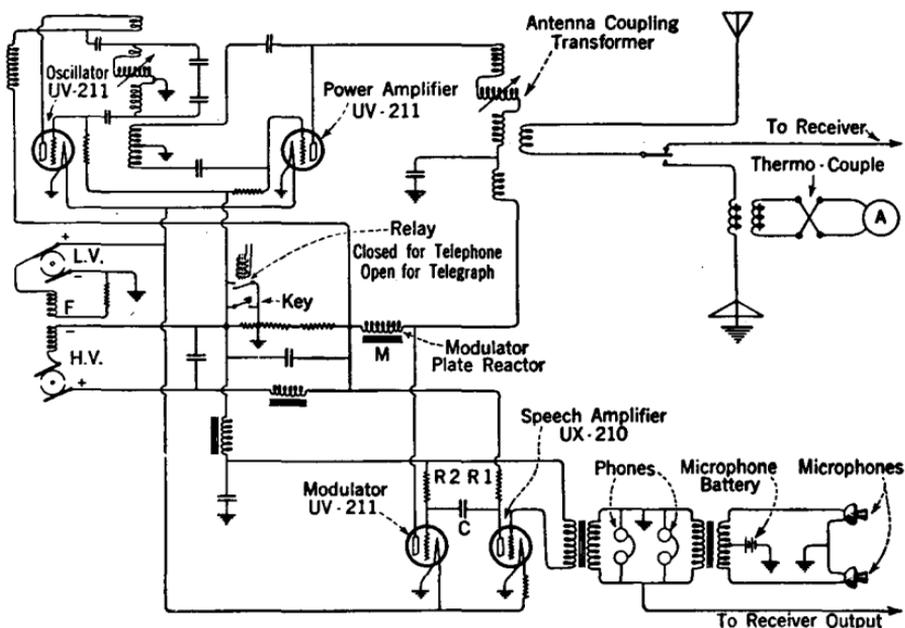
FIG. 446.—Schematic diagram of the ET-3653-A airplane transmitter.
