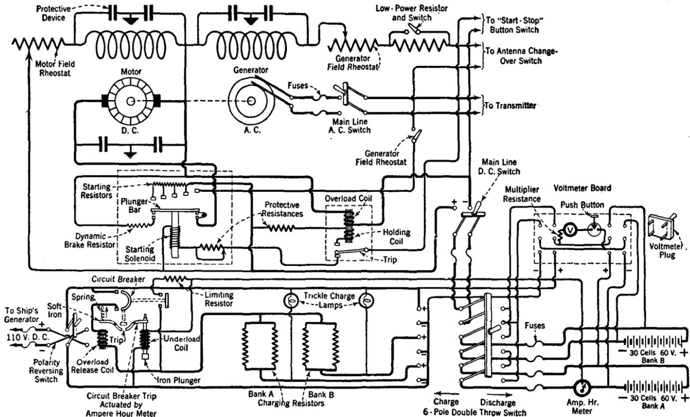
FIG. 72.—Schematic diagram of the d-c. and a-c. power circuits, and a 120-volt storage battery bank and charging equipment, of a radio transmitter. There are two condensers (not shown) which serve as a protective device across the generator armature. The motor and generator fields are protected by one set of condensers only, whereas two sets are shown in the diagram for clarity.
