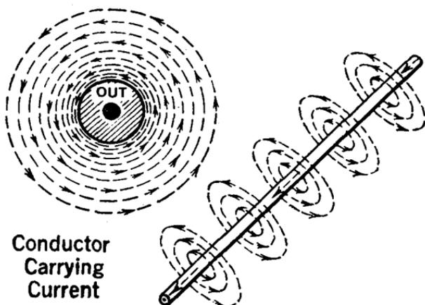
FIG. 5b.—Two views depicting the direction of lines of force about a conductor when the current is flowing toward the reader.
