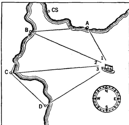
FIG. 423.—A vessel's position (bearing) is obtained by the method suggested in this drawing.
