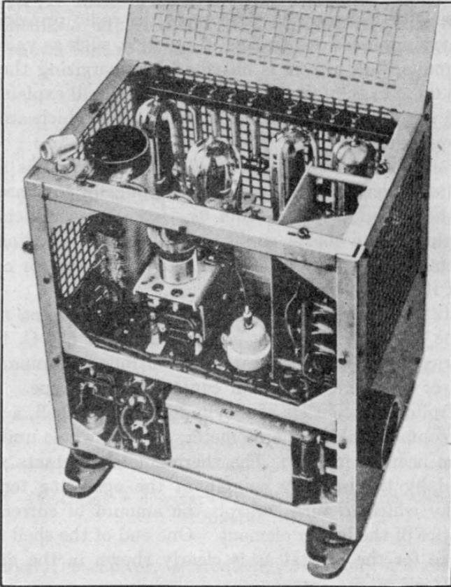
FIG. 460.—An interior view of the Western Electric Model 8-A airplane transmitter.
