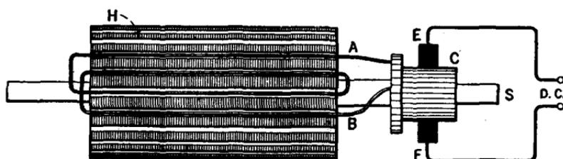
FIG. 55.—Drum-wound armature.
