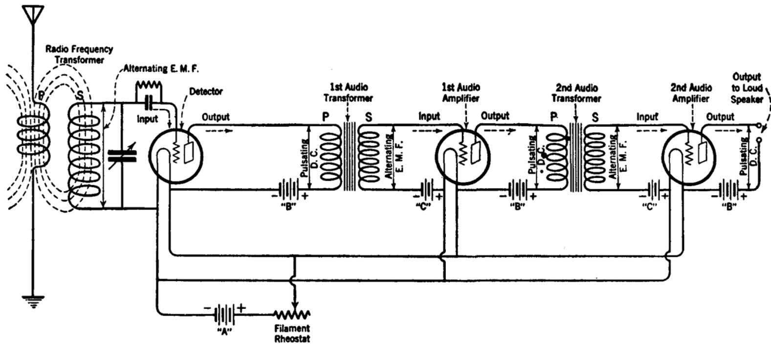
FIG. 170.—Showing the fundamental process upon which all vacuum tube circuits are operated, i.e., (1) the input energy is always in the form of an alternating voltage applied to the grid, and (2) the output energy is always in the form of a pulsating direct current. (The rise and fall of the d-c. values is called the alternating component.)
