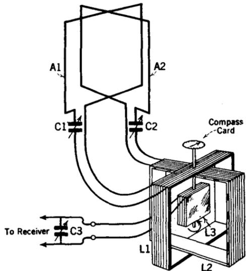
FIG. 424.—The general arrangement of the components in the Bellini-Tosi Goniometer.
