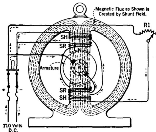
FIG. 36.—Differentially wound d-c generator.
