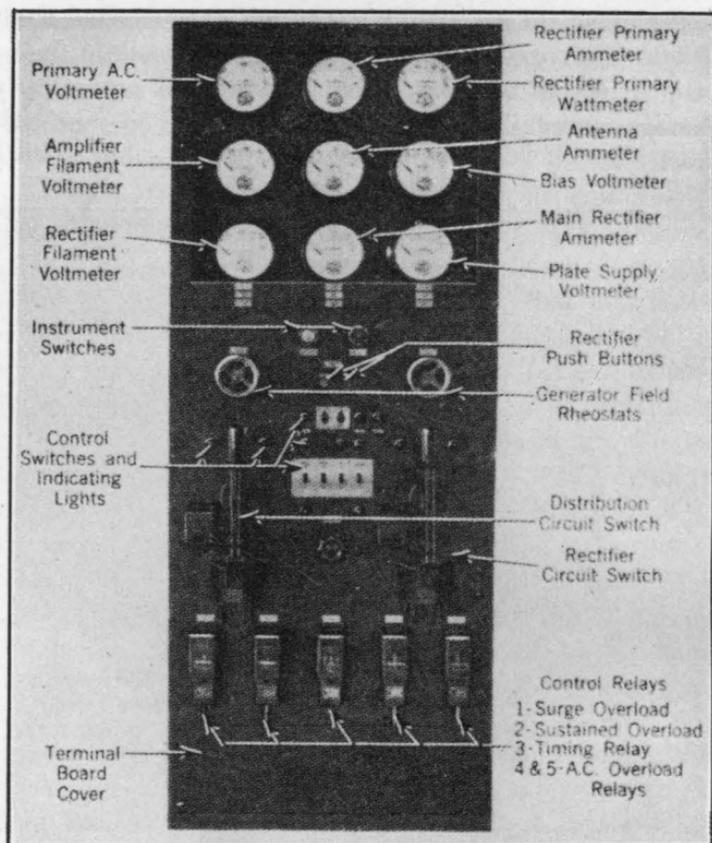
Fig. 507.—The power-control panel of the RCA Model 50-B broadcast transmitter.
