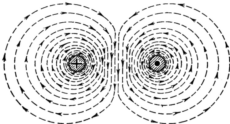
FIG. 8.—Showing the repulsion of magnetic fields between parallel conductors when the current in each is flowing in opposite directions.
