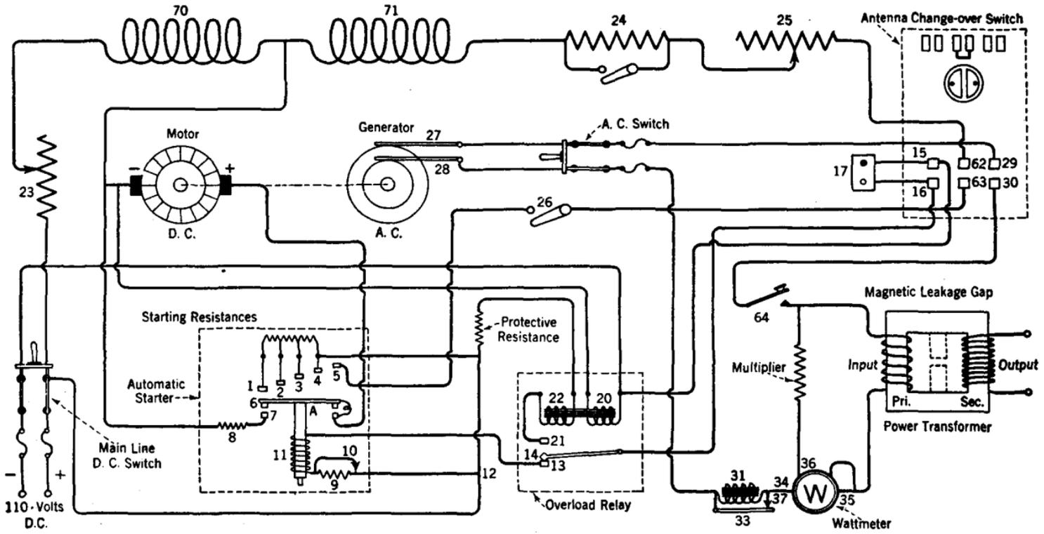
FIG. 50.—Illustrating the “finger” type automatic starter connected in the power circuit of a spark transmitter. Refer to the drawing on page 94 concerning the use of protective condensers.
