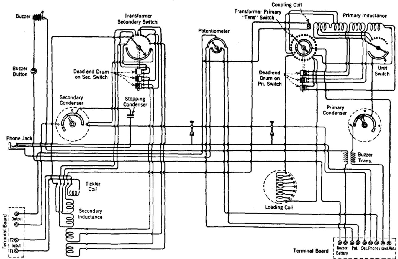
FIG. 242a.—Schematic wiring diagram of the type 106-D commercial receiver. The vacuum tube detector and amplifier unit are connected at the terminal board in the lower left of the diagram.
