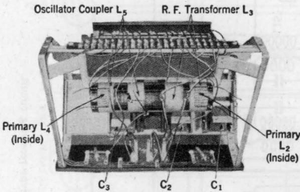
FIG. 204a.—Interior view of eight-tube super-heterodyne receiver.
