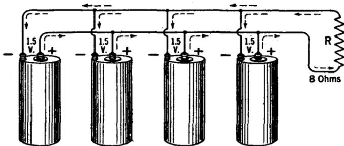
FIG. 13.—Dry cells connected in parallel.
