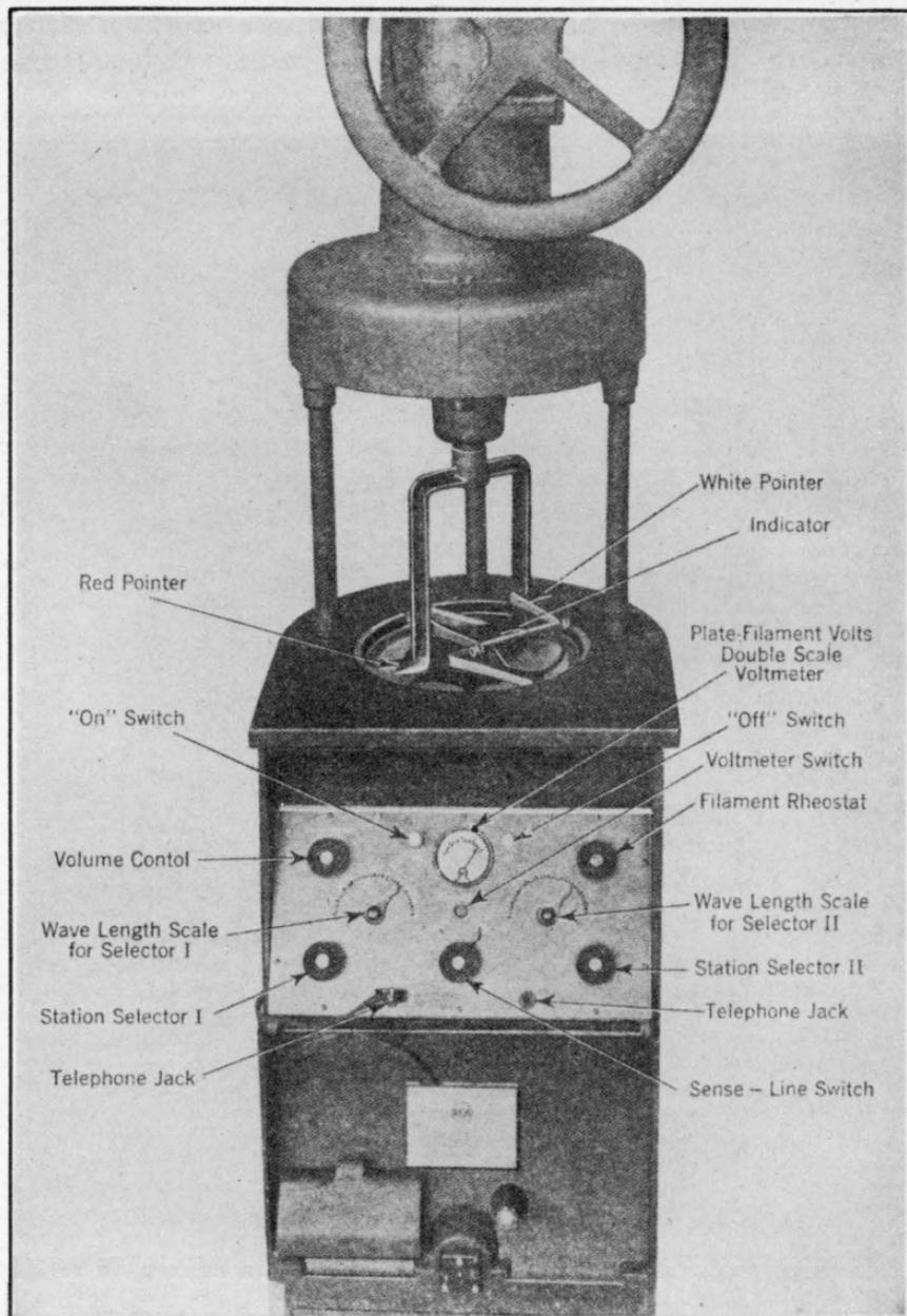
FIG. 416.—One type RCA radio direction finder showing receiver controls and indicator. The rotating element with the red and white pointer is clearly shown mounted directly over the compass scale.
