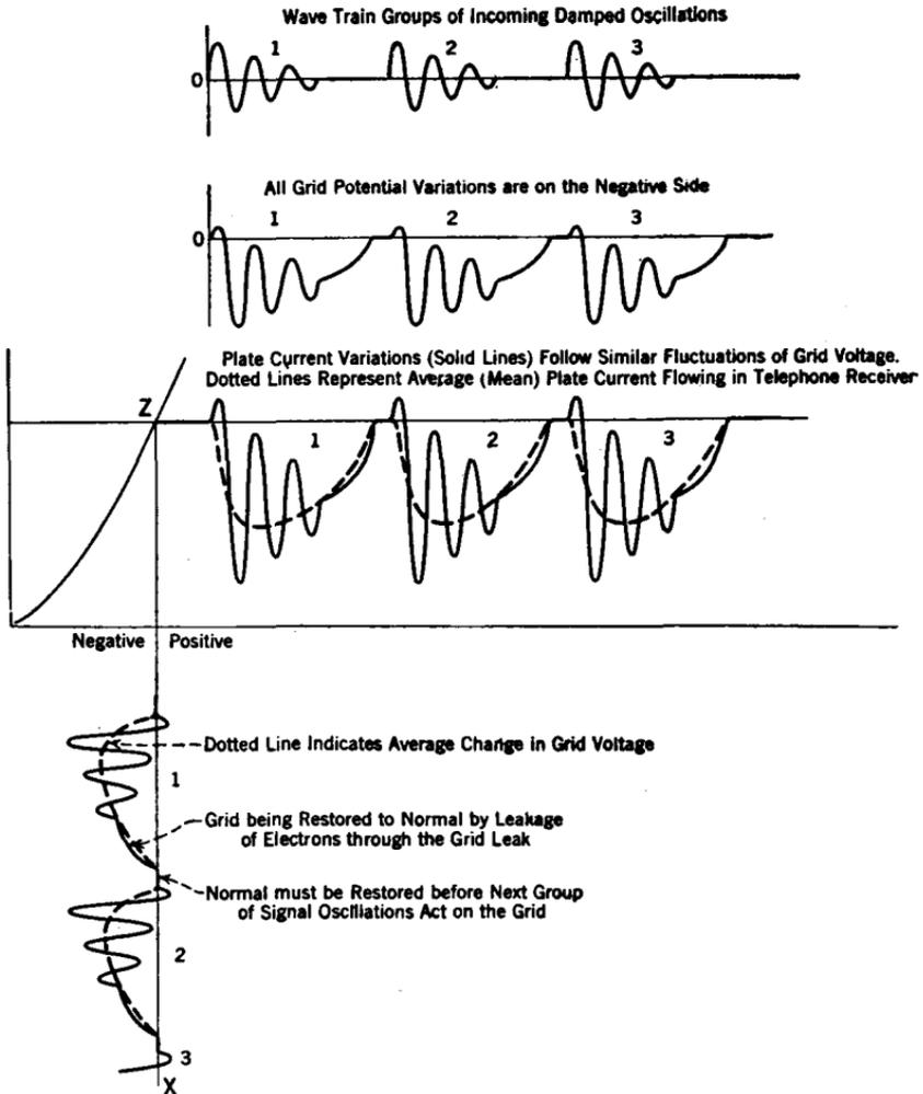
FIG. 165.—These curves depict the action of a signal wave setting up audio-frequency variations in the plate current of a detector tube when a combination grid leak and condenser is used.
