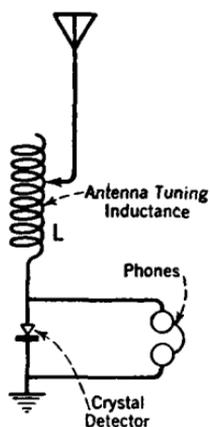
FIG. 184.—A simple radio receiving circuit.
