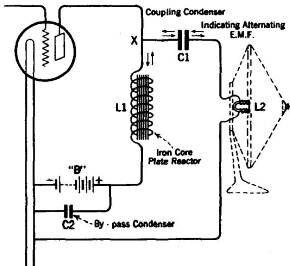
FIG. 266.—One method of coupling the output of a power amplifier tube to a loudspeaker known as “choke coil” or “impedance” coupling. The plate direct current does not flow through the speaker windings. The coupling condenser permits the passage of audio-frequencies from the plate circuit to the loudspeaker.
