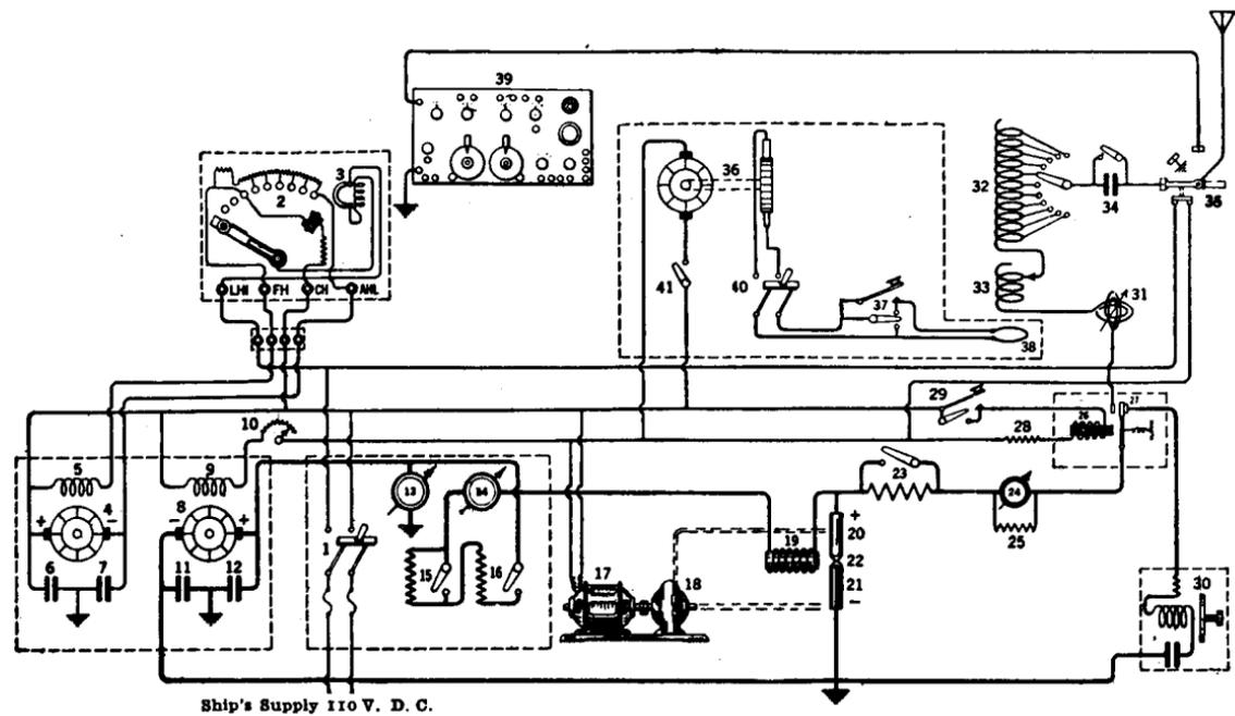
FIG. 410.—Complete schematic wiring diagram of the 2-kw. Federal arc transmitter models K and Q. The back-shunt method of signaling is employed in this transmitter. The numbered parts are as follows:
