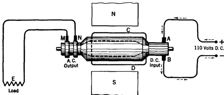
FIG. 43.—An elementary diagram of a rotary converter.
