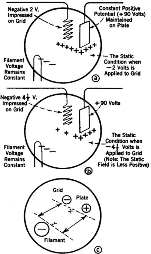
FIG. 131.—A representation of the comparative effects between the electrodes in a vacuum tube.
