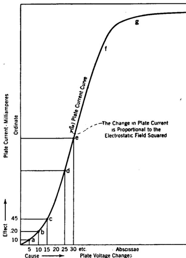
Fig. 150.—Plate-current variations plotted against changing plate-voltage values.
