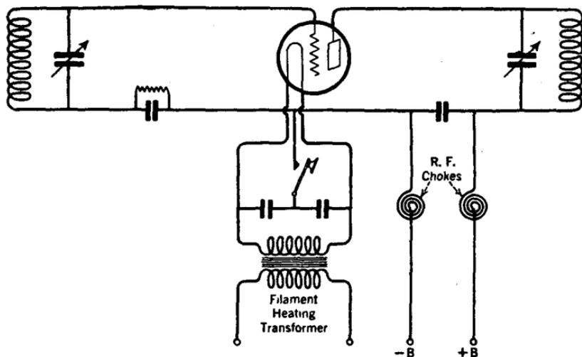
FIG. 330.—Series feed type tuned-plate tuned-grid oscillator.
