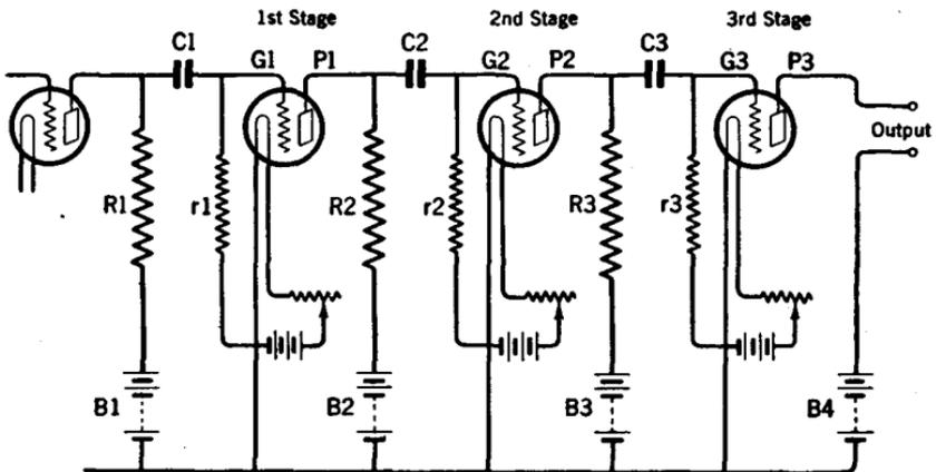
FIG. 208.—A typical resistance coupled amplifier circuit.
