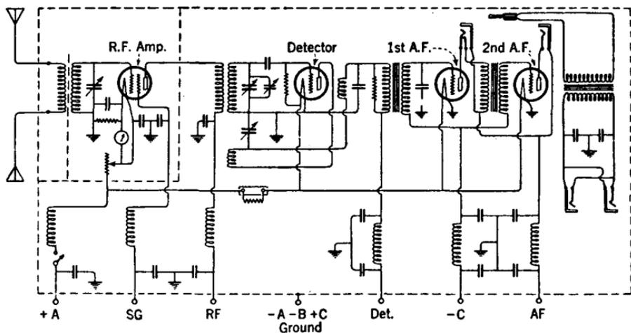
FIG. 457.—Schematic diagram of a short-wave receiver, model AR-1496-D, which is provided with plug-in coils to cover a frequency range of 3750 to 25,000 kc. (12-80 meters).
