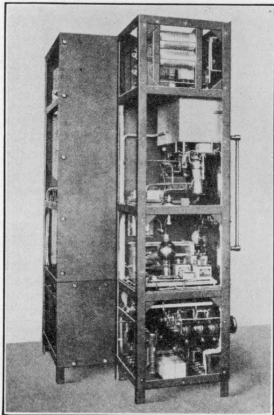
FIG. 385b.—Left side view of 1-kw. high frequency transmitter, Model ET-3656.
