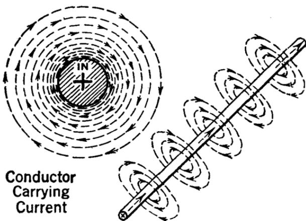
FIG. 5a.—Views showing the direction of lines of force about a conductor when the current is flowing away from the reader.
