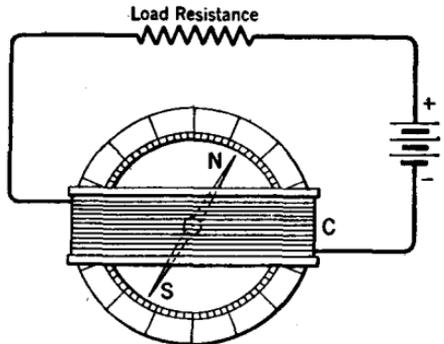
FIG. 81.—Galvanometer connected in a simple d-c. circuit.
