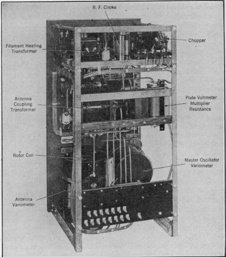
FIG. 361c.—Rear view of ET-3627-A tube transmitter.
