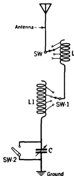
FIG. 180.—One type of an antenna system of a receiving circuit.
