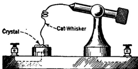
FIG. 183.—A mounted crystal detector.
