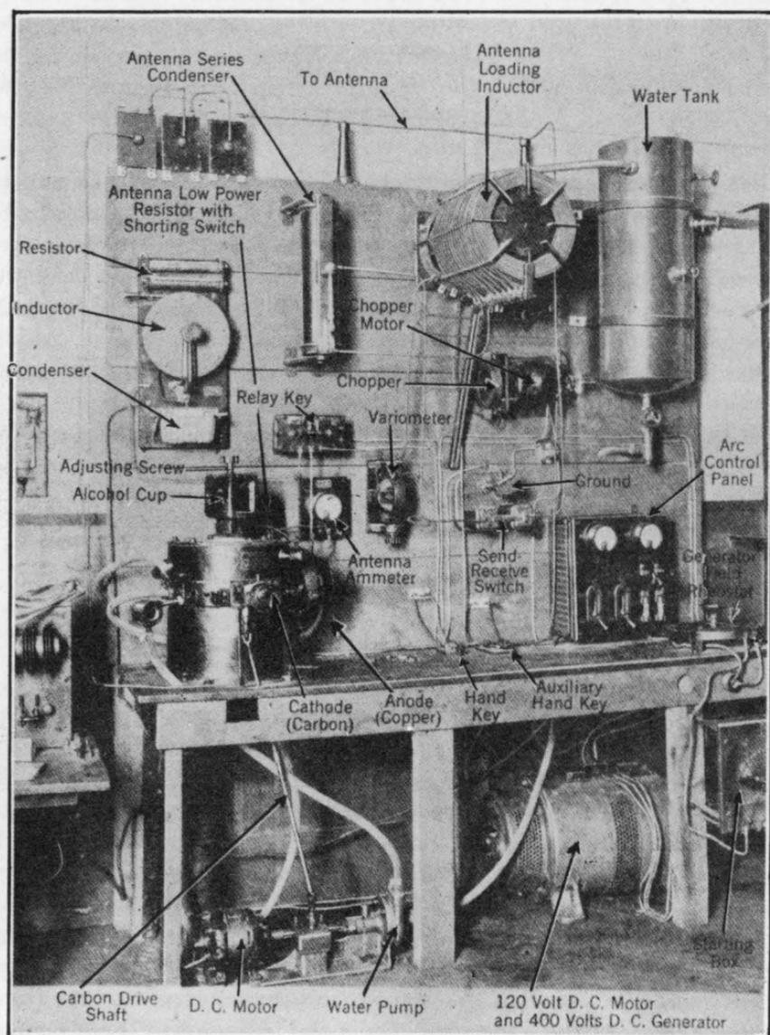
FIG. 403.—The 2-kw. Federal arc transmitter.
