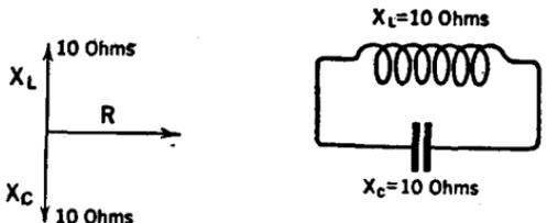
FIG. 99.—If the reactances of a circuit are equal, the only opposition then present is the actual ohmic resistance.
