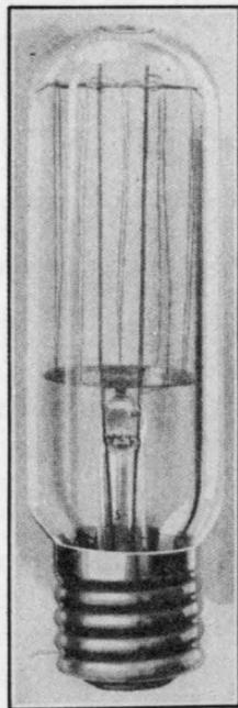
FIG. 243a. — Type UV-876 current regulator tube.
