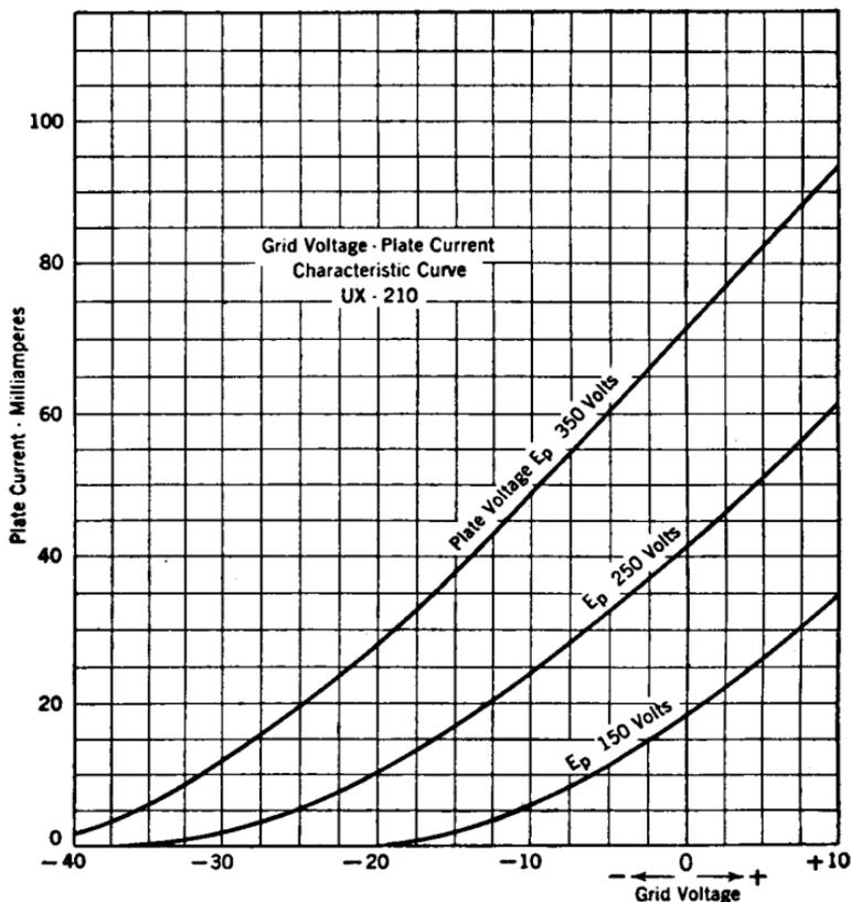
FIG. 176.—Characteristic curves of a 7.5-watt vacuum tube when operated at various plate potentials.
