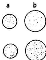
FIG. 132.—Illustrating that an electric charge of a certain magnitude is more concentrated on a small body than on a large one.
