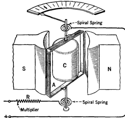
FIG. 82.—Illustrating the operation of a d-c. voltmeter.
