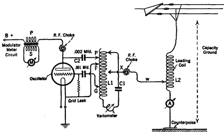
FIG. 336.—The oscillator circuit of a broadcast transmitter showing the tank circuit consisting of  $L_1C_1$  coupled to the antenna by a single feed wire. The radio-frequency choke is used to suppress harmonic radiation.
