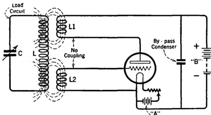
FIG. 324.—Fundamental diagram of the Meissner oscillator circuit.
