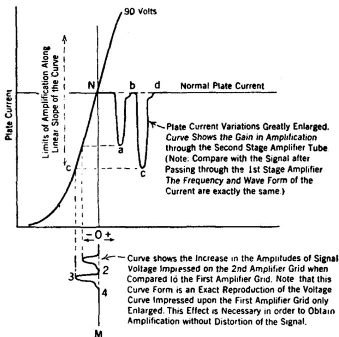
FIG. 173.--Curves illustrating the principle of audio-frequency amplification.
