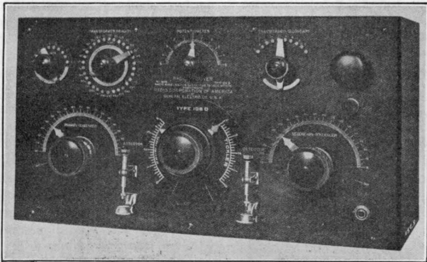
FIG. 241.—Type 106-D commercial receiver.
