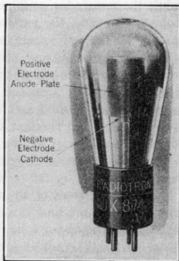
FIG. 252.—Voltage regulator tube, type UX-874.
