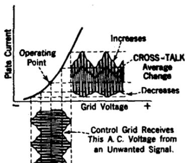
FIG. 226f.—Curves showing that cross-talk is due to the operating point shifting along different locations on the lower knee by the grid bias from an unwanted signal which modulates the desired signal.
