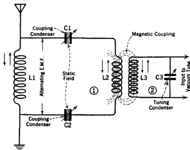
FIG. 265.—A receiving set may employ electrostatic (condenser) coupling between the antenna and the tuned circuit associated with the vacuum tube.
