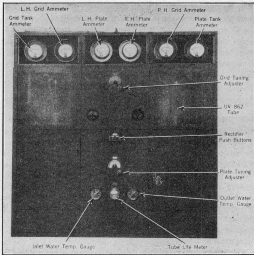
FIG. 501.—The RCA 50-kw. amplifier panel.
