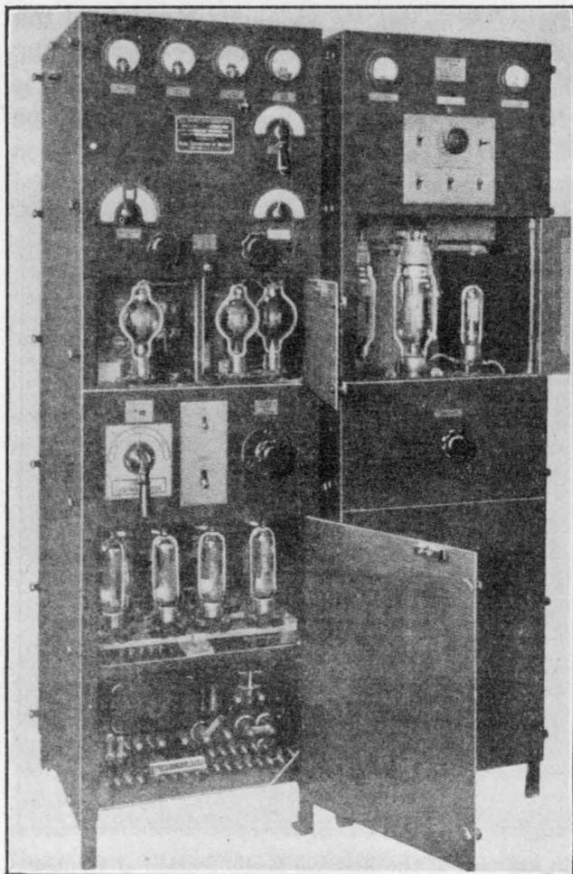
FIG. 442.—The RCA type ET-3666 telegraph and telephone transmitter for use at airports. The radio-frequency unit is the left-hand section of the transmitter; the modulator is on the right.
