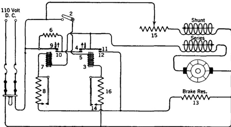
FIG. 49.—Automatic starter connected to a compound-wound motor.
