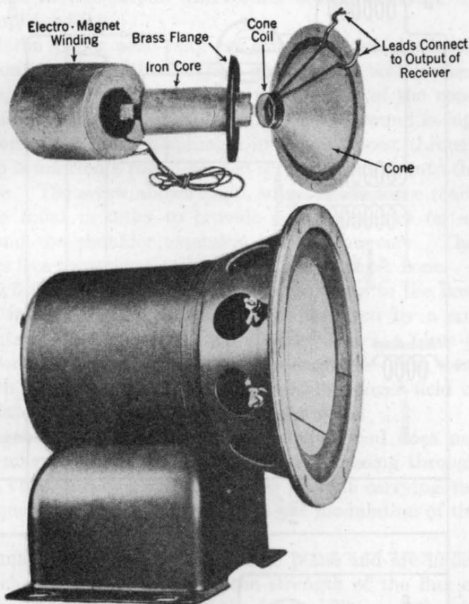
FIG. 234.—The three essential parts and complete assembly of the electrodynamic type loudspeaker.
