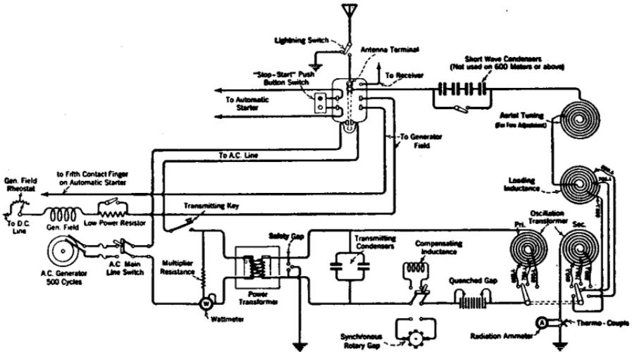
FIG. 389.—The circuits of a spark transmitter from the a-c. source of supply to the antenna.
