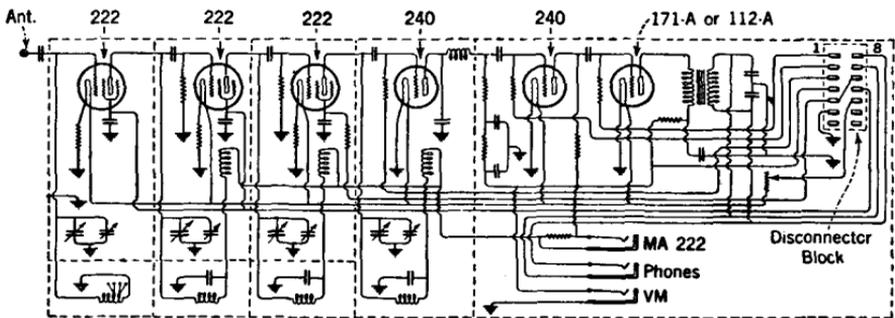
FIG. 453.—Schematic diagram of an aircraft beacon receiver consisting of three stages of tuned radio-frequency amplification, a detector, and two stages of audio-frequency amplification.
