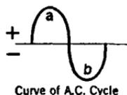
FIG. 133.—Showing the alternations of current induced in a circuit composed of inductance and capacitance.
