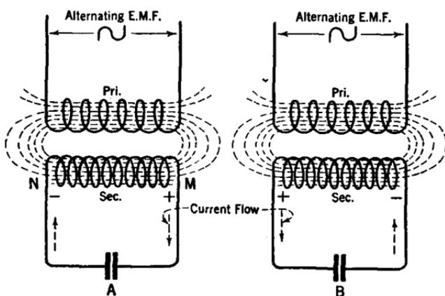
Fig. 133 show how a condenser is charged by an alternating electromotive force. The primary and secondary windings are illustrated. When an alternating current flows in the primary (*Pri.*) the changing flux around *Pri.* induces an alternating voltage in secondary *Sec.* The curve of one cycle of this induced alternating e.m.f. is shown. One cycle is sufficient to explain the action.
