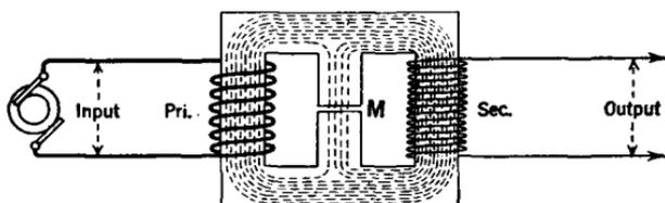
FIG. 396.—A conventional diagram of a closed core power transformer equipped with a magnetic leakage gap.
