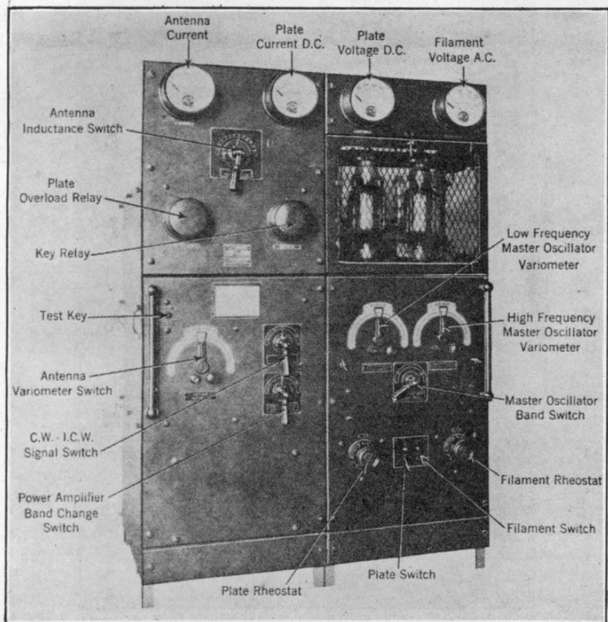
FIG. 363.—Front view of 2-kw. radio telegraph tube transmitter, model ET-3638.
