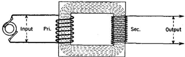
FIG. 394.—A conventional diagram of a closed core power transformer with the flux permeating the iron core.
