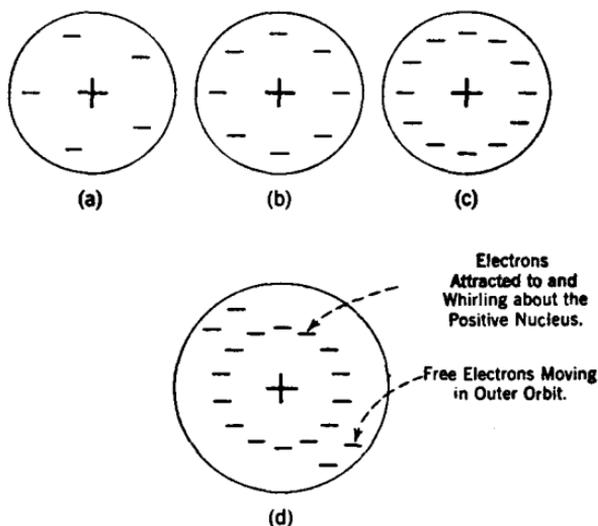
FIG. 142.—A graphical illustration of different atoms showing how electrons might be arranged in numerical groups. The electrons are rapidly whirling about and held in attraction by a positive electric charge.
