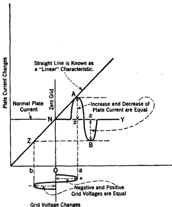
FIG. 172.—A chart for explaining a linear characteristic. Note that proportional changes are in a direct ratio. If the distance from *O* to *a* equals the distance from *O* to *b*, then *x* to *A* must equal *x* to *B* since *N* to *A* equals *N* to *Z*. (The straight diagonal line could be made steeper and different values of grid voltages could be applied.)
