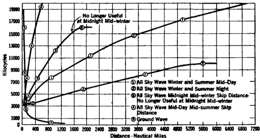
FIG. 381b.—These curves show the relative distances (communication range) that short waves of different frequencies may carry during the summer and winter months.
