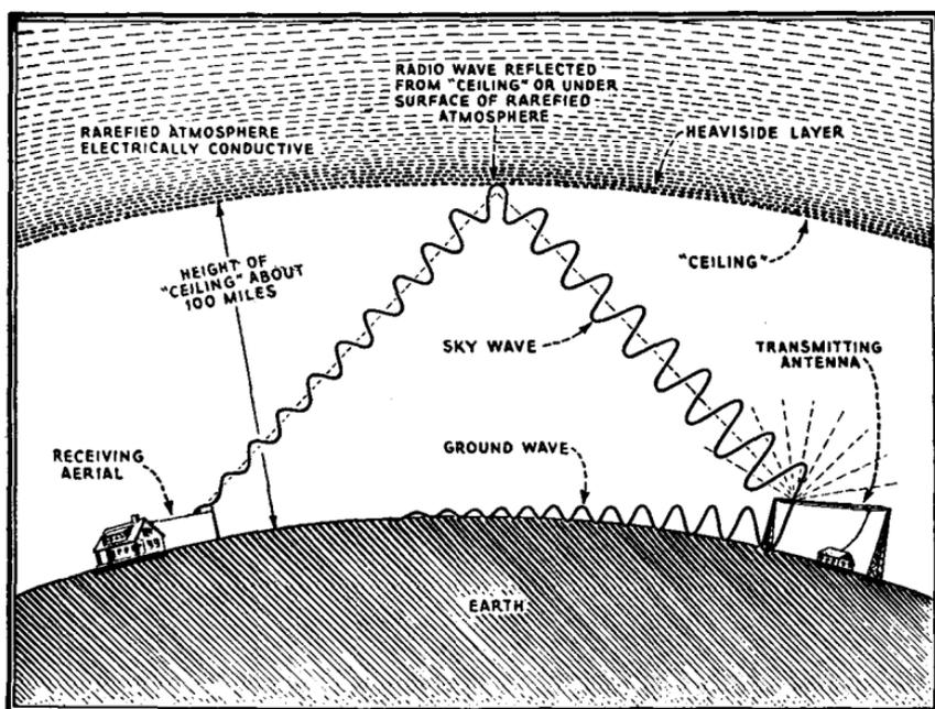
FIG. 285.—A graphical explanation of the Heaviside-Kennelly theory of radio wave propagation between sundown and sunrise.
