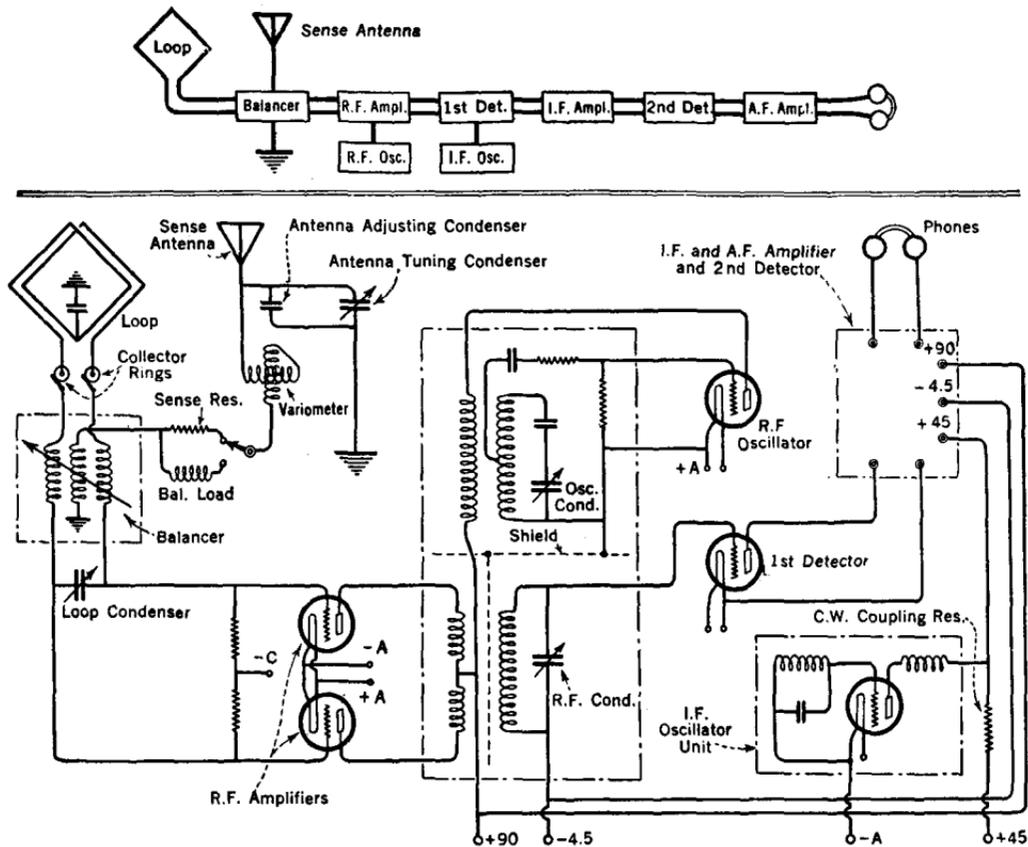
FIG. 417.—Schematic diagram of a standard marine direction finder which operates in conjunction with a super-heterodyne receiver.
