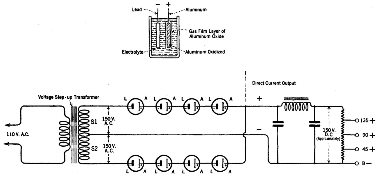
FIG. 249.—Circuit arrangement showing how several electrolytic jars are connected to provide full wave rectification. The upper sketch illustrates the principle upon which an electrolytic rectifier operates.
