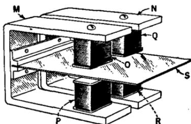
FIG. 436.—Construction of a reed converter.
