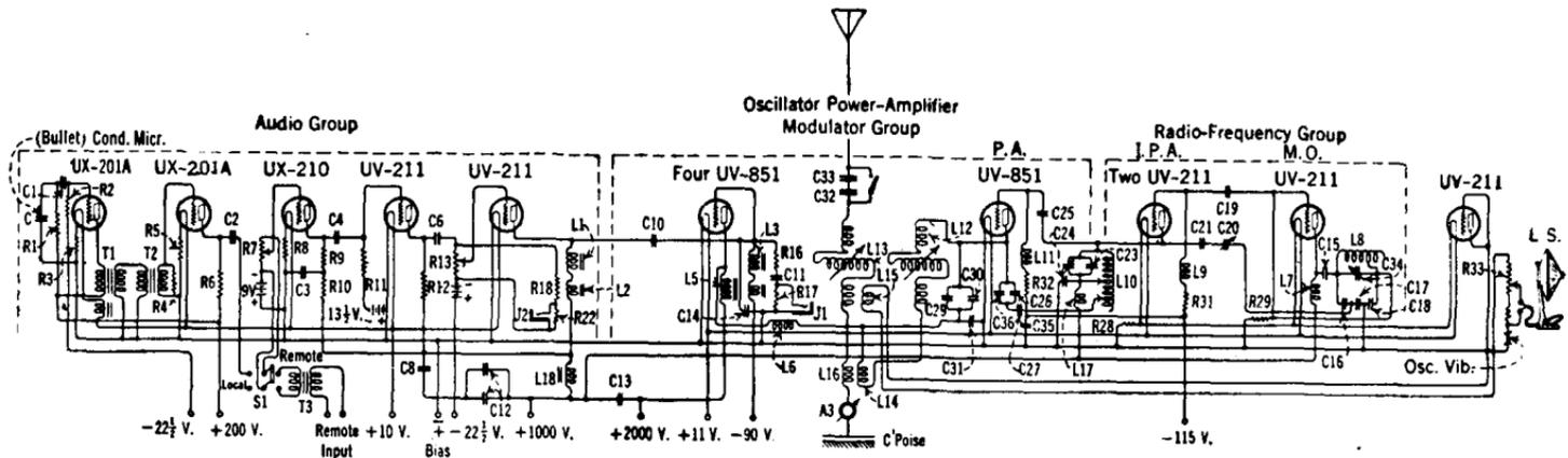
Fig. 319.—Schematic circuit diagram of a standard 1-kw. broadcast transmitter. Note particularly how the condenser type microphone is connected in the circuit and supplied with a potential of about 200 volts through resistance R<sub>1</sub>. Also how the variable resistances R<sub>7</sub> and R<sub>13</sub> are arranged to control modulation, called volume control. When a remote microphone is used its input power will be sufficient to be delivered to the grid of the UX-210 tube.
