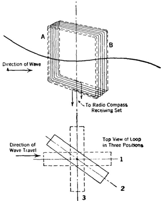
FIG. 420.—As shown by this drawing a maximum signal will be heard with the loop in position 1, whereas when in position 3 a minimum or no signal will be heard.
