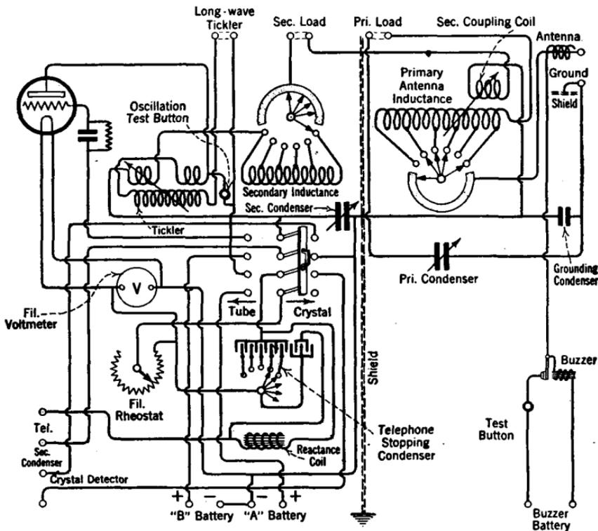
FIG. 236.—Wiring diagram of the IP-501 commercial receiver.
