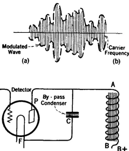
FIG. 262.—This diagram shows why a small bypass condenser is placed between plate and filament of a detector tube. The condenser serves to bypass the carrier frequency, i.e., the radio-frequency component of the plate current. The modulation or audio component passes through the plate coil AB.
