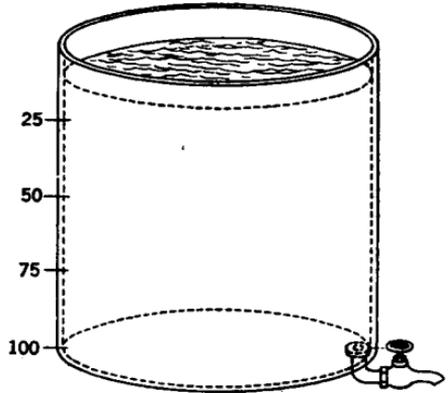
FIG. 89.—Illustrating pressure levels in a tank of water. This is a simple analogy for the difference of electrical pressure in a circuit.
