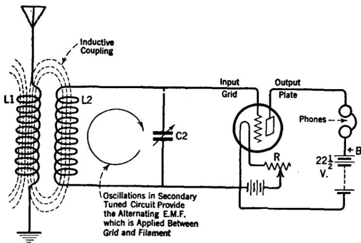
FIG. 156.—A fundamental vacuum tube detector circuit.
