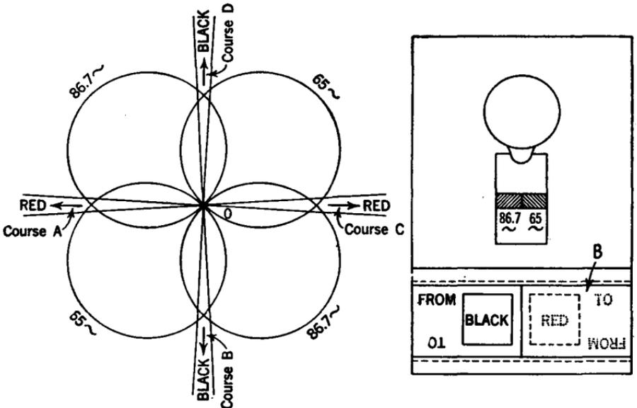
FIG. 433.—Diagram showing how the four beacon courses are produced in the directions where the radio intensities from the two antennas are equal; also reed indicator with shutter system to fit indication to red or black courses.
