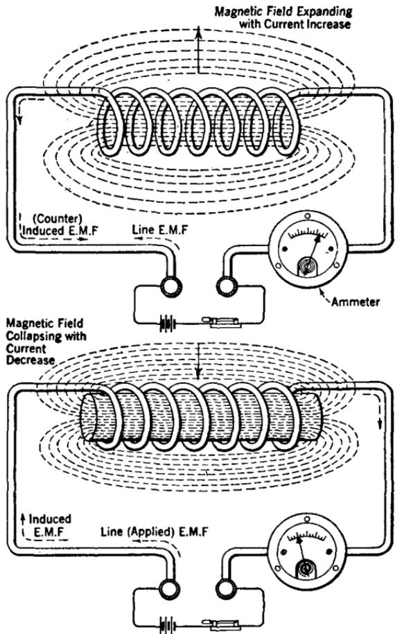
FIG. 100.—Demonstrating the momentary effect of self-inductance in a circuit when the current is made to undergo a change.
