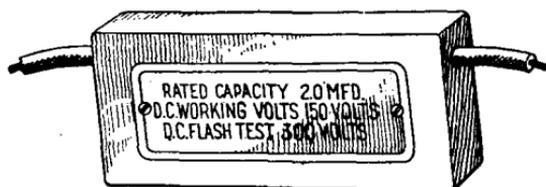
FIG. 260.—A type of low-voltage condenser employing specially treated paper as the dielectric and tinfoil as the conducting material (plates).
