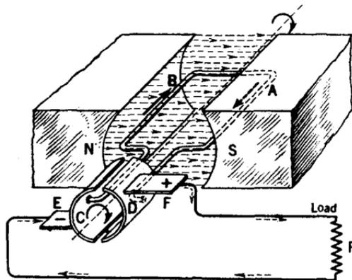
FIG. 31.—Showing how an armature of a d-c. generator is connected to commutator segments to supply a direct current to the external or load circuit.
