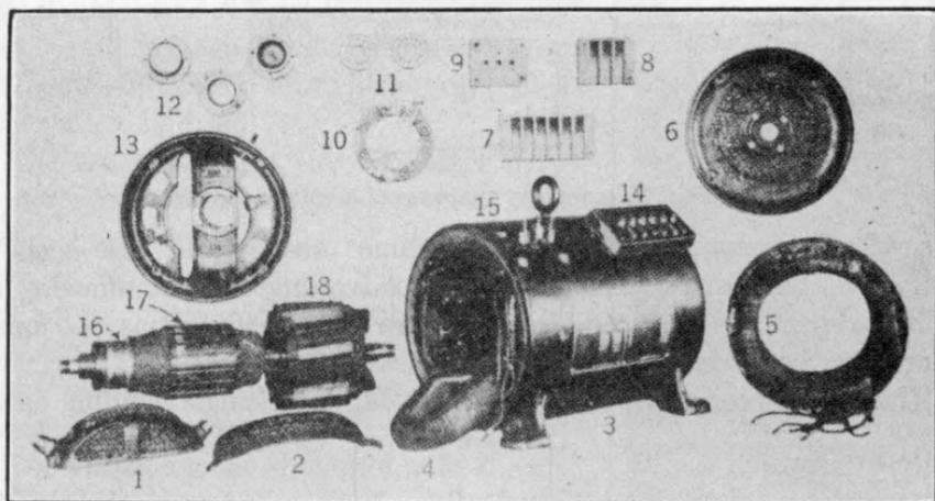
FIG. 42.—Disassembled Holtzer-Cabot 2-k.w. motor-generator.
