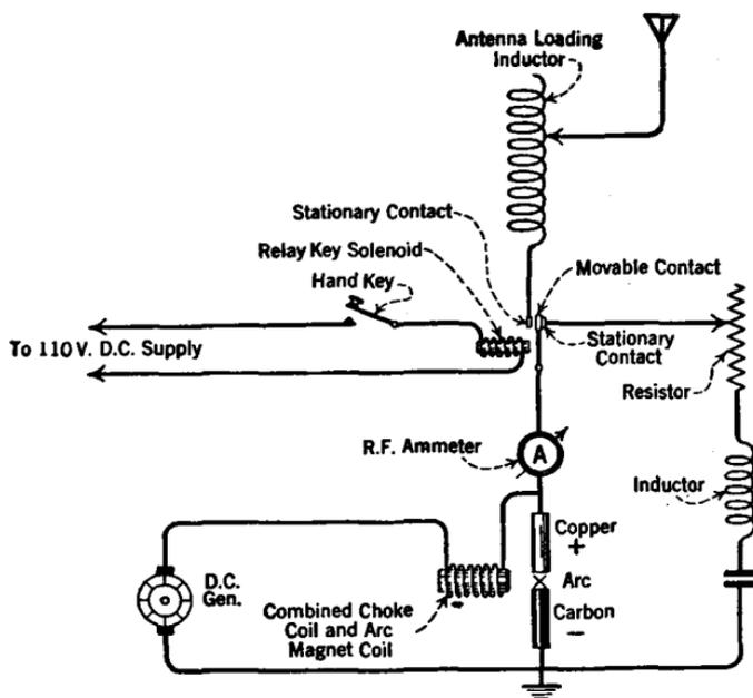
FIG. 405.—A fundamental arc diagram showing the circuit arrangement for the back shunt method of signaling.
