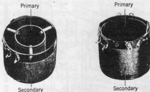
FIG. 211.—Showing on the left a loosely coupled radio-frequency transformer; on the right a closely coupled r.f. transformer.
