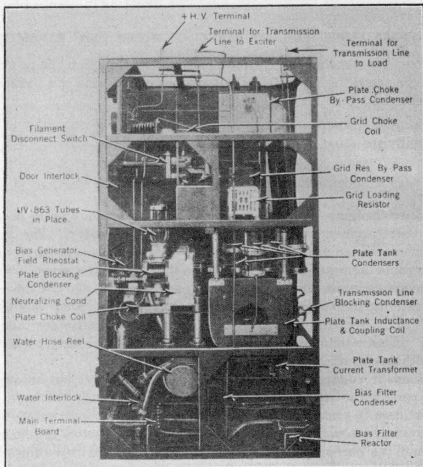
FIG. 500.—End view of a 5-kw. amplifier panel.
