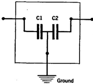
FIG. 52.—Protective device for motor-generator windings.
