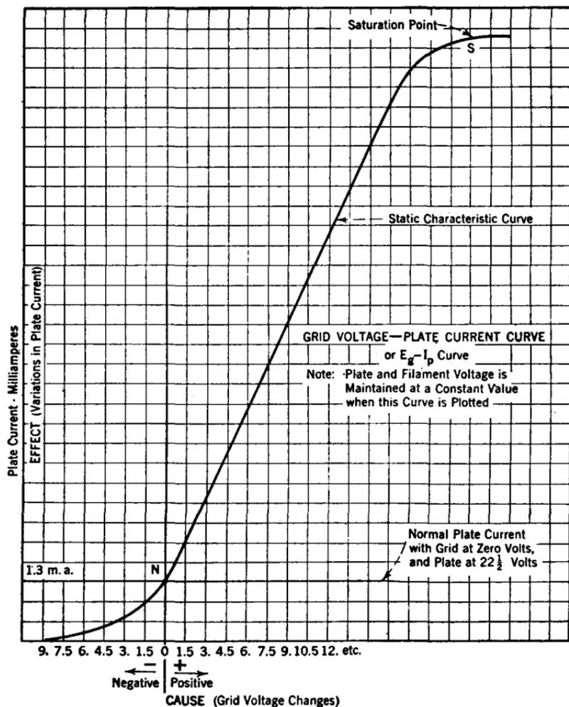
FIG. 155.—Plate current variations plotted against changing grid voltage values.
