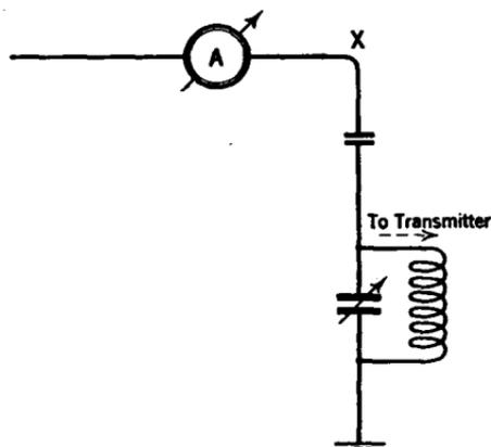
FIG. 377a.—One method of constructing an antenna for short wave transmission. This is known as the single wire voltage feed system.
