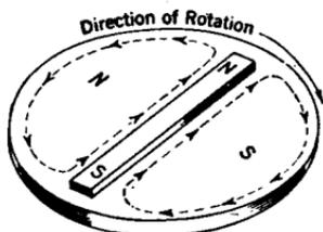
FIG. 56.—Showing how eddy currents are produced.
