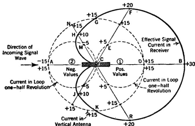
FIG. 426.—Depicting unilateral characteristics. The effective strength of the signal shown by the heart-shaped curve (cardioid) is obtained by combining the loop current and the vertical antenna current while rotating the loop.
