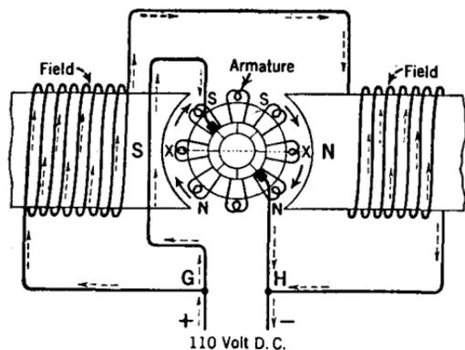
FIG. 32.—This view shows why a d-c. motor armature is set into rotation when the field and armature coils are supplied with current from a d-c. source.
