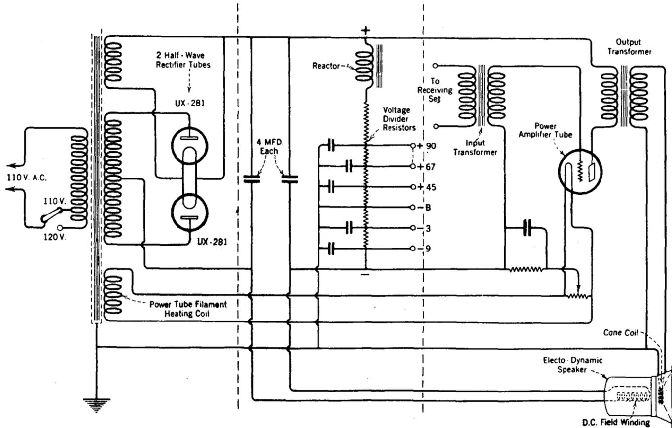
FIG. 234a.—A schematic diagram of a complete socket power unit, including the power amplifier circuit of a receiver. The diagram clearly shows how the field winding of an electrodynamic speaker is energized by the output of the rectifier.
