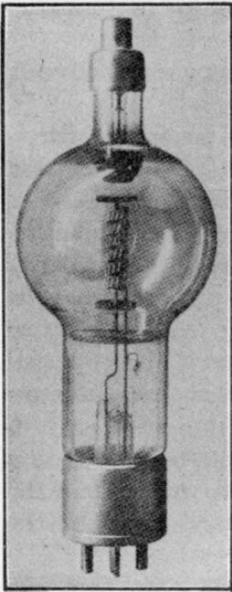
FIG. 508.—UV-869 transmitting tube.
