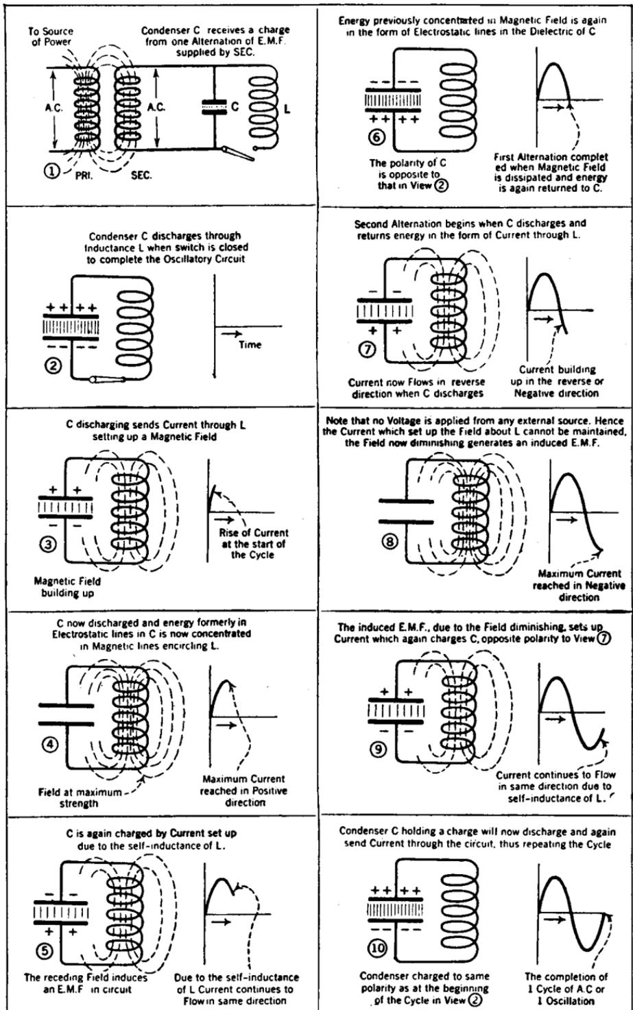
FIG. 273.—The principles which govern the production of radio-frequency current in an oscillatory circuit by the discharge of a condenser through an inductance.
