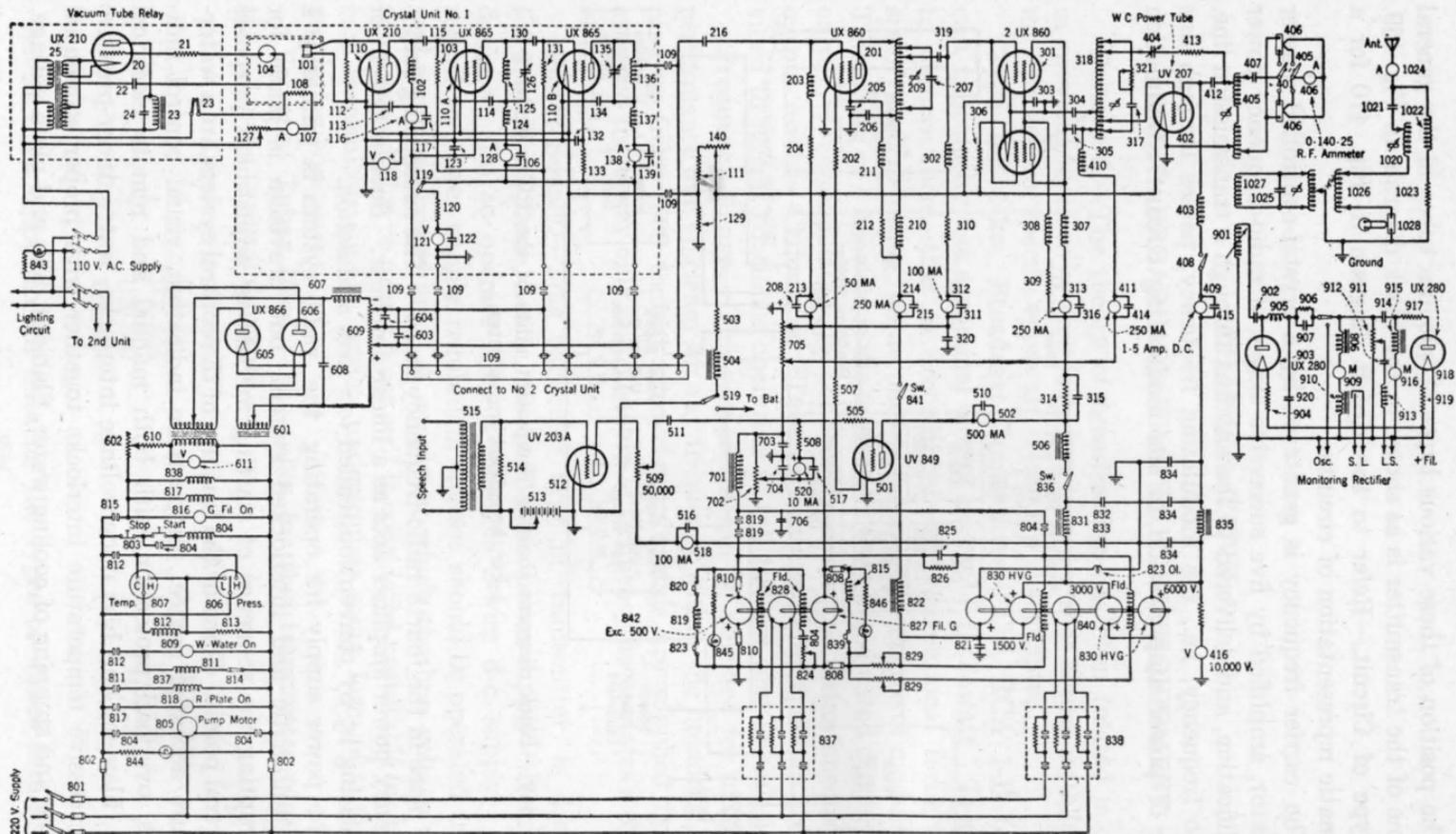
FIG. 470.—Schematic diagram of the circuits in the RCA 1-kw. broadcast transmitter Model 1-B.
