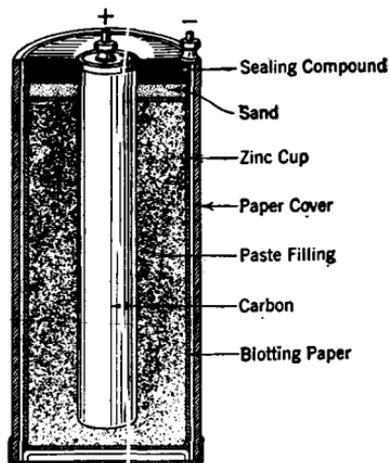
FIG. 11.—Cross-sectional view showing the construction of a dry cell.
