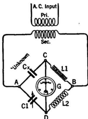
two parallel paths of the bridge is obtained from the secondary of a transformer, an alternating current being supplied to the input or primary side. The unknown condenser is connected in the branch of the circuit between A and C. The alternating current which flows through this condenser must also flow through resistance coil  $L_1$ . A standard variable condenser calibrated in units of microfarads is connected in the other branch of the circuit ADB.
