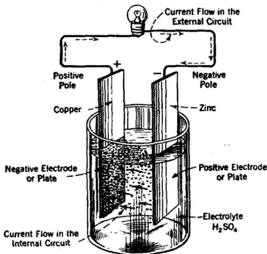
FIG. 10.—The voltaic cell.
