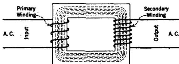
FIG. 25.—A schematic diagram of an iron core step-up transformer.
