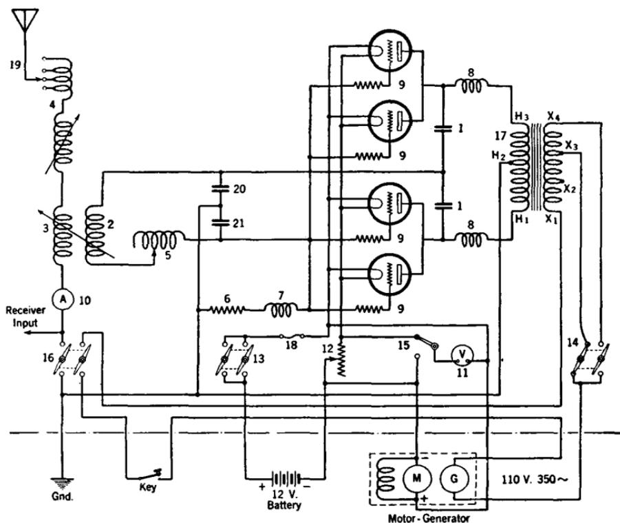
Fig. 372.—Schematic diagram of the ET-3650 telegraph transmitter.
