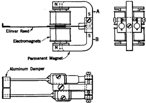
FIG. 432.—Sketches of reed indicator construction.
