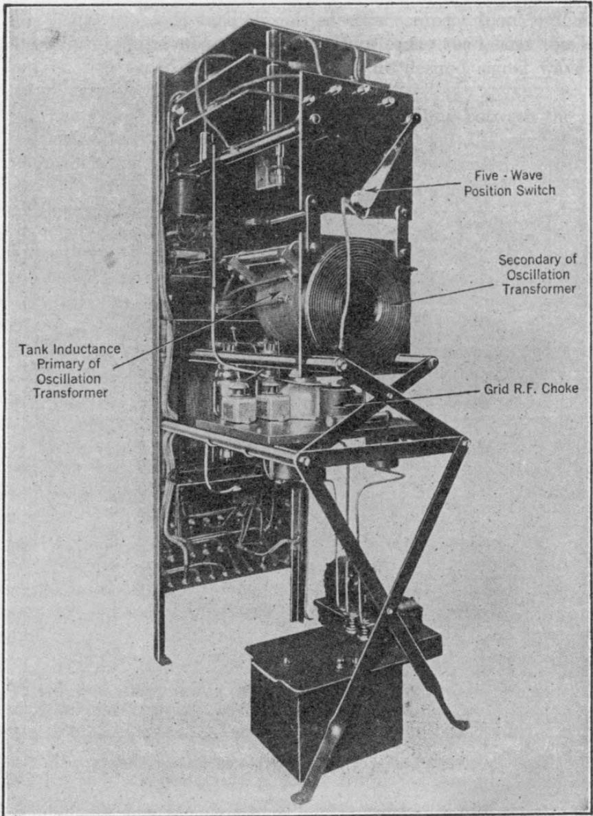
FIG. 343a.—Rear view of converted P-8 vacuum tube transmitter model ET-3628.
