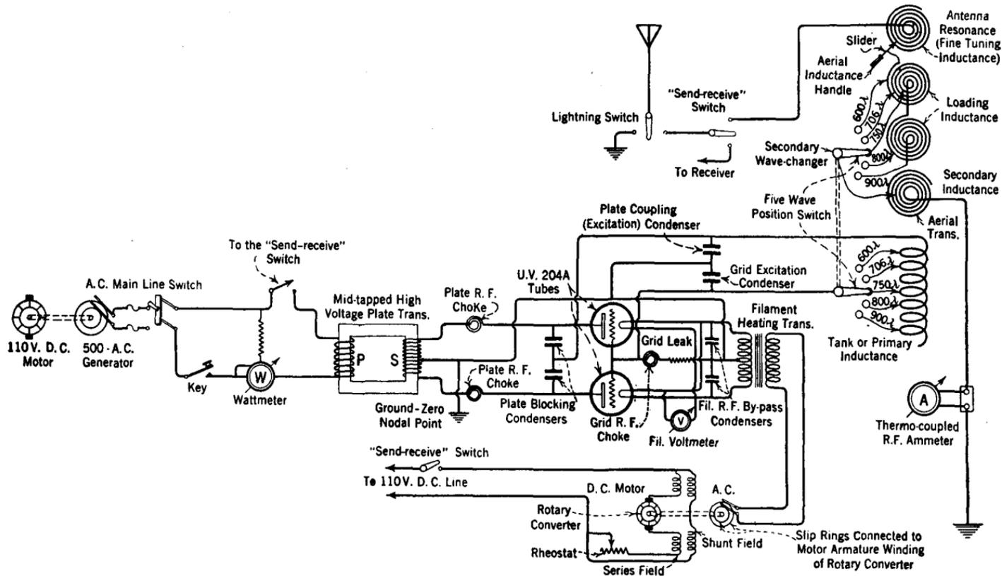
FIG. 344.—Complete schematic diagram of the ET-3628 tube transmitter employing two UV-204A tubes operating “back to back” in a self-rectifying circuit to produce full wave A.C.C.W. transmission. The radiated wave is of the tone-modulated variety. The Colpitts type oscillator circuit consists of the tank inductance, the plate coupling condenser and the grid excitation condenser. The plates of the UV-204A tubes are energized by the 500-cycle high-voltage output of the mid-tapped transformer.
