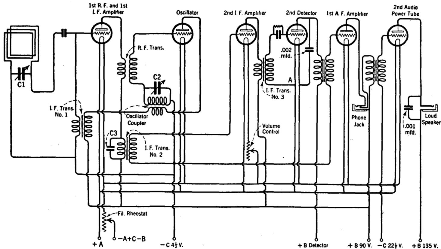
FIG. 203.—A schematic diagram of a six-tube super-heterodyne, second harmonic, receiver employing a loop aerial.
