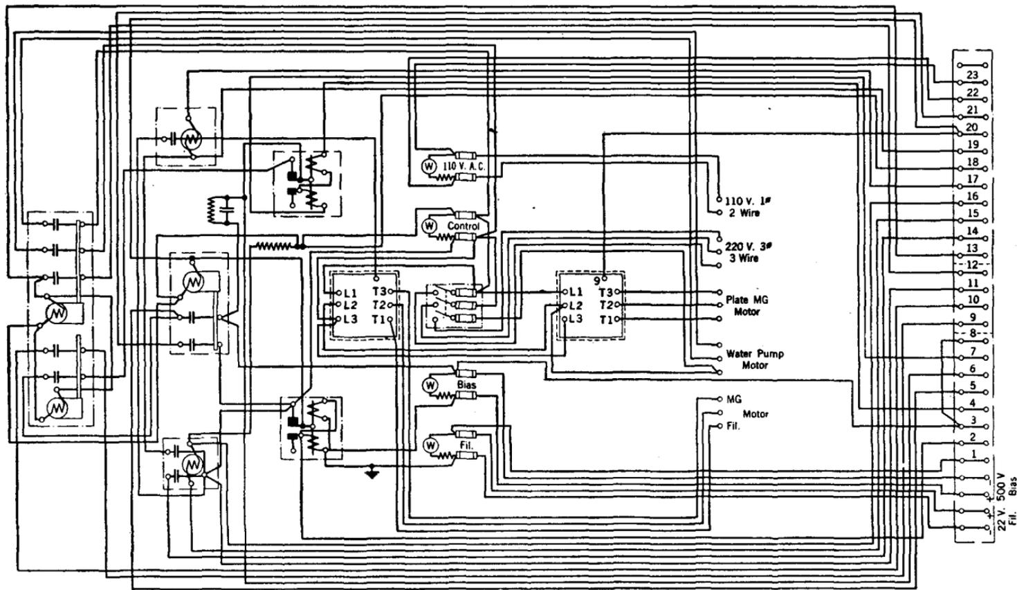
FIG. 478.—Connection wiring diagram for the a-c. power-control panel of the RCA 1-kw. broadcast transmitter.
