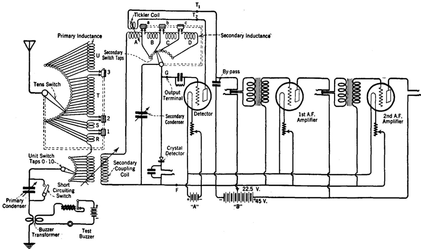
FIG. 240.—Fundamental diagram of type 106-D commercial receiver with detector and two-stage amplifier.
