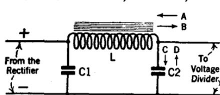
Fig. 254.—How a filter system of the "brute force" type is arranged.
