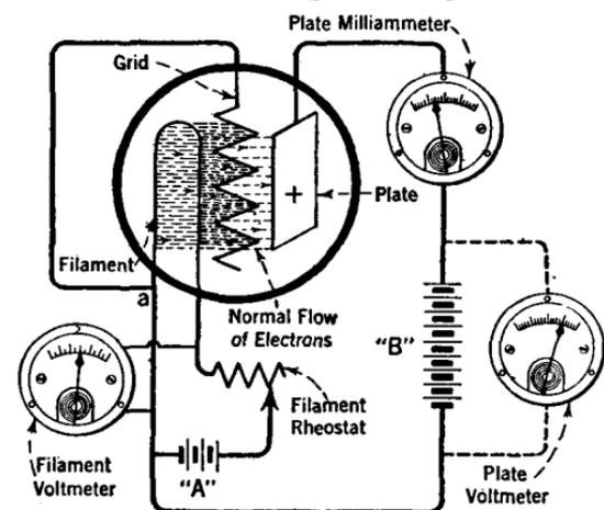
FIG. 145.—A fundamental three-element vacuum-tube circuit.
