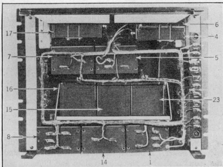
FIG. 517.—Rear view of RCA type 12A amplifier.
