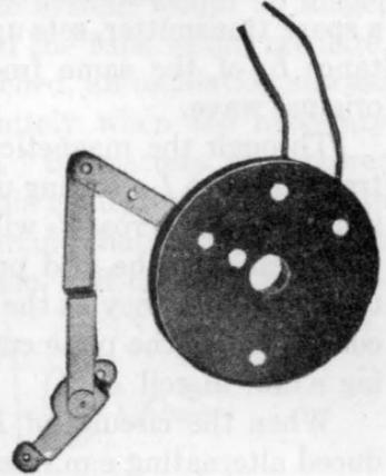
FIG. 206a.—A tickler coil mounted to permit lateral movement. *The coil can be in and out of inductive relation to the grid coil (not shown).*
