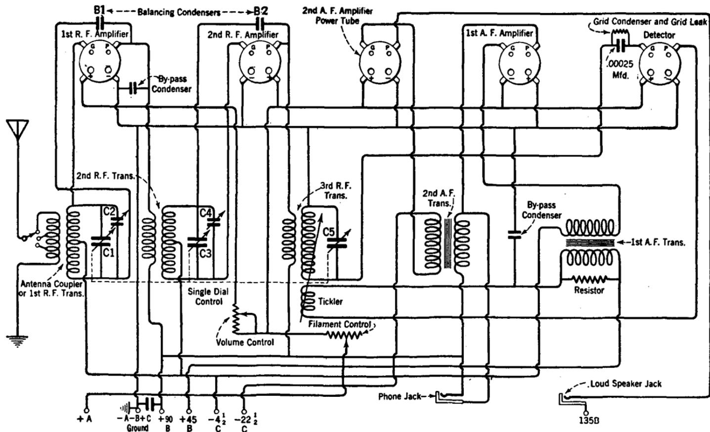
FIG. 216.—A schematic diagram of a five-tube balanced receiver of the tuned radio-frequency type employing a regenerative detector.
