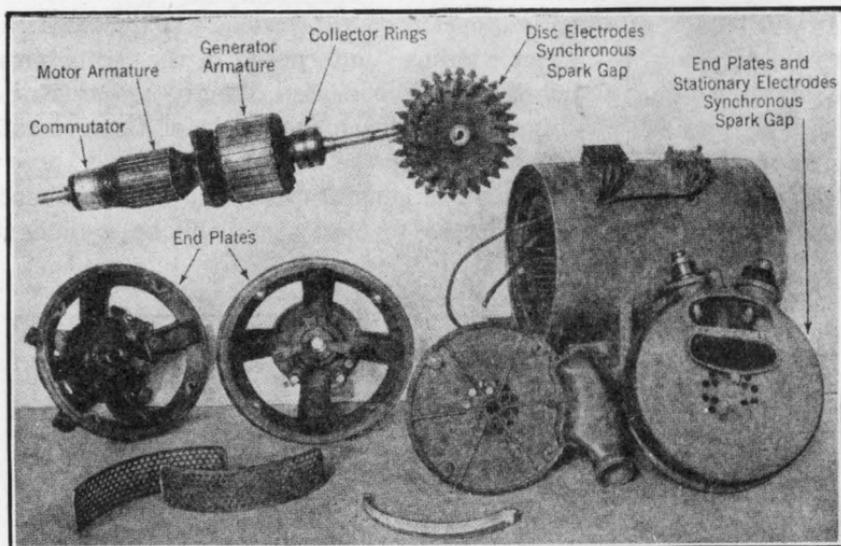
FIG. 40.—General Electric 2-kw. 500-cycle motor-generator.
