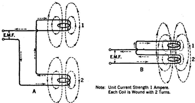
FIG. 190.—Another circuit for illustrating the principles of mutual inductance.
