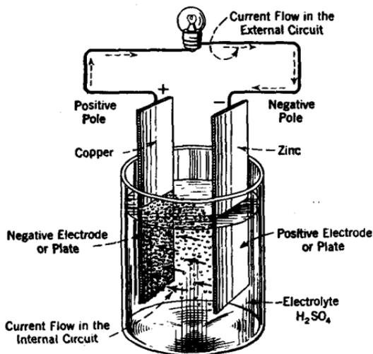
FIG. 10.—The voltaic cell.
