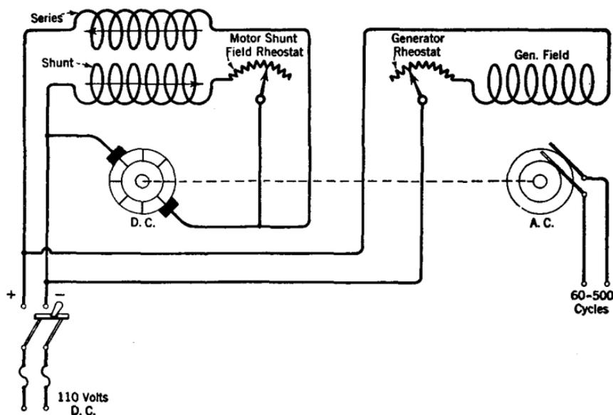
FIG. 39.—Diagram of a differential d-c. motor coupled to an a-c. generator.
