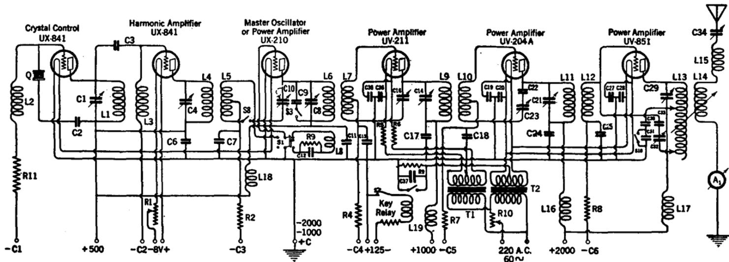
FIG. 309.—Circuits of a 1-kw. High Frequency Transmitter.
