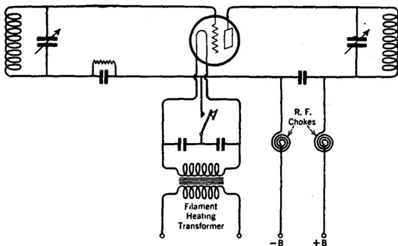
FIG. 330.—Series feed type tuned-plate tuned-grid oscillator.
