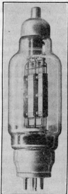
FIG. 487.—Type UV-849 transmitting tube.
