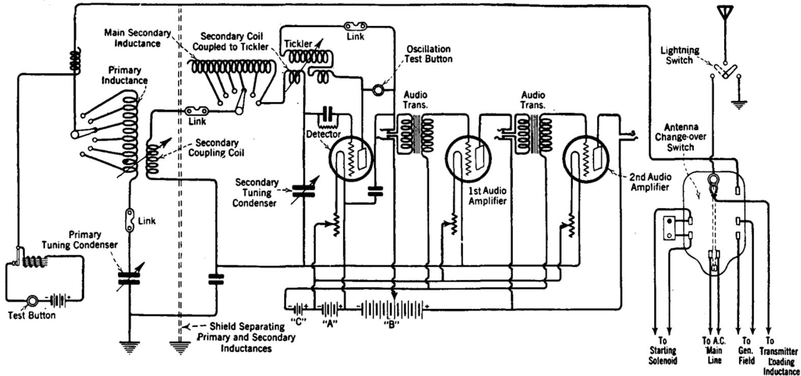
FIG. 236a.—Schematic diagram of the IP-501 commercial receiver with audio-amplifier system and connected to the type "I" antenna changeover switch. The three links are removed when the long-wave loading unit is attached to the receiver.
