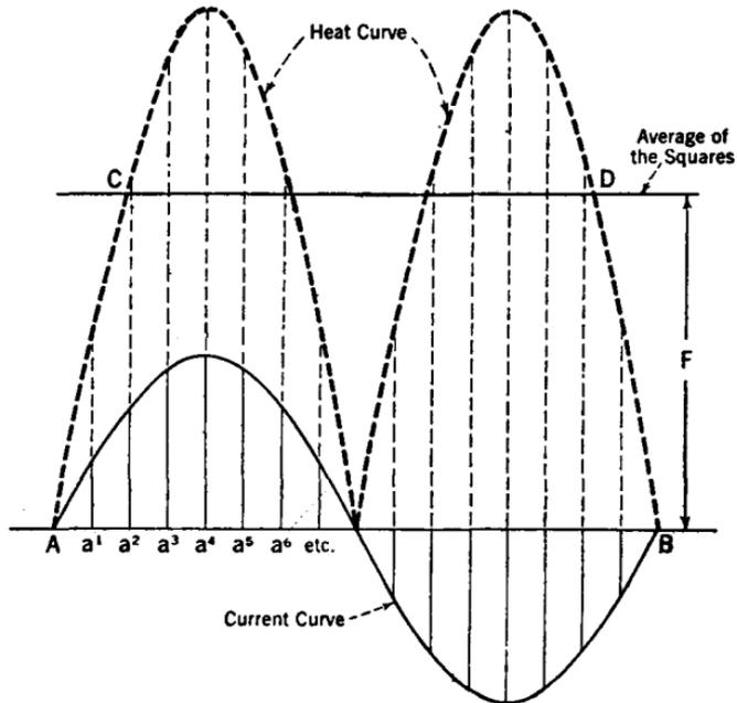
FIG. 107.—A graphical representation of the heating effect of alternating current.
