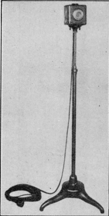
FIG. 512.—Condenser microphone, amplifier and program stand.
