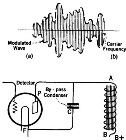
With the above considerations in mind, we will illustrate several of the practical uses of condensers in radio circuits. In Fig. 262 a condenser, called a *bypass* condenser, is connected between the plate and
