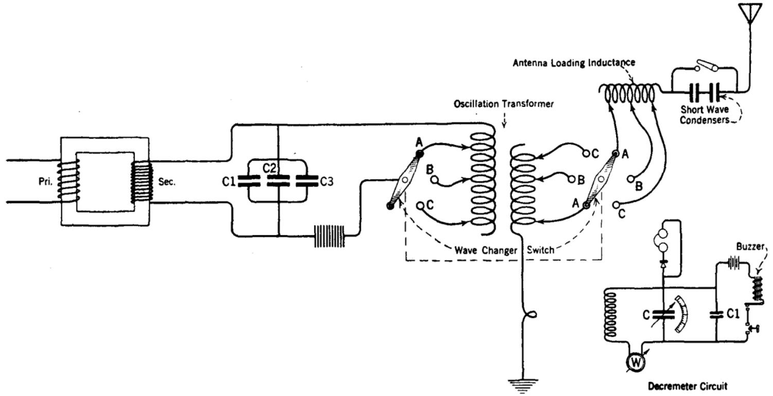
FIG. 294.—Showing the use of a decrometer to measure or indicate characteristics of the emitted wave of a spark transmitter.
