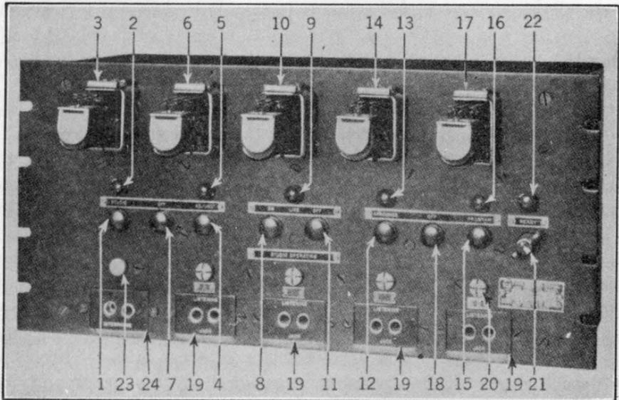
FIG. 519.—Front view of RCA type 18B signal and control panel with relay covers removed.
