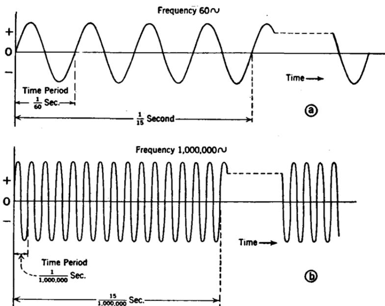
FIG. 93.—Showing the time periods of a low frequency and a high frequency alternating current.
