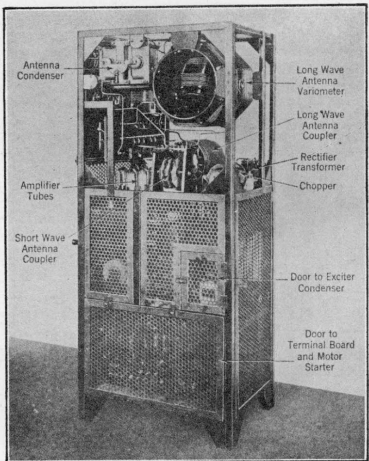
FIG. 347.—Right side view of ET-3626 tube transmitter.
