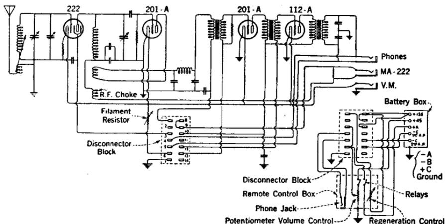
FIG. 456.—A schematic diagram of the RCA type AR-1308 aircraft communication receiver.
