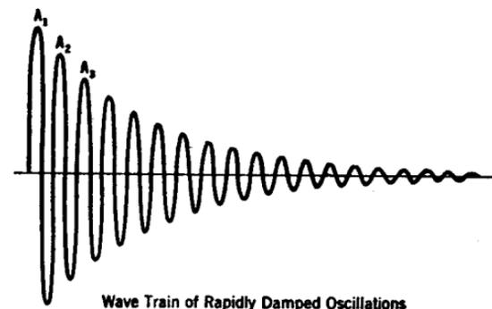
Wave Train of Rapidly Damped Oscillations
