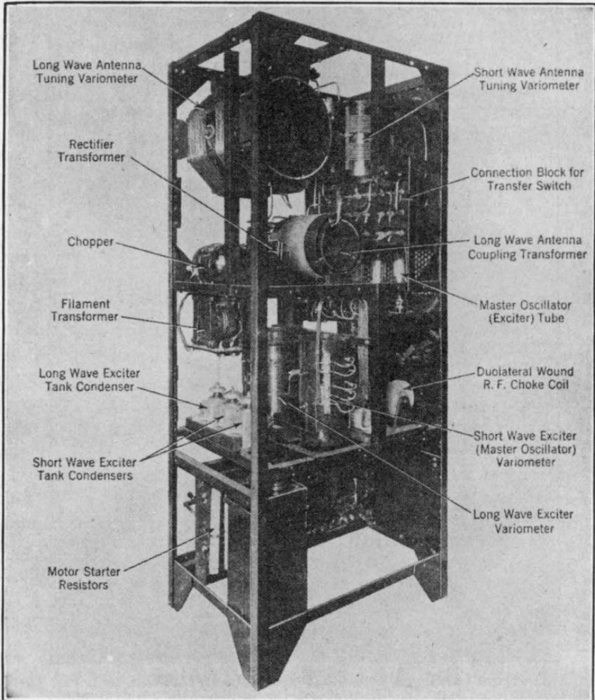
FIG. 346.—Rear view of vacuum tube transmitter type ET-3626.
