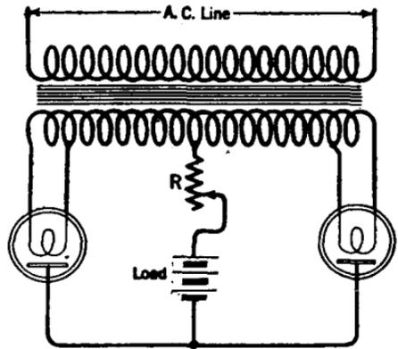
FIG. 78.—Full-wave rectifier circuit for battery charging.
