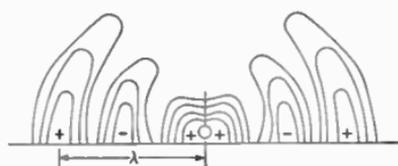
The capacity effect then exists between the antenna and the earth. The distribution of the electrostatic lines of force from a grounded antenna is as shown in Fig. 2. This figure also shows the probable
