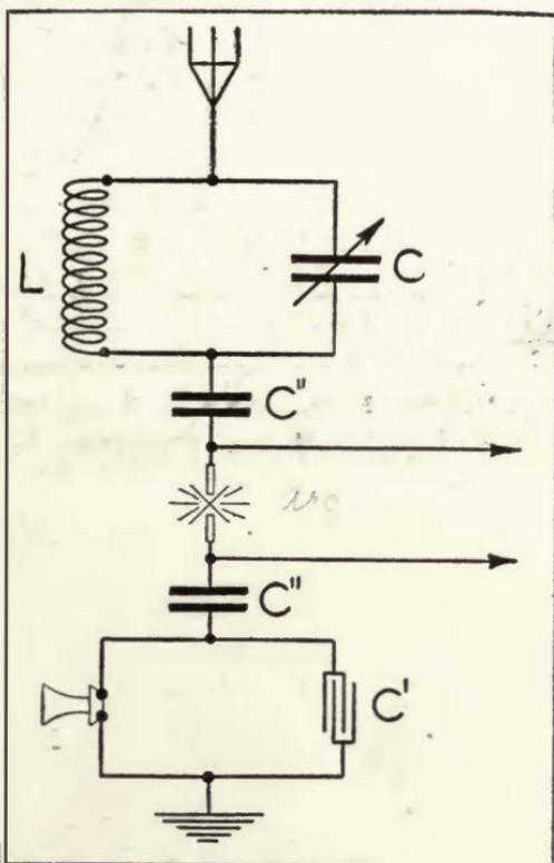
FIGURE 15—Fly-wheel Poulsen arc circuit for radio telephony.
