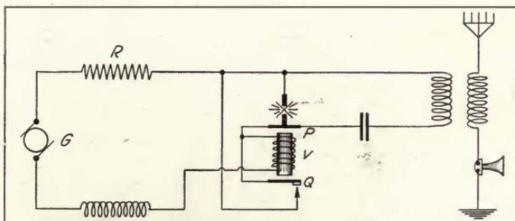
FIGURE 54—T. Y. K. radiophone transmitter.
