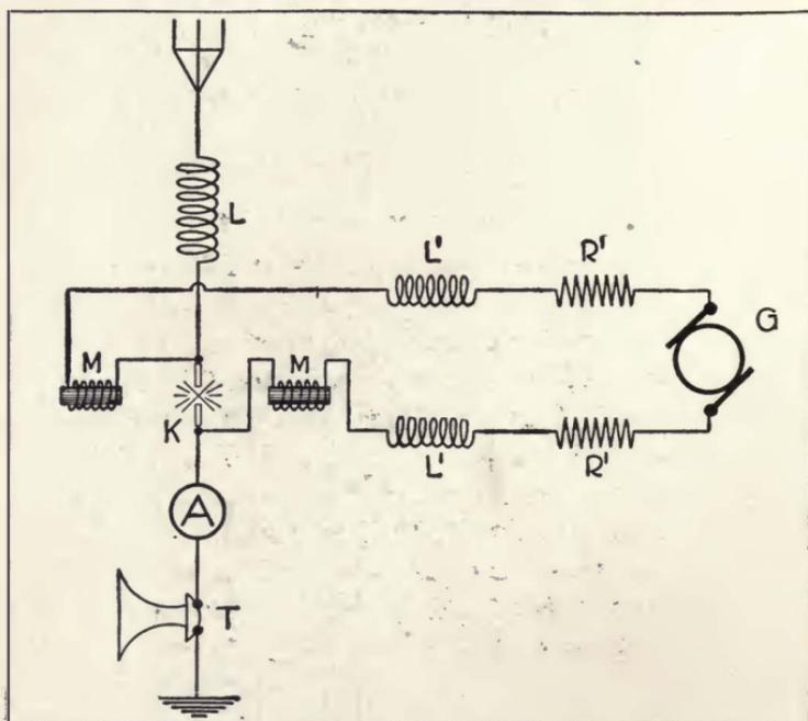
FIGURE 10—Typical arc radiophone transmitter.
