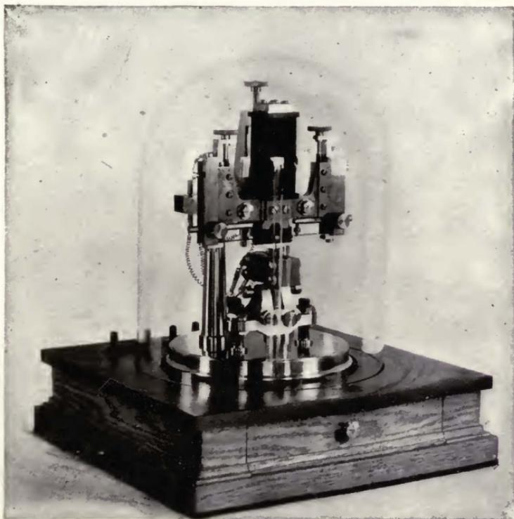
FIGURE 135—Fessenden heavy current telephone relay.
