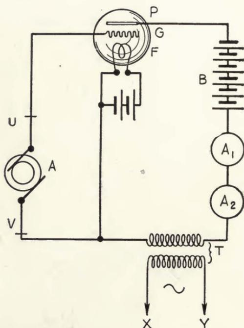
FIGURE 77—Amplification of alternating current energy.
