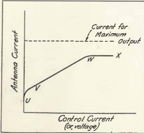
FIGURE 128—Typical incomplete non-linear modulation control curve.
