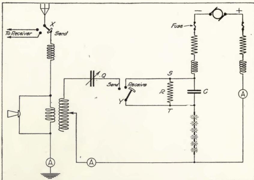
FIGURE 26—Telefunken series arc radio transmitter.
