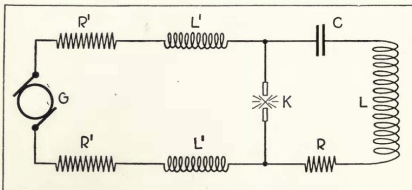
FIGURE 9—Typical arc circuit.
