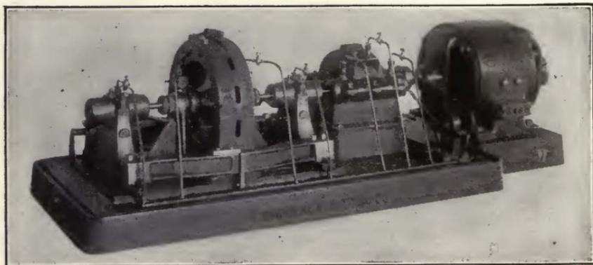
FIGURE 122—Recent type of 2 K.V.A., 100,000 cycle Alexanderson alternator.
