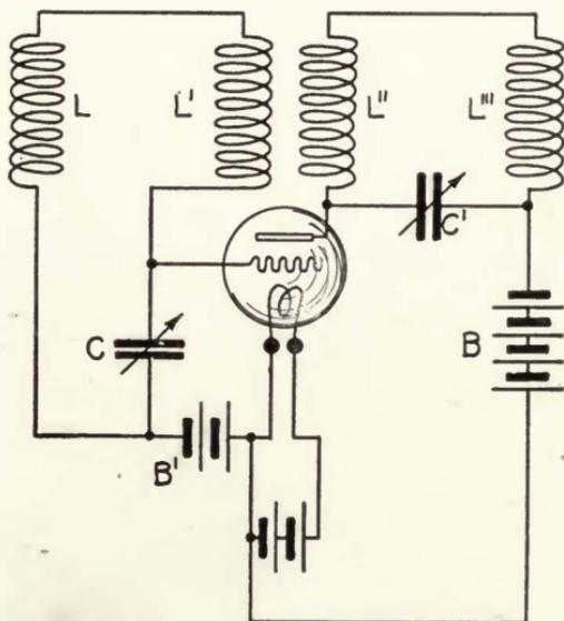
FIGURE 84—Marconi Company-Franklin Circuit, 1914.
