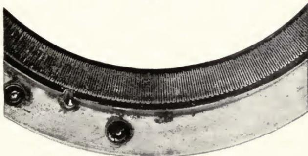
FIGURE 117—Portion of armature winding of 100,000 cycle Alexanderson alternator; 600-slot type.
