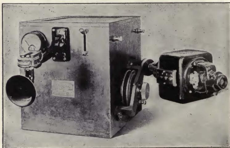
FIGURE 61—de Forest D. C. radiophone transmitter.
