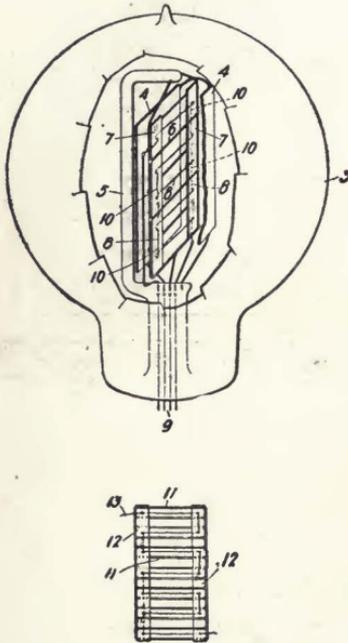
FIGURE 211—Western Electric Company—van der Bijl amplifier tube, 1915.
