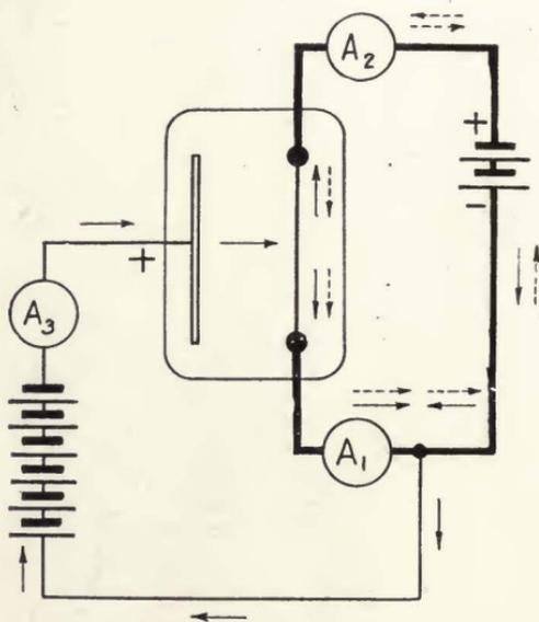
FIGURE 74—Illustrating Combined Lighting and Thermionic Currents.
