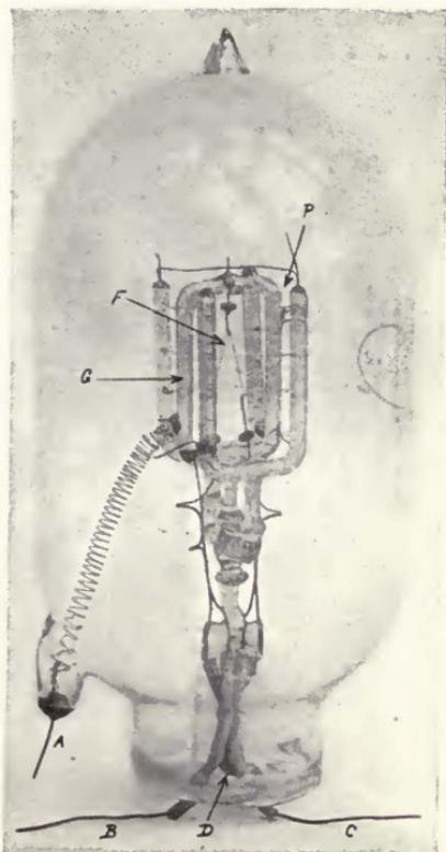
FIGURE 214 — General Electric Company-White small pliotron amplifier.
