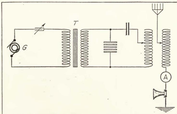
FIGURE 64—de Forest radiophone transmitter—A. C. type.
