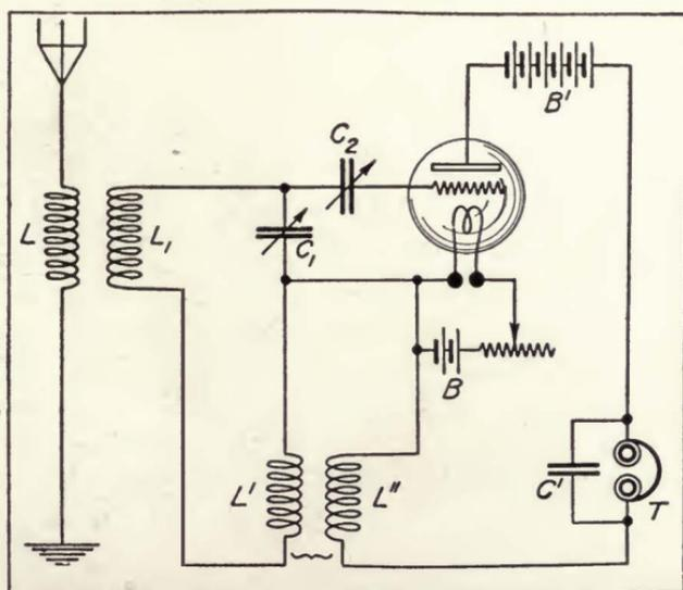
FIGURE 202—Armstrong regenerative circuit for radio frequency amplification.
