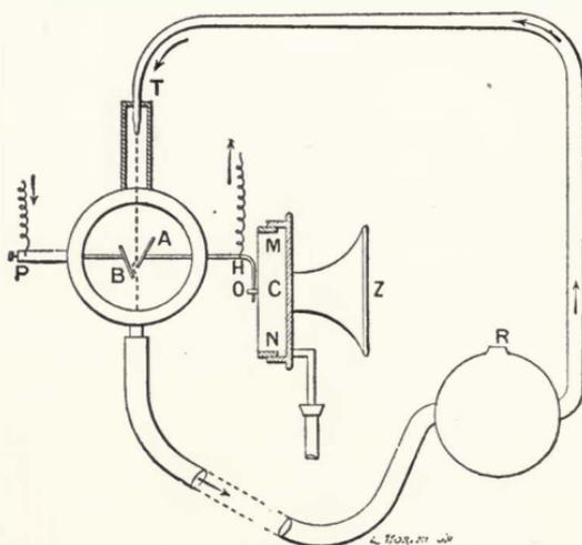
FIGURE 148—Vanni's liquid microphone.
