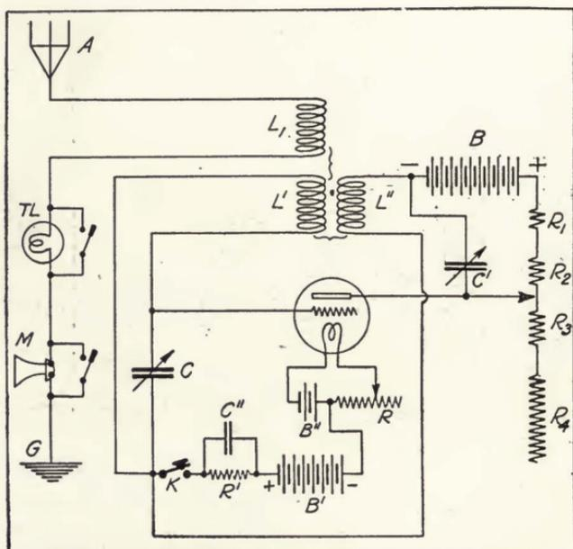
FIGURE 153—Marconi Company radiophone transmitter.
