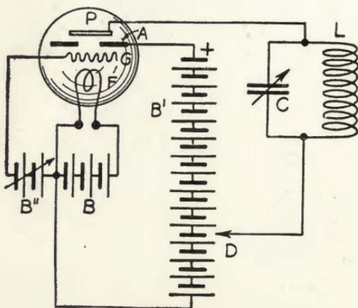
FIGURE 99—General Electric Company—Hull pliodynatron controlled oscillator.
