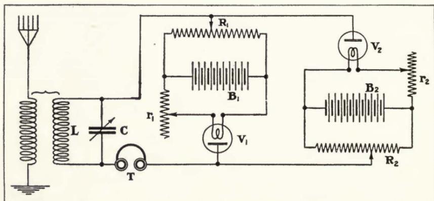
FIGURE 215—Marconi Company-Round balanced valve receiver.
