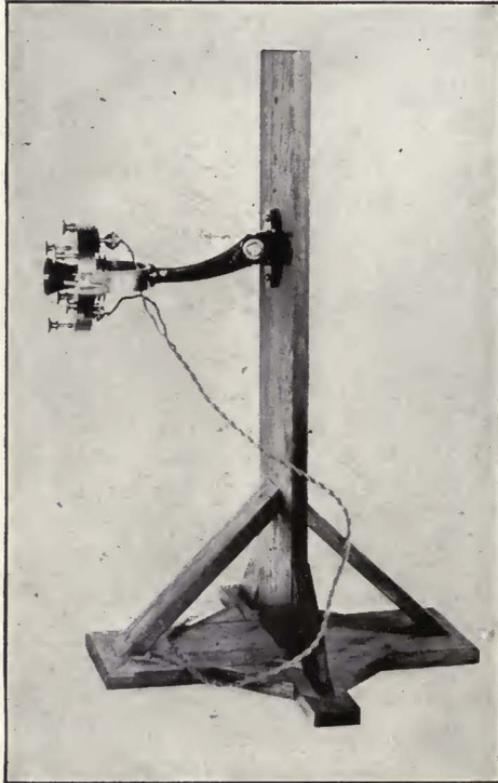
FIGURE 134—National Electric Signaling Company-Fessenden high current transmitter.
