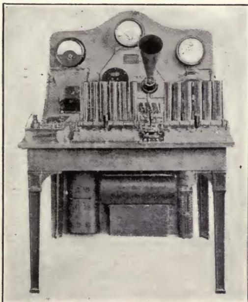
FIGURE 25—Telefunken Company series arc radiophone transmitter.
