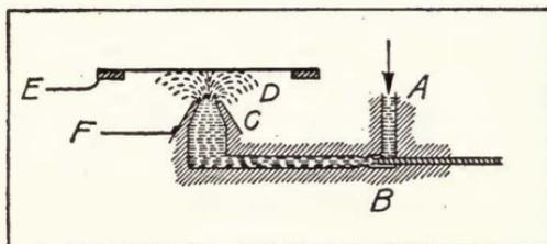
FIGURE 147—Essential parts of Chambers liquid microphone.
