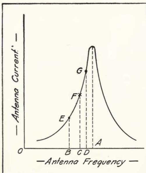
FIGURE 138—Detuning characteristic of radiophone transmitter.
