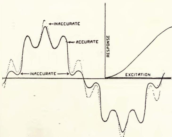
FIGURE 8—Complex non-linear distortion.
