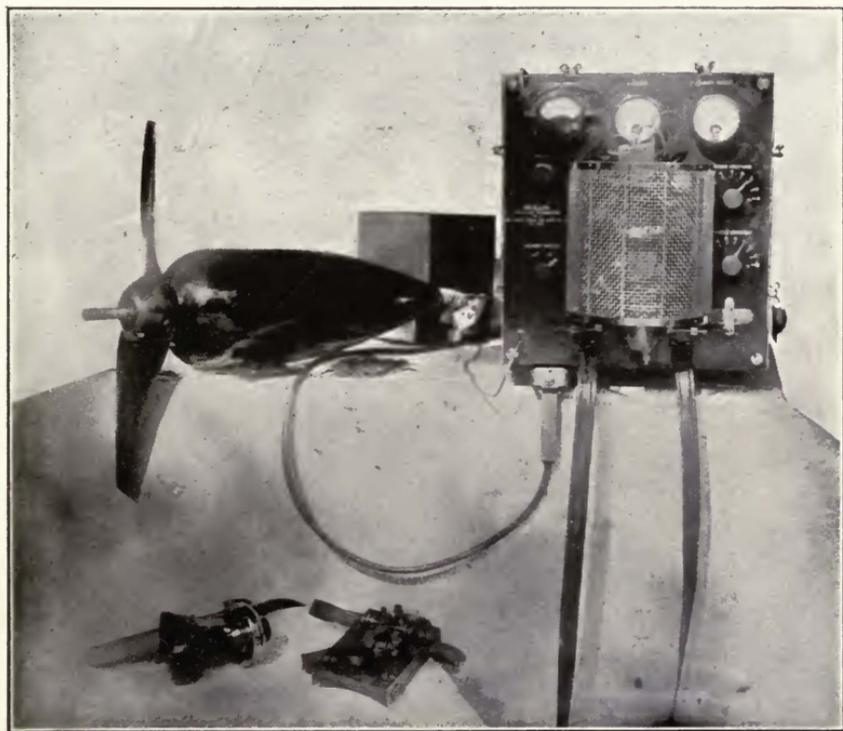
FIGURE 164—de Forest 0.25 K.W. oscillation radiophone and radio telegraph transmitter.
