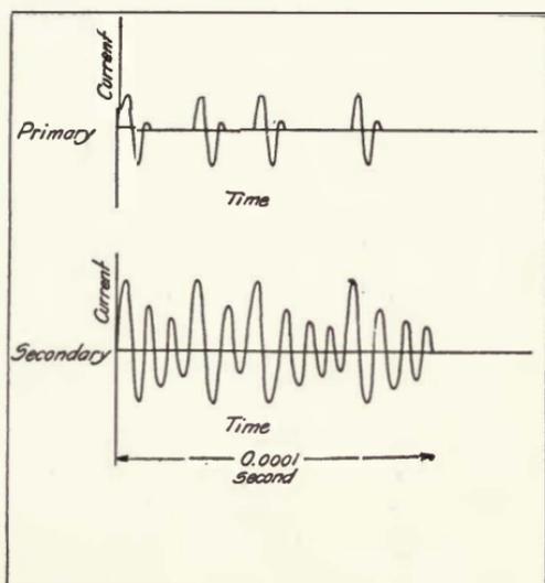
FIGURE 32—Irregular radio-frequent spark excitation of antenna.
