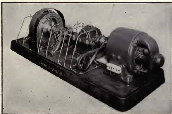
FIGURE 121—Intermediate type of Alexanderson alternator.
