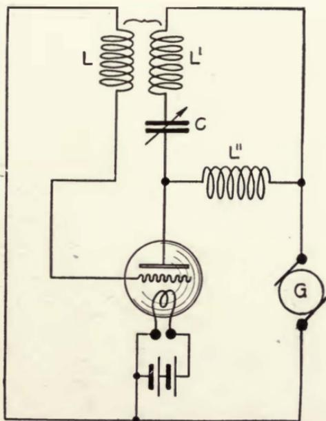
FIGURE S2—Arco-Meissner oscillating circuit.
