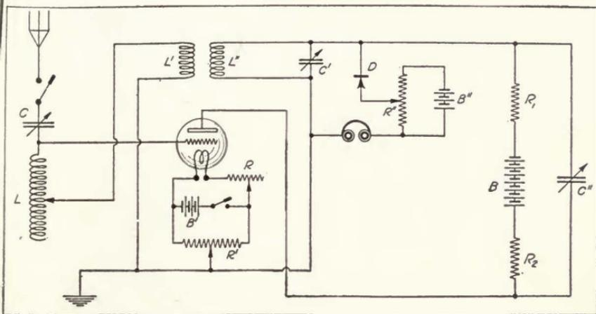
FIGURE 210—Marconi Company radiophone receiver.
