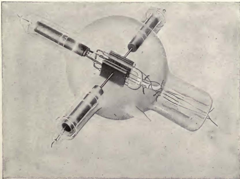
FIGURE 101—General Electric Company-Hull pliodynatron controlled oscillator.
