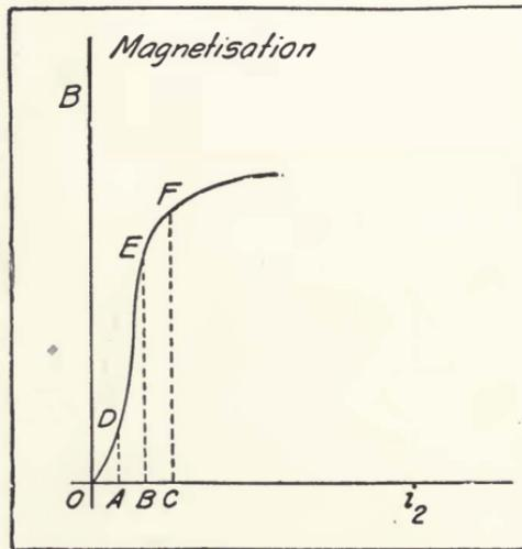
FIGURE 182—Iron magnetisation curve.
