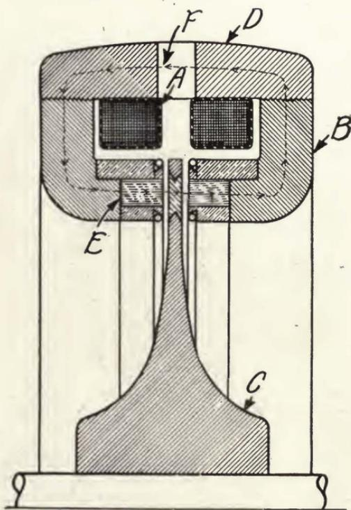
FIGURE 114—General Electric Company—Alexanderson alternator.
