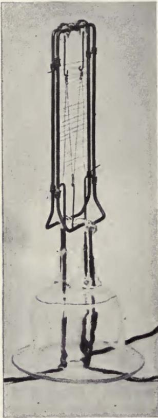
FIGURE 90—Filament and grid element of plotron.
