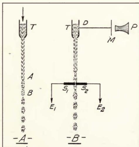
FIGURE 150—Essential parts of Majorana's liquid microphone.
