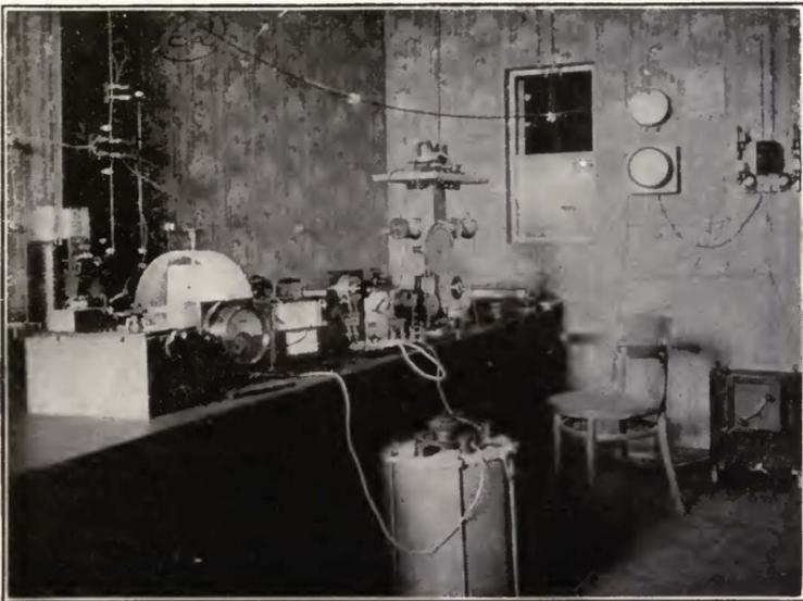
FIGURE 36—Ruhmer's radiophone transmitter.
