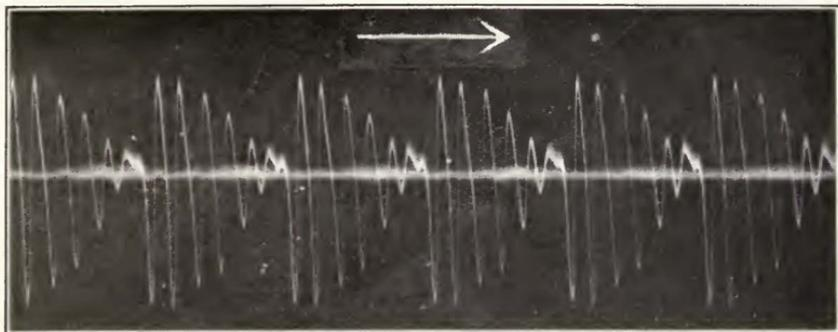
FIGURE 2—Oscillogram of vowel sounds "ah."
