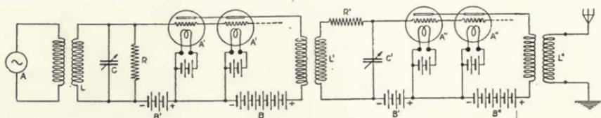
FIGURE 94—Western Electric Company-Heising oscillator—amplifier arrangement.
