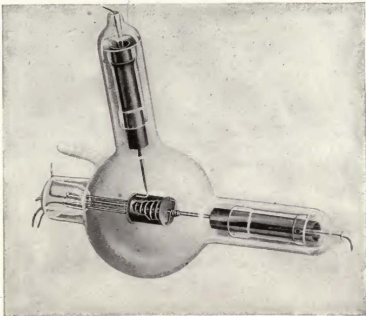
FIGURE 100—General Electric Company-Hull dynatron, showing internal structure.
