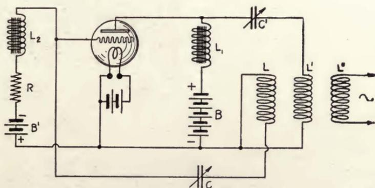
FIGURE 93—Western Electric Company—Colpitts oscillating circuit.
