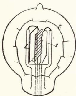
FIGURE 213 — Western Electric Company, Nicolson-and-Hull amplifier tube, 1914.
