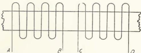
FIGURE 105—Portion of rotor or stator winding of Goldschmidt alternator (developed).
