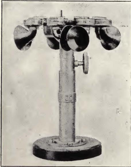
FIGURE 132—Ditcham multiple microphone transmitter.
