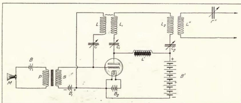
FIGURE 166—Western Electric Company-Colpitts modulation system, 1914.
