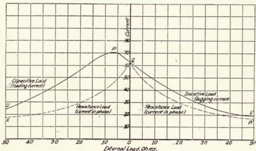
FIGURE 190—Load characteristics of 50 K. W., 50,000 cycle Alexanderson alternator.
