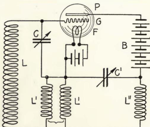
FIGURE 80—Plate circuit tuning in oscillating circuit.
