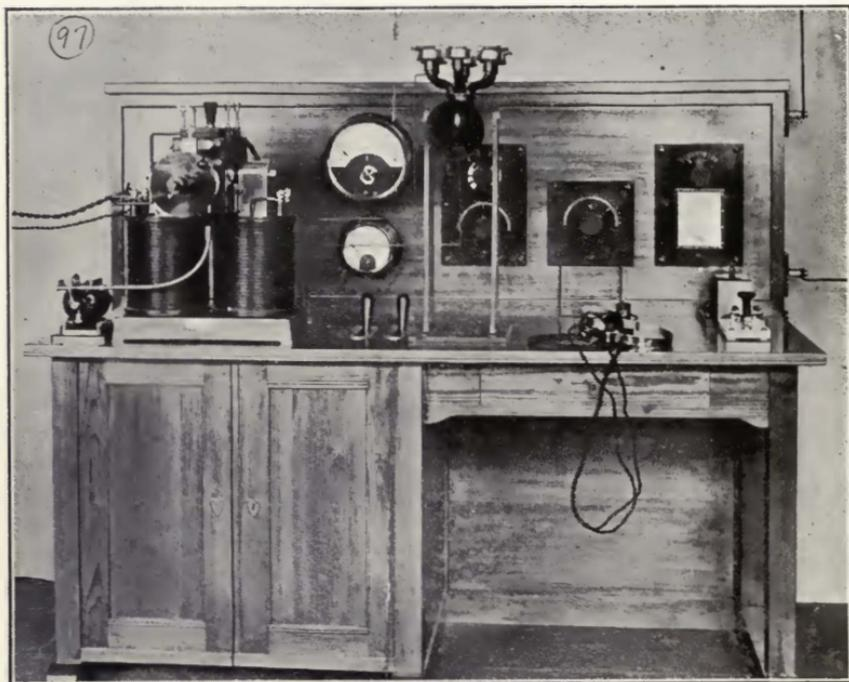
FIGURE 21—Berliner-Poulsen arc ship radiophone station.
