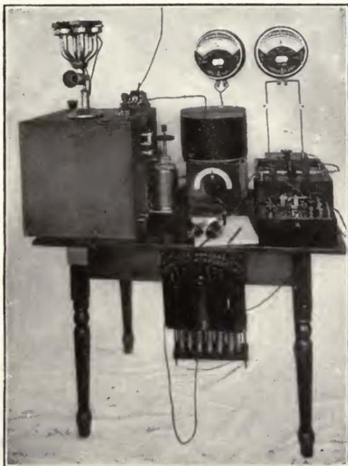
FIGURE 38—Dubilier radiophone transmitter and receiver.
