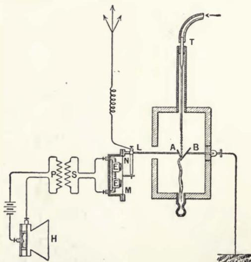
FIGURE 149—Vanni's liquid microphone relay.
