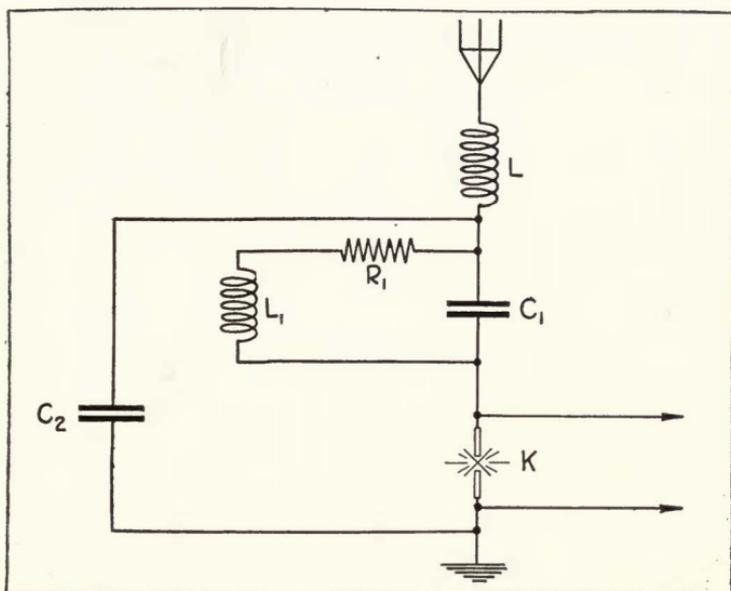
FIGURE 11—Fuller's method of increasing arc efficiency.
