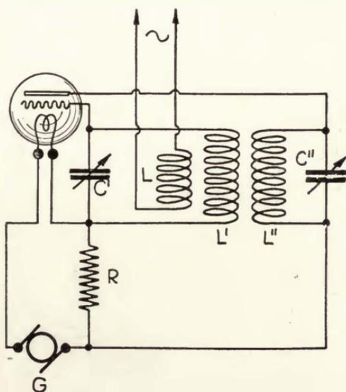
FIGURE 89—General Electric Company oscillating circuit.
