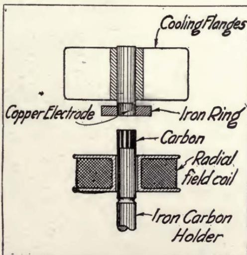
FIGURE 17—Construction of Lorenz-Poulsen arc for radio telephony.
