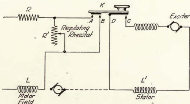
FIGURE 104—Goldschmidt alternator speed constancy system.
