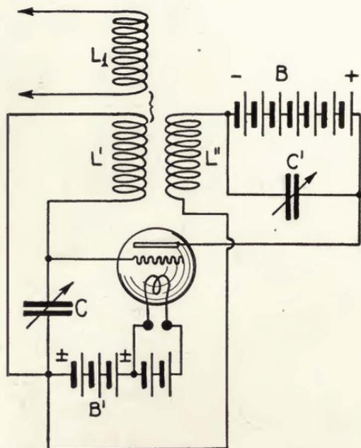
FIGURE 85—English Marconi Company oscillating circuit; modified form.
