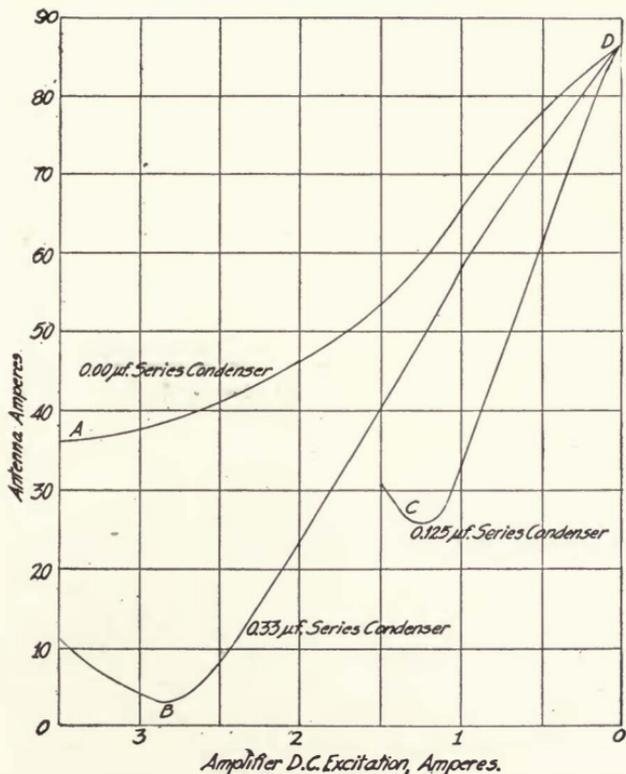
FIGURE 199—Control characteristics of magnetic amplifier.
