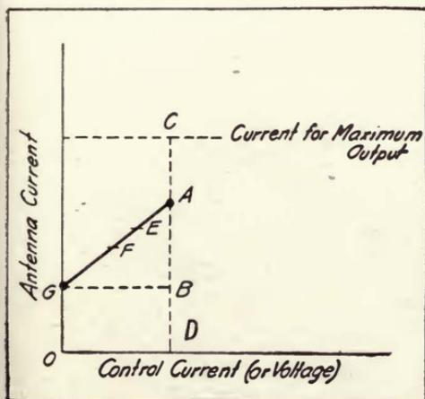
FIGURE 127—Incomplete linear modulation control curve.
