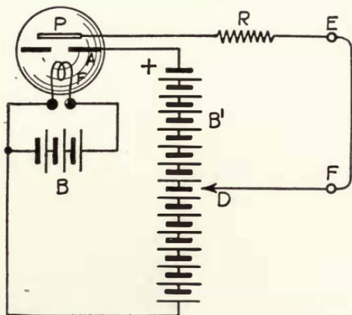
FIGURE 96—General Electric Company—Hull dynatron amplifier circuit.
