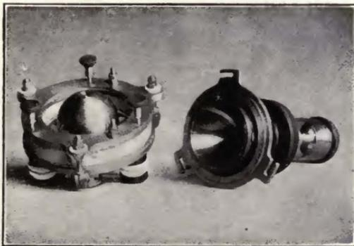
FIGURE 42—Interior of Scheller "multi-toné" gap.
