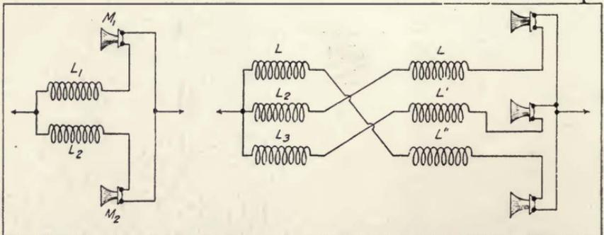
FIGURE 133—R. Goldschmidt's method of utilizing microphones in parallel.
