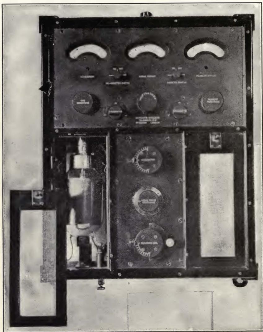
FIGURE 156—Marconi Company Sustained Wave Bulb Transmitter.
