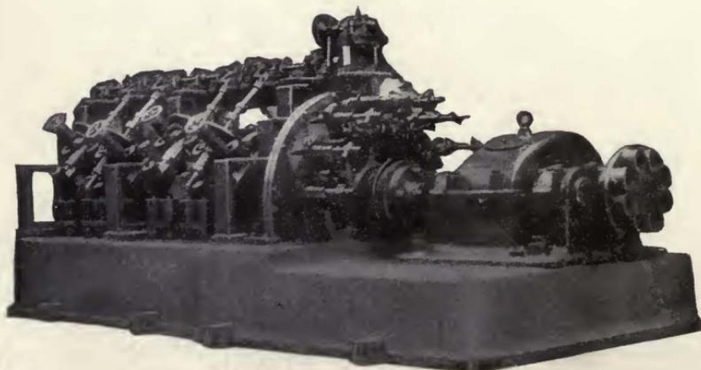
FIGURE 70—Marconi Company "Timed Spark" Discharger.
