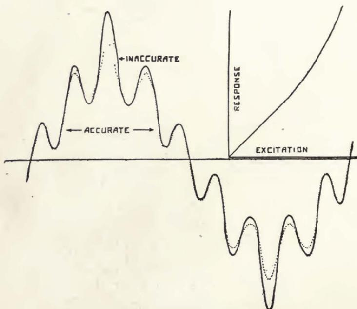
FIGURE 7—Non-linear distortion.
