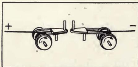
FIGURE 35—Ruhmer moving wire arc for radio telephony.
