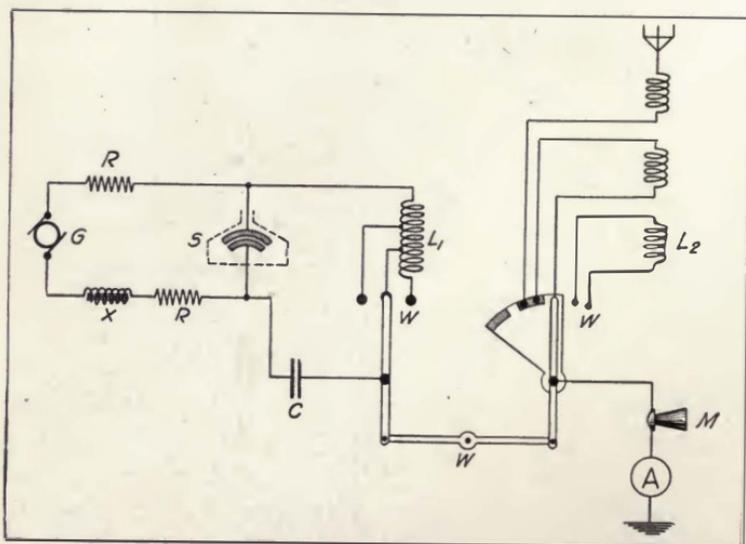
FIGURE 40—Lorenz Company radiophone transmitter.
