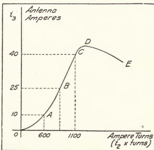
FIGURE 181—Control characteristic of resonant circuit containing iron core inductance of variable magnetisation.
