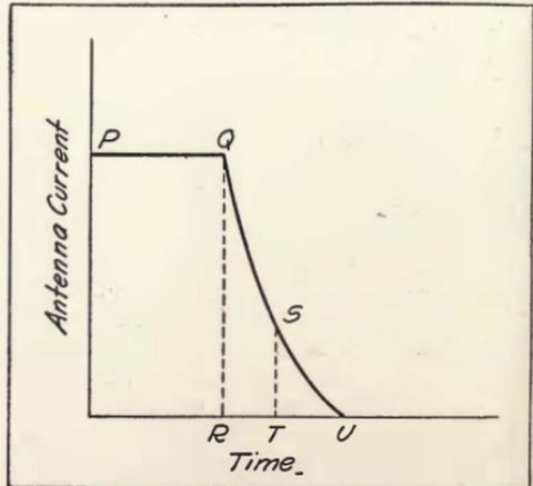
FIGURE 129—Dynamic characteristic of falling current for unstable control system.
