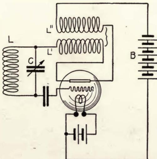
FIGURE 87—de Forest oscillating circuit, 1915.
