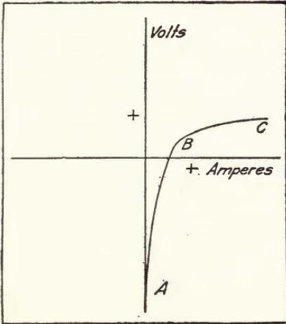
FIGURE 175—Grid potential-plate current characteristic of a pliodynatron.
