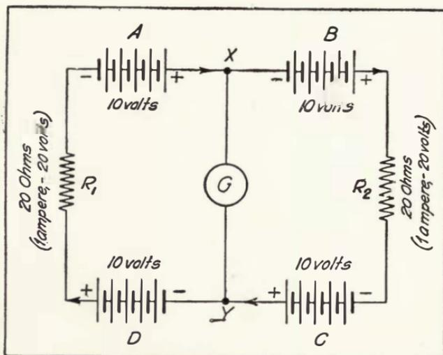
FIGURE 222—Principle of Fessenden duplex system.
