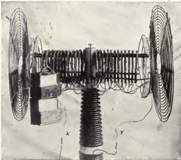
FIGURE 179—Step-up transformer for radio-frequency high voltage transformation.
