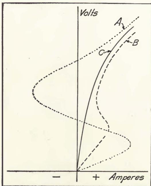
FIGURE 174—Characteristics of dynatron in various magnetic fields.
