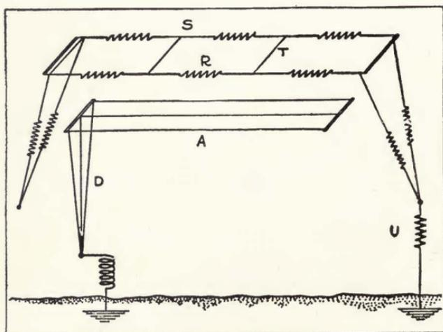
FIGURE 217—Dieckmann shielding cage for stray reduction.
