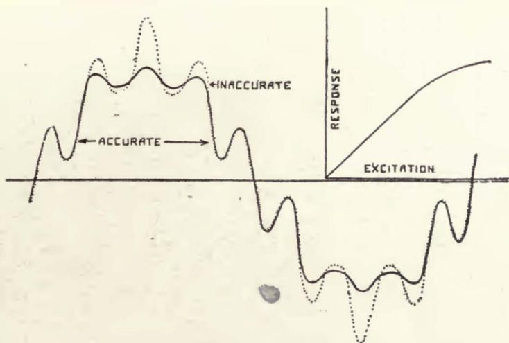
FIGURE 6—Non-linear distortion.
