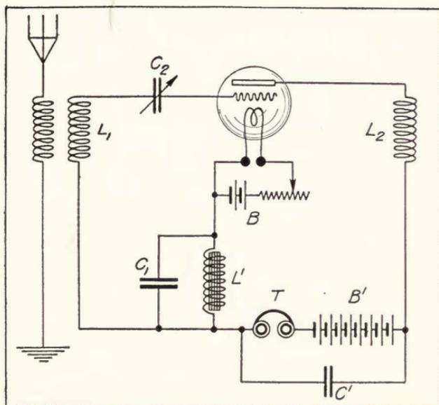
FIGURE 204—Armstrong regenerative circuit for radio frequency amplification.
