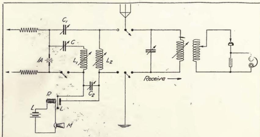
FIGURE 37—Dubilier radiophone transmitter and receiver.
