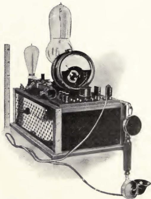
FIGURE 151—Telefunken Company-Meissner radiophone transmitter, 1913.
