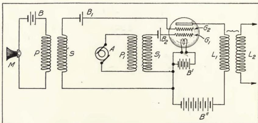
FIGURE 167—Western Electric Company—Heising modulation control system, 1915.
