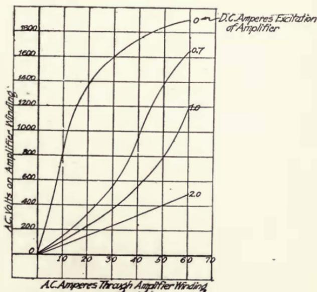
FIGURE 195—Characteristics of Alexanderson magnetic amplifier.
