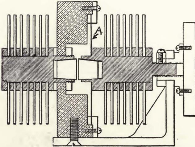
FIGURE 48—Cross section of Chaffee gap. Designed by Cutting and Washington.
