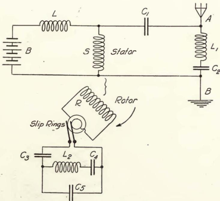
FIGURE 103—Winding of Goldschmidt alternator.
