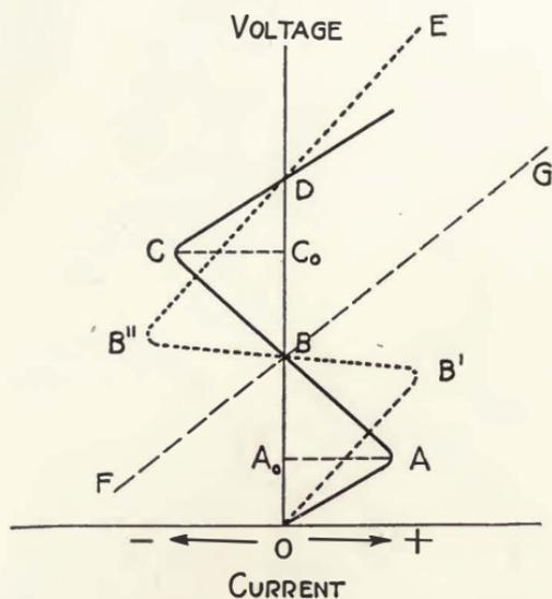
FIGURE 97—Dynatron voltage amplifier characteristics.
