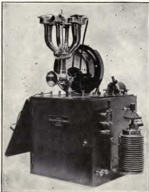
FIGURE 39—Complete Dubilier radiophone transmitter.
