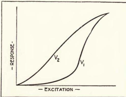
FIGURE 216—Valve characteristics with different auxiliary potentials.
