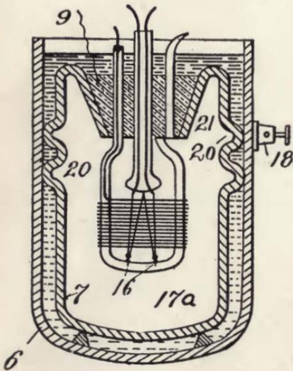
FIGURE 88—de Forest high-power tube construction.
