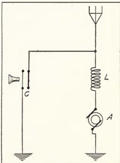
FIGURE 137—Fessenden condenser transmitter for radiophone work.
