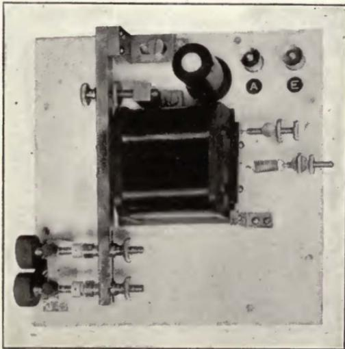
FIGURE 56—Equilibrator and spark gaps of T. Y. K. radiophone transmitter.
