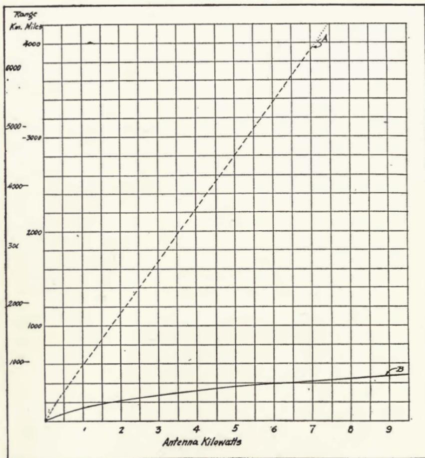
FIGURE 220—Relation between range and antenna power in radio telephony.
