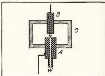
FIGURE 65—Diagrammatic representation of Moretti arc.
