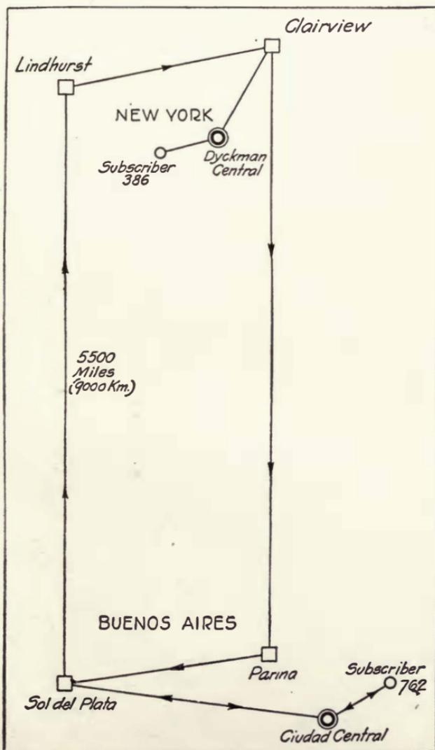
FIGURE 226—Typical duplex long distance radiophone system.
