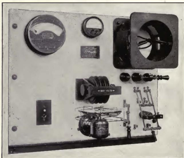
FIGURE 63—de Forest 2 k.w. radiophone panel transmitter.
