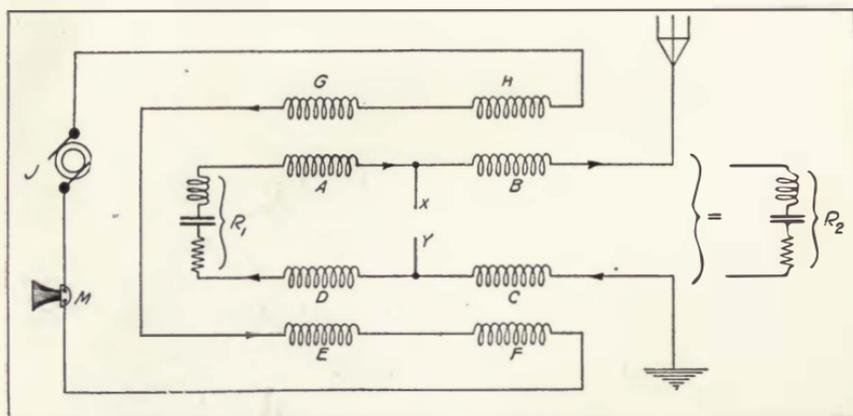
FIGURE 223—Fessenden duplex system for radio telephony.
