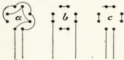
FIGURE 144—Connection arrangements of Egner-Holmström high current microphone.
