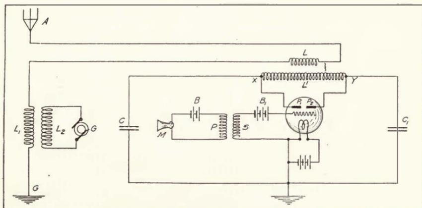
FIGURE 178—General Electric Company-Alexanderson alternator-plotron control radiophone transmitter.
