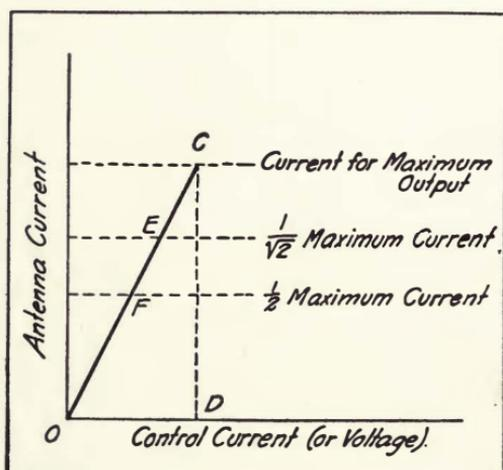
FIGURE 126—Complete linear modulation control curve.
