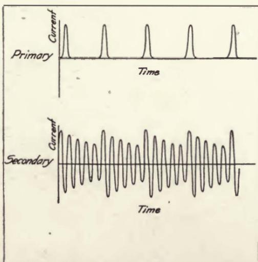
FIGURE 33—Regular radio-frequent impulse excitation of antenna.
