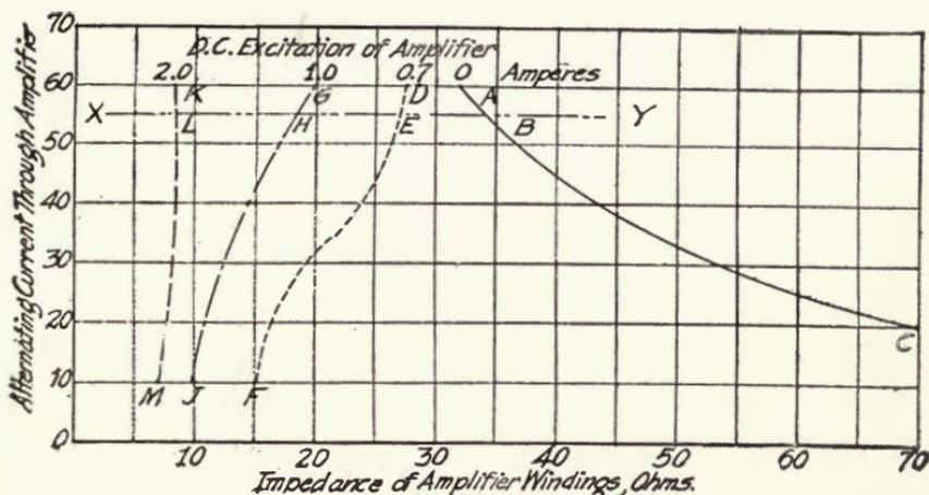
FIGURE 194—Characteristics of Alexanderson Magnetic Amplifier.
