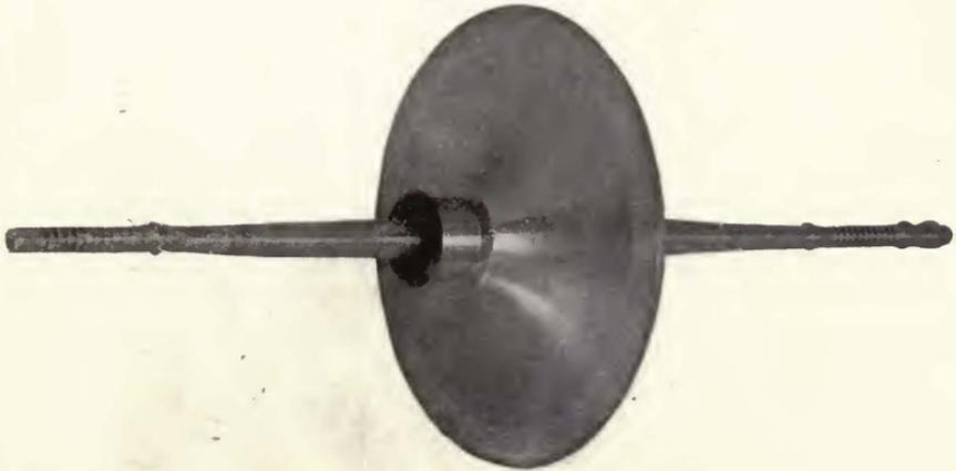
FIGURE 115—Rotor and shaft of 100,000 cycle Alexanderson alternator.
