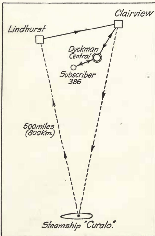
FIGURE 225—Typical ship-to-shore radiophone system.
