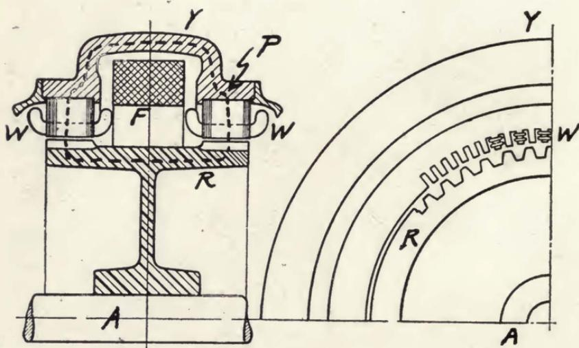
FIGURE 112—General arrangement of Telefunken radio frequency alternator.
