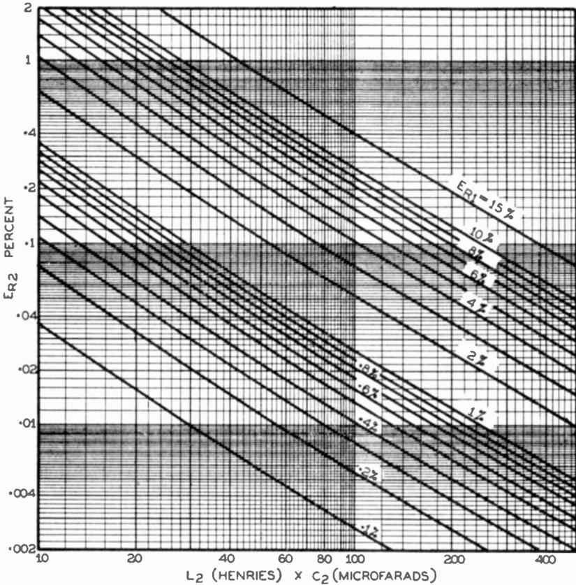
Figure 3: Calculation of the ripple voltage ( $E_{R_2}$ ) at the output of the second or any subsequent stage of a filter ( $L_2C_2$ ) when the ripple voltage ( $E_{R_1}$ ) at the input to this stage is known, for full wave rectification and a 50 c/s supply. These curves also apply in the case of a condenser input filter for the first choke and following condenser ( $L_1C_1$  in Fig. 4).
