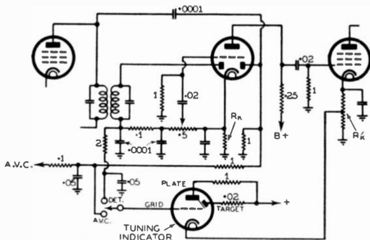
Figure 2: Circuit diagram illustrating the application of the Magic Eye Tuning Indicator. With the switch in the "Det." position the grid of the tuning indicator is connected through a 2 megohm resistor to the detector diode circuit. With the switch in the "A.V.C." position it is connected directly to the A.V.C. line. The cathode of the Tuning Indicator is returned to a suitable tapping point on the cathode bias resistor of the power valve.
