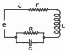
Figure 5. General case of series circuit.
