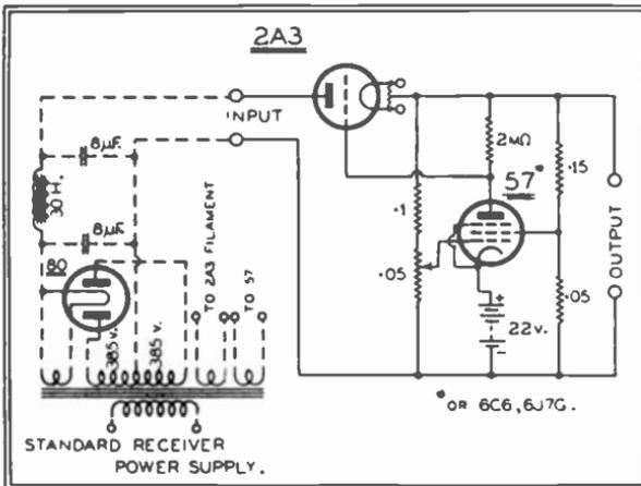
Figure 4. Typical valve type voltage regulator capable of delivering 180 v., D.C., at current drains up to 80 mA.
