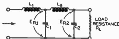
Figure 7: Two stage choke input filter.
