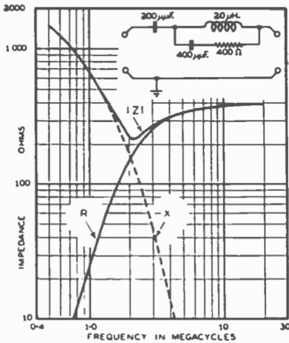
Figure 3 (Inset): Dummy antenna for all frequencies.
