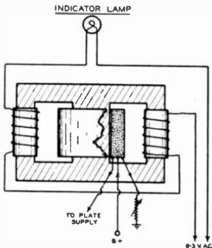
Figure 1. Saturated Reactor Tuning Indicator.
