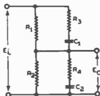
Figure 10. General filter circuit for constant voltage input. In the following treatment (Figures 11-18, inclusive), the values selected for the components as a basis for the frequency characteristics are:—
