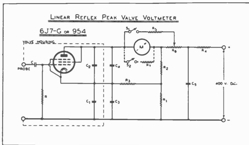
Figure 1. A.C. Operated Linear Reflex Peak Voltmeter.
