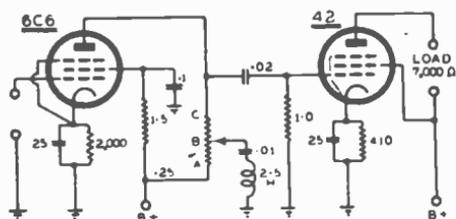
Figure 6 (above) and Figure 7 (right). Frequency characteristics shown in Fig. 7 correspond to positions A, B and C, respectively, of control in Fig. 6.
