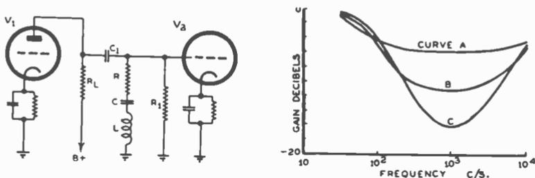
Figure 4 (left) and figure 5 (right). Frequency Characteristics in fig. 5 are obtained when  $V_1 =$  Pentode;  $R_L = 0.25$  megohm;  $L = 2.5$  henries;  $C = 0.01 \mu\text{F.}$ ;  $C_1 = 0.5 \mu\text{F.}$  or higher;  $R_1 = 1.0$  megohm; and  $R$  is (curve A), 0.2 megohm, (curve B), 75,000 ohms, (curve C), 35,000 ohms.
