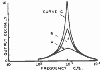
Figure 2 (left) and figure 3 (right). Frequency Characteristics in fig. 3 are obtained when V1 = Pentode; RL = 40,000 ohms; L = 2.5 henries; C = 0.01  $\mu$ F.; C1 = 0.02  $\mu$ F. or higher; R1 = 1.0 megohm; and R is (curve C), infinity, (curve B), 50,000 ohms, (curve A), 15,000 ohms.
