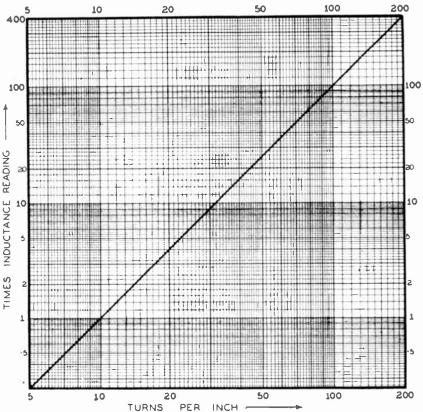
Figure 4: Winding pitch correction for Figure 3.
