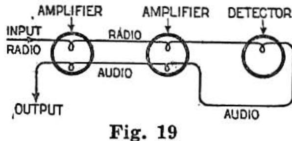
tion, proposed by Latour. Fig. 19 shows a reverse feed method for proportioning inputs and outputs. Fig. 20
