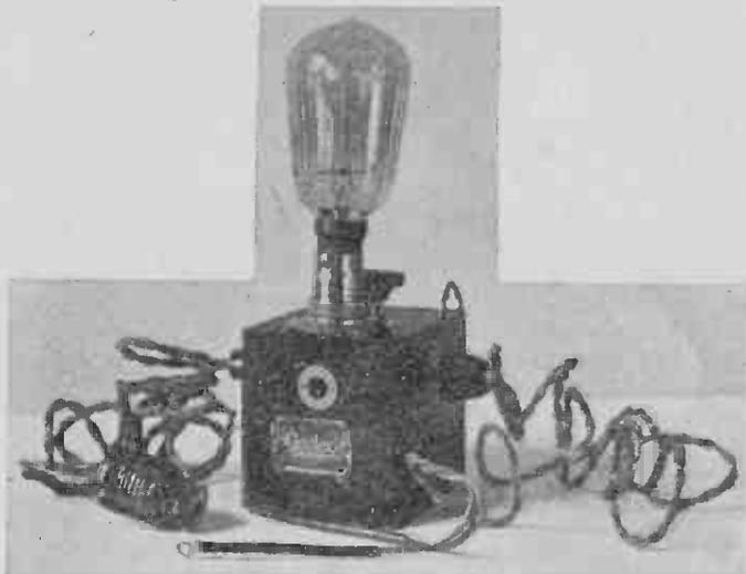
FIG. 29.—A single-lamp alternating charging half-cycle rectifier.
