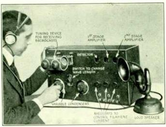
The higher priced set shown above will receive wave lengths from 200 to 20,000 meters. A special tuning device brings in broadcasts with unusual clearness.
