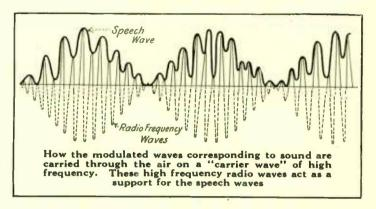
vary with the sound vibrations. Once the sounds have thus been converted into electric waves, some method must be adopted at the receiving stations to convert the electric waves back into sound waves, so that the man listening at the phones will have the words translated for him in the sender's own voice.
