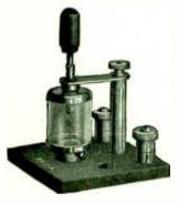
The sensitiveness of a crystal detector is seriously affected by dust, dirt and oil. The interesting detector at the left is made with a glass covering over the crystal, to protect it from these substances. The normal receiving range of such a set, properly installed and under favorable conditions, is about 10 to 25 miles
