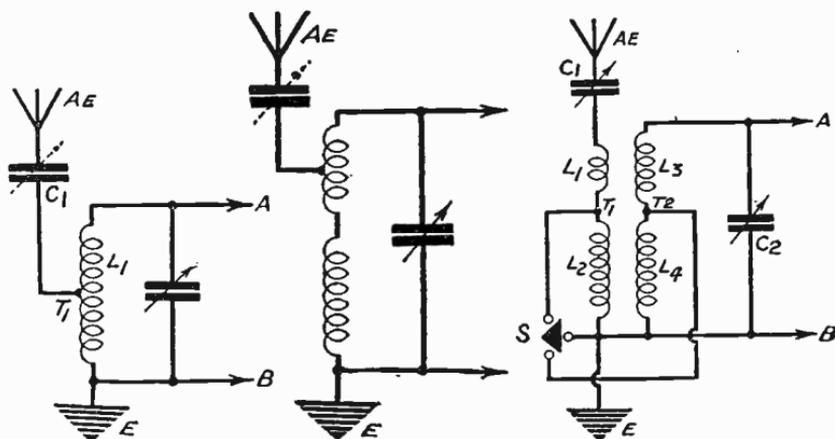
Fig. 55—Equivalent circuit when on medium waves
