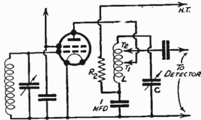
Fig. 265—Anode and grid tapings on anode coil
