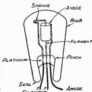
Fig. 85—Shows construction of simple diode valve
