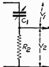
Fig. 385—L.F. potentials developed across  $C_1$  and  $R_2$
