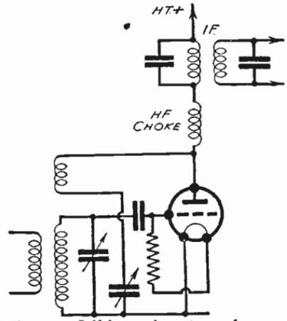
Fig. 479—Self-heterodyne type of super-heterodyne frequently used for short-wave reception
