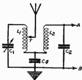
Fig. 68—Capacity-coupled band-pass with tapped aerial coil
