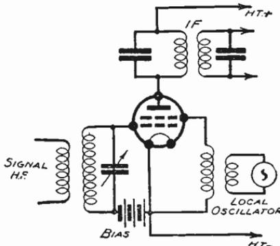
Fig. 478—Double-grid mixer valve circuit ; local oscillations are fed to a separate grid
