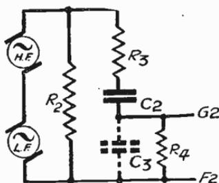
Fig. 220—The network of resistances and capacities equivalent to Fig. 219
