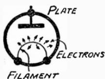
Fig. 77—Showing the introduction of a metal plate
