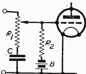
Fig. 356a—This arrangement causes less reduction of bass
