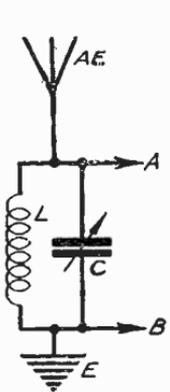
Fig. 32—Parallel aerial condenser tuning method
