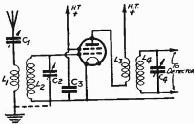
Fig. 266—Use of H.F. transformer with S.G. valve
