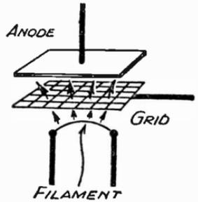
Fig. 89—Open mesh grid which controls electrons
