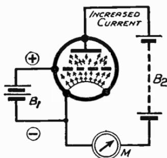
Fig. 95—Positive voltage on grid increases anode current
