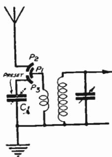
Fig. 329 — Differential condenser reduces mistuning
