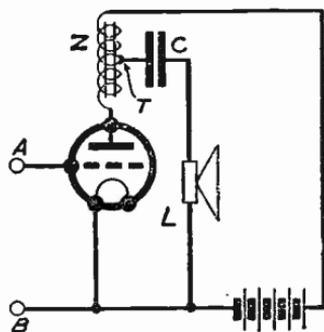
Fig. 137—Tapped output choke which gives step-down effect; speaker is parallel-fed
