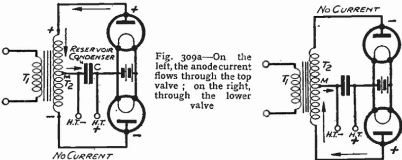
Fig. 309a—On the left, the anode current flows through the top valve; on the right, through the lower valve
