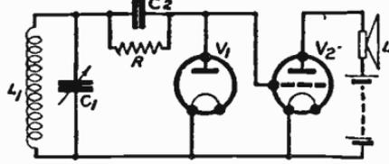
Fig. 182—The connection shown above results in H.F. on the grid of  $V_2$
