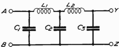
Fig. 400—An alternative series arrangement of L.F. filters
