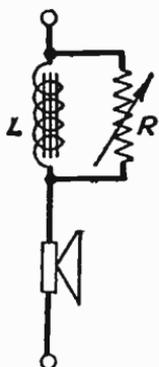
Fig. 370—Increasing  $R$  reduces treble
