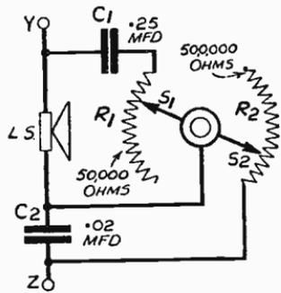
Fig. 373 — Double rheostat affects bass and treble simultaneously
