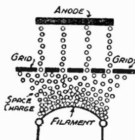
Fig. 99—A cloud of electrons form a space-charge
