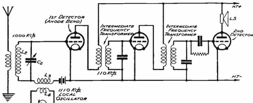
Fig. 470—A complete simple superheterodyne receiver showing the grid injector system and the use of intermediate-frequency circuits
