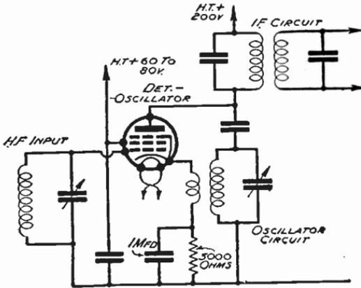
Fig. 497—A self-oscillating H.F. pentode is here used as first detector
