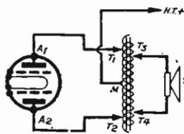
Fig. 288a—An output choke is often used in Class B
