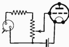
Fig. 404—Use of resistance in series with potentiometer
