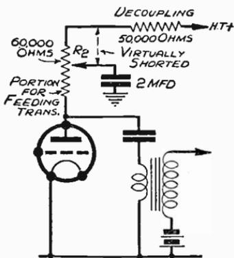
Fig. 348—Slider on  $R_2$  controls amount of amplification
