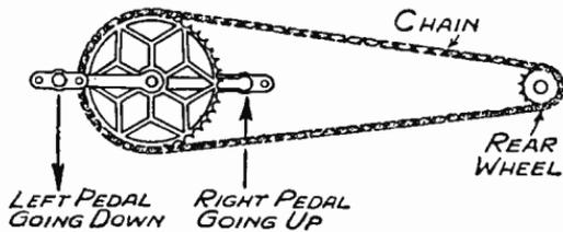
Fig. 284—A cyclist normally uses a “Q.P.P.” system, using pedals in turn
