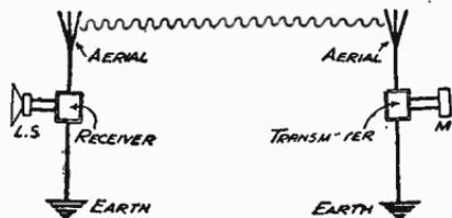
Fig. 8.—A skeleton representation of a transmitter sending to a receiving station
