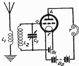
Fig. 193—An unusual valve detector circuit which relies on grid damping
