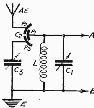
Fig. 49—Differential condenser to avoid altering tuning
