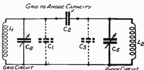
Fig. 292—Theoretical network showing valve capacities
