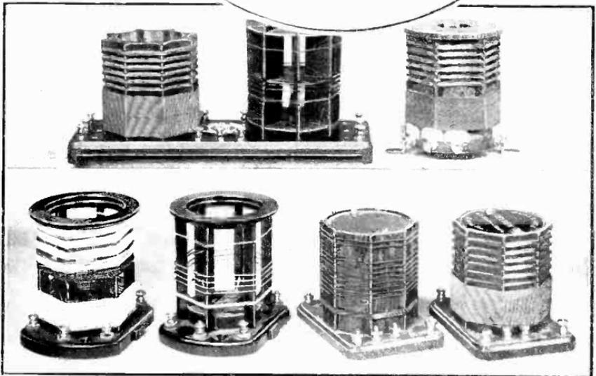
DIFFERENT TYPES OF AIR-CORE COILS
