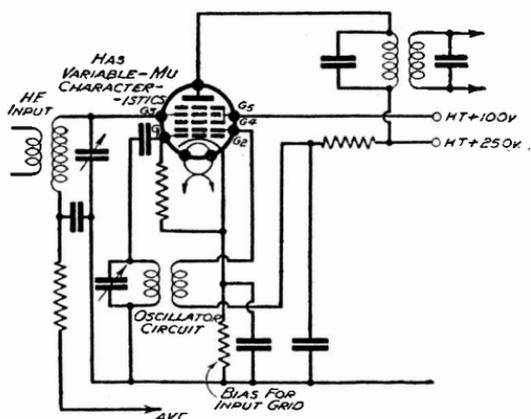
Fig. 500—The Pentagrid valve in which the "grids" nearest the cathode constitute the grid and anode of an oscillator
