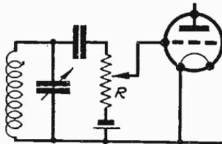
Fig. 333—Use of stopping condenser to prevent shorting bias
