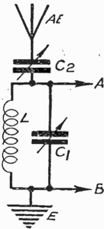
Fig. 34—Use of a small series condenser
