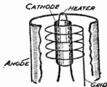
Fig. 442—Arrangement of an indirectly-heated valve
