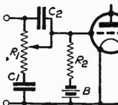
Fig. 356b—A greater proportion of treble and bass are maintained
