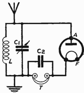
Fig. 84—Diode in use as a wireless detector
