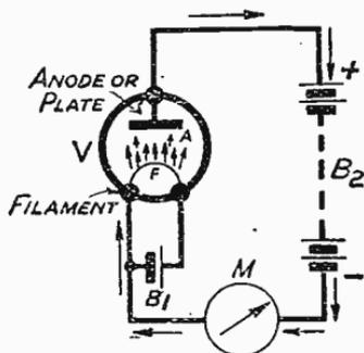
Fig. 78—Anode current is produced by applying a positive voltage to anode
