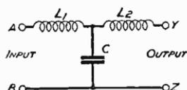
Fig. 397—A symmetrical low-frequency filter
