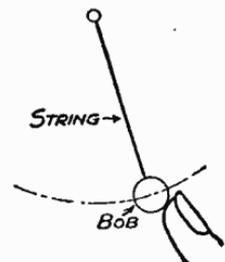
Fig. 154—Keeping a pendulum swinging by correctly-timed taps
