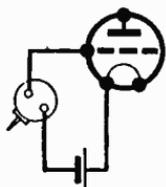
Fig. 402 — Simplest pick-up circuit
