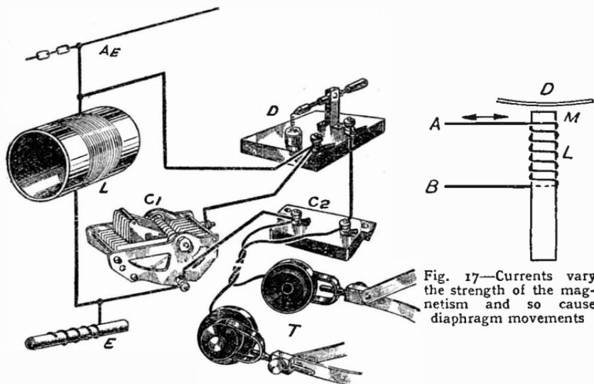
Fig. 16 (b)—Pictorial representation of the simple receiver shown in Fig. 16
