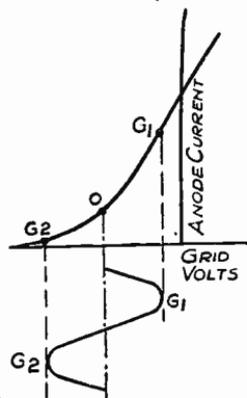
Fig. 282—Q.P.P. circuits operate valves at bottom bend
