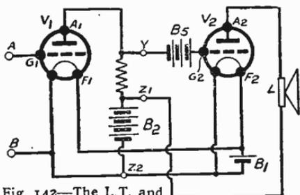
Fig. 142—The L.T. and H.T. batteries are now common; a grid battery remains necessary
