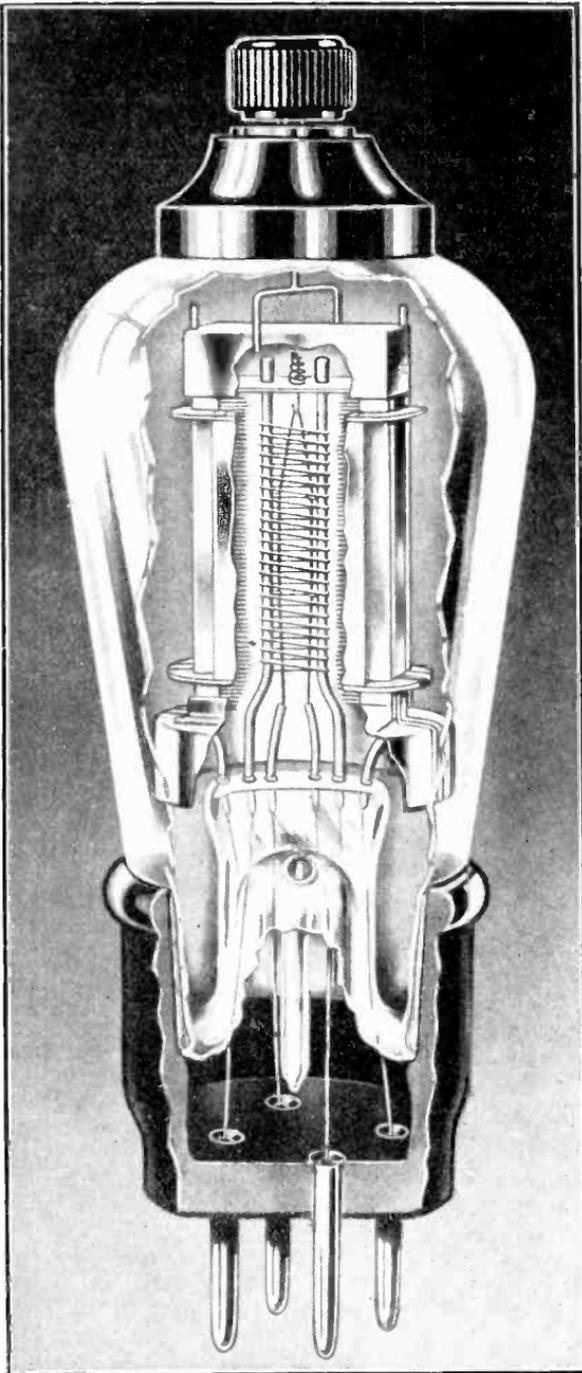
MODERN COSSOR SCREEN-GRID VALVE CONSTRUCTION
