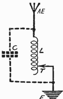
Fig. 24—Dotted lines show the equivalent of the aerial capacity
