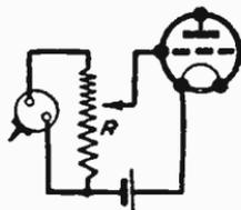
Fig. 355—Graded potentiometer for pick-up volume control
