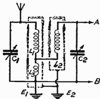
Fig. 66a—Auto-coupling using inductance common to both circuits
