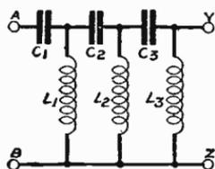
Fig. 244—This combination of condensers and inductances passes on the H.F.
