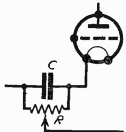
Fig. 344a—Tapping the L.F. output from a detector
