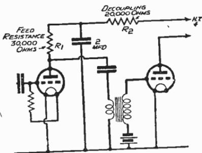
Fig. 256—How a resistance-fed transformer may be decoupled
