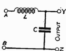
Fig. 395—To explain the cut-off filter
