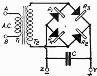
Fig. 318—Metal rectifiers arranged in bridge formation
