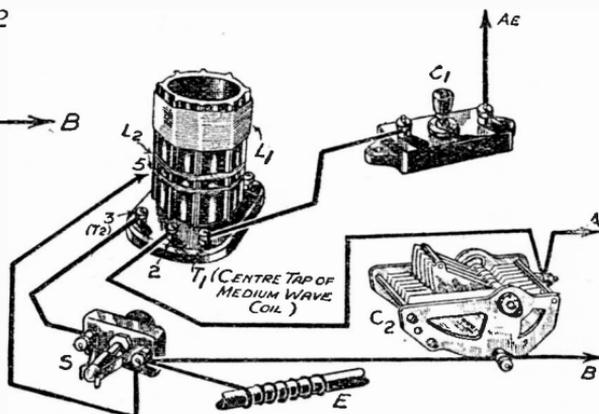
tapping on the coil  $L_1$  and by the use of the variable condenser  $C_1$ , which may be either a preset variable (i.e., semi-variable) or a solid dielectric variable condenser, if it is not desired to use an ordinary air dielectric variable condenser.
