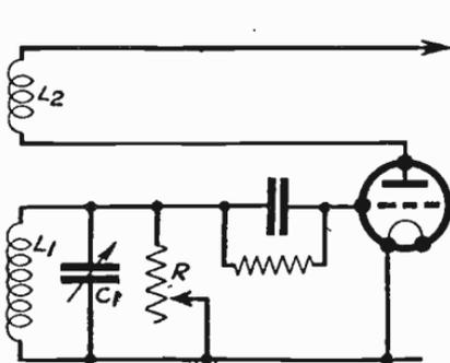
Fig. 169—A parallel variable resistance varies damping of circuit, thus altering reaction
