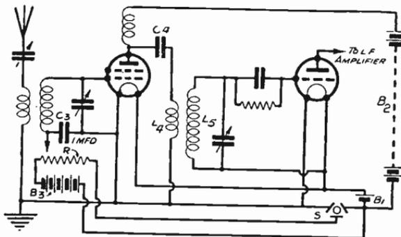
Fig. 269—A three-point switch cuts out potentiometer battery as well as L.T.
