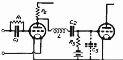
Fig. 217—Sometimes an H.F. choke by itself is used as a stopper
