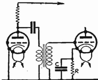
Fig. 449—Showing typical use of a self-bias resistance
