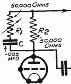
Fig. 381—Tone-controlling a resistance amplifier
