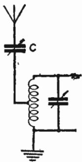
Fig. 328 — Combined tapping and series condenser
