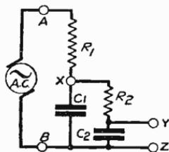
Fig. 240—Two resistance-capacity filters
