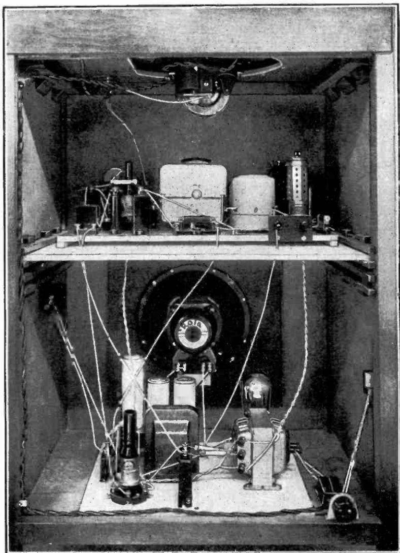
THE COMPLETE A.C. MAINS RECEIVER ARRANGED AS A
