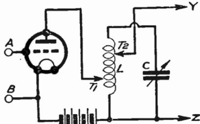
Fig. 114—Tapping the grid circuit results in less grid circuit damping
