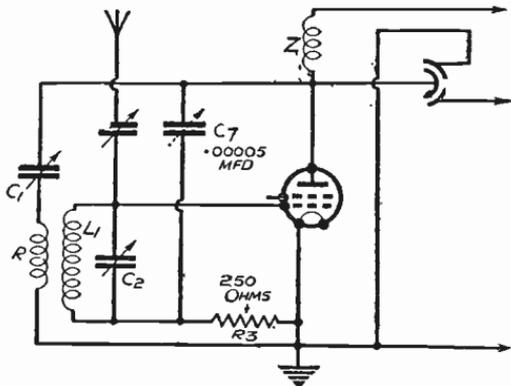
Fig. 305—Showing use of a phase reverser in aerial reaction circuit
