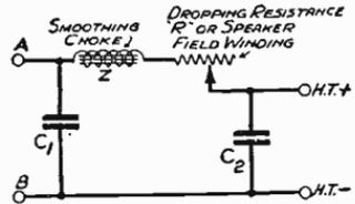
Fig. 310—Use of a resistance for voltage dropping
