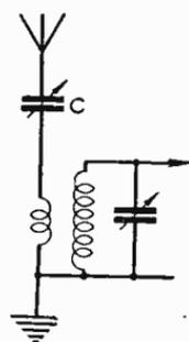
Fig. 327—This arrangement produces little effect on tuning
