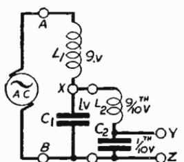
Fig. 239—Use of two filters in series
