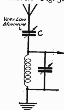
Fig. 324—Series condenser controls volume
