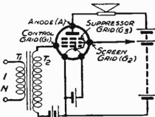
Fig. 272—Suppressor gr.d prevents negative resistance
