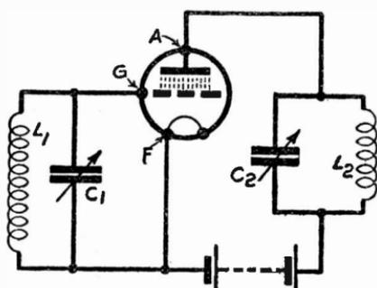
Fig. 291—Capacity coupling inside triode promotes self-oscillation
