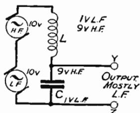
Fig. 210—H.F. is filtered out by this arrangement
