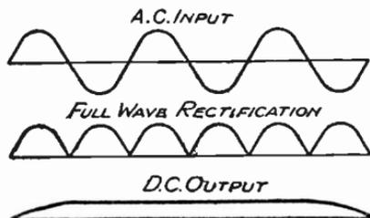
Fig. 189—Graphical representation of full-wave rectification
