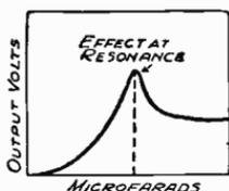
Fig. 388—Resonance increases the bass response
