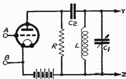
Fig. 115—A parallel-resonant tuned anode circuit, using resistance
