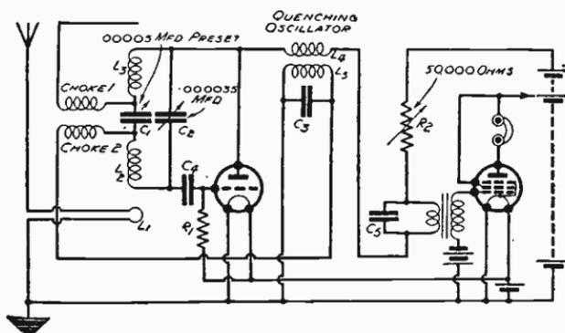
Fig 504.—An ultra-short-wave receiving circuit of the super-regenerative type. The reaction valve acts as its own quencher and wavelengths of 5 metres may be received
