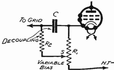
Fig. 448—A slider on the self-bias resistance varies grid voltage
