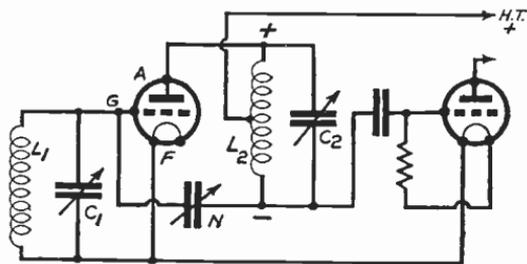
Fig. 295—Tapped anode coil enables valve capacity to be neutralised
