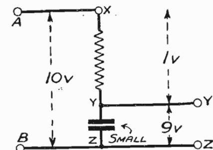
Fig. 207—A resistance and small condenser will give a greater output of low notes
