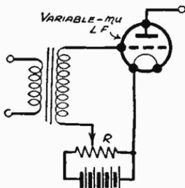
Fig. 359—A variable-mu L.F. valve is shown
