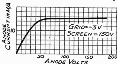
Fig. 273—Characteristic curve of typical pentode valve
