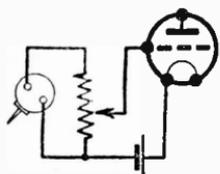
Fig. 403—Pick-up with volume control and bias
