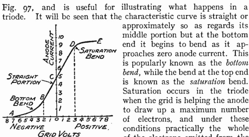
Fig. 97—Characteristic curve of a three-electrode valve
