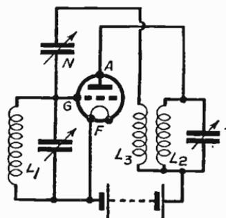
Fig. 293—Use of neutralising winding and condenser
