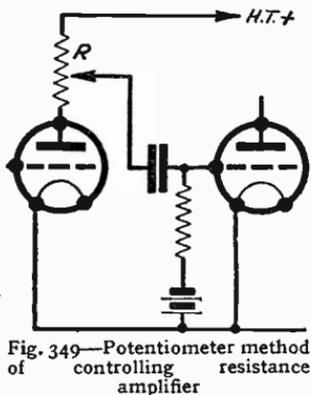
Fig. 349—Potentiometer method of controlling resistance amplifier
