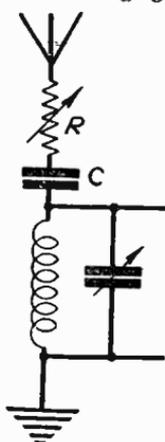
Fig. 326—A fixed condenser is sometimes inserted
