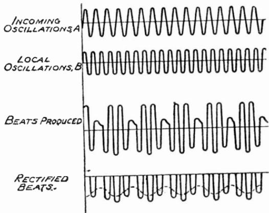
Fig. 466—Graphical representation of the effect of two sets of oscillations of differing frequency
