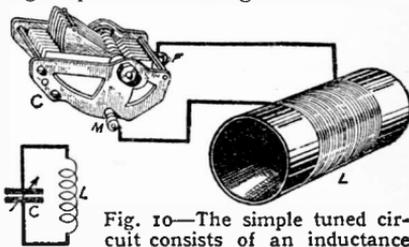
Fig. 10—The simple tuned circuit consists of an inductance and variable condenser
