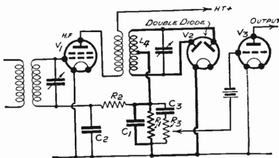
Fig. 425.—A double-diode detector is shown in use for A.V.C. purposes
