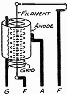
Fig. 90—Construction of cylindrical type of valve.
