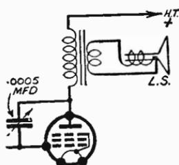
Fig. 386—Use of reverse reaction to reduce "top"
