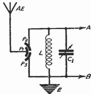
Fig. 48—Use of differential condenser for feeding circuit
