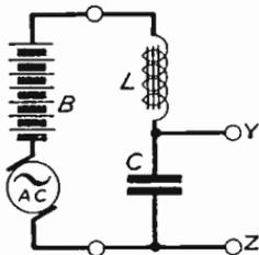
Fig. 242—Use of iron-core choke filter
