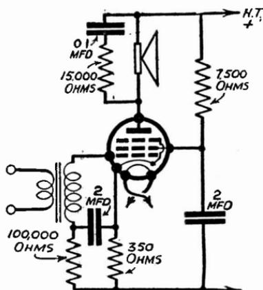
Fig. 277—Typical circuit for using mains pentode; note grid decoupling arrangement for smoothing out the grid-bias potential; a resistance of 100,000 ohms and a 2-mfd. condenser is arranged as shown.
