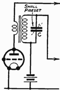
Fig. 376—Reducing treble by condenser across secondary
