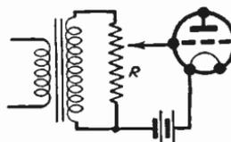
Fig. 353—Commonly used potentiometer arrangement across transformer secondary
