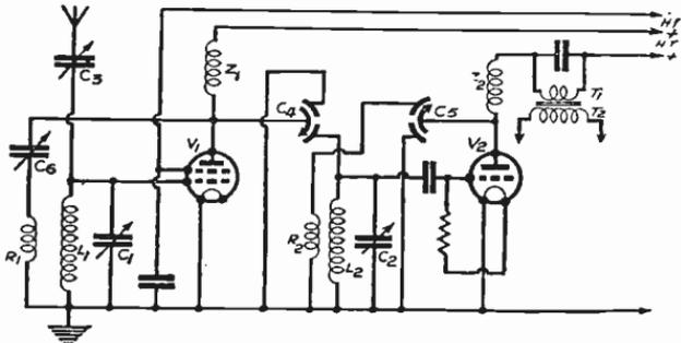
Fig. 304—A double-reaction circuit in which each anode circuit provides reaction
