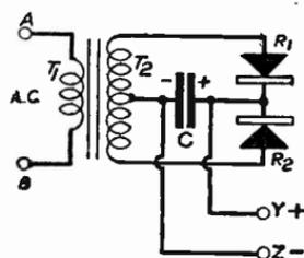
Fig. 317—A full-wave metal rectifier system
