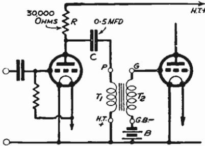
Fig. 252—Simple parallel-fed transformer using an anode resistance
