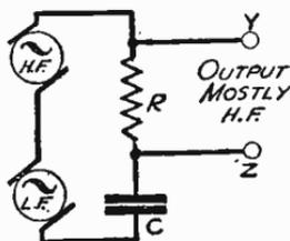
Fig. 213—The same circuit with H.F. output
