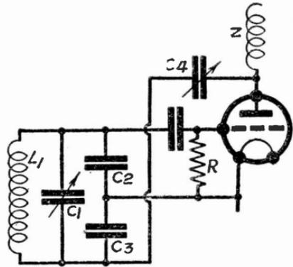
Fig. 167—Instead of a tapping on the coil itself, two condensers are used
