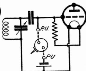
Fig. 412—Suitable for occasional use of pick-up
