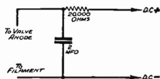
Fig. 249—Another method which however, causes a drop in the H.T. voltage
