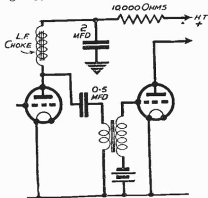
Fig. 257—Method of decoupling a choke-fed L.F. transformer
