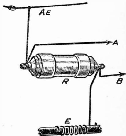
Fig. 20—A pictorial equivalent of the aperiodic aerial circuit. The system is rarely used
