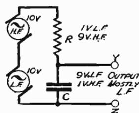
Fig. 212—Connections to give an L.F. output
