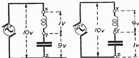
Fig. 208—The identical circuit may give a large or small condenser voltage according to frequency
