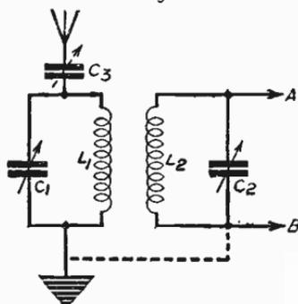
Fig. 62—Loose-coupled input tuner for selectivity
