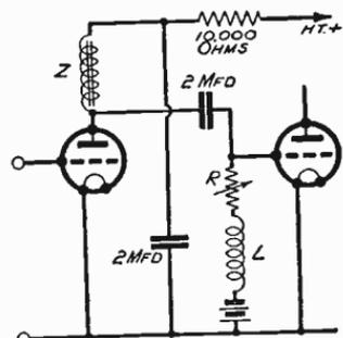
Fig. 394—Tone-corrector circuits as applied to grid circuit
