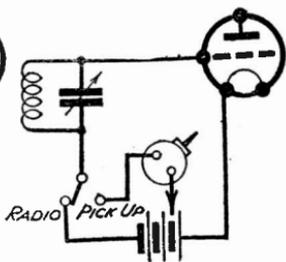
Fig. 411—A much better arrangement with separate bias
