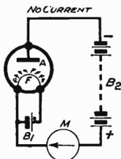
Fig. 79—No anode current is produced if anode is negative
