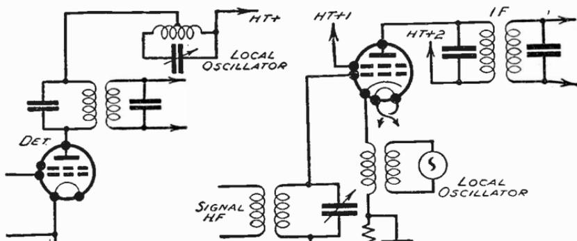
Fig. 476—The applied local oscillator voltages may be reduced by tapping the oscillator circuit
