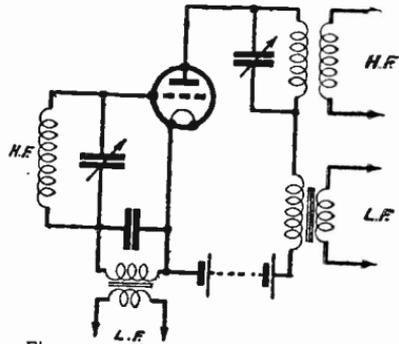
Fig. 299—Simple reflex circuit which amplifies H.F. and L.F.
