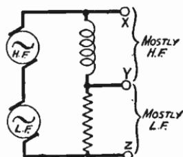
Fig. 226—Theoretical arrangement of inductance-resistance filter
