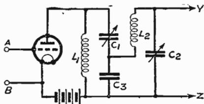
Fig. 127—A large condenser common to both circuits couples the two circuits
