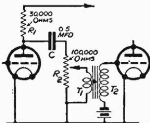
Fig. 356—A special volume control on L.F. circuit
