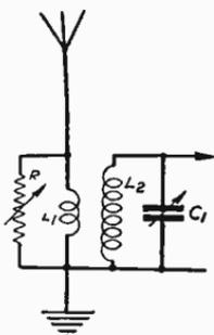
Fig. 334—Variable resistance by-passes H.F. currents
