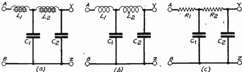
Fig. 243—Three forms of filter which pass on the low-frequencies and tend to "short-circuit" the higher frequencies
