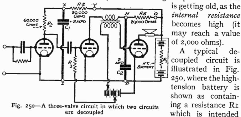
Fig. 250—A three-valve circuit in which two circuits are decoupled
