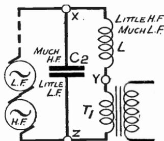
Fig. 232—Theoretical network corresponding to the Fig. 231 arrangement
