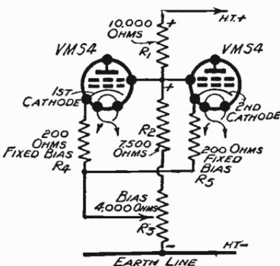
Fig. 459—Resistance network for two variable-mu S.G. valves
