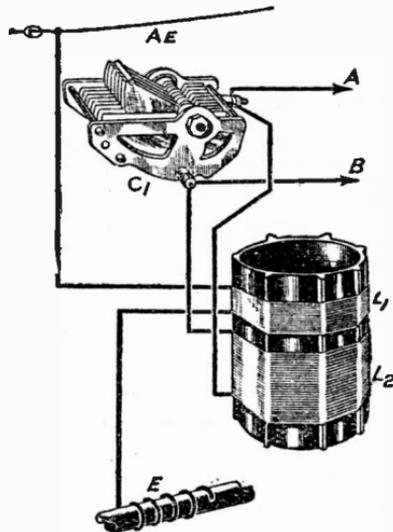
Fig. 39—Pictorial form of the circuit of Fig. 38
