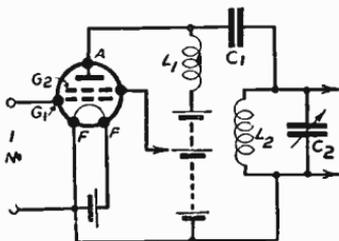
Fig. 259—Simple screen-grid H.F. amplifier
