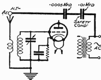
Fig. 458—A condenser (or two for safety) between mains and aerial terminals
