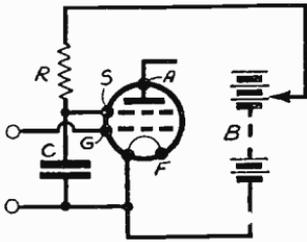
Fig. 247—Decoupling the screen of an S.G. valve
