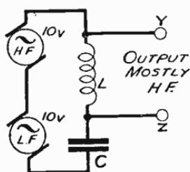
Fig. 211—This particular connection gives an H.F. output
