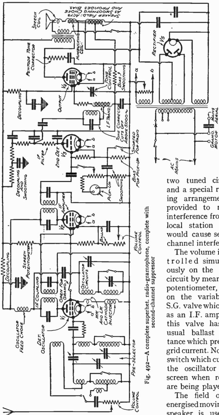
Fig. 492—A complete superhet. radio-gramophone, complete with second-channel suppressor
