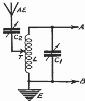
Fig. 46—Combined tapped coil and series feed condenser
