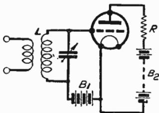
Fig. 431—A triode may be used as a limiter
