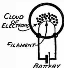
Fig. 76—Filament heated to incandescence and emitting electrons
