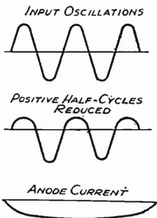
Fig. 195—Graphical representation of grid damping detection
