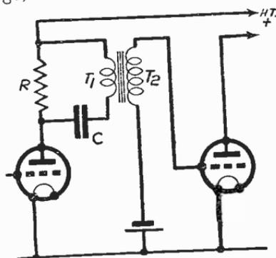
Fig. 258—This connection reduces interaction and hum
