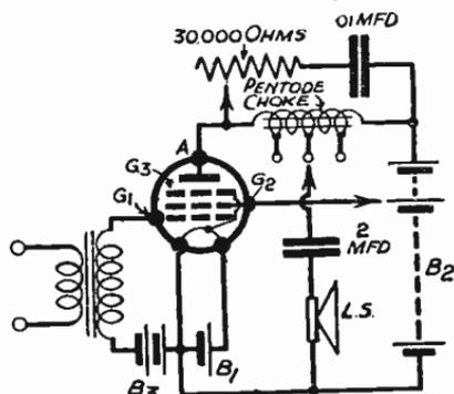
Fig. 275—Tone-corrector circuit applied to output choke
