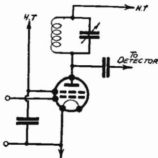
Fig. 263—Plain tuned anode coupling can be applied to S.G. valves
