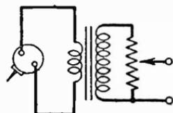
Fig. 422—An L.F. transformer is sometimes used to connect the pick-up to the amplifying valve; the potentiometer may be connected across its secondary
