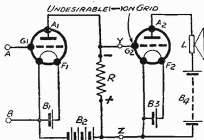
Fig. 139—Theoretical resistance-coupled L.F. amplifier
