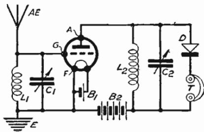
Fig. 110—A complete wireless receiver employing tuned anode H.F. coupling and a crystal detector
