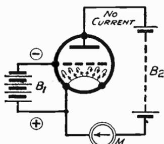
Fig. 94—Anode current cut off by large negative voltage
