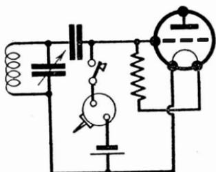
Fig. 413—Simple arrangement for switching-in pick-up
