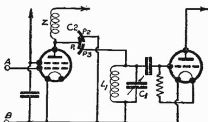
Fig. 123—Screen-grid valve, followed by differential anode coupling
