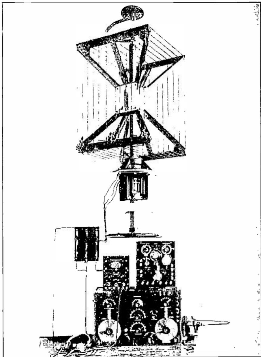
UNITED STATES NAVY RADIO COMPASS, THE DIRECTIONAL EFFECT BEING DUE TO THE LOOP-AERIAL
