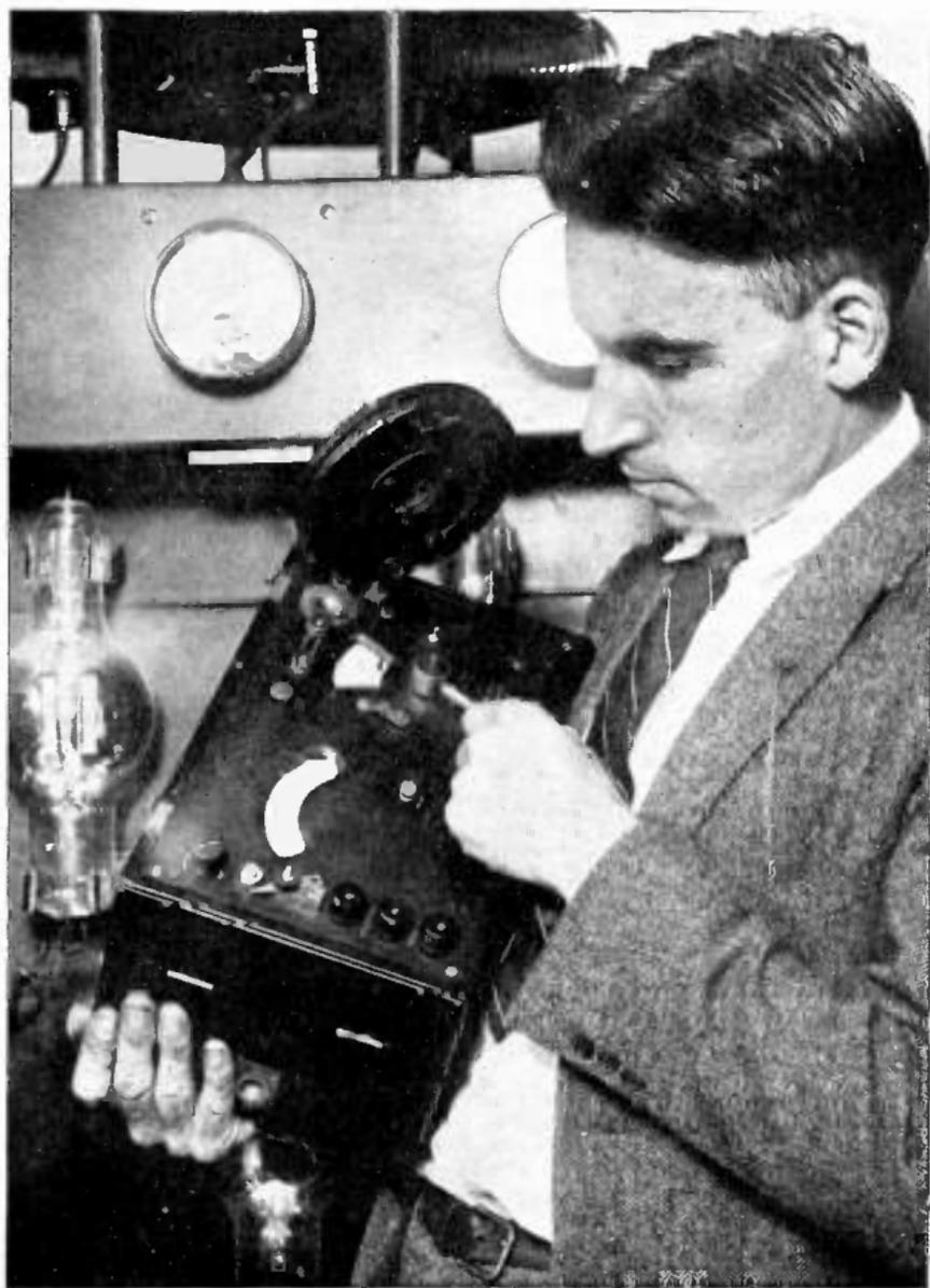
ADJUSTING WAVE LENGTHS WITH A WAVE METER
