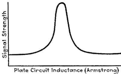
FIG. 181.—Variation of signal strength with plate-circuit inductance for the regenerative triode of Fig. 180. (Armstrong.)
