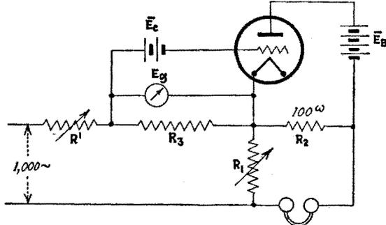
FIG. 194.—Circuits for the second method of obtaining experimentally the regeneration characteristics of a triode.
