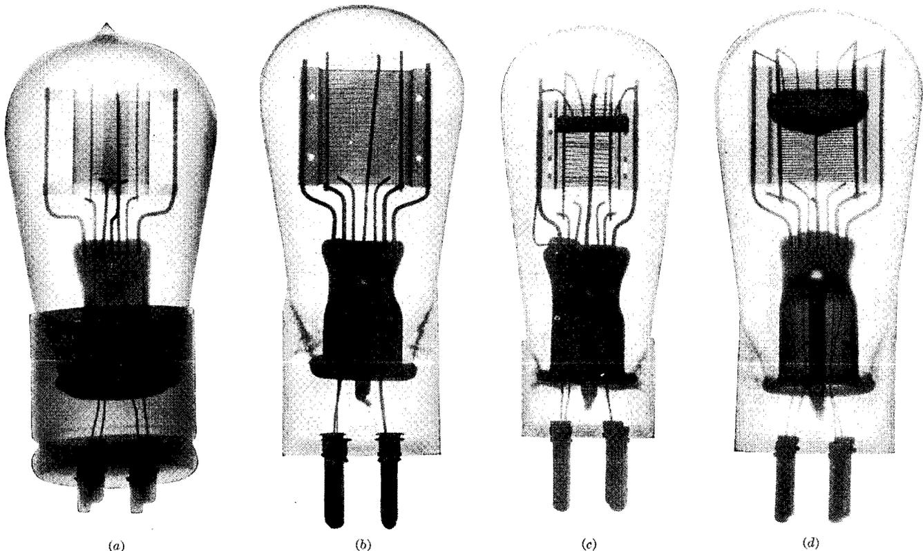
PLATE II.—X-ray photographs of vacuum tubes. (a) Triode, UV-201; (b) triode, type 201A, (c) triode, type 230; (d) triode, type 240.
