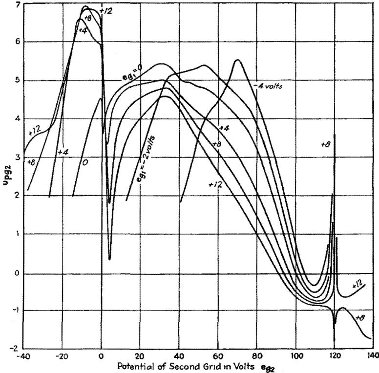
FIG. 323.—Curves of  $u_{pg_2}$  vs.  $e_{g_2}$  for a tetrode. (French Bigrl tube.)
