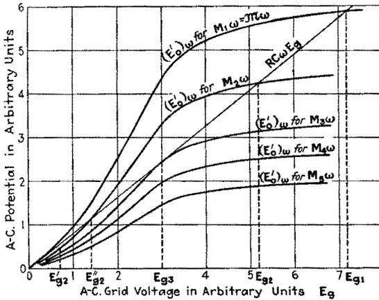
FIG. 190.—Curves of  $(E'_0)_\omega$  vs.  $E_g$  for large-signal regeneration.
