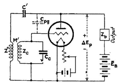
FIG. 250.—Hazeltine's method of neutralization by voltage balance.
