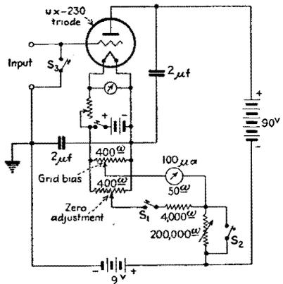
FIG. 318.—Vacuum-tube voltmeter
