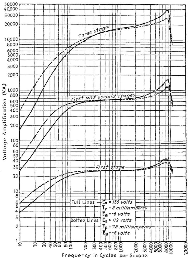
Fig. 244.—Voltage amplification of a three-stage transformer-coupled amplifier. Transformers type TL. UX 201A triode.
