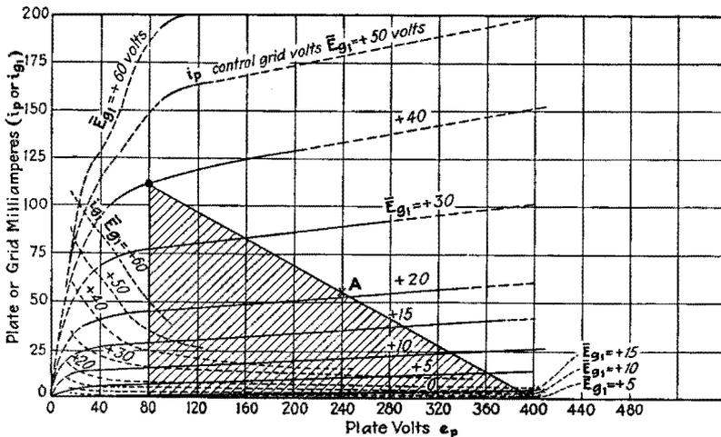
FIG. 336.—Curves of  $i_p$  vs.  $e_p$  for tetrode type 46 used as Class B amplifier.  $\bar{E}_{c1} = \bar{E}_{c2}$ . (R.C.A. Radiotron Handbook.)
