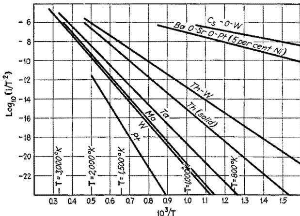
FIG. 13.—Comparison of emission from various kinds of surfaces.
