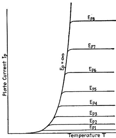
*Plate current vs. temperature for diode*
