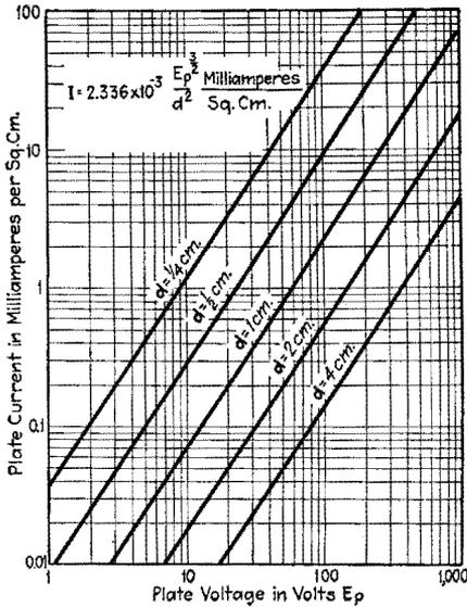
FIG. 18.—Space-charge saturation current between parallel plane electrodes.
