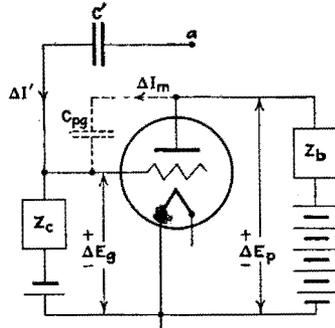
FIG. 252.—Neutralization by current balance.
