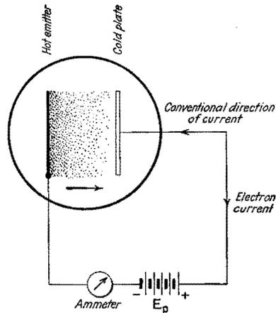
FIG. 15.—Diagrammatic illustration of space charge.
