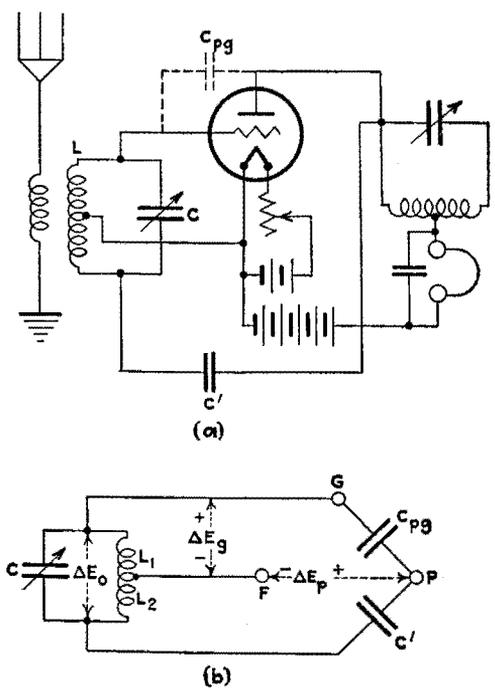
FIG. 251.—Rice's method of neutralization.
