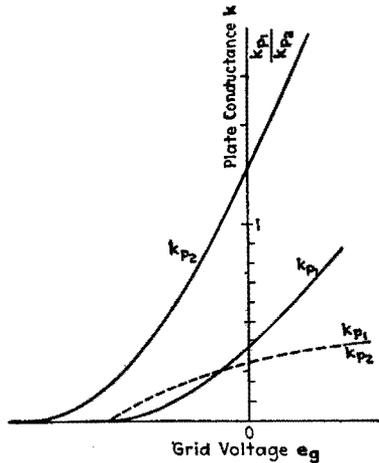
Fig. 87.—Ratio of plate conductances of two triodes.
