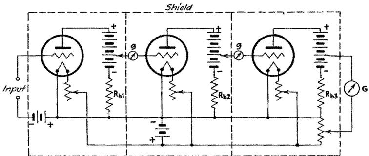
FIG. 234.—Direct-current amplifier.
