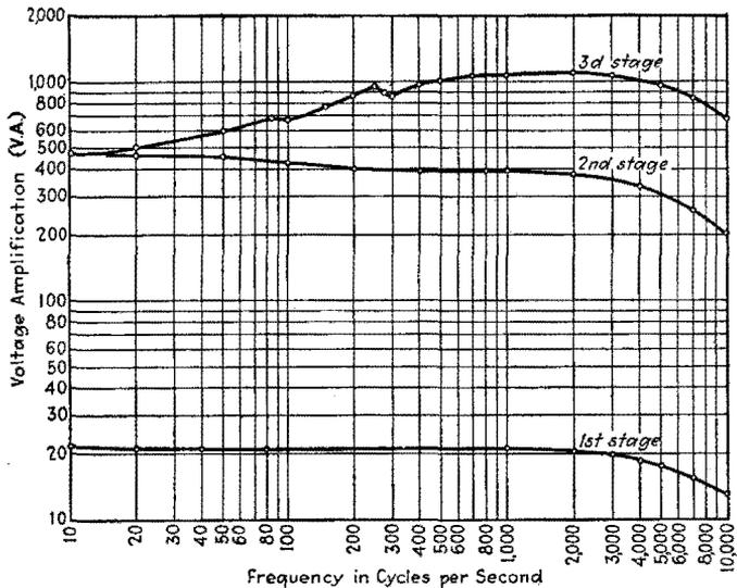
FIG. 230.—Voltage amplification of a three-stage resistance-coupled amplifier measured by a vacuum-tube voltmeter.
