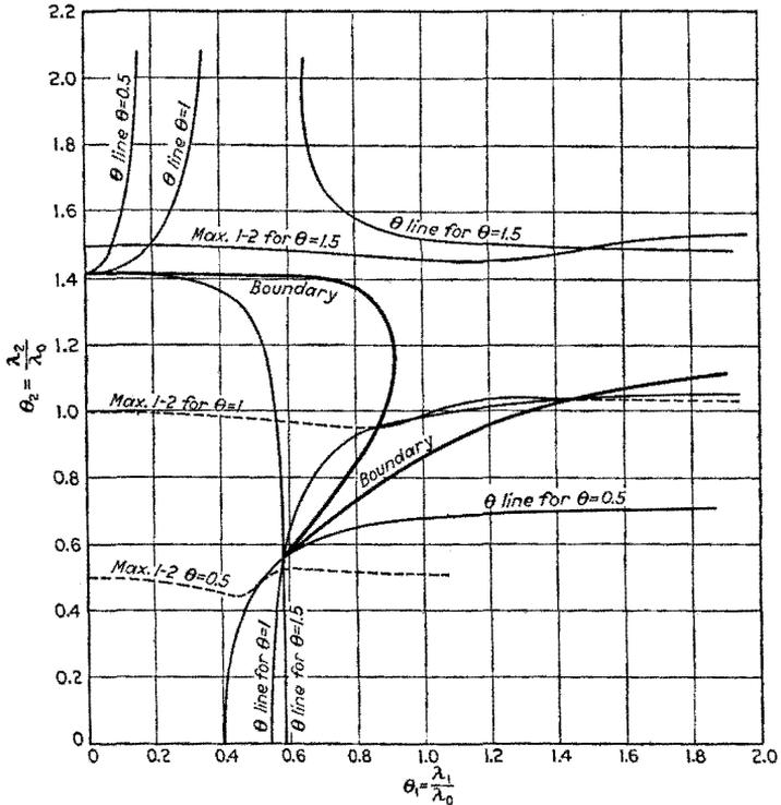
FIG. 219.—Oscillation-boundary curve for variable regenerative effect.
