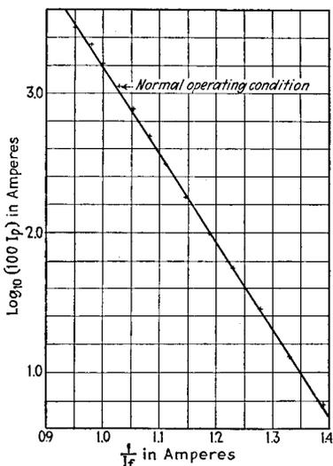
FIG. 30.—Emission of a tungsten filament ( $UV = 201$ ).
