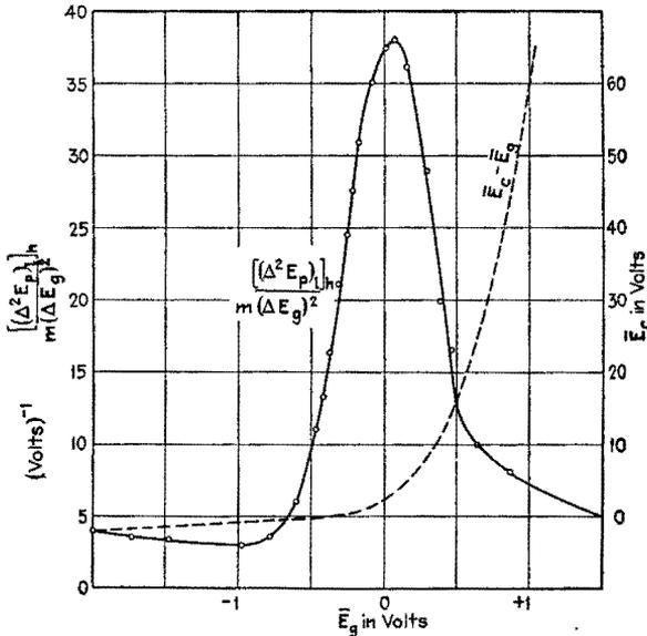
FIG. 284.—Grid-circuit detection.  $u_p = 20$ ;  $\bar{E}_B = 60$  volts;  $R_c = 2.94$  megohms;  $C_c = 200\mu\text{f}$ ;  $\omega = 2\pi 1,000$  radians per second.
