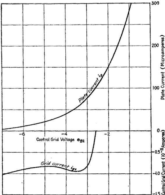
FIG. 345.—Average characteristics of tetrode type FP54.  $\bar{E}_f = 2.5$  volts;  $\bar{E}_{o1} = 4$  volts;  $\bar{E}_p = 6$  volts.
