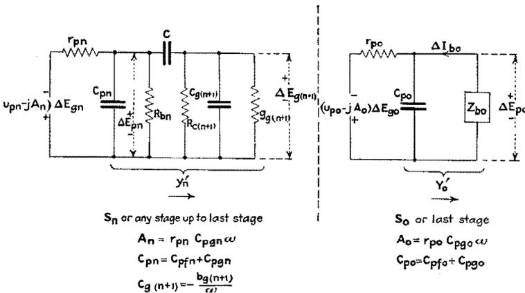
FIG. 226.—Equivalent a-c. circuits of the  $n$ th stage and last stage of a resistance-coupled amplifier.
