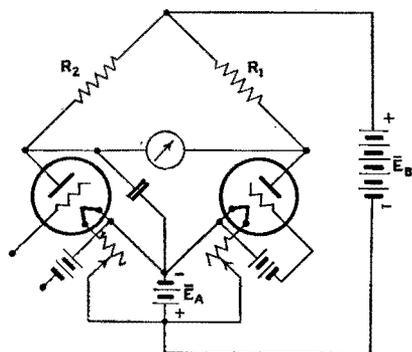
FIG. 315.—Bridge-type vacuum-tube voltmeter with balancing triode.
