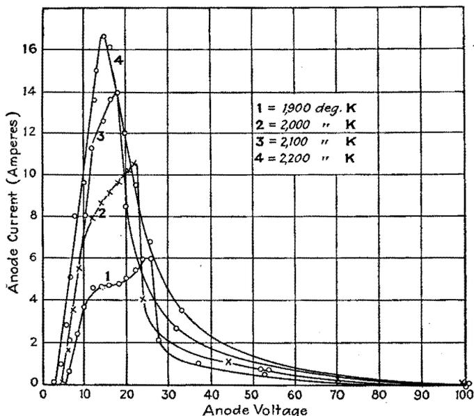
FIG. 124.—Characteristics of a thoriated filament in mercury vapor at 0.005-mm. pressure. (Hull.)
