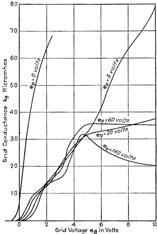
Fig. 70.—Grid variational conductance of a triode (UV 201).
