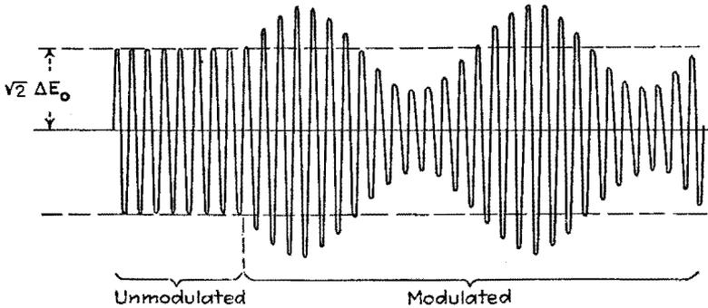
FIG. 261.—Sinusoidally modulated voltage.
