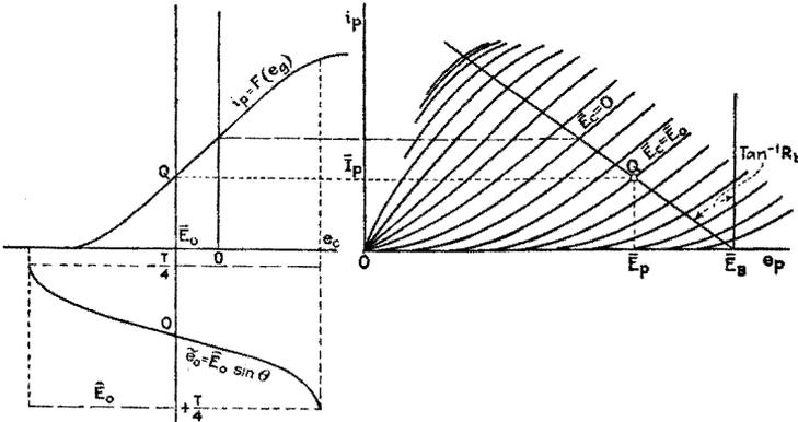
FIG. 298.—The characteristic curve for the plate circuit of a triode having a pure resistance as plate load.
