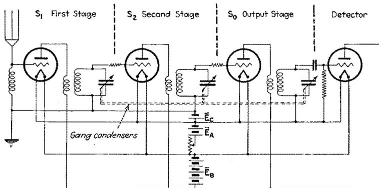
FIG. 245.—Multistage tuned radio-frequency amplifier feeding a detector.
