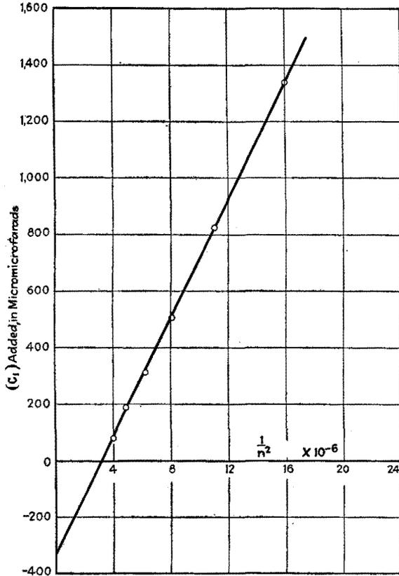
FIG. 11.—Determination of the distributed capacitance of the primary winding of transformer AD1.
