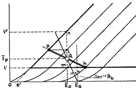
FIG. 172.—Construction for maximum undistorted power output when  $\bar{E}_p$  is given.
