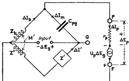
FIG. 253.—General circuit for neutralization by current balance.
