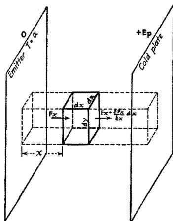
FIG. 16.—Flow of electrons between parallel plane electrodes.
