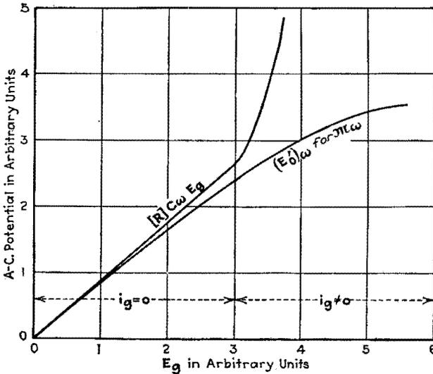
FIG. 188.—The circuit line when grid current flows.
