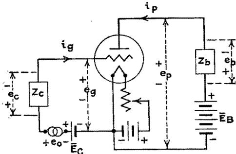
FIG. 90.—Circuits of the triode.
