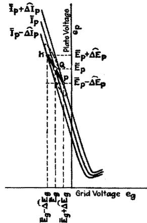
FIG. 100.—Path of operation on the  $e_p - e_g$  chart. Path on the plane region of the characteristic surface.  $\Delta e_g = \Delta E_g \sin \omega t$ .
