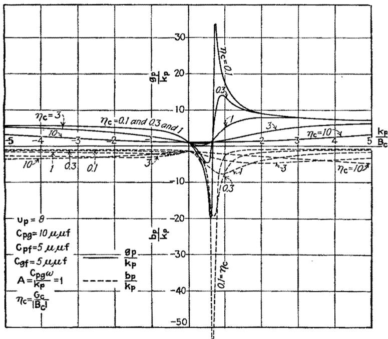
FIG. 155.—Components of the internal output admittance of a triode for various values of  $\eta_c$  when  $k_a = 0$ .  $\eta_c = G_c/|B_c|$ .
