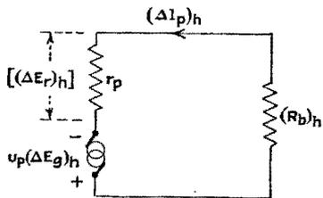
FIG. 279.—Equivalent plate circuit for the high-frequency currents.
