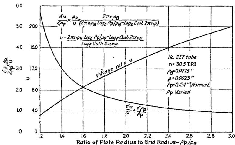
FIG. 83.—Variation of  $u$  with ratio of plate radius to grid radius for a triode having cylindrical electrodes. Plate radius varied.
