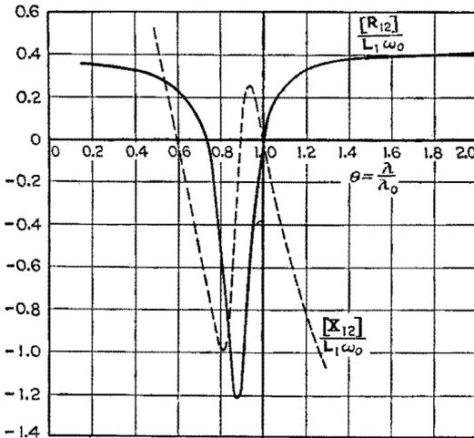
FIG. 213.—Resistance and reactance of coupled circuits as viewed from the primary circuit. Conditions:  $\theta_1 = 0.794$ ;  $[\theta_2] = 0.880$ ;  $\eta_1 = 0.4$ ;  $[\eta_2] = -0.2$ ;  $[\tau] = 0.5$ .
