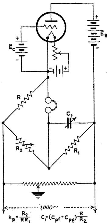
FIG. 119.—First method for the measurement of  $k_p$ .
