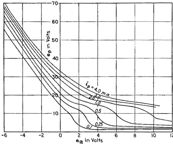
FIG. 128.—Curves of constant plate current in mercury vapor at a pressure of 0.002 mm.
