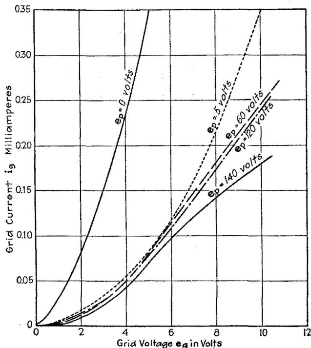
FIG. 64.—Static characteristic curves of a triode.  $i_g - e_g$  curves for constant plate voltage (UV 201).
