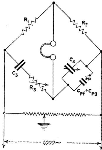
FIG. 145.—Capacitance bridge.
