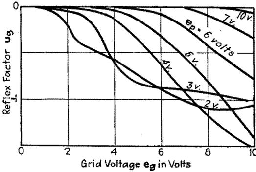
FIG. 71.—Reflex factor of a triode (UV 201).
