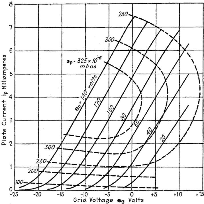
FIG. 72.—Contours of transconductance of a triode (UV 201).
