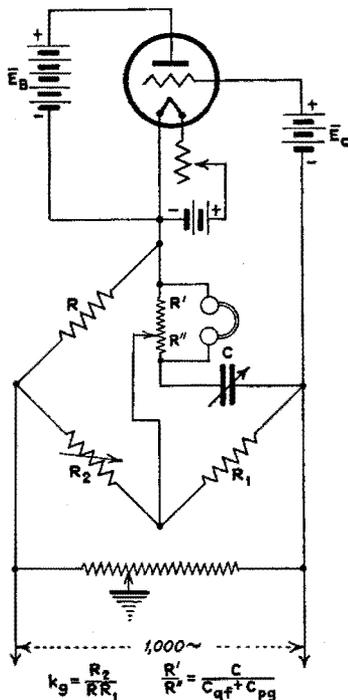
FIG. 122.—Second method for the measurement of  $k_g$ .
