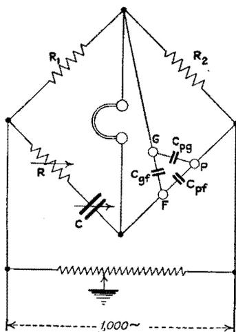
FIG. 147.—Capacitance bridge for directly measuring tube capacitances.
