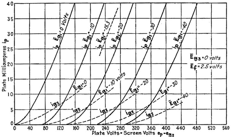
FIG. 338.—Curves of  $i_p$  vs.  $e_p$  of pentode type 247.  $e_{a_2} = e_p$ . (R.C.A. Radiotron Handbook.)
