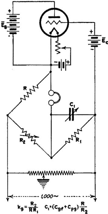
FIG. 121.—First method for the measurement of  $k_g$ .
