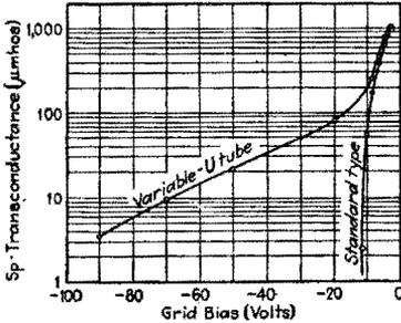
FIG. 343.—Curves of  $s_p$  vs.  $e_1$  for variable-u tetrode.
