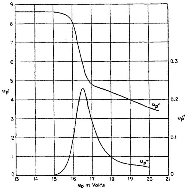
FIG. 130.—Components of  $u_p$  for a triode containing gas.  $u_p = u_p' + ju_p''$
