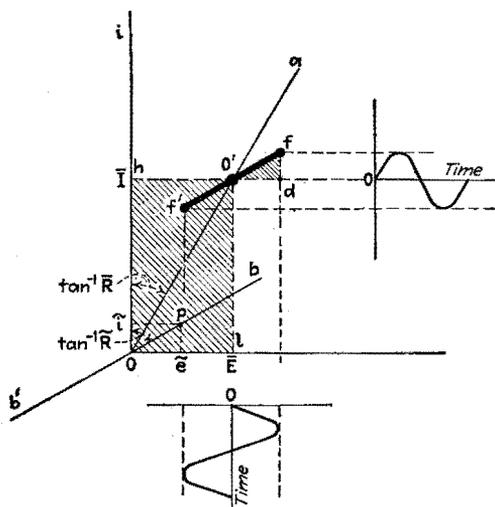
FIG. 2.—Characteristic of a conductor having a different resistance for alternating and direct currents.
