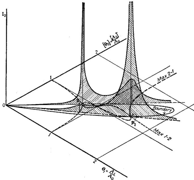
FIG. 217.—Sections of space model for secondary current.  $[R_{21}] = 0$ .  $\eta_1 = 0.4$ .  $[\eta_2] = -0.2$ .  $[\tau] = 0.5$ .
