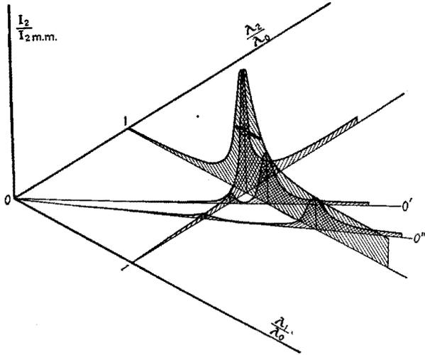
FIG. 205.—Sections of the space model for  $I_2$ . Critical coupling.  $\eta_1 > \eta_2$ .
