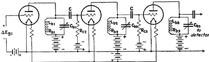
FIG. 238.—Multistage tuned impedance-coupled amplifier for radio frequencies.
