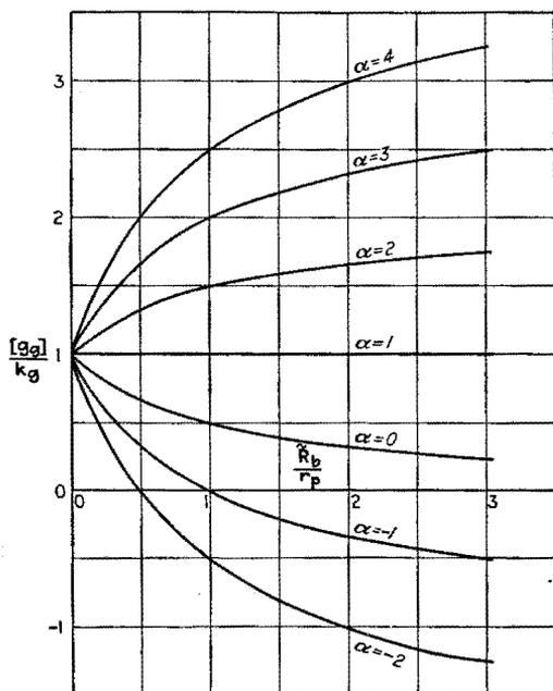
FIG. 141.—Values of  $[g_g]/k_g$  for  $X_b = 0$  and negligible tube capacitances.
