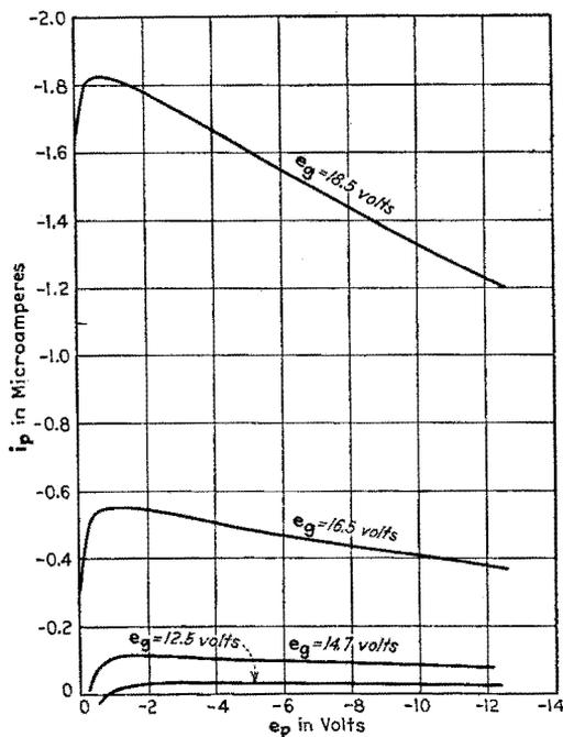
FIG. 134.—Positive-ion current vs. plate voltage for constant grid voltage in a triode containing mercury vapor at a pressure of 0.0016 mm.
