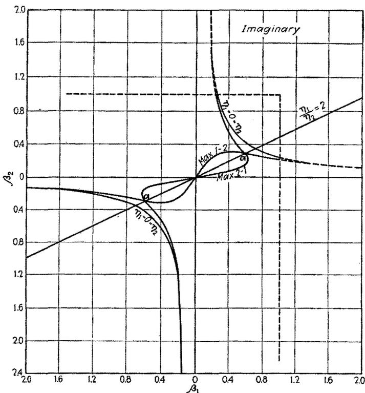
FIG. 198.—Curves of  $\beta_1$  vs.  $\beta_2$  for max.  $I_2$ .  $\eta_1 = 0.4$ .  $\eta_2 = 0.2$ .  $\tau = 0.5$ .
