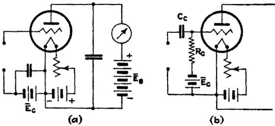
FIG. 312.—Simple vacuum-tube voltmeter.
