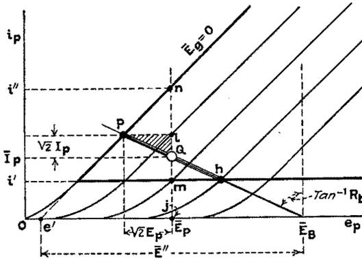
Fig. 171.—Construction for maximum undistorted power output when  $\bar{E}_B$  is given.
