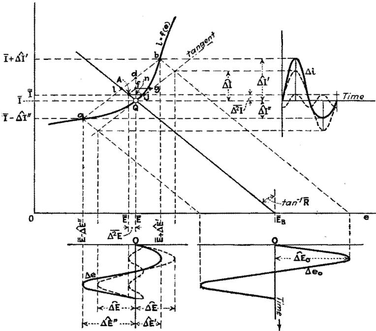
Fig. 265.—Rectification by two-electrode non-linear element in series with a resistance load.
