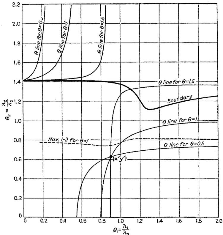
FIG. 222.—Oscillation-boundary curve for variable regenerative effect.
