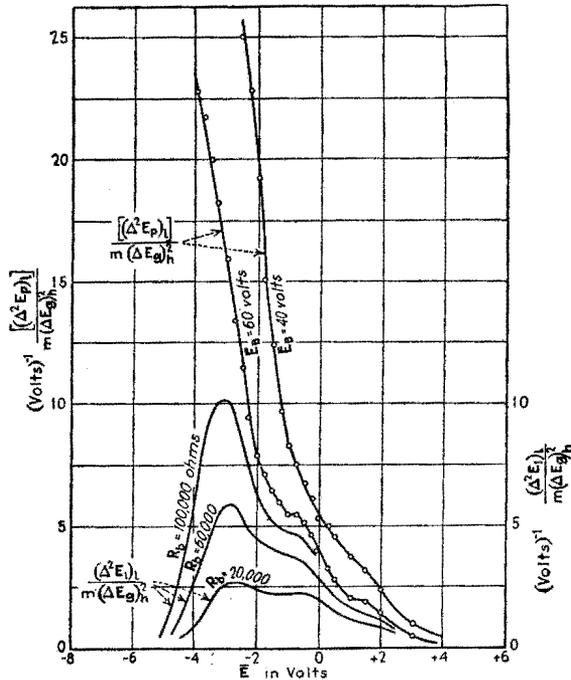
FIG. 286.—Plate-circuit detection.  $u_p = 20$ .
