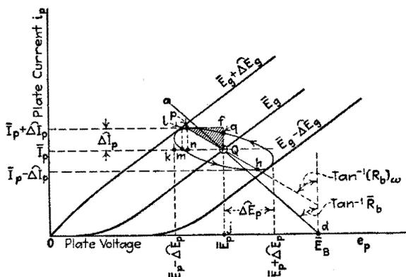
FIG. 103.—Path of operation on the plane region of the characteristic surface.  $\bar{R}_b \neq \tilde{R}_b$  and  $X_b \neq 0$ .  $\Delta e_g = \Delta \bar{E}_g \sin \omega t$ . Arrows give direction for capacitive reactance.
