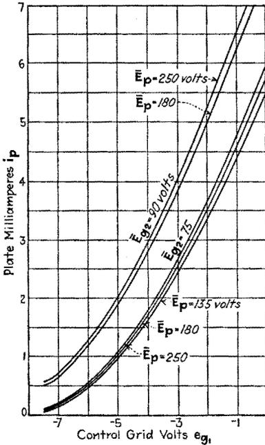
FIG. 325.—Curves of  $i_p$  vs.  $e_{g1}$  for tetrode UY224. (R.C.A. Radiotron Handbook).
