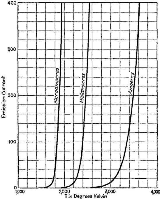
FIG. 12.—Saturation current for tungsten.  $E = \infty$ .
