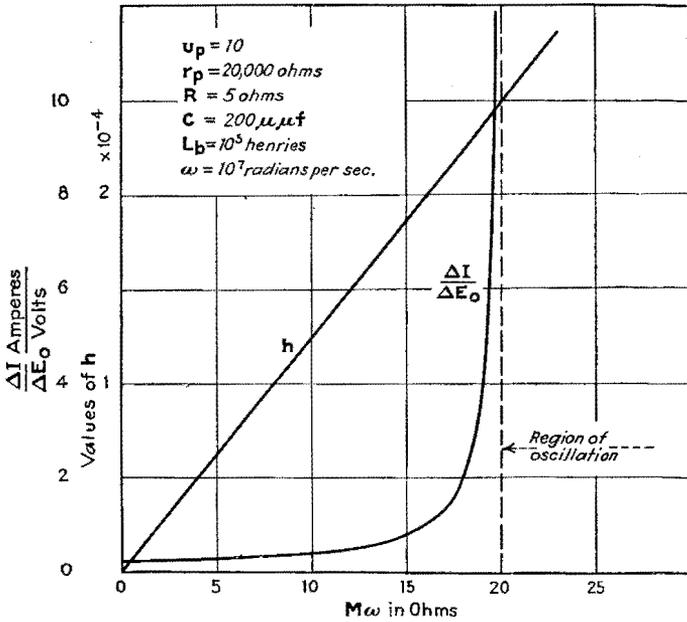
FIG. 176.—Variation of resonance current with feed-back coupling.
