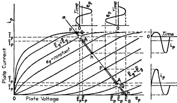
FIG. 104.—Paths of operation on curved regions of the characteristic surface. Pure resistance as plate load.  $R_b = R_b$ .  $e_g = \bar{E}_g \sin \omega t$ .
