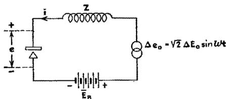
FIG. 264.—Diode detector with load.
