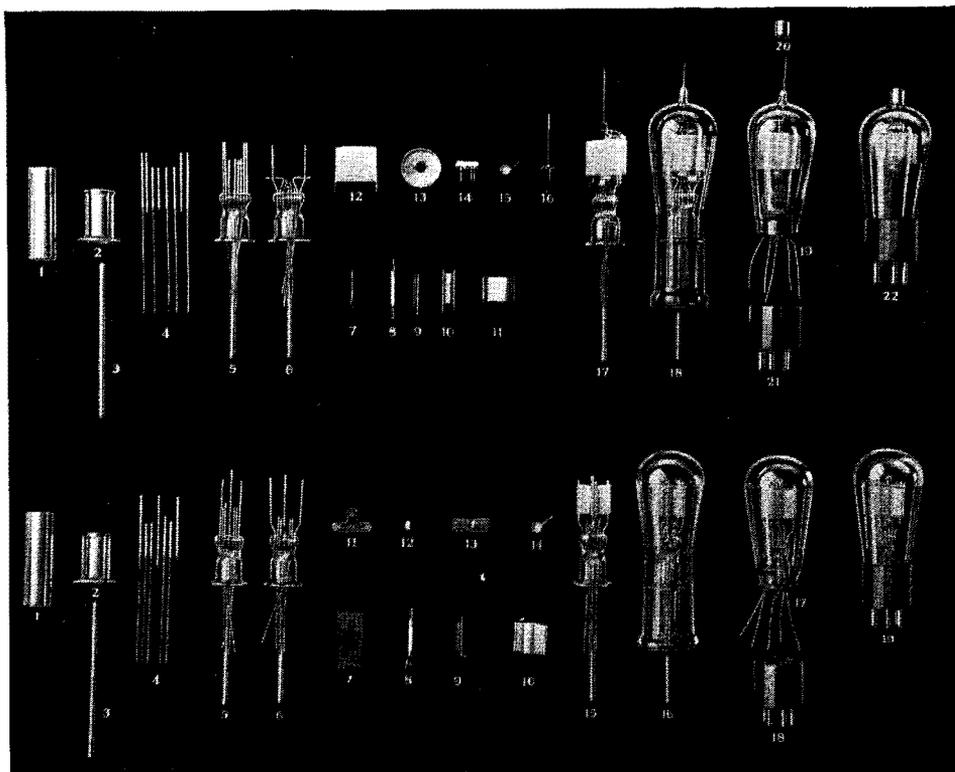
PLATE I.—Construction of modern vacuum tubes. (Courtesy of R.C.A. Radiotron Company.)
