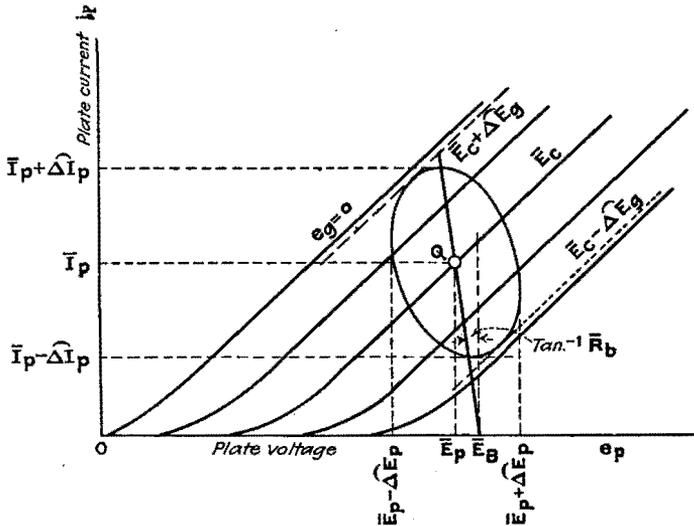
FIG. 164.—Path of operation for amplifier having an inductive plate load.
