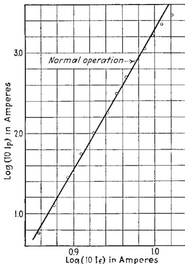
FIG. 31.—Emission of a tungsten filament ( $UV = 201$ ).
