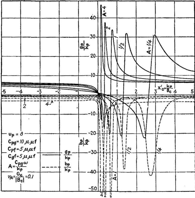
Fig. 154.—Components of the internal output admittance of a triode for various values of  $A$  when  $k_v = 0$ .
