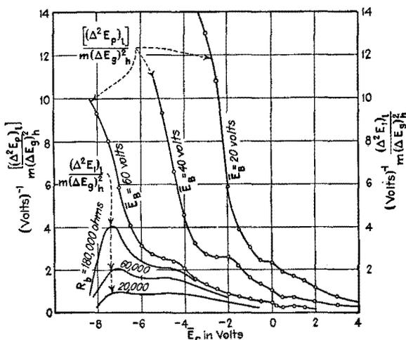
FIG. 285.—Plate-circuit detection. UX201A.  $u_p = 8.5$ .
