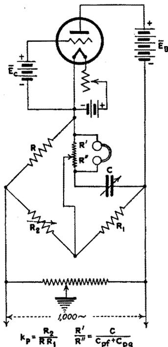
FIG. 120.—Second method for the measurement of  $k_p$ .
