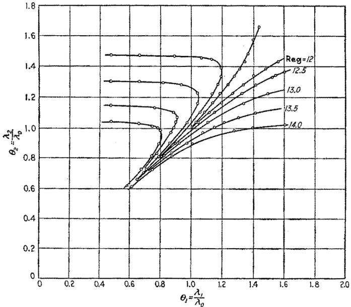
FIG. 224-2.—Experimental boundary curves. Effect of varying regeneration.  $\lambda_0 = 600$  meters.
