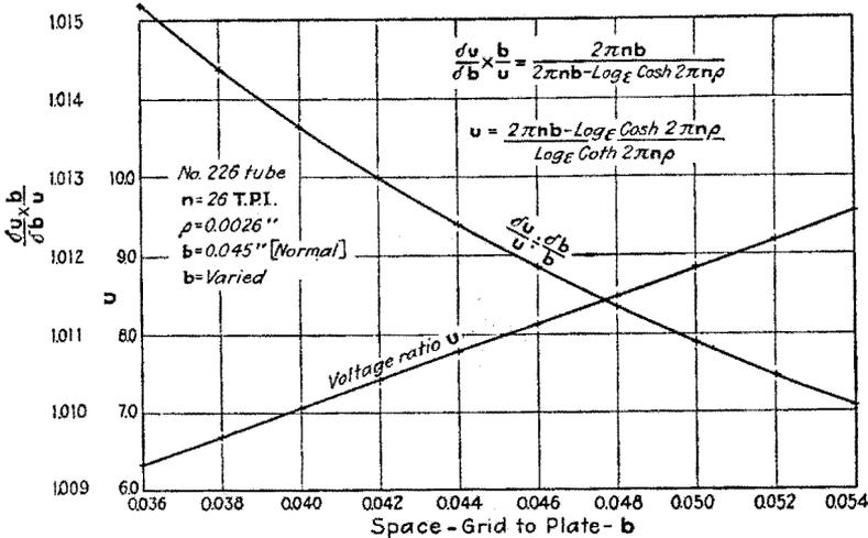
FIG. 80.—Variation of  $u$  with distance from grid to plate for a triode having plane electrodes.
