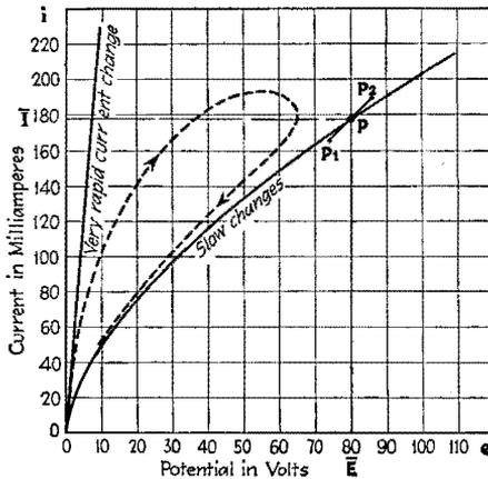
FIG. 8.—Current-voltage characteristic curve of a tungsten-lamp filament.
