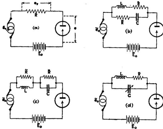
FIG. 294.—Circuits containing a nonlinear element.
