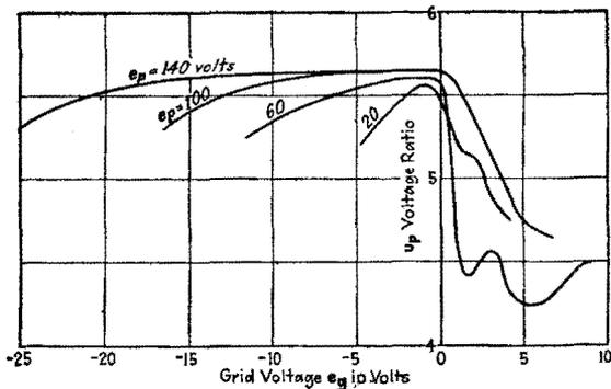
FIG. 68.—Voltage ratio of a triode (UV 201).
