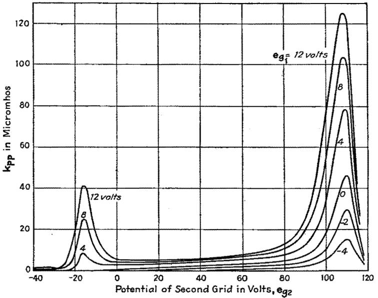
FIG. 321.—Curves of  $k_{pp}$  vs.  $e_{g_2}$  for a tetrode. (French Bigril tube.)
