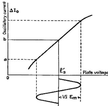
FIG. 273.—Characteristic of oscillator.
