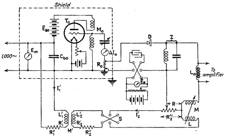
FIG. 271.—Measurement of detection by diode.
