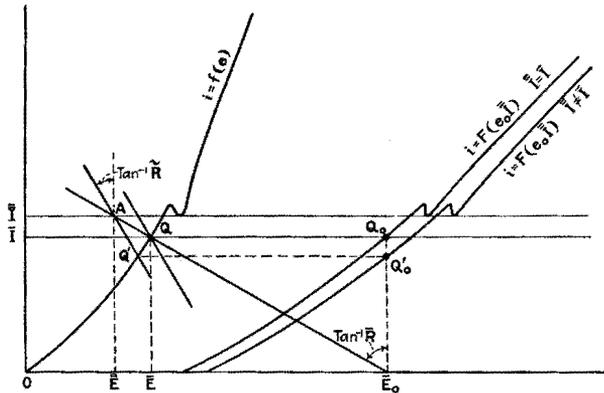
FIG. 295.—Curves of  $i = F(e_0, \bar{I})$  derived from curve of  $i = f(e)$ , showing transformation of a kink in the curve.
