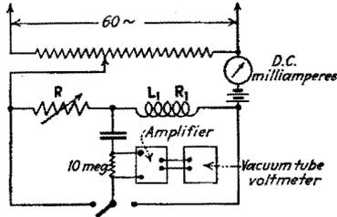
FIG. 8.—Method of measuring  $L_1$  with a steady current flowing through the winding.
