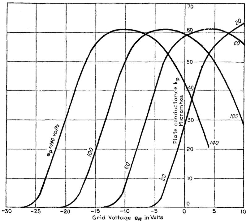
FIG. 67.—Plate variational conductance of a triode (UV 201).
