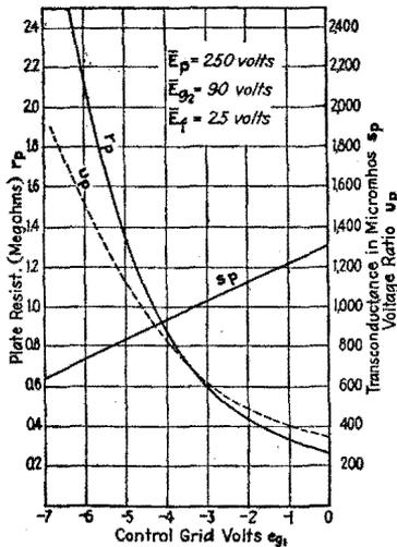
FIG. 329.—Equivalent triode coefficients of tetrode UY224 plotted against  $e_{g_1}$ . (R.C.A. Radiotron Handbook.)
