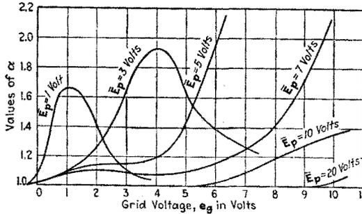
FIG. 139.—Values of  $\alpha$  for a high-vacuum triode (UV201).
