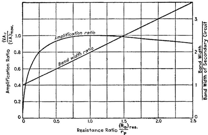
Fig. 170.—Variation of (V.A.) and selectivity with mutual inductance of the tuned transformer.
