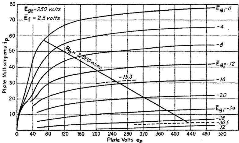
FIG. 339.—Curves of  $i_p$  vs.  $e_p$  for pentode type 247 with suppressor grid.  $\bar{E}_{a_3} = 250$  volts;  $\bar{E}_{a_3} = 0$ . (R.C.A. Radiotron Handbook.)
