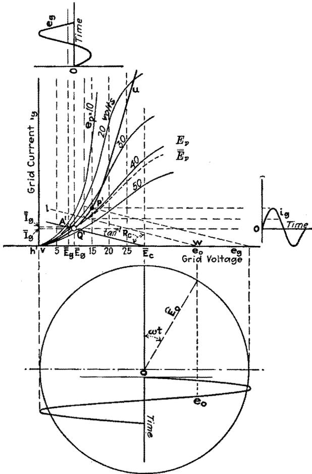
FIG. 108.—Path of operation on the grid-current surface when  $\bar{R}_b = \bar{R}_b$  and  $\bar{R}_c = \bar{R}_c$ .
