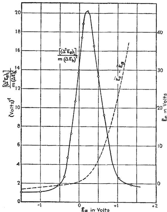
FIG. 283.—Grid-circuit detection.  $u_p = 8.5$ ;  $\bar{E}_B = 60$  volts;  $R_c = 2.94$  megohms;  $C_c = 200\mu\text{mf}$ ;  $\omega = 2\pi 1,000$  radians per second.
