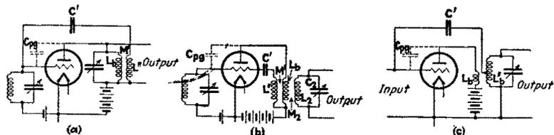
FIG. 255.—Methods of neutralization by current balances.
