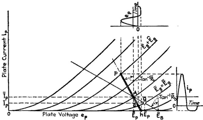
FIG. 105.—Path of operation on a curved region of the characteristic surface  $\bar{R}_b \neq \bar{R}_b$ .  $e_g = \bar{E}_g \sin \omega t$ .
