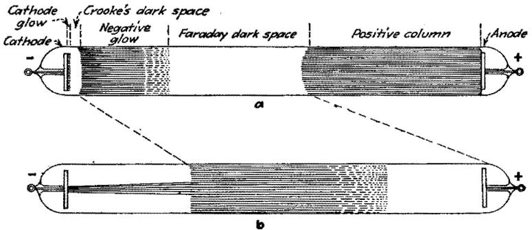
FIG. 6.—Electric discharge through a gas at reduced pressure.
