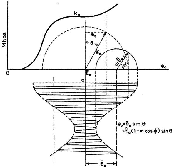
FIG. 291.—Calculation of the magnitude of the current of modulation frequency.
