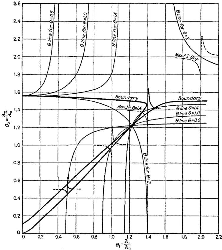
Fig. 220.—Oscillation-boundary curve for variable regenerative effect.
