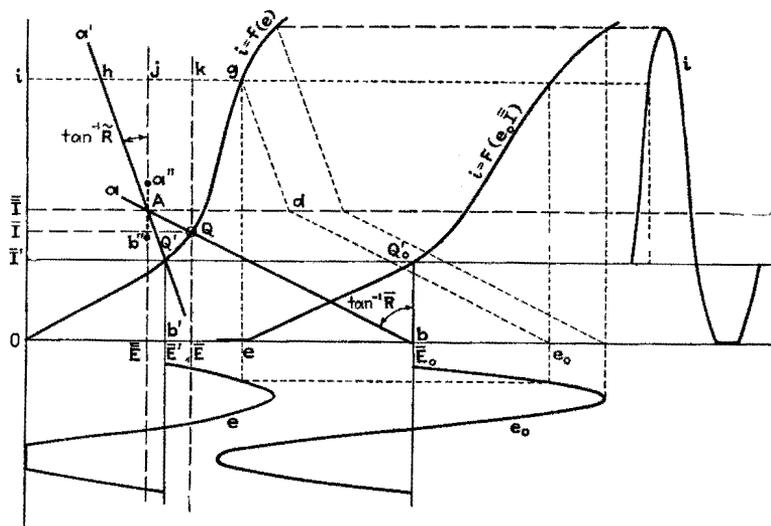
FIG. 296.—Method of the derivation of the curve of  $i = F(e_0, \bar{I})$  from the curve of  $i = f(e)$  when  $\bar{R} \neq \hat{R}$ .
