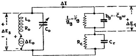
FIG. 281.—Equivalent grid circuit of the triode detector.
