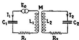
Fig. 196.—Magnetically coupled circuits.
