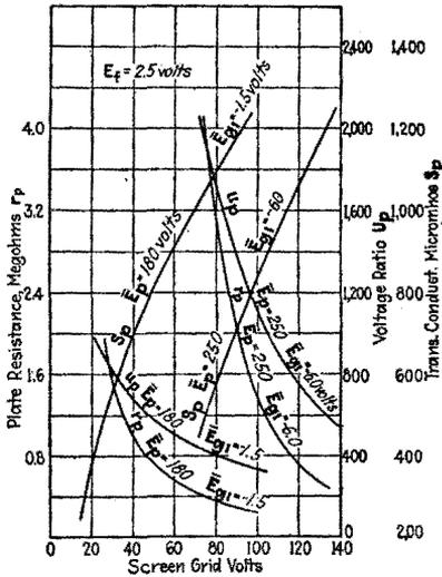
FIG. 330.—Equivalent triode coefficients of tetrode UY224, plotted against  $e_{s_2}$ . (R.C.A. Radiotron Handbook.)
