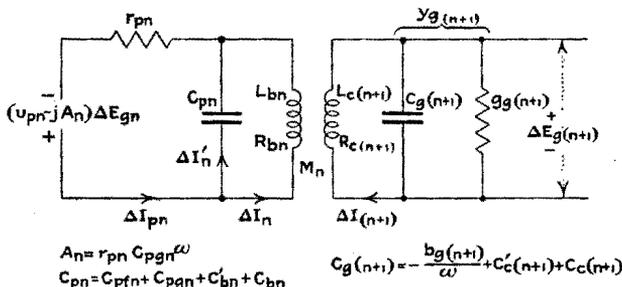
FIG. 241.—Equivalent a-c. circuits of the transformer-coupled amplifier.
