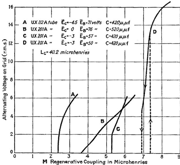
FIG. 189.—Variation of the voltage across the oscillatory circuit of Fig. 184 as the regenerative coupling is varied.
