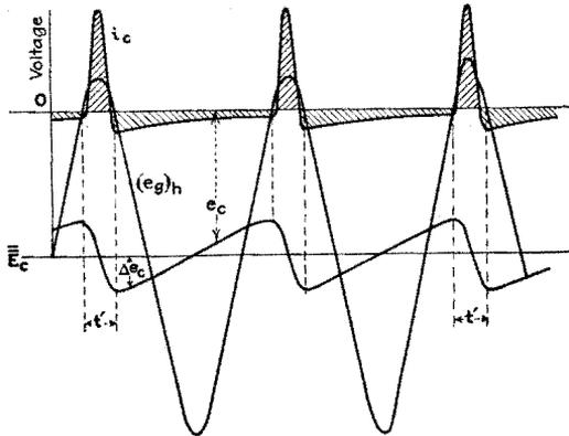
FIG. 308.—Voltages and grid current in grid-circuit detection.
