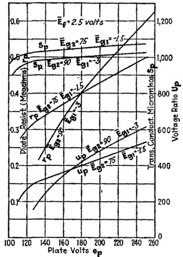
FIG. 331.—Equivalent triode coefficients of tetrode UY224 plotted against  $e_p$ . (R.C.A. Radiotron Handbook.)
