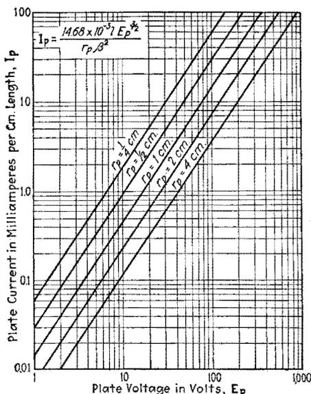
FIG. 21.—Space-charge saturation current between cylindrical electrodes.  $\beta^2 = 1$ .
