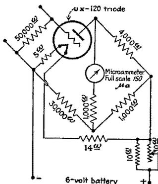
FIG. 316.—Portable bridge-type thermionic voltmeter. (General Electric Company.)
