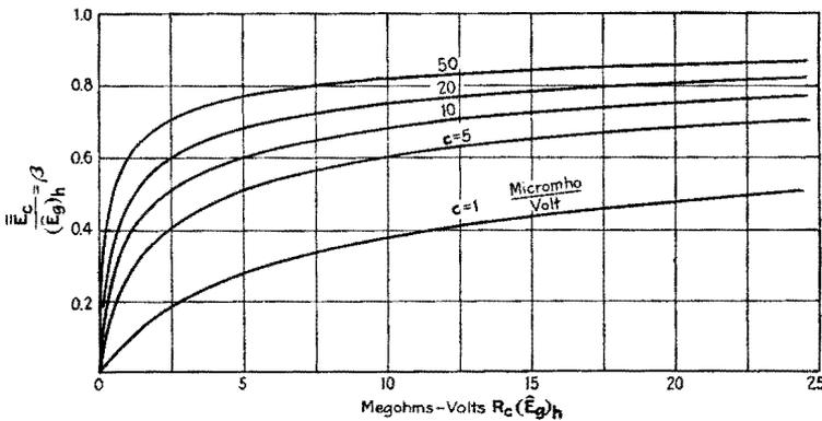
FIG. 309.—Values of  $\beta$  plotted against  $R_c(\bar{E}_g)_h$ .
