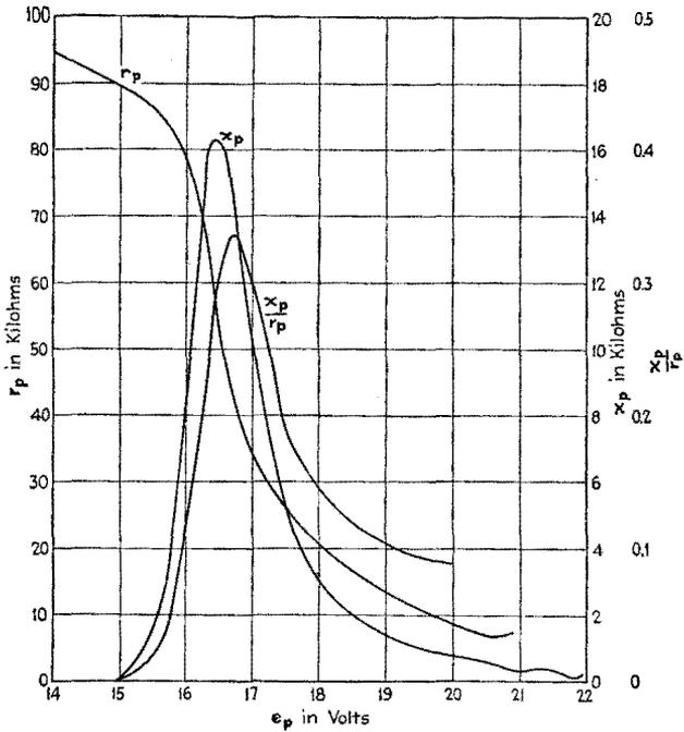
FIG. 131.—Components of  $z_p$  for a triode containing gas.  $z_p = r_p + jx_p$ .  $e_g = 0$ .
