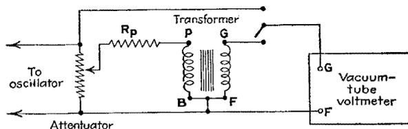
Fig. 1.—Method of determining the voltage ratio of an audio transformer, using a vacuum-tube voltmeter.
