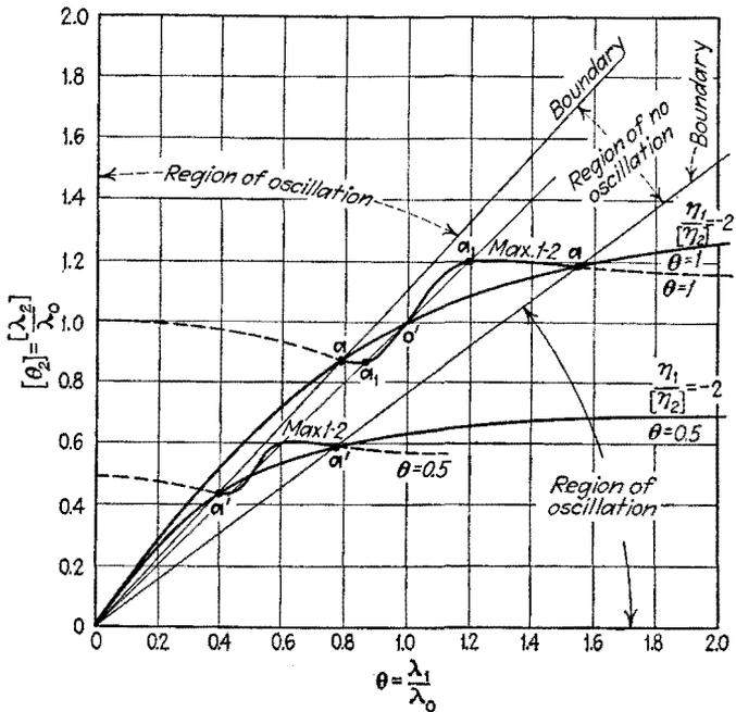
FIG. 211.—Oscillation boundary lines for constant regenerative effect. Condition of constant  $\eta$ .  $[r] = 0.5$ .  $\eta_1 = 0.4$ .  $[\eta_2] = -0.2$ .
