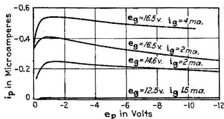
FIG. 135.—Positive-ion current vs. plate voltage for constant grid voltage and grid current in a triode containing mercury vapor at a pressure of 0.0016 mm.
