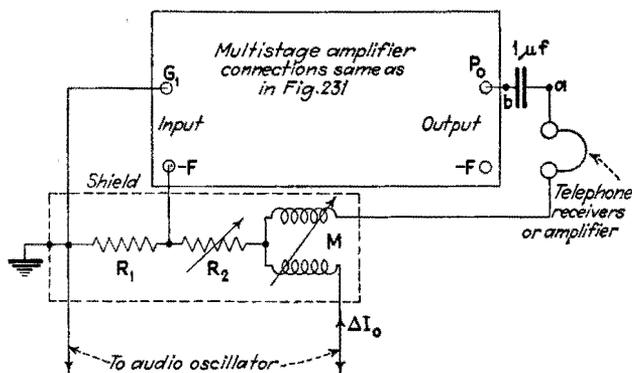
FIG. 232.—Balance method of measuring the voltage amplification of a multi-stage amplifier.
