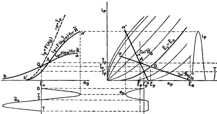
FIG. 299.—Curves for the path of operation for the plate circuit of a triode when  $R_b \neq \bar{R}_b$ .
