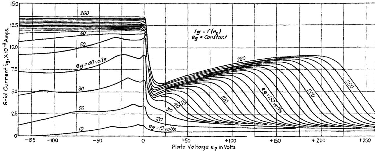
FIG. 59.—Static characteristic curves of the grid current of a triode. Curves of constant grid voltage. (van der Pol.)
