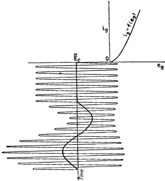
FIG. 307.—Grid-circuit detection with large-signal voltage.
