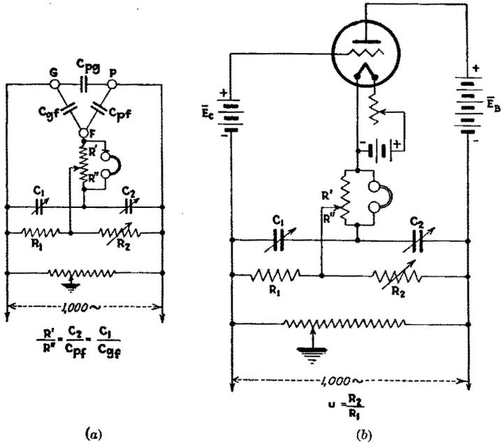
FIG. 117.—Second method for the measurement of  $u$ , and  $u_p$  (if  $i_g = 0$ ).
