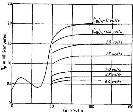
FIG. 334.—Grid-circuit detection characteristics of tetrode ER224.  $\bar{E}_A = 2.5$  volts;  $\bar{E}_{u_2} = 45$  volts.
