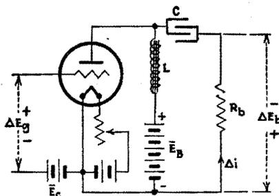
Fig. 161.—Resistance-loaded amplifier using parallel feed.
