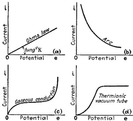
FIG. 7.—Forms of  $e$ - $i$  characteristic curves.
