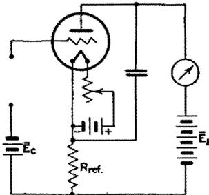
FIG. 317.—Reflexed vacuum-tube voltmeter.
