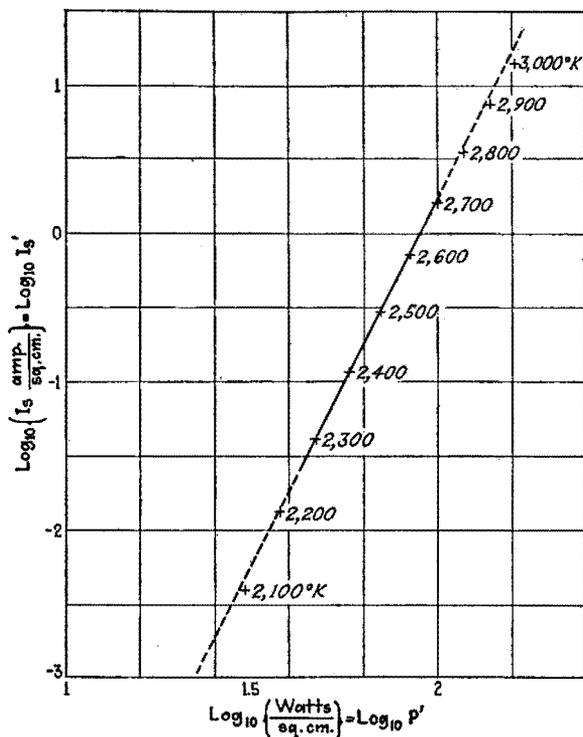
FIG. 43.—Emission-power curve for tungsten.
