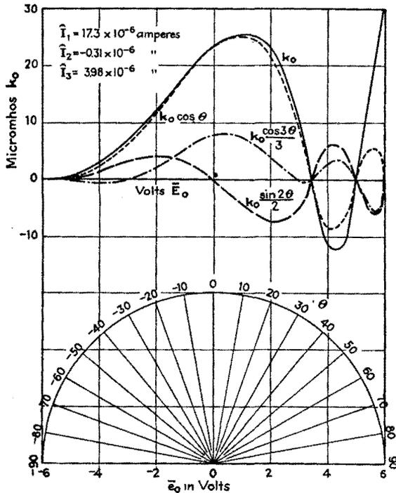
FIG. 300.—Method of calculating the magnitudes of the fundamental and harmonic components of current from the curve of  $k_0$ . Example 2.
