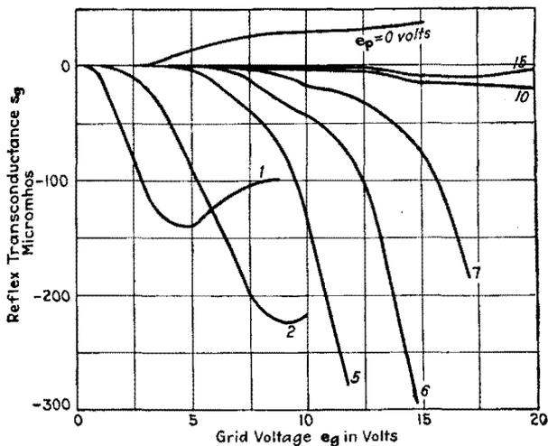
FIG. 69.—Reflex transconductance of a triode (UV 201).
