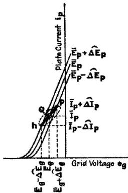
FIG. 99.—Path of operation on the  $i_p - e_g$  chart. Path on the plane region of the characteristic surface.  $\Delta e_g = \Delta E_g \sin \omega t$ .
