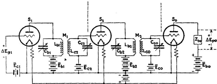
Fig. 240.—Multistage transformer-coupled amplifier.
