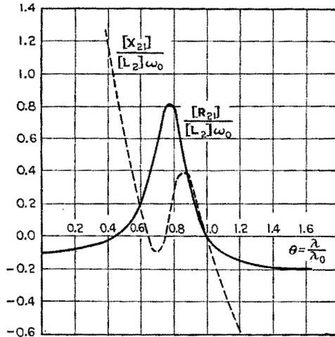
FIG. 212.—Resistance and reactance of coupled circuits as viewed from the secondary circuit. Conditions:  $\theta_1 = 0.794$ ;  $[\theta_2] = 0.880$ ;  $\eta_1 = 0.4$ ;  $[\eta_2] = -0.2$ ;  $[\tau] = 0.5$ .
