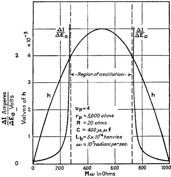
FIG. 177.—Variation of resonance current with feed-back coupling.
