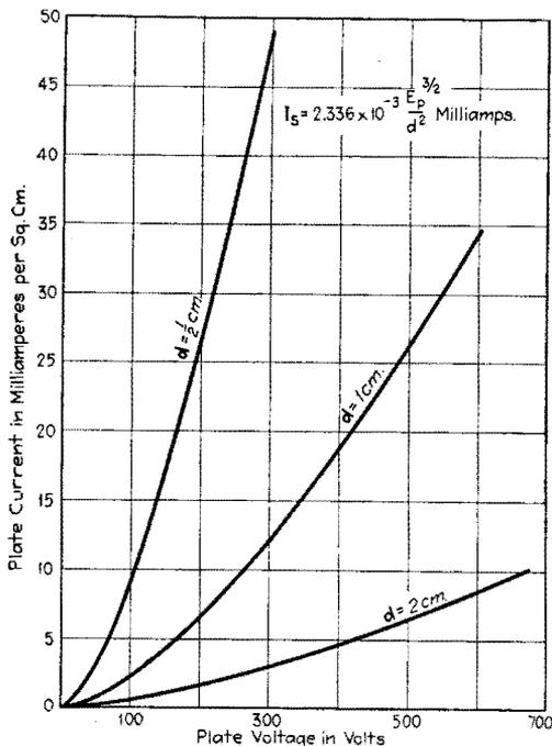
FIG. 17.—Space-charge saturation current between parallel plane electrodes.
