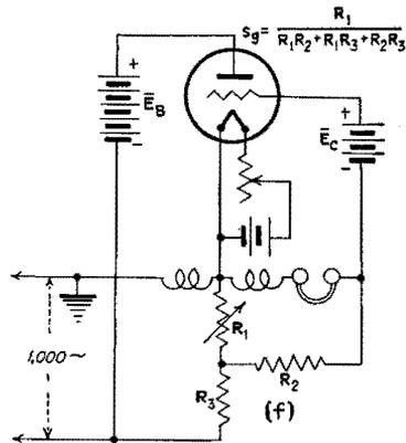
FIG. 123.—Circuits for the measurement of  $s_p$  and  $s_g$ .
