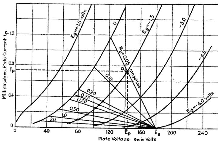
FIG. 227.—Plate-current plate-voltage diagram for a resistance-coupled amplifier.
