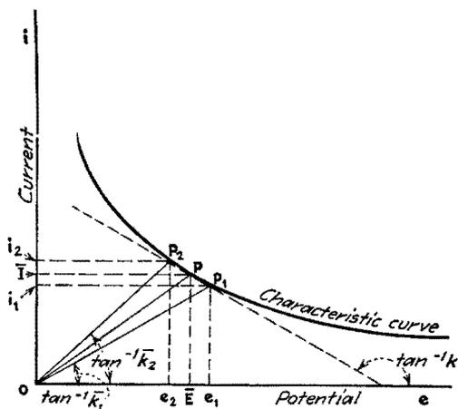
FIG. 9.—Characteristic curve of an arc.
