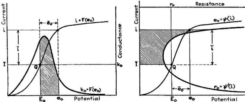
FIG. 287.—Calculation of  $\bar{i}$  and  $\bar{e}_0$  from curves of  $k_0$  and  $r_0$ .
