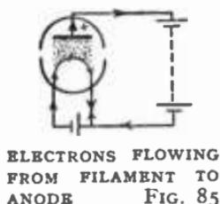
ELECTRONS FLOWING FROM FILAMENT TO ANODE FIG. 85
