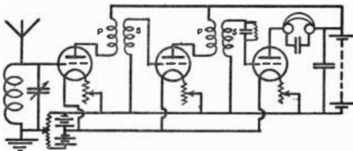
AMPLIFICATION BY MEANS OF APERIODIC H.F. TRANSFORMERS
