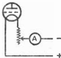
AN AMMETER IN THE VALVE FILAMENT CIRCUIT
