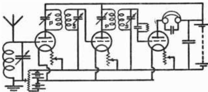
AMPLIFICATION BY MEANS OF H.F. TRANSFORMERS WITH PRIMARIES AND SECONDARIES TUNED
