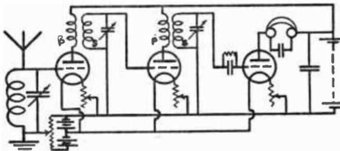
AMPLIFICATION BY MEANS OF H.F. TRANSFORMERS WITH SECONDARIES TUNED
