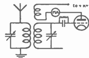
A MILLIAMMETER IN THE ANODE CIRCUIT
