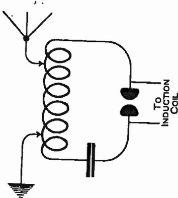
FIG. 18.—Oscillatory circuits of directly coupled transmitter
