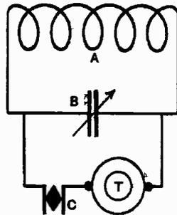
FIG. 139.—Connections of Marconi wave meter
