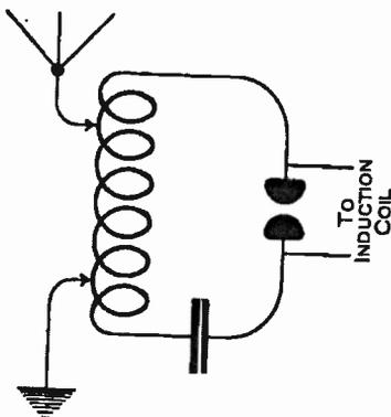
FIG. 18.—Oscillatory circuits of directly coupled transmitter
