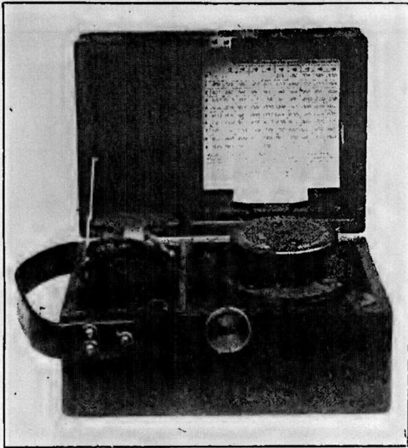
FIG. 138.—Marconi wave meter
