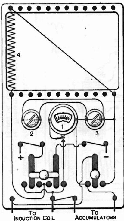
FIG. 78.—Marconi marine type charging switchboard
