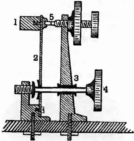
FIG. 75.—Showing construction of contact-breaker
