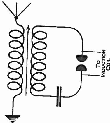
FIG. 19.—Oscillatory circuits of inductively coupled transmitter
