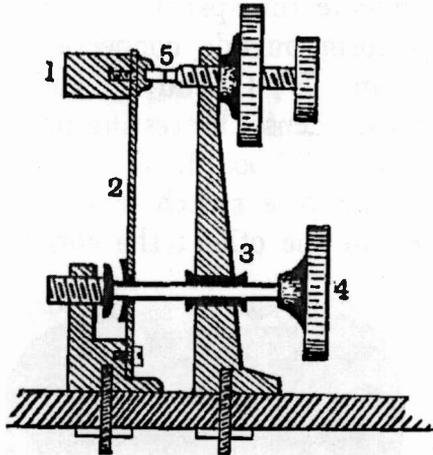
FIG. 75.—Showing construction of contact-breaker
