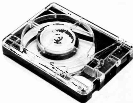
**FIGURE 2.25** An audio cartridge. The tape comes off the hub at the center, runs left to right across the front, and returns to the outside of the reel.
