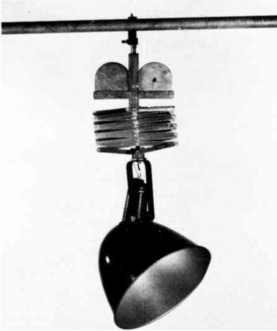
*FIGURE 1.24* A scoop on a pantograph
