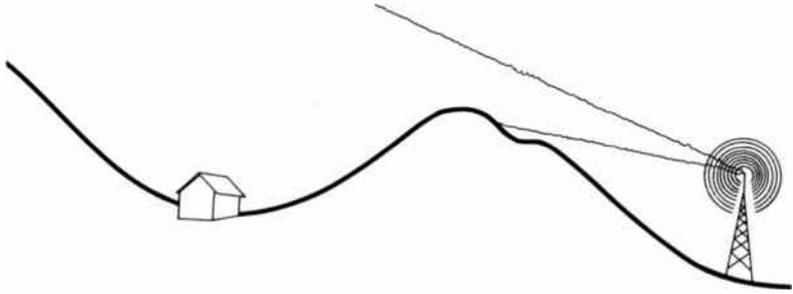
FIGURE 7.1 Signals blocked
