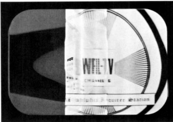
*Fig. 18·24 Open  $B+$  boost capacitor. (RCA.)*
