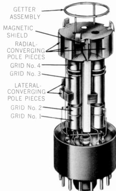
Fig. 25·18 Assembly of three electron guns in 21FJP22 color kinescope. (RCA.)
