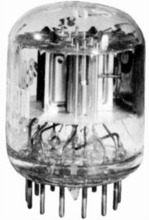
Fig. 6·9 Compactron multifunction tube 6B10, combining two diodes and two triodes. Height 1½ in. (GE.)
