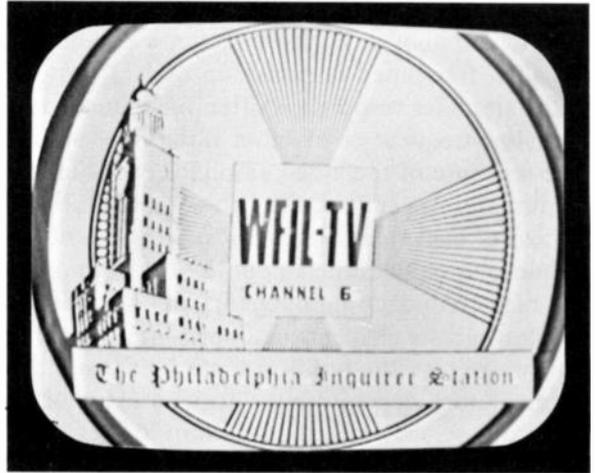
circle, indicating video-frequency response up to 4 Mc. The divisions in the widest part of the vertical wedges correspond to a video frequency of about 2 Mc.
