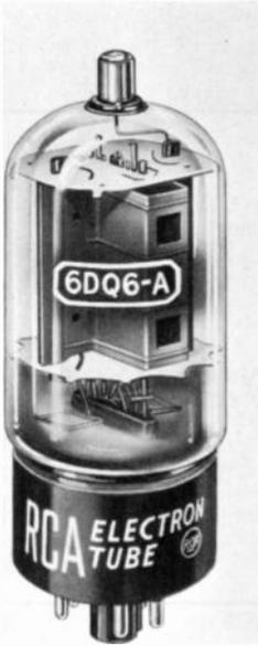
Fig. 6·11 Horizontal power output tube with octal base. Top cap is the plate. (RCA.)
