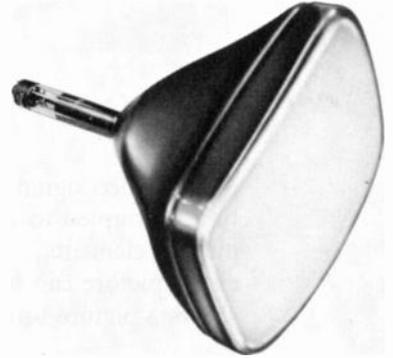
signals, which are then amplified and detected in the receiver. The detector output includes the desired video signal containing the information needed to reproduce the picture. Then the recovered video signal is amplified and coupled to an image-reproducing tube that converts the electric signal back into picture elements in the same degree of black or white.
