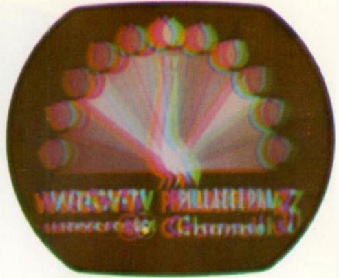
Plate II Color fringing caused by incorrect convergence. (RCA.)
