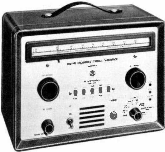
Fig. 20·15 Crystal-calibrated marker, oscillator. (RCA.)
