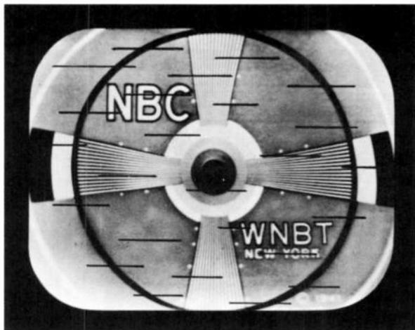
*Fig. 23·4 Short horizontal black streaks caused by auto-ignition interference.*
