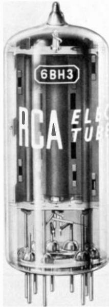
Fig. 6·12 Half-wave power rectifier tube 6BH3 for damper diode in horizontal output circuit. This is a novar tube with dark heater. (RCA.)
