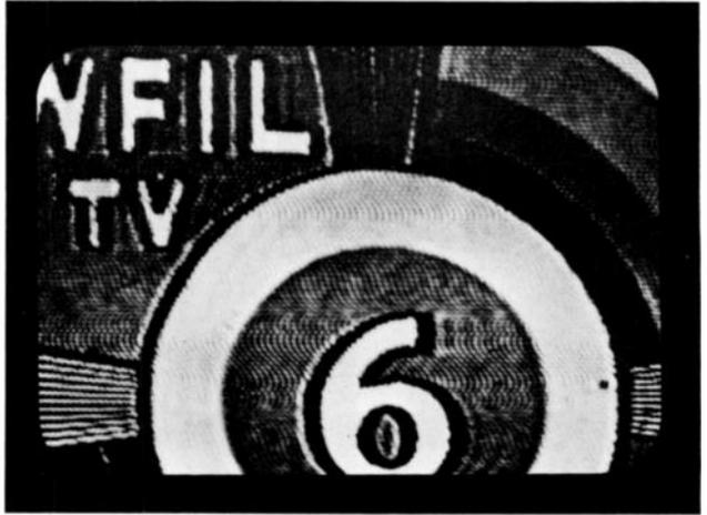
Fig. 23·5 *Fine herringbone-weave or wormy effect of 4.5-Mc beat in picture. (RCA.)*
