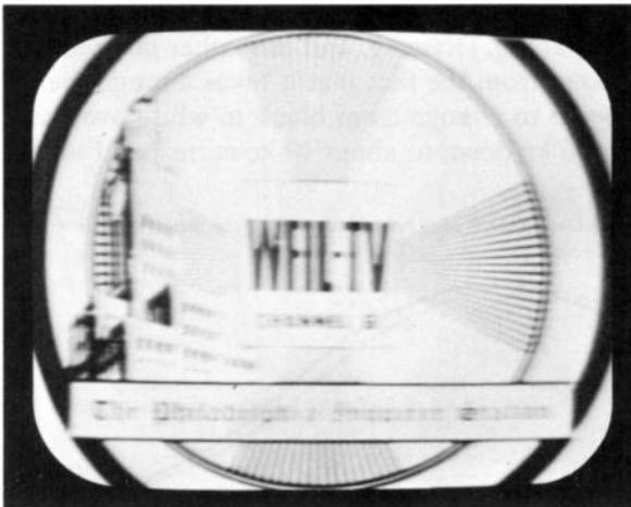
Fig. 9·13 Test pattern illustrating loss of low-video signal frequencies. Background is weak, lettering is not solid, and the side wedges have weaker intensity than the wedges at top and bottom. (RCA Pict-O-Guide.)
