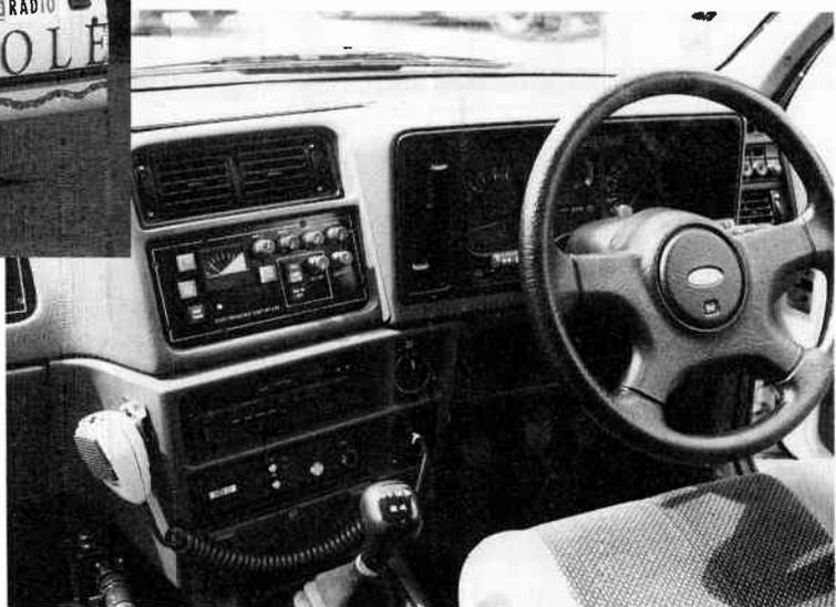
**Figure 44** (Left) The radio car with its tall pump-up aerial acts like a mobile studio for sending on-the-spot reports back to the station. (Right) The idea is to keep the operation as simple as possible so that even the most non-technical of reporters can cover a breaking story without having to bring an engineer along to press the buttons (Andrew Boyd)
