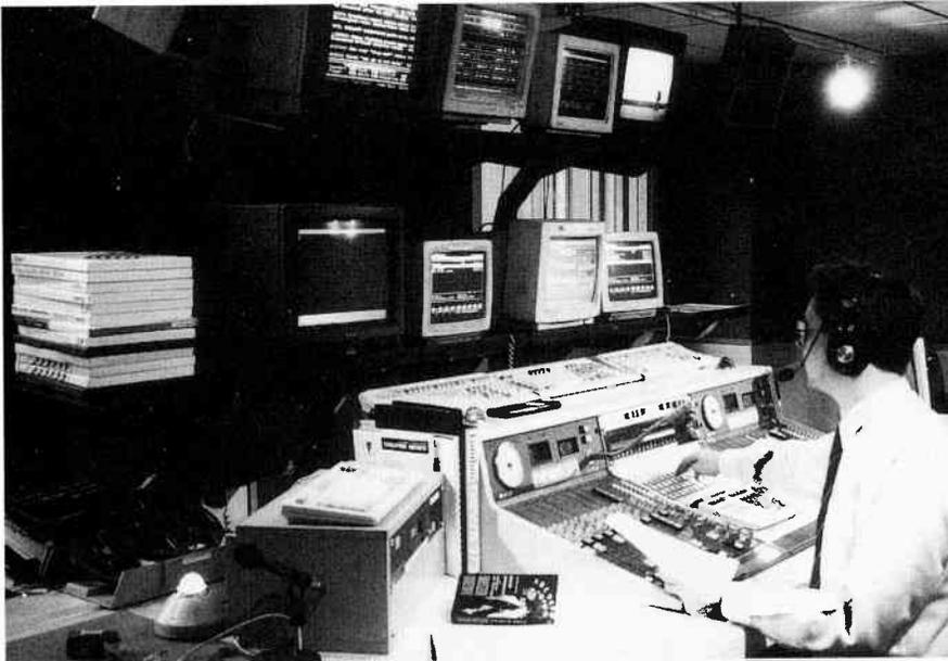
**Figure 62** (top) The radio studio is undergoing a transformation. No fewer than eight TV screens and monitors grace this studio in London as audio is played to air from computer hard disk. But the revolution still has some way to run. . . notice the stack of tapes on the left (Andrew Boyd)
