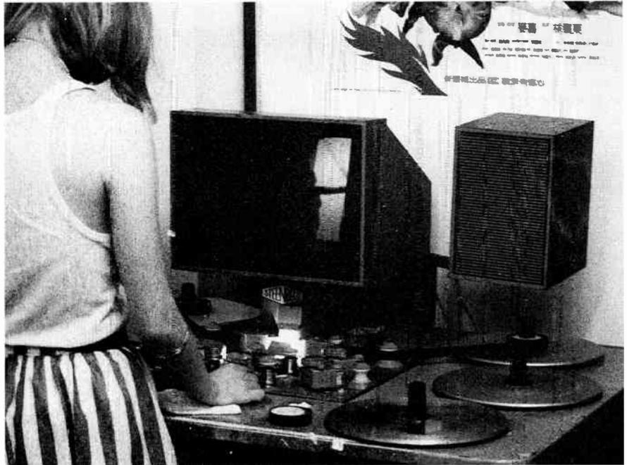
**Figure 92** The Steenbeck flatbed editing machine permits the editor to review the film on screen while listening to the soundtrack (Andrew Boyd)
