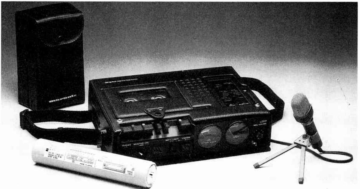
It has a *tape selector* to set the correct bias and equalisation for the cassette tape. *Normal* is used for ferric oxide tapes, *Cro2* for aluminium dioxide and similar, and *metal* for metal tapes.
