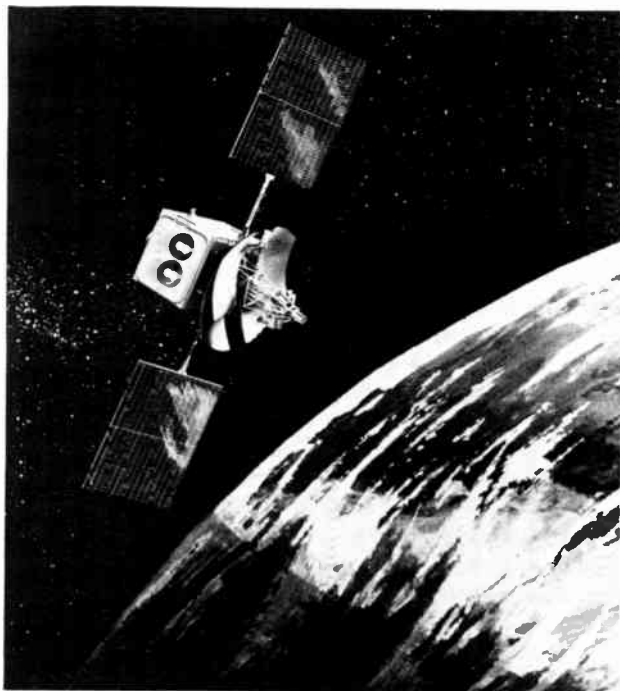
Figure 5-9 RCA's Satcom satellite, which is part of RCA's domestic satellite system. Satcom II has 75 square feet of solar cells mounted on two panels continuously pointed at the sun. The cells produce 740 watts of power sufficient to charge its batteries and drive the operating functions of the 1,000-pound spacecraft. Satcom III, operational in 1980, is devoted primarily to serving cable television systems.
