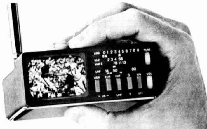
Figure 3-24 Small circuitry has made possible portable television receivers the size of portable radios. The set shown measures 4" × 6 3/4" × 1 3/4". A 2" diagonal screen produces black and white images with the detail of larger sets. (Sinclair Radionics, Inc.)
