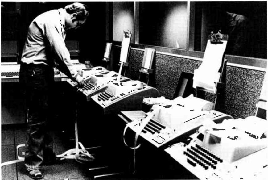
Figure 8-5 Connecting point for the PBS communication teletype link with affiliate stations. (Stan Cahill & PBS)
