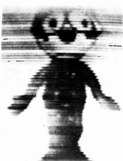
Figure 3-19 In 1928, television was progressing through its experimental era which showed the clarity of a 60-line picture in black and white (left). The television picture was produced by putting Felix the Cat in front of a television camera flanked by high intensity spotlights (right). (RCA)
