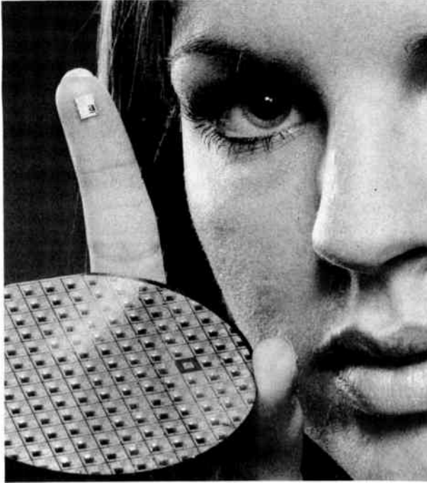
Figure 3-18 The transistor chip on the woman's finger has a circuit capacity of thousands of single transistors. (Rockwell International)
