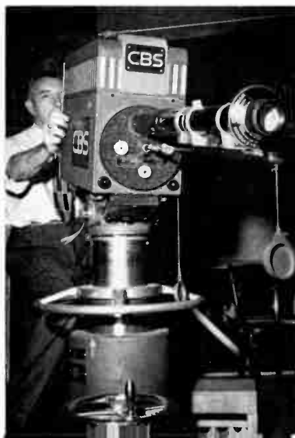
34. Zoomar Lens Makes Instantaneous Cutting Possible. It can go from long shots to close-ups, wide angles to close-ups, and vice versa, without switching cameras. (Photo by courtesy of the Columbia Broadcasting System.)
