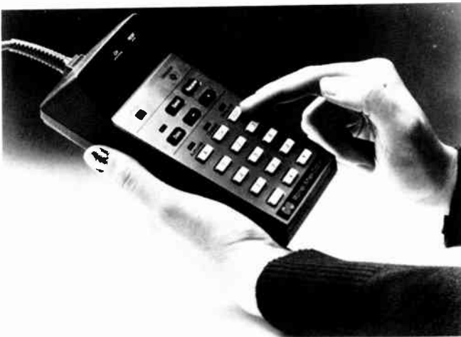
FIGURE 8-5 Hand-held two-way home terminals permit the subscriber to access many more services than are available with one-way systems. (Warner Amex)
