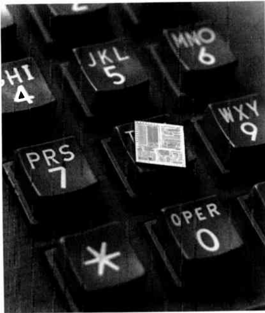
FIGURE 5-3 The microprocessor made possible the microcomputer. Smaller than the key on a telephone, these tiny devices can contain more than 100,000 transistor circuits and are capable of making over a million calculations every second. (Bell Labs)
