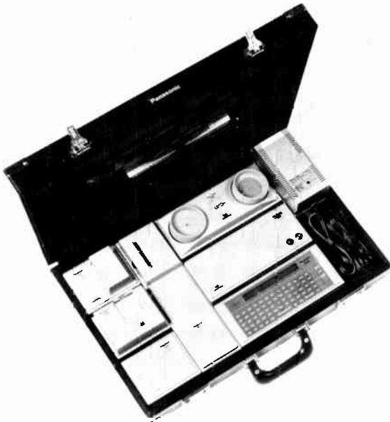
FIGURE 5-5 The move to portability resulted in many companies marketing personal computers which were easy to take to job sites, transport on trips, and included modems which could be used to access distant data banks. This component model designed for a briefcase was manufactured by Panasonic. (Panasonic)
