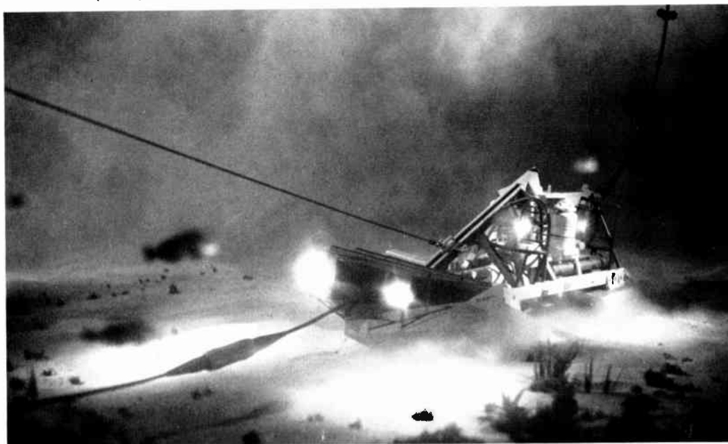
FIGURE 7-11 An ocean cable-laying machine called the Sea Plow IV is used to install transatlantic cable. Such cables serve many of the functions of satellites, aggravating the discussion of the regulatory framework and cost-effectiveness of the two communication systems. (AT&T)
