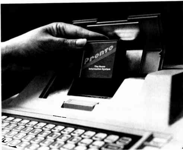
FIGURE 9-8 Electronic banking is one of the services provided by videotext. One of the early systems was New York's Chemical Bank, which inaugurated the "Pronto" system. The system operated by using a special Atari personal computer. Balance inquiry, bill-paying, funds transfer, and electronic mail were some of the features announced at the introduction of the Pronto system. (Chemical Bank)
