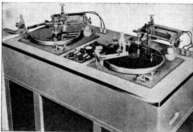
Fig. 20. A disc recorder for making transcriptions. By using both tables, programs of any length can be recorded without a break. (Courtesy Presto Corp.)
