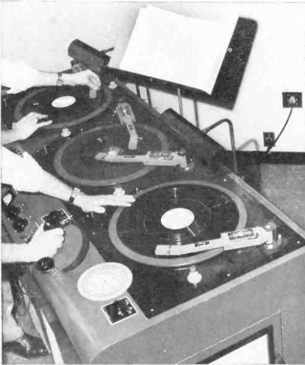
FIG. 40. Sound recordings upon the turntables. Notice how the recordings are held with the needle set upon the record, the turntable revolving, until the cue is picked up by the operator. The circular mat in the foreground is a stroboscopic disc used to test the constancy of the revolving speed of the turntable. When seen by the light of a neon lamp from a 60-cycle current, the outer circle of teeth will seem to remain stationary when the disc is revolving at 33\frac{1}{3} revolutions per minute. The inner circle will appear stationary when the disc is revolving at 78.26 revolutions per minute.
