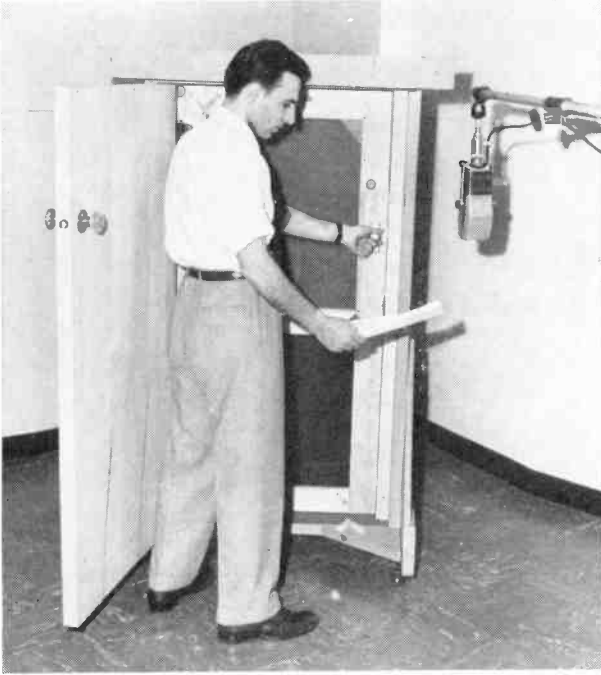
FIG. 44. The sound operator is picking up the sound of the opening of a door with the microphone close to the door. Equipment shown is a combination of three doors, heavy outside door, screen door, and indoor door, all in one frame.
