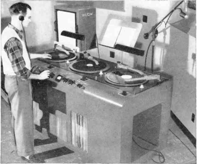
FIG. 39. Sound table. Four pickup heads, three turntables, mixers, record racks in the front, speaker set into recess at the end of the sound table. ( University of Michigan. )
