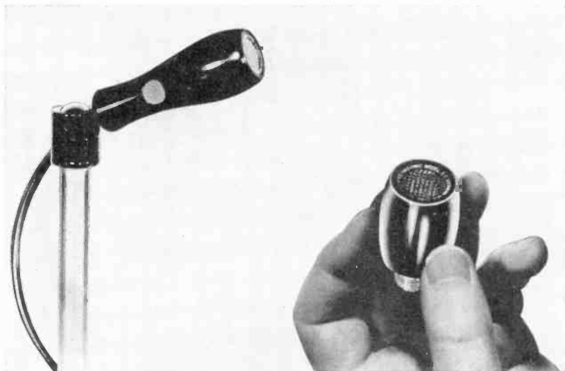
FIG. 10. Tru Sonic model C-1C microphone system. Condenser type. The oscillator/demodulator (amplifier) unit is separate from the microphone. ( Stephens Manufacturing Corporation. )
