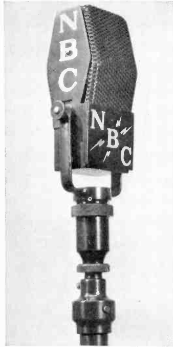
FIG. 3. Bidirectional velocity or ribbon microphone. (R.C.A.)
