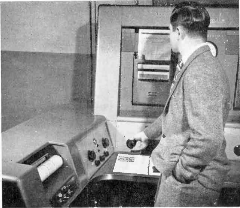
FIG. 27. Facsimile scanner to the left and receiving unit to the right as used at the University of Missouri.
