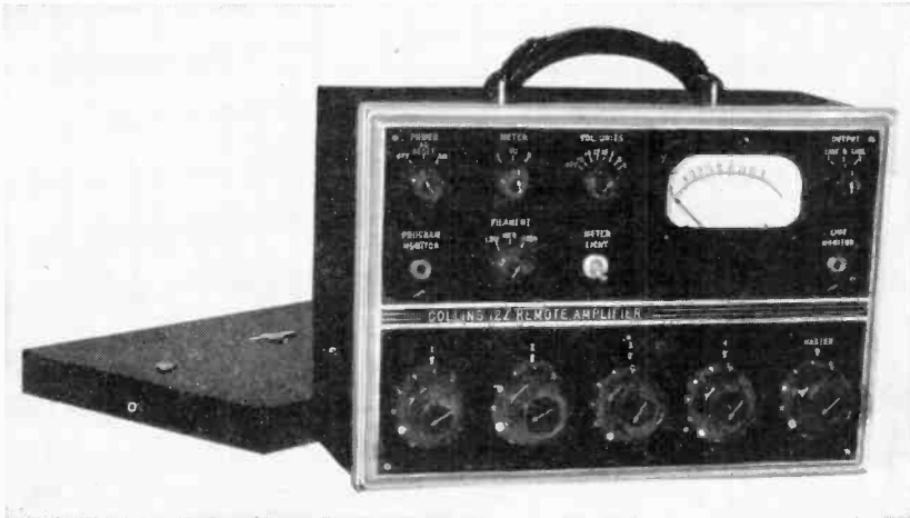
FIG. 31. A remote amplifier and microphone are used for man-on-the-street programs and for most remote pickups where there is not a permanent installation. (Collins Radio Company.)
