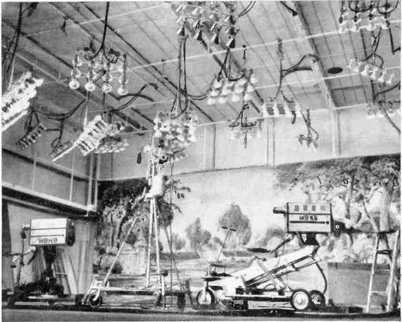
FIG. 23. Studio lighting systems, mechanically controlled, adapted to the most advanced lighting techniques for basic work, modeling, or back lighting, as well as specialized items of equipment needed in television operation, are shown in a typical studio layout. (R.C.A.)
