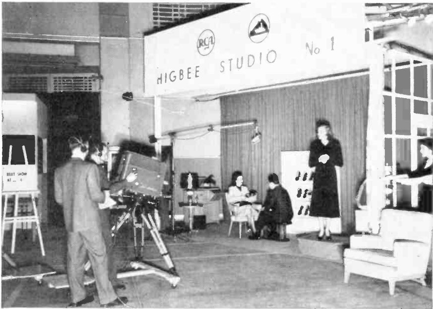
FIG. 24. Intra-store (closed-circuit) television. Dramatized commercial originating in the Higbee Company School Salon. The program was speeded considerably by having the camera switch from the salesman starting to fit the shoes on the model to the second girl at the right wearing the shoes being described. (R.C.A.)
