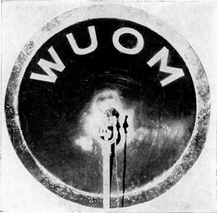
FIG. 13. Parabolic attachment.
