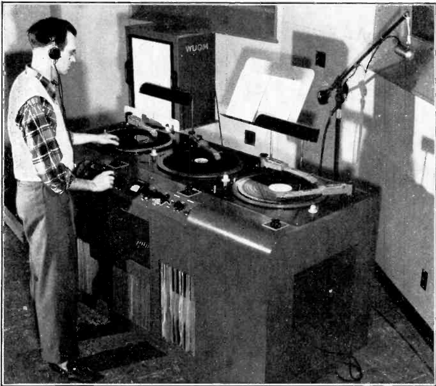
FIG. 42A. Sound table. Four pickup heads, three turntables, mixers, record racks in the front, speaker set into recess at end of sound table.
