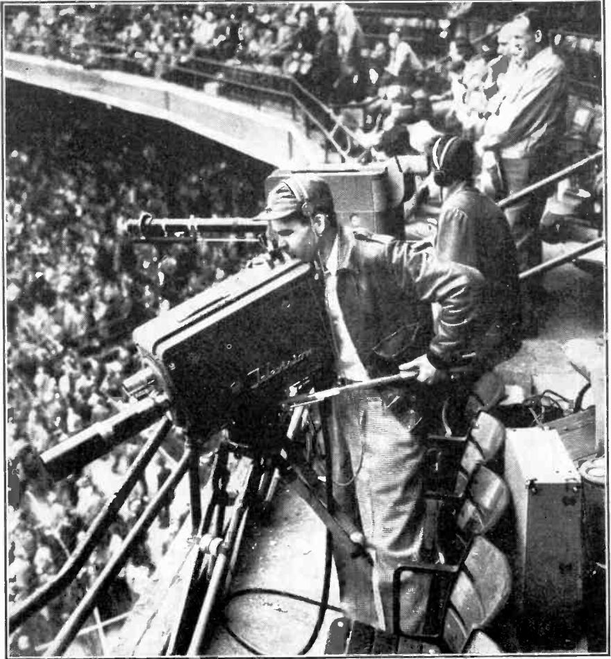
FIG. 29. Placement of cameras on second deck at Comiskey Park (Chicago) for WGN-TV telecasts of White Sox baseball games. Note use of external sight on foreground camera, and use of zoomar on the rear camera.
