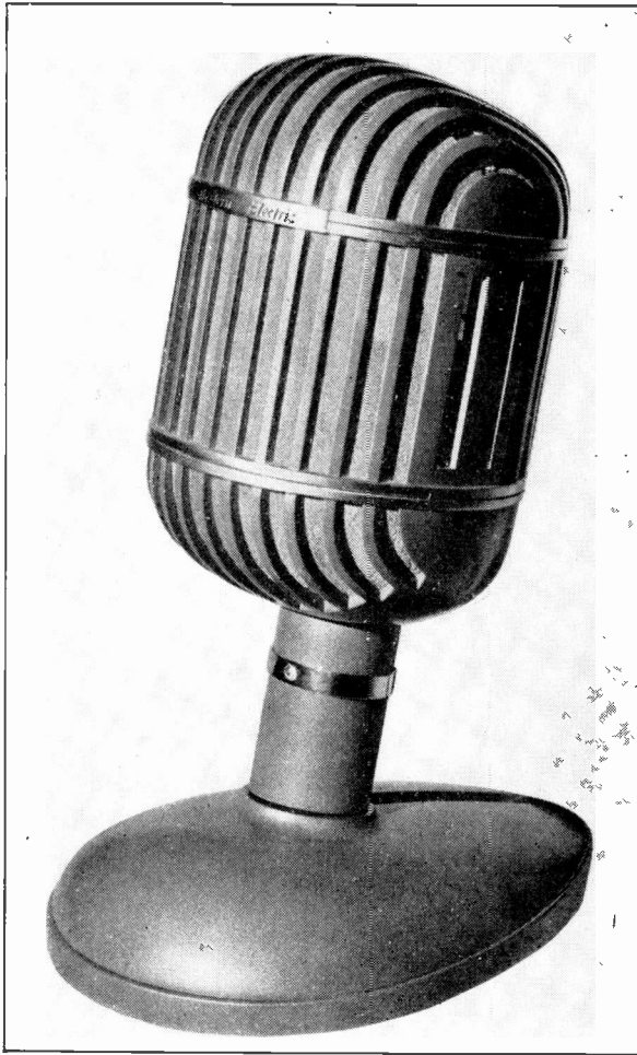
FIG. 6. The Multimike, a development of the cardioid microphone combining the features of the velocity and the dynamic microphones. ( Western Electric Company. )
