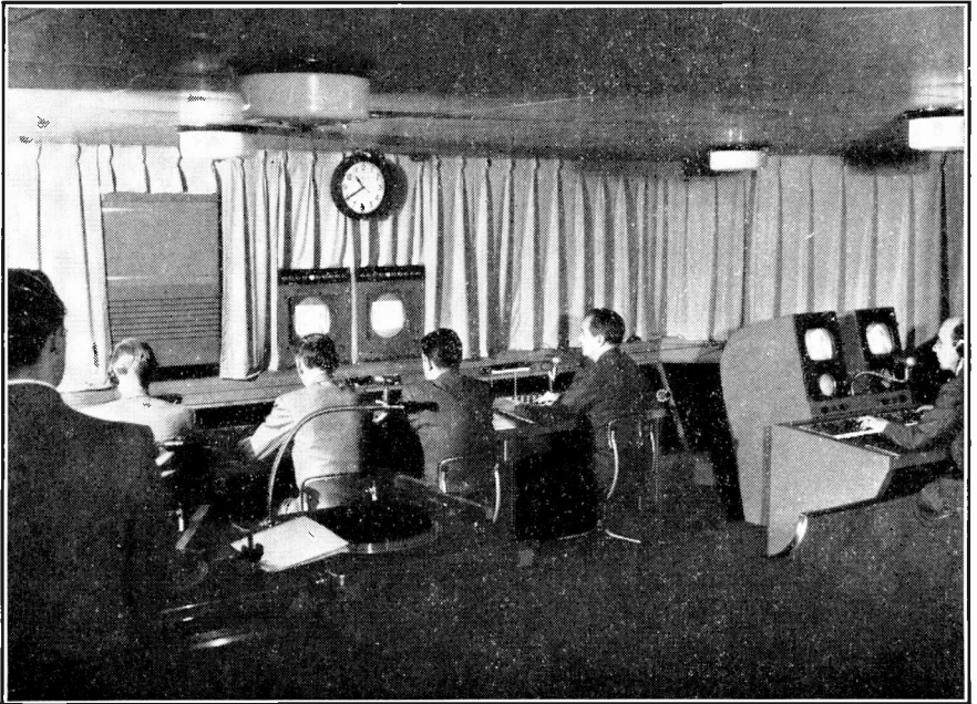
FIG. 81. Control room in studio 8-G, N.B.C., New York. Note that curtains cut off view into the studio.
