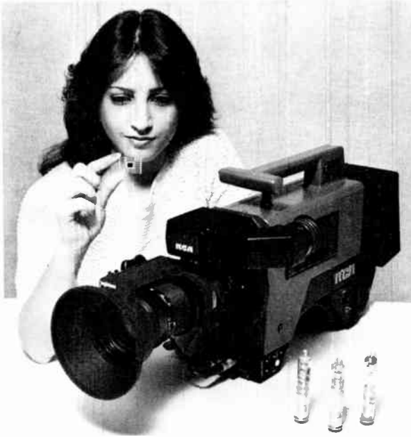
Figure 12.8 Tubeless electronic minicamera. An operator can hoist a self-contained minicamera to shoulder and take it places not easily accessible to larger studio cameras. This particular minicamera, RCA's CCD-1, made use of a technological revolution, the charge-coupled device (CCD). The small gadget being held above the camera is one of three CCD chips used instead of camera tubes in this RCA camera. (Photograph courtesy of RCA Corp. Used by permission of General Electric Co.)
