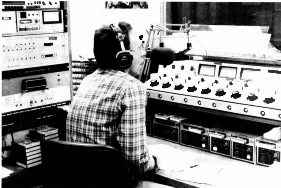
Figure 6.1 Radio combo operation. In front of the operator is the audio console. Meters at the top of the console indicate relative loudness of the audio signal. The microphone, over the console, is on an adjustable boom. Note the stack of audiocassette cartridges (lower left) and the line of cartridge playback units (below the console); this station "carts" (transfers to audiocassette cartridges) all records, and the operator plays the cartridges instead of records over the air.
