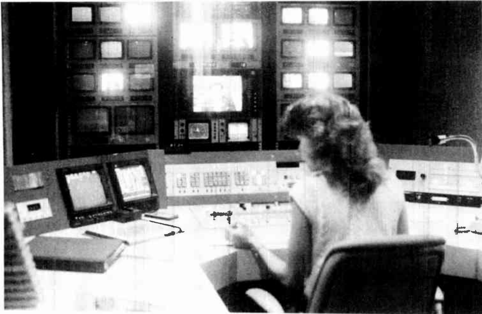
Figure 6.13 Duty director. At Orlando's Channel 2, the duty director's station is a centrally located, glass-enclosed booth. A computer feeds an electronic version of the program log to a video monitor (lower left). The switching equipment (lower center, in front of the duty director) handles video and audio simultaneously, so one person operates both. In the background—actually on the other side of the booth's glass wall—video monitors show the various program sources available.
