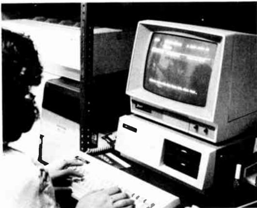
Figure 5.11 Computerized station traffic system. An operator enters program and commercial information into the computer. The computer, in turn, generates the station's daily program log (being typed on the printer in the background).
