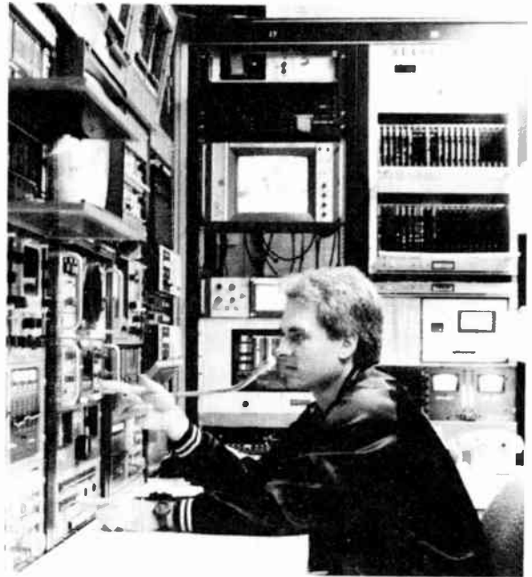
Figure 19.4 Television station master control. Central processing and switching point for Orlando's channel 2.
