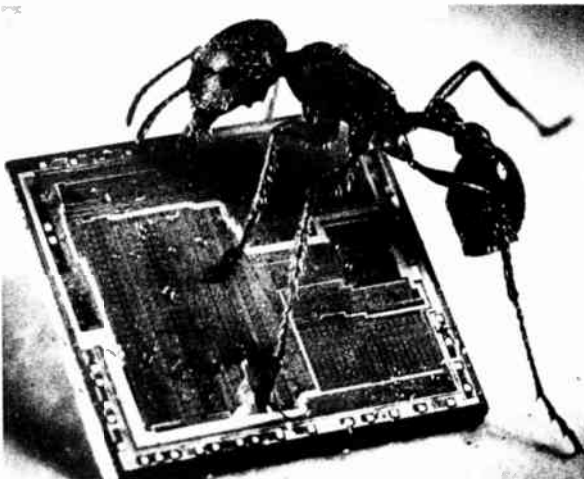
Figure 5.1 Evolution of solid-state electronics. Computer chip from the late 1980s. This tiny device contains the equivalent of thousands of transistors and their associated circuits. (Source: AP/Wide World.)
