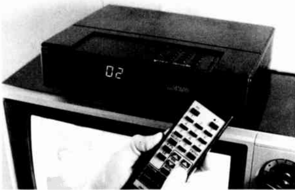
Figure 12.24 Cable adapter box. The subscriber end of the Jerrald IMPULSE 7000 system by General Instrument consists of this sophisticated, feature-packed addressable converter. The subscriber may operate the converter using either the control buttons on top of the box or the remote control. Among the many features of the IMPULSE 7000: channel selection; volume control; mute button; favorite-channel programming; last-channel recall; parental-control channel lock-out; time-controlled programming (for unattended VCR recording); response capability for video opinion polling; and both planned and impulse pay-per-view event buying. (Converter courtesy of Cox Cable-University City.)
