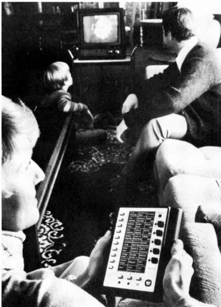
Figure 5.4 Interactive television: The late Qube. A Qube subscriber used a home terminal connected to the television receiver to participate in interactive programming. (Photograph courtesy of Warner Communications, Inc. Used by permission.)
