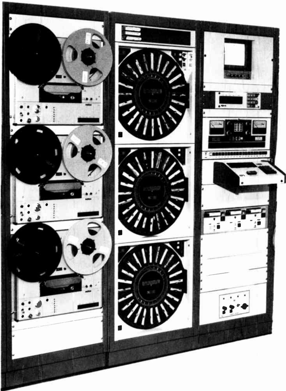
Figure 11.10 Radio automation. An automation unit combines computer and mechanical technologies. Radio automation entails setting up a machine to carry out standard technical procedures and to play back recorded programming elements in such way as to simulate the "live" production process. On this unit, the control panel for the programmer is the device that juts out about midway down the right rack. The three large wheels in the middle rack hold tape cartridges of commercials and will select, load, and play back the proper cartridge as programmed. (Photograph courtesy of Sonc-Mag Corporation.)
