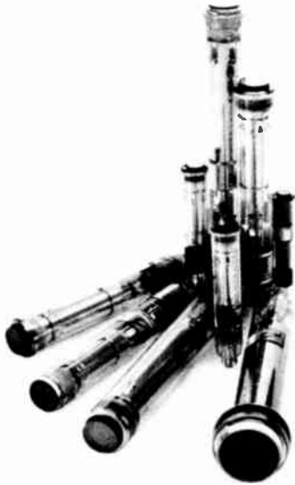
Figure 12.2 Plumbicon camera tubes. They come in various sizes and styles for various cameras and applications. (Photograph courtesy of Amperex Electronic Company. Used by permission. Plumbicon is a registered trademark of Philips.)
