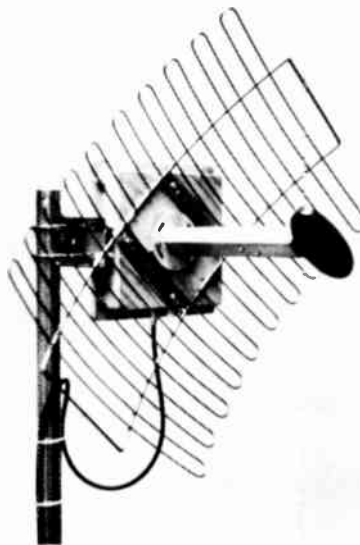
Figure 5.5 MDS/ITFS receiving antenna. This antenna features low wind resistance and is partially parabolic in shape. The square box behind it is the down-converter; it converts the signal from microwaves to frequencies that can be utilized by the television receiver. From the down-converter, the signal goes to a controller box that sits atop the receiver. The controller allows the consumer to select among broadcast and MDS/ITFS signals. (Photograph courtesy of Texscan Corporation. Used by permission.)
