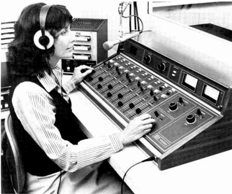
Figure 4-8 Control boards, also called "audio control consoles," have either slide bars called sliders or tuning knobs called pots to control the various functions. Audio control consoles can range anywhere from a few audio channels in smaller stations to large production studio models. (Broadcast Electronics, Inc., Quincy, ILL.)
