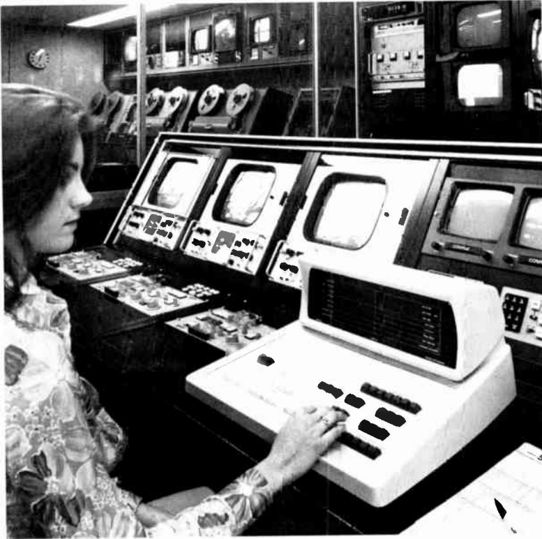
Figure 3-18 Computers interfaced with switching and editing equipment eliminate the burden of second guessing editing decisions. (Datatron, Inc.)
