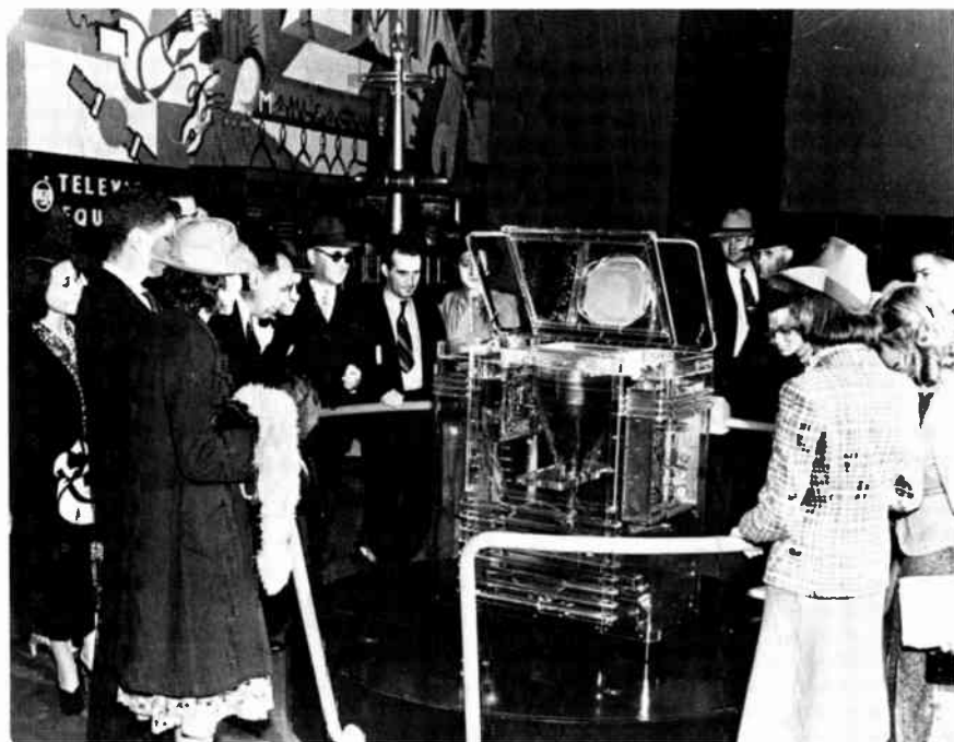
Figure 2-5 Television receiver in a glass case greeted visitors at the 1939 New York World's Fair. An 8" × 10" screen was reflected on a mirrored cabinet top. (RCA)
