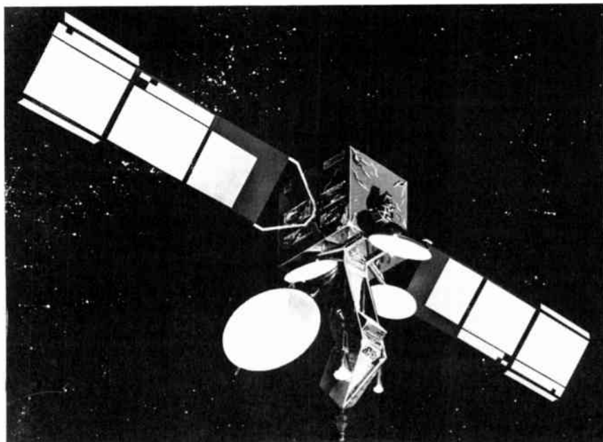
Figure 3-6 The INTELSAT V system is the most sophisticated satellite communication program yet developed. It is responsible for meeting the communication needs of much of the world during the early 1980s. (Aero Nutronic Ford)
