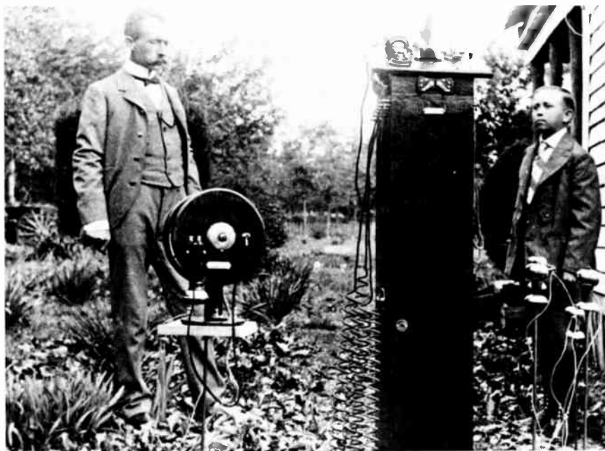
Figure 1-11 Even before Marconi's transatlantic wireless contact, an inventor named Nathan B. Stubblefield (left) transmitted voice by wireless over a short distance using a method of electrical interference known as induction. The method was unsatisfactory for long distance communication but Stubblefield has nevertheless been accorded a place among early broadcast pioneers. His son Bernard (right) became an employee of Westinghouse. (Murray, Kentucky Chamber of Commerce)
