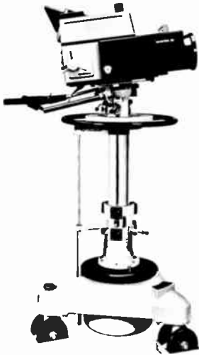
Figure 4-20 Larger camera pedestals still work on the theory of tripod support but are much larger, and primarily used for studio work. Many are pneumatically controlled and use compressed gas to raise and lower the camera into position. The steering ring permits the camera operator to both steer the camera and control the elevation. (W. Vinten, Limited)
