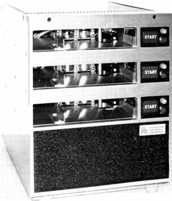
Figure 4-6 Cartridge tape machines permit production flexibility in many areas of station operations. Many stations find placing songs on cartridge tape can eliminate missed cues in live disc jockey applications. In the news studio, audio actualities (voices of news makers) are first placed on cartridge tapes and then integrated into the newscast. (International Tapetronics Corp.)
