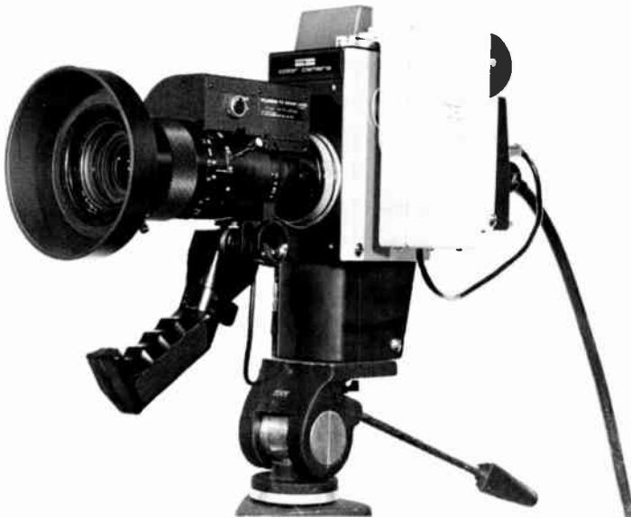
Figure 4-16 Changes in television design have made cameras more versatile. The camera seen here can be used either on a fixed pedestal or hand held for remote work. The eyepiece for the view-finder is located in the upper right. The handle, in the lower left, is used to steady the camera for hand-held applications. This particular unit is equipped with a zoom lens. (Hitachi)
