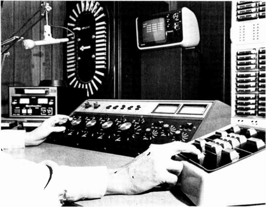
Figure 3-17 A computer-based system with a video screen (top center) shows the disc jockey the event on the air, the next event to go on the air, and the seventeen events that follow it. An "enter" line accepts the next event to be scheduled by the disc jockey and a clock automatically resets each time an event is started on the air. The key board in the lower right is used by the disc jockey to control the pre-recorded programming with the convenience of being able to retrieve, position, play, and return material automatically while retaining the spontaneity of a live operation. (Courtesy of IGM, Bellingham, Washington)
