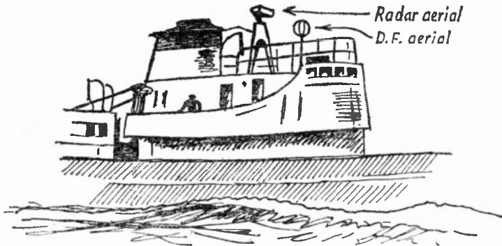
The bridge of the trawler shown on page 67. Radar and DF aeriaks help with the navigation of the ship
