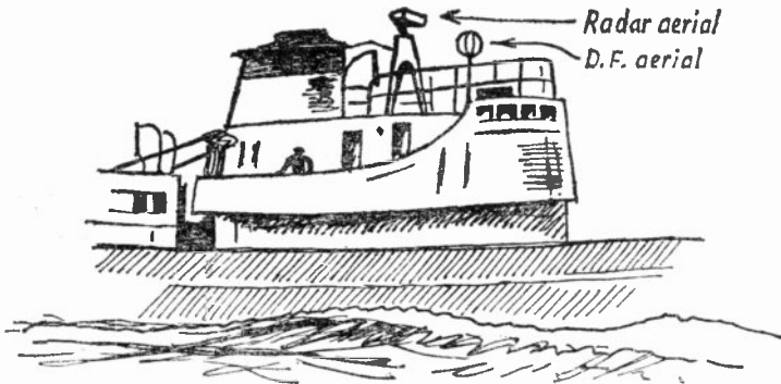
The bridge of the trawler shown on page 67. Radar and DF aeriels help with the navigation of the ship
